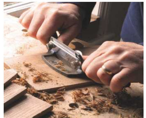
28 Removing saw marks in elm with a Stanley No.80 cabinet scraper
