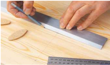
8 Mark biscuit positions on the side panels for top and bottom boards. Check that both left and right are matching
