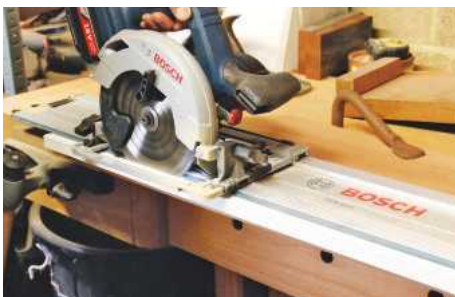
I found that cutting melamine-coated boards was quick and easy...
