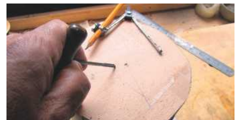
10 There are clever tools for finding a centre accurately, but drawing a couple of pairs of arcs from anywhere on the edge with an old school compass does the job just as well
