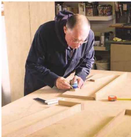
5 Marking out the rounded front edges using a suitable tin as a template
