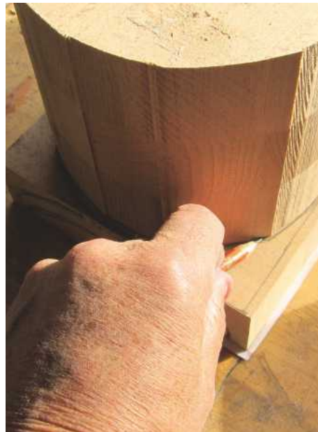
8 The trimmed bowl became a template for the lid. The idea was to make bowl and lid into a single flowing barrel shape, before separating them to work on the insides
