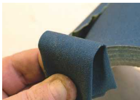
2 ... can be creased and folded without delaminating
