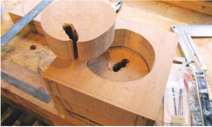
5 The base of the hole in the top layer served as a template for the top of the next layer, which again was cut out at a slight angle to match the planned shape of the outside
