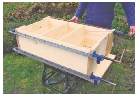
15 With substantial pads for the cramps, glue the side panels in place and remove excess glue while wet
