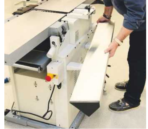
A couple of brackets keep the fence stowed safely on board
