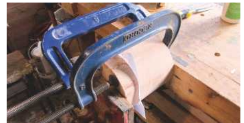
9 Since it was important that the glue-joints shouldn't fail on the lathe, I used maximum clamping pressure, both in gluing up the bowl and in attaching the lid over a paper gasket
