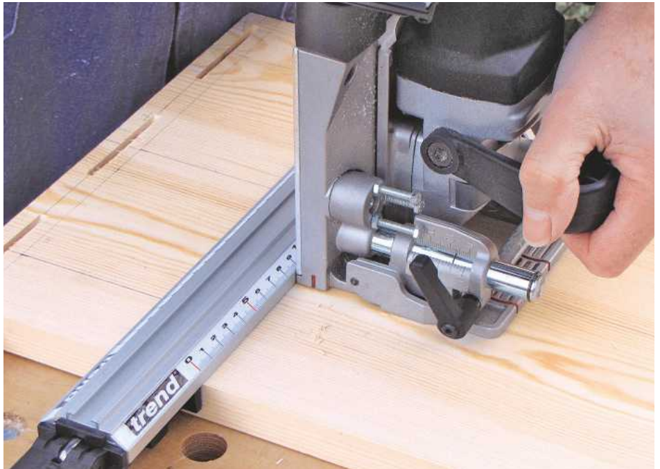
9 Using a Clamp System or batten as a guide across the boards, cut the slots with a biscuit joiner
