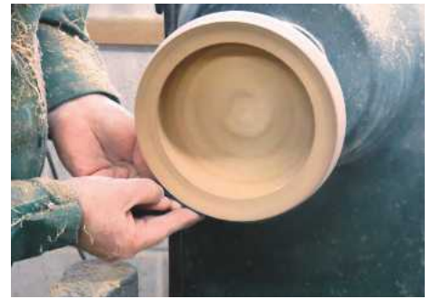
6 Sand in the bottom quarter – between 6 o'clock and 9 o'clock
