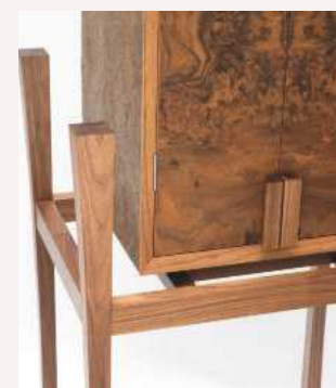
The walnut legs curve inwards on two of the faces, lightening the appearance of the whole base of the cabinet
