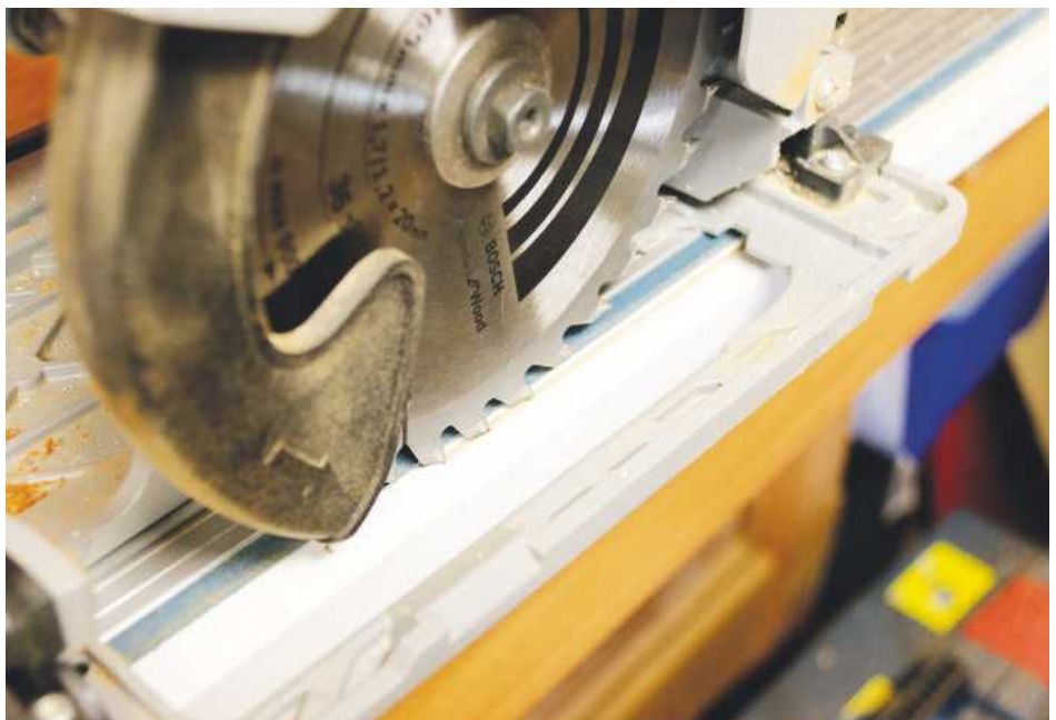
... although I found that making a shallow scoring cut first eliminates the problem
