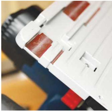
Alongside the Bosch narrow slot, the wider slot is Festool rail compatible
