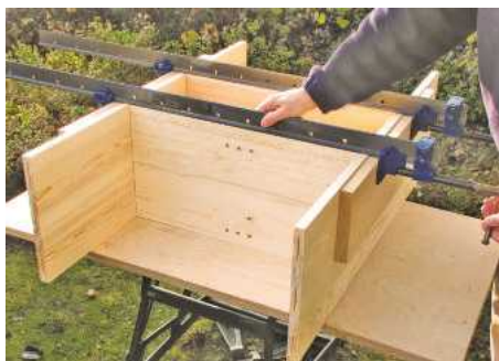
14 Glue the two vertical dividers to the top and bottom panels first. Check for square when cramping
