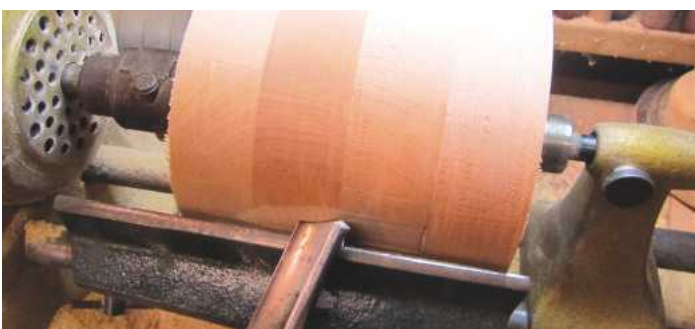
11 A heavy spindle roughing gouge makes short work of turning the assembled lid and bowl to a reasonably clean cylinder, ready for a parting tool to cut a spigot on each end
