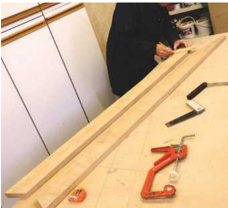
10 Using a scrap piece of side stuff, the trench widths are marked out
