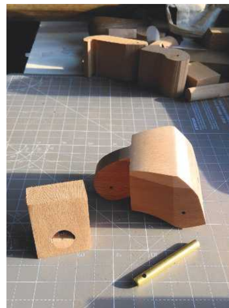
2 Head blank and body. The head has been drilled and plugged with half a dowel, the body cleaned up and drilled with 3mm holes for the connecting pins
