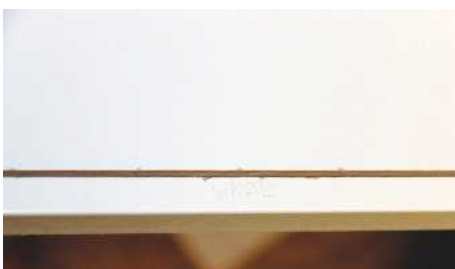
... but the resulting cut showed some chipping on the cut edge...
