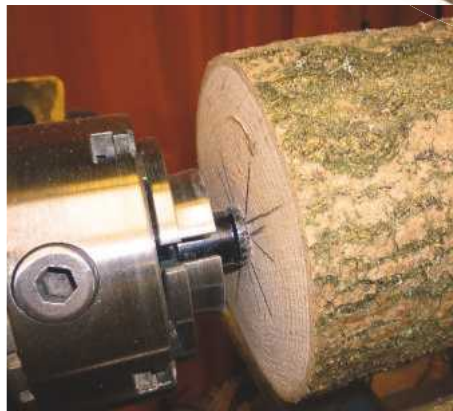
3 I use Steb centre drives to hold the material between centres, but a two- or four-prong drive will work equally well. A tailstock revolving drive can be Steb, ring or cone centre
