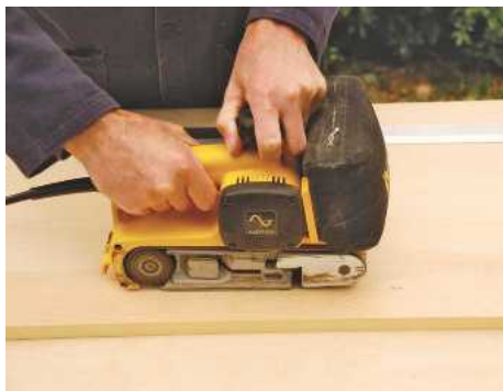
2 Clean up joints with a belt sander once the glue has dried. Use a bench plane for truing the surface
