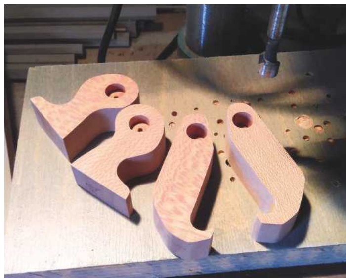
4 The arms and legs have a 15mm recess drilled part-way to house the star-lock washers
