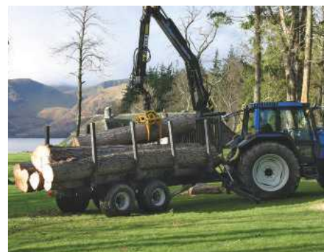
This tractor with Botex forestry trailer is capable of lifting 2.5 tons
