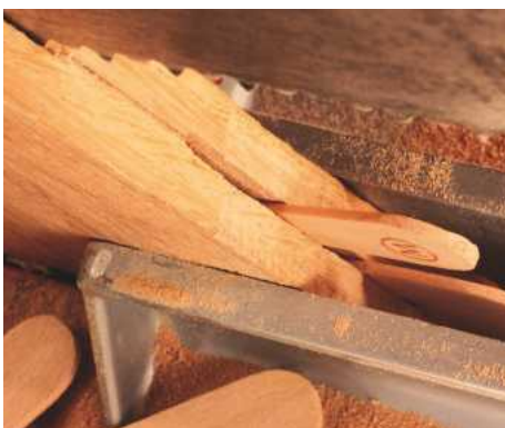
26 A lolly stick keeps the lower kerf open in the vice
