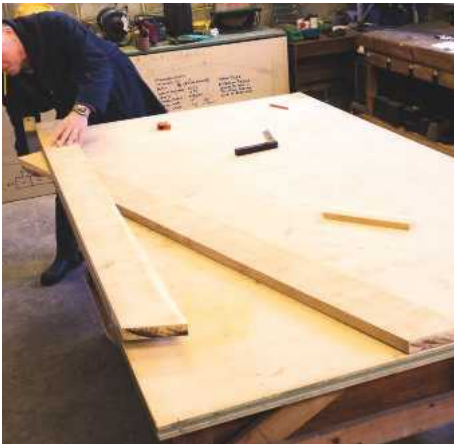
7 Working off the bench, using one leg as a straight edge, the back angles are marked
