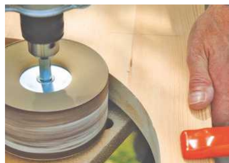
6 Cramp side panels together and clean up the curve with a sanding drum, mounted in a drill stand
