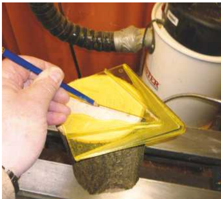
2 Use a centre finder with the 60° angle to locate the centre of branchwood, or go corner to corner if you're using square stock
