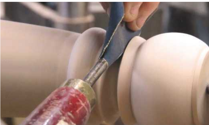
15 A dowel or shaft of a gouge can be used as an aid when sanding coves
