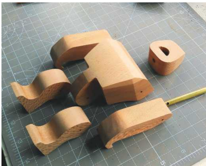
3 Ready for test assembly; note 6mm brass tube (drilled) to secure the head to the body
