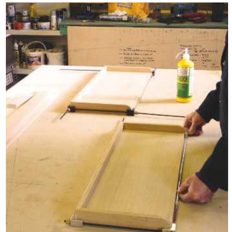
6 Two at a time, the three-sided, wrap around edging is glued on
