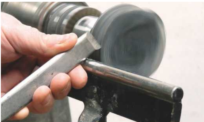
22 Slice off worn out hook-and-loop with a skew chisel
