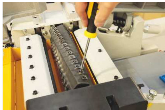
Cutters are self-setting and swapped with a Torx driver
