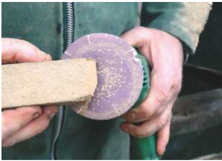
4 Use a rubber abrasive cleaning stick to clean your abrasive
