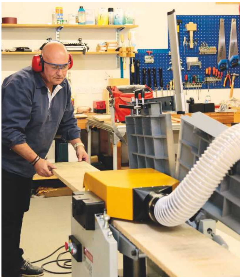
With the beds up there's excellent access to the thicknesser
