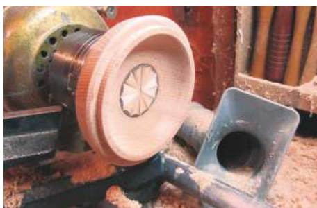
16 The veneer insert is less than a millimetre thick, so it's important to keep clear of it while working through the grits, until you get to the final stages of burnishing
