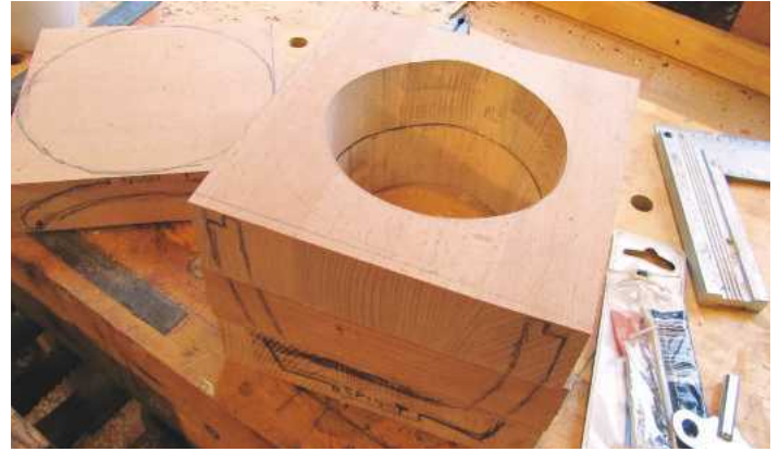
6 The bowl's three layers – two with cut-outs, the bottom layer left intact – lined up pretty well from the scrollsaw. The walls were left thick at this stage to ensure a strong glue-joint
