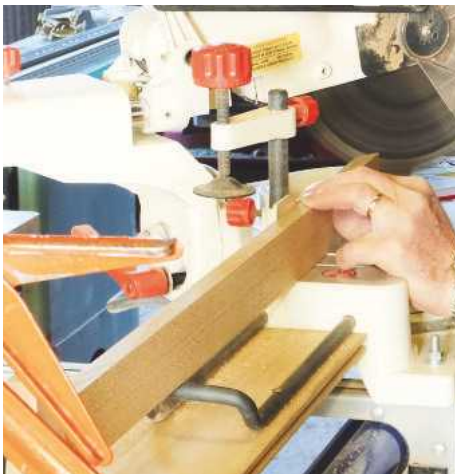
4 Cutting the mitre joints for the sides and back of the shelves
