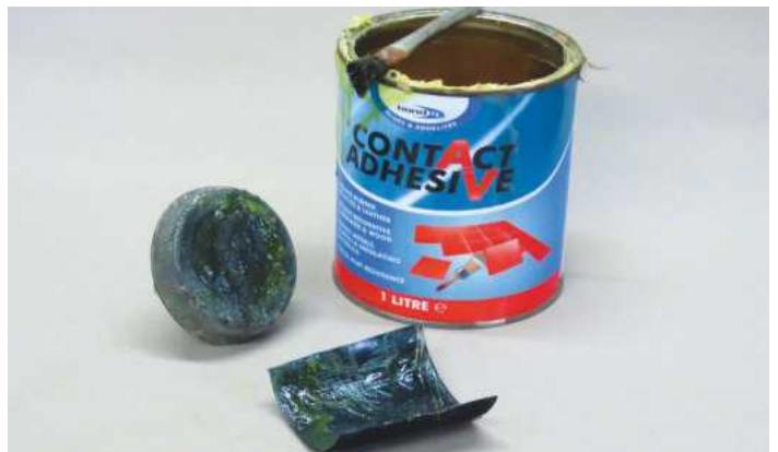
23 Contact adhesive offers better adhesion than the self-adhesive on the Velcro
