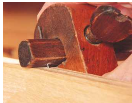
20 Marking the edge of an elm board for resawing
