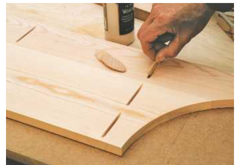
13 Cut slots in the ends of the top and bottom panels. Glue size 20 biscuits into the slots and you're then ready to assemble the cabinet
