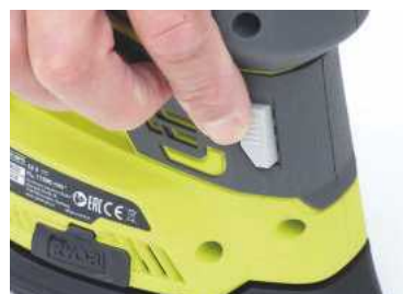
Power on/off is via the push-through button, reached from either side of the nose
