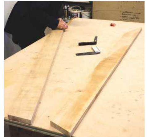
9 Marking the shelf positions onto each leg directly from the laying out drawing
