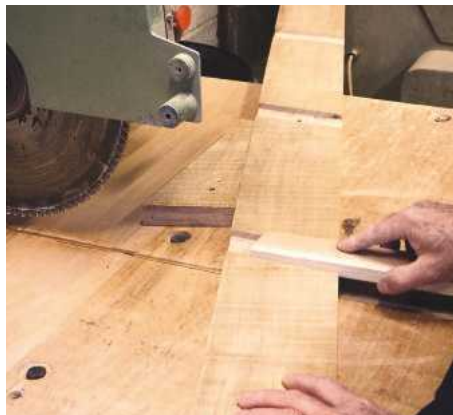
11 With care the trenches can be cut on a pull over cross-cut saw
