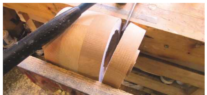
12 Once the cylinder had been curved at both ends into a continuous barrel shape, a couple of taps with a chisel split the paper gasket and released the lid
