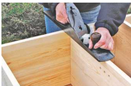
17 With a finely-set fore plane, true up the front and rear panel edges, checking them with a straightedge
