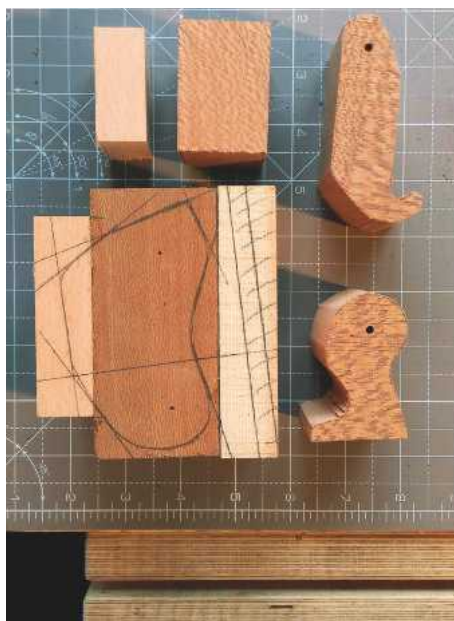
1 A sacrificial softwood block is glued to the back of the body; the offcut forms a supportive sled for further shaping. Note chest in beech and rough-cut arm and leg
