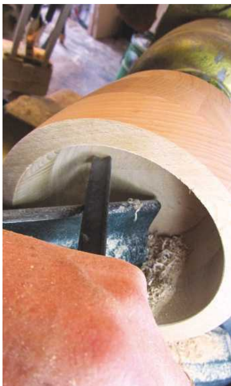
13 Fine cuts with a scraper gradually smoothed the sides and the joints between the pieces. Pull cuts from the centre with a bowl gouge gradually hollowed out the bottom
