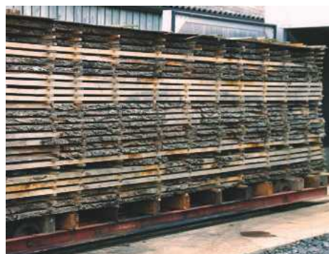
An oak stack being loaded into the heat vent kiln
