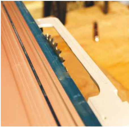
Viewed from beneath you can see the blade snug to the rubber strip
