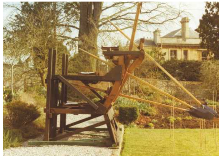
A mock-up section was built to test the proposed arrangement of the oarsmen system as suggested by Sinclair Morrison. Following the testing, an important improvement was made to the position of the thranite rowers
