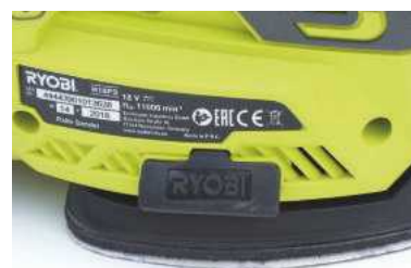
A rubber flap at the lower edge of the tool is flipped open...
