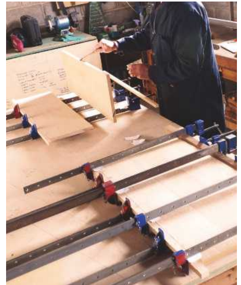
3 One of the first jobs is to get the solid edging glued onto the oak-faced MDF
