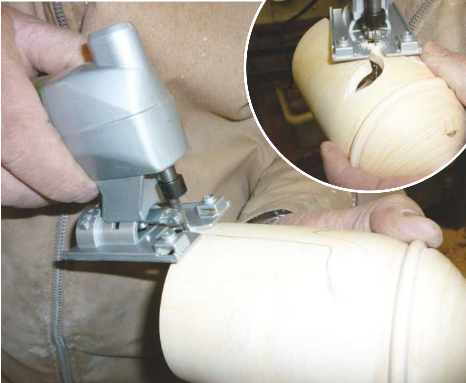
13 I use a small Proxxon jigsaw to cut out the eyes, taking great care to hold the piece securely and always keeping the cutting edge away from the fingers
