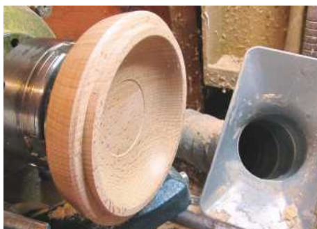
14 A shallow flat-bottomed recess made space for a decorative veneer – the only part that cost any money. A chamfer round the outside edge made it easier to grasp the lid
