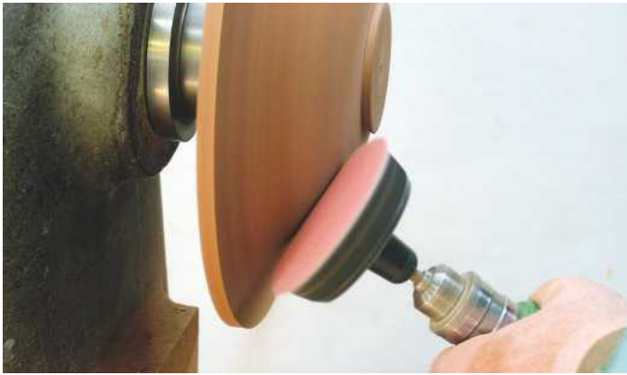
17 Use just the edge of the disc when power sanding...
