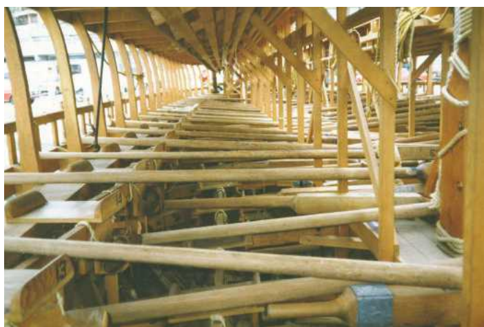
Detail of the trireme outriggers used by the top level rowers
