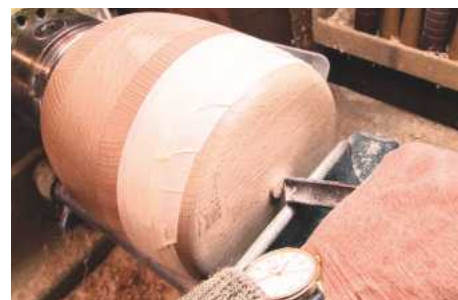
17 The bowl was held safely between centres while most of the spigot was turned away. For the final part, I added insurance in the form of several layers of masking tape
