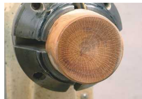
3 Overzealous sanding can result in heat checks
