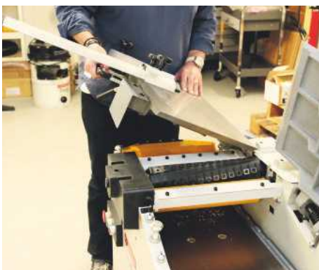
Both beds lift away on spring-assisted hinges
