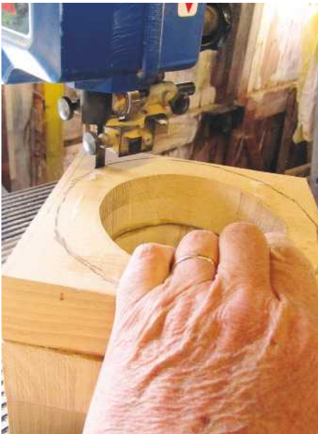
7 Once the glue had dried, the three layers were trimmed roughly to shape on the bandsaw. The outside was left vertical so that, once turned, the walls would thicken towards the base
