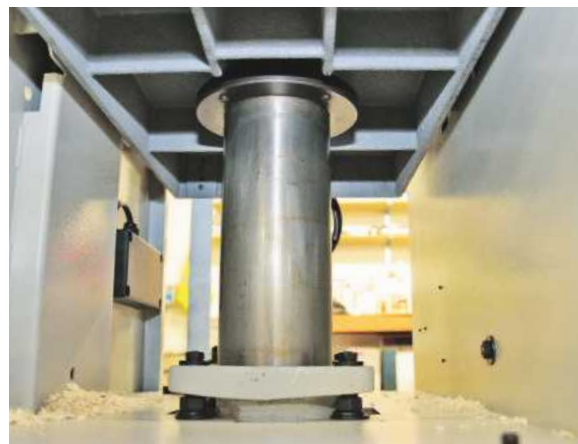
A substantial central ram controls the rise and fall of the table
