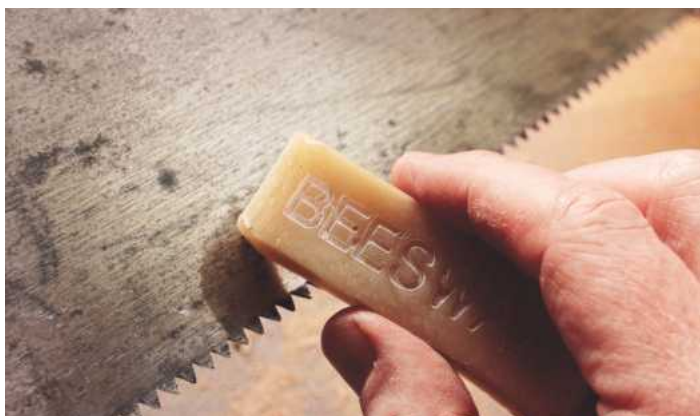
21 Applying beeswax to the saw blade to reduce friction
