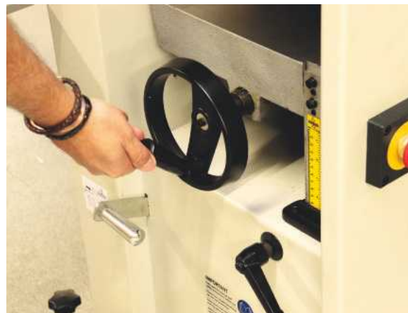
There's a fold-in handle on the thicknesser to stop it from getting hit
