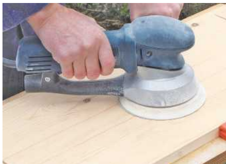
12 Sanding inside surfaces before assembly makes final cabinet cleaning-up easier. Use 120 grit abrasive
