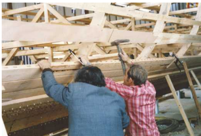
The hull was made secure with tenons between each plank
