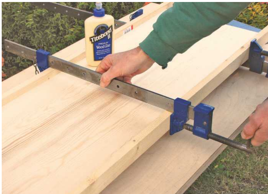
1 To get sufficient width, glue boards together with PVA adhesive. Sash cramps above and below keep them flat
