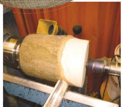
4 Using a spindle roughing gouge, turn the blank into a cylinder measuring 100mm diameter
