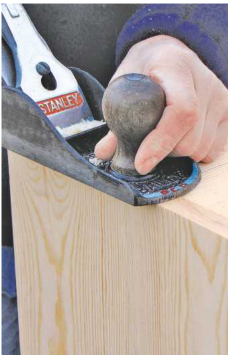
16 Once the glue has dried, trim the side panels flush with the top. Plane from both ends towards the centre
