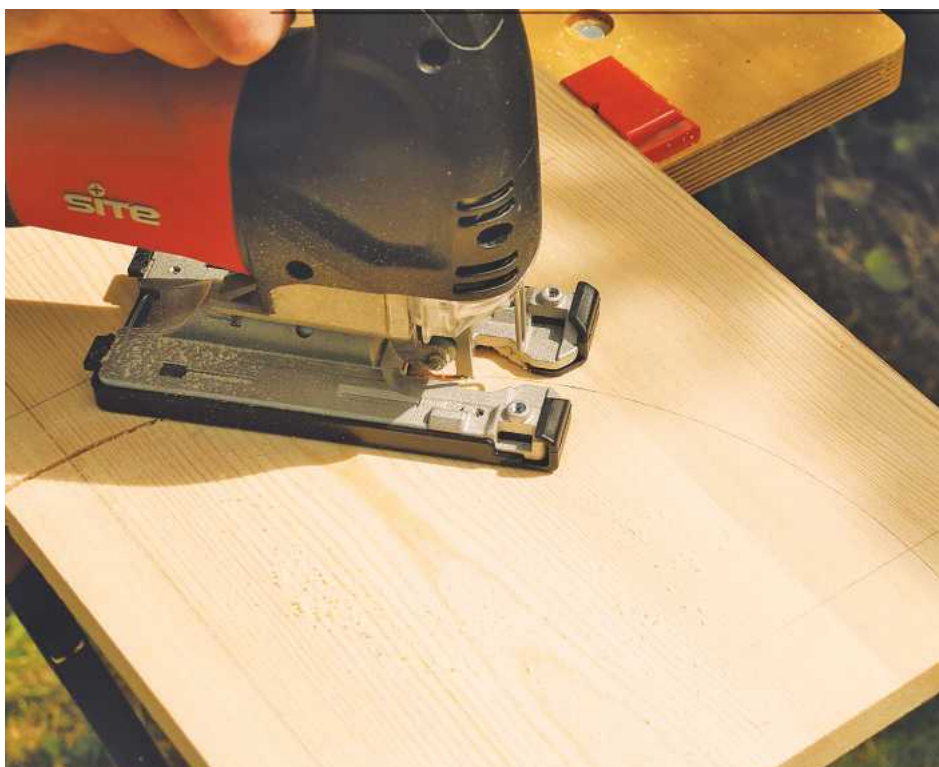
5 Cut out the template with a craft knife and transfer to the timber. Use a jigsaw on the lower curve
