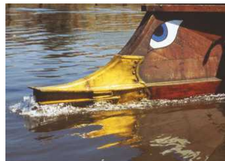
The fearsome ram cuts through the water during tests on the Thames
