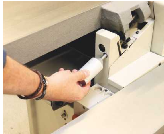
The surfacer depth of cut adjuster is located at the back
