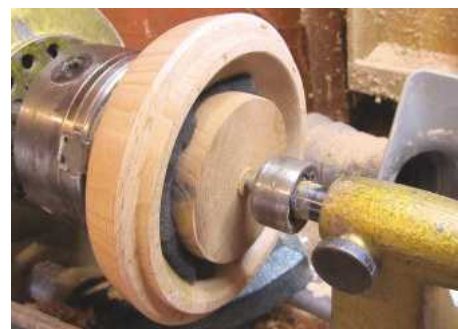
15 A tiny smear of glue in the recess (not on the veneer) is enough to hold the insert. Too much and you risk staining. Clingfilm between veneer and clamp avoids the risk of sticking
