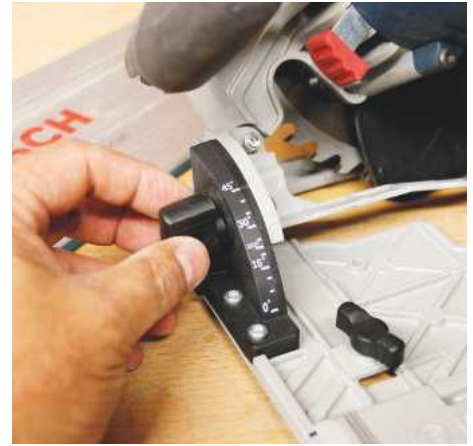
Angles are locked with front and back knobs to help keep things rigid
