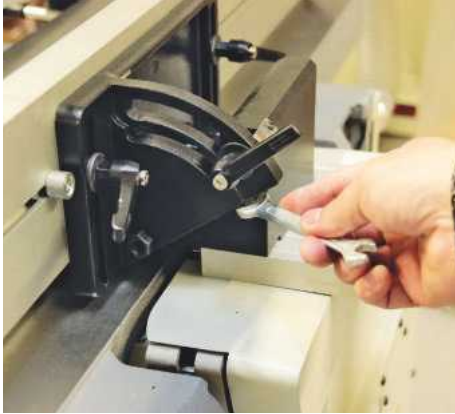
Adjustments can be made to the fence stops for 90 and 45° positions
