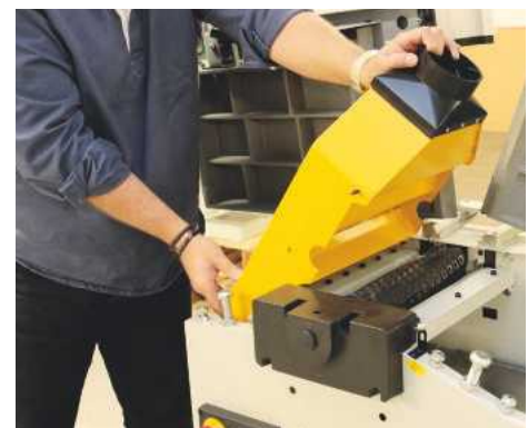
The built-in extractor hood hinges into place to cover the block
