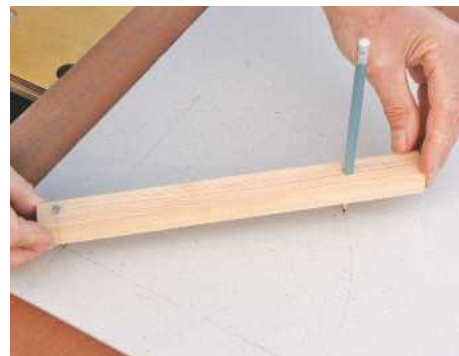
4 A card template is useful for the side panel profile. To draw a suitable radius, make a simple trammel
