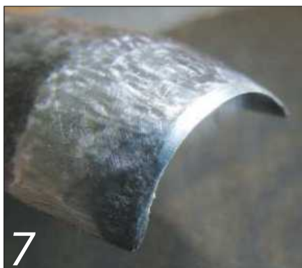
7 After honing a secondary bevel on a finer stone
