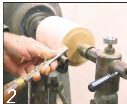
2 Square off one end and cut a chucking spigot
