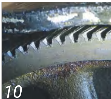
10 The skewed gear teeth mesh smoothly with the axle
