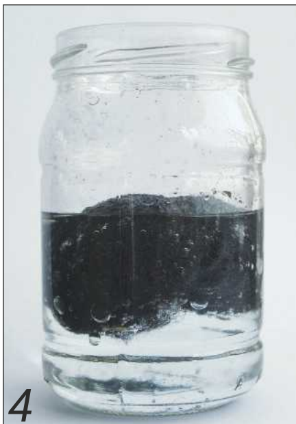
4 The bubbles make the iron float and show the reaction is taking place
