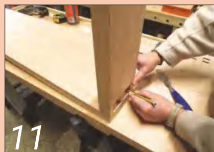
11 ... and using the pins as templates to mark out the tails
