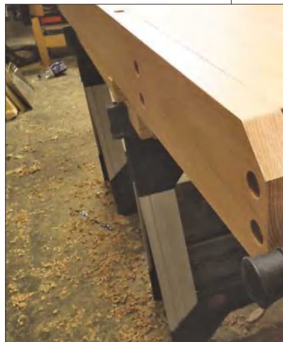
19 Using the well material as a gauge, the apron material was marked up
