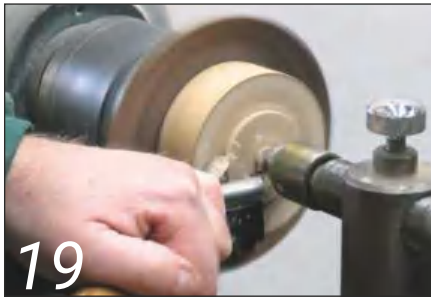
19 Reverse chuck the base onto a dolly to remove the chucking spigot
