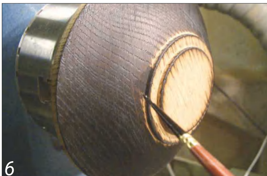
6 Touch in where necessary. Indian ink is good for this, applied with a small brush
