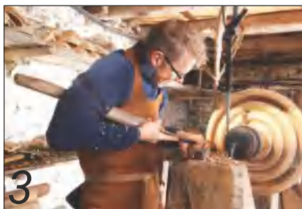
3 This technique of using the interior of a bowl to form further bowls saves so much on waste
