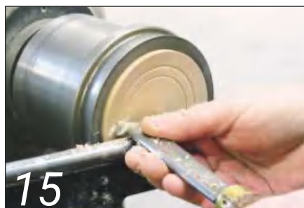
15 I cut a number of decorative beads on the top of the lid with a skew chisel
