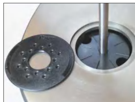
With the lower spindle washer fitted correctly, work can proceed
