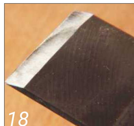
18 Hollow bevel developed on the grinding wheel
