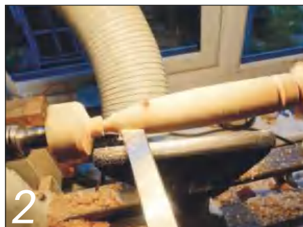
2 Turning the fuselage
