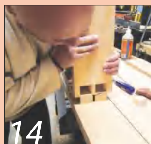
14 The joints are given a quick test fit but without driving fully home
