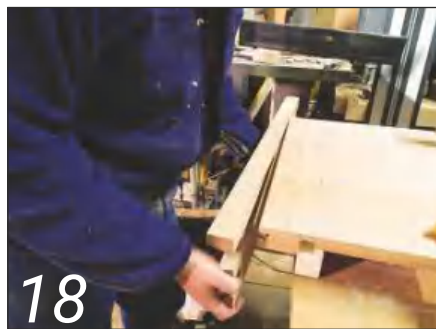
18 Make a test fit with the tongue in place to ensure that the joint will close
