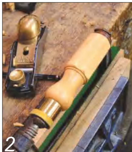
Great care had to be taken with planing up the facets so as not to tear up the grain
