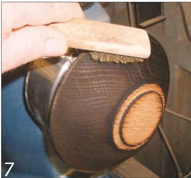
7 Wire-brushing removes loose charcoal and emphasises texture
