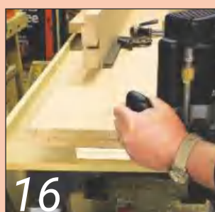
16 ... the end of the tops are grooved to take a ply tongue...
