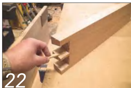
22 ... then the dovetails are glued up...
