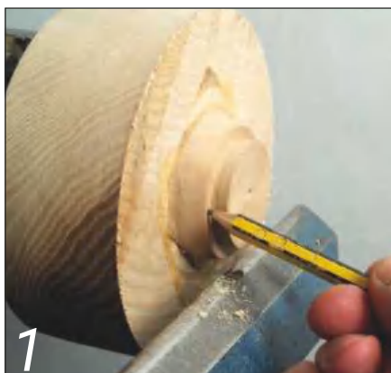
1 The face must be angled in the correct direction for the work to be properly supported
