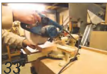
33 The jaw facing was shaped by first cutting the groove of the quirk...
