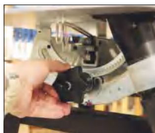
The rack and pinion alters the arm so that the table remains flat and level
