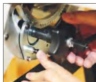
An indented rack and pinion trunnion sits below the table
