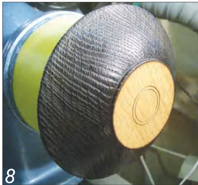
8 Very black and beautifully textured after sealing and polishing
