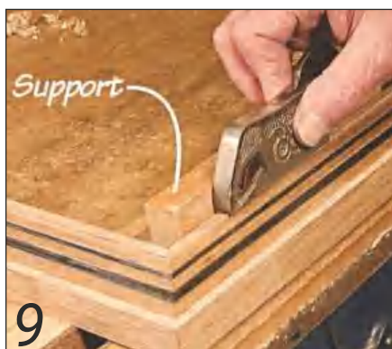
9 A bull-nose rebate plane comes in handy for a narrow surface
