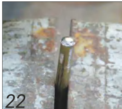
22 Flare over one end of the rod so that it cannot go through the 6mm hole
