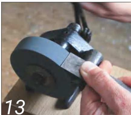
13 Finger positions while grinding
