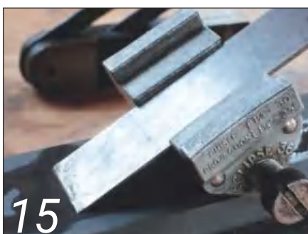
15 The 25mm chisel is mounted in the guide's lower position
