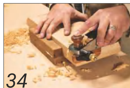
34 ... sawing away the bulk of the waste, and finishing the profile with a block plane
