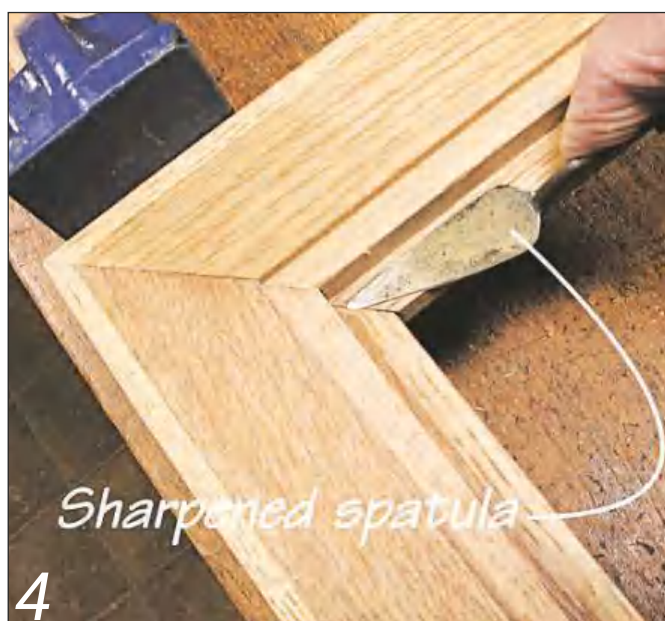
Improvising a tool for marking the difference in levels...
