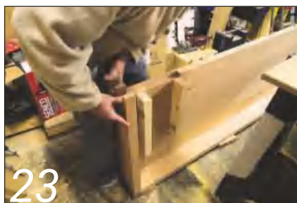
23 ... and with the front apron on the floor, the end aprons are set into place
