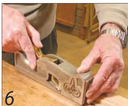
6 My shoulder plane corrects the router's less than perfect job
