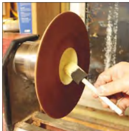
A pre-sealed piece allows the paints to build a solid colour easily
