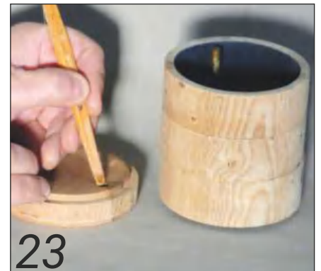
23 Reassemble the box and epoxy the rod into the hole in the lid
