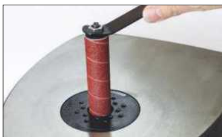
Tightening the spindle top nut to hold the drum and sleeve in place
