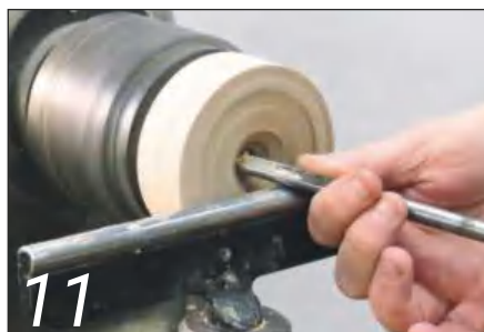
11 ... then make cuts from this hole towards the rim
