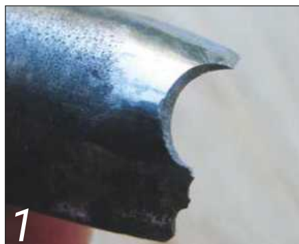
1 The damaged gouge before grinding
