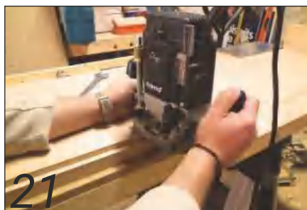
21 ... and on the underside a rebate was cut for the opposing edges of the tool well...
