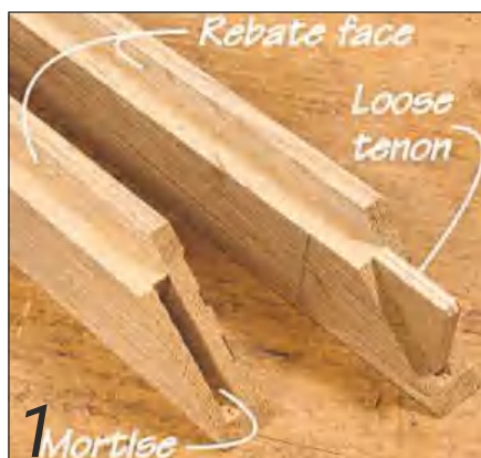
The machined mortises and loose tenons simplify a difficult joint
