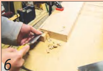
6 The joint is cut using a tenon saw and paring with a chisel
