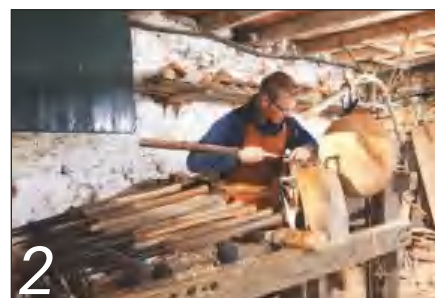
You can see just how large the bowl is here – from a 510mm 'mummy' bowl, Robin can get five bowls
