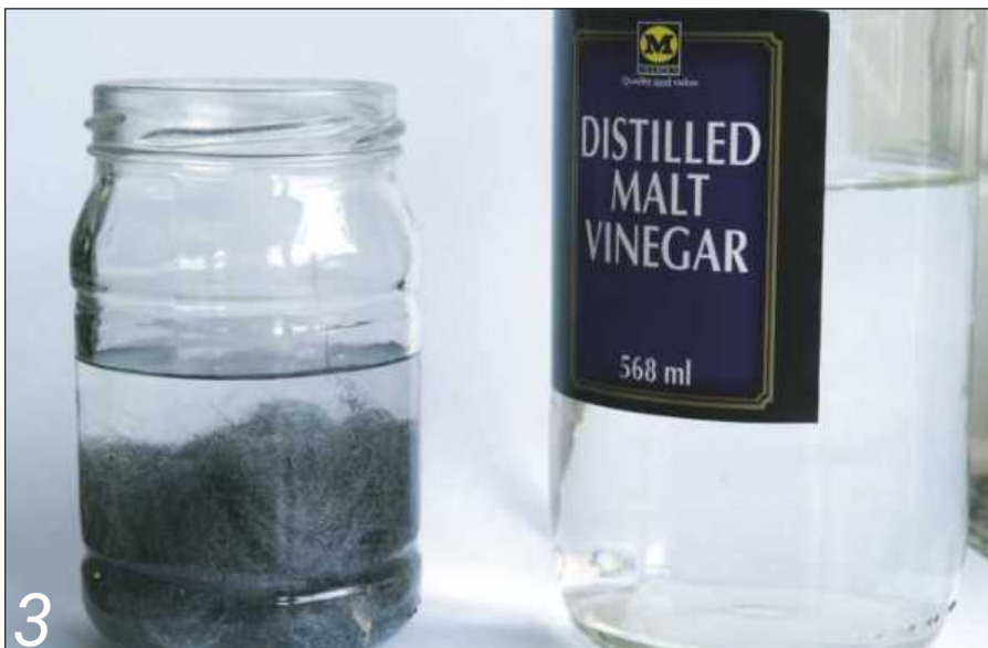
Steel wool and 'white' vinegar make an ebonising mixture that works better than you might expect from such a home brew. I can't see why regular malt vinegar wouldn't do just as well
