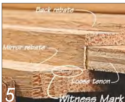
5 ... and making a mark to show how much has to be removed
