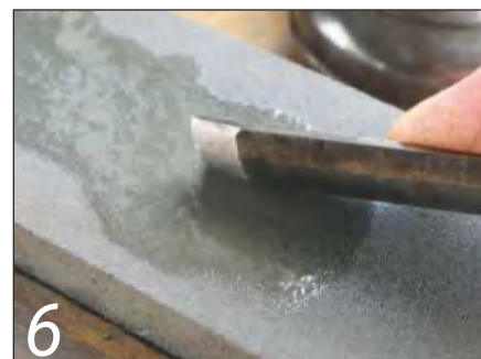
Smoothing the new bevel by working on an oil stone
