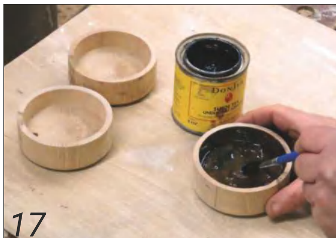
17 Paint on a generous amount of adhesive...
