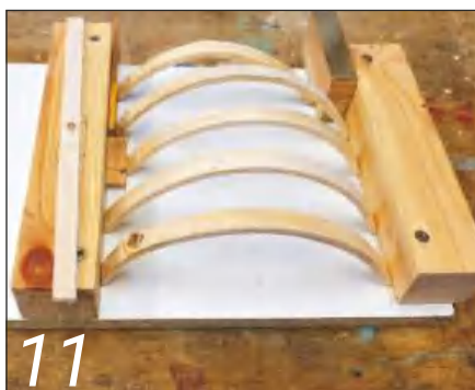
11 Rainbow rods are left in the jig overnight. They're not all the same length – note packing pieces to maintain the arc
