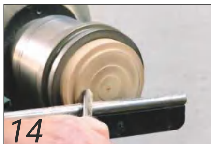
14 Mount the middle tier and face off the spigot, then reverse it and hollow as before
