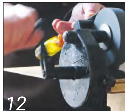
12 One hand for the chisel and one for turning while grinding a 25mm chisel
