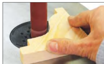
Successful shaping with the aid of a small drum...
