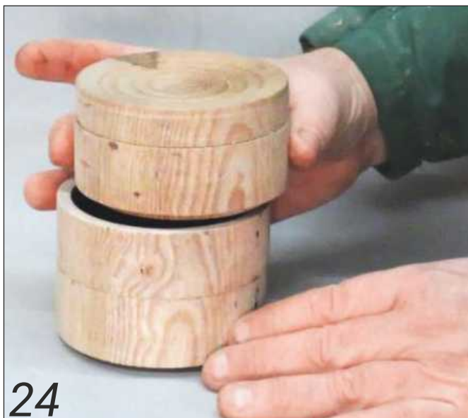
24 Check the rod moves in the stepped hole to allow each tier to open freely
