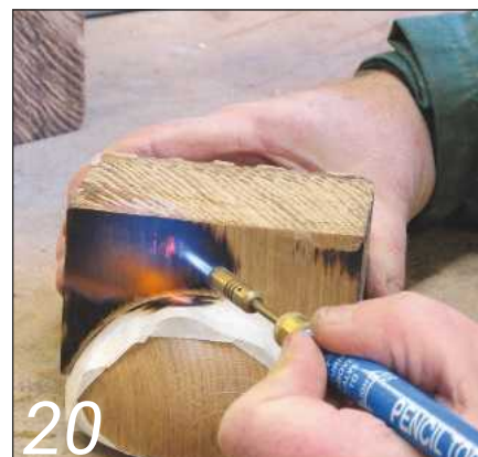
20 Scorch the areas that need texturing using a small gas torch...
