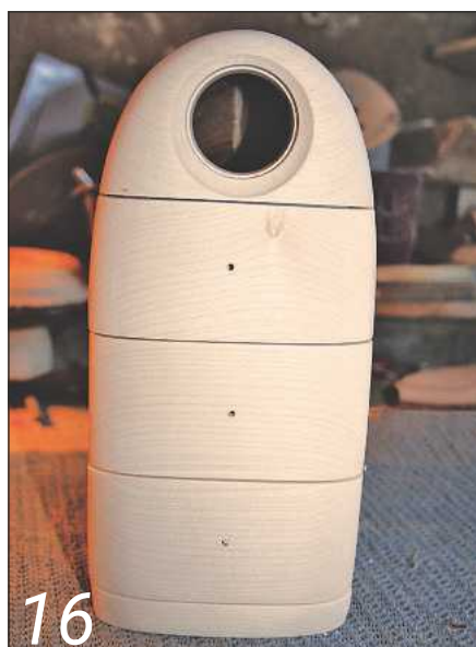
16 Glue the drawer fronts to their respective drawer boxes, and drill them ready for handles
