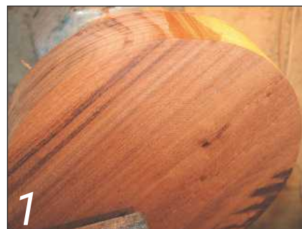
1 Mount the blank for the body and turn the face and edge to size
