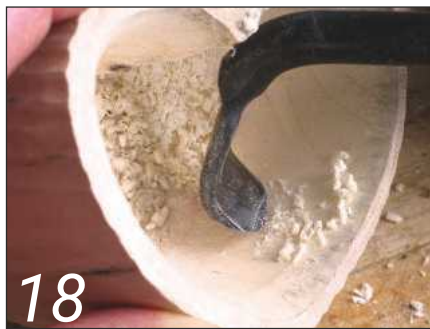
The curved scraper (ex-tyre lever) takes tiny shavings
