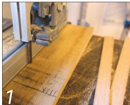
1 Cutting the strips – less waste is generated if you use a bandsaw
