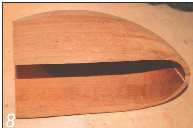
8 ... cut off the waste. For a cleaner finish, cut fractionally shy of the mark and then sand back afterwards
