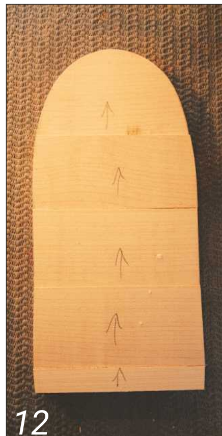
12 When choosing the timber for the drawer fronts, consider the balance of the grain and how it will fit within the shape of the unit
