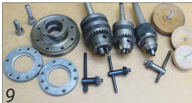
9 Many 'home-made' means of workholding can be devised, such as simple screw chucks
