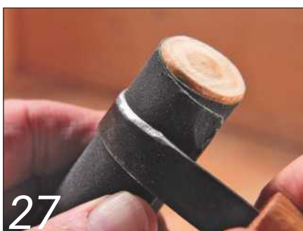
Removing burrs inside the curve
