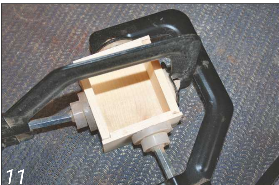
11 The drawer boxes are made up using lap joints
