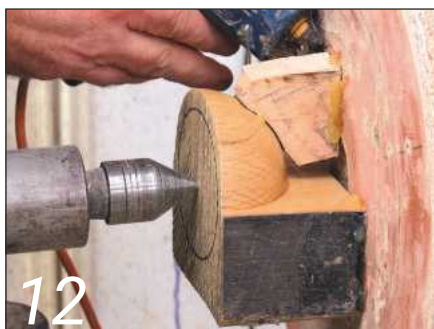
12 Glue in a supporting block under the bowl part
