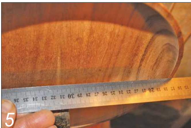
5 Check that the bowl's face is flat; accuracy is important here if you're to get a good joint later
