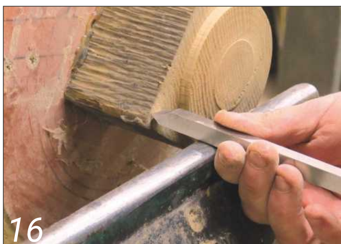
16 ... and a hardwood scraper to remove the waste wood to the left of this groove
