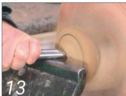
13 Flatten the top surface using a pull cut
