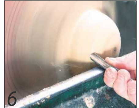
Change to a small spindle gouge to finalise the shape...
