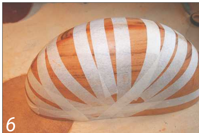
6 Masking tape makes a versatile cramping tool when gluing the halves of the bowl together
