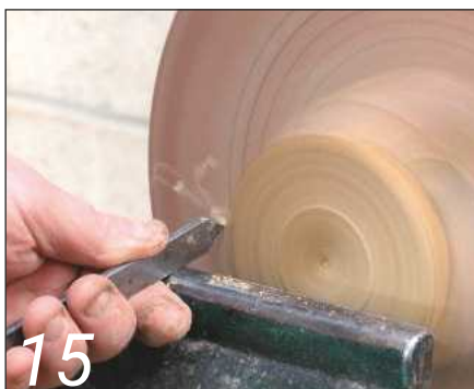
15 Use a parting tool to cut a groove on this mark...
