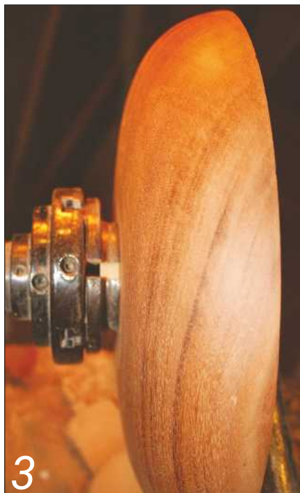
3 Remount the blank to turn the bowl's inside. Be sure it's running true to avoid an uneven wall
