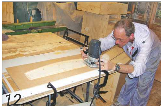
The drawer fronts were routed to create a false panel
