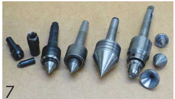
7 Tailstock centres. On the left is a 'dead' centre used with an auger for boring very deep holes. The one on the right has changeable tips for different purposes
