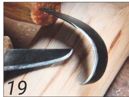
Short and hook knives made from old saw plate
