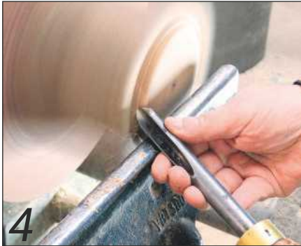
... using the bottom wing of the gouge
