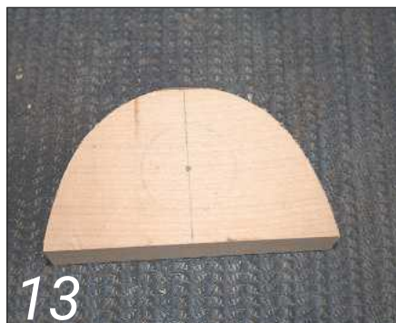
13 The position of the clock insert was marked to mount on the lathe, ready to turn
