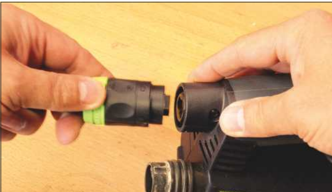
Festool's interchangeable power lead is fitted on this sander
