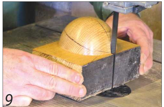
Use a bandsaw to cut the piece in half – centrelines drawn earlier will help
