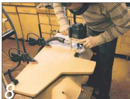
8 The sides were shaped using a bearing-guided cutter in a router
