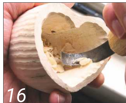
16 Working on the interior with a home-made hook knife
