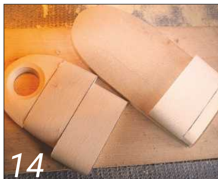
14 Shape the face timbers to match the template and round over the edges
