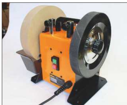
The leather stopping wheel to the fore; the support arm will fit in either orientation for maximum range
