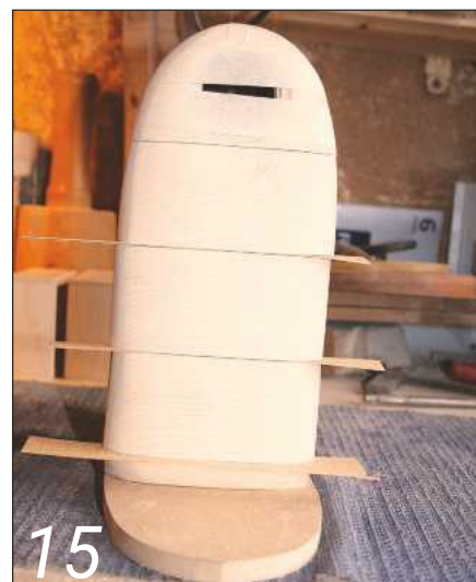
15 Glue the base section in place, and use a slip of veneer to space the drawer fronts evenly, as shown
