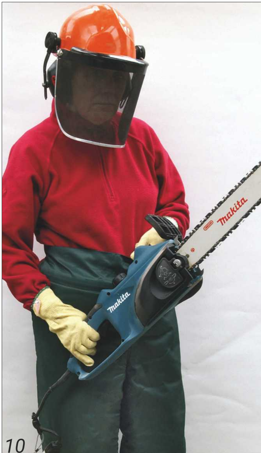
Chainsaw protective clothing: ear defenders, hard hat, steel mesh facemask, Kevlar gloves, padded trousers and steel toe cap boots. All slightly too big for my long-suffering model
