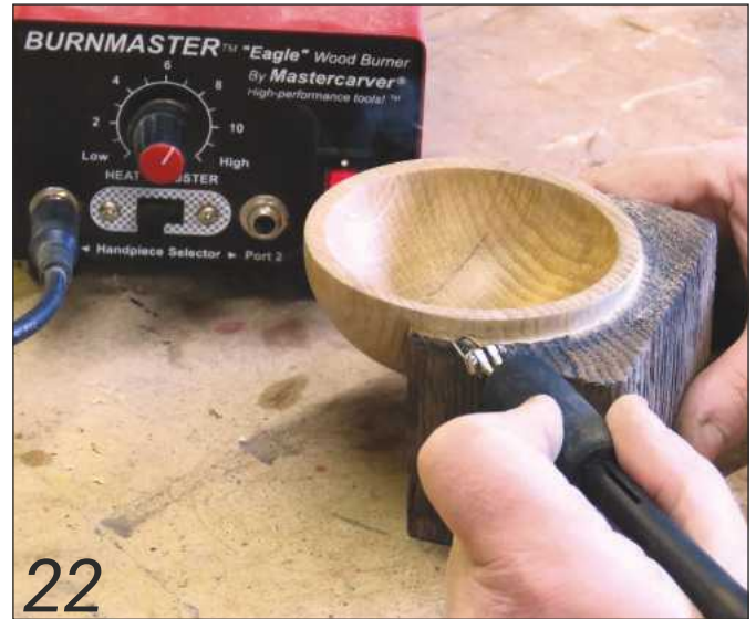
Further texturing can be done using a pyrography machine
