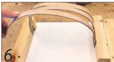
6 Into the cooling jig. Strips can now be handled without gloves
