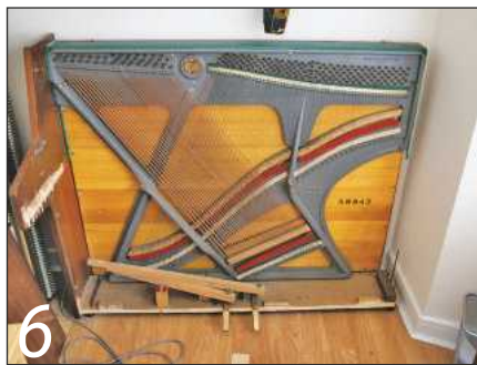
6 One side of the panel was removed and replaced before the other was tackled
