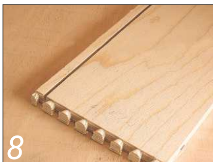
8 For the drawer boxes, dovetails were used to join the drawer sides to the fronts...
