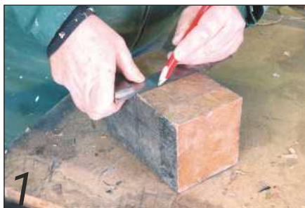
1 Mark a centreline around all four faces and the centre of one face
