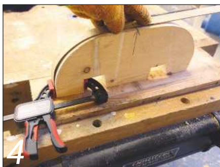
4 Clamping one end to the former jig
