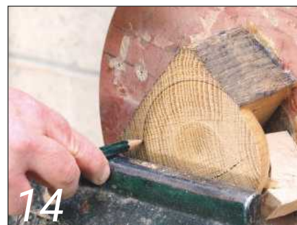
14 Mark the circumference of the outside of the bowl's rim
