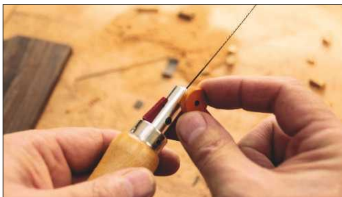
The blade is securely held in place with two anodised aluminium knurled knobs
