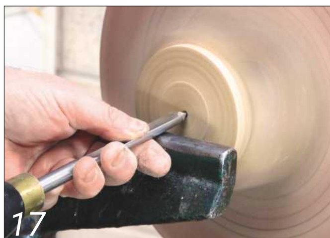
17 Drill a hole in the centre of the bowl with a spindle gouge...
