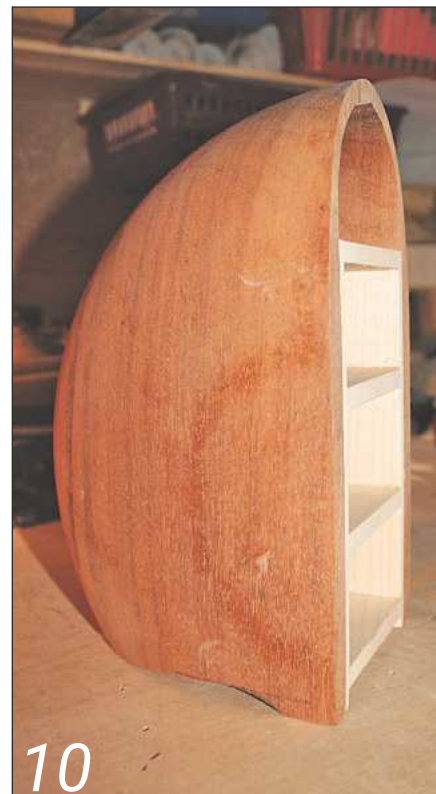
10 Check the drawer carcass fits neatly in the body before gluing it into place
