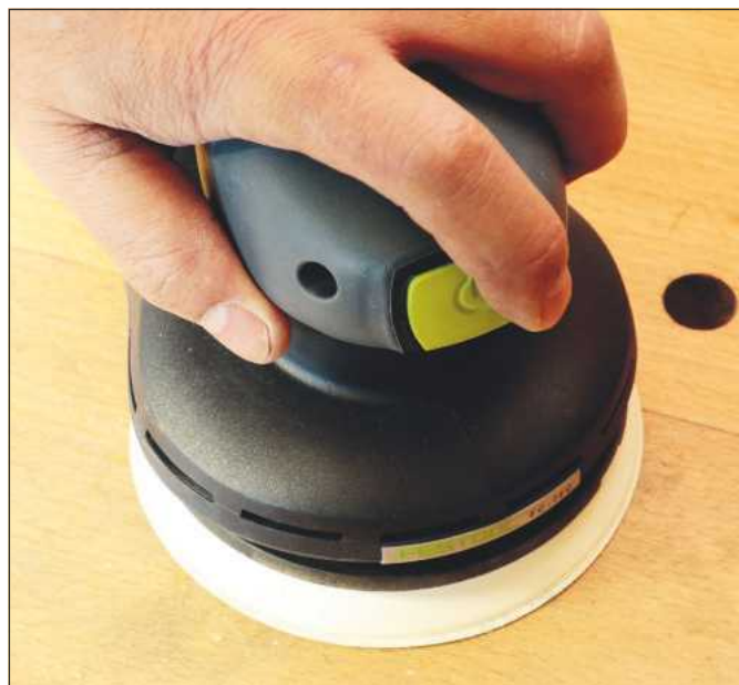
The power switch on the ETS EC 125/3 EQ toggles through the extractor detection as required
