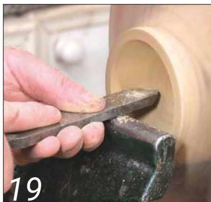
19 Make gentle cuts with a round-nosed scraper to clean up the end-grain
