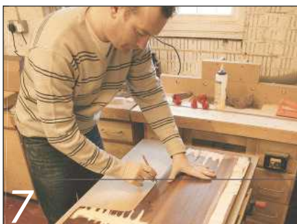
7 For the new sides, I laid the old ones onto the stock and drew around them
