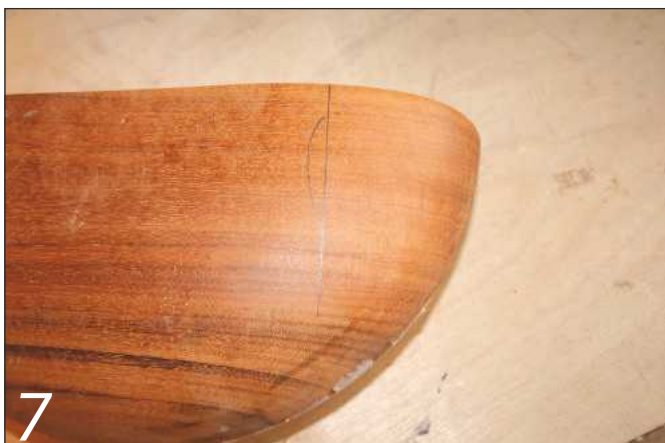
7 To form the flat base of the unit, measure from the centre of the blank and square across the face and down each side, then...
