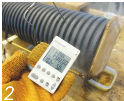
2 Probe and temperature gauge – not essential but nice to know it got to 100°C
