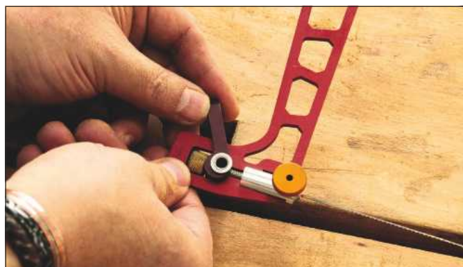
A combination of the knurled rear screw and the cam lever are used to set the tension
