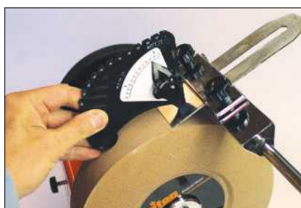
Checking the correct grinding angle
