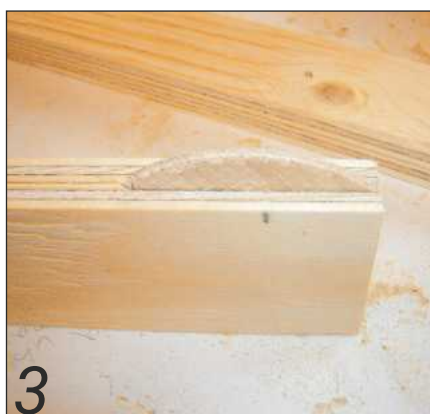
The four main drawer frames were assembled with No.20 biscuits...
