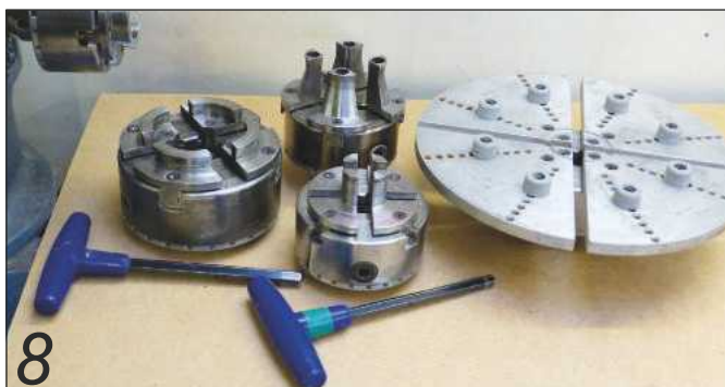
8 Four-jaw scroll chucks have transformed the turning of bowls and hollow forms with their ease of use
