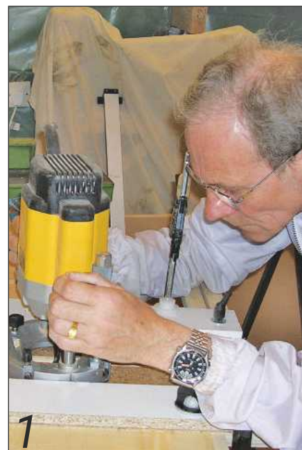
I used a homemade jig to rout the housings in the sides for the drawer frames...
