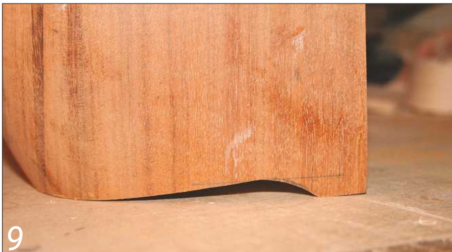
9 You can add some detail to the base of the piece by shaping the cut, which can be rather attractive
