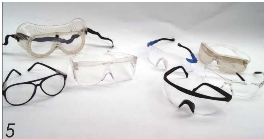
The safety glasses on the left can all be worn over ordinary spectacles; those on the right cannot. Note that most of them try to enclose the sides and some enclose the top as well. Ordinary spectacles do not do this
