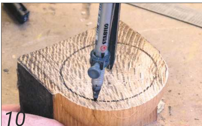
Use a pair of compasses to find the centre of the bowl – a bit of trial and error
