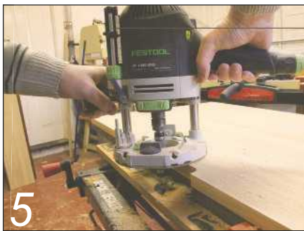
5 The final shape was machined using the original as a template
