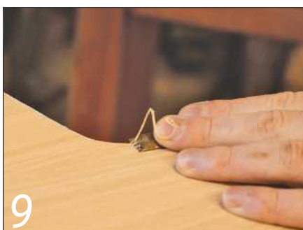
9 After being attached, the edge pieces were trimmed using a sharp chisel
