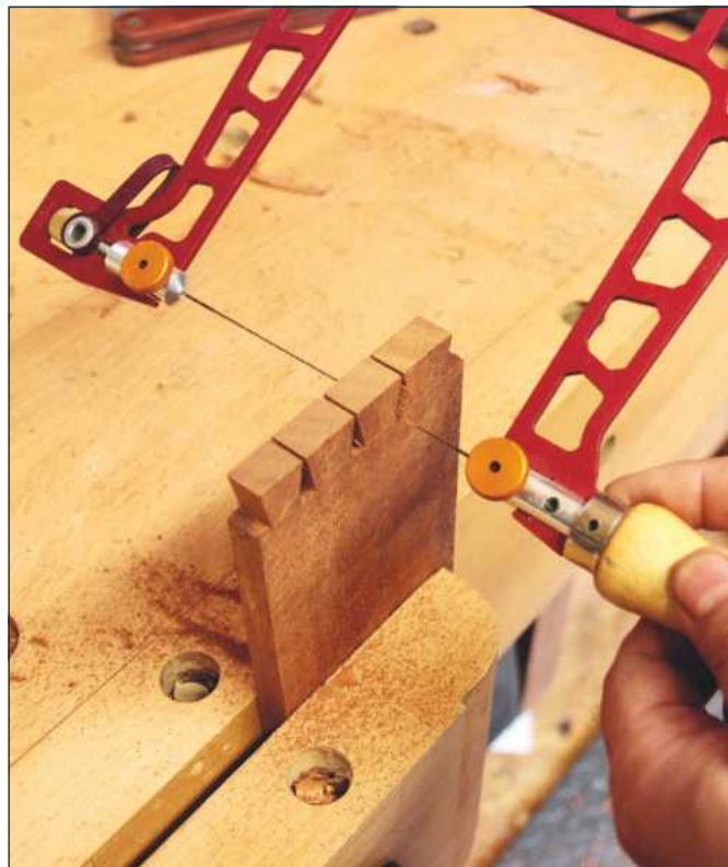
The frame is very light weight for cutting in sideways orientation, such as on dovetail work
