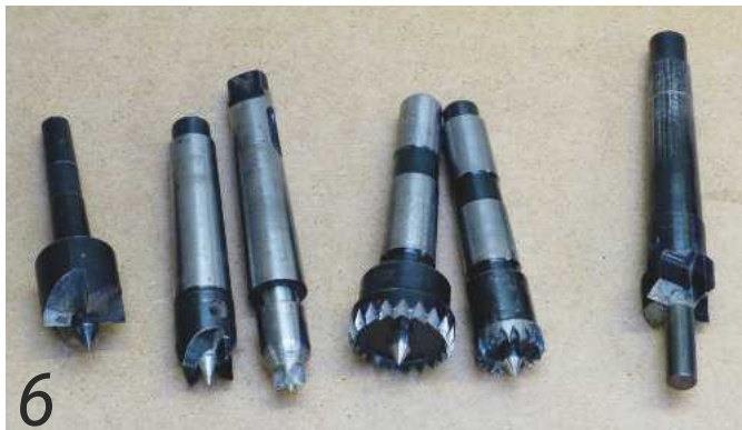
6 Four-prong drive centres are often supplied with lathes but may not be the best choice for beginners
