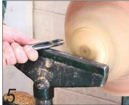
A push cut helps to flatten the base
