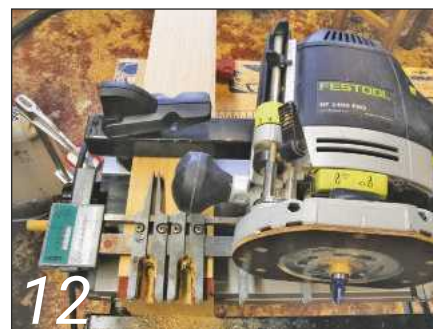
12 The dowel rebates for the lid were machined using a router and a dovetail jig
