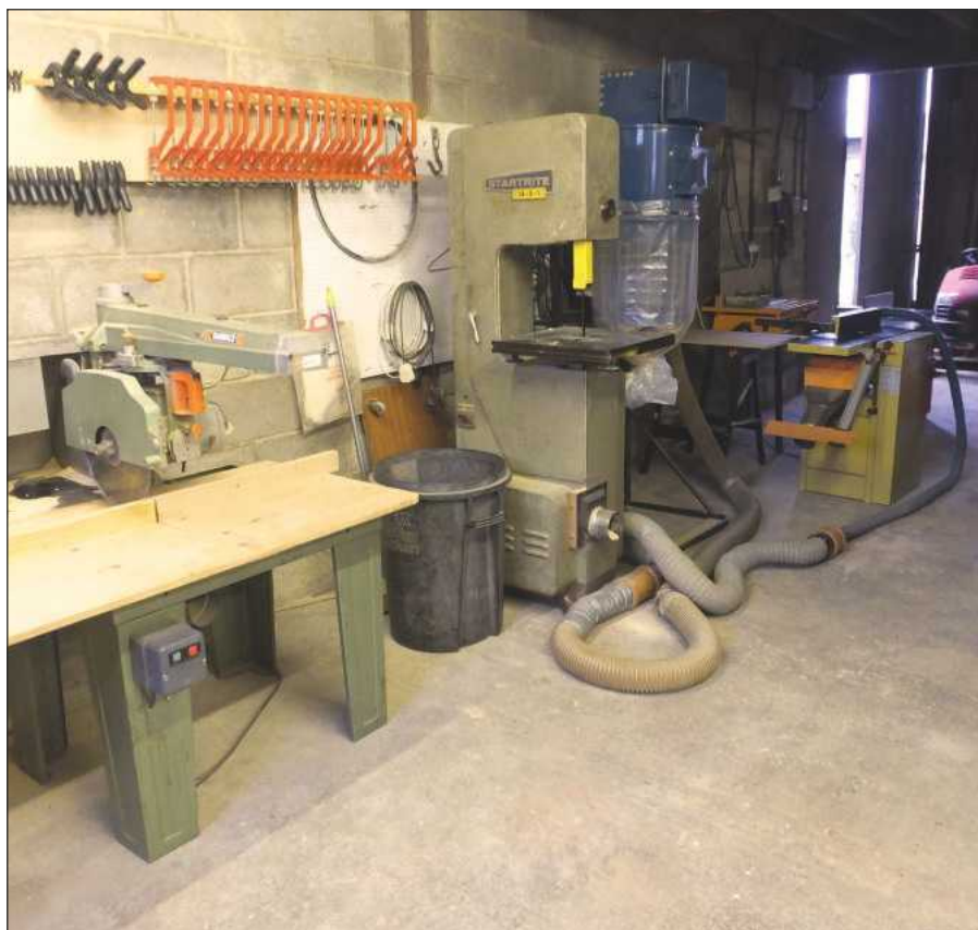
The big bandsaw and extraction system ready for action
