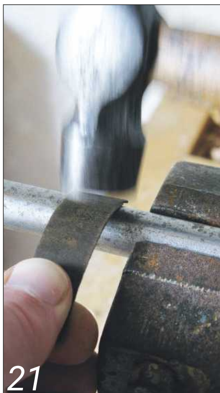
Forming the hook around a steel bar
