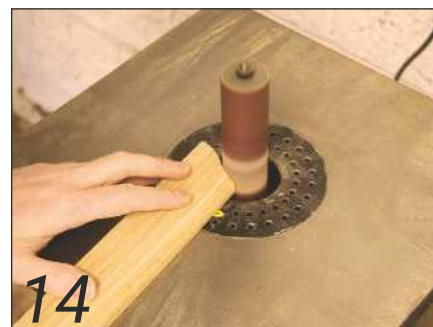
14 The music stand pieces were rough-cut on the bandsaw and shaped by a bobbin sander
