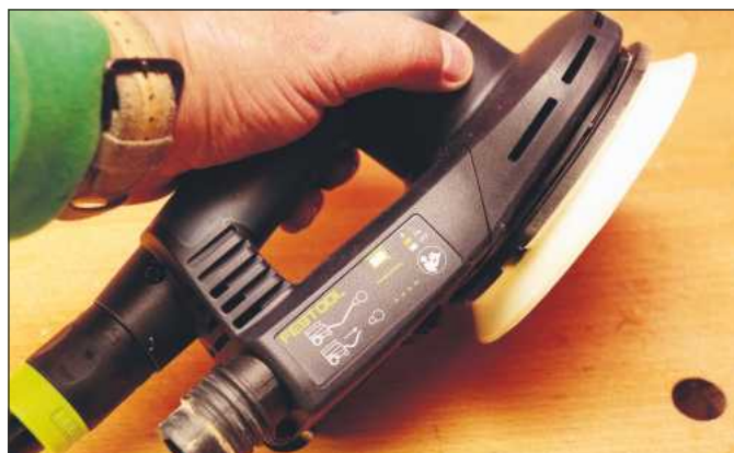
The LED indicator tells you whether the sander is set for extraction detection
