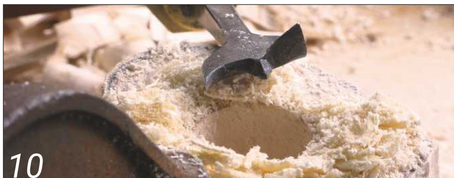
10 Boring the 'pilot' hole with a centre bit
