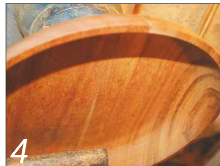
4 Turn out the inside of the bowl using a template to maintain an even wall thickness
