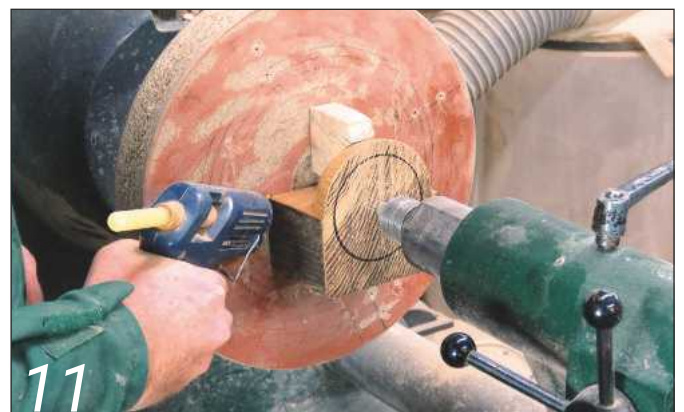
Use the tailstock again to centre the piece and glue it to the faceplate
