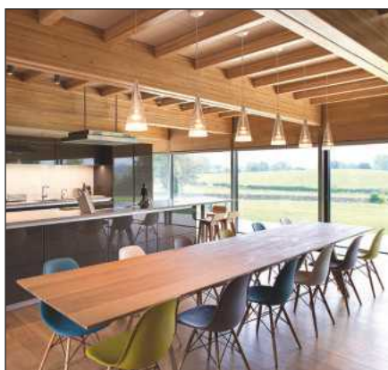
A combination of American white oak, European oak and some stainless steel has been used for the superstructure of Contour House
