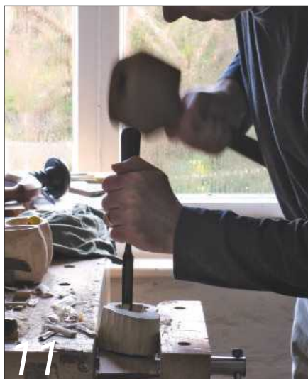
11 Enlarging the interior with a 12mm gouge
