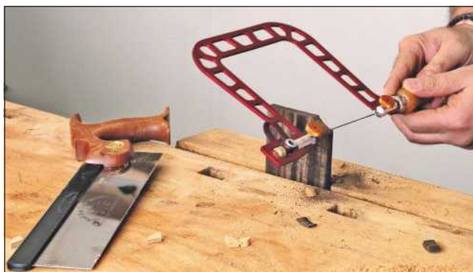
Even on dense stock the blade remains taut with minimal bow
