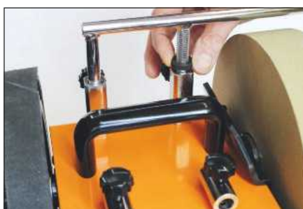
The support arm is fully adjustable and locks into position
