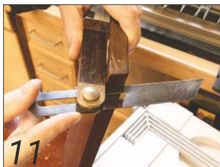
11 An angle gauge was used to set the planer fence for cutting the larger sections' edges
