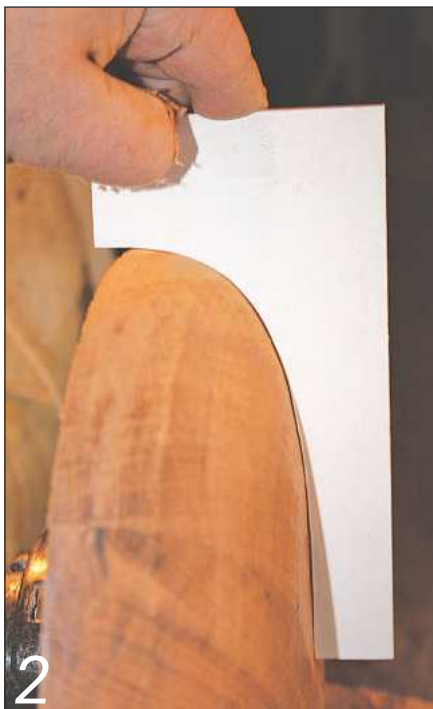
2 If necessary, use a template to help you turn the outer face of the blank to shape
