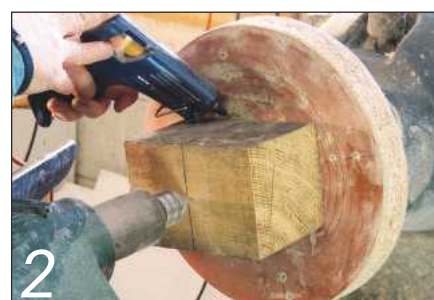
2 Use the tailstock to centre the piece and glue it to a faceplate
