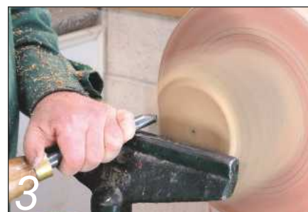
3 Make pull cuts to start shaping the outside...
