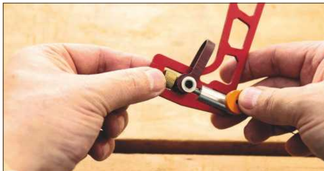
Once set correctly, the tension lever on the saw sits back vertically
