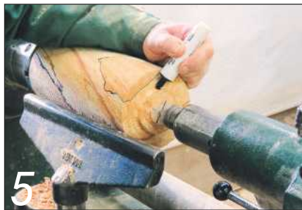
5 Mark a witness point on both spigots to help with alignment later
