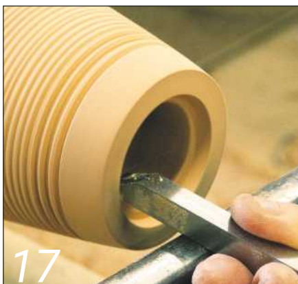
17 Carefully cut the step in the bottom for the plug...
