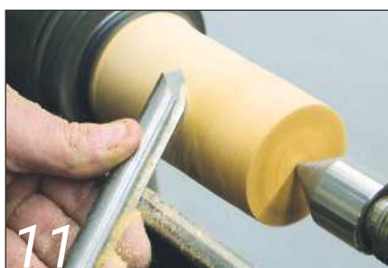
11 Practice this cut, keeping the cutting edge at about 45° to the wood
