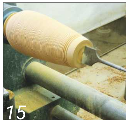
15 Drill about three-quarters of the way down...
