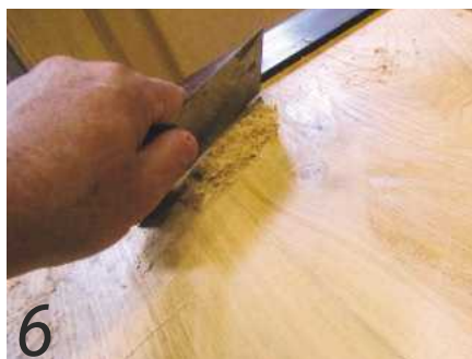
6 Once the glue had dried, a few minutes of work with a scraper reduced the damage to a barely visible pair of parallel lines
