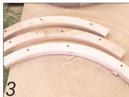
Curved pieces for the pull out blinds
