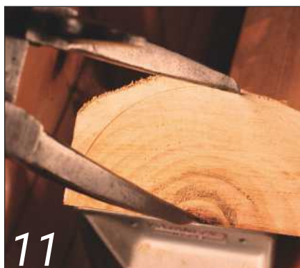
Scribing a handle with wing dividers
