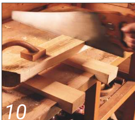
Sawing ends square supported by bench hooks and holdfasts
