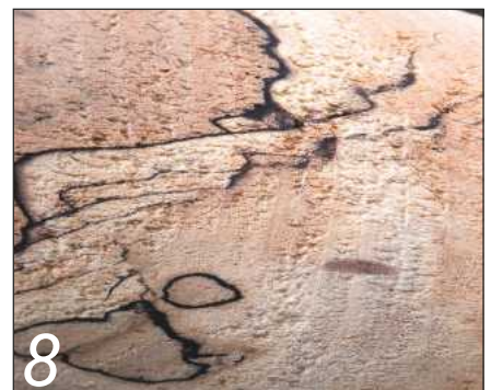
8 Spalted wood can tear-out very badly
