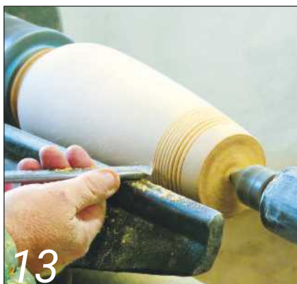
13 Use the point of a skew to make a series of 'V' cuts...
