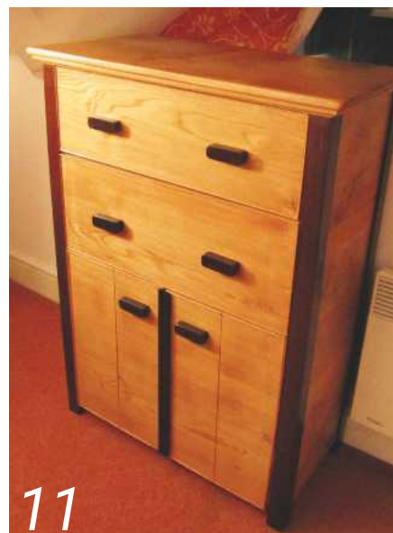
11 With the repairs finished, sanded and oiled, the piece was ready for a new and more elegant life. One mistake stayed untouched: the front leg near the camera still bows out to the side at the bottom. But, even at its worst, the gap is less than 5mm – too small, in my view, to justify major reconstruction
