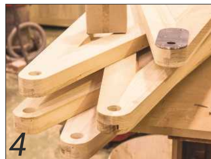
4 Finished roof fold out sections
