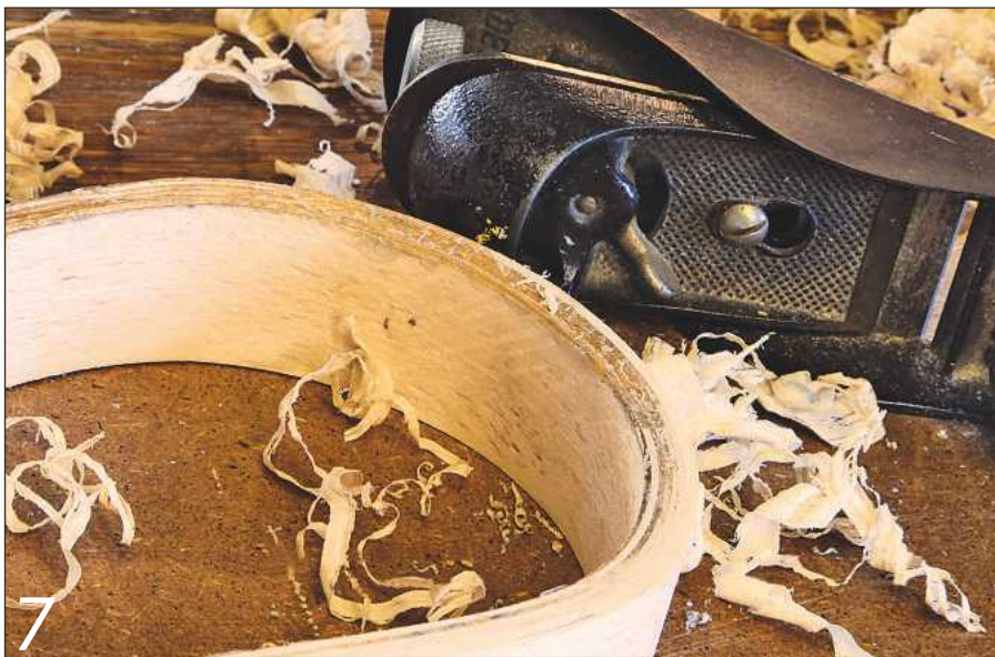
A bit of work with the block plane revealed some respectable glue lines...
