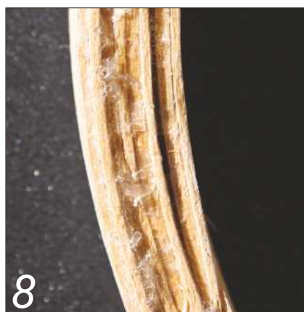
8 ... and some flaws, too. A snugger fit between the formers and veneers would help prevent voids like this
