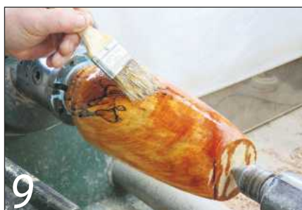
9 Give the piece a liberal coat of sanding sealer...
