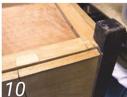
10 Some parts survived intact. The dovetailed beech frame (from an old kitchen worktop) didn't shift, and the magnets let into the bottom (behind thin pine lids) continued to work. Note that the bulk of the corner post doesn't reach the frame. It's simply a small wenge block glued into the L-shaped corner for appearance
