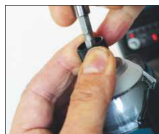
Fitting a screwdriver bit into the sprung sleeve
