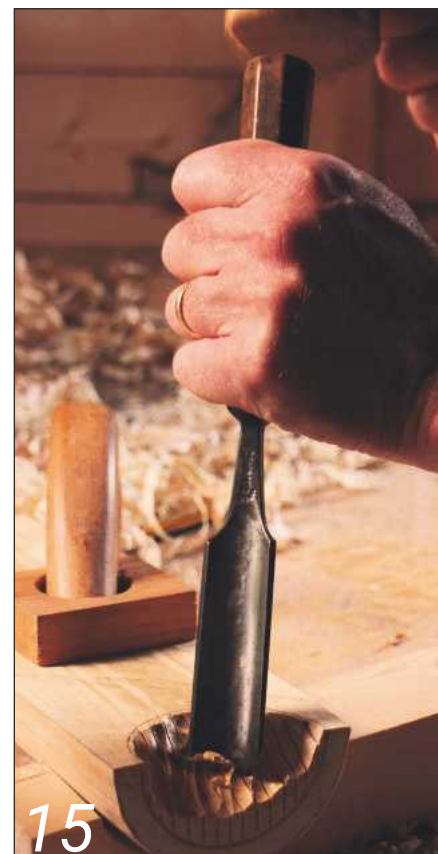
15 Removing waste with a 25mm gouge
