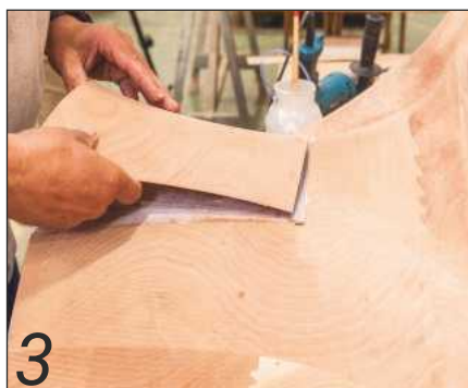
3 American cherry components being glued into place
