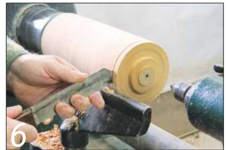
6 Part off the plug and put aside
