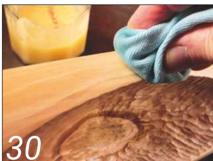
Applying the finish with a cotton cloth
