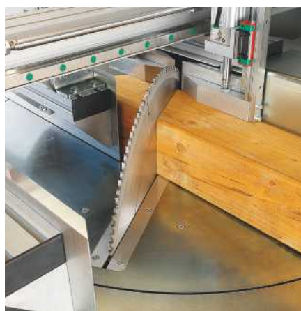
Automatic angle cutting on a Salvador S600
