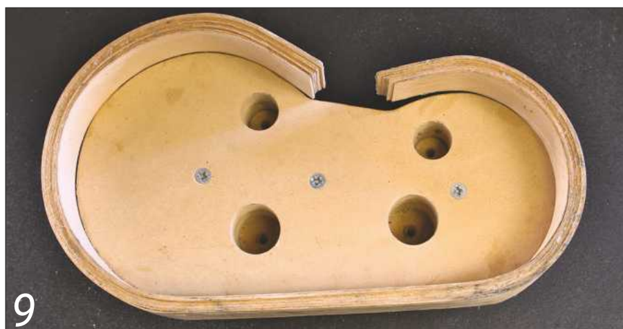
9 The glued veneers didn't move much when released; the apparent movement at the end of the small radius is actually due to the veneers not being cramped all the way round the bend
