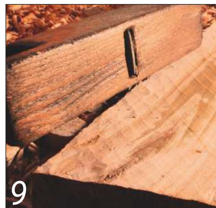
The rippled surface left by the scrub plane
