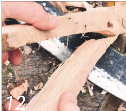
Oops! Where grain swerved around a knot the split ran to the side
