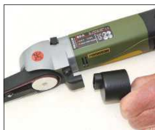
It also comes with an effective device to fit a standard dust extractor hose
