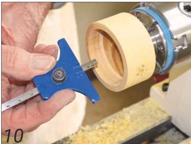
10 Hollow out the lid. A depth gauge is useful to judge how deep to go
