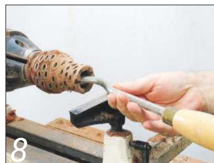
8 Open up the inside by scraping the internal wall
