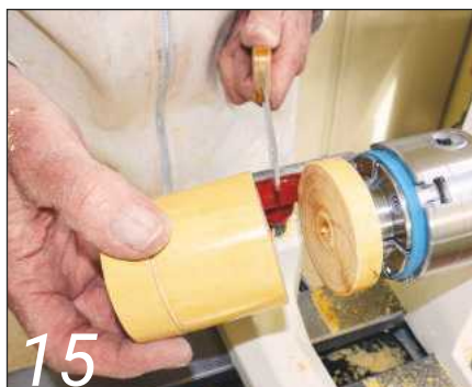
15 Part off the box at the base
