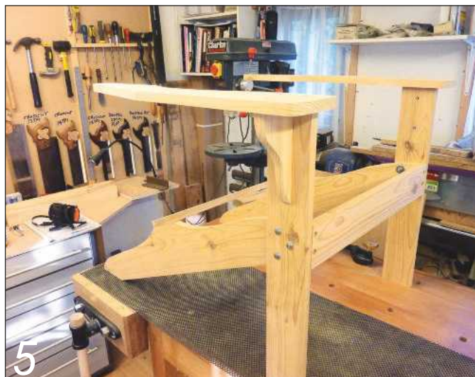
5 Attach the arm brackets and arms
