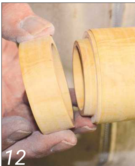
12 Hollow out the body and make a spigot to fit inside the lid. Take very delicate cuts to adjust the diameter of the spigot to produce a satisfactory fit for the lid – this is a matter of judgement. Cut a second very small shoulder on the outer edge of the body. When the lid is in position on the completed box, this secondary recess disguises the fact that the grain does not match up precisely because some of the wood has been removed during parting off
