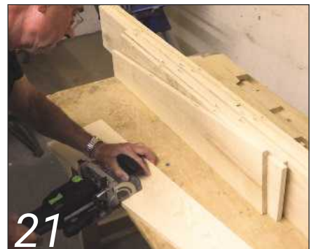
The thin stuff for the side panels needed to be jointed to make the width
