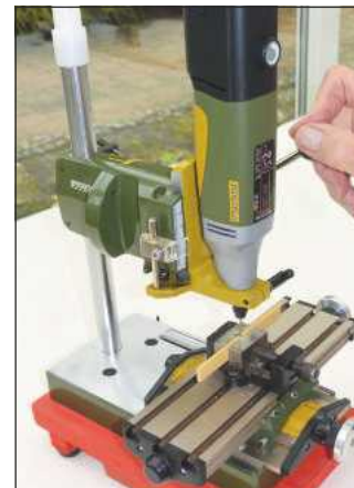
For more precise and accurate work, it is best used in the drill stand, shown here with the x/y table and small machine vice
