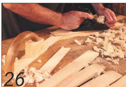
26 The planing setup of holdfast and pivoting bird's mouth batten used for thin, narrow timber
