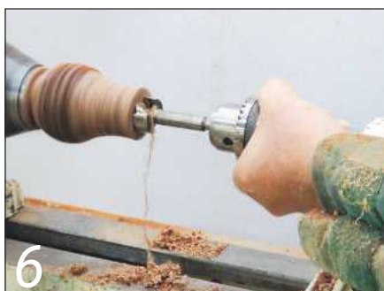
6 Bore a hole into the end, ready for hollowing
