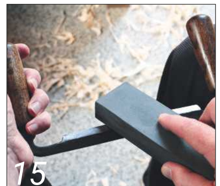
Honing the drawknife using a carborundum oil stone
