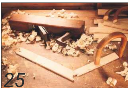
25 Using one bird's mouth batten to make another, clamped by a 'walking stick' holdfast
