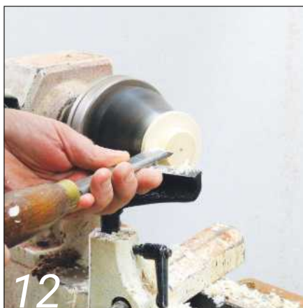
Turn a spigot on a scrap piece to fit the hole in the nut
