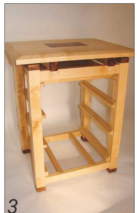
3 The top floats on the frame, sitting on two supports. Note cross-rails at bottom
