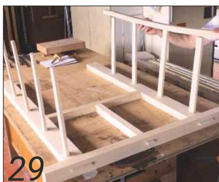
29 Side panel pieces are fitted
