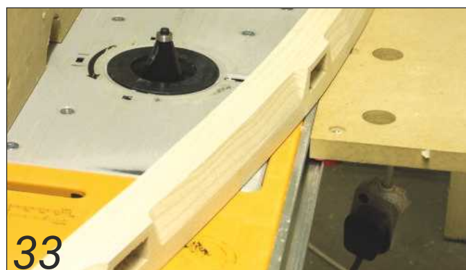
33 Once all the joints are made, the fancy bevelling can be applied
