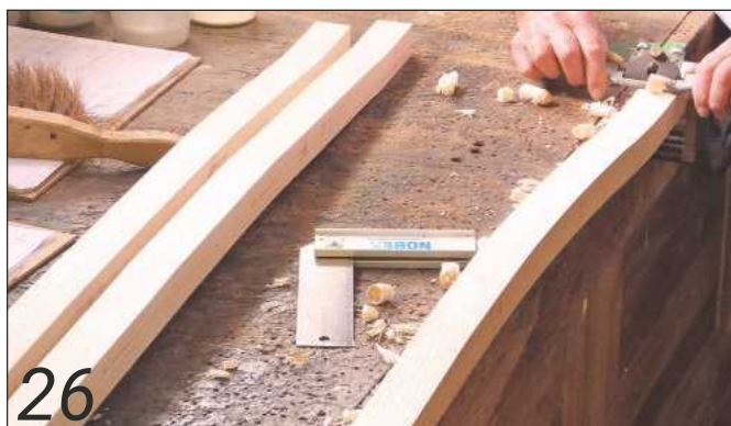
The spokeshave again, which was used to finish the top rails to shape
