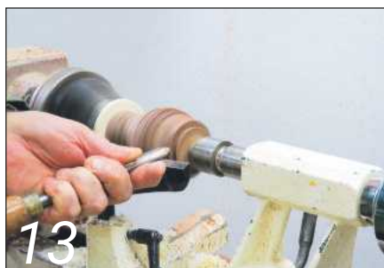
Mount the nut on this spigot and complete the bottom
