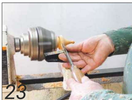
Finish the shaping using a spindle gouge
