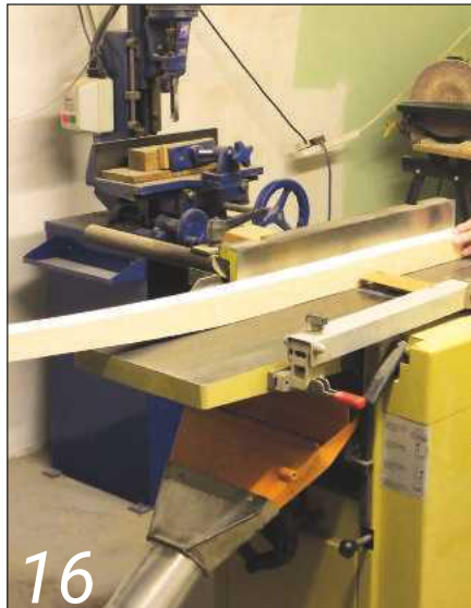
16 The face of the shafts that adjoins the frame needed to be squared up
