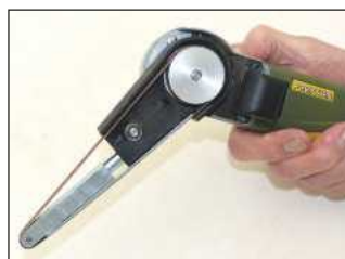
The machine has an adjustable arm, which can be rotated up to 60° from the horizontal
