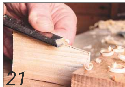
An approximately 6° slope gave the wedge good holding power
