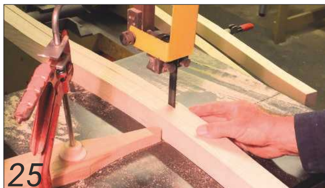
A bit of 'single point' cutting on the bandsaw finished the roughing out
