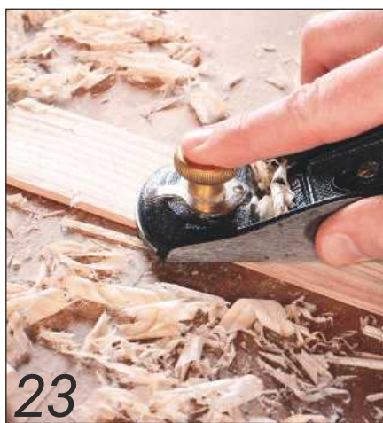
A shorter piece held against a dog with one hand while using the block plane
