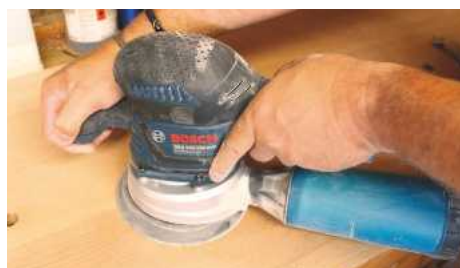
The final section of my bench was sanded with the new base and the M480 fitted
