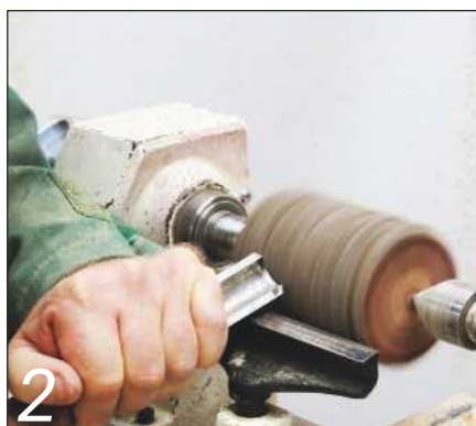
2 Rough it down to a cylinder...
