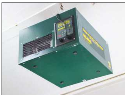
Suspended from the workshop ceiling; make sure your fixings are sound
