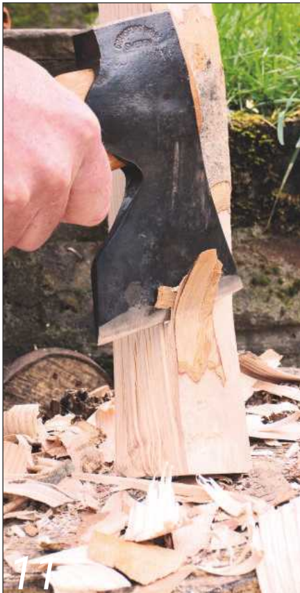
Hewing away splinters with the carpenter's axe
