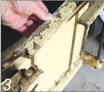
3 This outrider is so 'friable' that it falls apart at the touch
