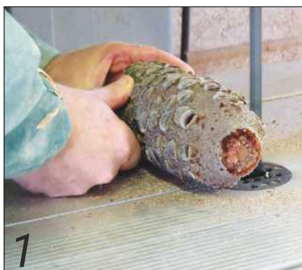
1 Cut a length of banksia nut on the bandsaw
