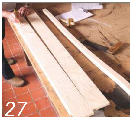
27 The sub frame is marked out to take the side and front panel stub tenons
