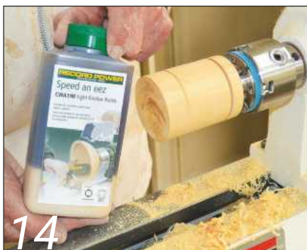
14 Two coats of friction polish applied to the rotating wood will produce a good, lasting shine
