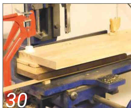
30 The front panel piece is jointed, and once again packed out to cant the mortise holes
