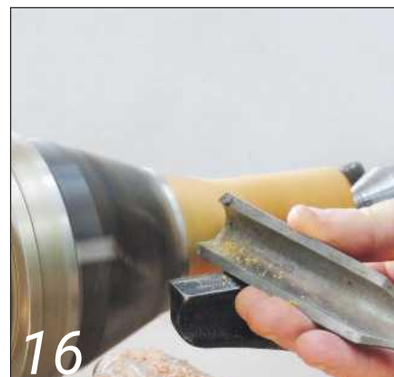
... but ensure to keep the tool away from the chuck
