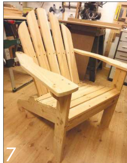
7 Assemble the back slats to give an evenly distributed fantail
