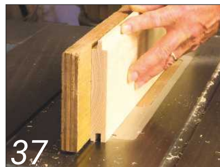
37 Making the tongue & grooved flooring from square planed stuff
