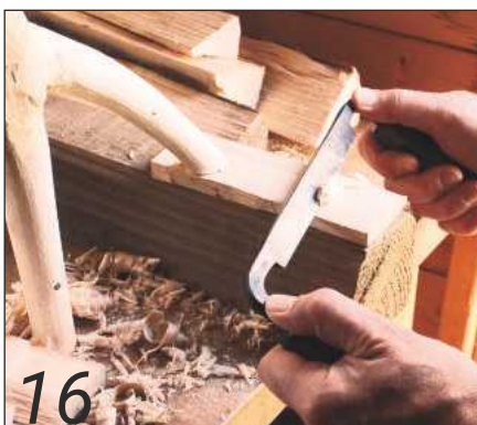
Using the drawknife on wood gripped by the grown ash holdfast
