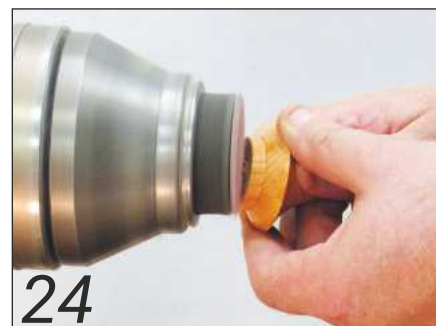
Sand the underside of the cap using a power sanding arbor
