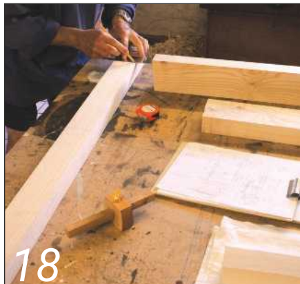
18 Having planed the stuff up, the sub frame is marked out
