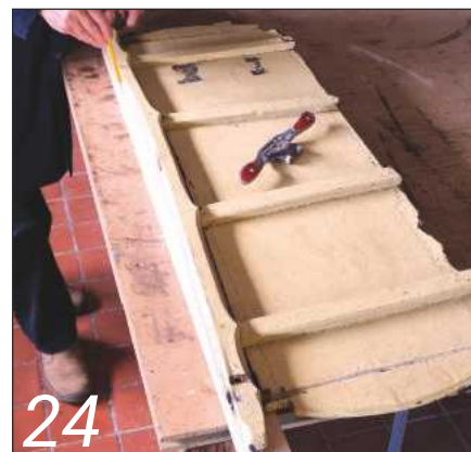
Each top face shape of the side panels was marked out from the originals
