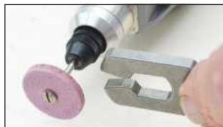
The collets are tightened using the spanner provided
