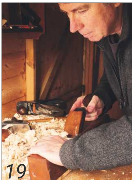
Planing aslant on the wedge-shaped timber
