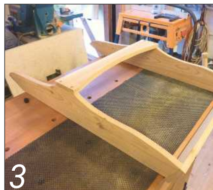
3 Side members, lower rear crosspiece and front crosspiece assembled
