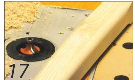
A large quarter-round cutter in the router shaped all the edges
