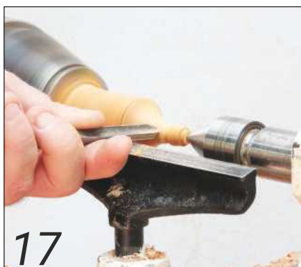
Start at the tailstock end and work from right to left
