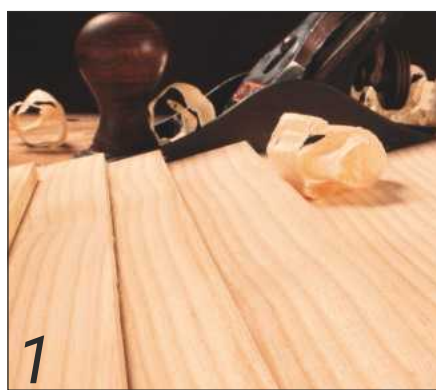
1 Ash from the log, planed flat, square and ready for use
