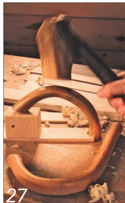
27 A softwood block spreads the down force of the holdfast beak, here being tightened with my branchwood mallet
