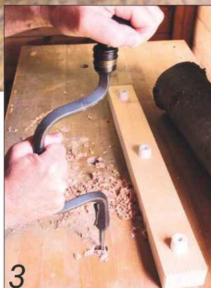
3 Adding a dog hole to extend the range of the bench stop
