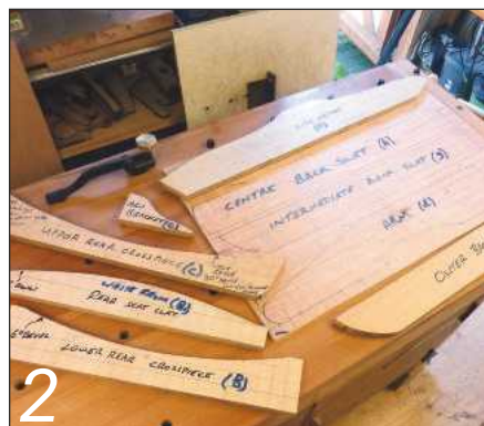
2 Templates for shaped components
