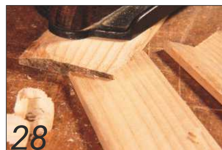
28 The right-angled notch of the bird's mouth batten clamps the work
