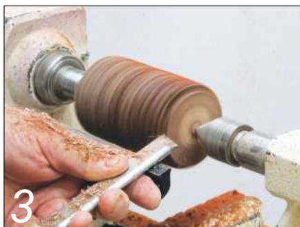
3 ... then cut a spigot for your chuck
