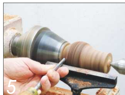
5 At this stage, keep the diameter large
