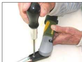
Tracking for the belt can be adjusted to the right or left and locked by a screw
