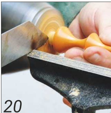
Part off using a narrow parting tool
