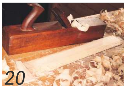
The wood was clamped between dogs using thin ash wedges for initial planing
