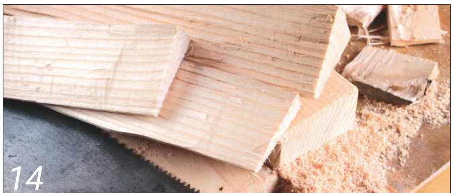
Riven wood has a triangular cross-section
