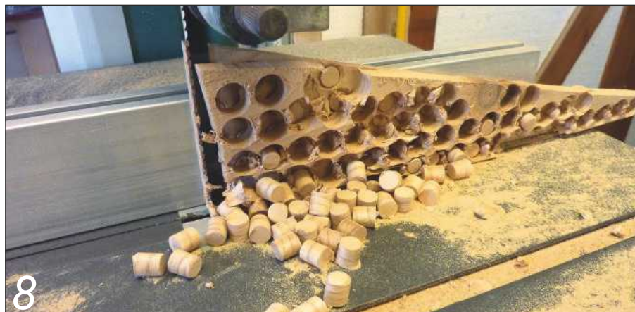
8 I cut lots of plugs using an offcut of cedar and then passed them through the bandsaw
