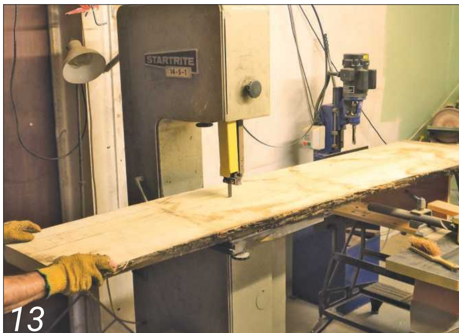
The first side profile of the pair of shafts was cut on the bandsaw
