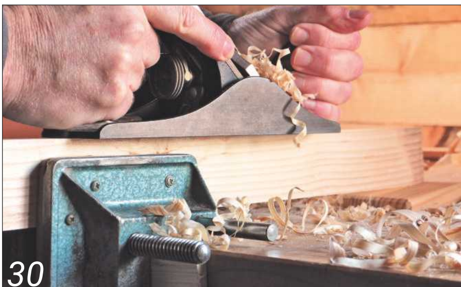
30 Edge planing with the Parry & Bott portable woodwork vice
