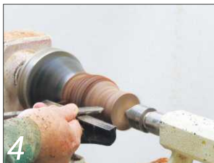
4 Initial shaping with the spindle gouge
