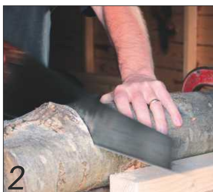
2 Sawing the forked end square using the big bench stop
