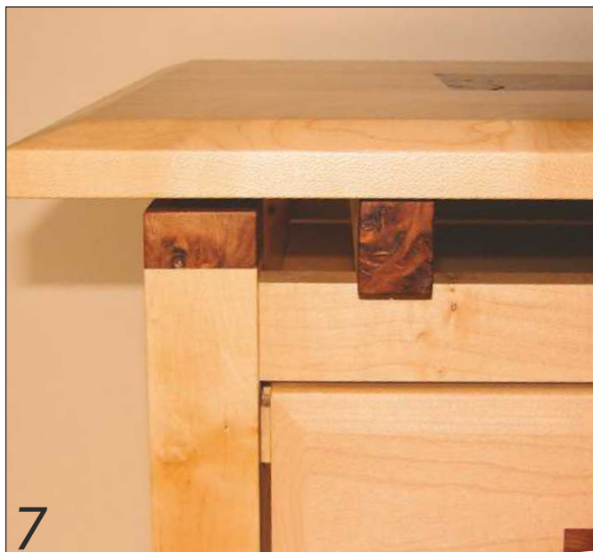
7 Detail of floating top and corner post
