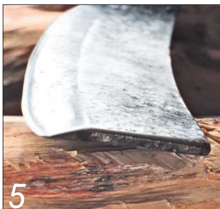
The Quirky Quercus froe is forged with a curved edge
