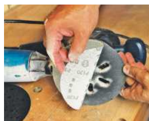
Fitting an M480 disc to the standard base, I proceeded to sand the top of my beech bench
