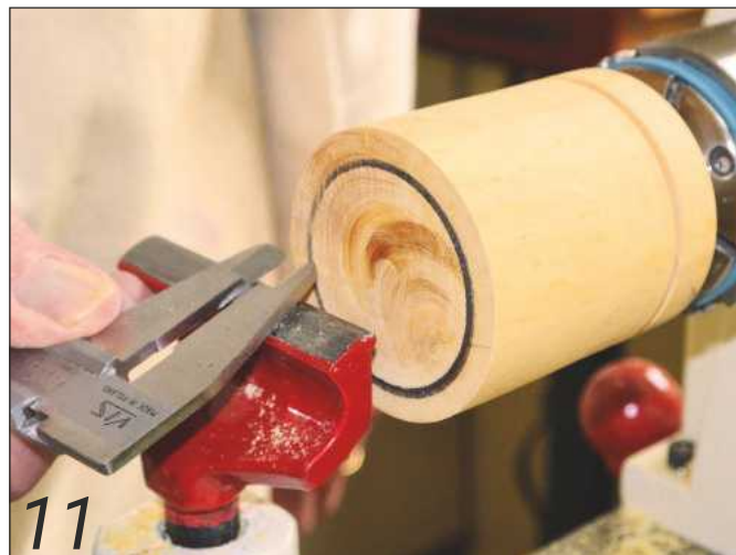
11 Remount the body blank and again, mark off the wall thickness
