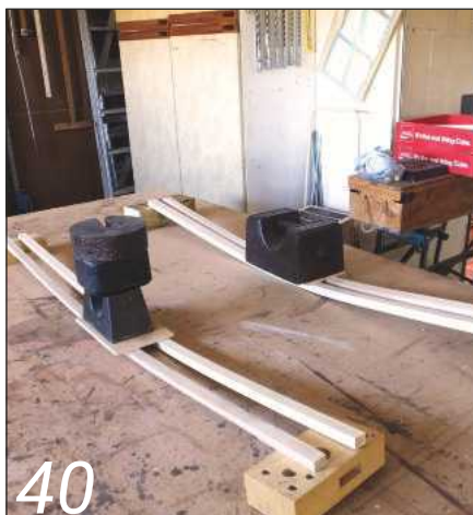
40 A weight just bends the outriders while they cool off
