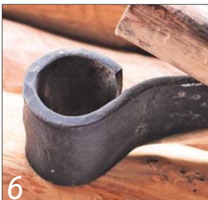
A one-piece forging has no weak spot of a weld at the handle eye
