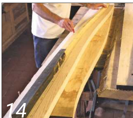
On this piece, I then marked out the full profile of both shafts and cut them out
