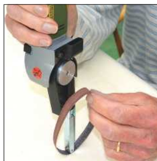
The belts are easily changed by pressing the end of the spring-loaded arm. They last a long time and can be de-clogged
