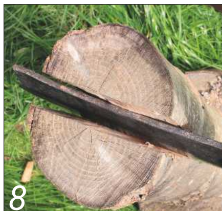
Levering the handle to twist the blade and extend the split
