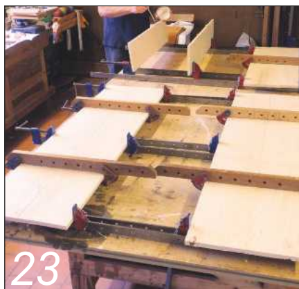
All clamped up bar the tail gate panel
