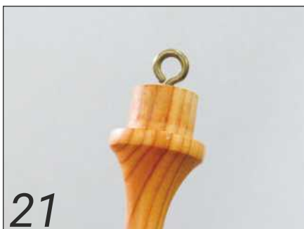
Screw an eye hook into the end of the finial
