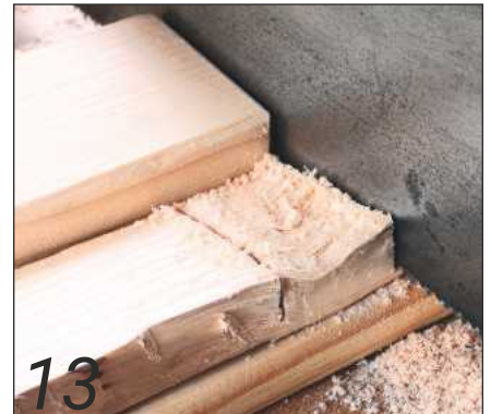
Sawing out awkward knots
