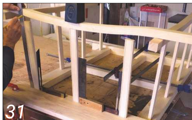
31 Marking out the positions of the mortise holes in the front, top rail
