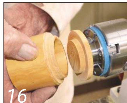
16 Using the remaining wood left in the jaws, form a spigot to produce a jam chuck
