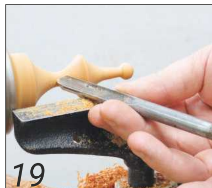
Cut both sides of the cove alternately
