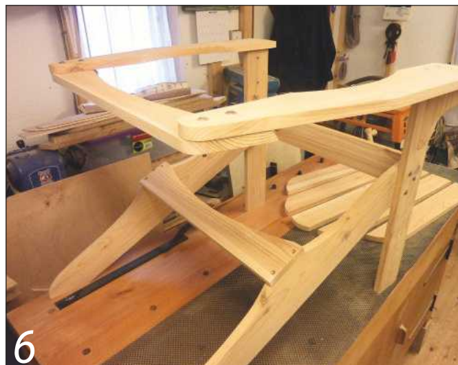
6 Secure the upper rear crosspiece beneath the arms with coach bolts
