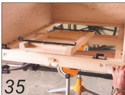
35 The tail gate hinge pins needed to be recessed to fit
