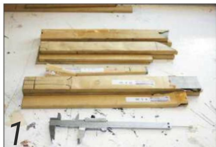
1 Tool blanks cut to length
