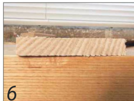
6 Quartersawn timber allows much less scope for the rings to straighten and results in a much more stable board
