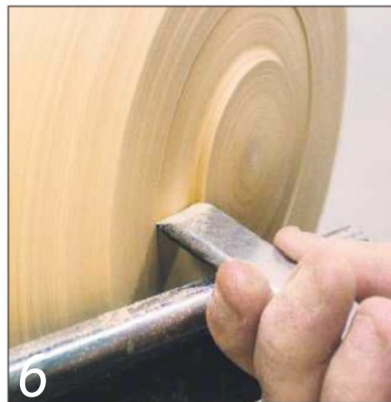
... and cut the dovetail with a skew
