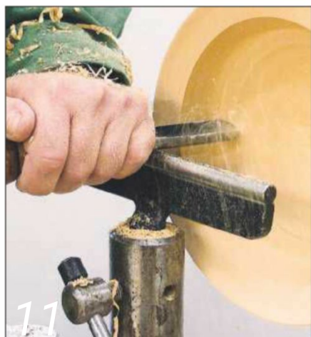
11 Cut a little wider and deeper with each pass
