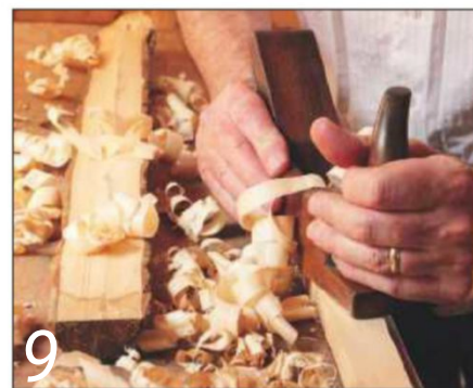
9 Flattening the maple with the Bismarck jack plane
