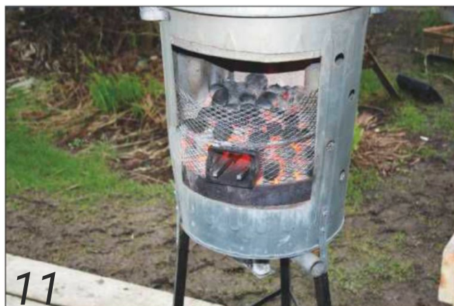
11 Improvised forge used to heat the tools
