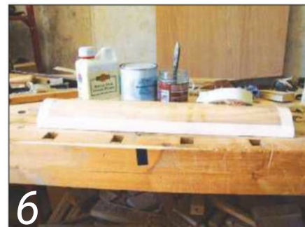
The outside edges of the trough were taped up before I began to apply the finish
