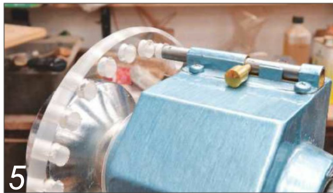
Indexing is a handy feature, although most lathes don't have it
