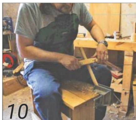
10 The feet were shaped up from ash offcuts using the same drawknife/spokeshave combination
