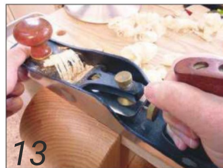
13 Taking twin shavings from two boards together – it's best to use a straight, rather than radiused, cutter for this
