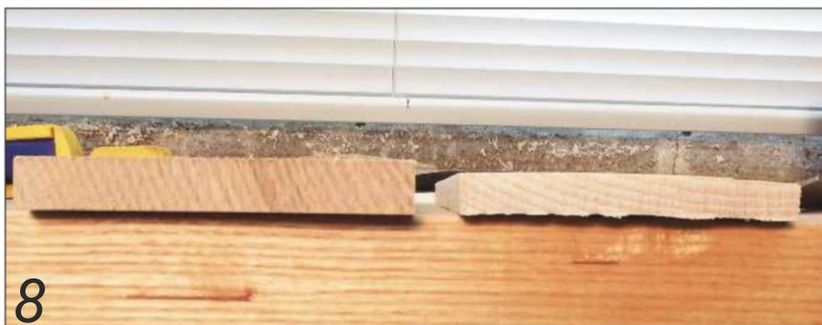
8 After a time in the offcuts rack, the quartered board is still flat while the plain-sawn one is distinctly cupped
