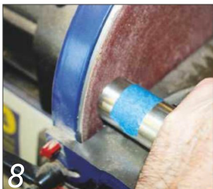
8 A ferrule being sanded square in the jig
