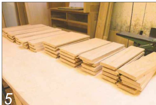
Some of the frame components cut to length
