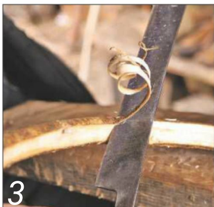
Using a drawknife to shave off any sharp edges of the hazel boole – the bottom of the basket
