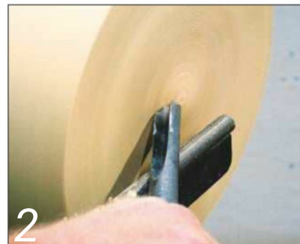
2 Roll the tool up for a bevel supported pull cut
