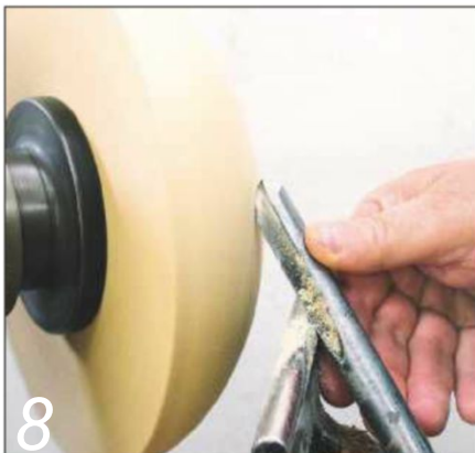
Make light finishing cuts, keeping the cutting edge at about 45°
