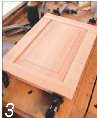
3 ... but for this raised and fielded panel there was no option but to joint up some wide boards
