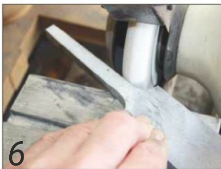
Shoulders being ground on the dressed wheel
