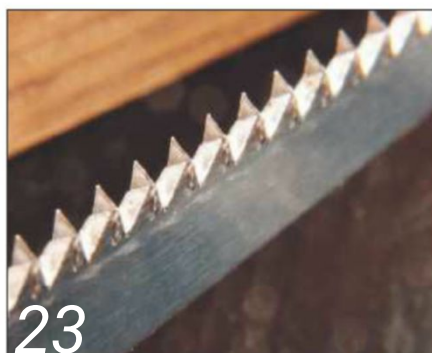
23 Close up on teeth, which are more cross-cut than rip
