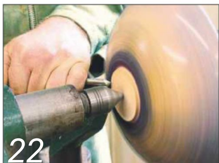
22 Reverse the bowl onto a wooden dolly to remove the chucking spigot
