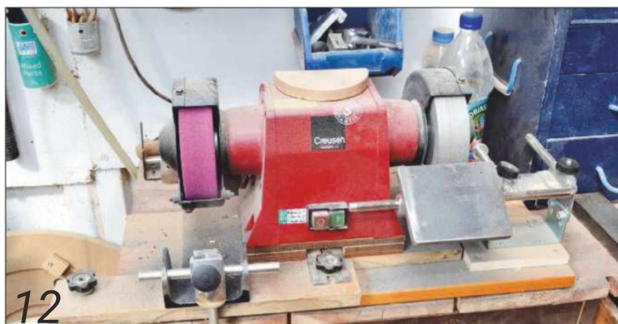
12 Dry grinders usually come with two wheels: one coarse and one fine grit
