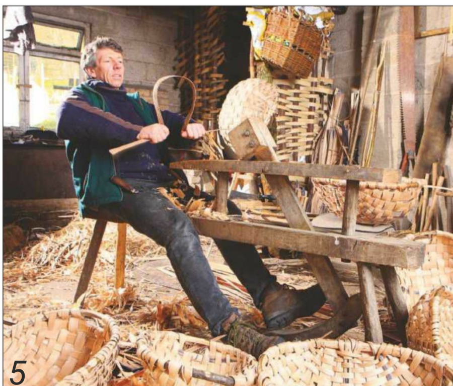
The flexibility of the spelk must be tested after dressing – which, it should be noted, takes some strain on the wrists
