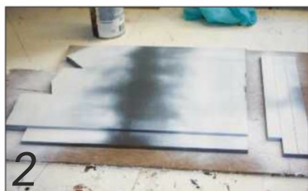
2 Coated with primer and ready for marking out
