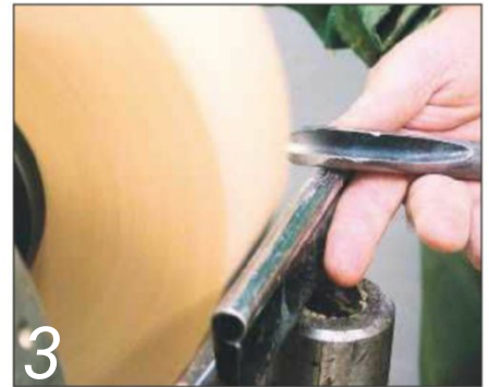
True up the edge of the blank with a push cut...
