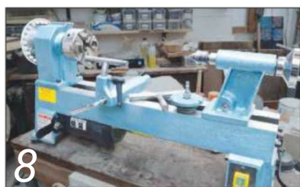
8 My £85 unbranded eBay lathe now features indexing, variable-speed and a vacuum system
