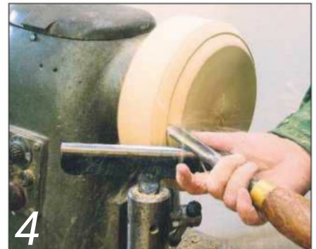
... and start cutting the outside curve
