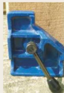
The accessory in question holds the toolrest when the headstock is manoeuvred for turning larger items
