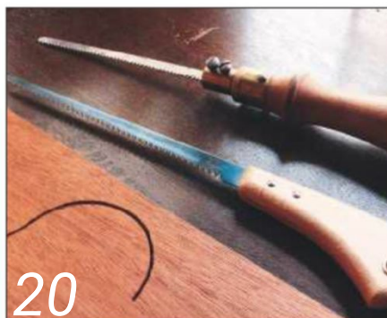
20 The Japanese keyhole saw and the western pad saw
