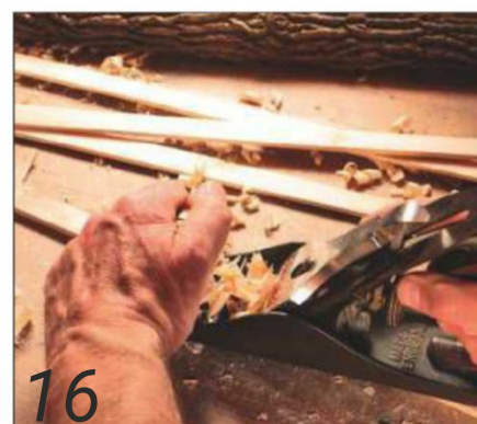
Smoothing away the saw marks with the Stanley No.4
