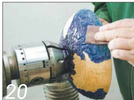
20 A gentle rub with a finger usually removes the masking fluid
