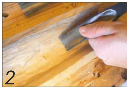
The inside of the trough was gouged out and refined with various tools
