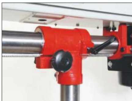
Radial arm support bracket with rack and pinion and locking lever
