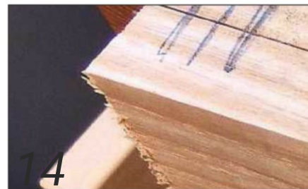
14 Pencil reference marks on each end of the boards help me to take stopped shavings, thereby creating a microscopic hollow in the length
