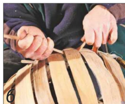
Owen slips on the second working-up taw
