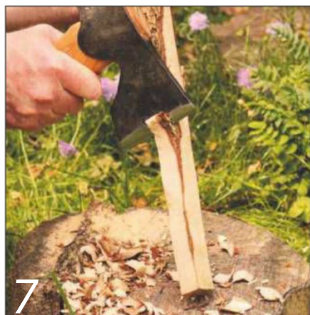
7 Squaring up half a maple log with the carpenter's axe
