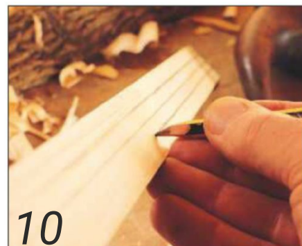
10 Marking for ripping to thickness by eye and pencil
