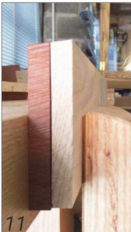
11 I've deliberately planed these two boards visibly out of square...
