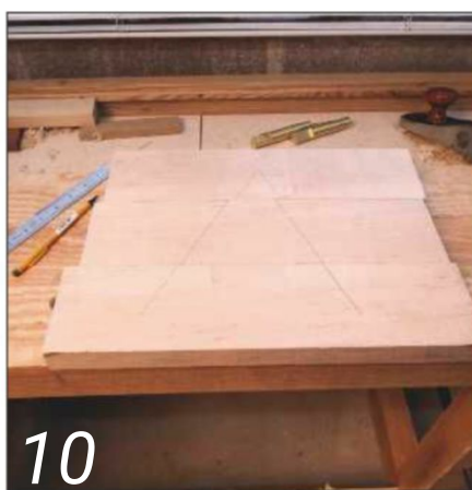
10 The 'cabinetmaker's triangle' is a simple way of ensuring the carefully-prepared boards are not then glued up in the wrong order
