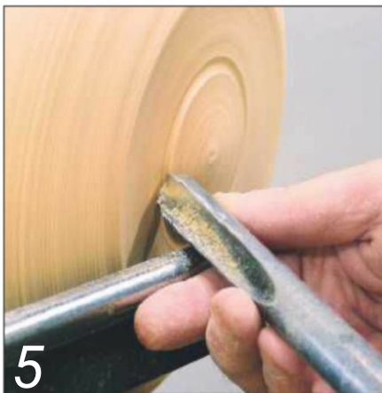
Cut the spigot using the tip of the bowl gouge...
