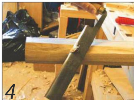
After trying several different tools, a drawknife was used to rough-shape the outside...
