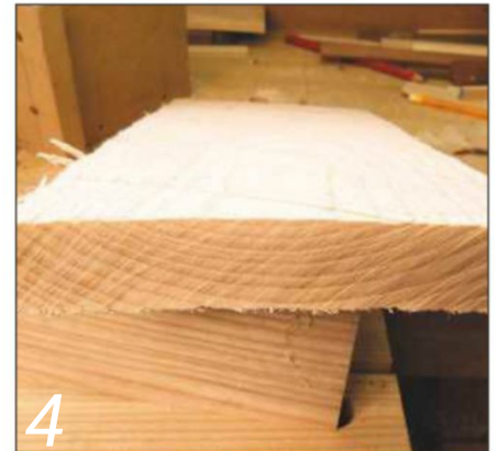
4 Plain sawn timber has the annular rings running across, which leaves the board vulnerable to cupping...
