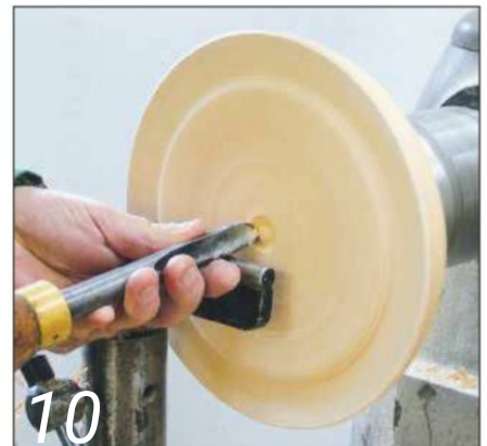
Start the hollowing process using the tip of the tool
