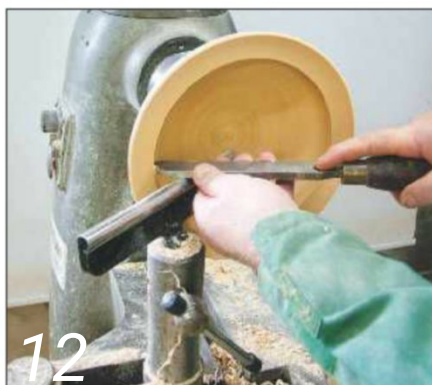
12 Use a round-nosed scraper to undercut the rim
