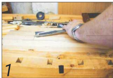
Two square, planed pieces were glued together to provide a blank for 'The Thing'
