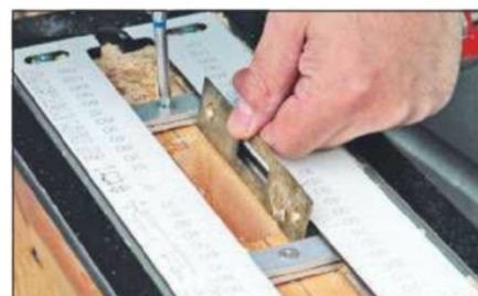
With the case routed and the jig still clamped, the stops are then adjusted for the faceplate
