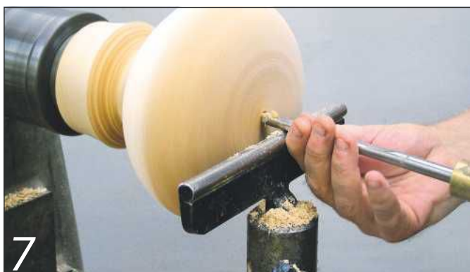
7 Start boring the hole using a spindle gouge
