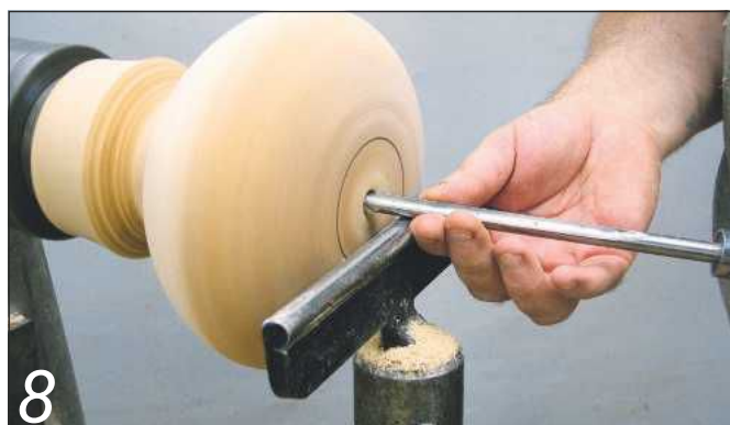
8 Hollow the vase, starting in the hole and swinging the handle away from you, making the cut on the left wing of the gouge
