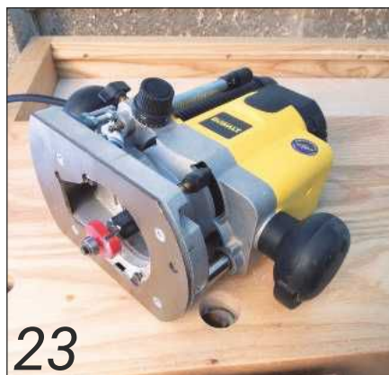
23 The rebate for the glass is best cut afterwards using a bearing-guided cutter in a hand-held router
