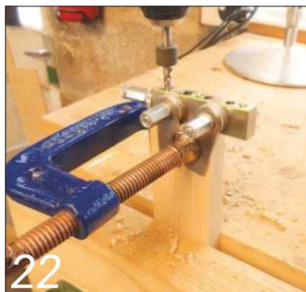
22 The glazed door is a simple dowelled construction, quickly made using my Jointmaster jig
