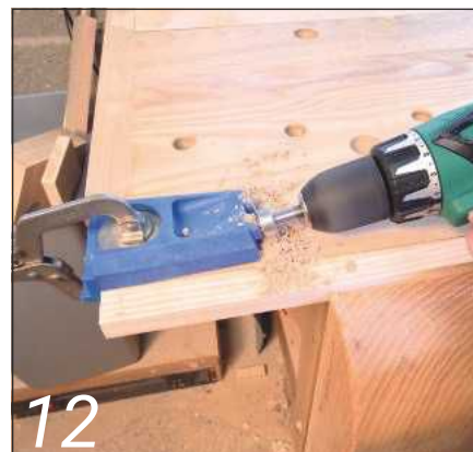
12 Shelf 1 can then be added using a pocket screw jig
