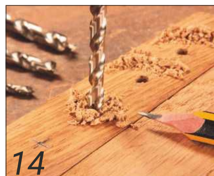
Tidy holes bored in oak by the Lee Valley bits
