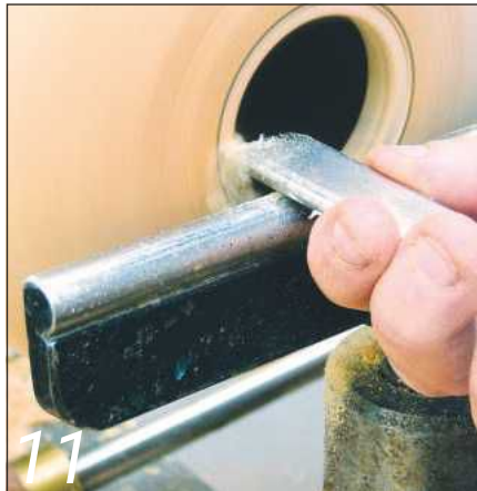
11 Cut a parallel-sided stepped recess at the vase's opening...
