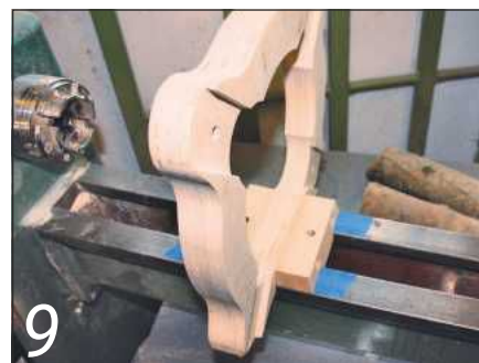
9 Feet glued with frame in position
