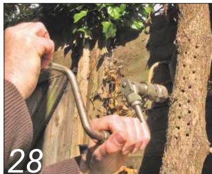
Boring nest holes for mining bees with the brace and auger bit
