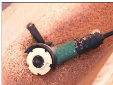
Note how dust can block the grinder's air vents
