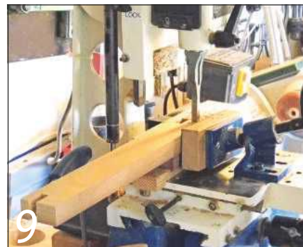
The front corners have a double bridled joint and the rear rail has twin mortises
