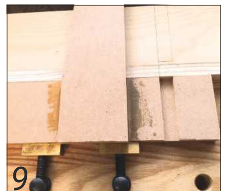
9 Positioning the T-square is then simplicity itself
