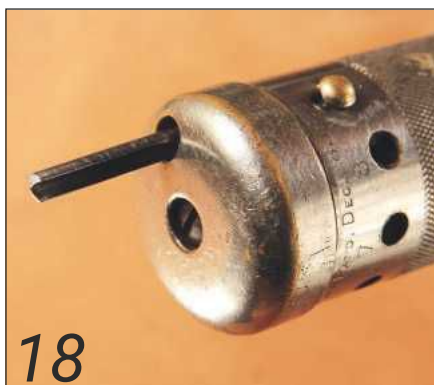
Eight bits are stored in the handle and the holes indicate their sizes
