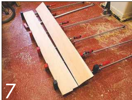
7 The leg fronts were glued up separately to give matching glue lines
