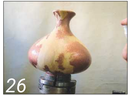
26 Lightly spray the ageing solution from a spray
