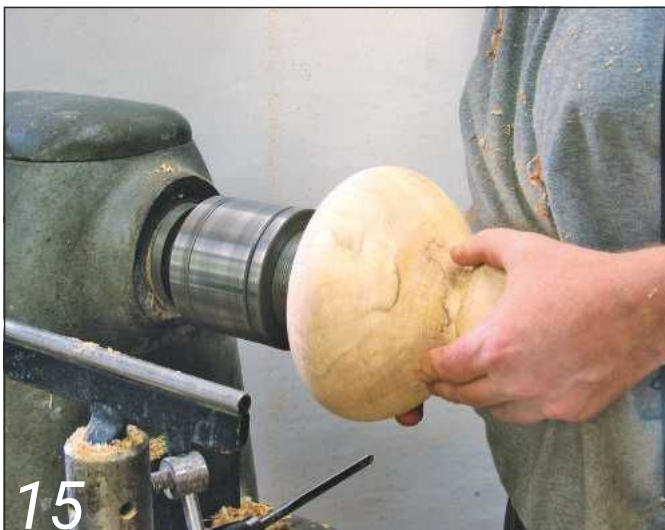
15 Offer up the vase and rub the corner of the stepped recess on the plug's chamfer...
