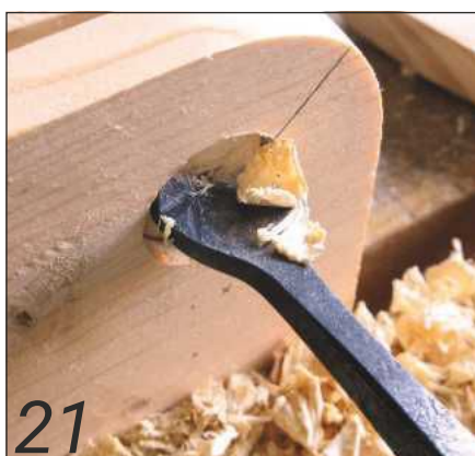
Centre bit boring a hole to hang a tea towel
