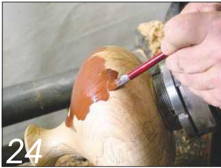
24 ... and apply two coats of primer...
