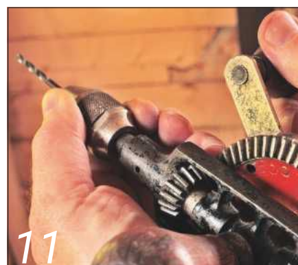
11 Tightening on the drill by turning the crank while holding the chuck firmly
