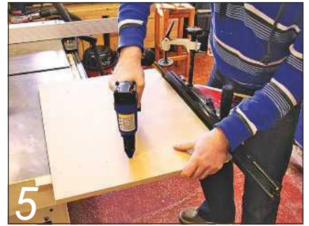
5 An offcut of 12mm MDF made a quick substitute for a 'zero clearance' insert...
