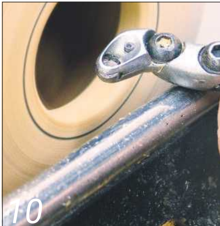
10 ... and a cranked or articulated tool to remove wood next to the opening
