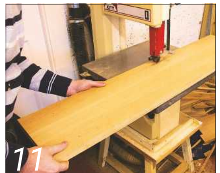
11 A thin blade in the bandsaw cuts away the bulk of the waste for the curve...
