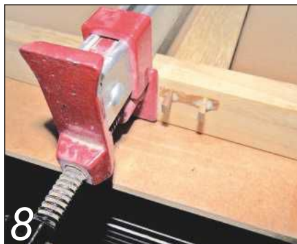
... checking for squareness, and inserting wedges in the tenons
