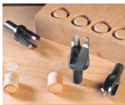
Veritas' Snug-Plug Cutters , as tested in WW Sept
