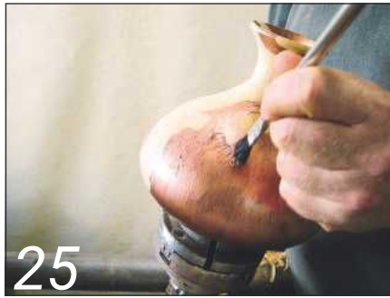
25 ... followed by two coats of metal reactive paint
