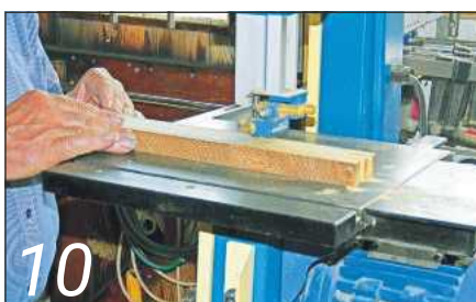
The curve on the top edges for the front and rear rails can be cut using a bandsaw
