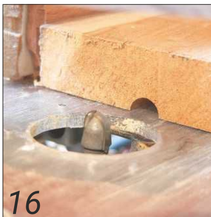
16 To create a long hole along the length of the centre table support, I routed semi-circular slots in the two pieces...
