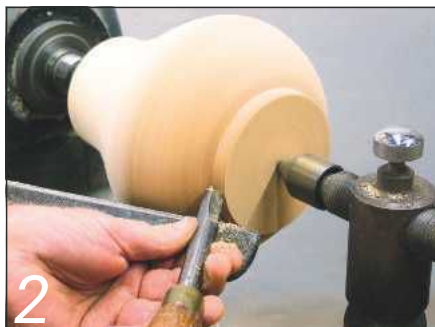
2 Refine the shape using a spindle gouge
