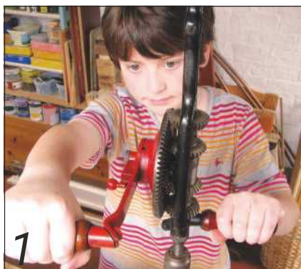
Tom using the massive Millers Falls 97 breast drill
