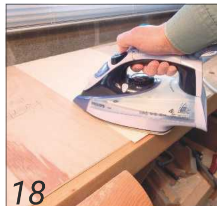
18 With the ply cut to size, I ironed on the veneer over the exposed area...
