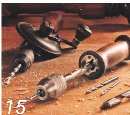
Goodell-Pratt No. 101 reciprocating drill designed for boat builders
