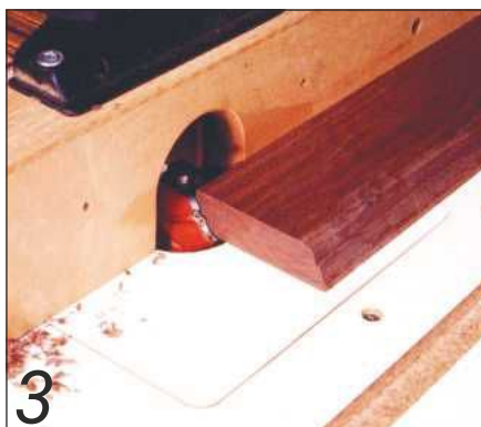
3 Rout an ogee profile into the edge of each mitred frame
