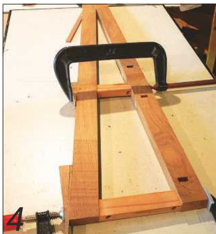
4 The wings were assembled on the bench, using wedges retained from the angle-shaping
