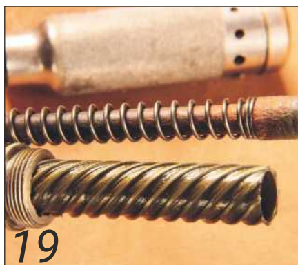
Spiral drive shaft, return spring and its wooden guide rod
