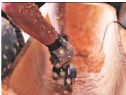
The cutter leaves gouge-like tool marks
