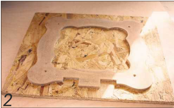
2 OSB base with template mounted
