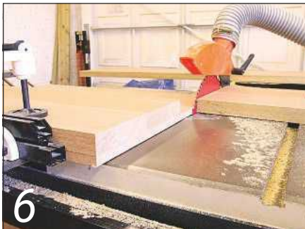
6 ... which produces tear-free cuts across the grain even when using a combination blade
