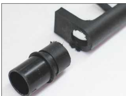
My simple modification to the dust bag frame enabled vacuum connection
