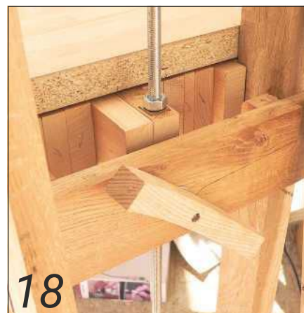
18 The rear table clamp has two vertical battens glued to it to keep it between the posts
