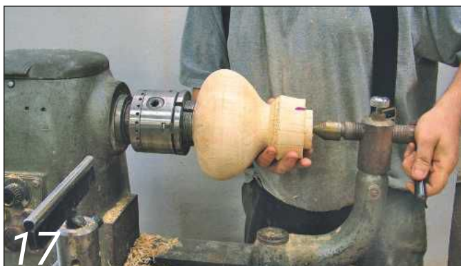
17 Glue the plug in place and use the tailstock as a clamp
