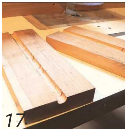
17 ... which were then glued together to provide the necessary long hole for the front-to-back rod
