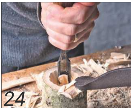
... and enlarging the hole with a gouge...
