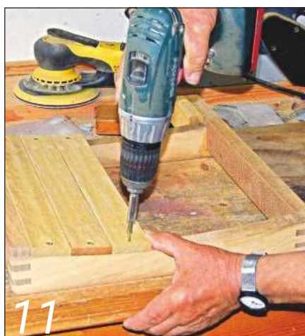
Prepare the seat slats and drill to take 25mm \times 4 countersunk screws, then screw in place
