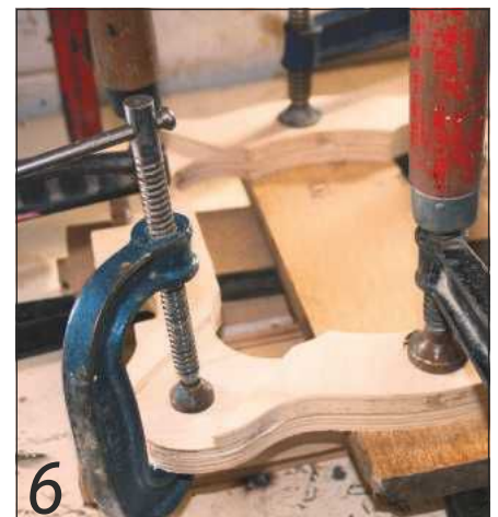
6 Part of the frame being glued
