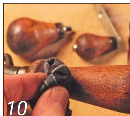
10 Treating the handles with boiled linseed oil
