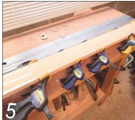
5 I had some remnants of ash-veneered MDF which, once edged with solid, would form the vertical sides. They were cut to width and edged
