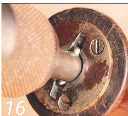
Pins on the spindle engage with the travelling handle to ease using the chuck
