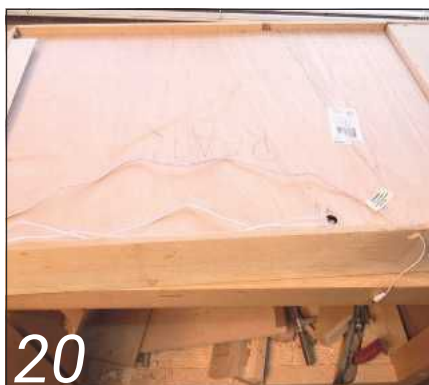
20 The final step for the carcass build is to screw the back panel to the cabinet
