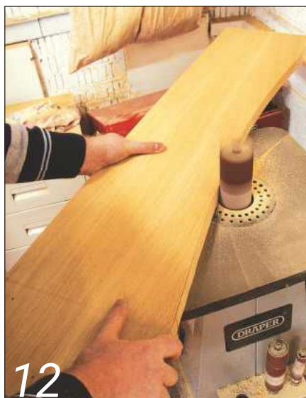
12 ... and then the bobbin sander was used with care; this looks simple but it's easy to dig in
