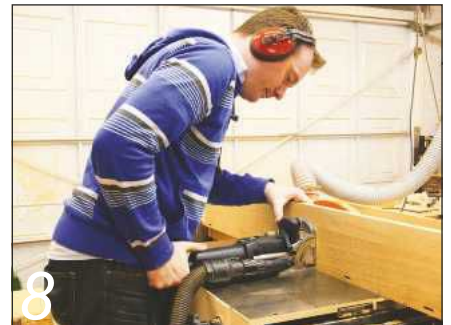
8 Cutting the mortises for the buttons, which will eventually hold the top
