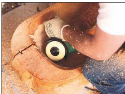
A firm grip is needed to control the grinder
