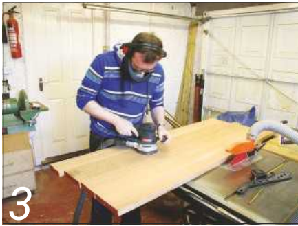
3 This enabled the components to be sanded quickly with a random orbital sander
