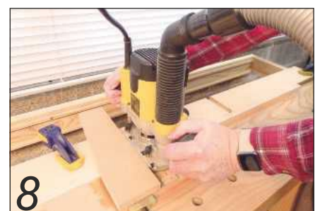
8 For the housings, I used a hand-held router with an 18mm straight cutter, run against a simple T-square guide
