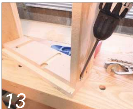
13 For assembling the joint, I find a scrap piece of MDF to brace against very useful
