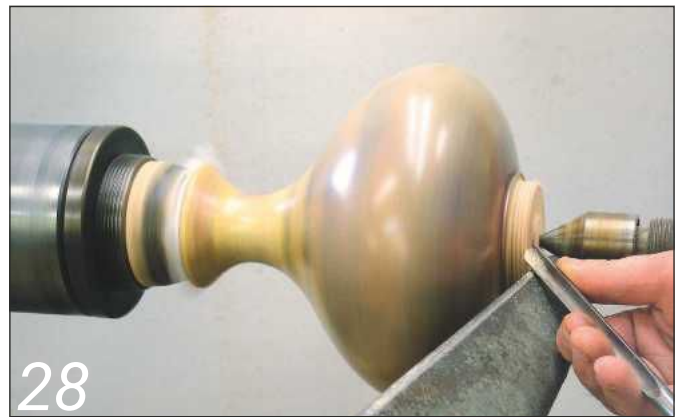
28 Reverse the piece onto a dolly and turn away the spigot
