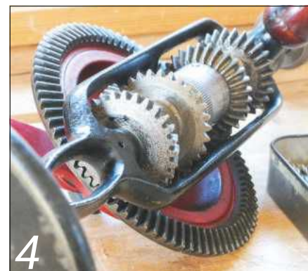
Four pinions flank the gearbox of the MF 97
