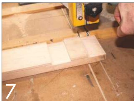
7 The foot is rebated on the radial arm saw
