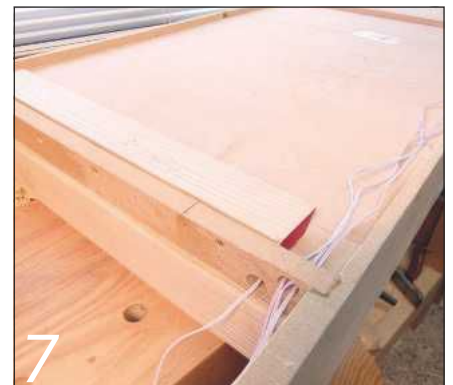
7 The top of the display section runs right to the back edge of the unit, providing a mounting for the French cleat
