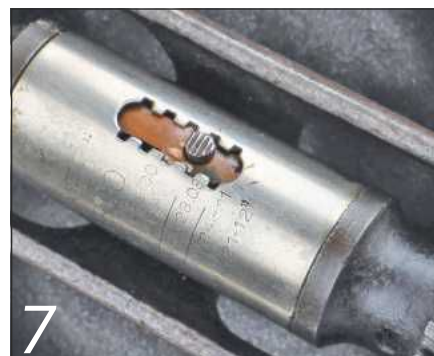
7 In-line gearbox of the Yankee 1530
