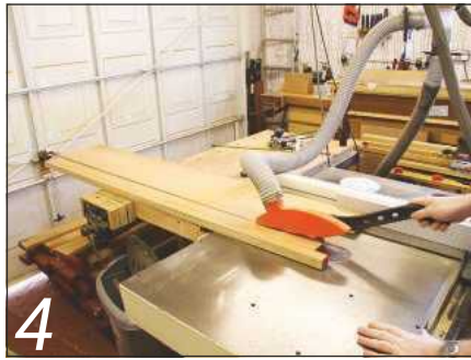
4 Again, ripping the parts to the correct width from one panel was a very quick task
