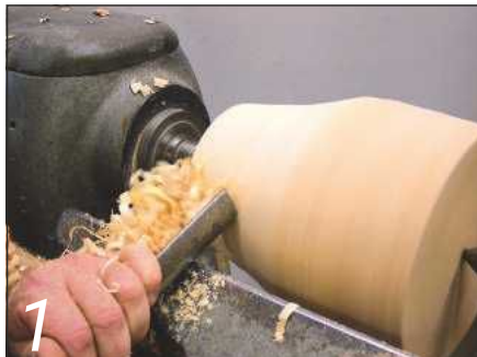
1 Turn your blank to a cylinder and start shaping
