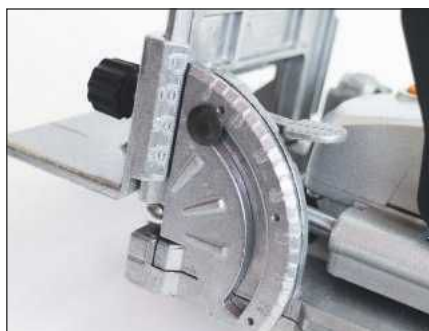
The supplementary fence fitted; note vertical scale
