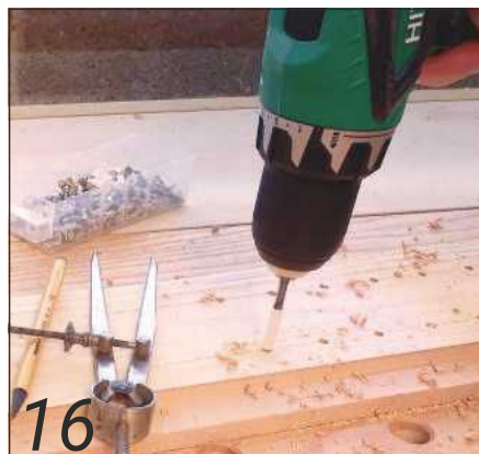
16 Drill the holes for the glass shelf supports in the display section
