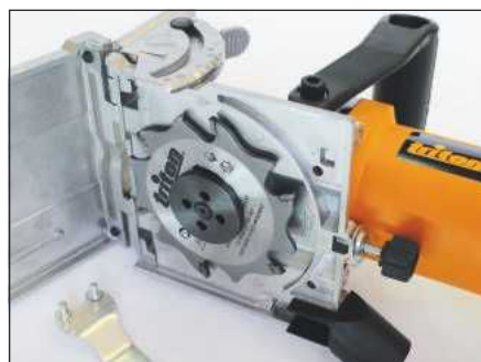
Easily accessible, the blade can be readily removed
