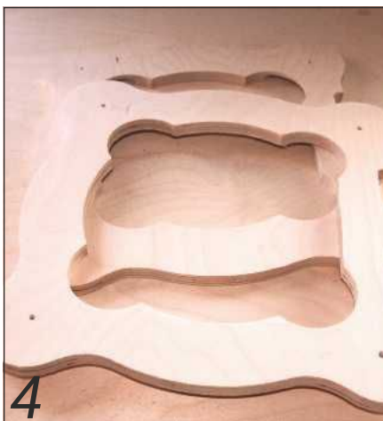
4 Two sections of the routed frame
