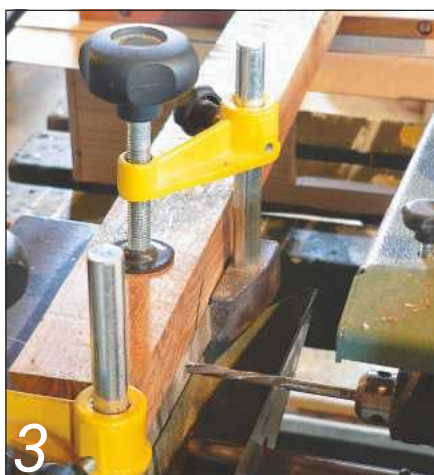
3 The slot mortiser cut the mortises for the 8mm loose tenons at the top of the posts
