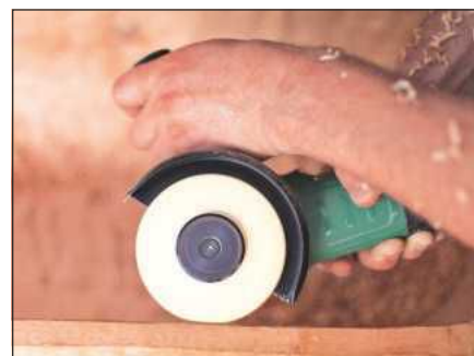
Shaping up to the vessel's rim
