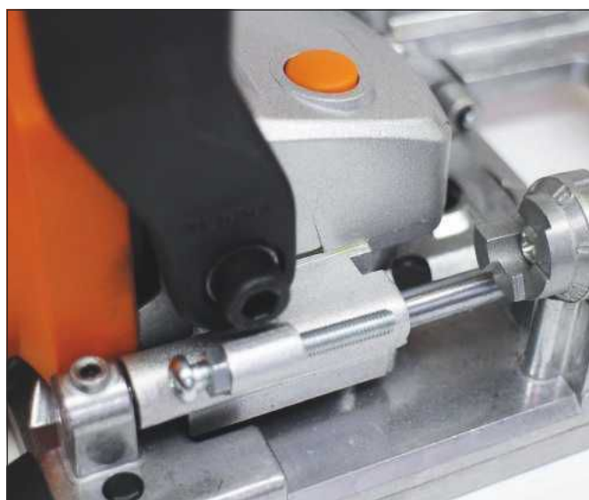
The turreted depth-setting adjustment
