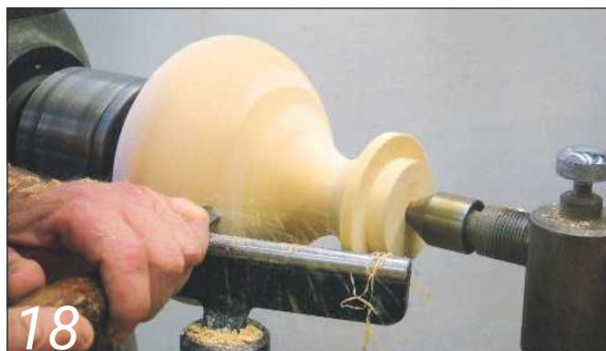
18 Do the final shaping of the outside using a spindle gouge....
