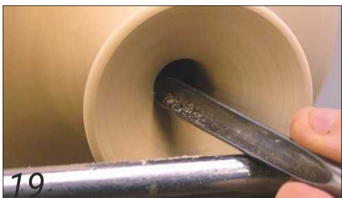
19 ... and carefully shape the inside neck, breaking through to the cavity
