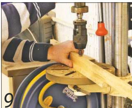
9 By countersinking for screws, replacing this part at a later date was made possible
