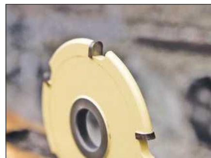
Detail of rounded profile tungsten tip
