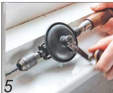
5 Ratchet action of the North Brothers Yankee 1530 is useful in tight spots
