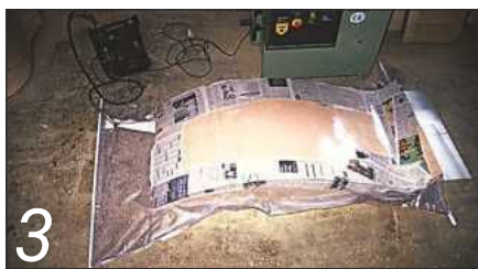
With glue applied, the boards can be positioned over the former and placed into the vacuum bag
