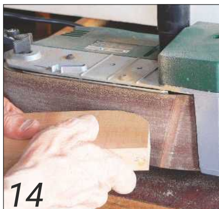
14 The table support ribs were shaped on the bandsaw, then on a belt sander clamped sideways to the bench
