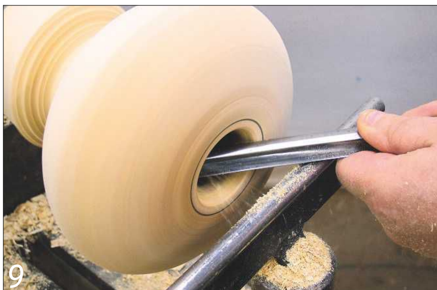
9 Use a bigger gouge to cut deeper into the cavity...
