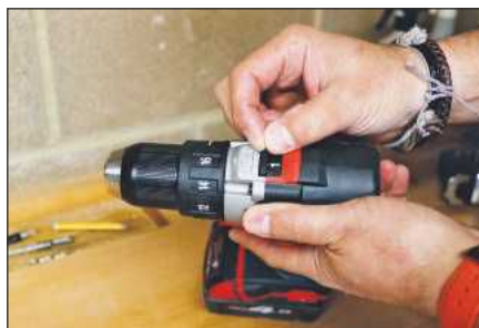
A top slider switches between the gears; max speed is nippy
