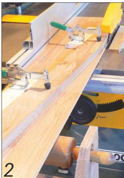
2 To cut the 9° angle at the top of the wing, I clamped it to another homemade sled
