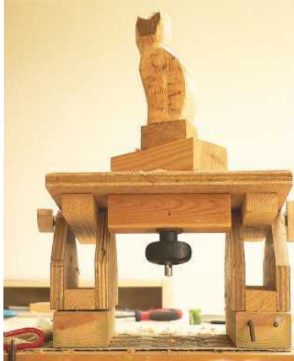
The original stand, which tilts but is clamped – at a fixed height – to the workbench
