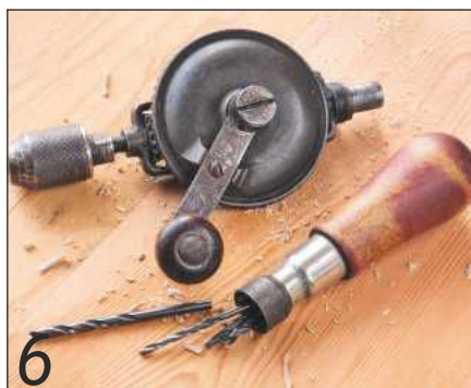
6 Drill bits housed in the Yankee 1530's detachable handle
