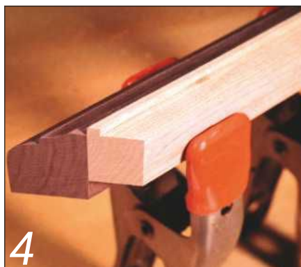
4 Face glue the two parts of the base together, making sure that the top of the rebate is lined up with the top of the walnut moulding
