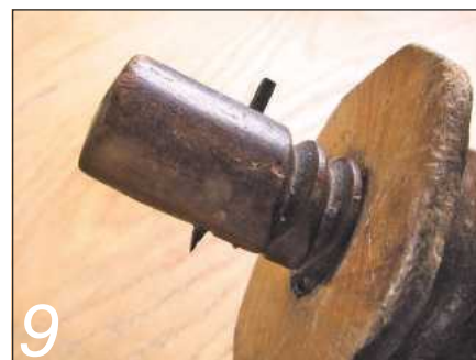
9 An example of a 19th-century marking gauge with threaded beam
