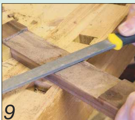
9 The neck slot was filed to ensure a good fit
