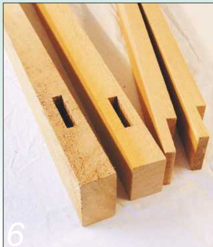
6 The mortise & tenon joints cut for the various frame pieces
