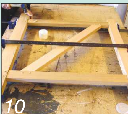
10 As you can see, each joint has two pegs driven into pre-drilled holes
