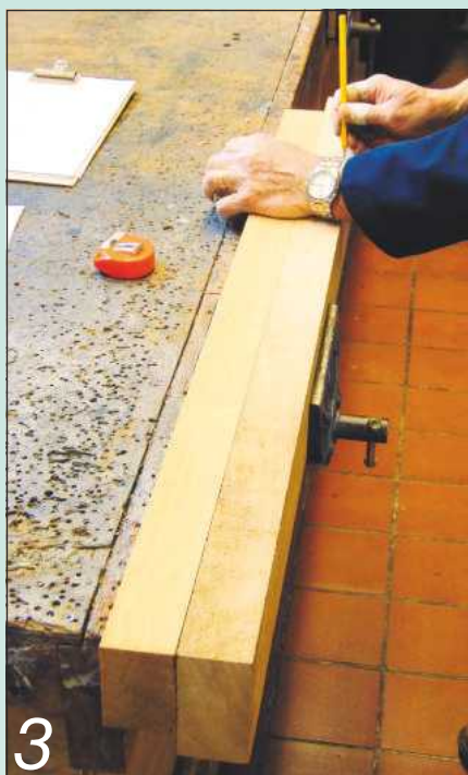
3 The two vertical stiles have their mortise positions marked out
