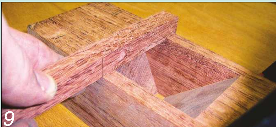
Clamp the plane together to mark the length of the cross pin
