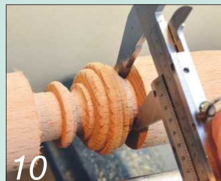
10 Stop frequently to check diameters
