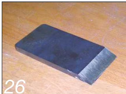
26 The primary bevel is ground on a bench grinder before heat treating
