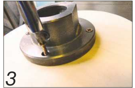
3 Screw the scrap plywood disc to a faceplate
