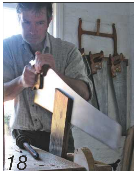
Both ends of the kerf can be inspected when it's standing vertical
