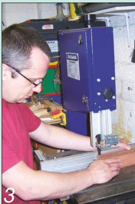
3 The bandsaw's minimal kerf helps retain the grain pattern on re-assembly...
