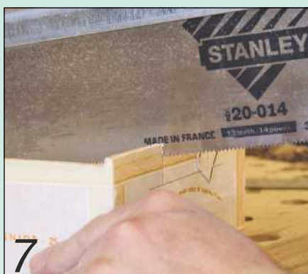
7 Sawing slots so the neck will fit into the box...
