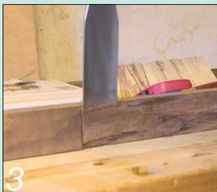
3 Chopping out the neck mortise to fit the cigar box (I managed to slip and cut into the good wood...)
