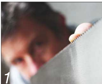
1 Checking the saw is straight and sharp
