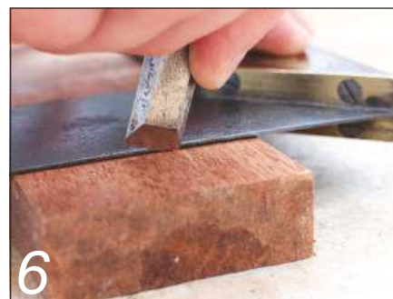
6 Using a chisel as a marking knife
