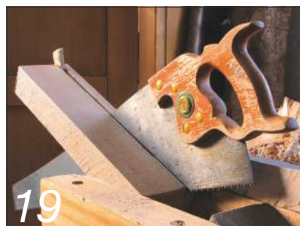
Timber tipped up in the vice makes for more comfortable sawing
