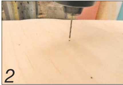
2 Mark and drill a disc of scrap plywood to attach to a faceplate, ready for the screws
