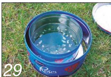
29 ... before quenching the blade in oil
