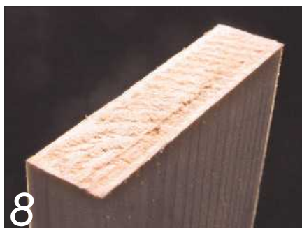
8 Clean all-round cut after marking with a knife
