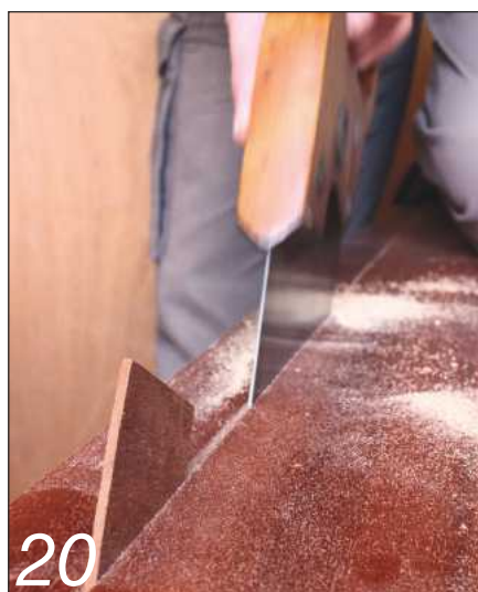
The kerf is wedged open with a sliver of timber to prevent binding
