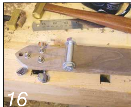
The 10mm bolt for a nut is shown in place, and will be held there by string pressure
