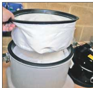
The third fine nylon-type mesh acts as the final filter
