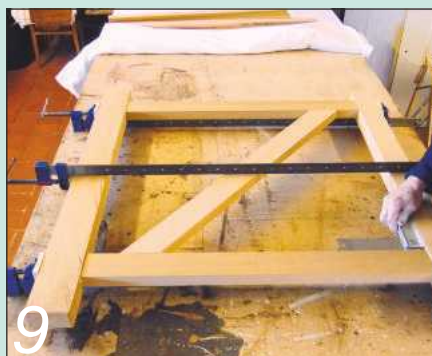
9 The gate frame is glued and cramped up and then checked for square
