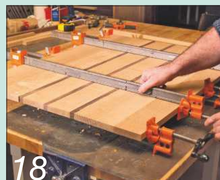
18 During clamping of the top, ensure to pay special attention to equalising the pressure from the top and the bottom
