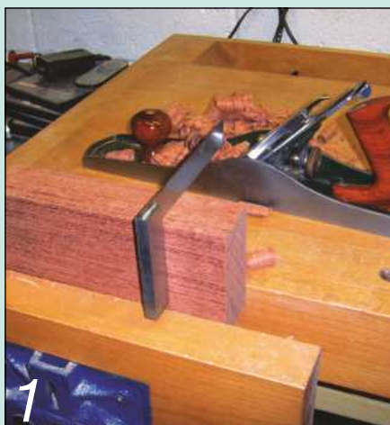
1 A side and a face of the blank need to be planed to give reference faces
