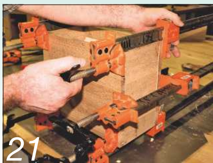
21 Glue and clamp the drawer together but allow the bottom to float without gluing
