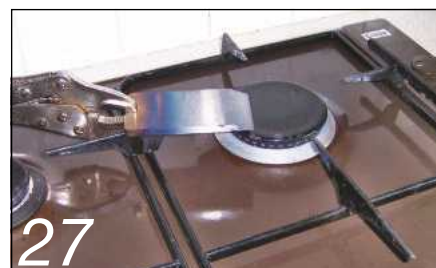
27 Pre-heat the blade to around 450°C on a gas ring...
