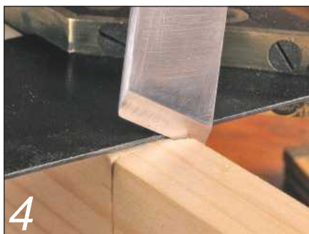
4 As you can see, the marking knife slots positively into its previous cut
