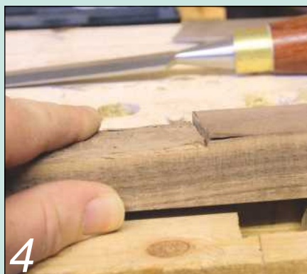
3 Chopping out the neck mortise to fit the cigar box (I managed to slip and cut into the good wood...)
