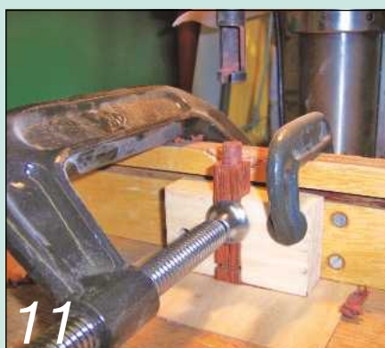
Cutting the round tenons on the drill press using a plug cutter
