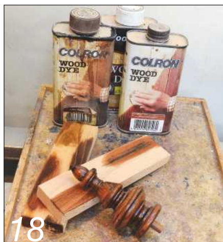
18 Mix until you achieve the correct colour and test on scrap wood
