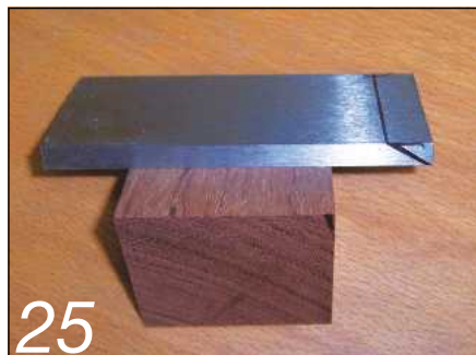
25 Mark the primary bevel before grinding – 30° in this case
