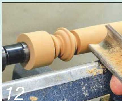
12 Reduce to the next required diameter with a spindle roughing gouge
