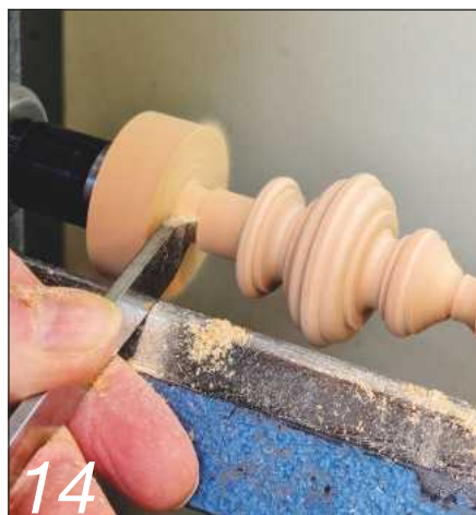
14 Reduce the spigot to the correct diameter...
