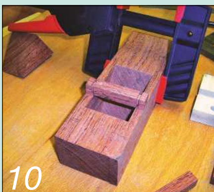
The shoulder cuts must align very accurately with the inside of the plane
