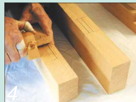
4 Gauge marks locate the mortise holes in the width
