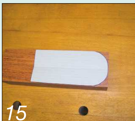
Transferring the curved shape to the plane from a cardboard template
