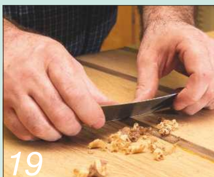
19 Once dry, remove the clamps and scrape the joints (top and bottom) with a well-sharpened card scraper
