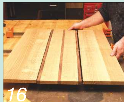
16 Once the panels for the top are ripped, lay them out to select the best appearance
