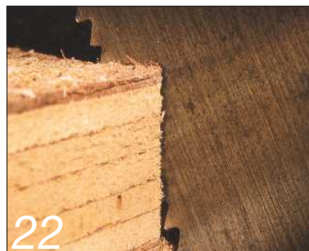
Sawing plywood on a sacrificial backing board
