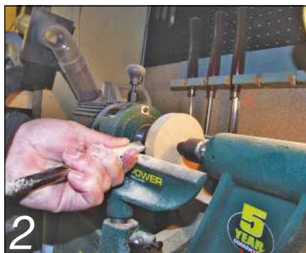
2 Turn the blanks to the circles you have scratched out, rolling the edges slightly
