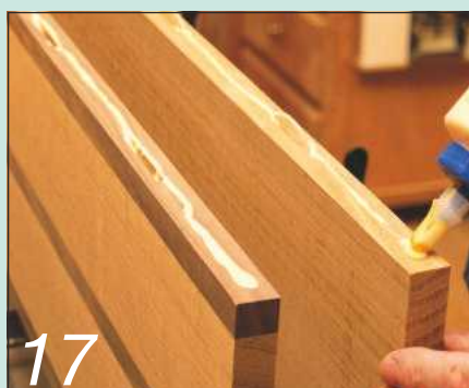
17 Mark the three panels for biscuits (or dowels) and then glue, biscuit and clamp them together
