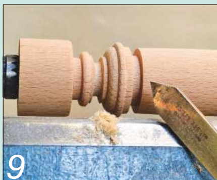
9 This narrow parting tool is just right for reducing fillets to size and as a scraper for small beads
