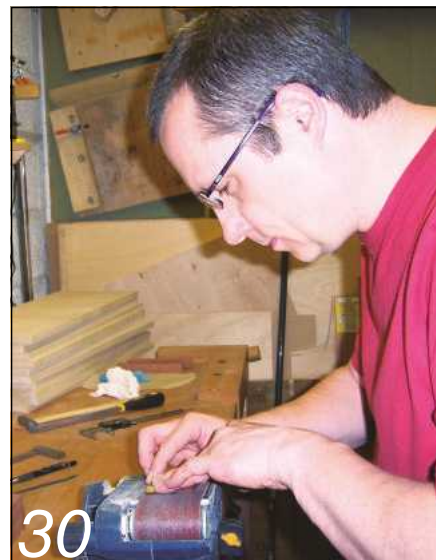
30 Clean up the blade on a slow-running belt sander
