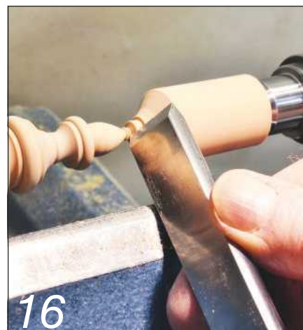
16 Hold the spigot in chuck jaws while completing the finial tip
