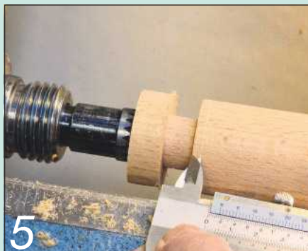
5 Vernier callipers are superb for these small measurements and mark the wood directly
