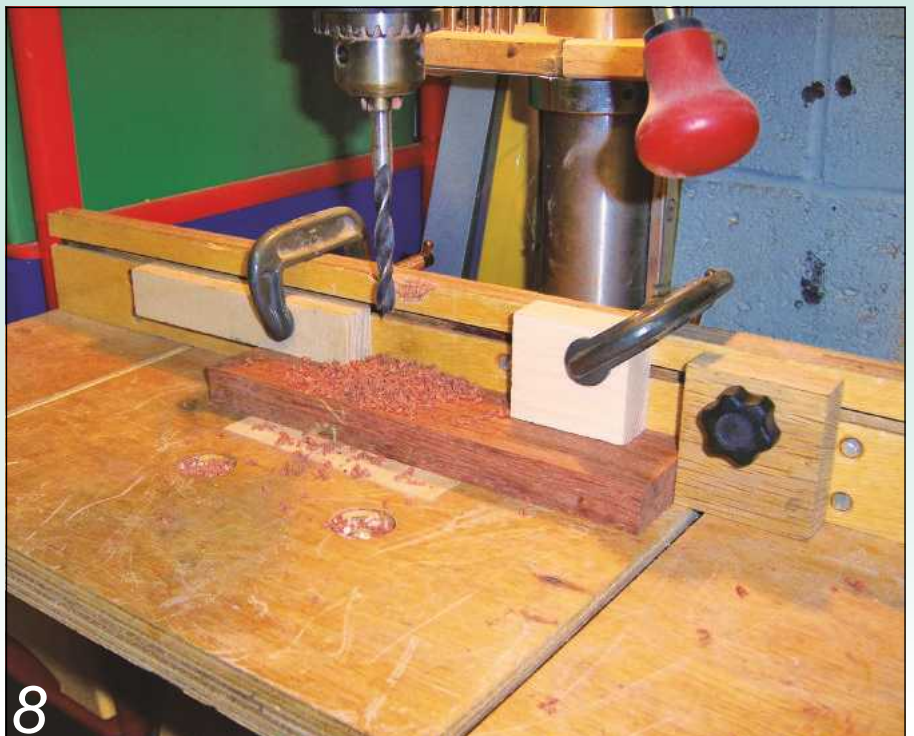
8 Clamp the side pieces together and drill the 6.25mm holes for the cross pin
