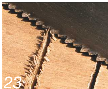
Plywood sawn with and without a backing board
