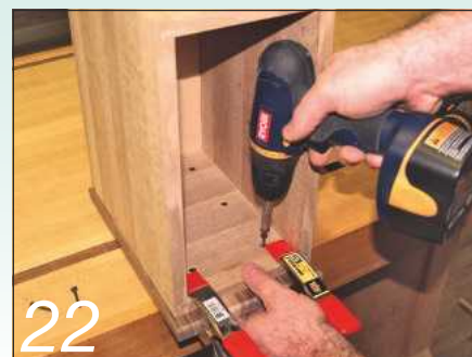
22 Screw the face to the drawer front using six 32mm screws driven into pre-drilled, countersunk pilot holes
