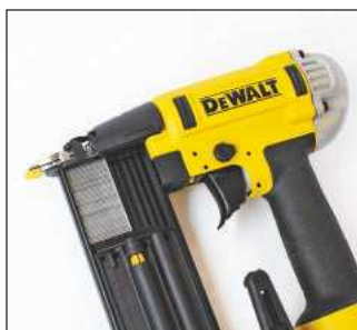
Magazine open, note yellow empty indicator and operation mode selector above trigger
