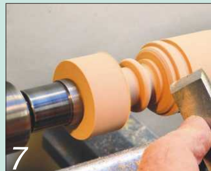
7 I gave up on the skew chisel and scraped the beads round instead
