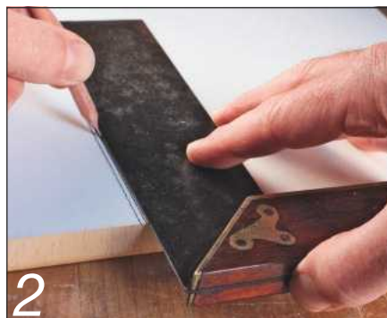
2 Testing the try square is a true right angle
