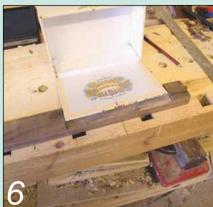
6 The slot I created had to be measured against the lid width for accuracy
