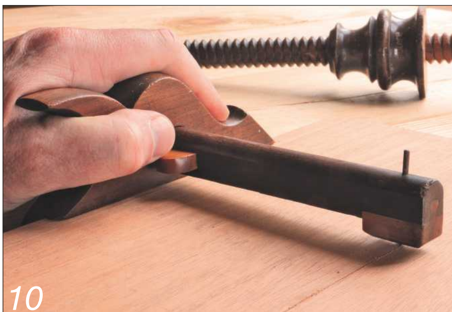
10 The panel gauge scribes far from the edge of a board
