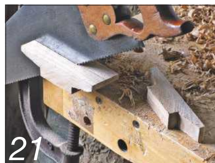
Odd shapes call for improvised clamping while making cleats
