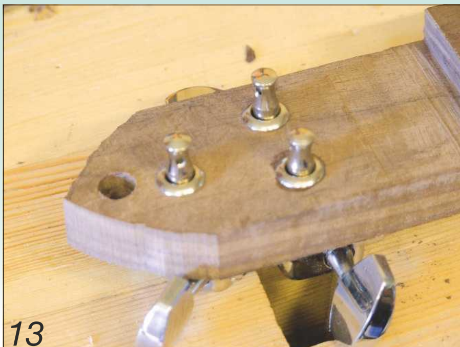
13 The machine heads are shown now in place, positioned so that the strings would not overlap or make contact with each other
