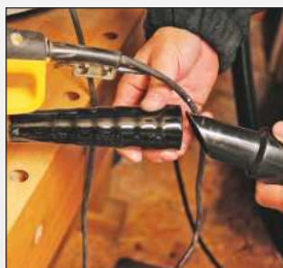
A simple tapered adaptor is supplied for power tools
