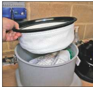
A second thick felt-like filter seals the drum
