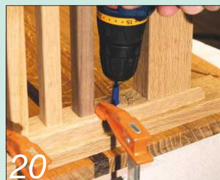
20 Extend the pilot holes into the desktop using a 1.5mm bit, again stopping the bit with masking tape to avoid drilling clear through the top
