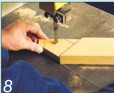
8 The brace tenons are finished on the bandsaw
