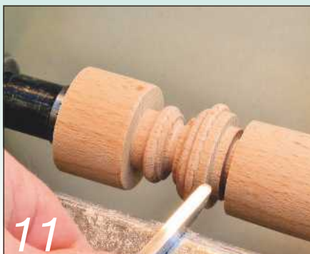
11 This home-made scraper is 3mm wide and 5mm deep for extra strength
