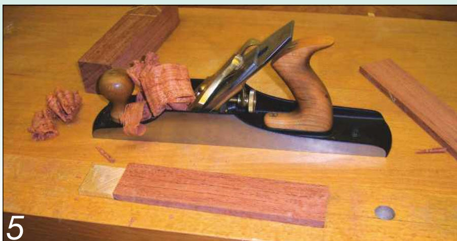
5 The cheek pieces were hand planed flat to ensure a thin glue-line upon re-assembly
