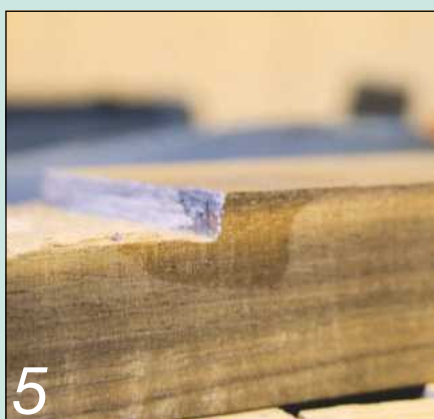
5 I executed an invisible repair using epoxy
