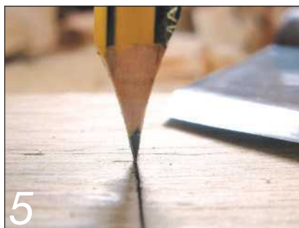
5 Using a sharp pencil to improve the visibility of a knifed line
