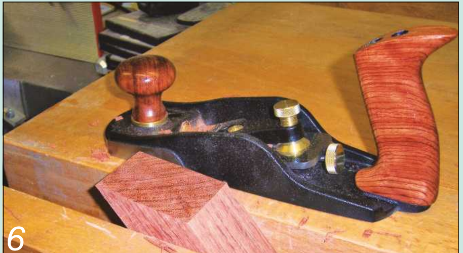
6 It is a good idea to clean up the angled faces to ensure a good bed for the blade
