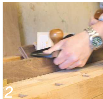
2 Planing the neck. It's vitally important that the neck should be flat and smooth to allow for the use of a slide
