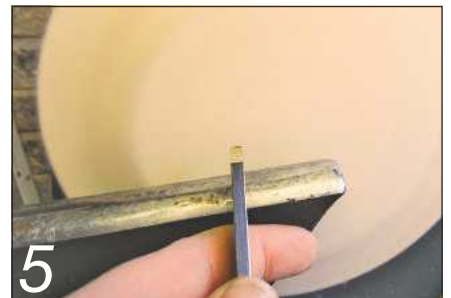
5 Using your 10mm parting tool, part a groove, the outer edge being 22.5mm from the centre of the piece
