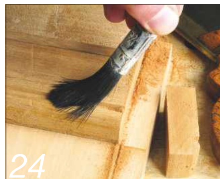
Brushing away the dust is safer than blowing it
