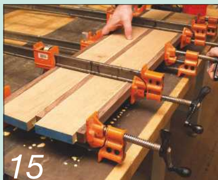
15 Glue and clamp the middle sub panel together, again leaving all five components as thick as possible until the glue cures
