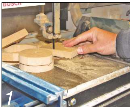
1 Scribe 75mm diameter circles on the MDF and bandsaw roughly to size
