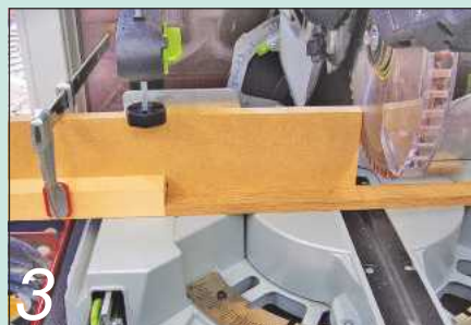
3 I cut the pieces to length using a chop saw, a sacrificial fence reducing tear-out
