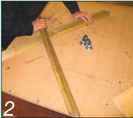
2 The next step is to mark out the halving joints for the cross over legs
