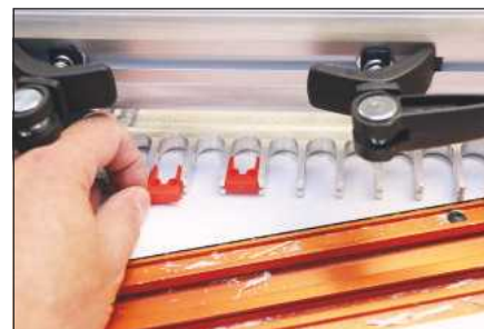
The red pegs slide into the comb for setting different tail spacings
