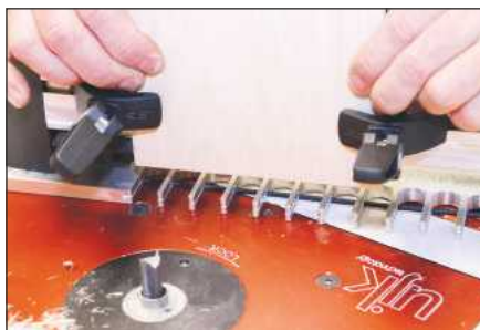
The black rod acts as a stop to limit the depth of cut on joints using thinner stock
