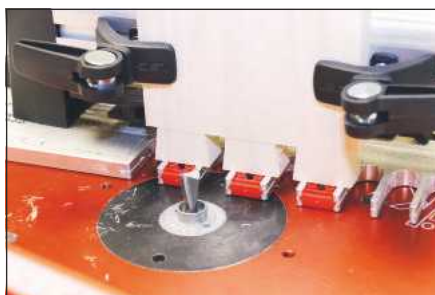
The pegs prevent the guidebush from making a cut
