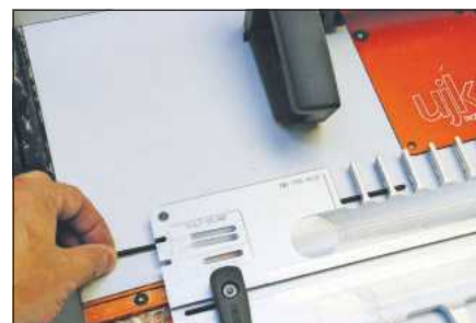
This black rod slides into a channel on the jig
