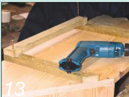
13 The handle, on the opposite ends to the castors, is a simple cross batten
