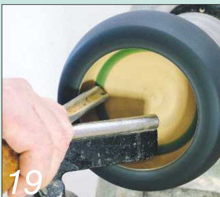
19 Swing the handle through about 100° while cutting the area coloured in green
