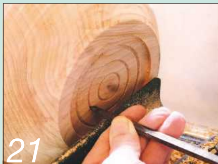
21 ... to form the recess for the dovetail chuck
