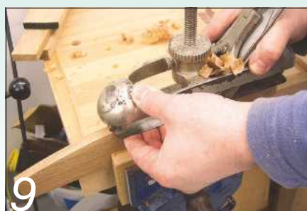
9 I cut the waste for the arch with the bandsaw and formed the arch shape with a compass plane
