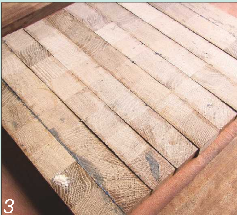
The chequerboard pattern of the slices lines up neatly, but the faces and edges need further work
