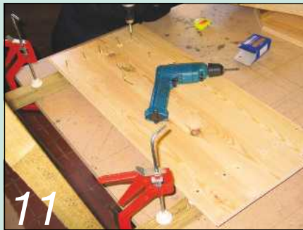
11 The ends can now be fixed directly to the sides
