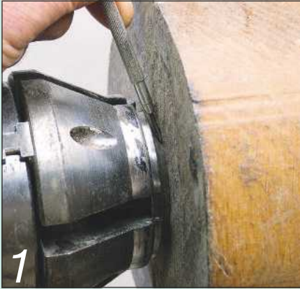
1 Make sure the blank sits firmly against the screw chuck
