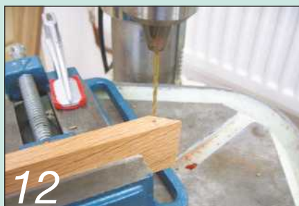
12 I drilled a hole through the support fractionally larger than the rod...
