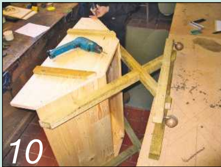
10 Position the leg assemblies on the bench, clamp them down and fix on the side boards
