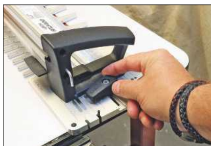
The top frame locks to the comb with the aid of these latches
