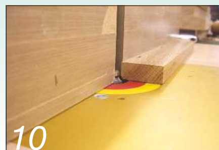
10 The bottom rail had a pencil radius cut on it, so the rounded corner would sit on the work surface
