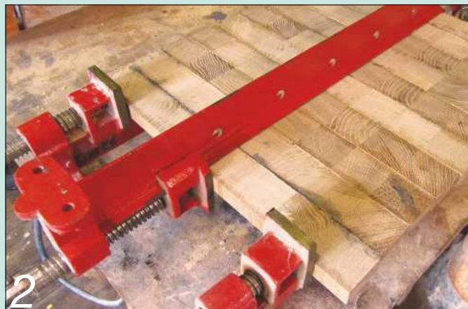
A clamp on top keeps the slices flat for glue-up. Waterproof PVA removes the need for any joints
