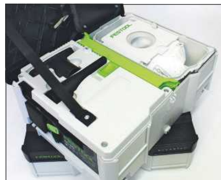
Inside the vacuum box; note tool housings and filter and bag unit...
