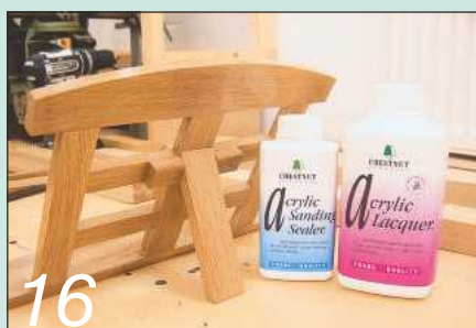
16 Finally, the stand was given a coat of Chestnut acrylic sealer and three coats of acrylic lacquer
