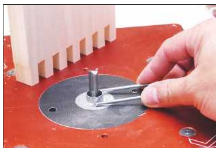
By moving the guidebush in small increments the fit of the joint can be adjusted
