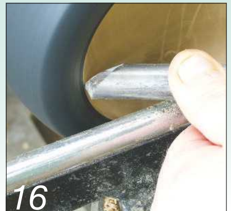
16 To increase the steepness of the cut the bevel needs to point in this direction
