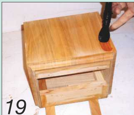
The first two coats of polish are applied using a polisher's mop
