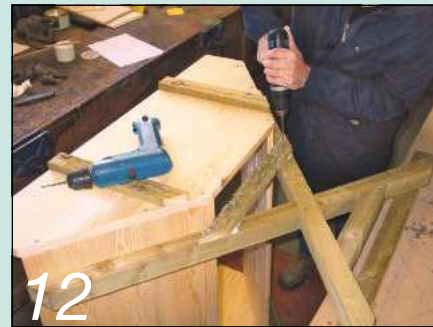
12 A pair of secondary braces are fitted underneath to support the bottom boards
