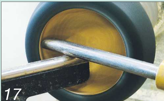
17 Keep the tool on its side to cut down the wall
