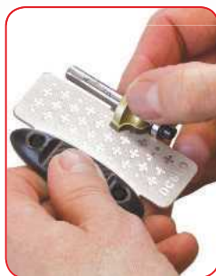
Specialist stone designed for router cutter sharpening.
