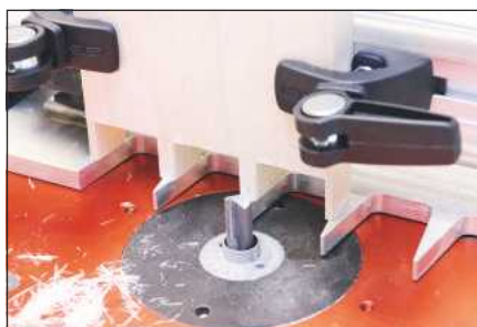
It makes a finer pin profile on through dovetails
