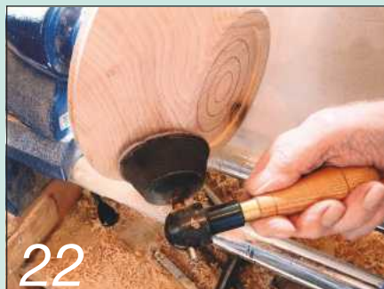
22 Using the free spinning disc sander on the outside of the bowl
