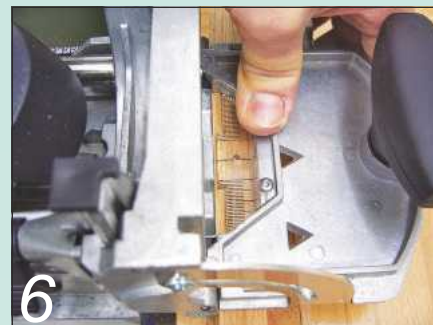
6 With the slots cut in the central components, the mid-rails were dry-fitted to the verticals...
