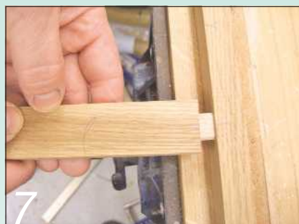
7 ... and the positions for the Dominoes on the top and bottom pieces marked and cut
