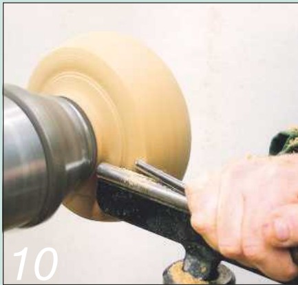
10 Cut the rim using a small gouge on its side
