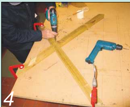
4 The legs are cramped directly to the drawing board before gluing and screwing
