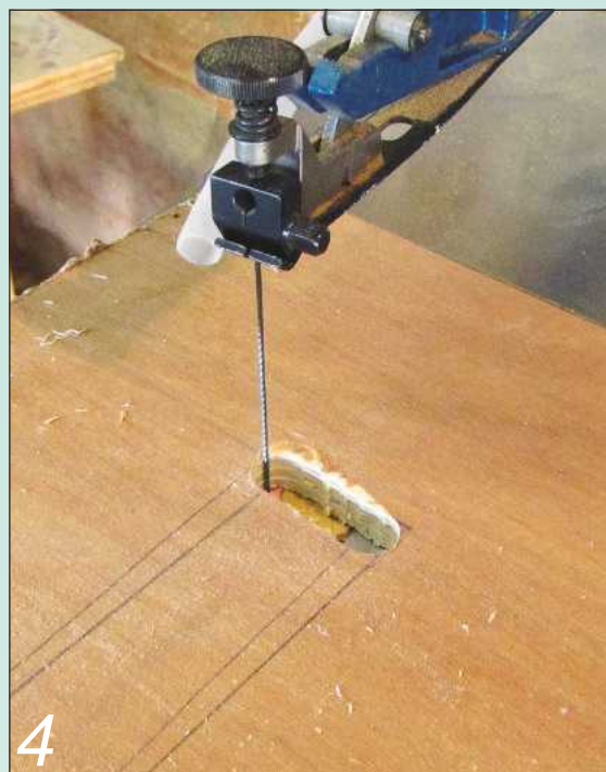
Creating a slot for a moving router is one way to flatten a face that's too big to go through a thicknesser
