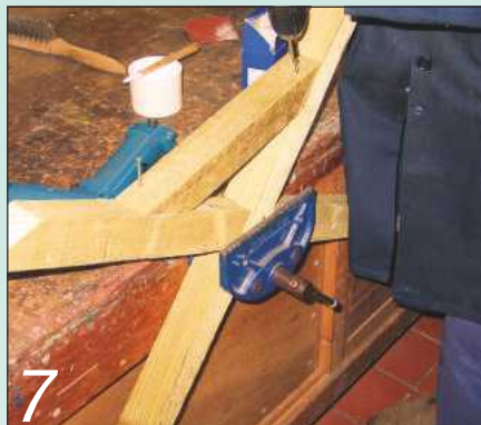
7 At the other end a brace is then glued and screwed on
