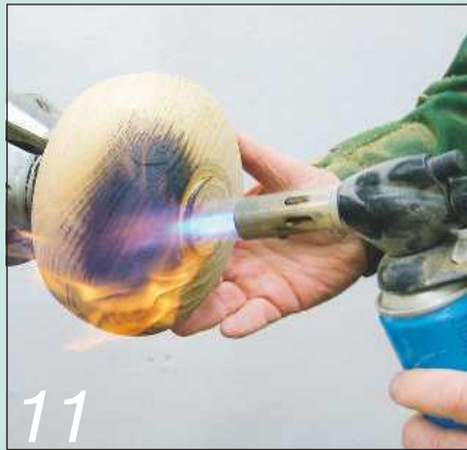
11 Heavily scorch the outside with a blowtorch...
