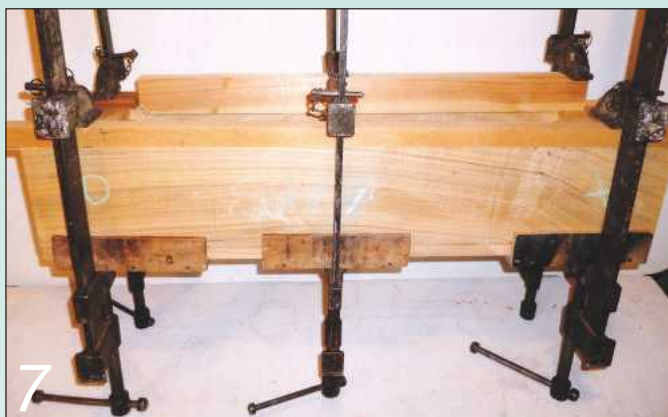
Cramped up and left to dry
