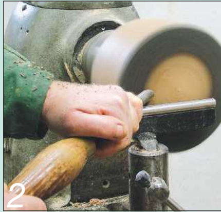
2 Use a pull cut to flatten the base...
