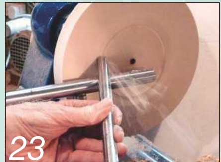
23 The hollowing is carried out with a bowl gouge
