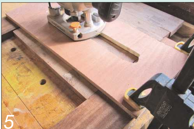
Sweeping a router across the faces – with the plywood and blocks holding it at a constant height – gets rid of most of the unevenness
