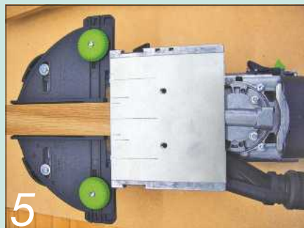
5 The small components that needed slots in their end-grain were securely held in place with the auxiliary fence
