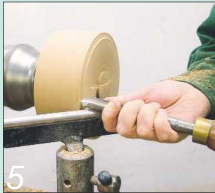
5 Begin shaping from the bottom corner...
