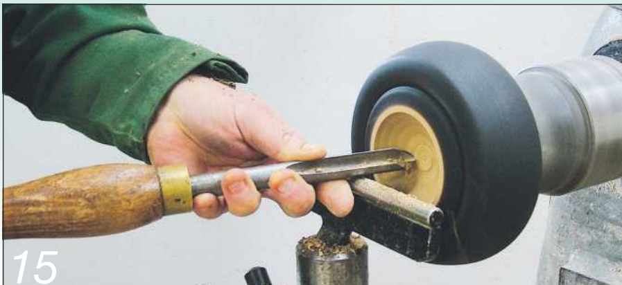
15 ... gently swing the hand to this position as you cut down the inside wall
