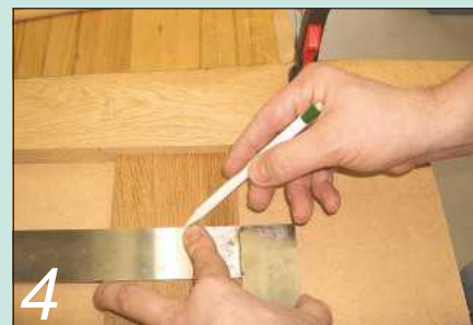
4 The centres of the middle rails were marked on the verticals, to get the positions for the Dominoes
