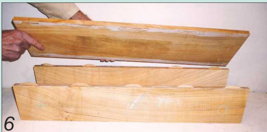
Glue applied and biscuits inserted
