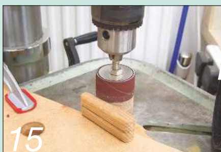
15 The two fingers that hold the pages in place were made from further pieces of the mid-rail
