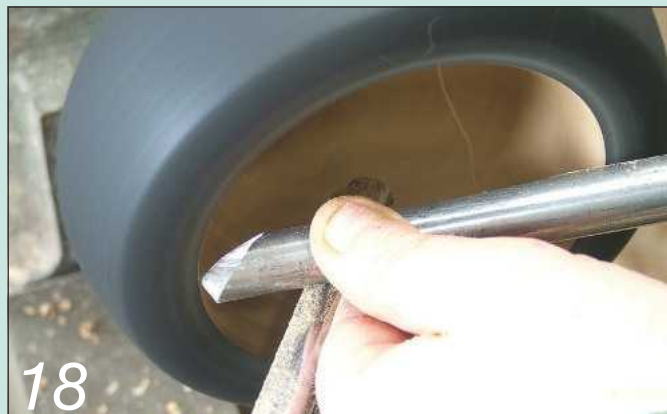
18 To undercut, the bevel needs to point under the rim
