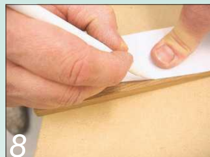
8 Using the paper template, I marked the shape of the top rail onto the timber
