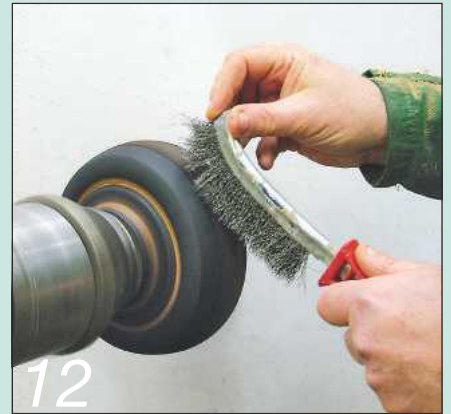
12 ... then brush off the resulting carbon with a stiff wire brush
