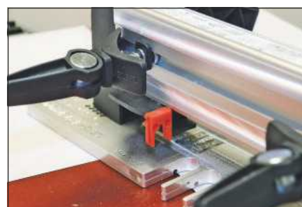
This small red peg sets the correct offset for comb joints
