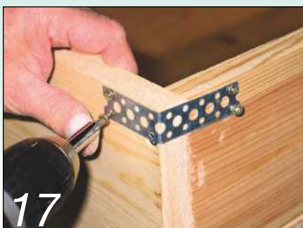
17 To add strength to the corners some masonry ties are moulded and screwed on
