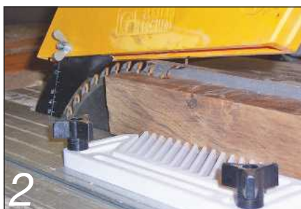
2 Set the fence to 25mm and cut the bevel forming the front slope. Use a pushstick!
