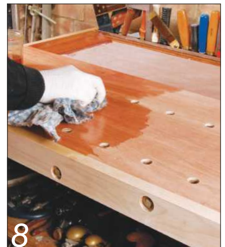
8 A couple of coats of an oil/varnish mixture gives adequate protection
