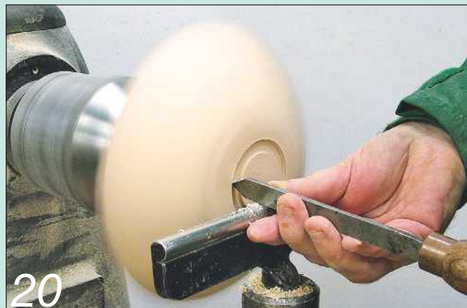
20 When all three sides are done, cut a chucking recess in the base of the bowl
