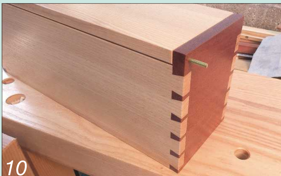
10 Some over-long pivot rods are useful here
