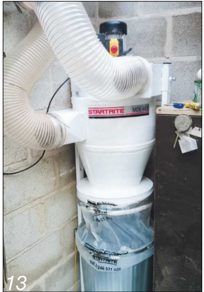
The new extraction system in situ and doing a great job of keeping the workshop dust-free
