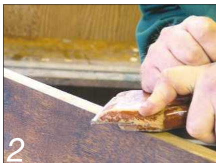
2 I used a paint scraper to remove the old glue
