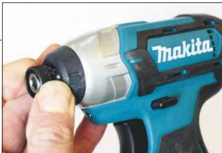
The sprung collar makes for quick bit changes
