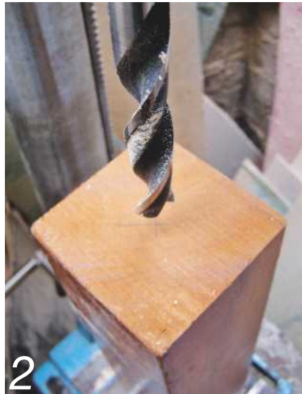
2 Mark the centre of the blank, hold it in a vice and drill a 16mm diameter hole
