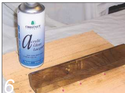
6 Complete the finishing process, burnishing as necessary
