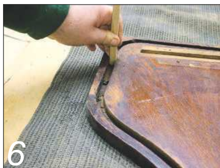
6 I used a scrap of wood to remove the grime from the channels...
