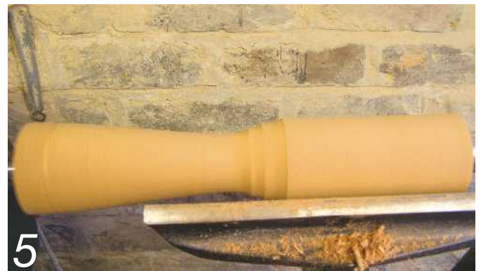
5 Start the lathe at 162rpm and begin rounding the blank using your spindle roughing gouge
