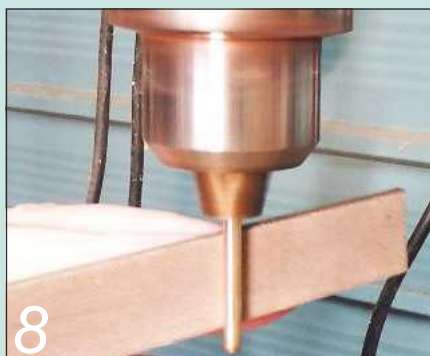
8 The pivot rod may need to be reduced slightly – I find a drill press and a file good for this
