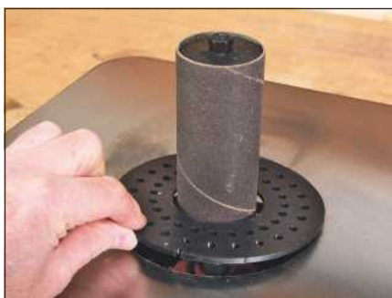
... and an insert fits the table recess
