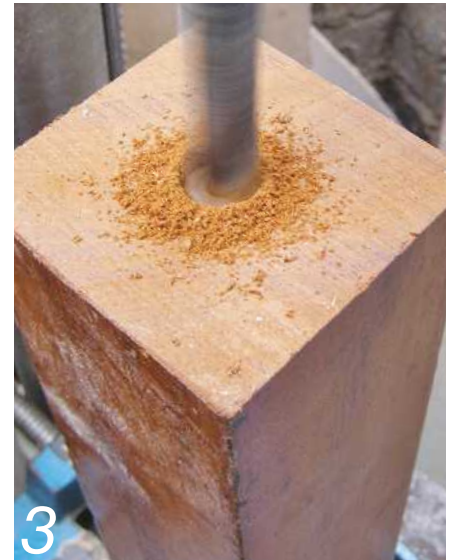
3 Drill 30-50mm deep; make sure the handle of the vice touches the pillar drill's neck
