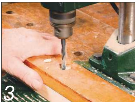
3 Using the old lippings as templates for drilling the new bolt holes
