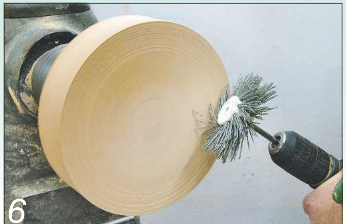
6 Clean up the textured area with an abrasive flap wheel
