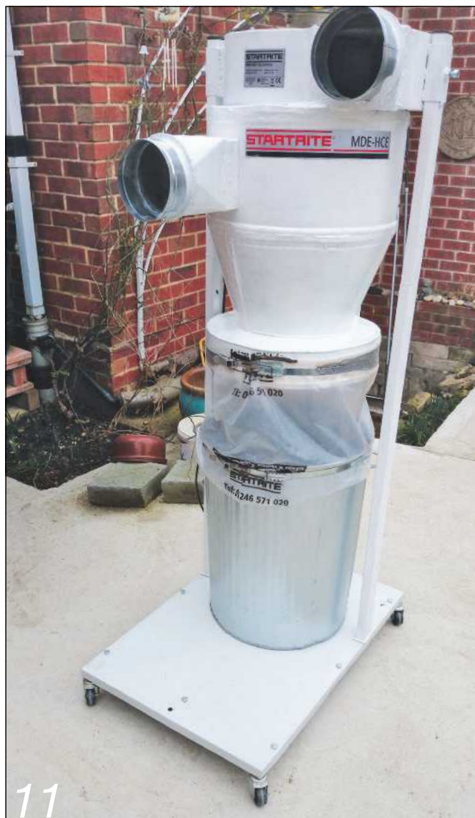
The waste bin attached using bungee straps
