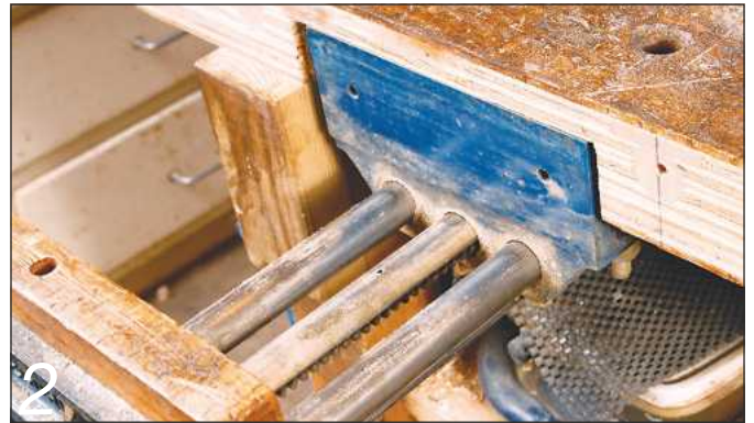
2 The vices are rebated into the top before fitting the lippings
