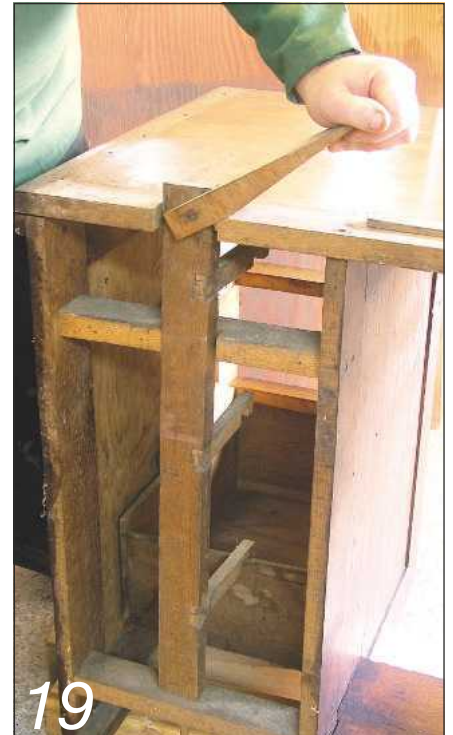
19 This photo shows the simple drawer locking mechanism...
