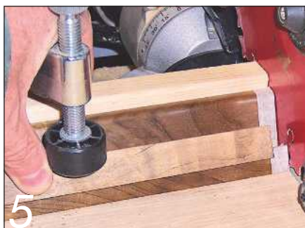
5 Trim the assembly at 80° to create the base and then cut the final 10° back slope
