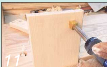
11 I marked my 'brand' on the underside of the lid using a hot iron – wear gloves as it's just too easy to unthinkingly touch the hot parts
