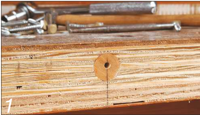
1 Beech plugs give a firm fixing for the edge lippings
