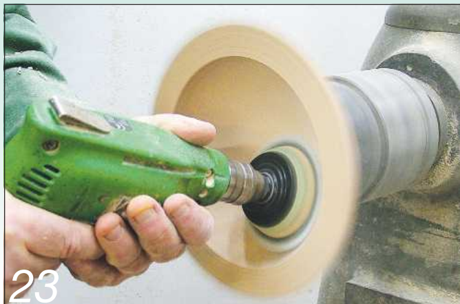
23 ... before power sanding to a finish and then oiling the bowl
