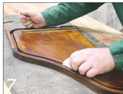
7 ... then waxed them to allow the tambour to slide more easily
