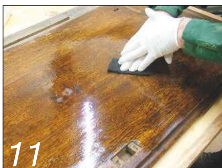
11 The desk top was cleaned with a boiled linseed oil and turpentine mixture
