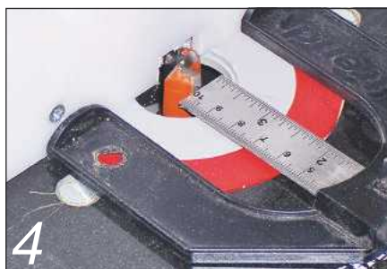
4 ... and rout a groove 5mm deep and 10.5mm wide, as shown
