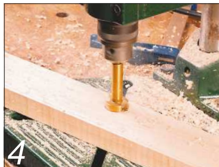
4 Counterboring the holes for the heads of the coach bolts
