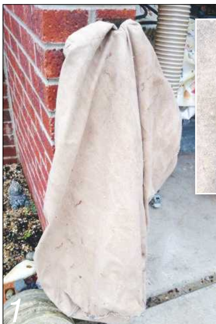
1 After use, I found that the cloth bag had become fibrous, and clogged up as a result
