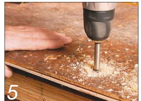
5 Again, the old top can be used as a template for the bench dog holes
