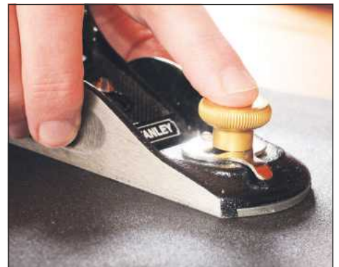
Robin Gates working the sole of his Stanley 9½ plane on WD40-soaked wet or dry abrasive paper
