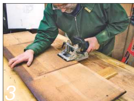
3 Biscuits helped strengthen and align this joint
