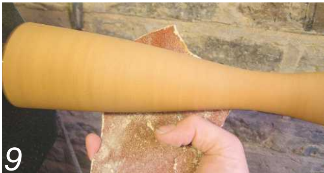
9 Finally, use 80 grit abrasive and 180-400 Wet and Dry to finish
