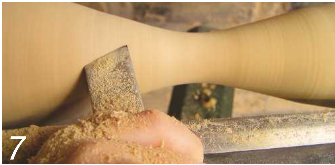
7 Using the skew chisel or the edge of the spindle roughing gouge...
