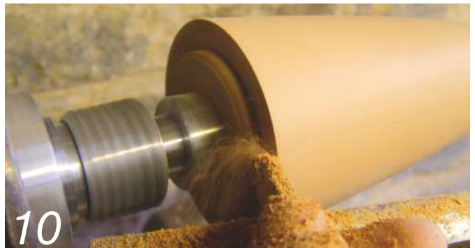
10 Turn the lathe down to part the base off the candlestick
