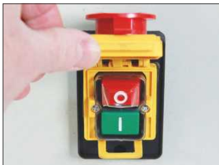
The shielded NVR switch
