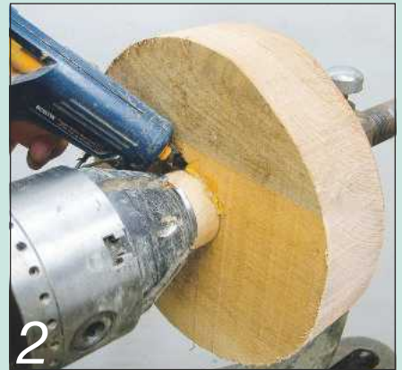
2 Hot-melt glue the spigot block to the bottom of the bowl
