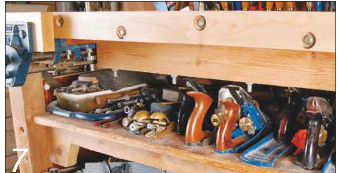
7 Bolting bracing beams under the top prevents it from sagging
