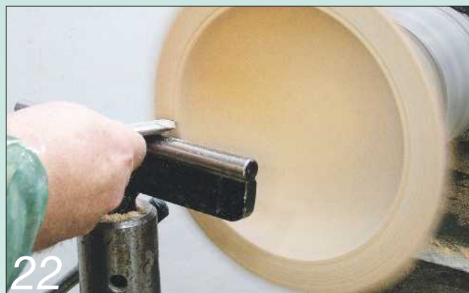
22 I cut a decorative bead using a skew chisel on its side...
