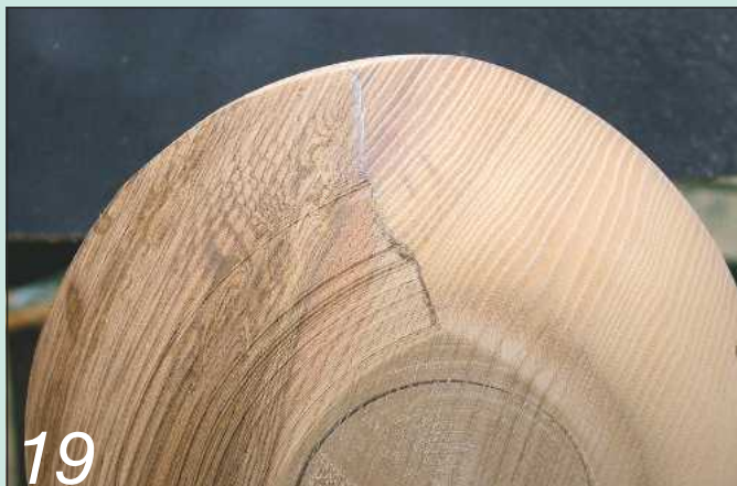
19 More wood needs to be taken away from the left of the pencil mark
