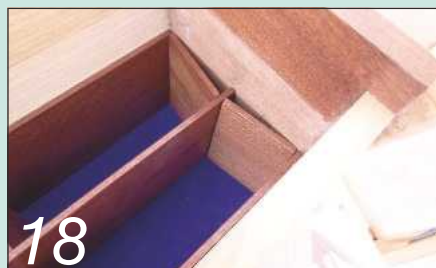
The lower trims come next – apply a dab of glue on the back of those short ones and push them firmly into place
