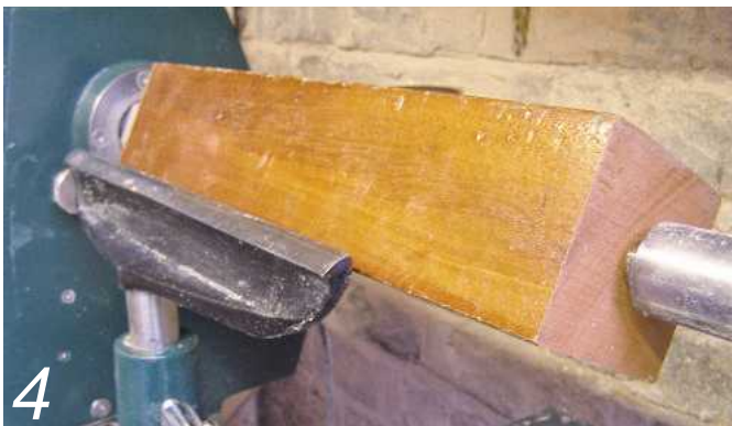
4 Mount the blank between centres on your lathe. A revolving centre will typically fit inside a 16mm hole
