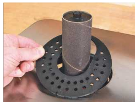
There is a slotted insert for table tilting
