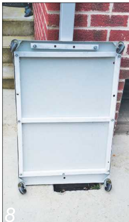
The frame strengthened the areas under the extractor supports
