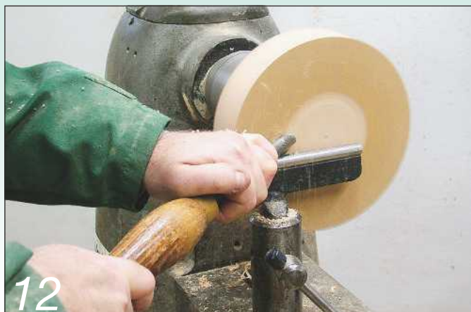
12 Mount the piece on the true centre and true up the blank's face
