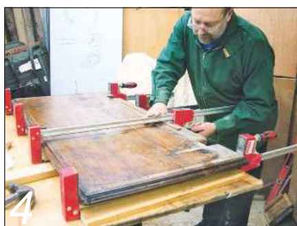
4 The repaired top glued and cramped
