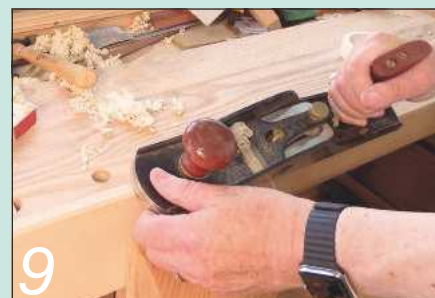
9 The lid's rear lower edge needs to be relieved to let the lid open. Begin by chamfering at 45° and then form a quadrant – test frequently as it may need less removed than you think
