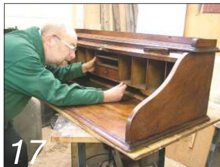
17 ... then the pigeon holes were reinstalled...
