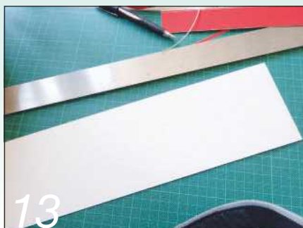
13 The card backing for the lining is best cut with a straightedge and scalpel on a cutting board
