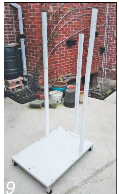
Lengthening the support arms to allow room for the collection bin
