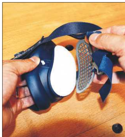
Once released, the grille hinges back out of the way to gain access to the filter
