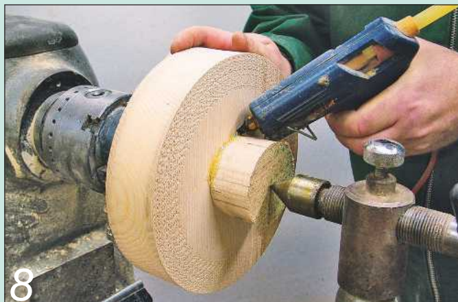
8 Hot-melt glue the second scrap to the top of the bowl and true it up
