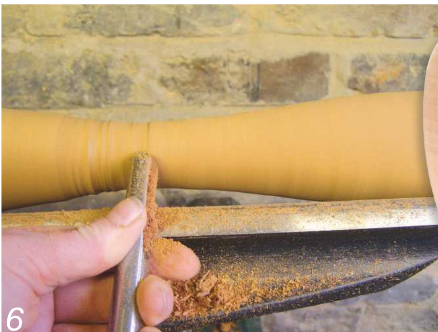
6 Use the spindle gouge to create beads or a symmetrical dip in the middle section of the timber
