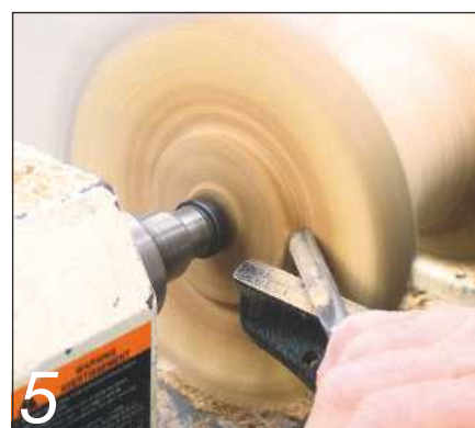
5 Cut a spigot to fit your chuck
