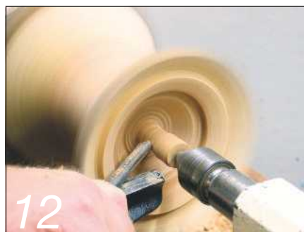
12 ...and continue to hollow the piece below it
