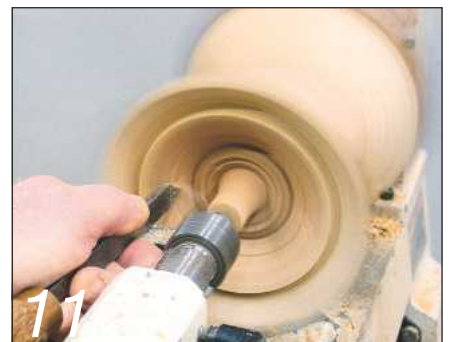
11 Cut a chucking recess at this end...
