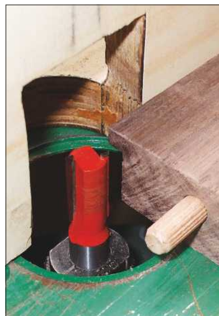
Cutting the rebates for the box bottom on my router table
