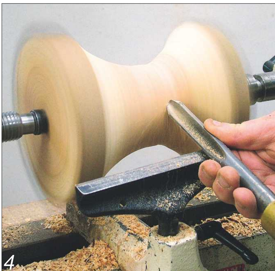
4 Turn a cove in the log, keeping the natural-edge at both ends
