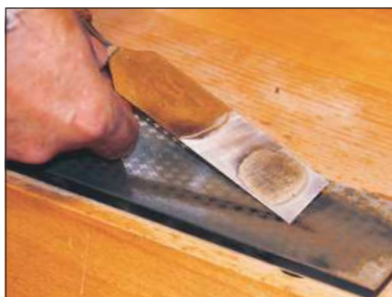
The bench stone proved flat when tested with this pre-flattened chisel
