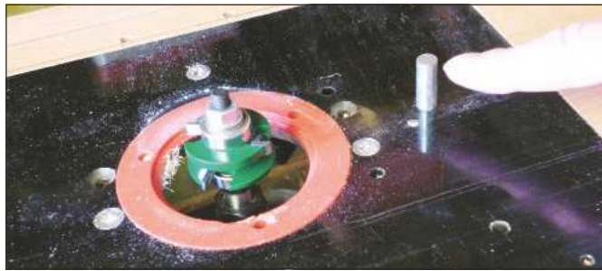
5 A lead-in pin is essential for curved work
