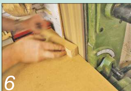
6 The profile was cut out on the bandsaw – not the best tool to cut the straights, really
