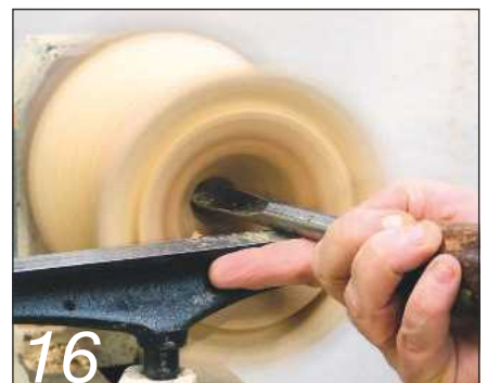
16 Widen the hole with a spindle gouge working from the smallest diameter to the larger
