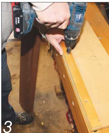
3 A second kicker batten is fixed lengthways down the jig
