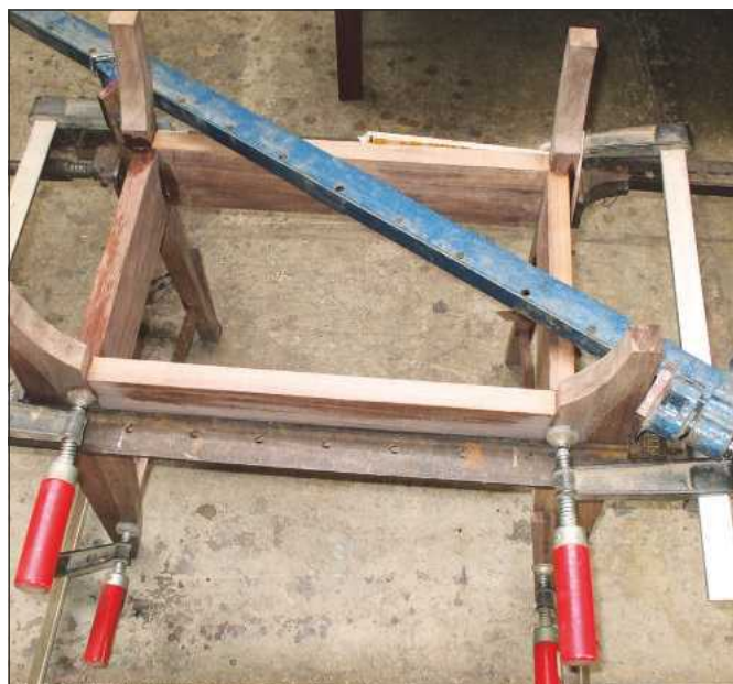
The diagonal clamp helps to keep things square
