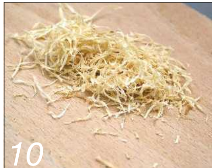
10 You should be getting fine spiral shavings at this stage
