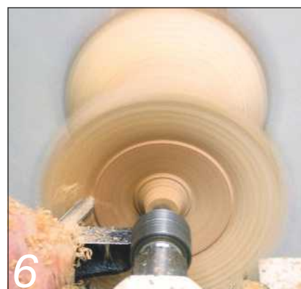
6 Mount the piece on the spigot and start to hollow at the tailstock end
