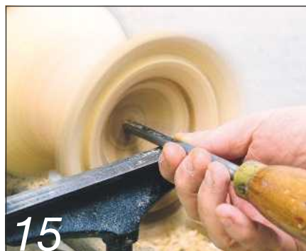
15 Use a spindle gouge to drill a hole right through the piece
