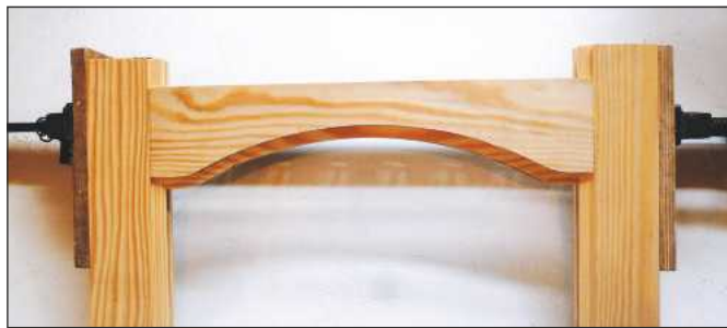
7 Scribing and profiling completed
