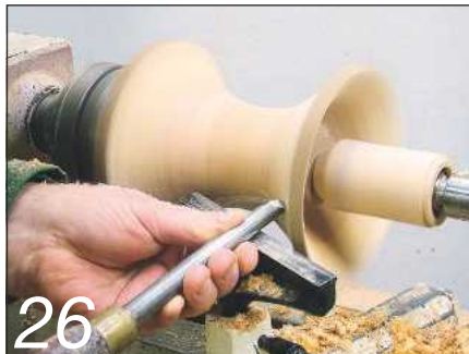
26 Refine the outside shape with a bowl gouge
