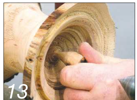
13 Turn the stub down and then twist it off by hand
