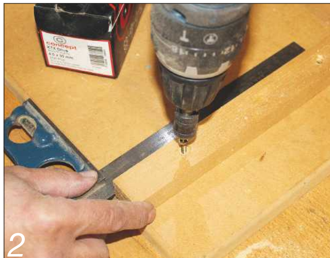
2 The jig is made by firstly screwing a batten squarely to act as a hook
