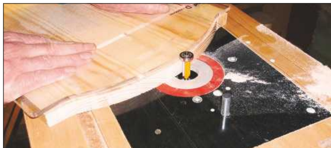
9 The sawn edge of the panel is smoothed using a plain cutter guided by the template
