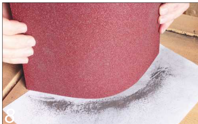
8 Tapping the sheet to remove swarf and spent grit
