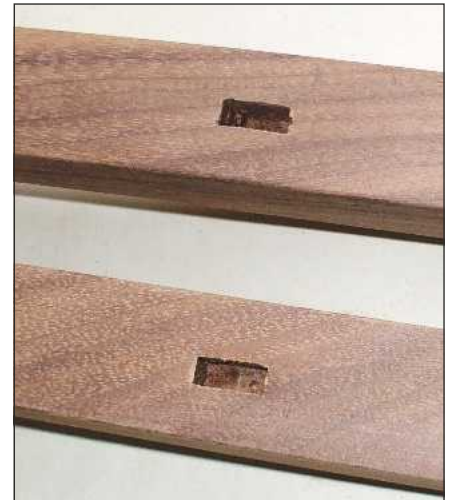
The mortises in the back legs, cleaned up prior to assembly
