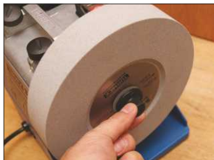
The EzyLock nut makes it easy to strip down the Tormek for stone swaps or maintenance
