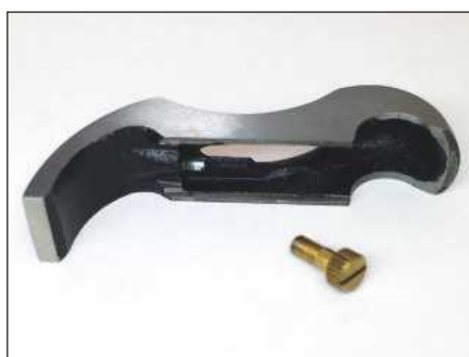
The adjustment screw ensures correct replacement of the upper body
