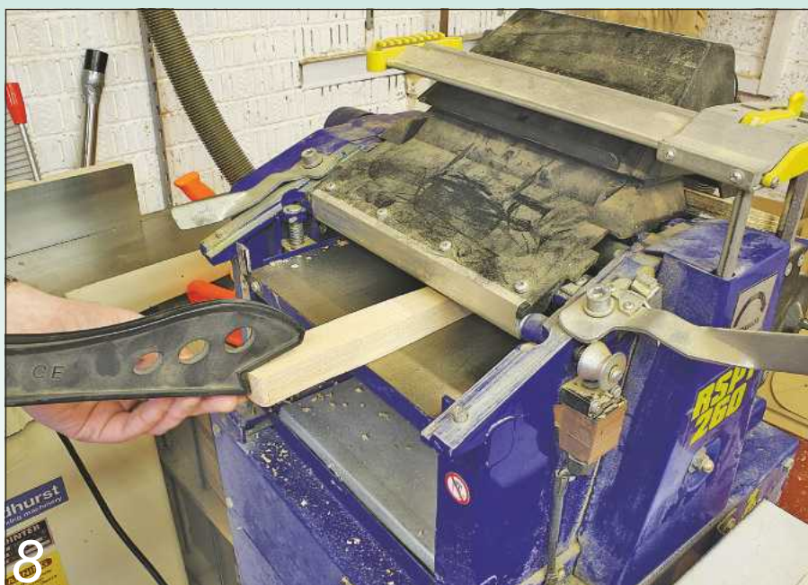
8 It's not usually wise to thickness once the profile is cut. Fortunately there was no breakout
