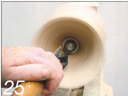
25 Turn away the last chucking point and blend in the curve
