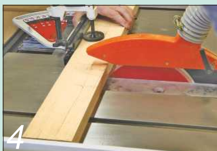
4 Continue down the sizes, reducing the platens as required until you have a full set of plugs
