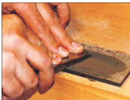
Smaller credit card hones work well for touching up router cutters
