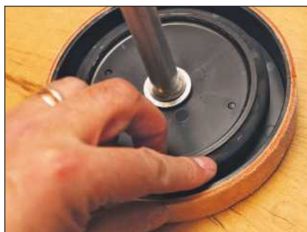
The roughened pin drives both wheels and rests against a rubber wheel for grip to drive
