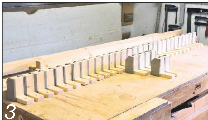
I used 2x1 softwood and offcuts of the screen MDF to make the shoes. The parts were simply glued and pinned together
