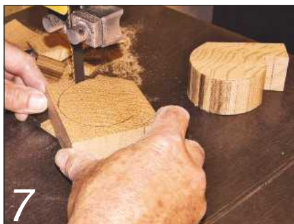
7 The curly bits are roughed out on the bandsaw
