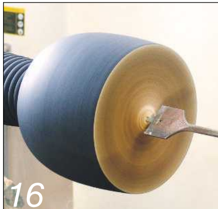
16 Mount the piece in your chuck and drill a hole in the top
