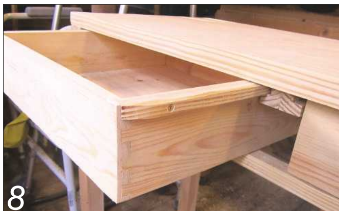
8 A thin offcut glued and screwed to the lip of the drawer fits easily into the L-shaped hanger, and holds the drawer just clear of the rail below
