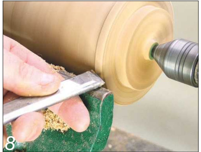
8 ...or, if you prefer, a skew chisel held on its side
