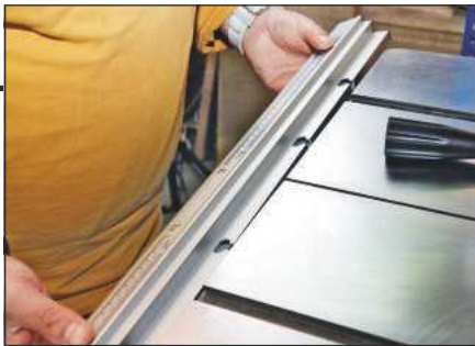
The fence rail removes easily for blade swapping
