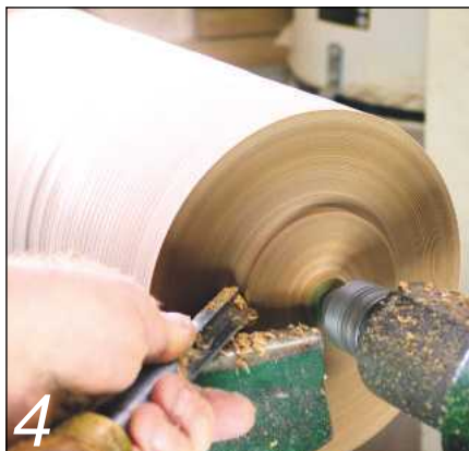
4 Cut the chucking spigot for your chuck
