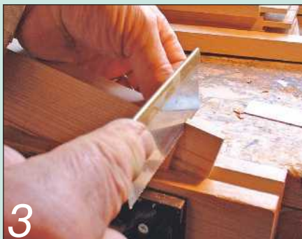
3 Cutting the angled haunch on the top rail's tenon using a fine-toothed gent's saw. This hides the end of the haunch
