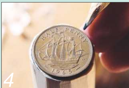
4 An old halfpenny makes a 25mm template for the shank
