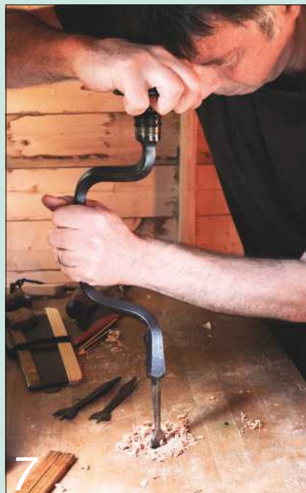
Boring holes in the bench for the holdfast shank, using the Scotch iron brace
