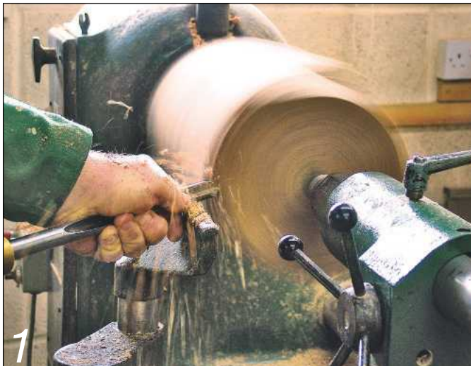
1 Mount the blank between centres and convert it to a cylinder
