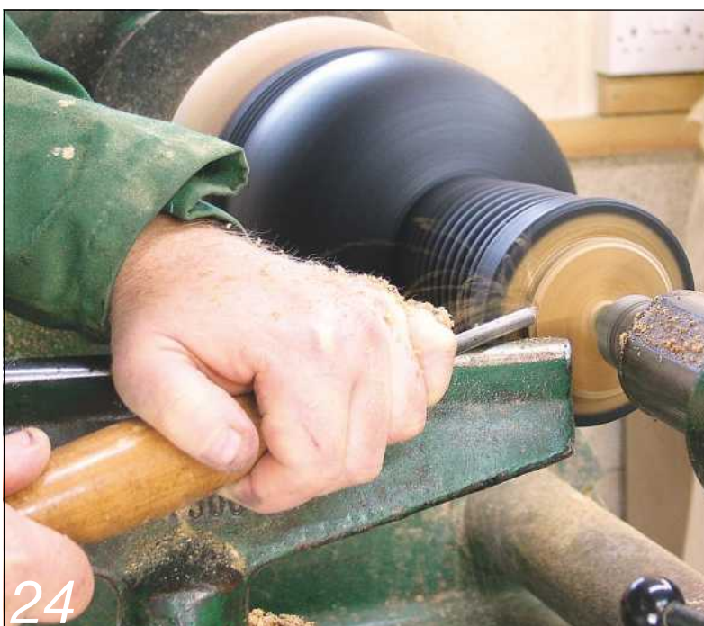
Finally, reverse chuck the piece onto a dolly to remove the chucking spigot
