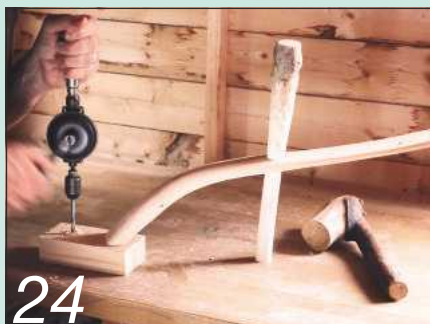
24 The two-part ash and hawthorn holdfast clamps work for drilling
