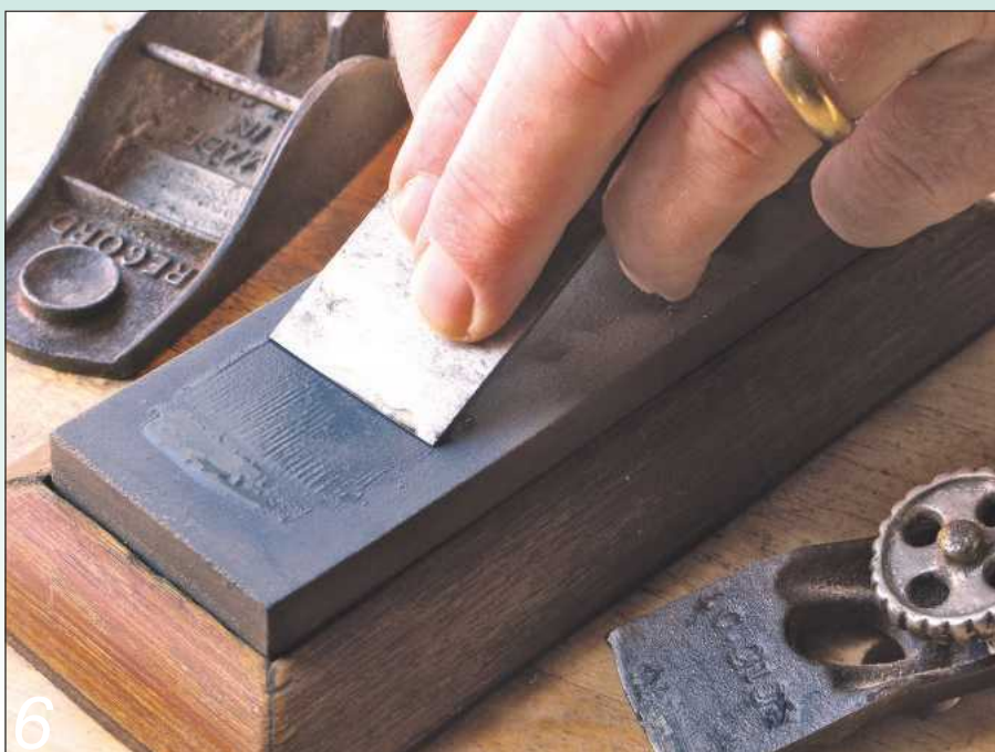
6 Sharpening the 102's blade
