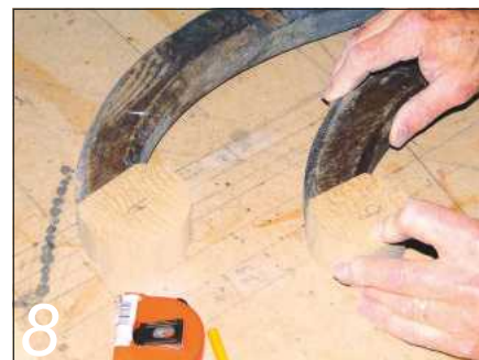
8 Checking for fit – they were both different thicknesses
