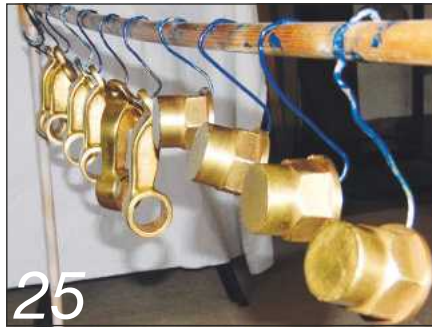
25 Once the brass has been finally cleaned up, each piece was sealed with spray lacquer
