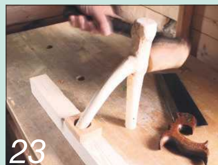
23 Releasing the natural hook holdfast with a tap on the back of the shank
