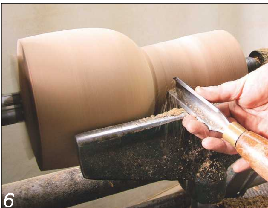
6 ...followed by the spindle roughing gouge
