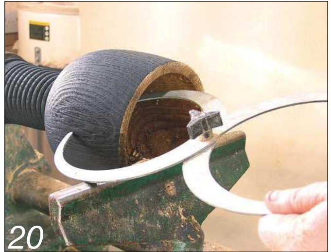
Regularly check for an even wall thickness
