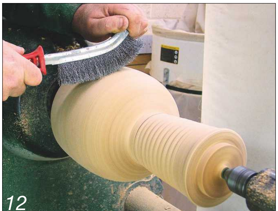
12 ...and a stiff wire brush picks out the softer fibres in the grain
