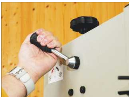
A tensioning lever allows fast blade swaps
