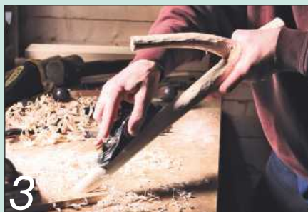
3 Shaping with a block plane leaves one hand free to hold the work
