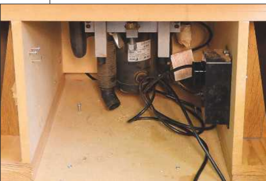
The electric router is much more manageable when up-ended under a table
