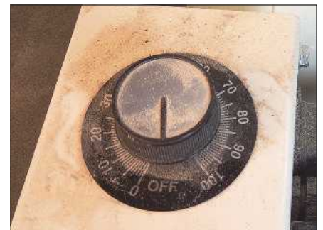
... but the belt is separately controlled from the variable-speed dial
