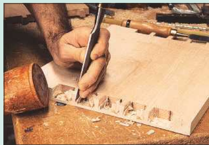
11 Use a wider straight chisel to pare the pins down to the knife marks
