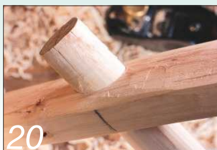
Start of test fitting while shaving the ash shank to fit the 25mm hole in the beak
