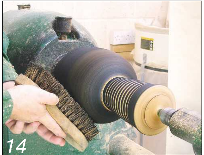
14 Use a scrubbing brush to remove the excess carbon
