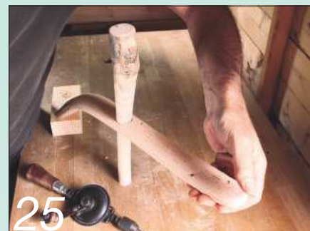
25 The two-part holdfast is released by pulling upwards on the rear extension
