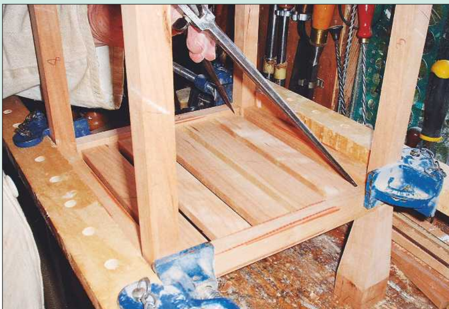
5 The mitres on the tenons must be cut very accurately, an important skill
