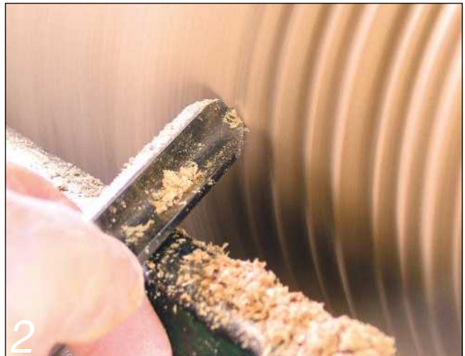
2 Use the swept-back bowl gouge to make chopping cuts...
