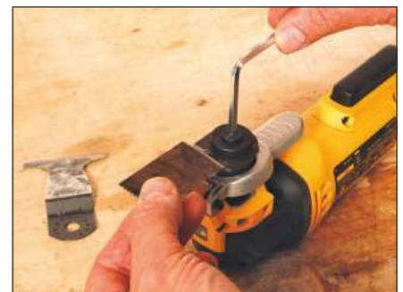
Fitting standard blades with the supplied adaptor
