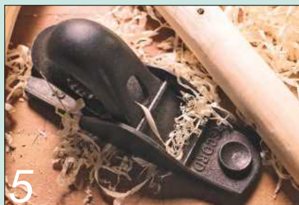
5 The nifty 102 block plane used for finishing
