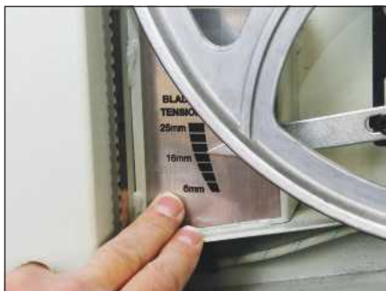
Tensioning can be assessed with the indicator
