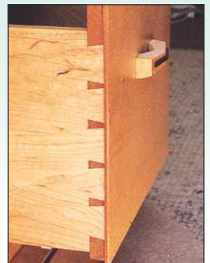
15 The finished joint. The lip on the bottom edge of the drawer hides the clearance required for hidden drawer guides
