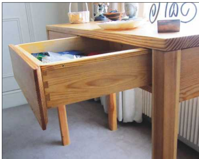
9 Both ends of the offcut are tapered to minimise the risk of binding or racking. The false fronts are chamfered at both ends so that they don't catch the legs or each other as the drawer closes, and along the bottom to provide a finger-sized lip
