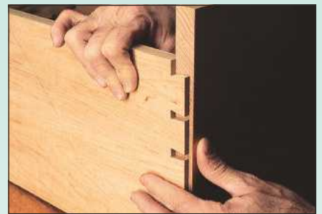
12 Check the final fit before assembly
