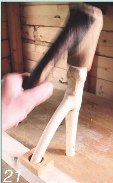
21 Setting the natural hook holdfast with a tap on the head
