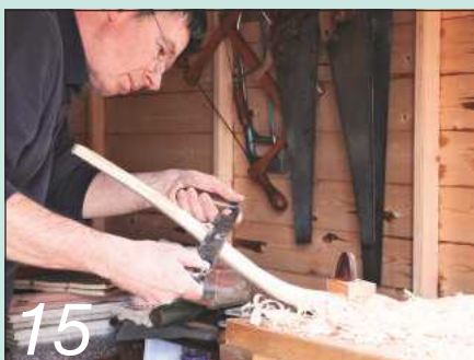
Further shaping of the hawthorn beak using a drawknife
