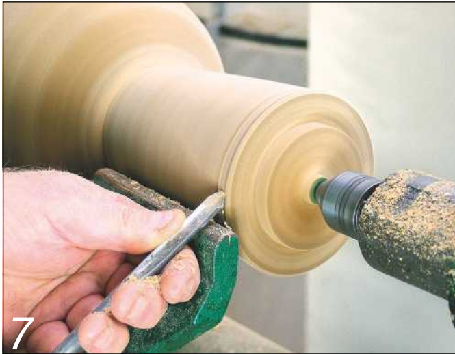
7 Cut a bead at the base using a spindle gouge...
