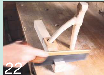
22 Clamping the work for sawing
