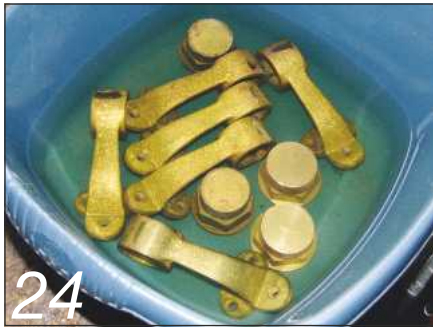
24 Soaking the brass parts in a hot solution to shift the worst of the muck
