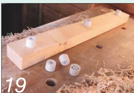
Door stops screwed to the bench stop locate with holes in the bench
