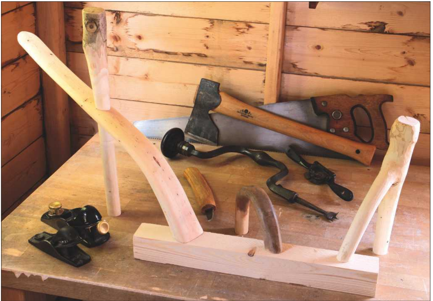
The three holdfasts and the tools used to make them. From left to right: two-part ash and hawthorn; chestnut crook walking stick; grown ash hook
