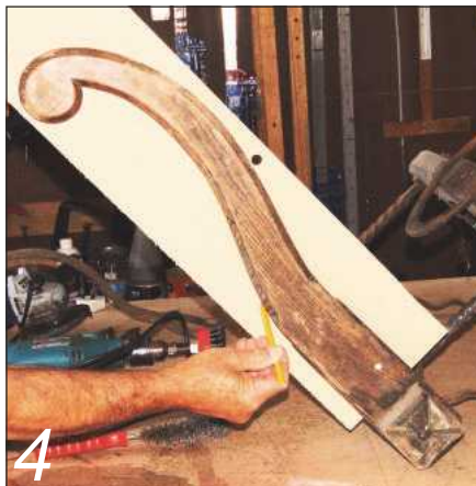
Making a template to repair two of the vertical arms
