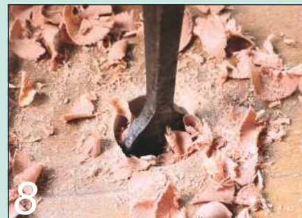
Close-up on the centre bit at work. Shavings are like pencil sharpenings
