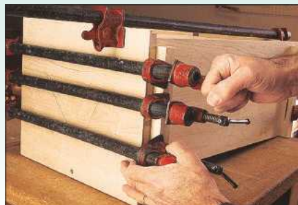
14 Use lots of clamps and check carefully that the drawer is square
