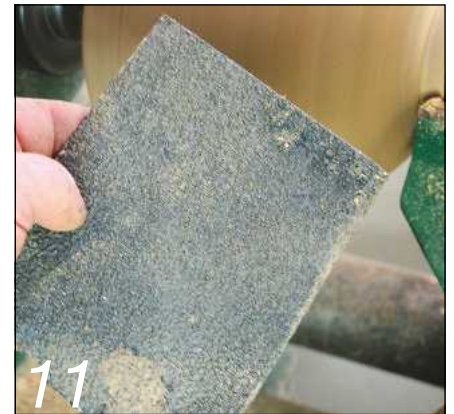
11 24 grit abrasive paper adds some nice texture – or scratches...
