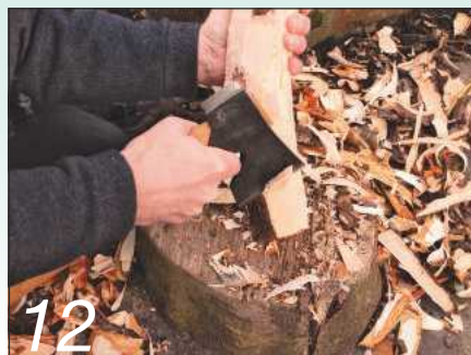
Preliminary shaping of the hawthorn with the carpenter's axe
