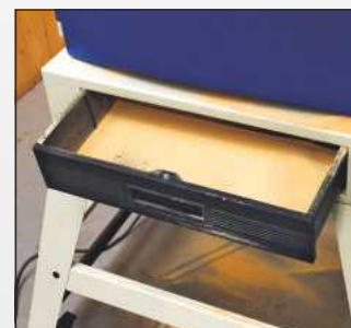
As an indication of the collection feature, this is from one rip cut
