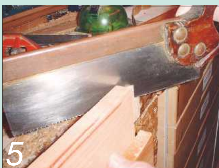
5 The mitres on the tenons must be cut very accurately, an important skill
