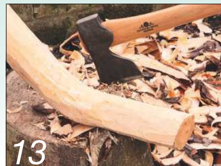
A natural curve benefits from the strength of continuous long grain
