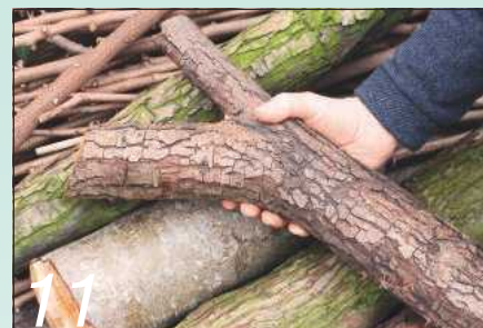
A natural curve of hawthorn for the beak of the two-part holdfast
