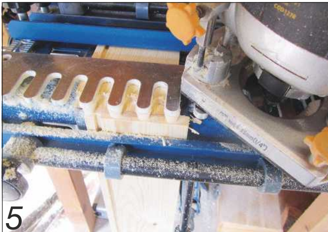
5 On most dovetail jigs, the stops – the silver slides visible just to the left of the wood, above and below the comb – move independently. But since the offset between the wood pieces is always the same, driven by the size of the teeth on the comb, the joint would be easier to cut accurately if the stops were fixed together
