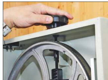
Initial tensioning is achieved with the top adjuster
