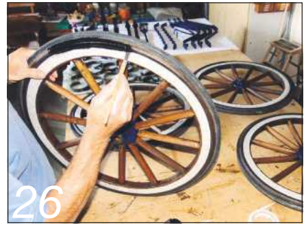
26 I had to mask off the rims of each wheel to paint the metalwork black
