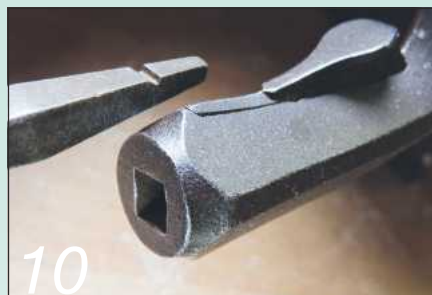
A notch in the bit's square shank locates with the clip in the brace
