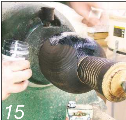
15 Apply ebony dye to give the piece a uniform shade of black
