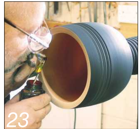
I stained the inside red using spirit-based stains and then oiled the piece
