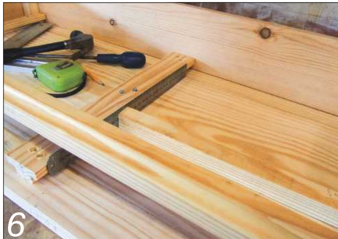
6 A spacer bar helps to make sure the hangers are parallel before they're screwed into place on the underside of the table top
