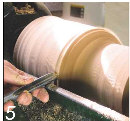
5 Shape the outside with the bowl gouge...
