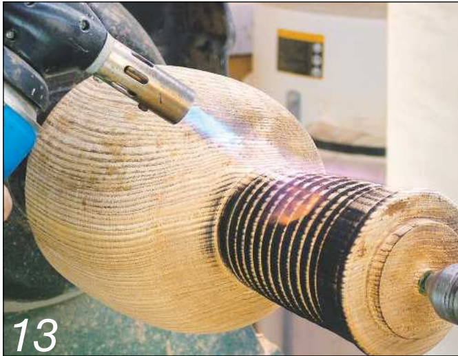
13 Give the whole of the outside a good scorching with a blowtorch
