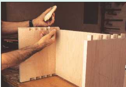
13 Generously apply glue to the pins and the spaces between them
