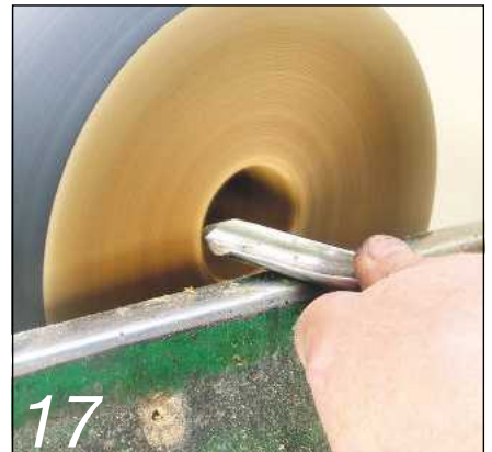
17 Use a spindle gouge to hollow the piece, starting in the hole...
