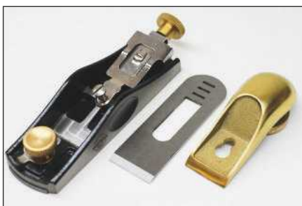
The basic component parts; note thickness of blade
