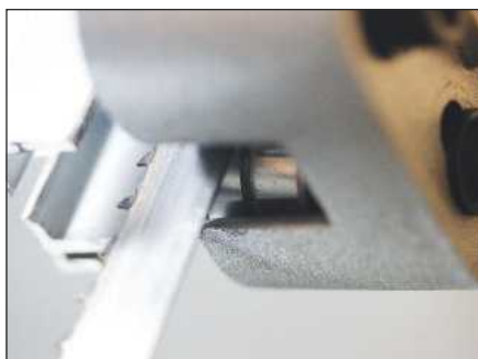
A neat feature is the use of double bearings for blade support
