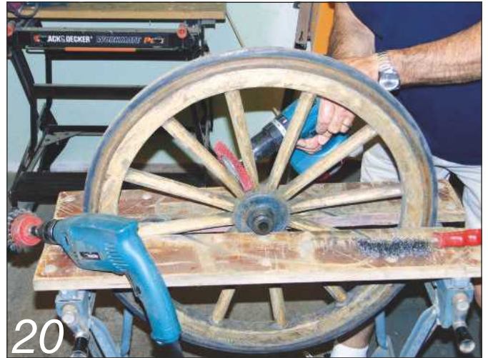
The wheels were cleaned up with a variety of powered wire brushes, etc.
