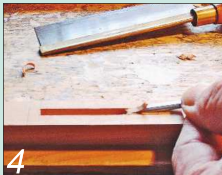
4 The waste is removed from the tapered haunch with a sharp chisel, a little at a time
