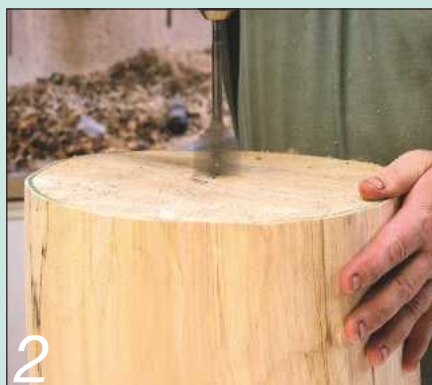
2 Drill a hole in the centre to match the diameter of the shaft of your four-prong drive
