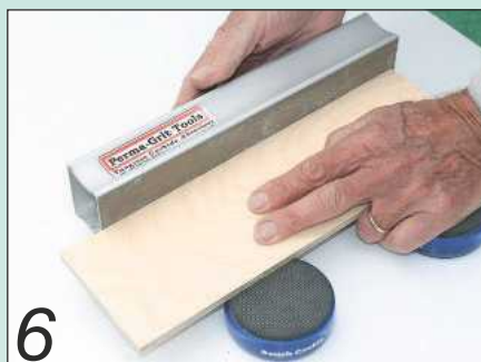
6 It's best to cut just on the waste side of the marked line and sand the edge back to it
