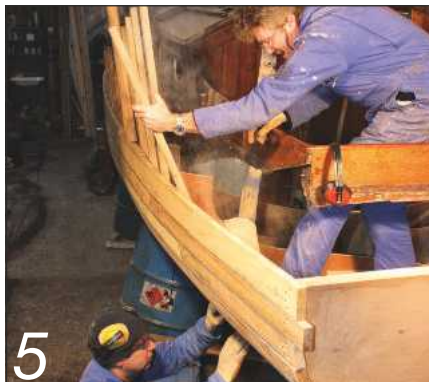
5 He holds the inboard end of the wood in place with one foot as he bends it to shape
