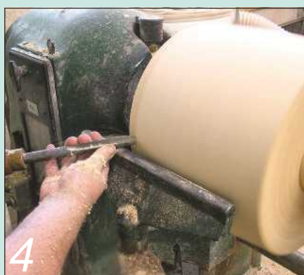
4 True up the circumference to create a blank that's just under 260mm in diameter
