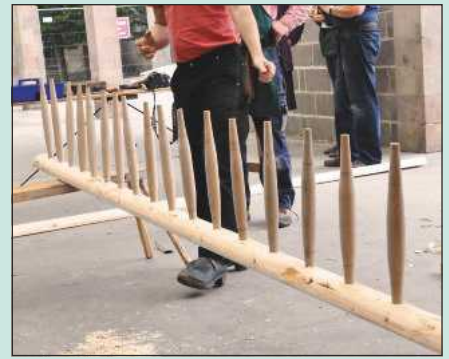
After fitting the rungs into their tapered holes in the first stile, we were ready for the tricky job of adding the other stile
