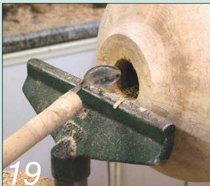
19 This home-made gadget is ideal for clearing shavings from the inside of hollow forms
