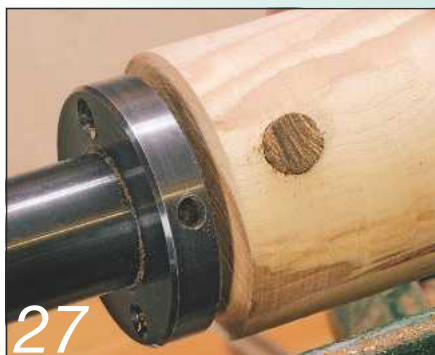
27 A cross dowel through the blank will ensure the firmest screw fixing
