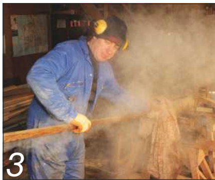
3 The steamed timber is removed from the tube; thick gloves are essential here!
