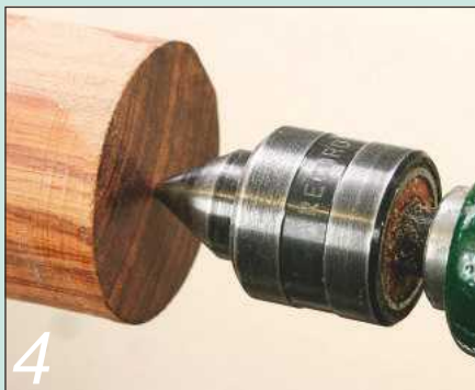
At the tailstock end, a revolving type centre is the ideal choice
