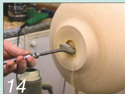
14 Drill a large-diameter hole down the centre of the piece to the depth of the hollowed area
