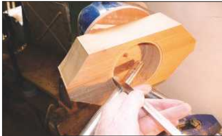
1 After trimming the blank roughly to shape, hollow out the central recess
