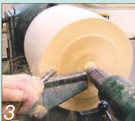
3 Use a ½in fingernail profile bowl gouge to make push cuts on the ends and cut a chucking spigot
