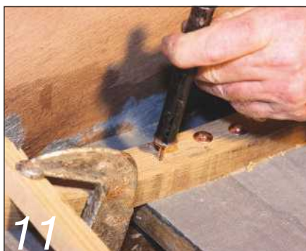
11 A special home-made punch helps to drive the copper rove onto the nail
