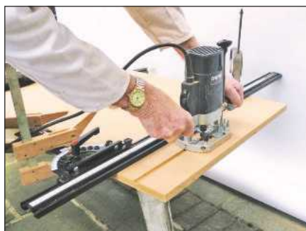
Forming a trench with a router was a quick and easy operation to carry out
