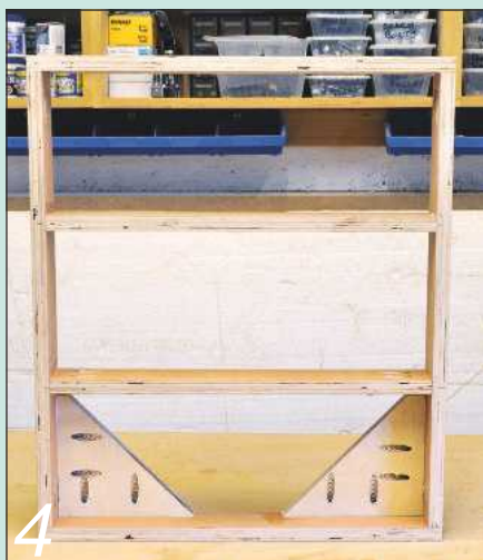
4 Similar smaller plywood triangles do the same job on the smaller base frame
