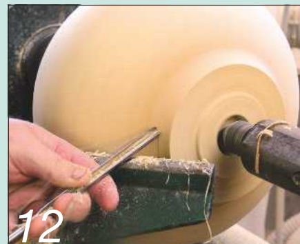
12 Start at the widest part and cut down to the narrowest part, taking very light cuts
