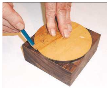
6 I used a circular plywood template to mark the curved corner lines
