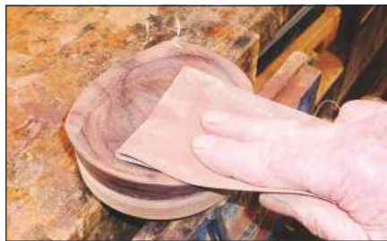
8 Hand sanding is the only practical way to complete the shaping of the lid
