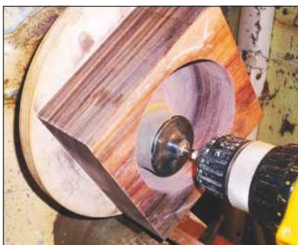
4 Sand the inside of the box using a small drum sander in a power drill
