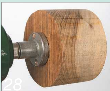
28 On cross-grain work a single screwchuck will hold surprisingly large pieces
