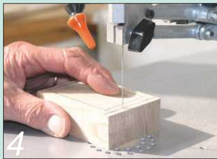
4 Most scrollsaws have sufficient power to cut wood up to 50mm thick with ease
