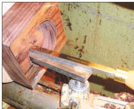
2 The Sorby platform support is a useful part of their tool rest system
