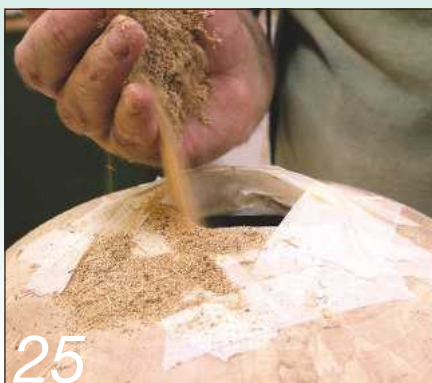
25 Then pour in a couple of handfuls of sawdust collected from the bandsaw and shake it around
