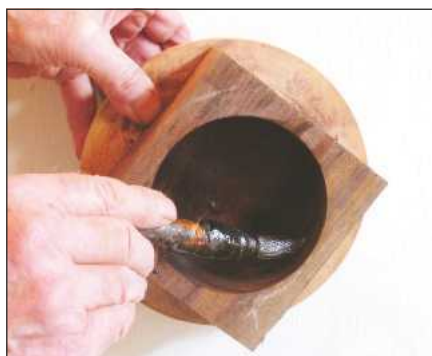
5 Take the faceplate off the lathe and apply lacquer to the recess
