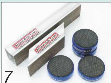
7 Bench Cookies will hold a sheet of ply firmly on the bench when marking out or sanding
