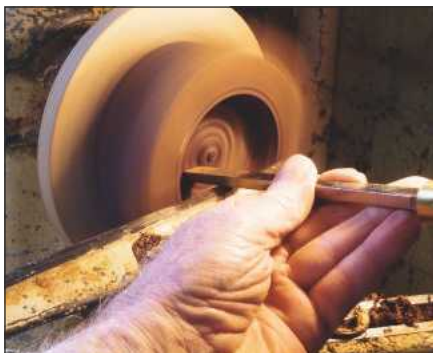
1 The hollowing out is done mostly with a square-ended scraper
