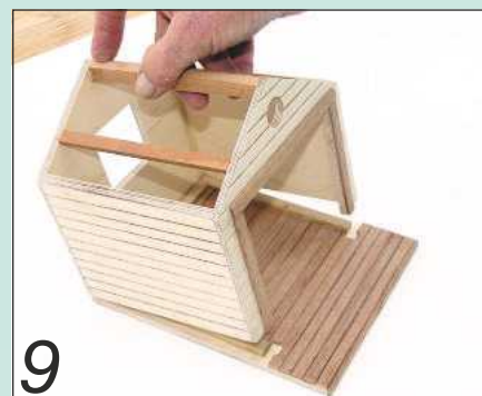
9 Glue the shell to the base, check that it sits squarely and set it aside to dry
