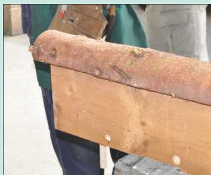
The raw stile is held on the edge of the timber by a peg driven up through it into a pre-drilled rung hole
