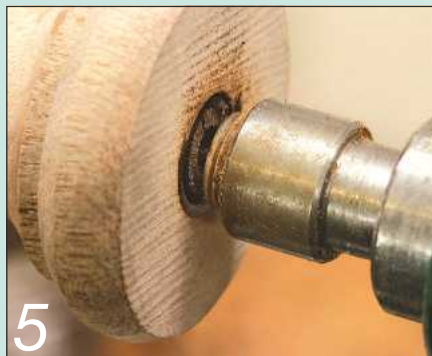
There's a real chance of burning the work with the 'dead' type of centre
