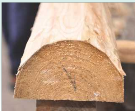
Three facets were planed on each side of the stile before a spokeshave was used to finish it to a round profile
