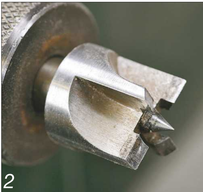
A 1in diameter drive centre with four prongs will cover most of your needs
