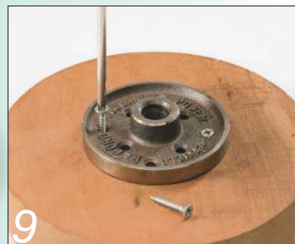
Steel faceplates are best because they don't distort when attached
