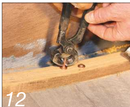
12 A pair of end cutters is then used to cut the nail just above the rove
