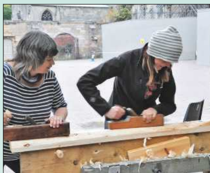
Here Heather and Chrissy coordinate their planing of the pole into a stile with a straight semi-circular profile
