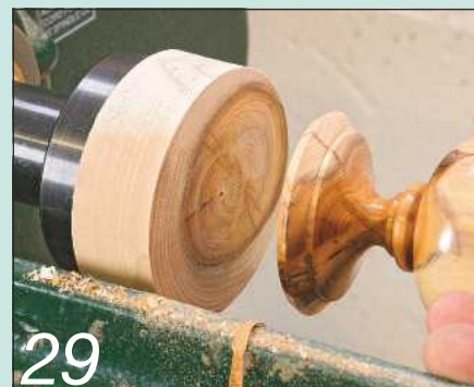
29 Parting off clear of the screw is wasteful when turning expensive wood
