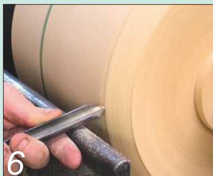
6 Start shaping the piece at the bottom with the ½in bowl gouge, working back to the line
