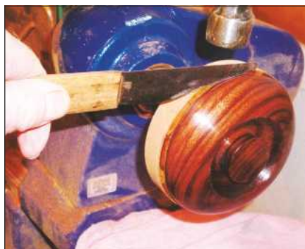
11 After finishing, prise the lid off the tape by inserting a knife blade and tapping it down
