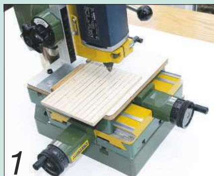
1 I used a small overhead router to simulate the tongued-and-grooved wall cladding
