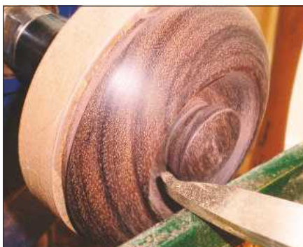
10 Reverse the lid, turn it to a dome shape and form the finger grip
