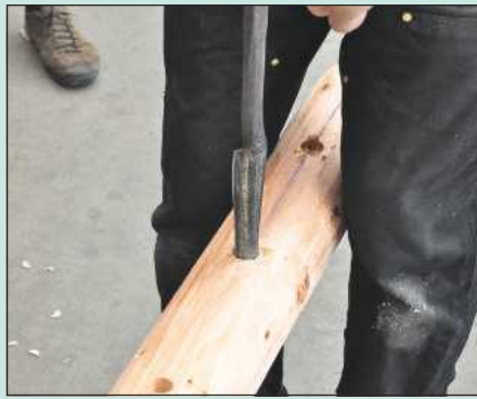
After all holes were drilled at ¾in diameter using a brace and auger bit, it was time to create the tapers
