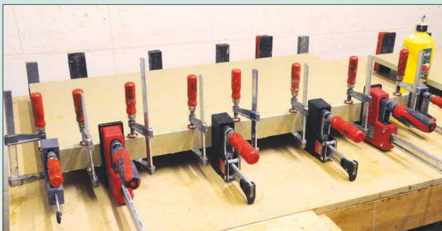
6 The top panels needed a mitred upstand. I cut this over-size to make machining safer...
