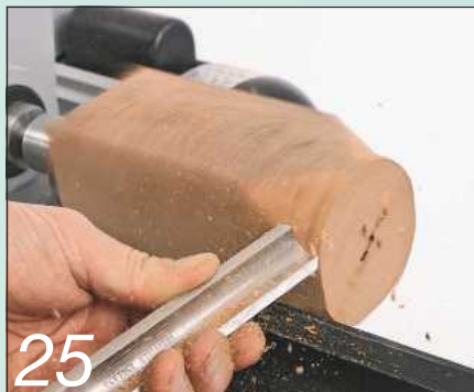
25 You should be able to hold a sizeable workpiece such as this with just a single screw
