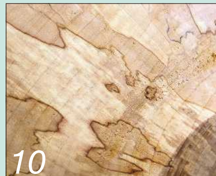
10 Spalting decays the wood and sometimes it's difficult to achieve a good finish
