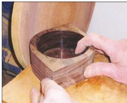
8 A disc sander is ideal for final shaping of the blank down to the lines
