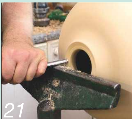
21 Then use a \frac{3}{8} in spindle gouge to clean up and shape the neck and opening of the vase
