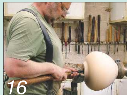
16 Keep the handle of the tool under your forearm for greater stability and control
