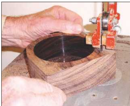
7 Remove the waste on the bandsaw, cutting just outside the marked lines
