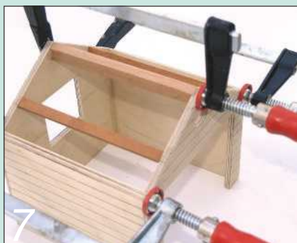
7 Cut and fit the three roof supporting bars and cramp up the building's shell
