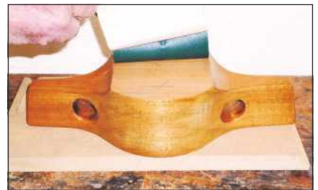
9 Lacquer and polish the box and lid, then add baize to the base
