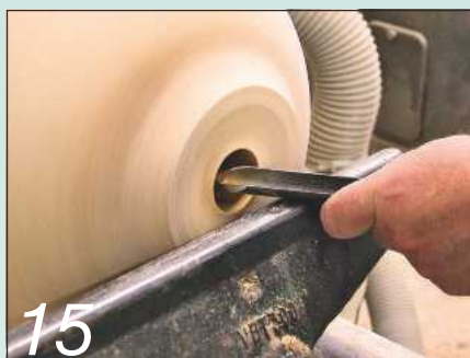
15 Push the gouge into the drilled hole and, as it cuts, push the handle away from you
