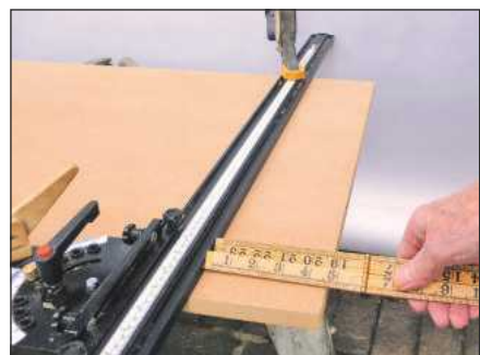
The guide must be accurately positioned and securely cramped to the workpiece
