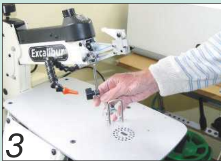
3 A hold-down device is useful as it stops the work jumping up on the upstroke
