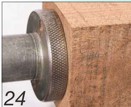
24 ...so the rim of the chuck fits tightly up against it and can't wobble
