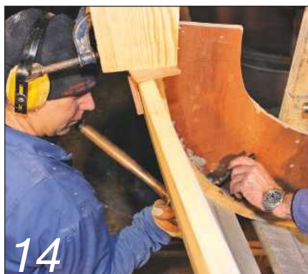
14 Dean ensures the nail remains in position by placing a dolly against its head
