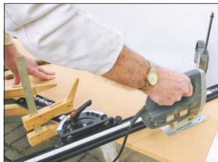
Note the positions of the three cramps when making a jigsaw cut at an angle
