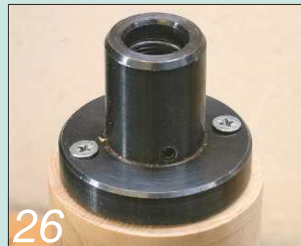
26 Use additional screw fixings for longer workpieces in softer wood
