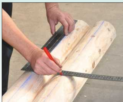
We stepped off the rung spacing with dividers on one stile and then squared the marks across to the second stile
