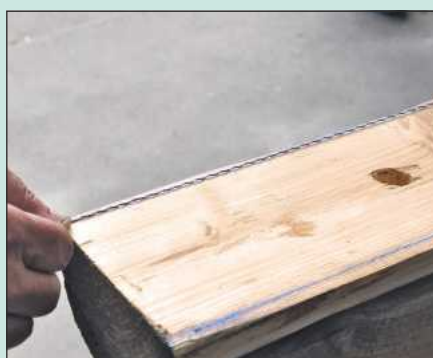
We used chalk lines – a crude but surprisingly accurate technique – to mark the straight outer edges of each stile
