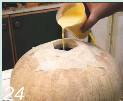
24 Pour enough diluted pva wood glue into the hole to cover the entire inside of the vase
