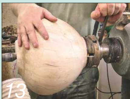
13 Keep checking the tightness of the chuck, particularly if the wood is at all wet
