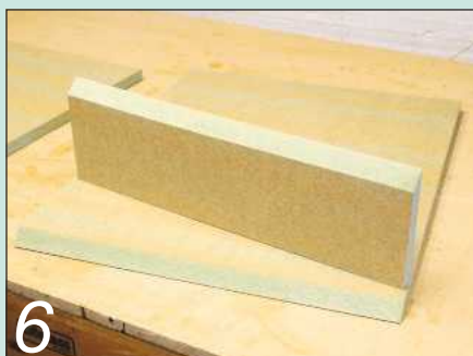
6 The top panels needed a mitred upstand. I cut this over-size to make machining safer...
