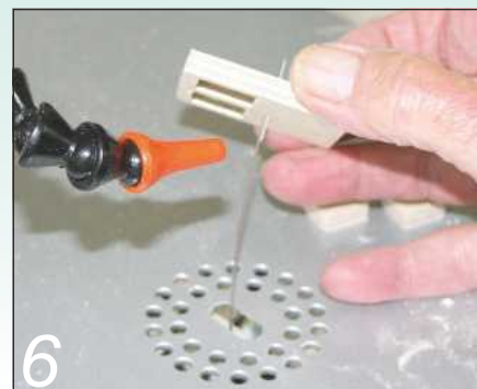
6 I prefer to thread the blade up through a pre-drilled hole before reattaching it
