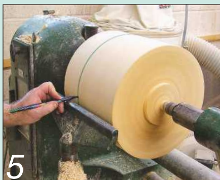
5 Mark a line on the piece about 100mm from the top to show the maximum diameter
