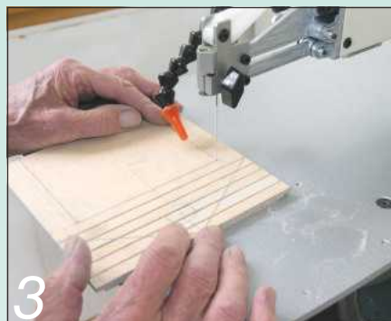
3 When cutting out door openings, first drill a small hole inside each internal corner
