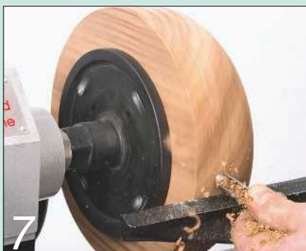
A faceplate allows free access to one end of the workpiece
