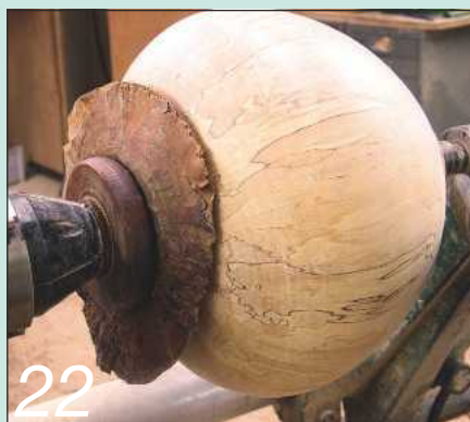
22 Reverse the vase onto a padded dolly and bring up the tailstock so you can clean up the base
