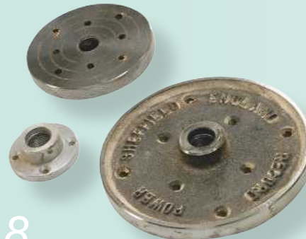
Faceplates come in a range of sizes, up to 6in in diameter
