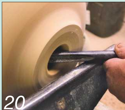
20 Use the edge of the opening for leverage to help remove wood from the inside wall
