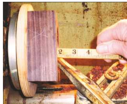
3 Check the depth of the recess by comparing the inside measurement with the outside
