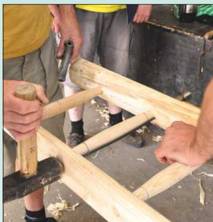
Each tie rod is fed through its pre-drilled holes (above), and the free end is then hammered over to lock it in place (left)
