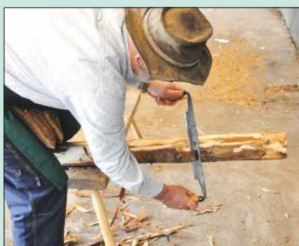
A traditional draw knife was the perfect tool to use for removing the bark from the two stiles evenly and quickly
