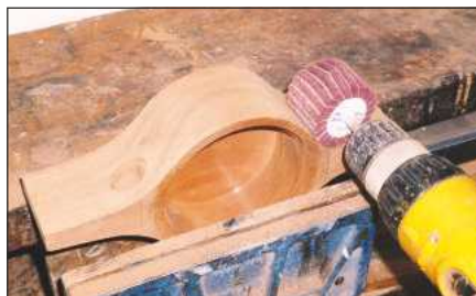
5 Round off the finger holes, then sand the wings to their final shape
