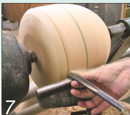
7 Then shape some of the top before blending the two curves together smoothly
