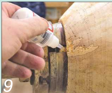
9 Reverse the piece onto the chuck and glue it in place for additional security
