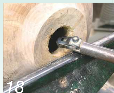
18 A specialist hollowing tool like this makes short work of cutting through endgrain
