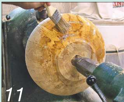
11 A liberal coat of thinned sanding sealer hardens up the soft wood fibres
