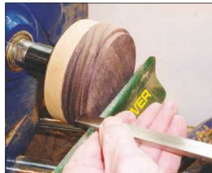
9 Stick the lid blank onto the ply and form a shallow rebate all round the edge
