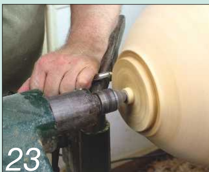
23 Use the \frac{3}{8} in spindle gouge again to remove the spigot and slightly dish the base
