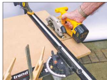
The guide was equally accurate when used with a hand-held circular saw
