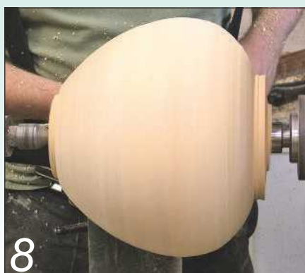
8 The final profile you achieve should resemble an egg rather than a rugby ball
