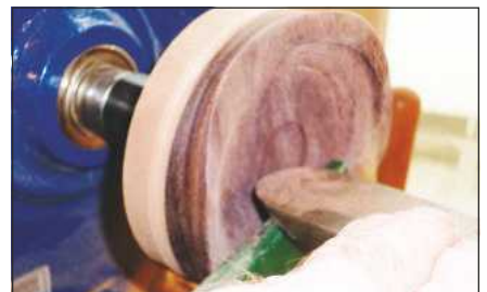
6 Turn the lid with splayed edges and dish the central area slightly
