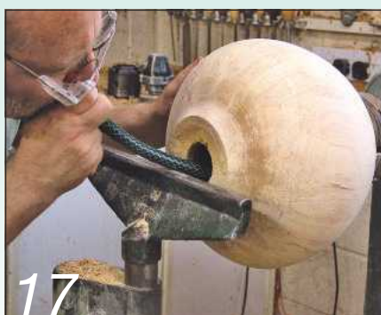
17 Stop the lathe frequently and blow out the build-up of shavings inside the vase
