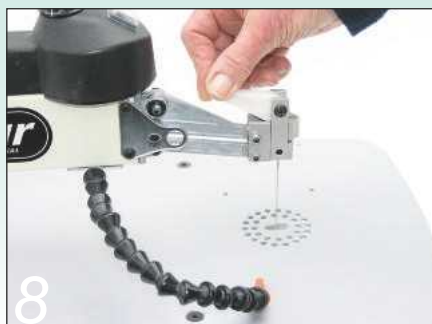
8 The holes in the table allow sawdust to be sucked down if the saw is attached to an extractor
