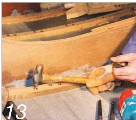
13 The rounded pein of the hammer is the ideal shape for clenching the nail over the rove
