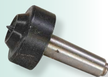
Cheaper dead centres often have small and inadequate bearings
