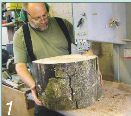
1 I first cut a 280mm diameter blank from the block to remove the radial checks
