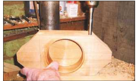
3 Bore the finger holes through the blank on the drill press, working from both sides
