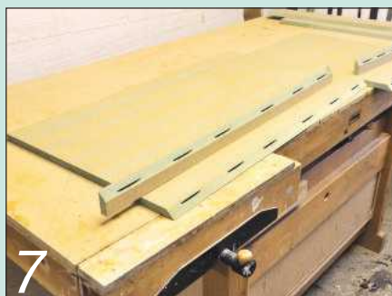
7 ... and only trimmed it down to 50mm wide once the biscuit slots had been cut in it
