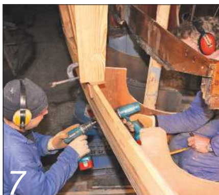
7 Dean countersinks the hole for the nail head once Jonathan has drilled the hole from inside
