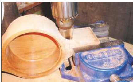
4 Trim the wings to shape, then enlarge the finger holes into a cone profile
