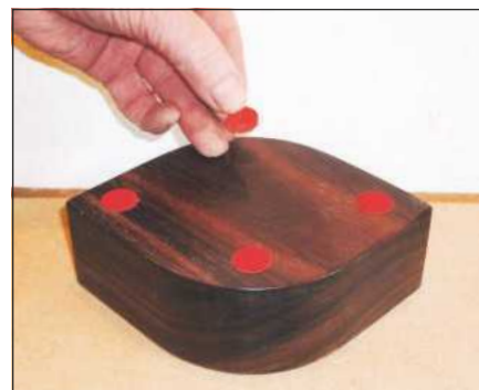
12 Punch out four self-adhesive felt discs and stick them on the underside of the box
