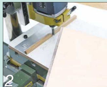
2 The same set-up is used to cut rebates along the edges of the walls
