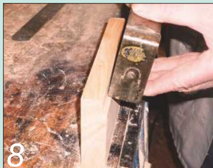
8 The edge of the rebates needed to be bevelled slightly – an ideal job for a shoulder plane
