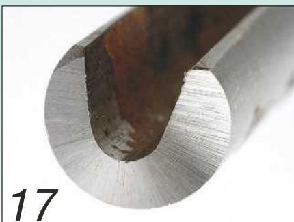
The bowl gouge is more U-shaped than the spindle gouge
