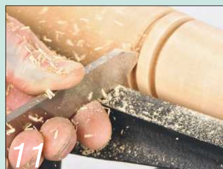
11 A parallel-section 1/8in parting tool is a good starter
