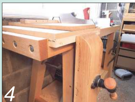
4 A batten underneath means I can secure the board in the vice for stability
