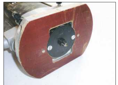
The guide bush and cutter are mounted in the router baseplate as shown
