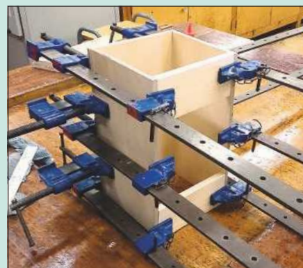
2 I used all the sash cramps I could find to secure the glued-up box assembly
