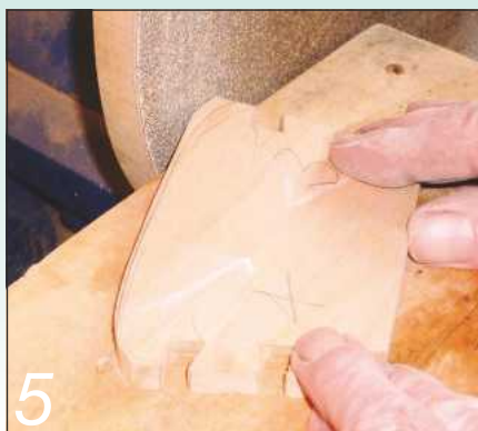
5 Shape the top edges of the two ends to a smooth curve on the disc sander, and check that they match
