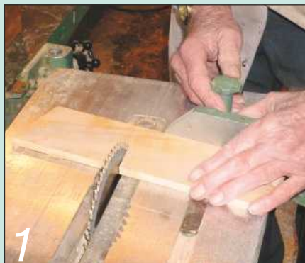
1 Cut the pieces for the ends to length with the ends splayed. The saw guard has been removed for clarity
