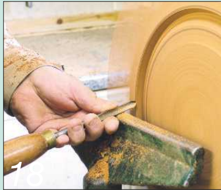
18 Work from both edges, as if you were cutting a cove on some spindle work
