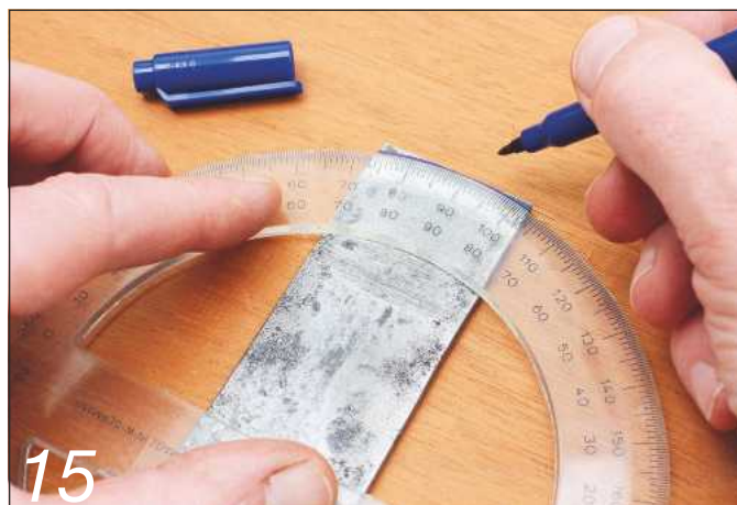
15 Converting a wooden Bismarck plane to a scrub plane began with marking a 3in radius on the iron
