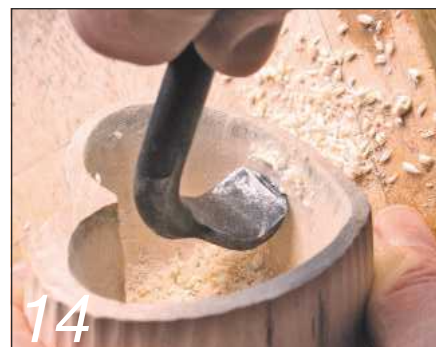
The gouge is used with a pulling action towards the rim, producing very fine shavings
