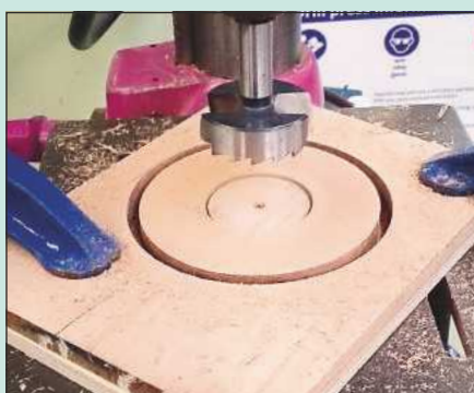
3 The decorative roundel for the end was initially formed on the pillar drill
