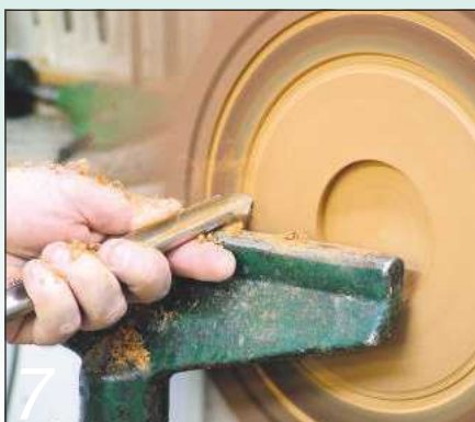
7 Cut a recess for your chuck and remove the waste area next to the foot
