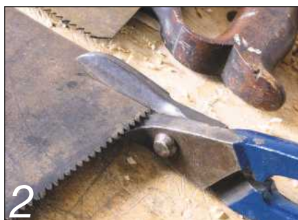
Gilbow metal shears cut saw plate, but it's hard going; wear a leather glove
