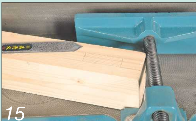
15 Mark up the mortise and cut in the lines to ensure a better finish. Mark both sides when cutting a through mortise
