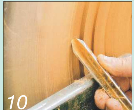
10 The view from another angle shows where the shaving should come off the tool
