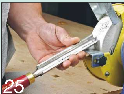
25 Many professional turners prefer to grind their tools freehand
