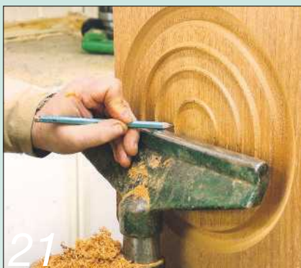
21 Mark out the equidistant positions of the notches using the lathe's indexing system
