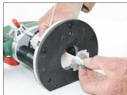
The guide bush fits into the base with a clever bayonet fitting; screws aren't needed
