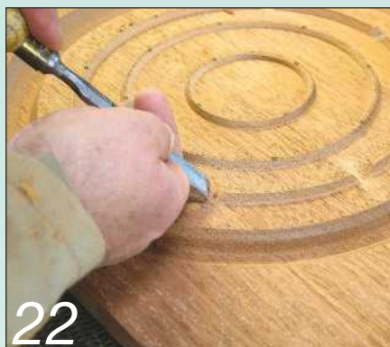
22 Remove the board from the chuck and cut all the notches carefully with a chisel
