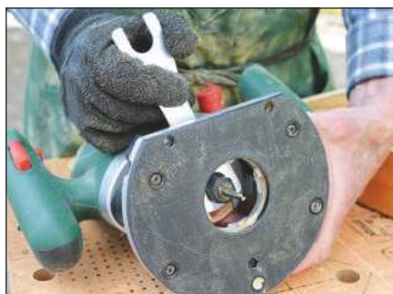
One spanner is all that is needed to secure and release the cutter
