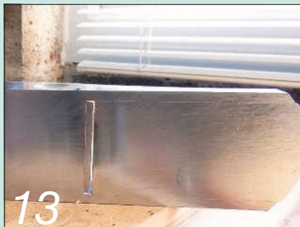
It's also important that the cutter edge is perfectly aligned to the sole
