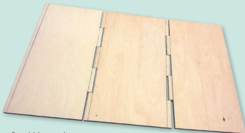
1 Long finger joints connect the main storage box components
