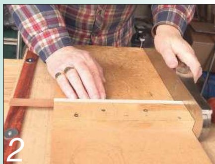
2 Making it double-sided means the datum surfaces of the workpiece are always in the right place
