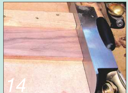
The No 9 mitre plane with its unusual 'hot dog' handle has a lot going for it
