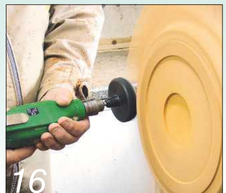
16 When power sanding, keep the sanding pad as vertical as possible
