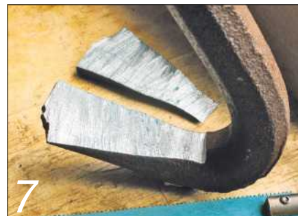
I next made a perpendicular saw cut to create the initial taper for the blade...
