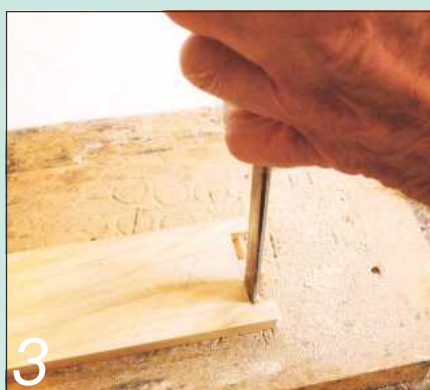
3 Mark out and cut the dovetail pins, using a tenon saw, a coping saw and then a chisel
