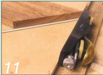
A block plane is ideal for tasks such as mitring banding using a 45° block as a jig
