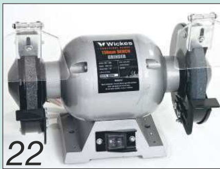
22 The narrow wheels on budget grinders can make the tool difficult to control
