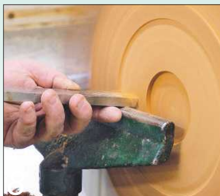
8 Use a square-ended scraper instead of a bowl gouge to finish the clean-up
