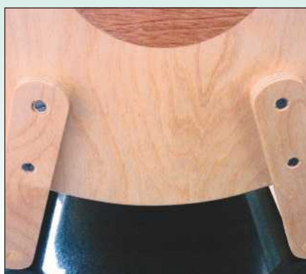
10 The splayed plywood legs are glued and screwed to the ends of the drum
