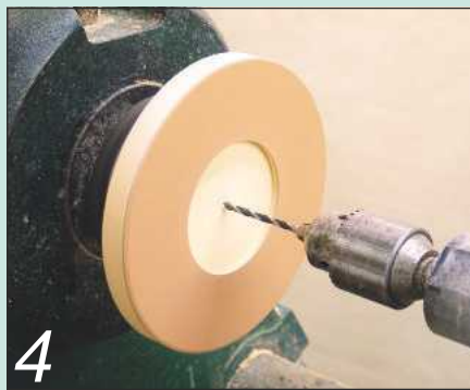
4 Drill a small hole in the centre using a bit fitted in a Jacobs chuck in the tailstock
