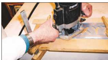
The templates sit between guide battens cramped to the workpiece as the cuts are made
