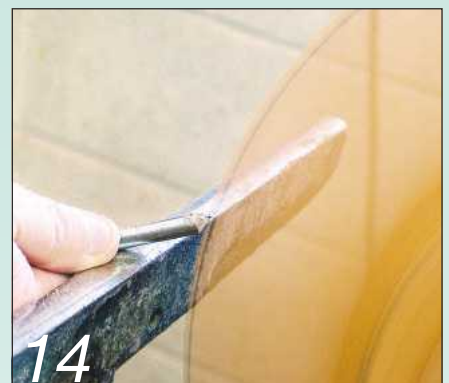
14 Take gentle cuts using a spindle gouge on its side to clean up the edge
