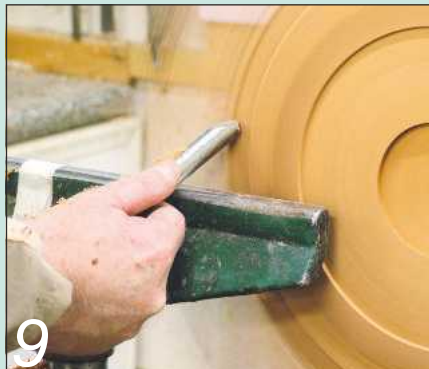
9 Keep the handle of the gouge right down when you're cutting the wings
