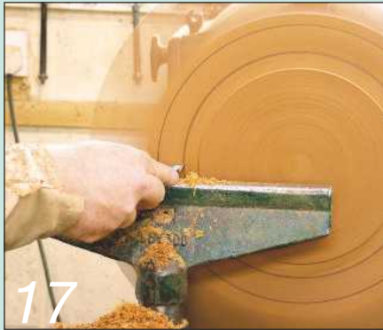
17 Mark the position of the moat; note the raised area left in the middle of the platter
