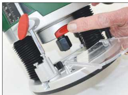
The red lever on the side of the router body locks the spindle shaft
