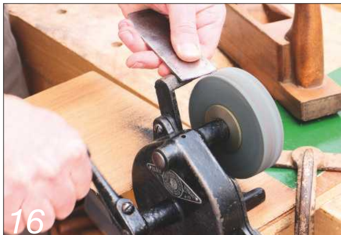
16 Grinding the scrub iron radius on the hand-cranked grinder was a slow but effective process
