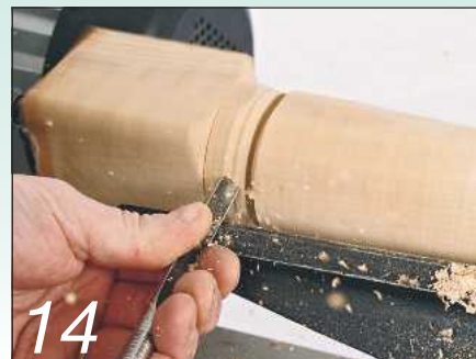
14 Your first spindle gouge should be the 3/8in size
