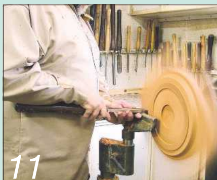
11 Note the position of the handle under my forearm in this alternative shot of the scraper
