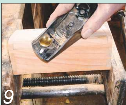
9 Create the curved profile of the top using jack, smoothing and block planes, followed by sanding
