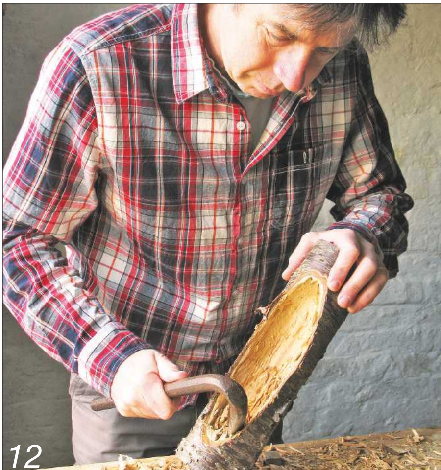
The 'eider' adze was remarkable effective at hollowing a rustic cherry log bowl
