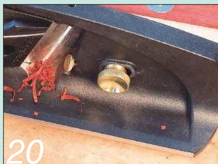
20 The smaller knob is positioned to stop the soleplate from contacting the blade
