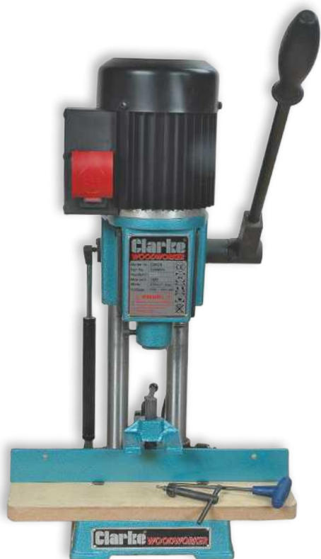
1 This small bench-top machine will cut a mortise up to 16mm wide in softwood
