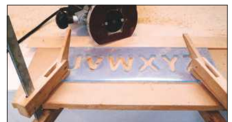
The template is moved along the guides to cut successive letter or number shapes
