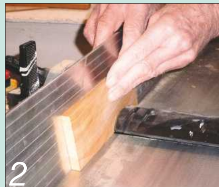
2 Plane the edges of the sides to the same angle. Again the machine guard has been removed
