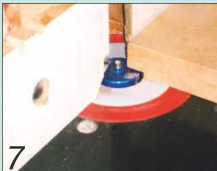
7 Cut the top to size and form the rebates along the long edges of this piece on the router table
