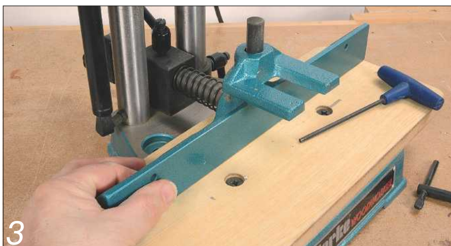
3 The fence of a small mortiser is adjusted by hand and locked into position
