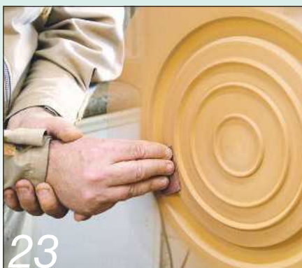
23 Power-sand the wings and then hand-sand the rest of the piece. Note my hand grip
