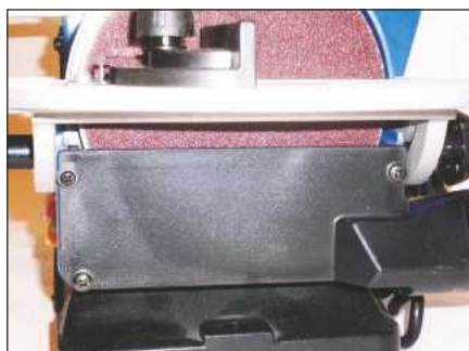
The disc guard below the table features a 45mm diameter dust outlet
