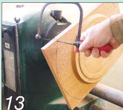
13 Remove the waste using a coping saw, cutting almost down to the line
