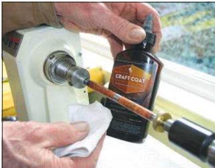
The product is easy to apply to pen barrels on the lathe as a friction coating
