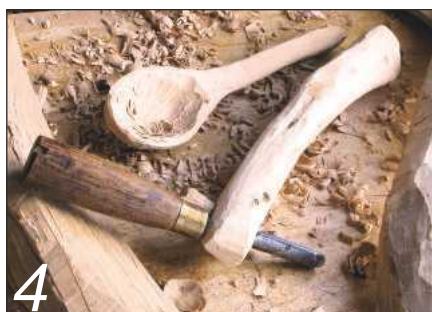
This small bowl adze was improvised from a gouge wedged into a sycamore handle
