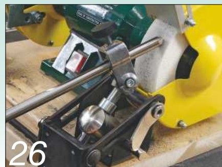
26 A jig such as this helps amateur turners to achieve professional-quality results
