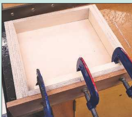
6 The storage drawer is a sturdy plywood box with a false front panel glued to it
