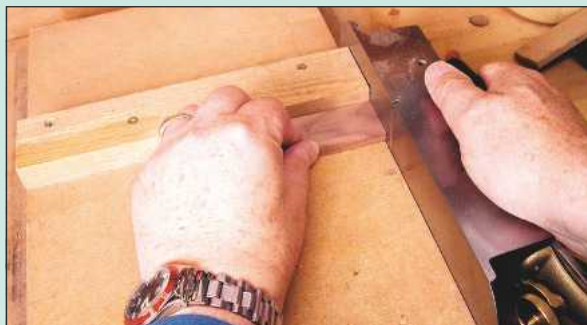
It's also important that the cutter edge is perfectly aligned to the sole
