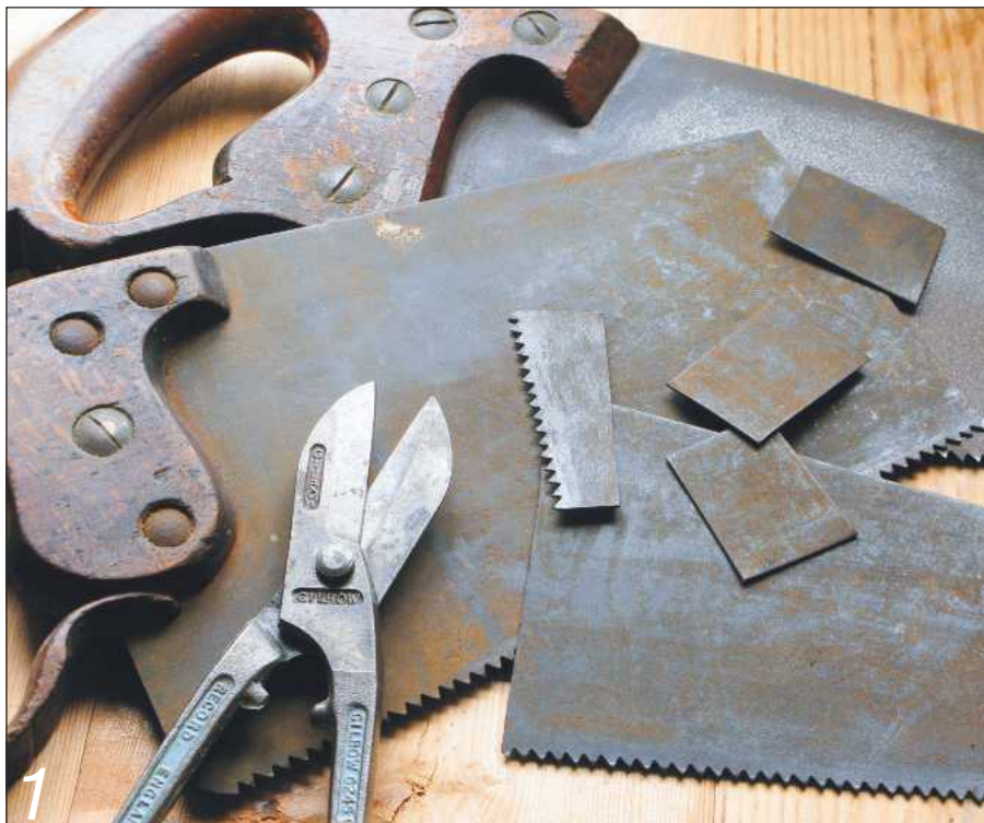
Old hand saws, bought on eBay, are a good source of high-quality steel
