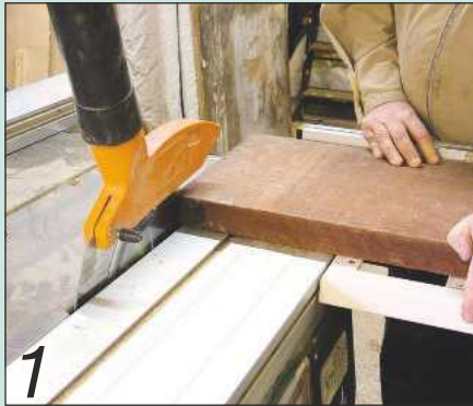
1 A table saw makes short work of squaring up the ends of the blank
