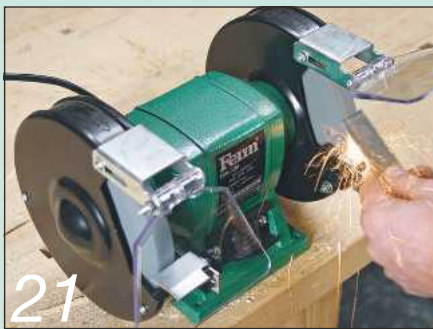
21 A standard double-ended grinder will do most of your sharpening work
