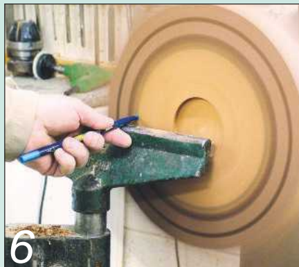
6 Clean up the blank and mark where the wings and the foot will be
