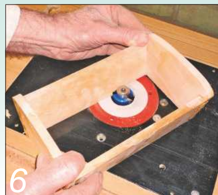
6 Assemble the sides and ends, then cut a rebate for the plywood base on the router table
