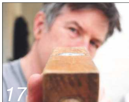
17 Sighting down the sole of the scrub plane shows the corners of the iron just inside the mouth
