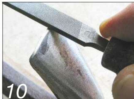
The last stage was filing a back bevel to help ease the blade out of the cut
