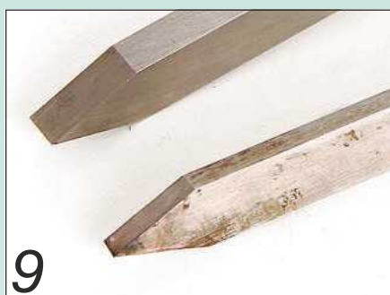
9 Parting tools form shoulders and separate finished work on the lathe
