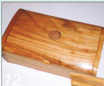
12 Stick the coin in place with epoxy resin adhesive and set it aside to allow the adhesive to set
