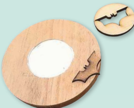
4 I used a laser machine to cut the small bat motifs for the inlay
