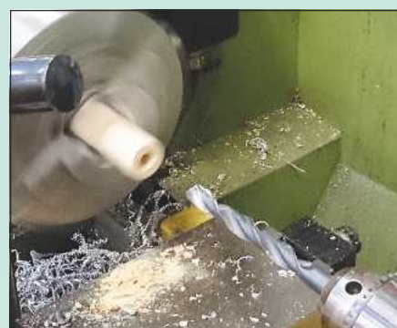
5 Drilling a leg stretcher rail was simple using a drill mounted on the engineering lathe
