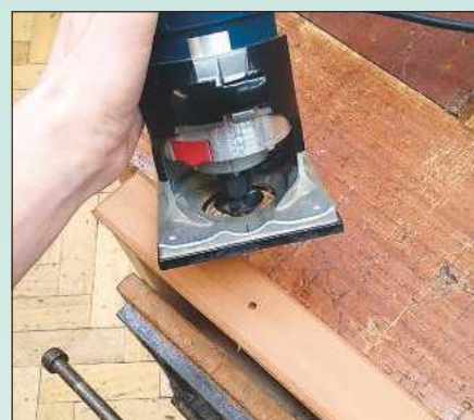
8 I added a small chamfer round the edges of the drawer front with a palm router
