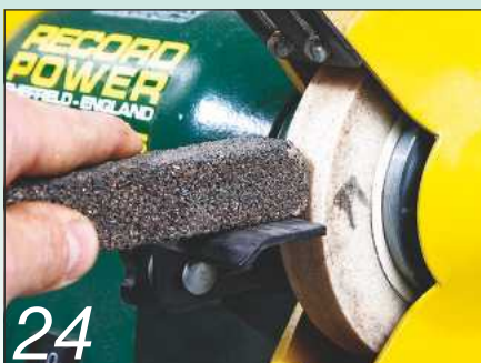
24 Clean your grinding wheels periodically with a dressing stick
