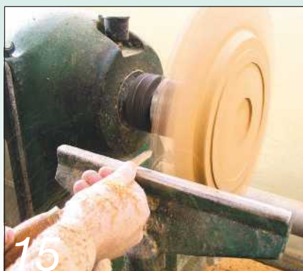
15 Cut in from both sides of the edges of the wings to avoid causing any breakout
