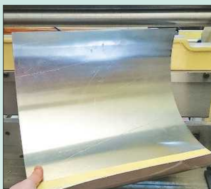
7 The aluminium sheet to form the rotating lid was carefully rolled into shape
