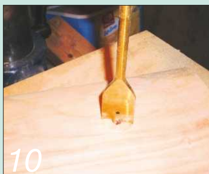
10 Drill a shallow hole to take the coin using a Forstner or saw-toothed bit of the correct size
