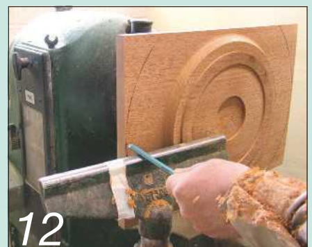
12 Stop the lathe and mark an arc on the extremities of the wings
