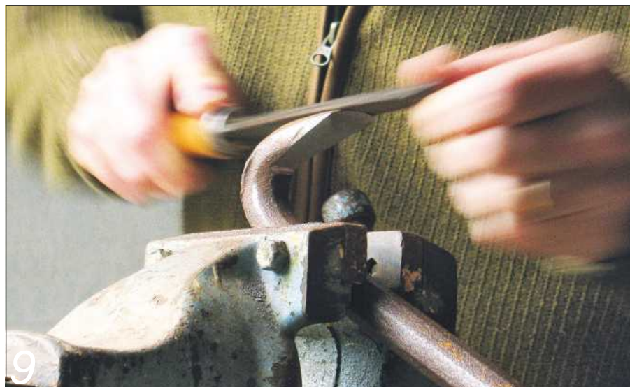
To file the cutting edge to shape, I clamped the wrecking bar in my engineer's vice
