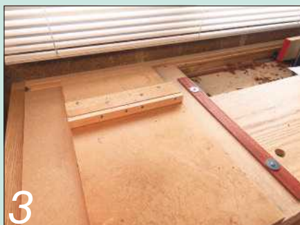
3 A recent adaptation is the extra guide to keep the shooting plane against the fence
