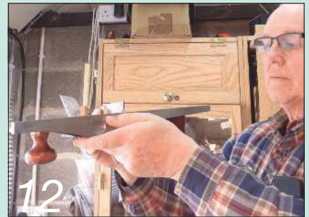
Check that the vertical sides of the plane's body are perfectly square
