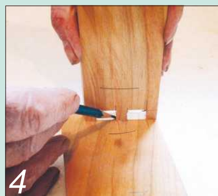
4 Then use the finished pins to mark out the corresponding tails and cut them as before
