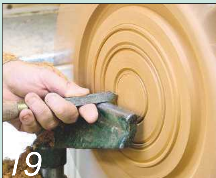
19 Use a modified parting tool to make a cut at each side of the rings
