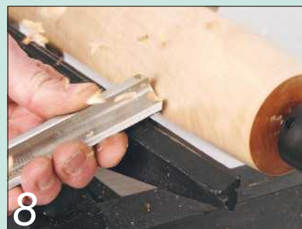
8 A 3/4in deep-fluted roughing gouge is the most useful size
