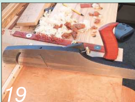
19 It also features a movable soleplate to adjust the mouth aperture
