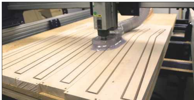
Cutting multiple components is easy on the CNC router
