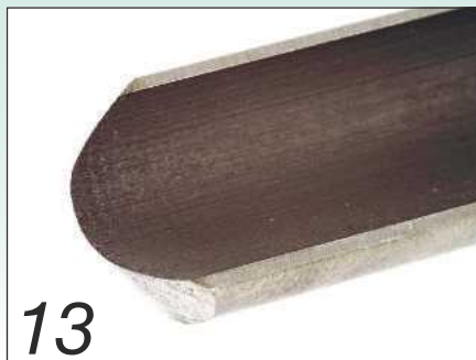
13 Most gouges are now machine-ground from a solid round bar
