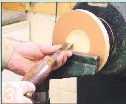
3 Prepare a circle of plywood and form a recess in it to fit your chuck
