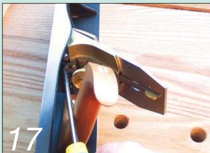
17 The Lie-Nielsen uses a traditional bedrock frog, adjustable without dismantling the plane
