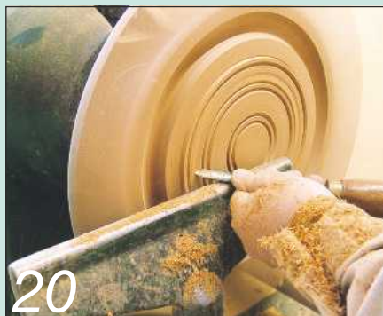
20 Use a spindle gouge to remove the area of waste wood from between the rings
