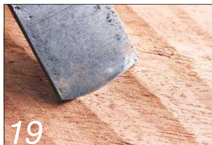
19 Here you can see the relationship between the scrub plane's iron and the flutes it cuts
