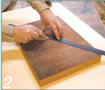
2 Find the centre of the blank by drawing two diagonal lines across it
