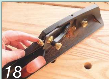
18 The Veritas plane uses a Norris adjuster featuring well-engineered screws
