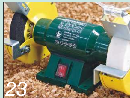
23 White grinding wheels are best for sharpening HSS tool blades
