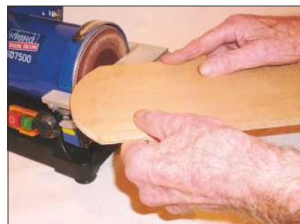
The sanding disc is ideal for smoothing a convex edge after bandsawing
