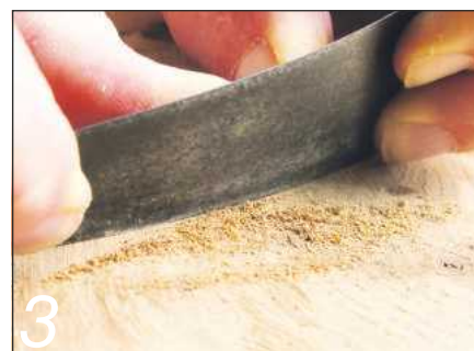
Using a saw-plate card scraper on elm produced fine shavings rather than dust
