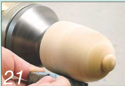
21 Sand the outside using a cork or foam block to protect your fingers
