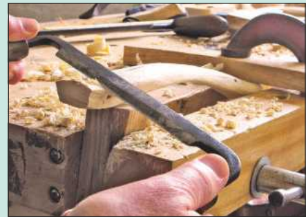
The bench brake is useful for small work too, such as this door handle taking shape
