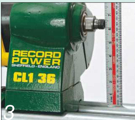
3 The swing should be at least 9in between the spindle and the bed
