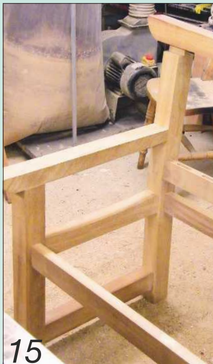
Link the end frames with the lower rails and dry-fit the upper back rail
