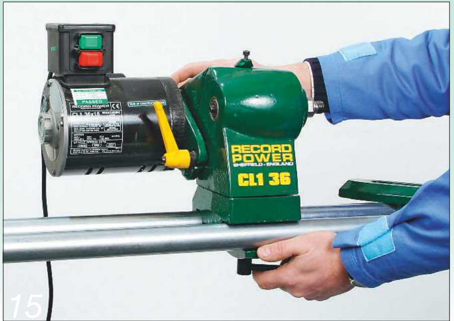
15 A headstock you can move along the bed is a big advantage
