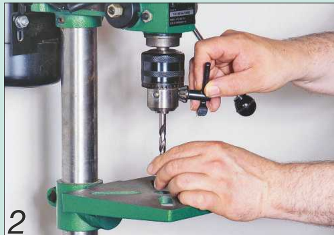
2 Rotate the bit between your fingers to centre it in the chuck
