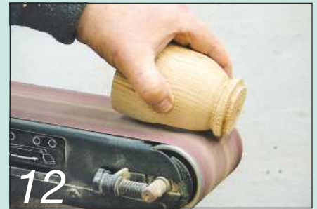
12 Sand a couple of shallow flats on the body using a belt sander
