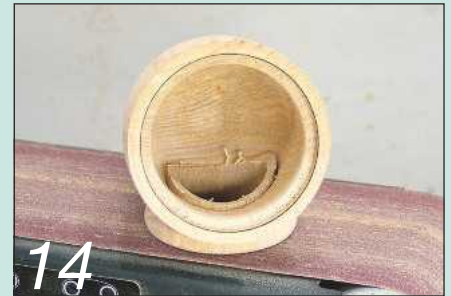
14 Keep trying the ring in the body until you have a perfect fit
