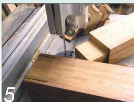
5 Remove most of the waste wood to create a slightly oversized tenon
