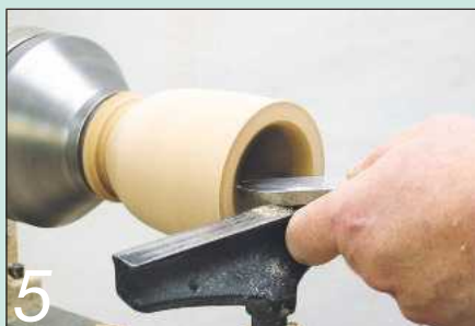
5 Switch to a round-nosed scraper to clean up the inside surface
