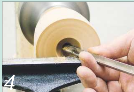
4 Then hollow out the interior of the blank as shown using the same gouge
