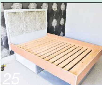
25 The headboard was fixed to the bed base and the upholstered panels added
