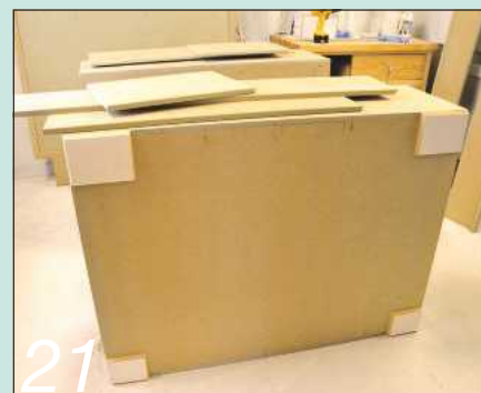
21 I used chamfered melamine-faced mdf to form sliding feet for the bed pods
