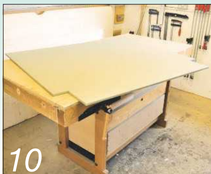
10 The back of the headboard is cut to size and shape from 12mm mdf
