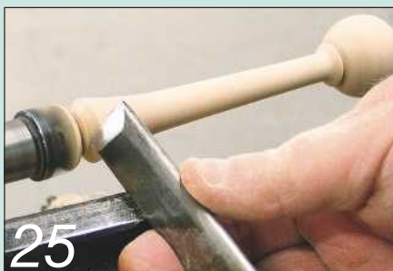
25 Part off the spoon handle using a slicing cut with the skew chisel
