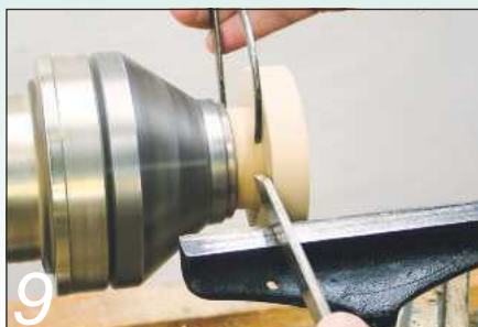
9 Turn a tenon on the ring blank to fit inside the hole in the body
