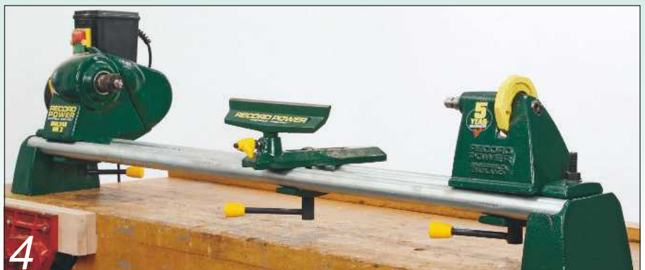
4 A bench-mounted model like this will suit most woodturning beginners
