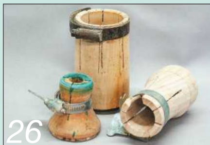
26 These home-made collet chucks are closed onto the work with a Jubilee clip
