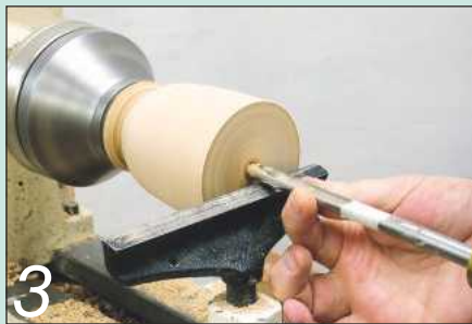
3 Use the spindle gouge to bore a hole down the centre of the blank
