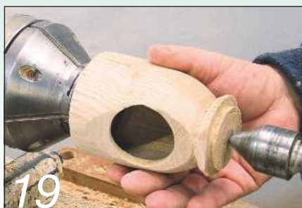
19 Glue the base into the body and re-mount its spigot securely on the lathe
