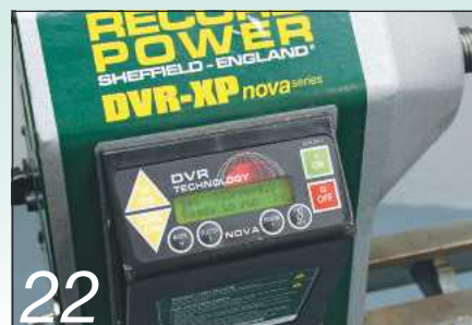
22 Electronic memory functions can remember your favourite speed settings
