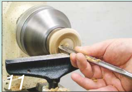
11 Continue the bead round to the front and then hollow out the ring
