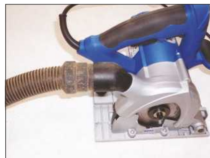
A vacuum extractor hose can be connected directly to the saw's dust outlet
