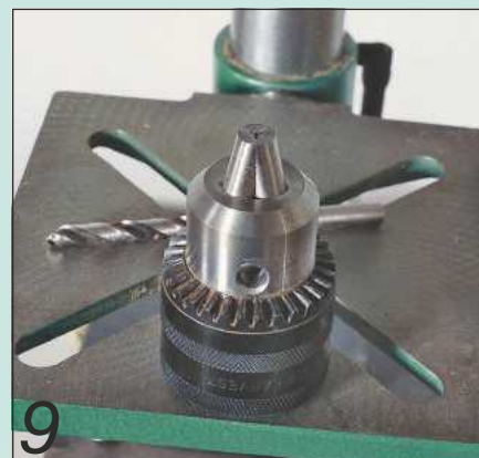
Remove the drill bit and close the jaws of the chuck fully
