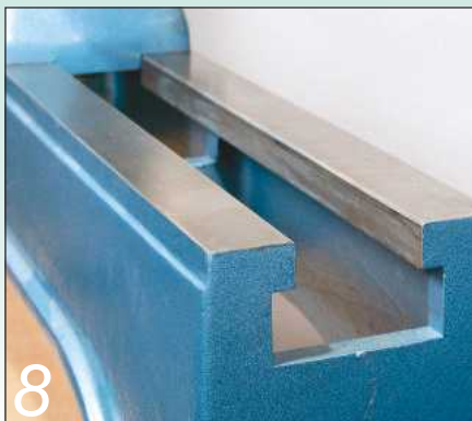
8 More expensive beds are solid castings that are almost a work of art
