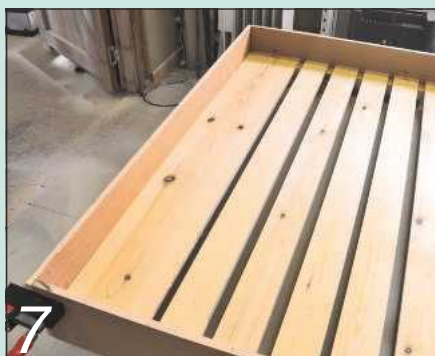
7 The last slat is double width to give extra support if someone sits on the end of the bed
