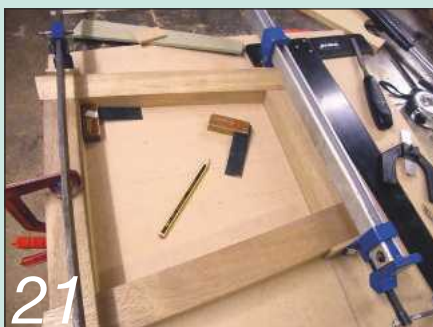
21 The table frame has no right angles; it's narrower to the rear and wider to the front
