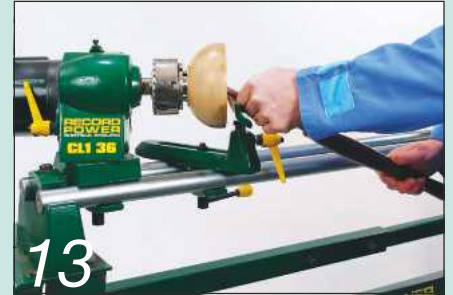
13 Swinging the head off-centre keeps tool handles clear of the bed
