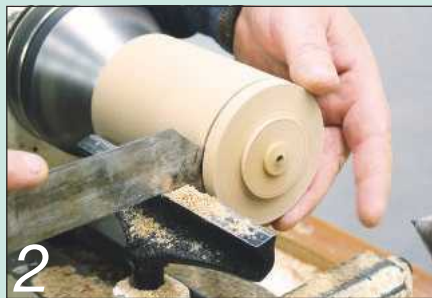
2 Turn another spigot and part off a 12mm length to form the base
