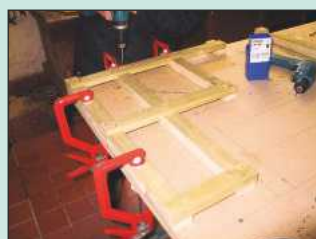
7 Drill clearance holes in the rails and drive in two fixing screws per joint
