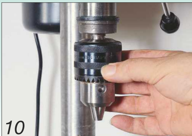
Fit the chuck back into the quill with a sharp upward movement
