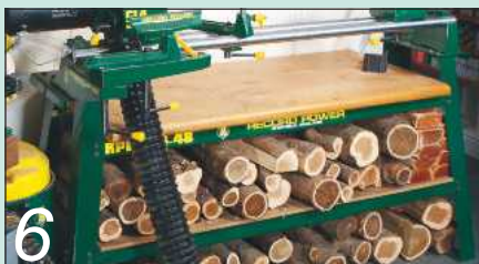
6 Under-bench storage helps to give a stand useful extra mass
