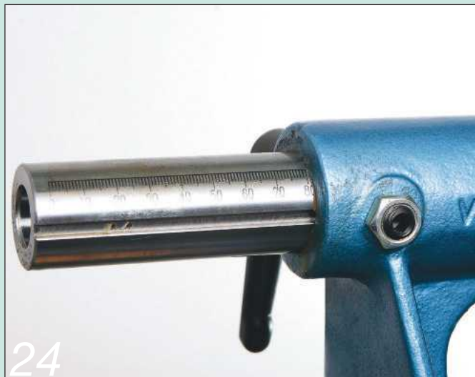
The tailstock barrel needs plenty of travel for drilling work
