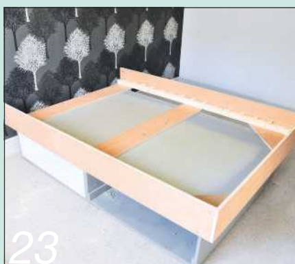
23 The mattress housing was then fixed to the base pods, again with connector bolts
