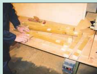
4 Check the fit of the rails in the leg housing joints, and ease them if necessary
