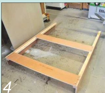
4 The bed's side rails are stiffened with softwood glued and linked with plywood stretchers
