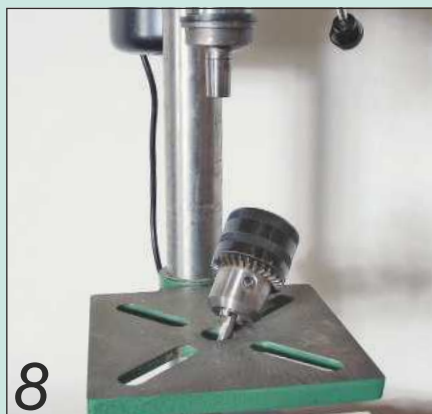
The chuck may fall out if adjusting it loosens the taper in the quill
