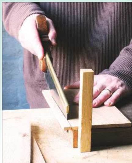
I could also rip a small board to width using a tall bench dog and a wood block
