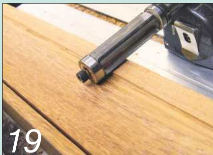
19 Replace the bearing and finish the trimming from the opposite side of the rail
