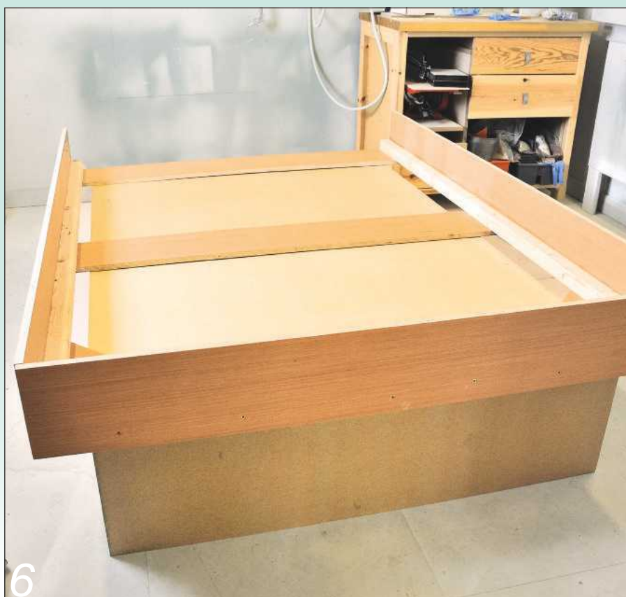
6 The mattress frame sits in top of the two base pods and overlaps them all round
