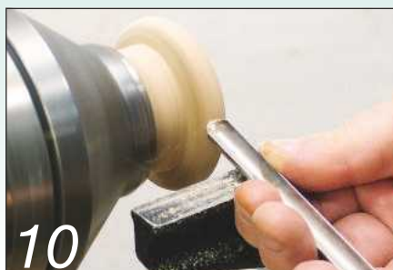
10 Next, turn a rounded bead on the remainder of the ring blank
