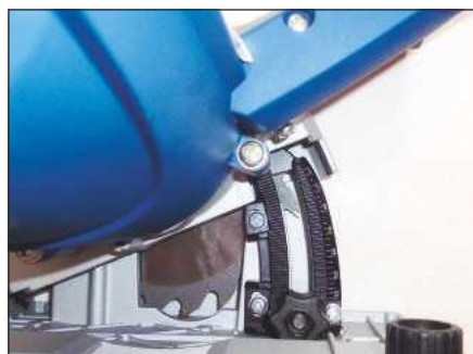
A clearly marked millimetre scale shows the depth of cut selected
