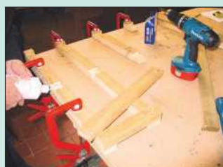
6 With all the legs cramped in place, apply plenty of glue and start to fix the rails
