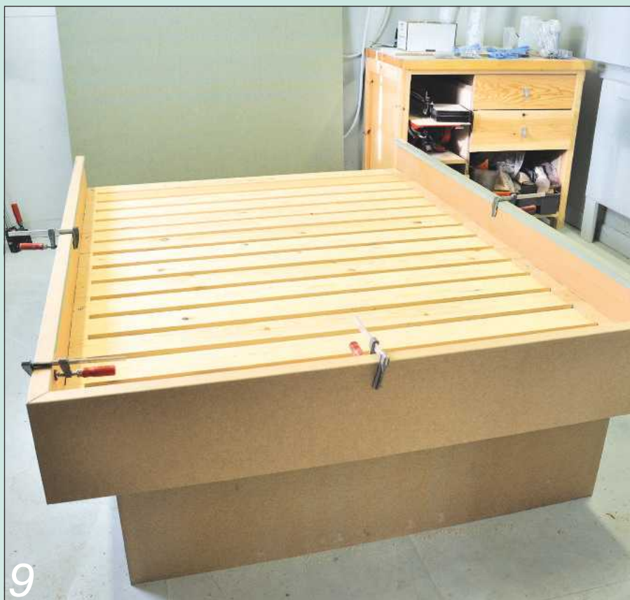
9 I then made mitred panels from 18mm mdf to fit over the plywood base sides
