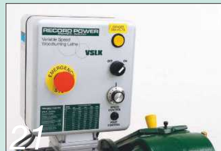
21 Modern electronic control offers infinite variation of speed
