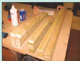
3 This is the finished stack of cut components, ready for the housing joints to be cut
