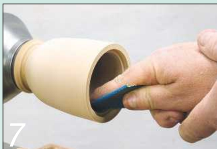
7 Sand the interior smooth, with just one finger holding the abrasive
