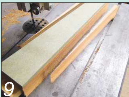
9 Cut away the waste wood on the bandsaw using the template as a guide
