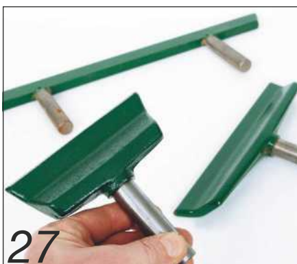
Toolrests are available in a range of different lengths; long ones need a second holder
