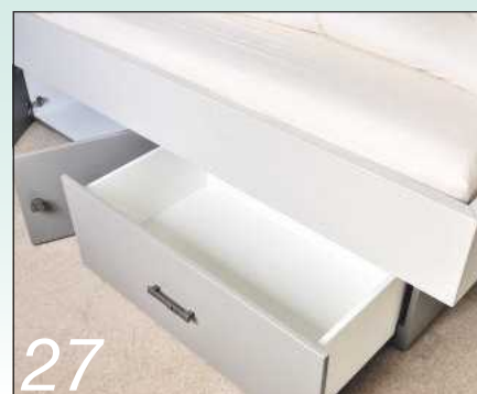
27 Finally, the doors and drawers were fitted in place and their handles attached
