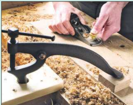
The holdfast mounted in the tool well eased the planing of small boards
