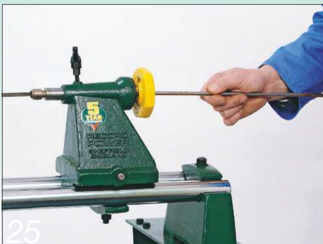
The barrel should be drilled through to allow for long-hole boring
