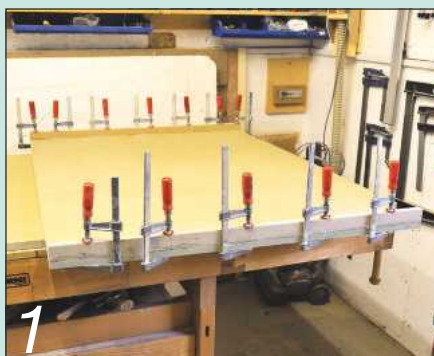
1 The top panels have a 30mm strip of mdf glued to each short edge to stiffen them
