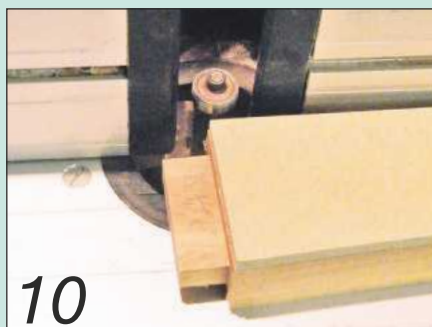
10 Then use the bearing-guided trimmer to give the slat a fine finish
