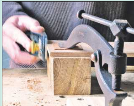
The holdfast and a wood block to raise the work combine for planing endgrain
