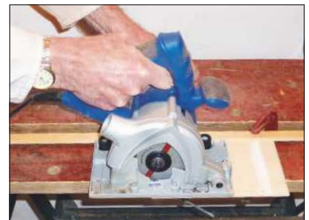
It also made a clean cut in a ceramic tile, cramped face down to minimise chipping
