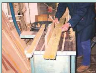
1 Some stock might need ripping down. Note that the saw guide has been removed here for clarity
