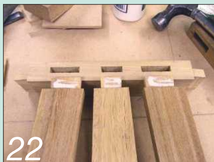
22 The three tapered table slats are glued in place in their angled frame
