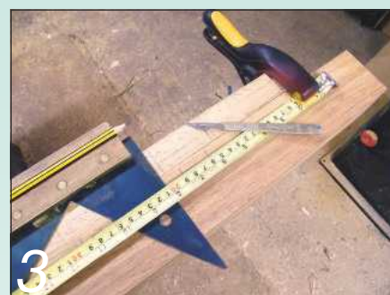
3 The back slats are tapered, so careful joint marking out is essential
