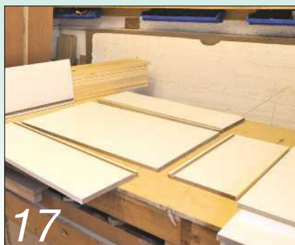
The drawers were made from 12 and 15mm thick melamine-faced mdf
