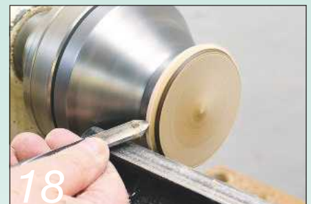
18 Turn the base down to the burnish line to ensure a good fit
