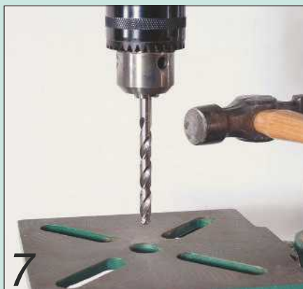
Tap the bit gently sideways with a hammer to align the chuck in the quill
