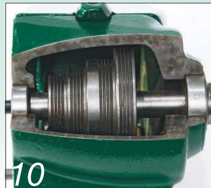
10 The bearings should be good-quality heavy-duty ball races
