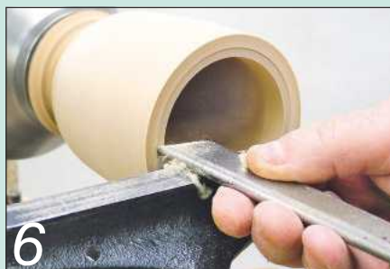
6 Cut a small step in the bottom of the body to receive the base
