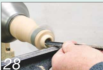
28 Take light cuts with a small spindle gouge to hollow out the bowl
