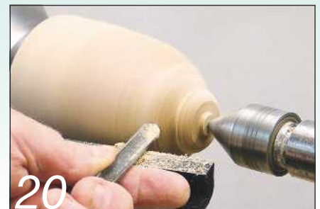
20 Finish turning the outside of the body using a \frac{3}{8} in spindle gouge
