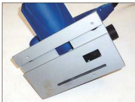
The underside of the soleplate has a groove for use with a guide rail
