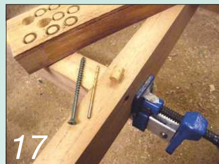
Screw the centre seat support rail in place and plug the counterbores
