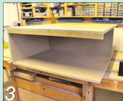
3 Each of the two base pods is assembled using biscuits to join the panels
