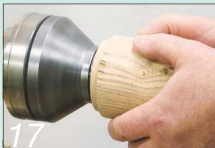
17 Offer up the body to the base and burnish a mark on the taper
