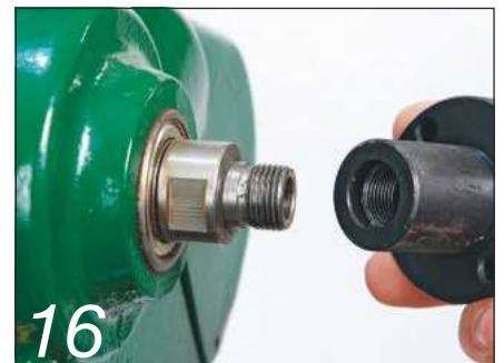
16 A spindle thread size of \frac{3}{4} in x 16 tpi is the industry standard
