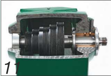
11 Tapered bronze-sleeved bearings give greater support than ball races
