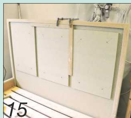
I clamped the small panels to the headboard before drilling mounting holes through the back
