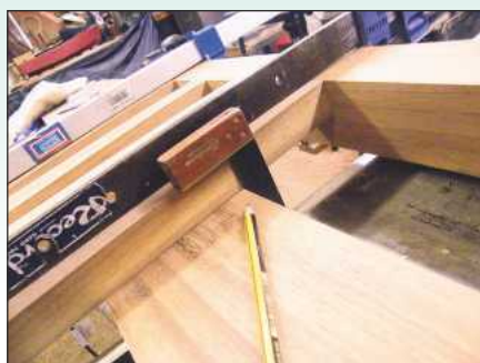
Use a try square to mark the location for the end of the mortise
