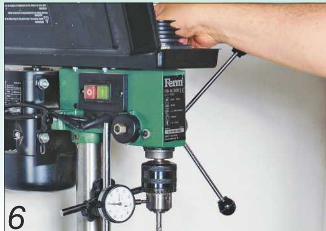
6 Rotate the chuck by pulling the drive bands by hand
