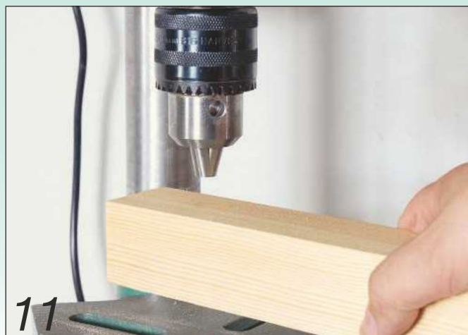
Give it a sharp blow with a block of wood to set it into the quill. Then re-check the alignment
