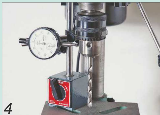
4 Use a dial gauge and magnetic stand to check the run-out
