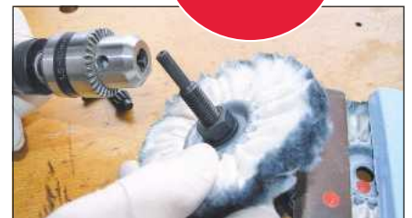
The standard 10mm diameter arbor fits through the hole in the mop
