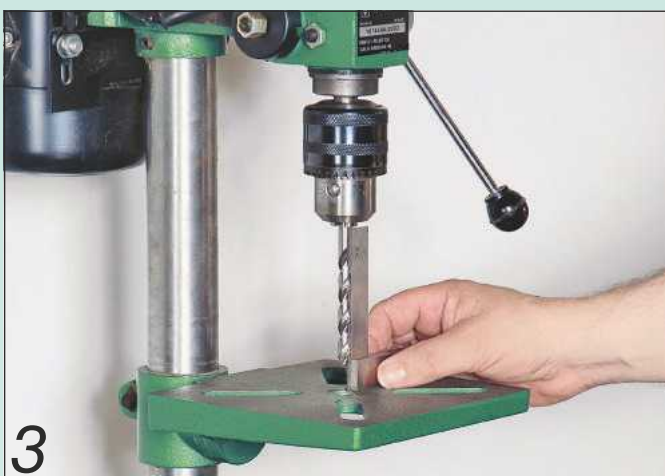
3 Use a square to check that the table is at 90° to the bit
