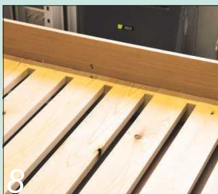
8 I glued small softwood blocks to the side rails between the slats to act as spacers
