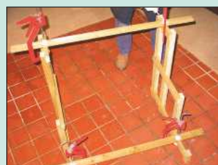
8 Cramp on a couple of slats as shown to help you space the end frames correctly
