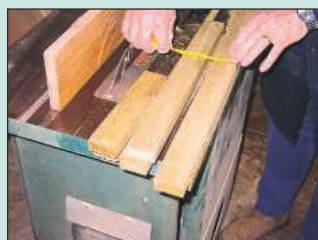
2 The rails should all be cut to the same width for ease of trenching later on
