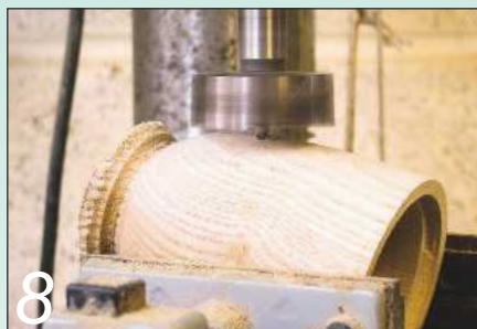
8 Use a 45mm diameter Forstner bit to drill a hole through the body
