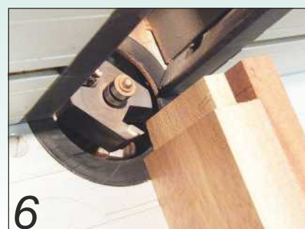
6 Then use a rebate cutter in the router table to cut accurate tenons quickly and easily
