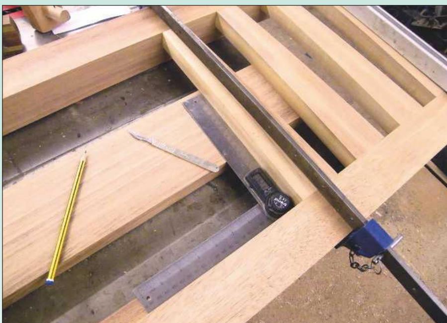
11 Use the angle of the slats to mark the cutting angles on the centre back rail
