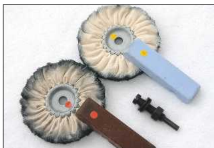
Each kit contains two or three polishing mops and appropriate compounds
