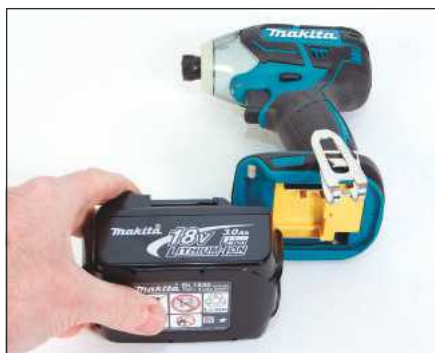
The battery slides onto the base of the tool. Any Makita 18V Li-ion battery can be used
