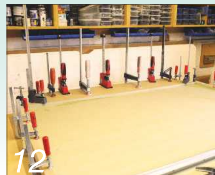
12 This support piece was then glued in place flush with the side mouldings
