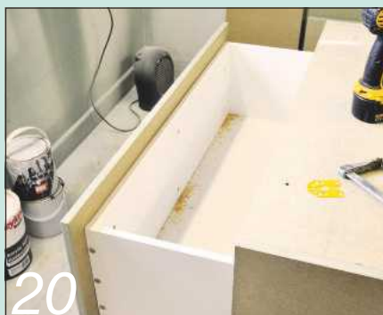
20 The plain mdf drawer fronts are simply screwed in place from inside the drawer box
