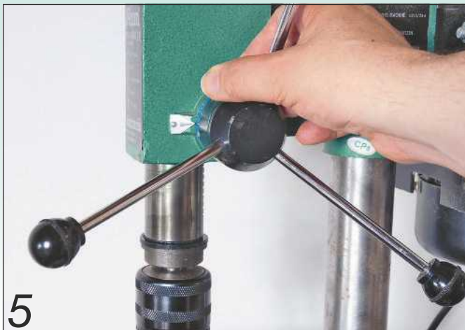
5 Use the depth stop to lock the quill in the down position
