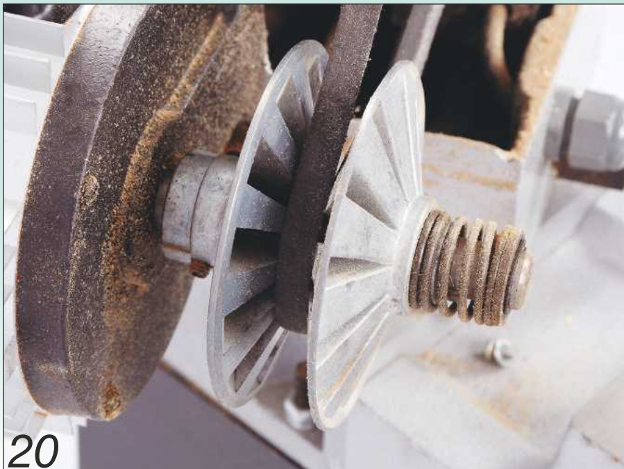
20 Some lathes use cone pulleys to change the lathe speed
