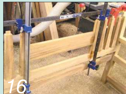
Glue the centre back rail and the two slats supporting its ends in place
