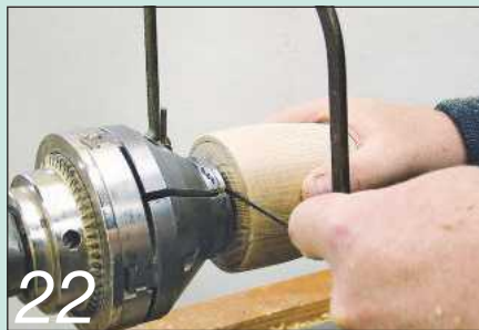
22 Partially part off the base spigot and finish the cut with a saw
