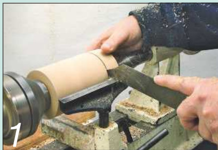
1 Turn spigots on both ends of the blank and part off the ring section
