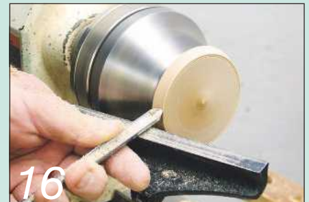
16 Turn a slight taper on the edge, at the diameter you've just marked
