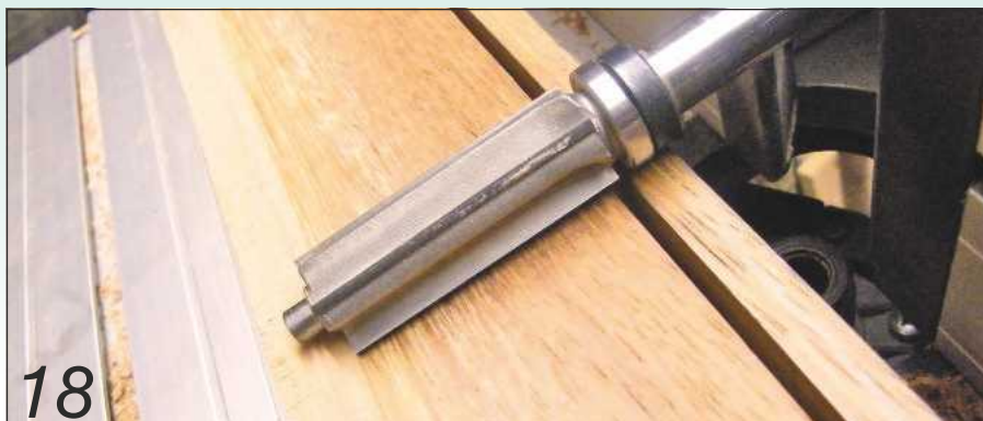
Remove the cutter's top bearing and trim the top rail before flipping it over
