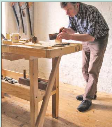
With diagonal braces fitted, the bench was rock solid for sawing
