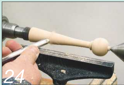
24 Turn the spoon handle using the same gouge and a skew chisel
