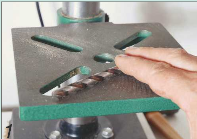
1 Check that the drill bit is straight by rolling it on the table
