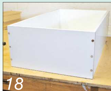
The simplest way of assembling the drawer boxes was to use Miller dowels
