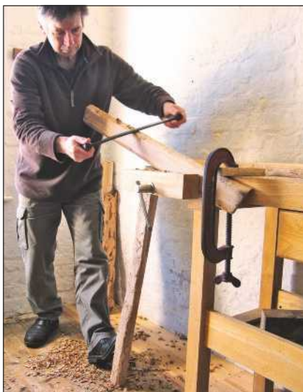
The bench brake was the ideal set-up for using a draw knife on a split log
