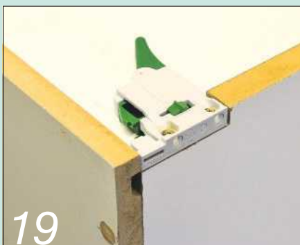
19 Undermount runners need a locking mechanism fitted into the front edge of the drawer
