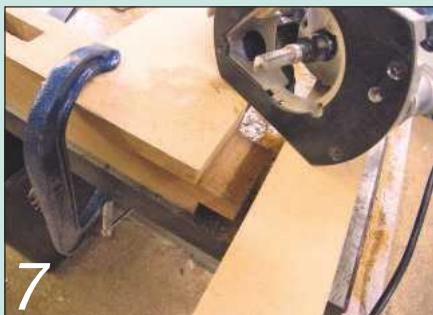
7 Note the use of the support piece of mdf to prevent the router tipping over
