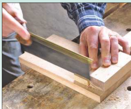
A well-made bench hook is invaluable for cross-cutting small stuff
