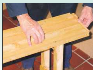
11 Space the intermediate slats by eye and use an offcut to make sure the ends are aligned
