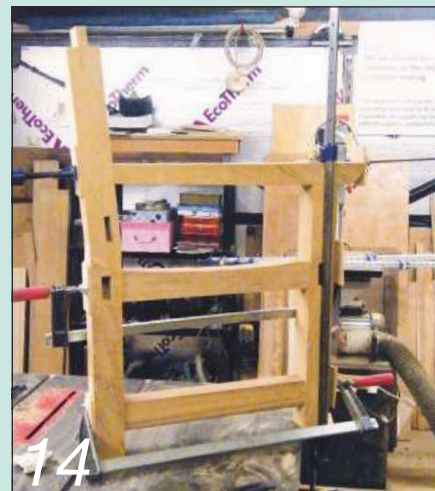
Glue the end frame components together using an exterior-quality adhesive
