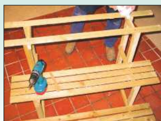
10 Add the inner slats to each level, gluing and screwing them on as before
