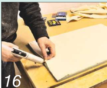
I glued three layers of curtain interlining to each panel, then stapled on the fabric cover
