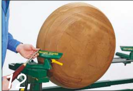
12 The headstock may have the facility to swing round through 90°
