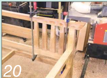
20 Glue and cramp the upper back rail in place; use softeners to protect the timber
