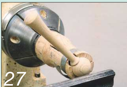
27 Mount the ball of the spoon in the collet chuck and spin it round
