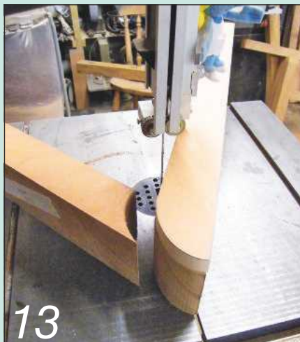
Make a template of the curve at the end of the armrest to aid cutting it to shape
