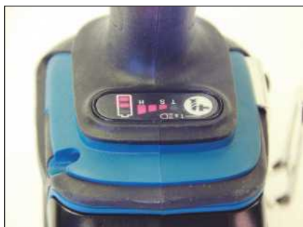
The battery level meter is located on the driver's control panel
