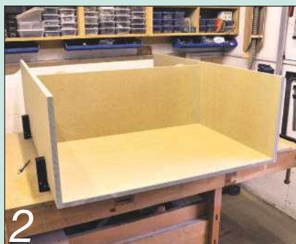
2 I fitted a central divider down the middle of each pod to stiffen the structure
