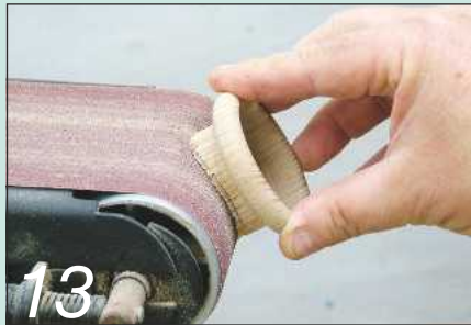
13 Shape the tenon on the belt sander to match the curve of the body
