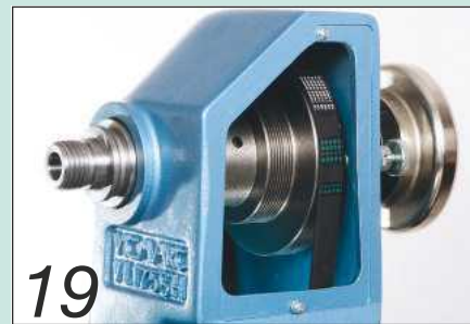
19 A three-or four-step pulley gives a speed range of 400-2000rpm
