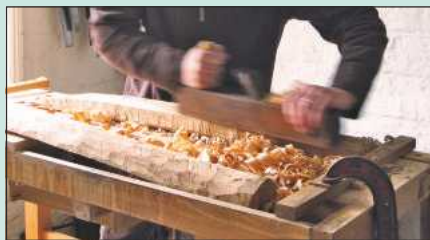
A planing stop clamped across the width facilitates planing a cherry brace
