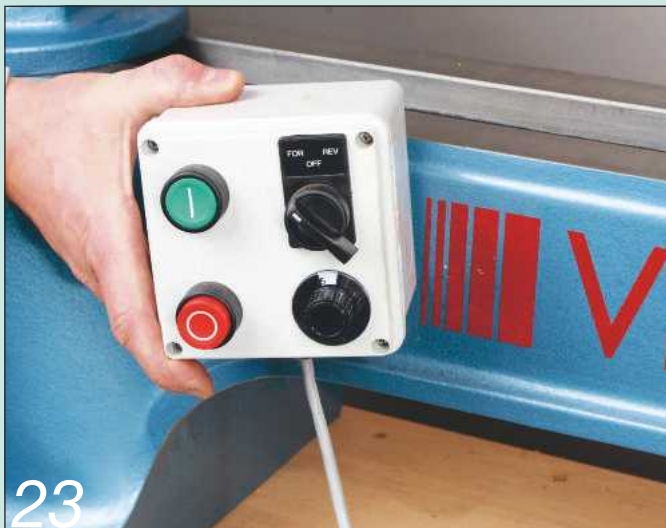
A magnetic switchbox can be fixed wherever you're working
