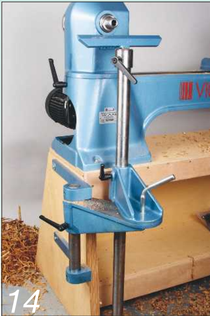
14 You'll need an additional tool rest for turning large-diameter bowls
