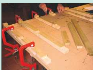
5 The first stage of assembly is to cramp a back leg to the bench top. Its square corner is a useful guide
