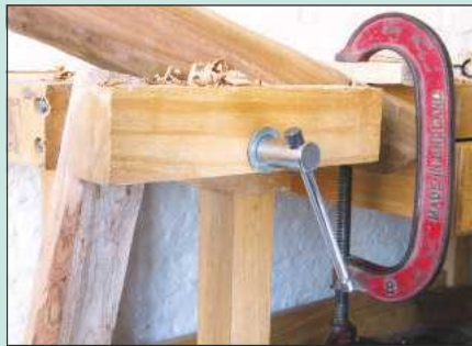
This close-up shows the workpiece held between the oak cross-bar and the elm leg
