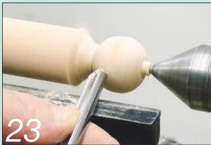
23 Turn the spoon blank to a cylinder and form a ball on one end
