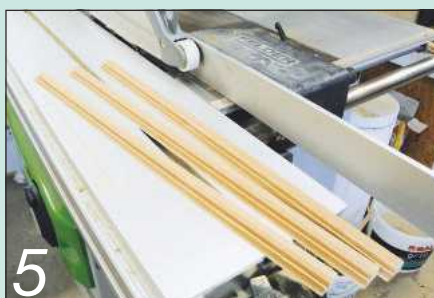
5 ... and then cut the machined board down to the width I require on the table saw
