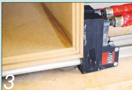
3 The corners need to align perfectly; otherwise the back panel will not sit flush
