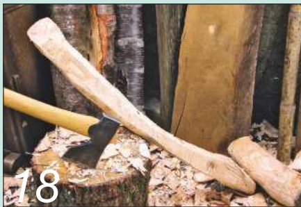
18 Hewing an S-shaped ash log gradually yielded the approximate shape of an adze handle
