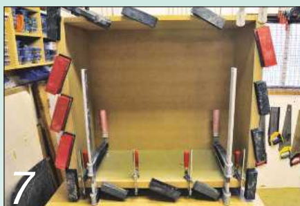
7 After fitting the back, I glued a piece of 18mm thick mdf into the base of the carcass
