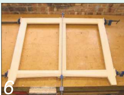
Use sash clamps while the glue dries
