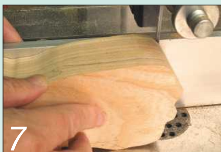
7 Rip the bottom off the blank on the bandsaw and set it aside
