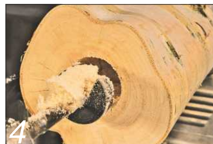
4 Use a large-diameter sawtooth bit to bore out the centre of the log
