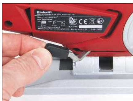
A lever on the side of the body releases the adjustable soleplate
