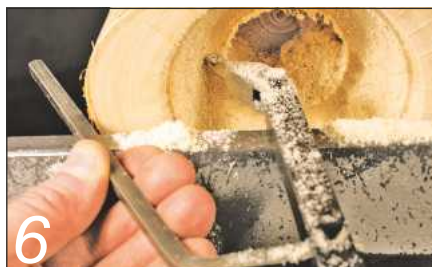
Option 2: hollowing the log with the BCT Versatool Hollowing System
