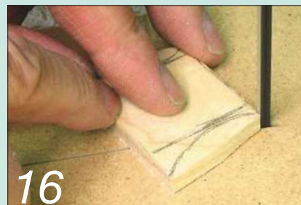
16 Carefully bandsaw out the pieces. A light touch on the sander will smooth the show edges
