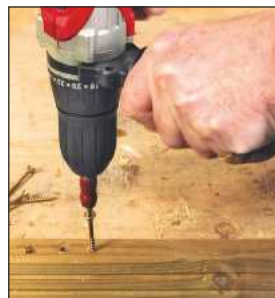
The tool is a competent screwdriver, thanks to 22 torque settings
