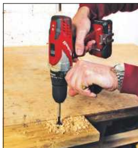
The drill happily bored large-diameter holes in wood and man-made boards
