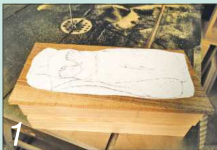
1 Stick the block and the motif pieces together, then stick the paper pattern to the top layer
