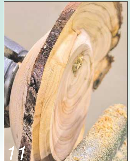
Before completing the hollowing, cut the rim to give an even wall thickness
