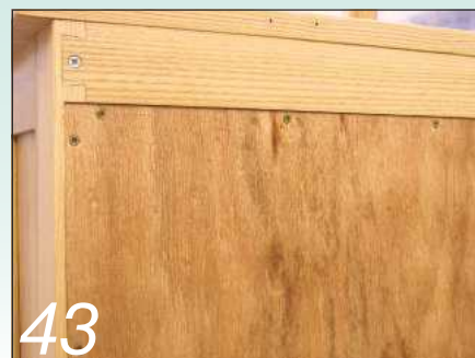
43 Finally, the two plywood back panels are screwed into their rebates
