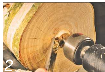
2 Slice one end of the log flat with a gouge or parting tool
