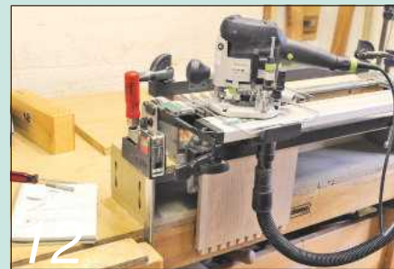
12 My Leigh jig is invaluable for repeat cutting of perfectly spaced dovetails
