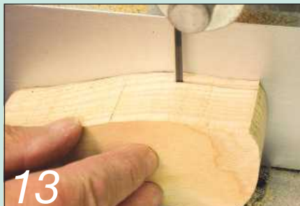
13 Rip off two 4mm thick pieces from the top of the 'waste'
