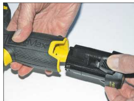
The slim Li-ion battery clicks neatly into place inside the handle
