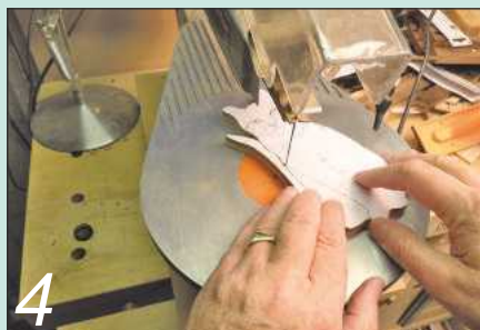
4 Remove the thin motif pieces and cut off the tail – best at the scrollsaw or with a hand fretsaw
