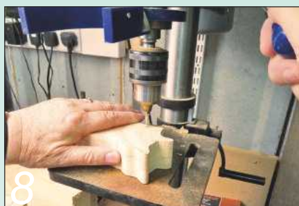
8 At the drill press, drill two 3mm holes through the main blank to ensure accurate positioning
