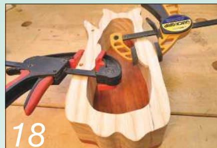
18 Glue the side-grips back in the position from which they came
