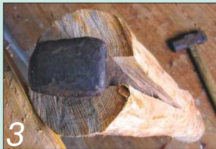
3 I start by using a wedge to split an elm log in half... and perhaps into quarters
