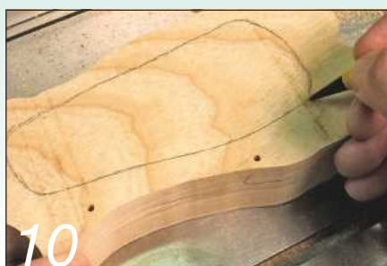
10 Sketch out the approximate shape of the internal compartment
