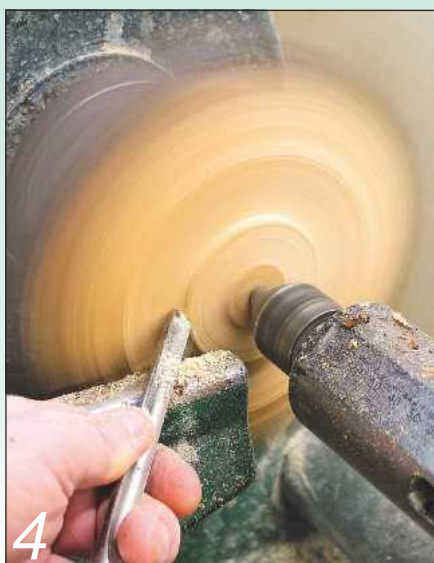
4 With the blank held between centres, start by cutting the chucking spigot
