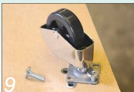
9 I used insert nuts and matching M6 bolts to mount the castors securely
