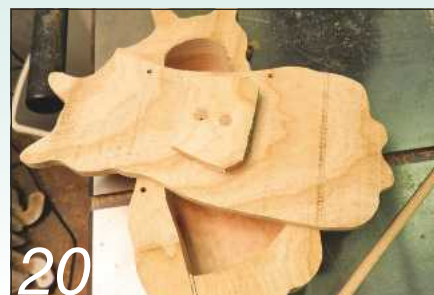
20 When the glue has dried, remove the lid and secure the pieces permanently with dowels
