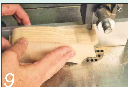
9 Now separate the lid on the bandsaw in the same way as you cut off the bottom
