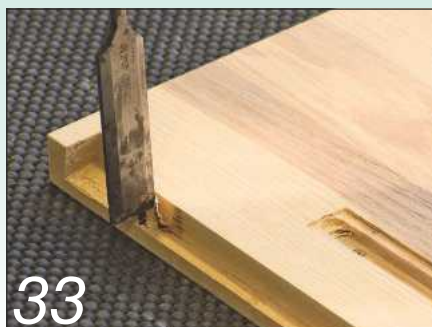
33 Form a stopped rebate for the rear panel
