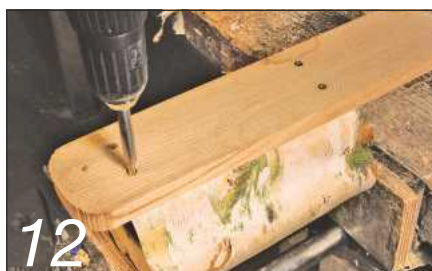
Cut the back plate to size and screw it securely to the back of the box
