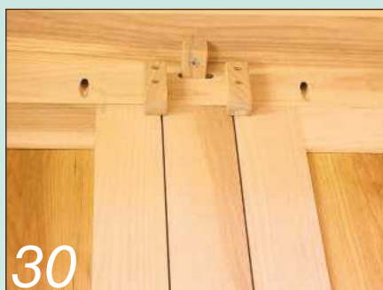
30 The stop block and door catches are installed
