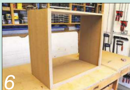
6 The face frame is fitted to three edges at the front of the carcass
