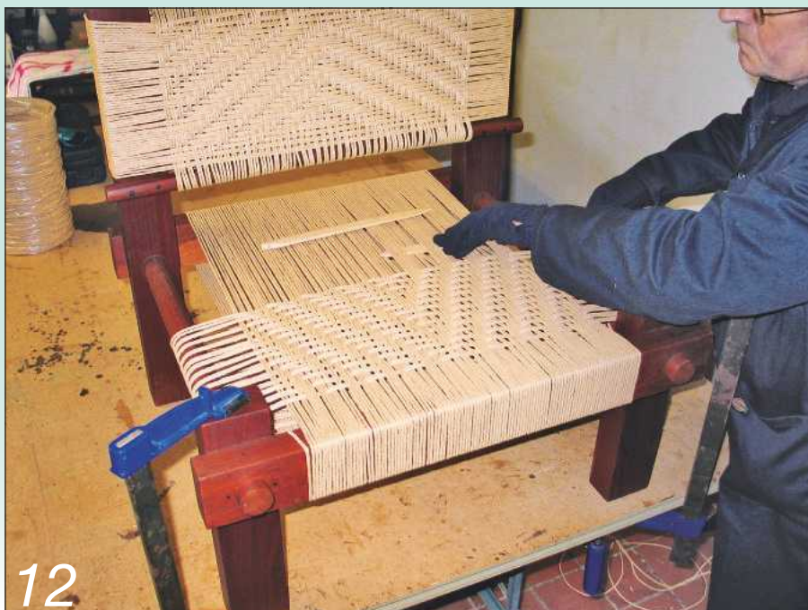
To weave the seat pattern, I started at the front and worked backwards, using my maple needle
