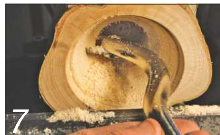
Option 3: working with the swan-necked Hollowmaster; note the long overhang
