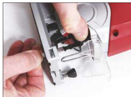
The tool-less blade change mechanism was a little stiff to operate
