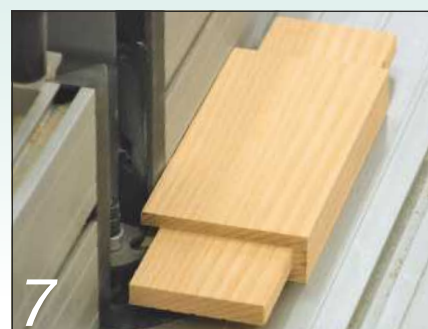
Cut grooves in the side frames for the panels
