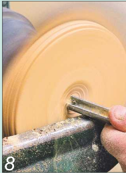
Start to hollow the bowl by cutting with the grain, just like hollowing a box
