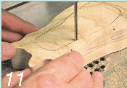
11 Feed the blade into the timber in the internal corner near a foot, and cut away the 'waste'
