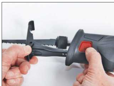
The machine foot can be released for adjustment by pressing this red button
