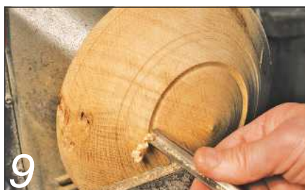
Use a bowl gouge to form the conical slope to the bird box roof
