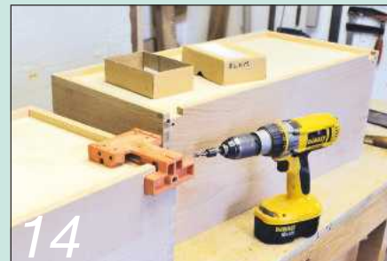
14 This Blum jig allows accurate drilling of the various mounting holes for the drawer runners
