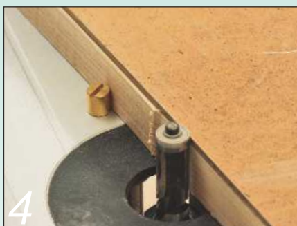
The arched rail is trimmed to a template
