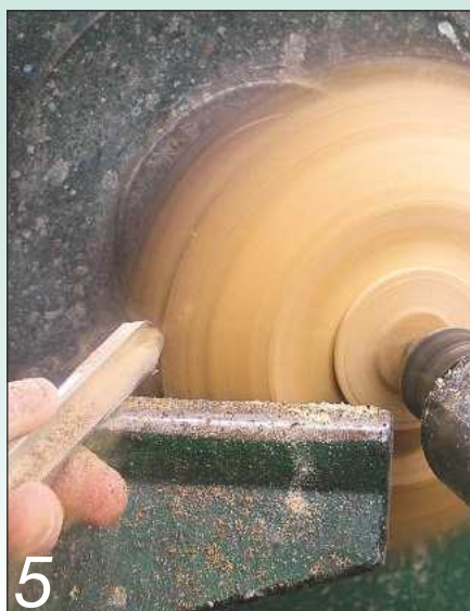
5 Change to a larger bowl gouge to shape the outside of the blank
