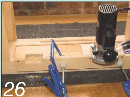
26 I cut the hinge recesses with a router and jig
