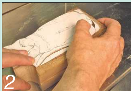
2 Bandsaw round the outline, keeping just a tad shy of the line
