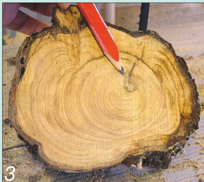
3 This section of rot near the pith will need the superglue treatment later
