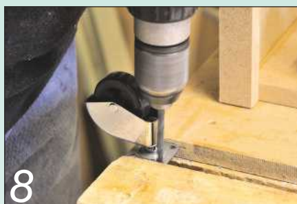
8 The mounting holes on the castor base plates needed to be enlarged
