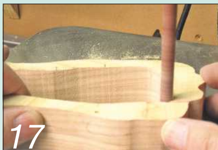
17 Bobbin-sand the cavity. Be careful to maintain the contour where the side-grips will fit
