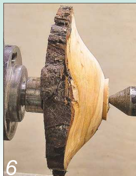
6 Cut an S-shaped curve on the underside, finishing up with a shape shown
