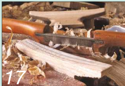
17 I've also made larger cleats from elm, dishing the tops of the horns with the spokeshave
