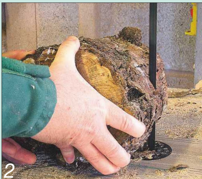
2 I was able to cut a similar unpromising piece of Leylandii on the bandsaw
