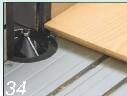
34 Chamfer the top along its front and side edges
