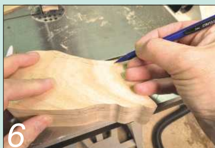
6 On the carcass, plot the positions of the two dowel holes at the widest points along the tail
