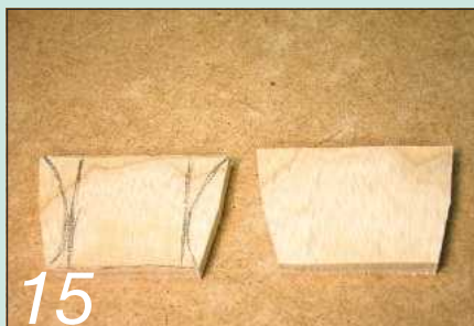
15 Left: the side pieces and boss. Right: the slider that will hold the lid in place
