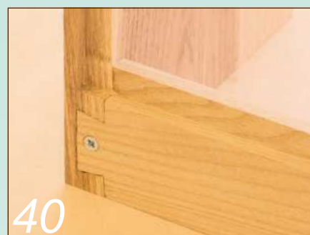
40 The upper unit's rear rail is held tight with a screw driven through the dovetail
