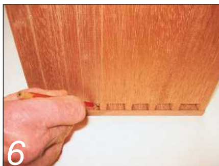
Mark the sockets on the chest sides directly from the dovetail pins
