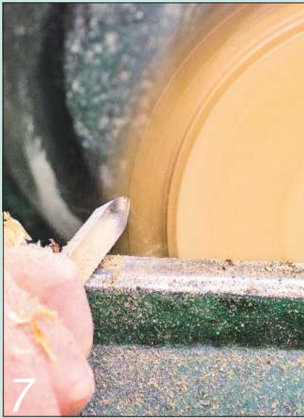
Use a small fingernail profile gouge to clean up the face of the bowl
