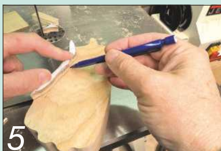
5 Draw carefully round the outline of the severed tail onto the blank
