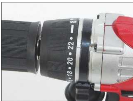
The torque ring is clearly numbered, but was rather stiff to turn
