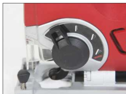
This large lever is moved to select the required pendulum setting
