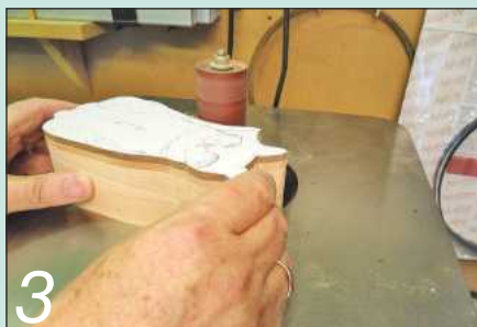
3 Sand back to the line. You'll need a small bobbin or drum for some of the nooks and crannies
