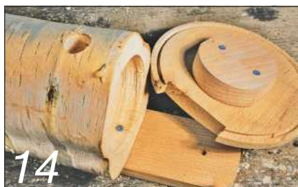
Cut a notch in the edge of the roof and fit it in place on the box
