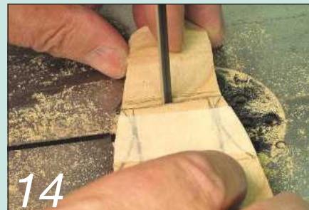
14 Tape the two pieces together and cut out the middle section
