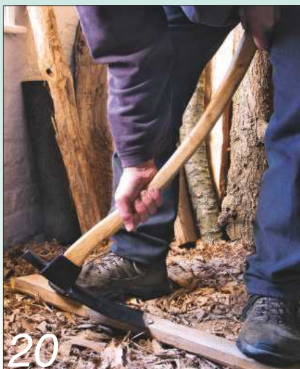
20 The adze was soon restored to use with its new handle, here working on a piece of elm
