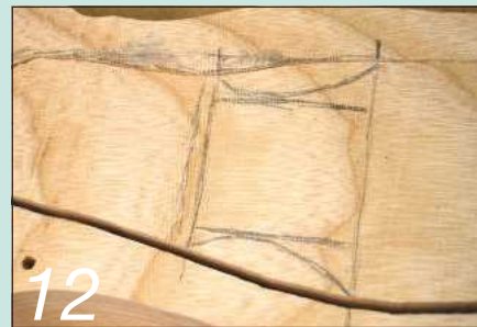
12 The 'waste' will provide the locking device. Mark on the top the outline of the side grips and the boss
