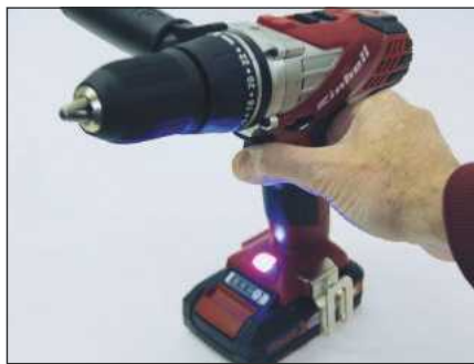
The bright LED work light in the base shines up towards the chuck
