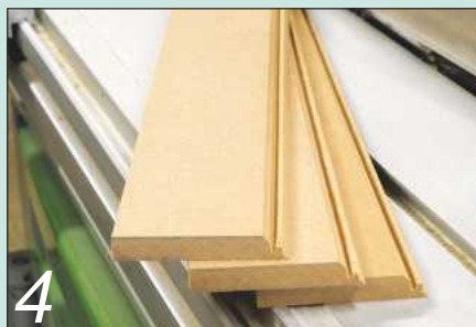
4 When I need a narrow strip, I always rout the moulding on a wider board first...
