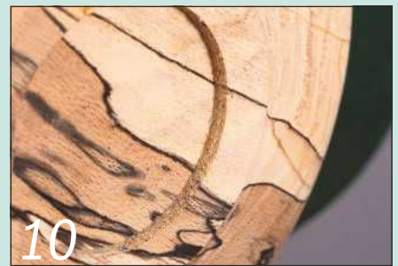
10 Even a sharp parting tool will leave somewhat ragged edges to the recess...
