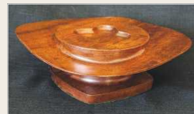
Image B is a piece of sapele 210mm square and 70mm high. This shows that the effect of the cam can be cancelled, with the lathe returning to circular cutting.
