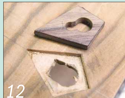
Use a small router cutter to form the recess and finish it with a chisel
