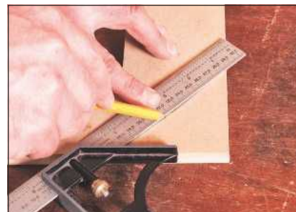
3 Bring the components together and mark the biscuit position across the joint
