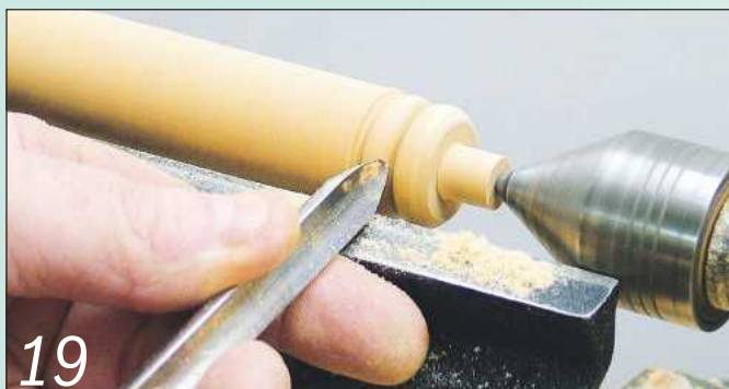
19 Begin shaping the handle with a few decorative beads next to the tenon
