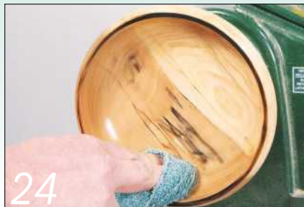
24 Wax the interior once more and buff it up to a soft natural sheen with a soft cloth
