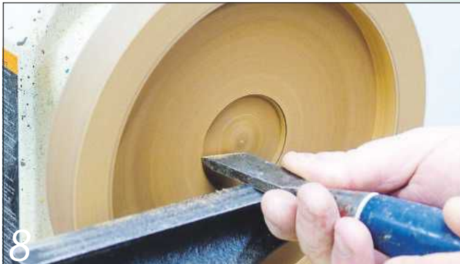
8 Cut a smaller dovetailed recess in the middle to fit the jaws of your chuck
