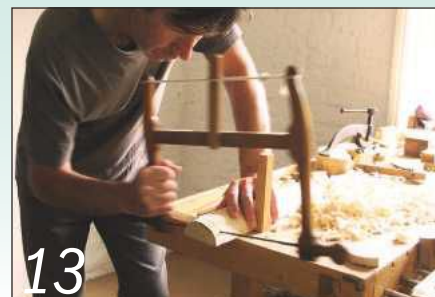
13 The saw is good for green woodworking too. I use a one-handed grip and a tall bench dog for support
