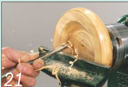
21 Start turning out the inside of the bowl with light, gentle cuts...
