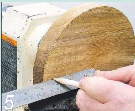
5 Mark the diameter of the mirror on the face of the piece with a pencil
