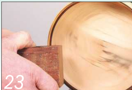
23 I charred the bowl's rim lightly for contrast by holding a block of hardwood against it
