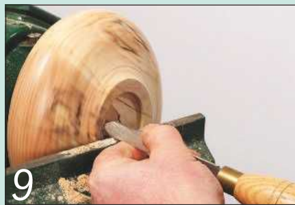
9 Cut the chucking recess to match the diameter of your chuck jaws
