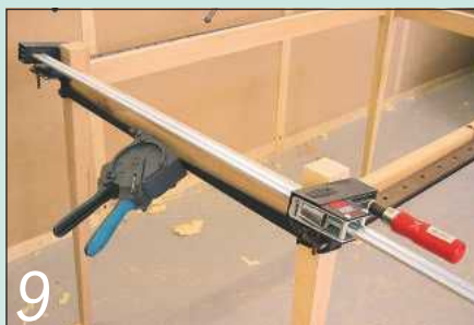
9 This excellent WolfCraft band clamp made all the difference during the glue-up
