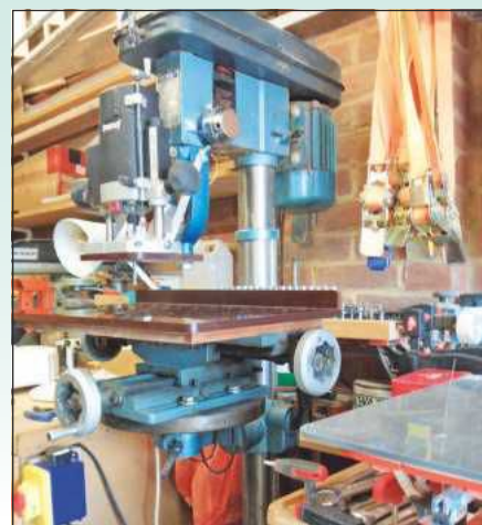
9 The finished overhead router is the culmination of many years development, and is a joy to use!
