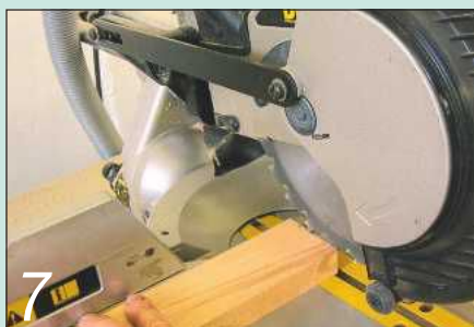
7 You can now make the final angled cut on the rail, removing only the absolute minimum
