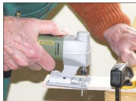
Thin workpieces must be securely cramped to the workbench to reduce vibration
