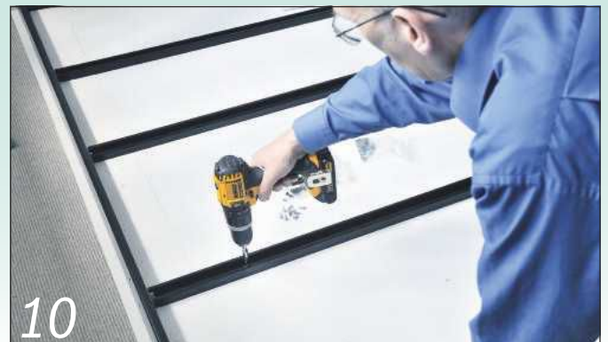
10 ...but I had to buy some shorter screws that wouldn't penetrate the face of the panel to fix the cross braces in place
