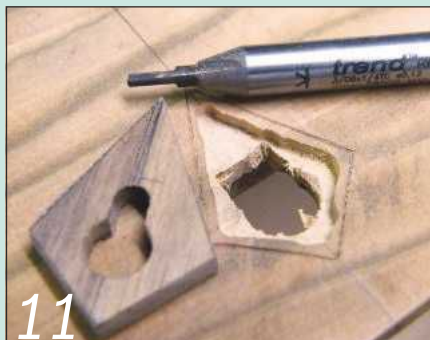
Mark out the escutcheon, cut it to shape and create the keyhole cutout in it
