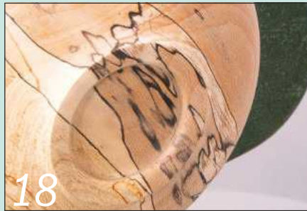
18 In sanding the bowl, I inadvertently rounded over the edges of the chuck recess!
