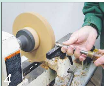
4 Then true up the edge using the same gouge, but this time with a push cut
