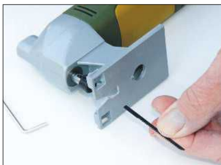
The blade is inserted into the head and locked with a small hex grub screw
