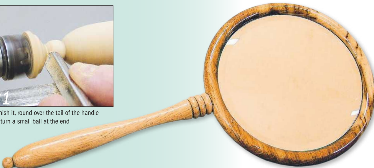
19 Begin shaping the handle with a few decorative beads next to the tenon
