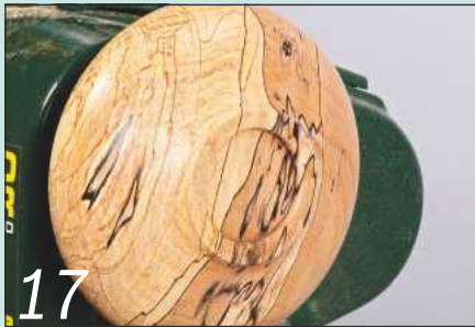
17 Repeat the sanding and sealing process several times to get a clean surface
