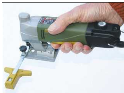
The fence is secured with two screwed knobs and is held reasonably firmly
