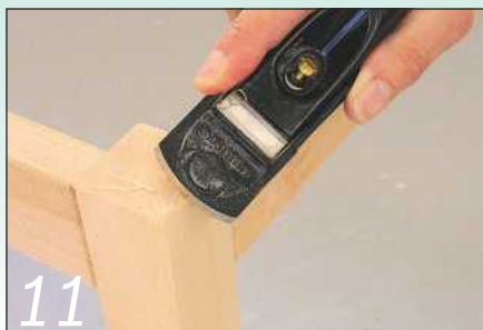
11 ...and the new cut edges chamfered gently with a small block plane to match the rest
