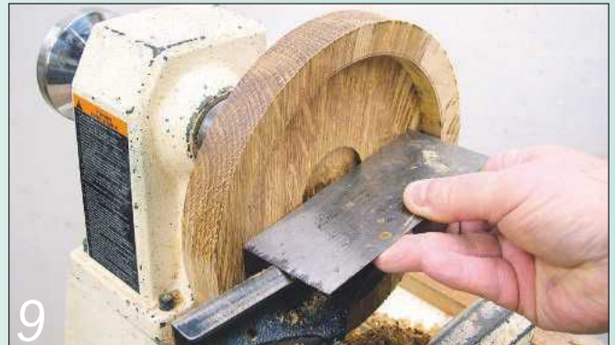
9 Check for flatness with a straightedge; I used a small cabinet scraper
