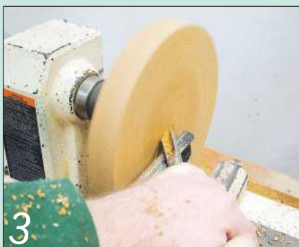
3 True up the top surface using a pull cut with a fingernail profile gouge
