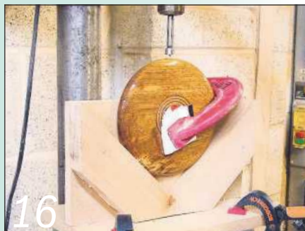
16 This simple home-made jig holds the workpiece truly vertical for precise edge drilling
