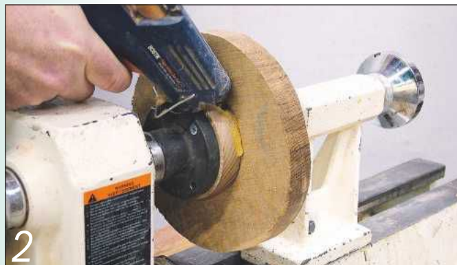
2 Stick the frame blank to a scrap wood disc screwed to a faceplate
