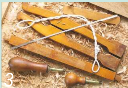
3 The bow saw can be dismantled in a few seconds for transport or storage
