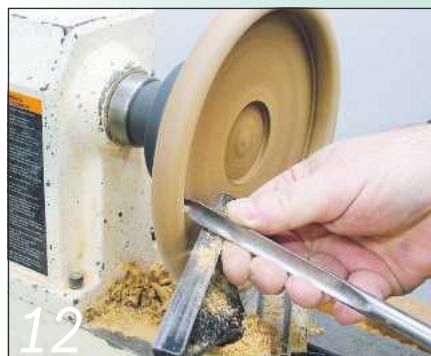
12 Continue the curve to round over the top of the recess using a pull cut
