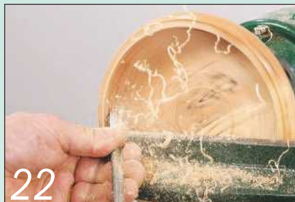
22 ...and don't be tempted to cut the walls of the bowl too thin; they may crack
