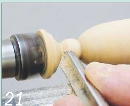
21 To finish it, round over the tail of the handle and turn a small ball at the end
