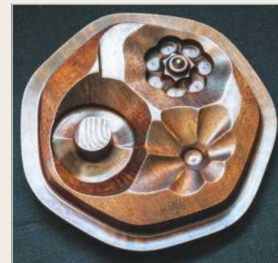
Image C features a piece of mahogany that has been shaped using random settings together with a seven-sided cam, also utilising the compound slide facility on the primary faceplate.
