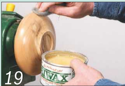
19 After sealing the outside of the bowl, apply some pastewax with a small pad of steel wool
