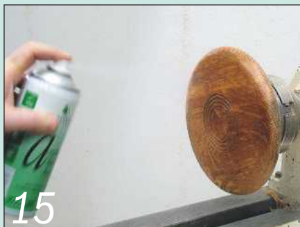
15 Turn the lathe at a very low speed or by hand when spraying on a lacquer finish
