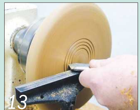
13 Cut a few decorative beads at the centre using a skew chisel as a scraper
