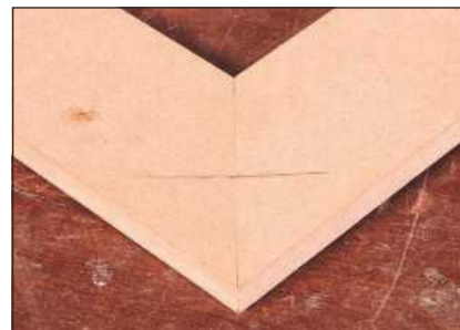
6 Glue the mating surfaces of the components and bring the joint together: perfection!
