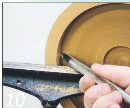
10 Undercut the edge of the recess a little to allow for movement of the wood
