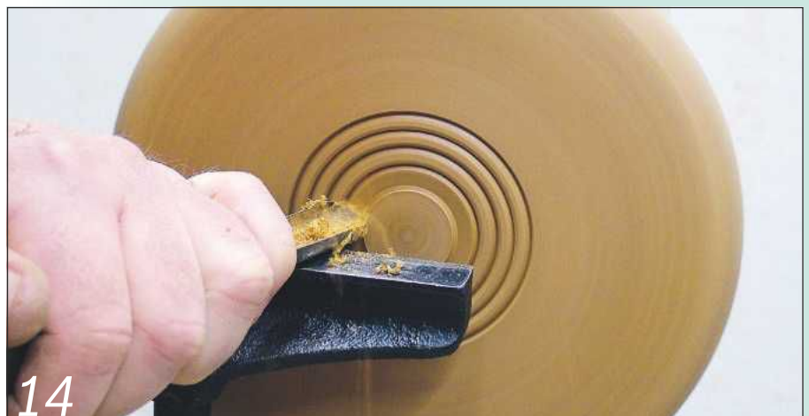
14 Then slightly dish the middle to stop the mirror rocking when it's put down on the dressing table
