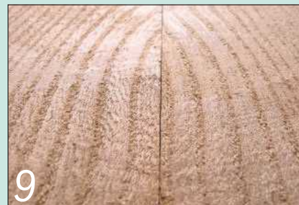
9 The resawn boards are book-matched, and are shown here after initial clean up
