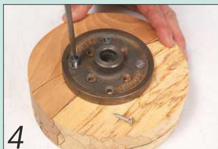
4 If the blank appears soft, use a faceplate and attach it with plenty of big screws
