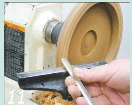
11 Now shape the rim. I opted for a simple curve cut with a spindle gouge
