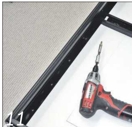
11 Access to the screws was awkward in places; using two hex bit holders in line helped
