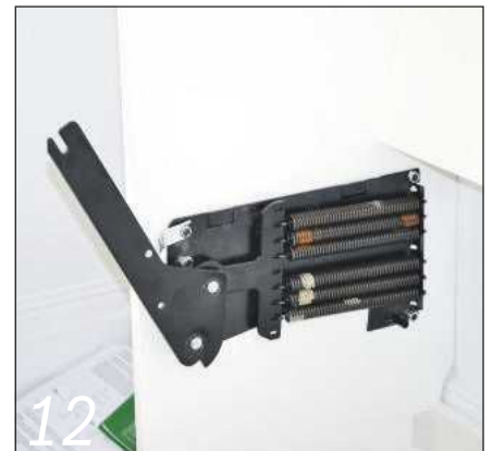
12 Once the metal frame was attached, the short arm of the lift mechanism was angled forward
