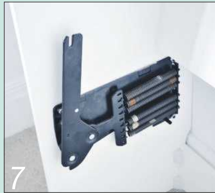
7 The number of springs counterbalances the weight of the mattress and panel
