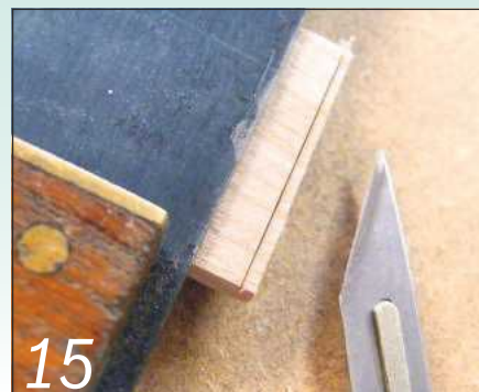
Use a sharp knife to score a line on each piece where the mitre will be
