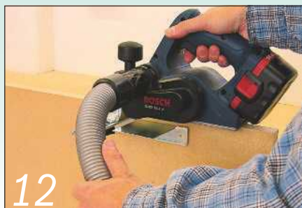
12 Plane the edges of the MDF top perfectly square, ready to take the lipping
