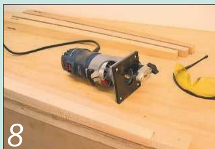
8 With all the parts machined, apply the chamfer to the edges with a palm router
