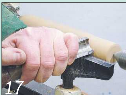
17 Mount the handle base between centres and turn it to a cylinder
