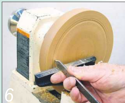
6 Use a parting tool to cut a groove just to the right of your pencil mark
