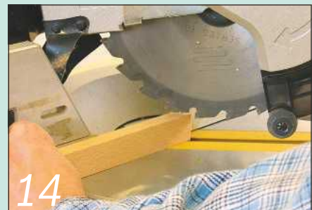
14 Mitre the lengths of edge trim carefully to fit round the perimeter of the top
