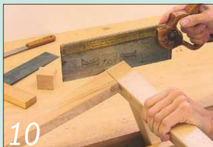
10 Once the frame is ready, the leg-tops can be trimmed flush with the side rails...
