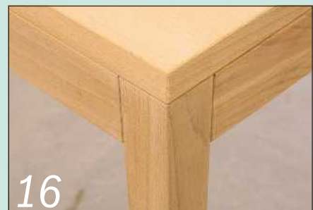
16 Match the edges of the table top with the chamfer on the outer corners of the legs
