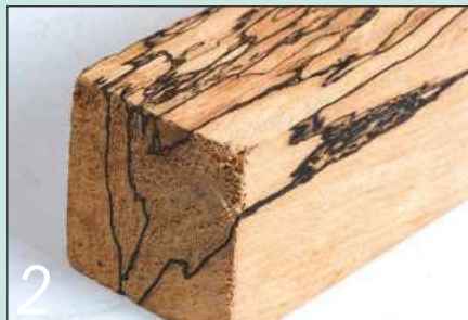
2 Even with the sharpest tools, little patches can be plucked out to quite a depth
