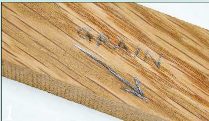
1 Avoid this type of short grain. The grain should run the entire length of the handle
