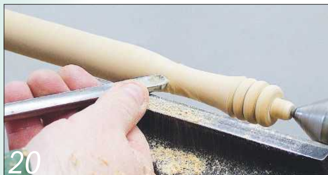
20 Then create a smoothly flowing curve along the rest of the handle
