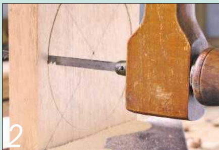
2 Although the teeth have a rip profile they must cut both with and across the grain when sawing curves
