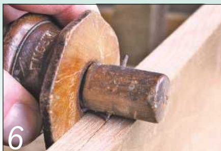
6 Mark a half-thickness line round the edge of a small board with a gauge, ready for resawing
