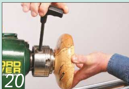
20 Make sure you reverse the work back onto the chuck perfectly square
