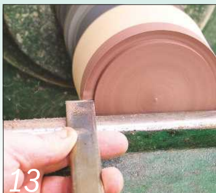
13 Use a skew chisel to cut a tenon that will be a tight fit inside the bowls
