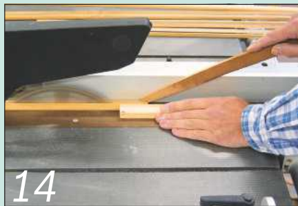
14 Cut the door panel mouldings on the table saw; note the push stick
