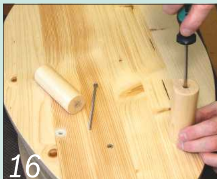
16 Assemble the stand by screwing the bolts into the adjusters, and check that the legs are vertical
