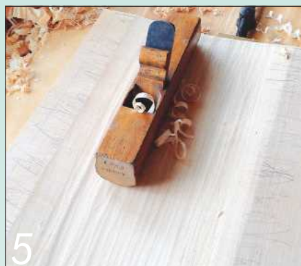
5 ...but this antique plane with its tight radius really scooped out the waste
