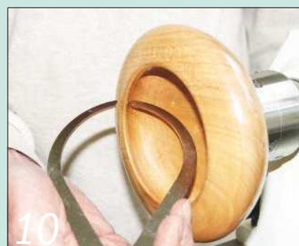
Check the wall thickness as you work. Aim for a final 6mm thickness
