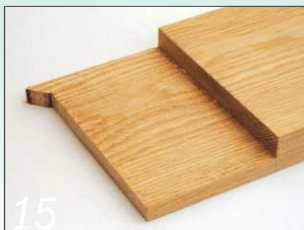
Then carefully clean the face with various planes. The bottom rail has the same shape, but the rail itself is much thinner to allow the vertical cladding to run in front of the rail
