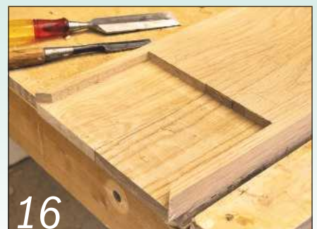
I cut the corresponding half-lap joints in the two stiles which have been temporarily clamped together. This time I used a router to remove most of the waste
