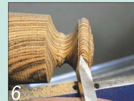
6 Round off the rim of the knob by rolling a parting tool over from side to side
