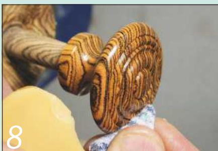
8 Sand the knob as smooth as possible, then apply shellac polish and wax
