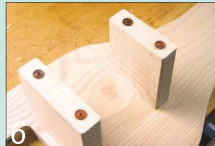
6 Drill dowel holes in the ends of each seat support. Use dowel pins to mark the seat
