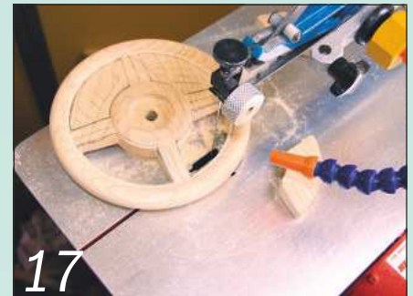
Turn the steering wheel to size, mark out the spoke positions and cut away the waste
