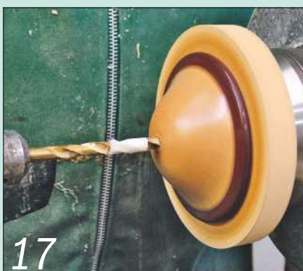
17 Drill a hole 8mm in diameter in the centre of each lid to take the handle
