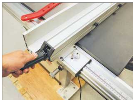
A large paddle lever locks the fence securely in the selected position
