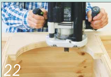
22 Rout the edges square with the arch jig and a bearing-guided cutter
