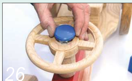
Glue the steering wheel cap in place over the locknut and fix the boot tray behind the seat
