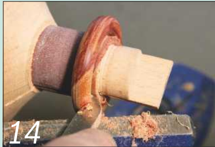
14 Then reverse the ring on the mandrel chuck to complete the other half
