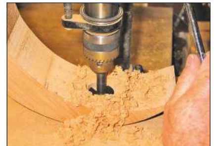
4 Drill the hole into some scrap wood. Final cleaning up will take away any breakout
