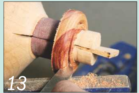
13 To form the ring, first scrape one side carefully with the ring scraper
