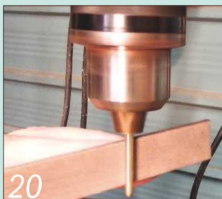
20 The brass rod for the pivots may need to be filed down in diameter for an easy sliding fit
