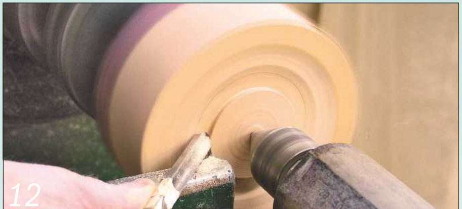
12 ...while you turn a chucking spigot on it. Take only very light cuts
