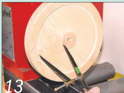
Mount the blank and turn a 5mm deep recess starting 20mm in from the wheel rim
