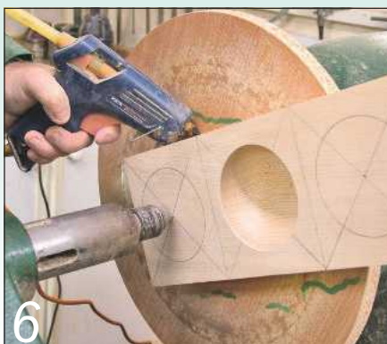
6 Use the tailstock centre to align the second bowl and glue it in place
