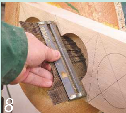
8 Use a profile gauge or a shaped cardboard template to check the bowl profile
