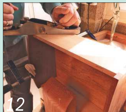
...before being cleaned up and the dovetails flushed down with a sharp plane
