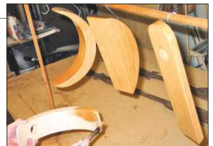
6 Seal the surfaces and hang them up to dry before applying the wax
