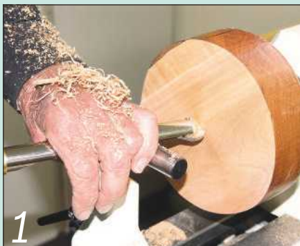
Face off the blank with the flat side of the shank resting on the toolrest
