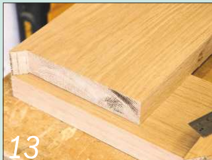
One advantage of laminating the frame is that the tenon doesn't need to be cut through the stile; here I've cut the top rail where it will be fitted into the stile in a modified half-lap joint
