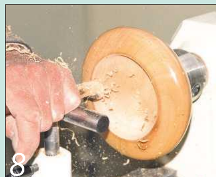
Carry on shaping and smoothing the inside of the bowl in the same way
