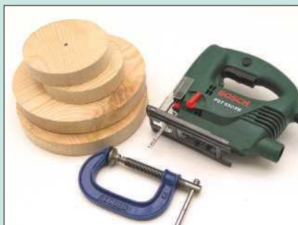
Draw out the wheel blanks, cramp them to your workbench and cut them out using a jigsaw
