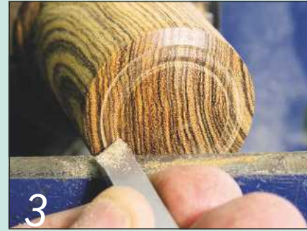
3 Form the section that's left between the two cuts into a rounded bead
