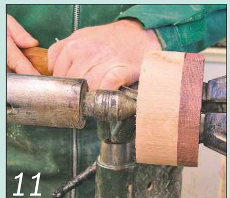
11 Use tailstock pressure to hold the blank against the open chuck jaws...
