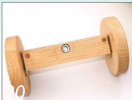
Assemble the fork with a dowel through each joint. Then drill a hole and glue in an M10 nut
