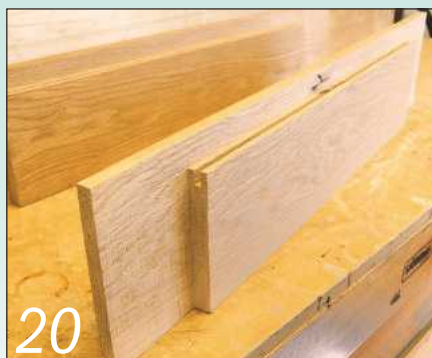
20 A deep rebate in the external face of the two top rails will allow me to screw the vertical boards in position. The final stage is to cut a groove round the inside edge of the frames to house the vertical boards
