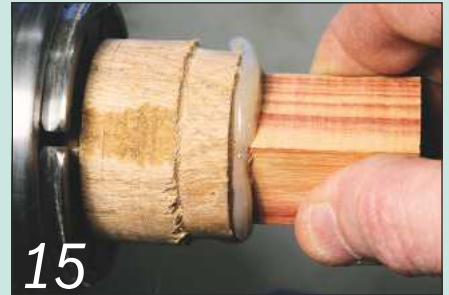
15 Stick the ring post blank to a cone chuck with a large blob of hot-melt adhesive
