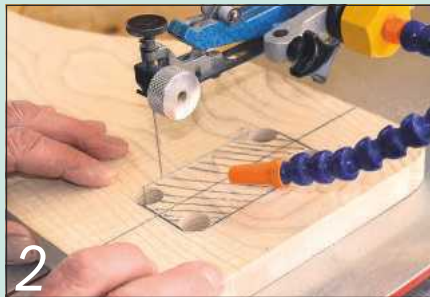
2 Cut out the waste using a scrollsaw if you have one. Use a jigsaw or coping saw otherwise
