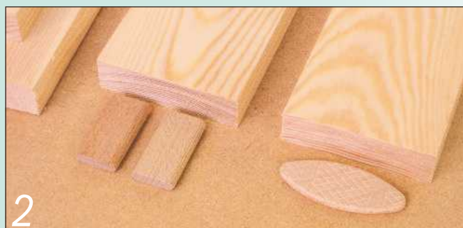
Dominoes are more suitable than biscuits for joining carcass rails
