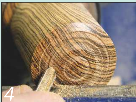
4 Complete the ogee moulding with the point of a 1/4 in spindle gouge
