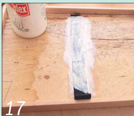
17 Before lining the tray, I stuck a looped length of ribbon to the base to provide a finger grip
