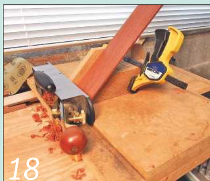
18 I mitred all the ends of the box linings using my birdhouse jig and a shooting board
