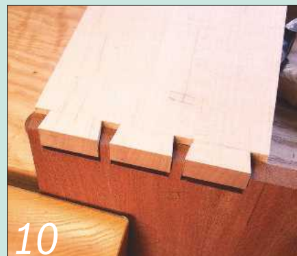
I tried a half-way test fit next. Never push dovetails fully home as this spoils the joint
