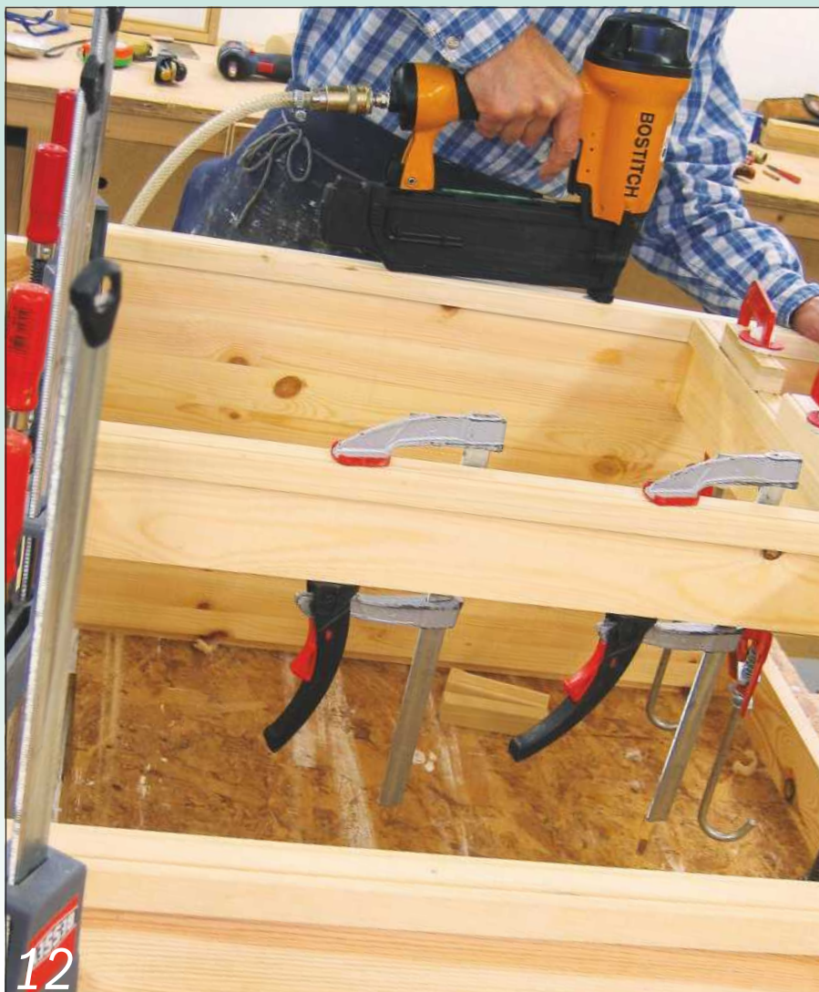
12 The assembled frame is glued, biscuit-jointed and pinned in place
