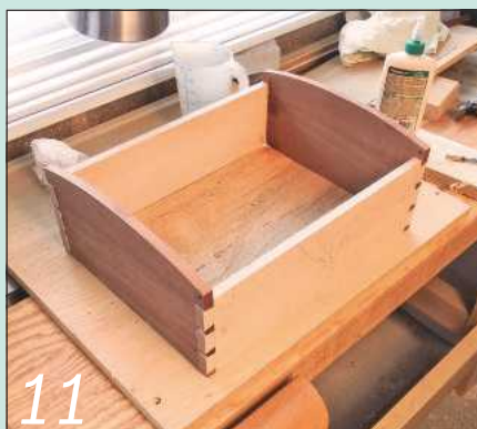
After glue-up and assembly, the box was left on a flat surface to dry...
