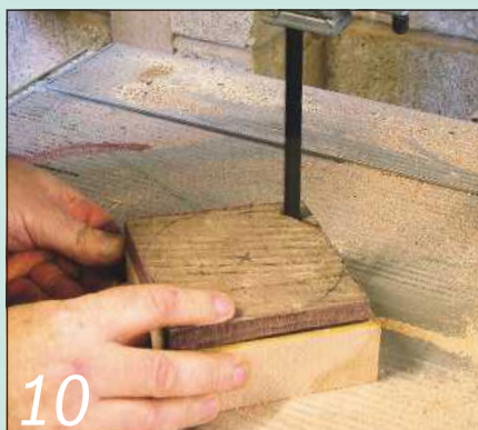
10 Cut the three laminated lid blocks to a circular shape on the bandsaw
