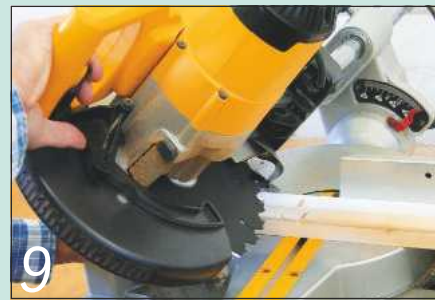
9 A mitre saw will produce a clean, accurate cut for the frame joints
