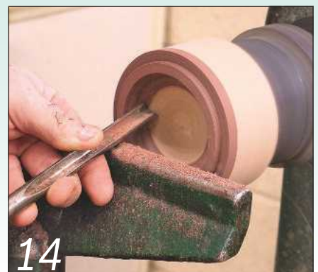
14 Next, start to hollow out the interior of the lid using a bowl gouge
