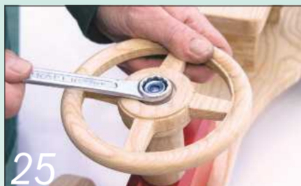
Apply glue to the column spigot, position the steering wheel and tighten its glued locknut
