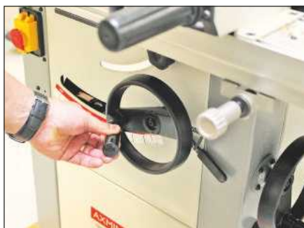
Rise and fall and tilt settings have separate adjustment wheels
