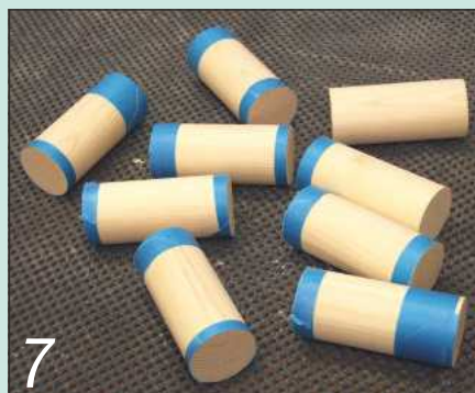
7 Use low-tack tape round the cutting lines to reduce breakout while cross-cutting the dowel
