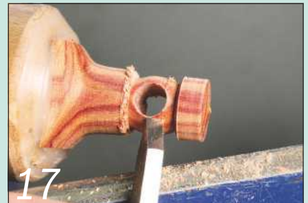
17 Use a parting tool to form a shallow radius between the two skew cuts
