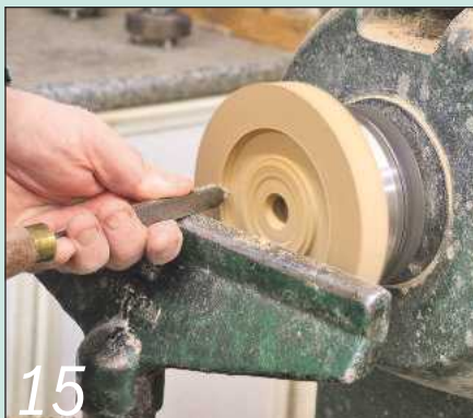
15 Make a jam chuck from a piece of scrap mdf to hold the lid by its tenon...
