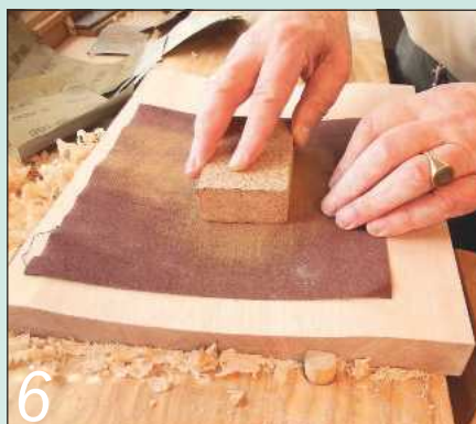
6 I used the lid as a former to shape a sanding block for smoothing the lid
