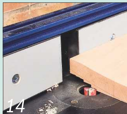
I removed most of the waste at the router table using its fine-adjustment system
