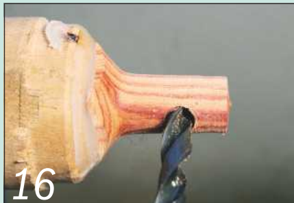
16 Drill a hole slowly through the post, taking care to avoid breakout as the bit emerges
