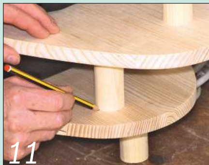
11 Choose your ideal shelf and leg arrangement and mark the leg positions on the shelves
