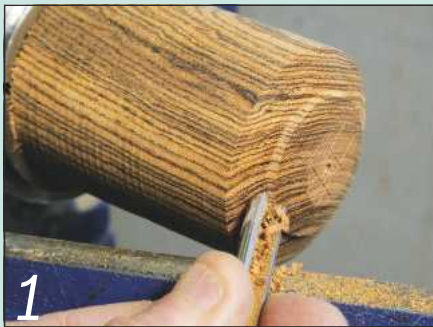
1 Slice carefully across the end of the work to form the dome of the knob
