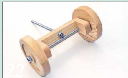
Fit the front axle and wheels to the fork assembly and glue the steering rod into the M10 nut
