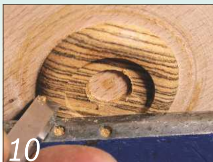
10 Use the same tool to form the small round moulding on the collar plate
