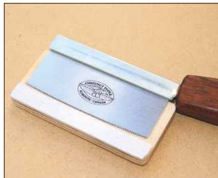
The aluminium edge strip protects the teeth when the guard is fitted
