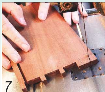
7 The dovetailed carcase ends were cut to shape on the bandsaw...
