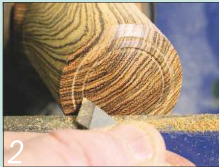
2 Cut two circles with the skew chisel to form the two edges of the bead
