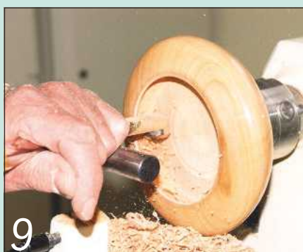
Use the cutter with the round end to start undercutting the bowl's rim
