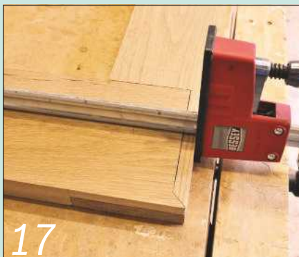
17 This is the resulting joint on the inside face of the frame. An added advantage with this type of joint is that there is less end grain exposed at the top and bottom of the door
