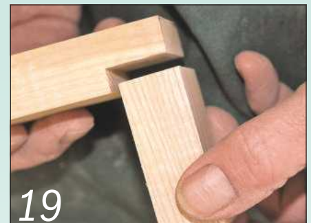
Cut out the three pieces that form the steering fork and cut half-lap joints to connect them
