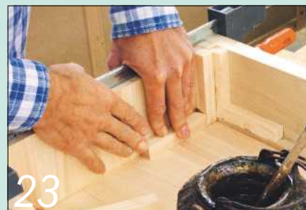
23 The glue pot gets a rare outing to secure old style glue blocks for reinforcement
