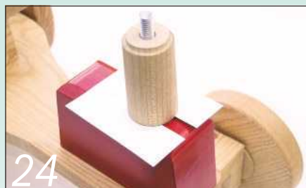
Add a temporary card spacer, fit the steering column and screw it down to the washer
