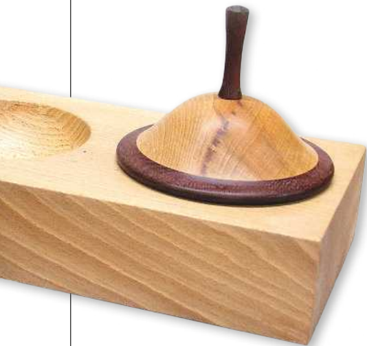
8 Use a profile gauge or a shaped cardboard template to check the bowl profile
