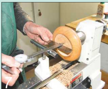
As you work, check the depth regularly using a straightedge and callipers
