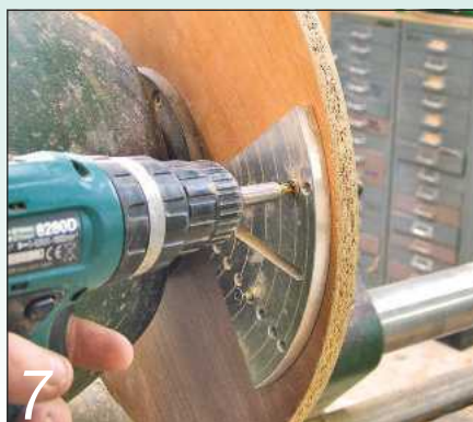
7 Screw weights to the back of the mdf faceplate to balance the piece
