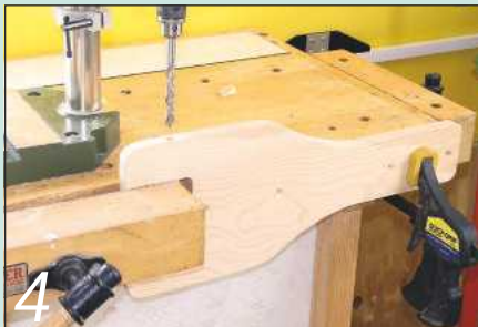
4 Drill a 10mm diameter hole for the axle through each edge of the chassis into the cut-out
