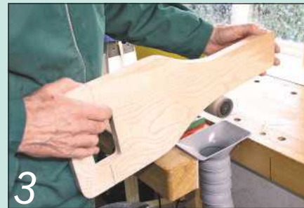
3 Sand and round off all the edges of the chassis using a drum sander
