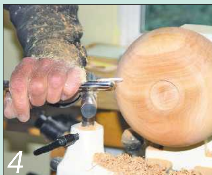
Turn the cutter over and set it so the straight edge does the cutting
