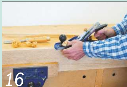
16 A sharp bench plane is a prerequisite for accurate edge jointing
