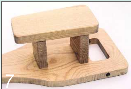
7 Glue the dowels into the holes in the seat supports and fit them to the seat and chassis
