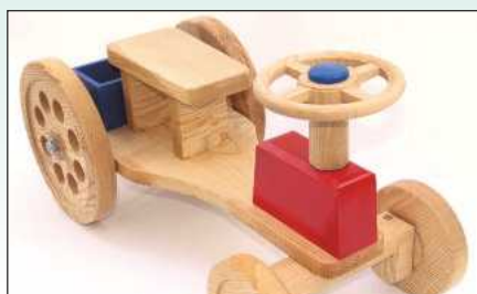
Apply glue to the column spigot, position the steering wheel and tighten its glued locknut
