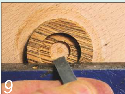
9 Cut the central hole and the recess for the knob shoulder with a scraper
