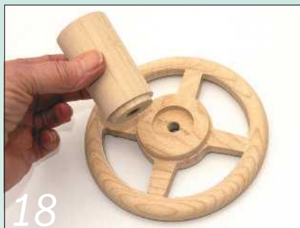
Turn the steering column to round, form a spigot on one end and drill a 10mm hole through it
