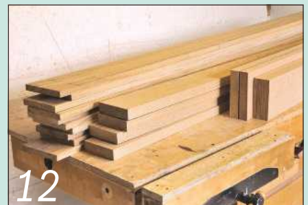
The door is laminated in two sections, so the parts must be machined to very tight tolerances with no snipe at the ends of the boards. To avoid this, I normally machine them overlong and trim 100mm off both ends
