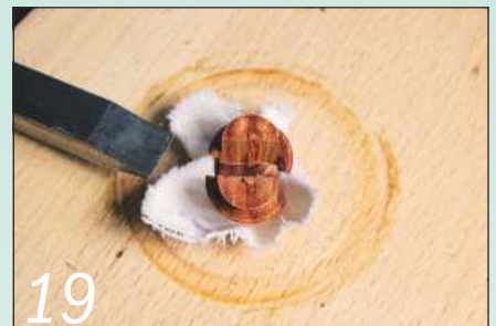
19 Split the post from the rear so the face isn't marked by the cutting edge
