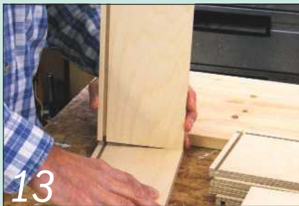
13 The drawers are simple 12mm birch ply boxes with a screw-on front
