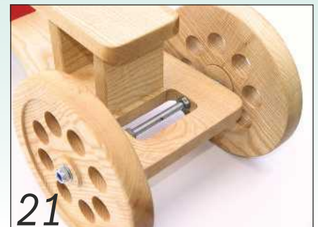
Thread the rear axle through the chassis, fit the wheels and secure them with locknuts
