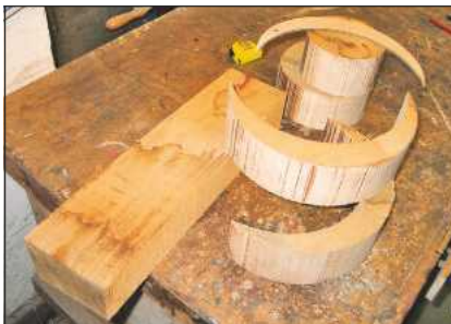
2 Cut out the crescent shapes. The edge block left over should make the other two stands
