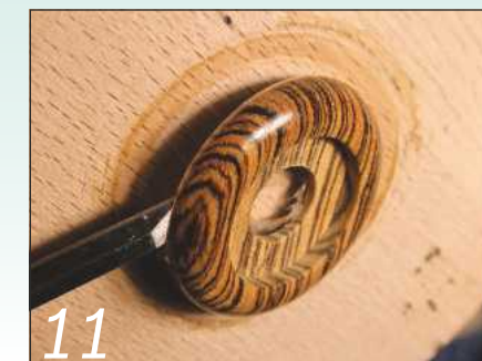
11 Sand, polish and wax the collar plate; then prise it gently off its faceplate
