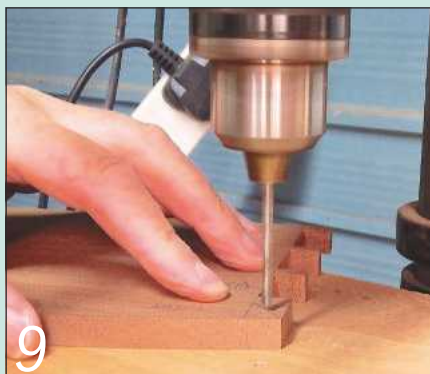
The pivot holes were bored on the drill press to ensure they were truly perpendicular
