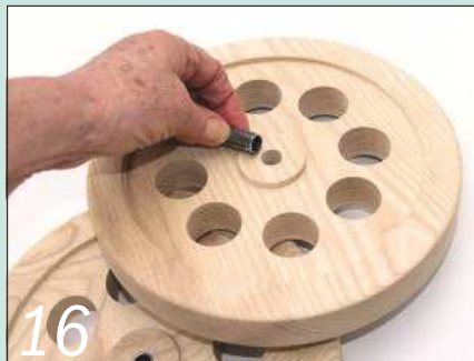
Drill a 12mm diameter hole in each wheel centre and glue the bushes in with Araldite
