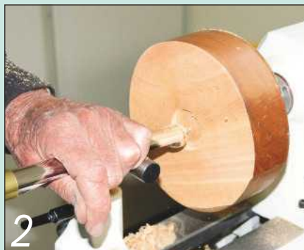
Switch to the square-ended cutter to form a recess for your chuck jaws
