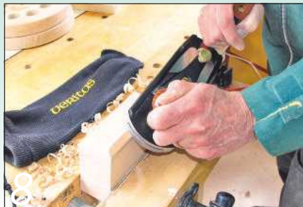
8 Cut the engine block to size, chamfer the top edges and sand it smooth
