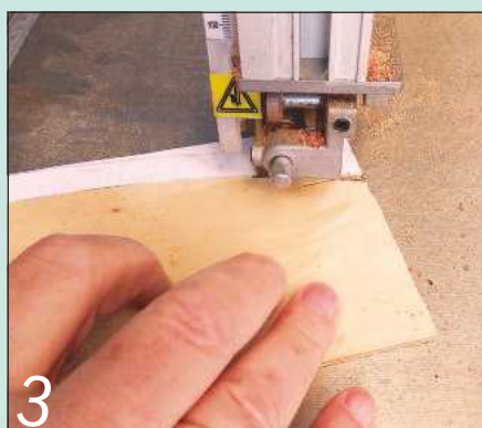
3 I prepared thin plywood templates for marking the curves on the lid and carcase ends
