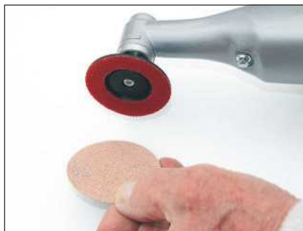
It's easy to fit and remove accessories using the rubber backing disc
