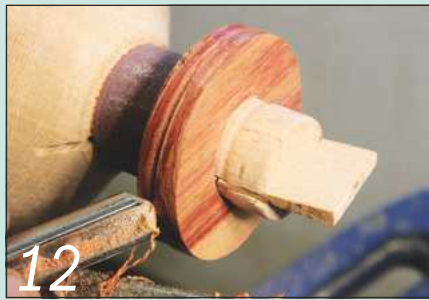
12 Mount the blank on a mandrel chuck and slice it to the correct diameter with a \frac{1}{4} in bowl gouge
