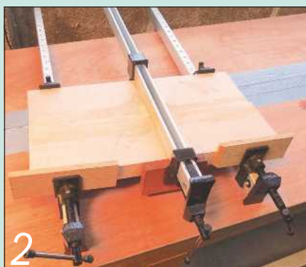
2 Three clamps, the central one across the top, help keep the glue-up flat
