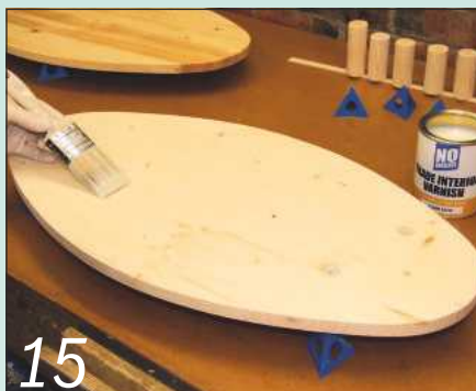
15 After a final sanding, apply three coats of water-based varnish to the various components
