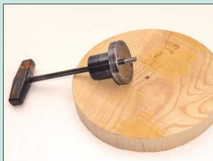
Mount each wheel blank in turn on a screw chuck. I used the Peter Child chuck shown here
