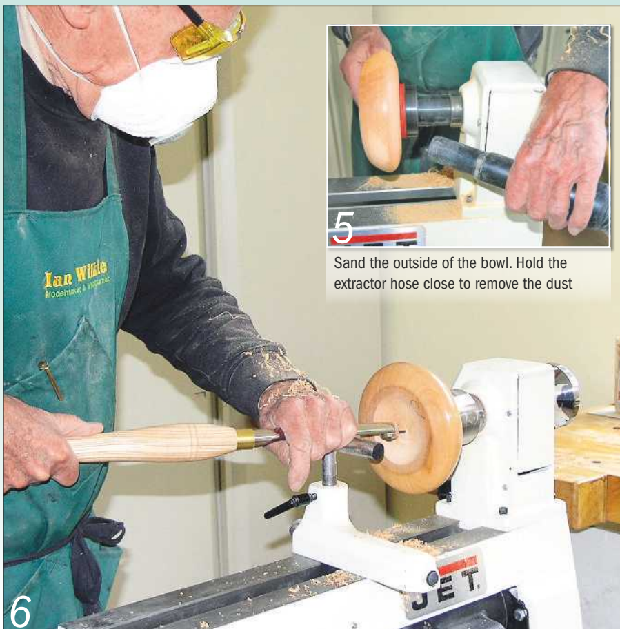
Mount the bowl in your scroll chuck jaws and start to hollow it out
