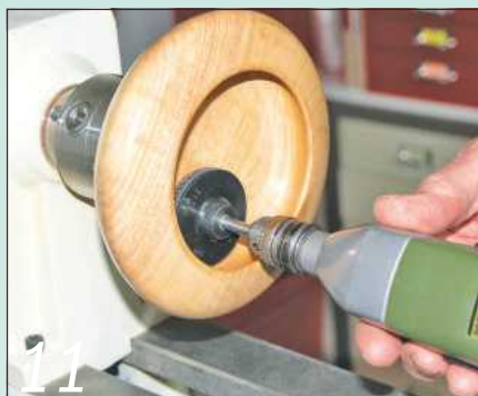
Sand the inside of the bowl with a sanding disc held in a small power drill
