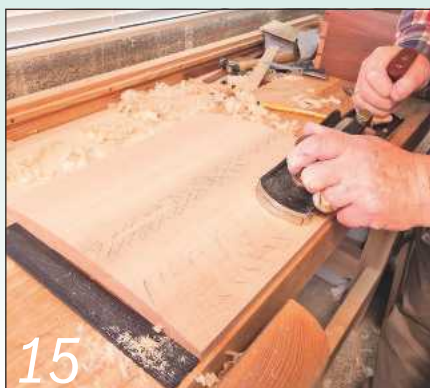
With most of the waste removed, my jack plane smoothed the final curve
