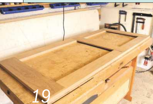
19 It was now time to dry-assemble the frame of the door. You can see here that the middle and bottom rails are thinner than the top rail
