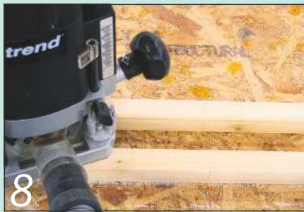
8 I routed lengths of scratch bead to frame the doors and drawers
