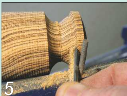
5 Slice down the neck of the knob with the point of the spindle gouge
