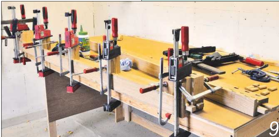
I assembled the side frames in sections, starting with the rails and glazing bars
