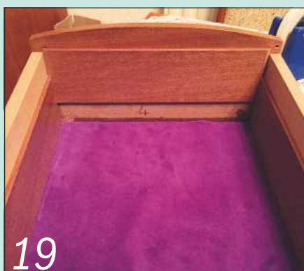
19 Repeatedly trimming and testing the mitres results in a close push fit
