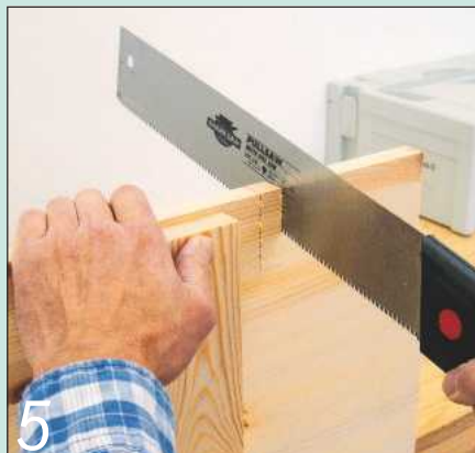
5 A pull saw is sometimes the best option for cutting out notches accurately
