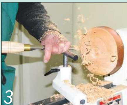
Return to the scraper blade and start shaping the outside of the bowl
