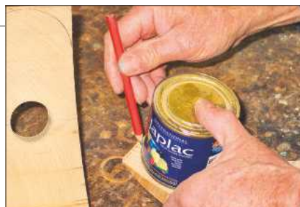
5 Use a suitable container to mark a round shape on each end. Cut it and sand it smooth
