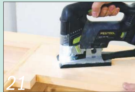
21 Mark out the arch curve and cut along the line with a jigsaw
