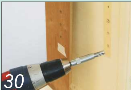
30 Make up a simple drilling jig if you plan to fit adjustable shelves
