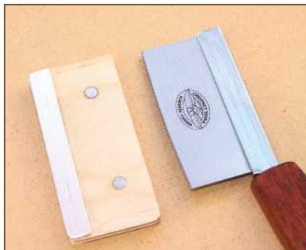
I made a simple guard from plywood and fitted two small magnets to grip the blade
