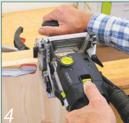
4 The Domino jointer benefits from additional support for its fence
