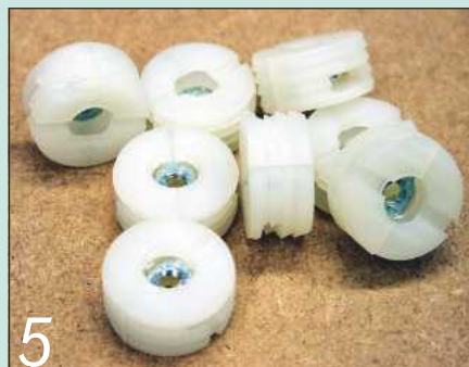
5 I used nylon drawer front adjusters linked by M4 bolts to connect the shelves to the legs
