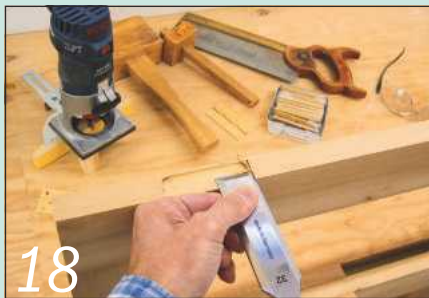
18 After routing out the hinge recesses, some hand squaring is needed
