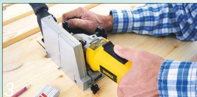
Here's a spot of very careful freehand biscuiting; if you're on the line it's fine
