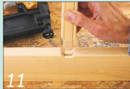
11 Dominos are perfect to use as loose tenons for assembling the frame
