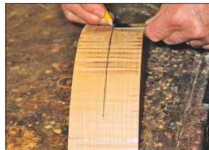
3 Find the centre line of the convex surface and mark the positions of the three holes
