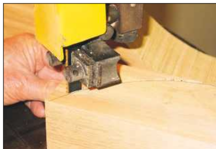
2 Cut out the rough shape of the convex curve on the bandsaw, or with a hand-held jigsaw
