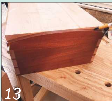
When the lid returned from the carver, I scribed its outside curve from the carcass end
