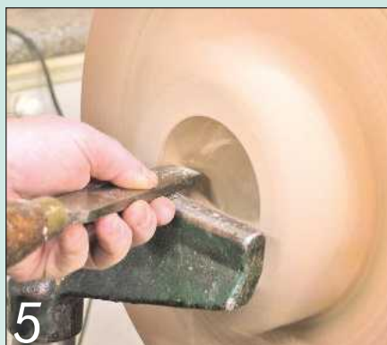
5 Clean up the interior if necessary using a round-nosed scraper
