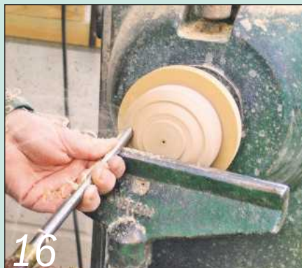
16 Mount the lid on the jam chuck and shape the outside as you wish
