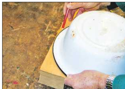
1 The convex shape of the stand can be marked out from whatever is to hand
