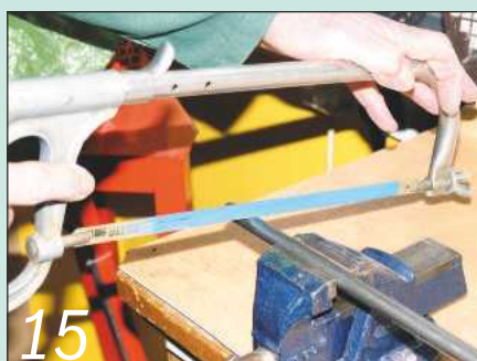
Cut four lengths of 25mm diameter steel tube to make bushes to fit into the wheels
