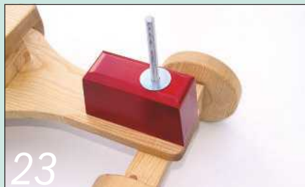
Pass the steering rod up through the tube in the engine block and fit a washer on top
