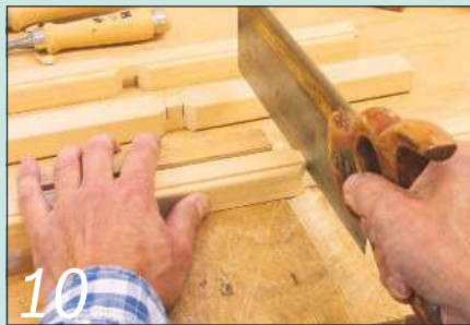
10 Use a tenon saw and a chisel to prepare the various cross-halving joints
