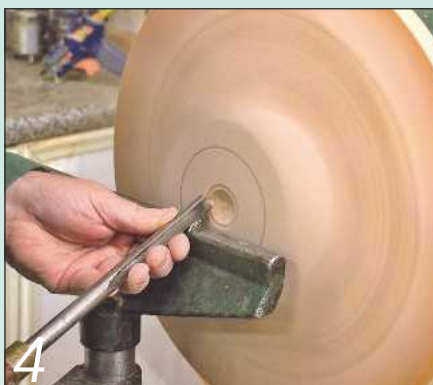
4 Start to hollow out the first bowl as normal using a bowl gouge
