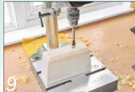
9 Mark the position of the steering rod on the block and drill a hole through it
