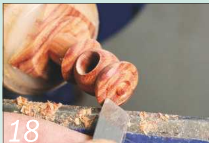
18 Hold the skew chisel flat on the tool rest to scrape the lines on the post top
