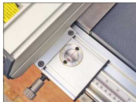
Rack-and-pinion adjustment is a great feature to have, as is the lens cursor
