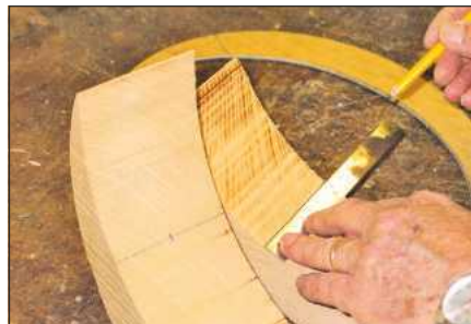
3 Mark the centre of the line across the crescent where the bottle neck hole will go
