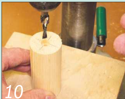
10 Drill a 5mm hole through each leg and add a counterbore in the bottom end of the lower legs
