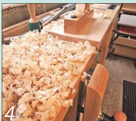
4 Trying to hollow the lid from scratch with a round-bottomed jack plane was unrealistic...
