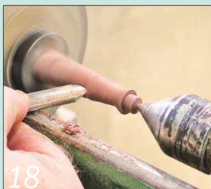
18 Use a spindle gouge to turn the handles to shape, then finish and fit them
