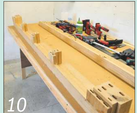
You can see here how the composite glazing bars work, as they await their dominos
