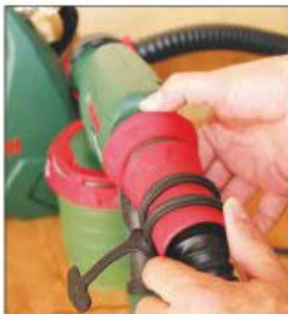
The airflow can be altered by rotating the twist ring on the gun
