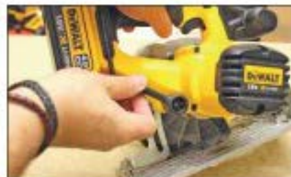
Cutting depths are selected and locked in position with this rear lever
