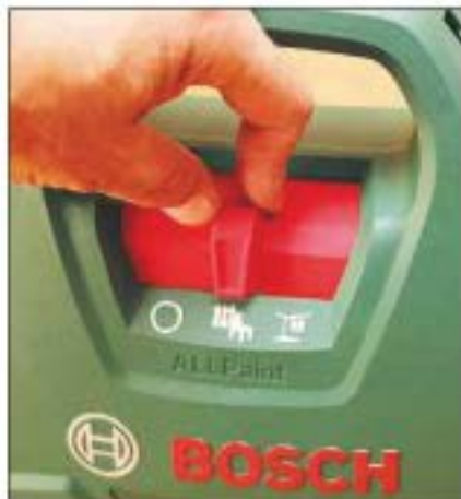
A simple slider sets the air power low rate through the gun
