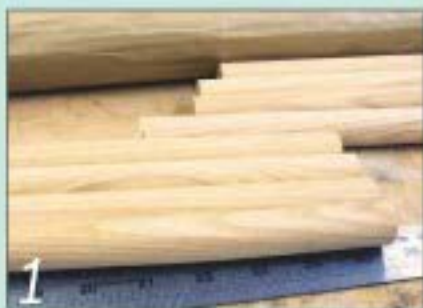
1 The ash dowels had a rough finish and needed a lot of hand sanding
