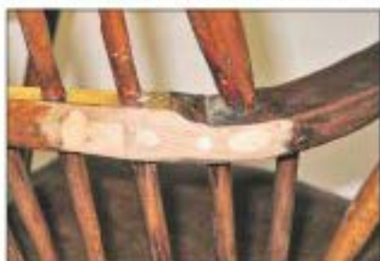
3 Once the glue had dried I cut away the excess, trimmed the plugs and sanded the joint smooth
