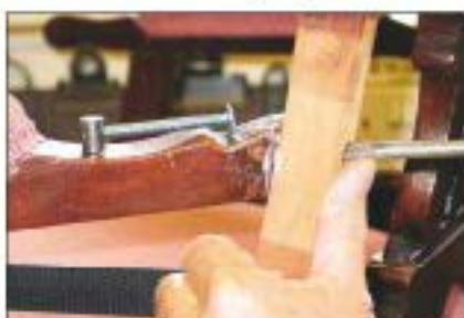
6 Finally the original arm is secured with a secret barrel nut and bolt reinforcement
