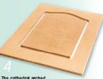
4 The cathedral arched panel and the template made from it
