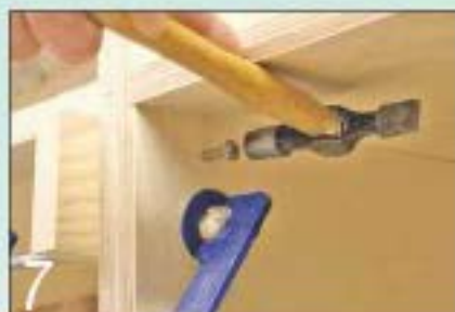
7 Joint the two carcasses together using concealed cabinet connector bolts
