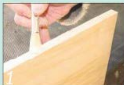
1 Glue the ash lipping to intermediate shelves and secure it with low-tack tape
