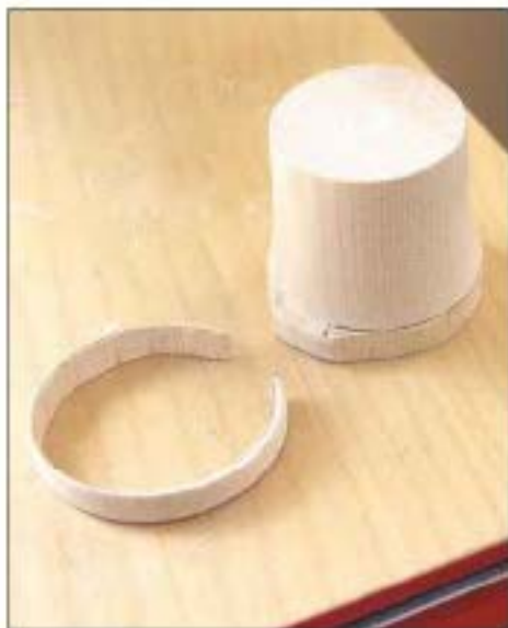
9 ...to leave just the pouring lip. Shape it and sand all the cut edges smooth
