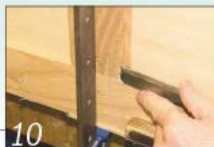
10 Cramp up each panel and remove any squeezed-out glue with an old chisel
