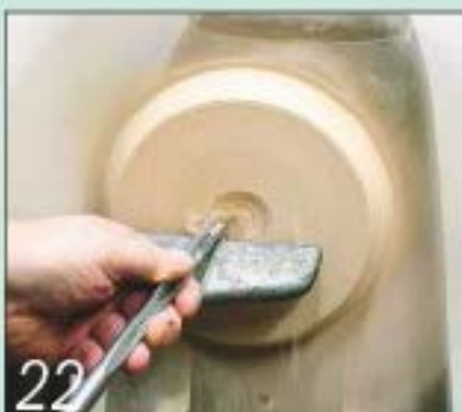
22 All that's left to do is to hollow out the centre of the bowl in the conventional way
