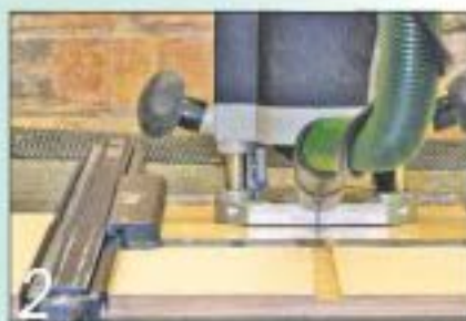
2 Cut the 4mm deep grooves for the shelves in the side panels using a router
