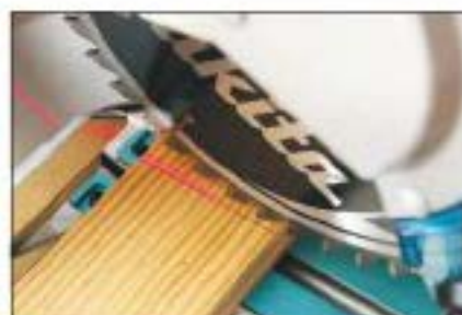
When the head descends you can see how far the laser is out of line
