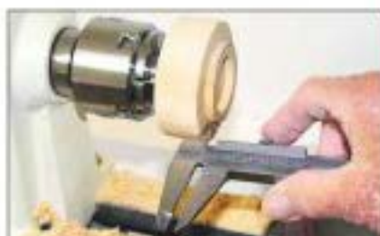
2 Turn a spigot on the underside of the lid blank to fit into the top of the pot
