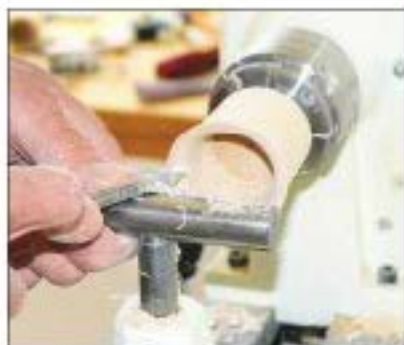
4 Widen out the rim using a beading tool, but don't make the edge sharp
