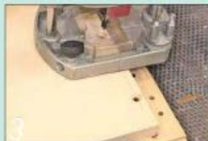
3 Drill the clearance holes for the screws in the sides and countersink them
