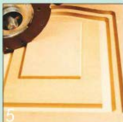
The first stage of the process uses a straight cutter and a 50mm guide bush
