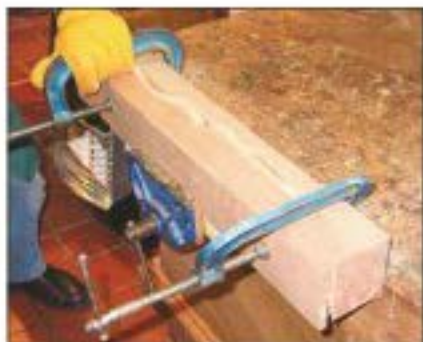
4 The hot and pliable splat is fitted between the two former blocks and securely cramped up
