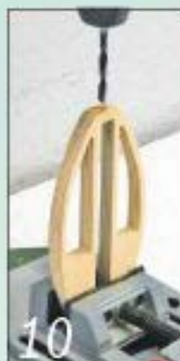
10 The end of the pendulum bob is drilled to take the adjuster rod
