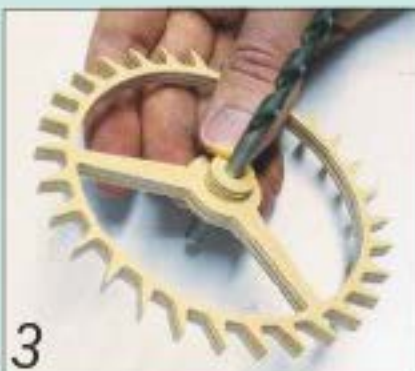
3 The escape wheel and spacer can be centred on a twist drill bit...
