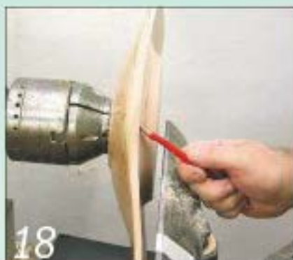
18 This photo shows that the wall near the centre of the platter needs to be much thinner
