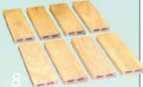
8 Groove and chamfer the rails for the side panels, ready for assembly
