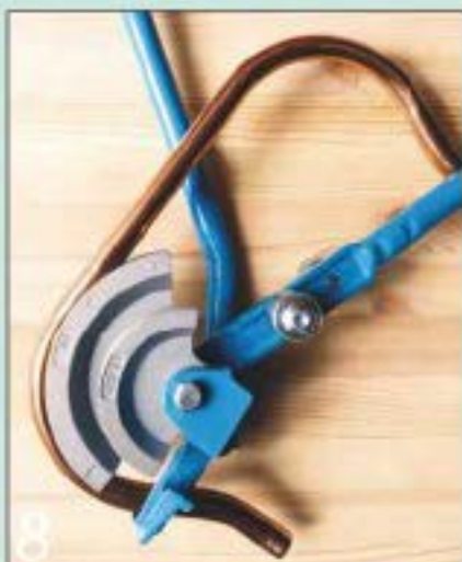
A pipe bending machine was essential for forming the gentle curves on the feet...
