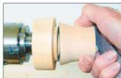
3 The spigot must be deep enough to fit securely in the teapot recess
