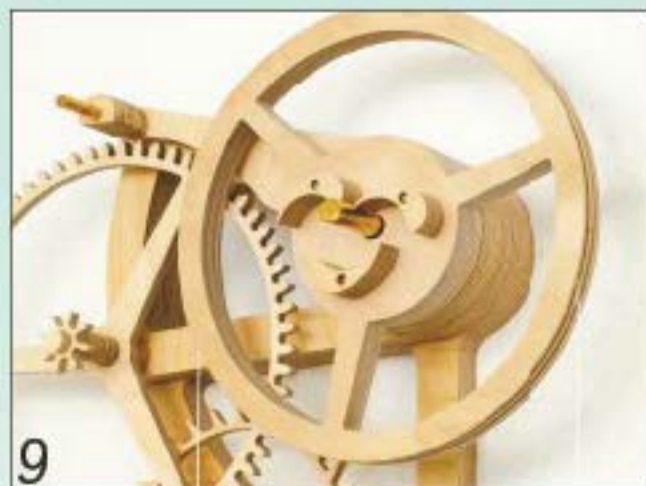
9 The ratchets will engage with the cog on the back of the hour wheel
