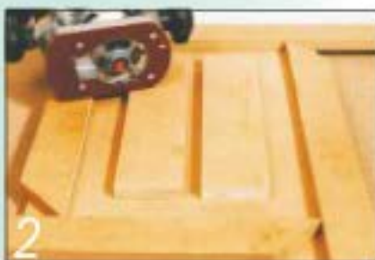
2 Straight strips of MDF taped to the panel guide the router
