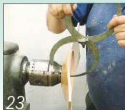
23 Use double-ended callipers to measure the wall thickness at the centre of the bowl
