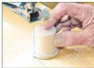
8 Mark the position of the pouring lip on the jug and cut away the surplus wood...
