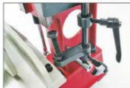
The depth of cut is controlled by stops on the side of the column
