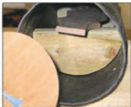
2 The flat splat is placed inside my home-made steamer, supported on two blocks
