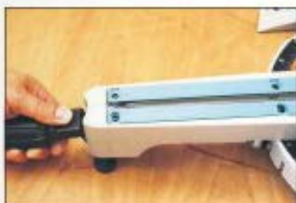
Mitre angles are set and locked with the large front handle
