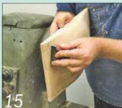
15 ...and then switch off the lathe before hand-sanding the wings, working with the grain
