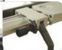
Micro fence setting scale to within 1/10th mm calibration.
