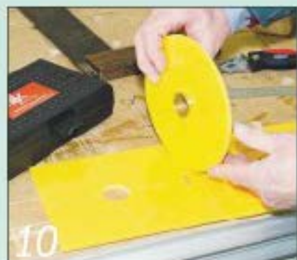
Next I made a 30mm hole through the centre of the spacer and put my guidebush through it
