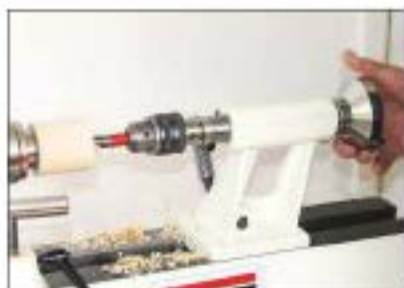
2 Drill the blank to a depth of 40mm with a 25mm saw-tooth Forstner bit
