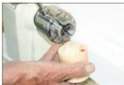
1 Mount the mug blank in the chuck jaws, tighten them up and face it off
