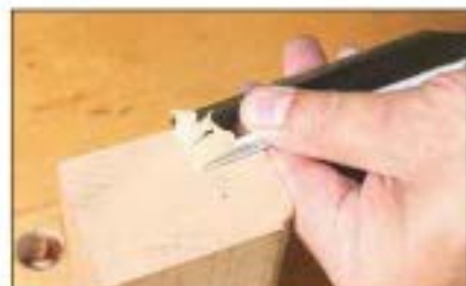
You can get very keen edges, which are essential for end-grain paring
