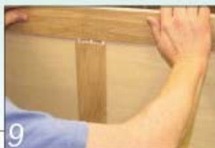
9 Assemble the side panels after slotting the veneered infill panels into place
