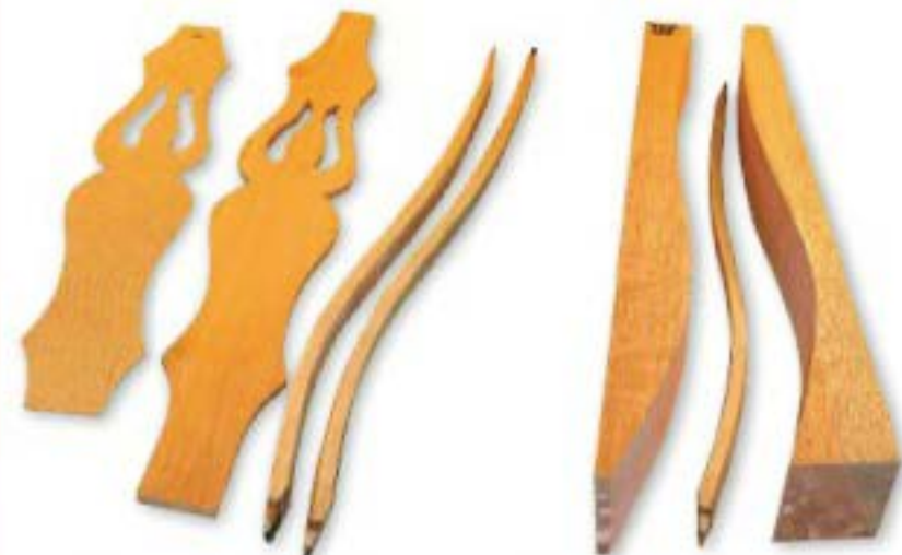
1 I used a template to prepare the new splat. The original back supports (right) show the curve I needed to copy
