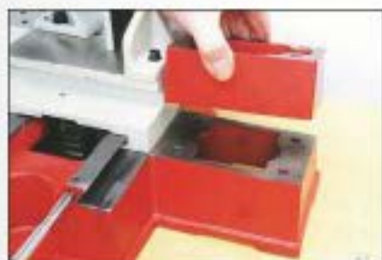
The optional riser block kit adds 50mm to the column height
