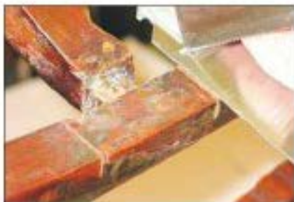
2 The vertical back rail had also apparently been patched and repaired several times before. I cut half of it away first
