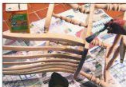
2 The first job was to treat the whole chair with a liberal coat of woodworm fluid
