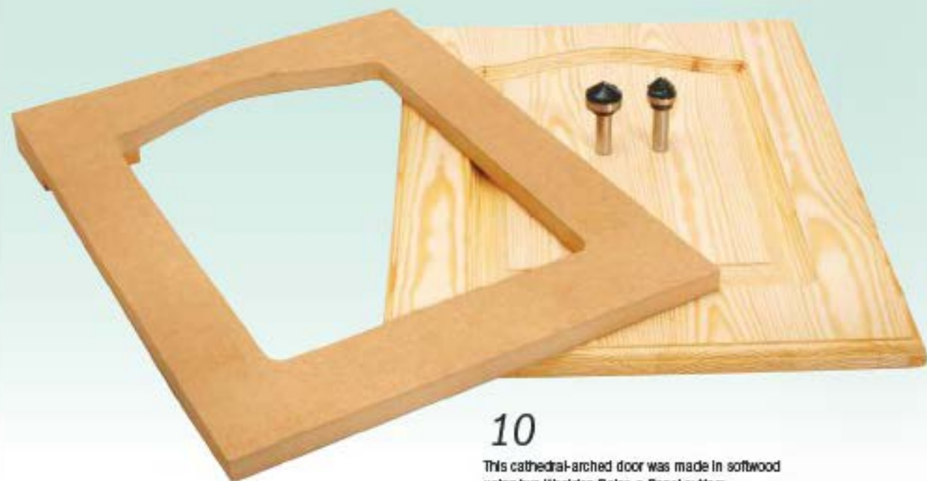
Use a bearing-guided ovolo cutter to mould the door edges
