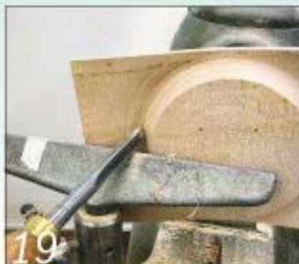
19 Keep the gouge well over on its side to prevent a dig-in from happening
