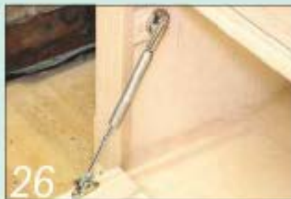
26 Position and fix the lower door stays. One had to be fitted with a spacer block
