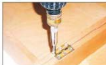
The drill guide centres the screw hole when fitting a butt hinge
