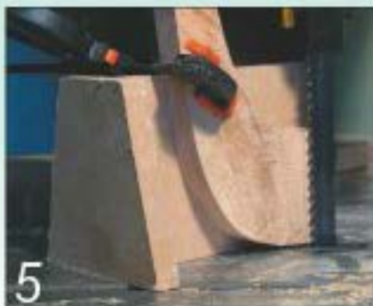
This jig holds the leg vertical in both planes for cutting the dovetail on a bandsaw
