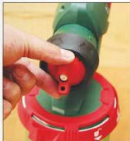
The horn rotates for vertical, spot and horizontal spray patterns
