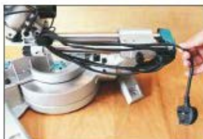
A couple of hooks for the storing the power cable on-board is a neat touch
