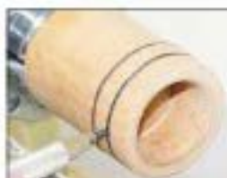
2 Mark off a series of rings 4mm wide along the cylinder
