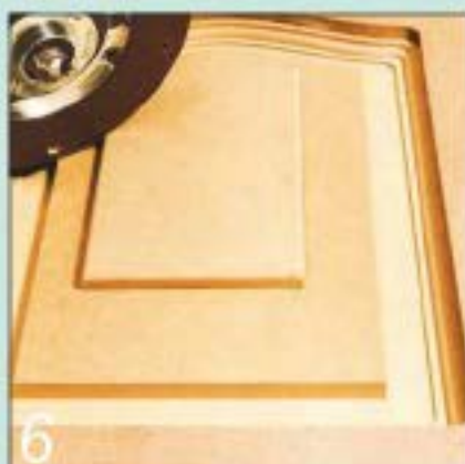
The second stage uses an ovolo cutter and a 32mm guide bush
