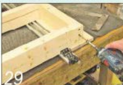
29 Make up the base frame from lengths of softwood using simple butt joints
