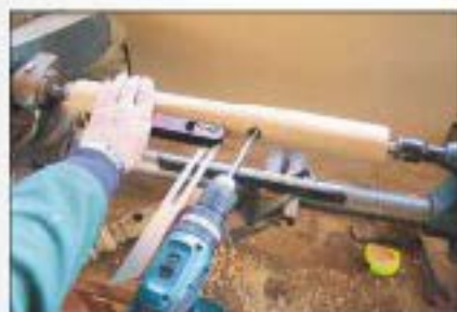
4 It's important to get the angle of the stretcher mortise hole right
