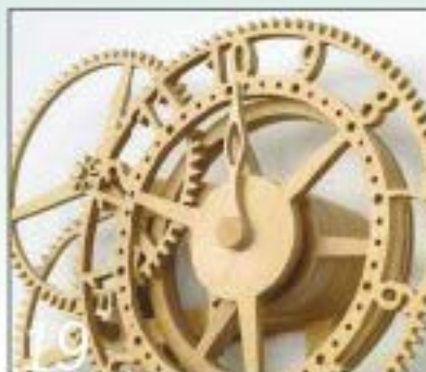
19 The hour wheel can now be set in position; note the fixed hour hand
