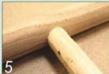
5 The cross bars were glued into their drilled holes in the two long side rails
