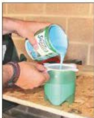
Thicker finishes have to be filtered first through the supplied sieve
