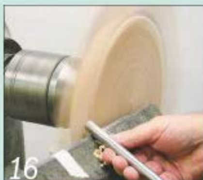
16 Use a bowl gouge to shape the wings. Leave the wood in the centre for stability
