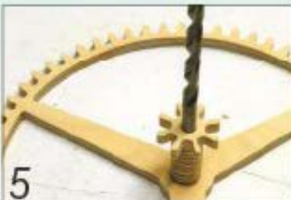
5 Align the gear, the small pinion and the spacer on a drill bit
