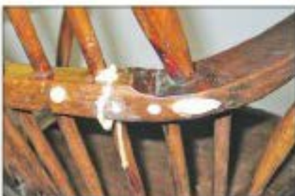
2 Once the bolt was inserted and tightened into its nut, I could plug and fill the various holes
