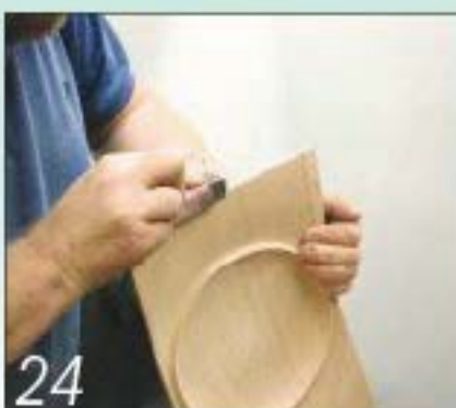
24 Sand the bowl, and don't forget about the edges, but turn the lathe off first!
