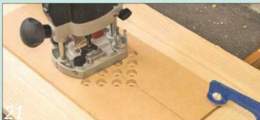
21 Cut the decorative diamond pattern using a home-made template and hand router
