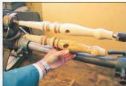
5 The replacement leg is turned and checked for detail against the original leg
