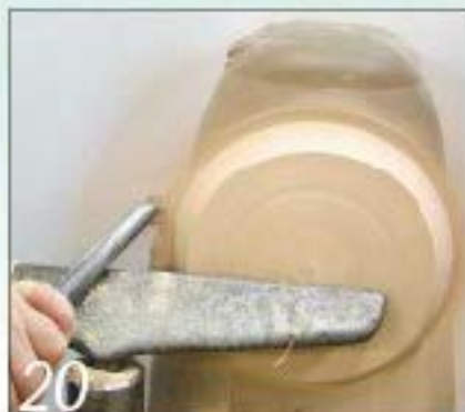
20 Again use the bottom wing of the fingernail gouge (or a scraper) to shear-cut the wings
