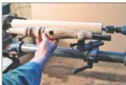
3 A beech blank is roughly turned on the lathe and compared to the original
