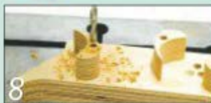
8 Drill the pivot holes in the ratchet blades after cutting them out
