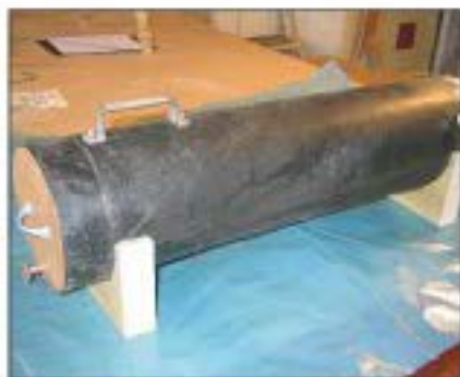
3 A wallpaper stripper produces the steam and a sealed metal tube makes the chamber
