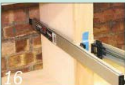
16 Cramp the face-frame muntin to just one carcass and leave until the glue is dry
