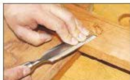
Paring waste from housings is an area where these chisels work well
