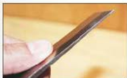
The lands (the blade edges) taper finely - ideal for cleaning into tight corners
