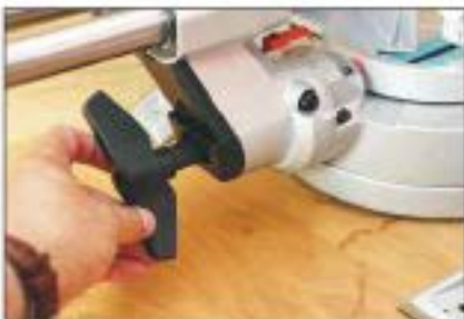
This large wingnut handle is easy to operate for setting bevel cuts
