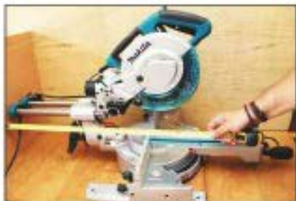
You need about 700mm of space to allow the full-length bars to run their arc
