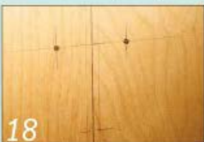
18 Cut the back panels slightly undersize and attach them with self-tapping screws
