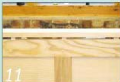
11 Fit the face-frame stiles to the side assemblies, using floating tenons to help align them
