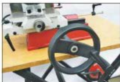
The lateral movement handwheel must overhang the front of the bench
