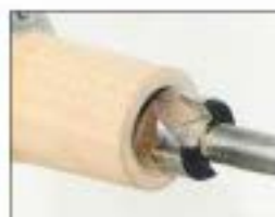
1 To make the handles, turn a cylinder and drill out its centre
