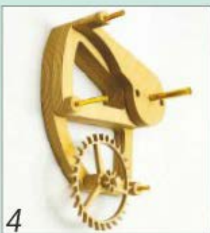
4 ...and fitted to the lowest frame arbor along with a pinion
