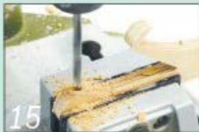
15 The anchor is drilled to accept the two small adjusting grub screws
