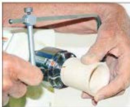
5 Partially part off the mug and finish the cut with a fine-toothed saw
