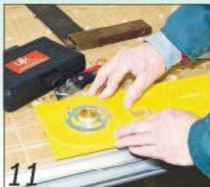
I then glued the spacer in place using the guidebush to match it to the hole in the main body
