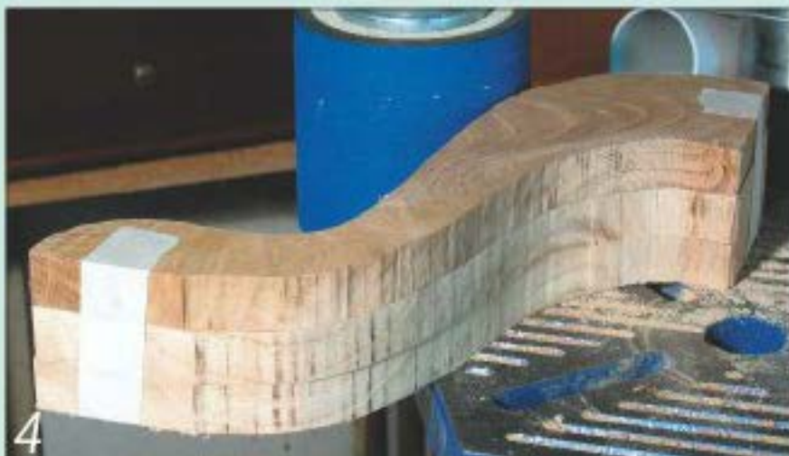
By taping the legs together, you can cut and sand them all in one go for accuracy and speed
