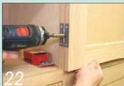
22 Attach each hinge leaf using a single screw. I add the rest during final assembly
