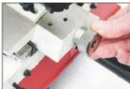
This knob controls the fore-and-aft movement of the table
