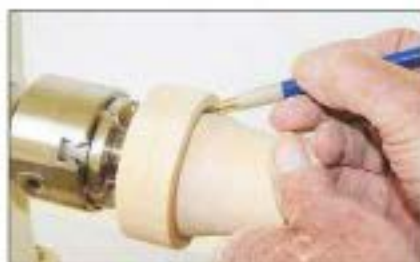
4 Push the pot onto the lid spigot and draw a line round the pot circumference
