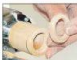
3 Shape a ring using a beading tool and part it off. Repeat as necessary.
