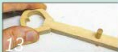
13 The pendulum head has a V-shaped internal pin to reduce friction
