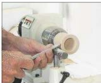
3 Shape the outside of the mug, tapering down to 35mm diameter at the base
