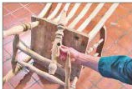
1 This is the well-worn and worm-ridden leg that needed replacing
