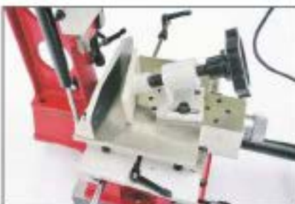
The adjustable work cramp can be set for tapered workpieces
