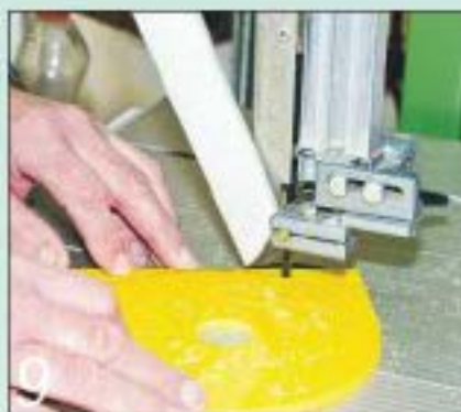
I cut a guidebush spacer on the bandsaw to the same diameter as my router base
