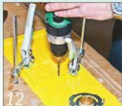
The slide assembly parts are held in place with clamps so the two screw holes can be drilled
