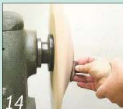
14 If you prefer, you can hand-sand the solid part of the bowl while it rotates...
