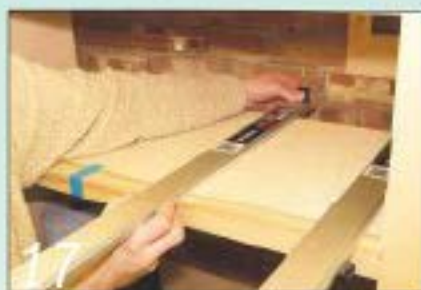
17 Attach the face-frame rails using glue and floating tenons. Again, cramp until dry
