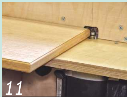
11 Cut the ovolo moulding all round the tabletops using the table router
