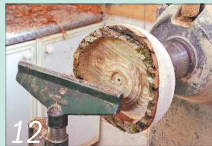
12 Work on the first 25-35mm of the rim before going any deeper
