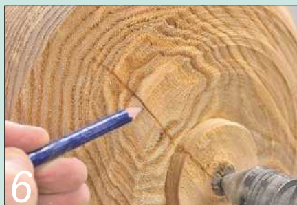
6 Wood can be so frustrating sometimes. This split will have to go!
