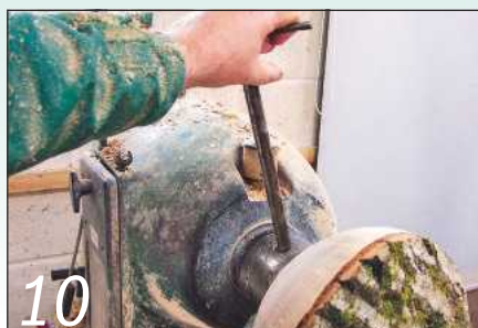
10 Keep checking the tightness of the chuck. Remember that this is wet wood
