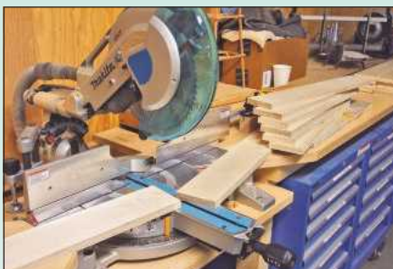
The 60 plywood surface slats are cut to length one by one on the chop saw
