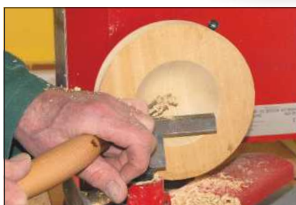
3 Reverse the bowl onto the chuck jaws and hollow it out with a bowl gouge
