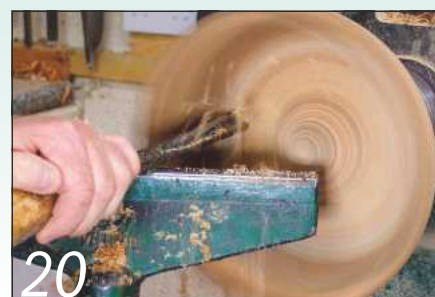
20 The steeper bevel angle allow me to cut round sharp curves more easily
