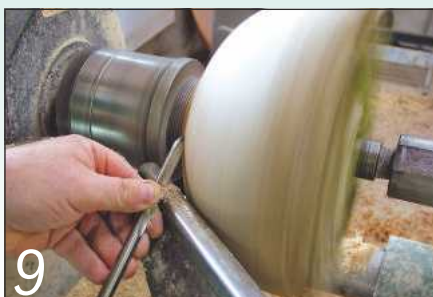
9 Finalise the external shape of the bowl using a shear cut with a smaller gouge
