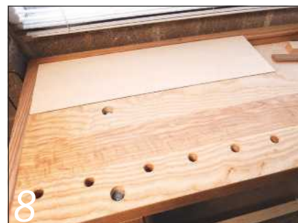
8 The tool well on this bench can be filled in when a wider flat surface is needed for assembly work
