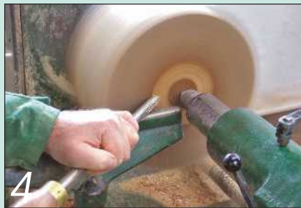
4 Use a pull cut with a fingernail gouge to flatten the base of the blank...
