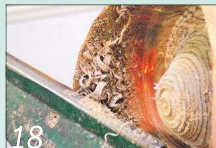
18 Finish this step before moving on. A lamp behind the work helps to reveal the wall thickness
