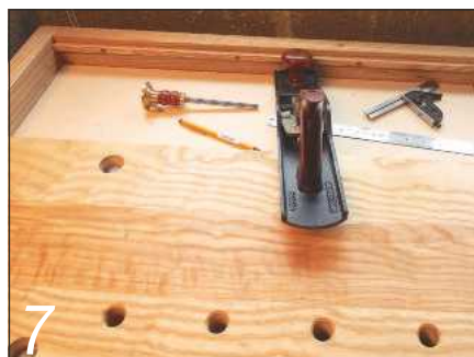
7 A tool well can be a positive benefit on a small bench, clearly defining working and storage areas
