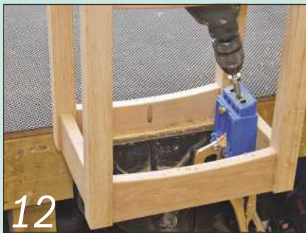
12 Drill holes for attaching the tabletops using a pocket-hole screw jig
