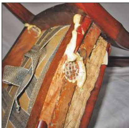
3 Here you can see how the foamed Gorilla glue has filled the gaps and secured the break
