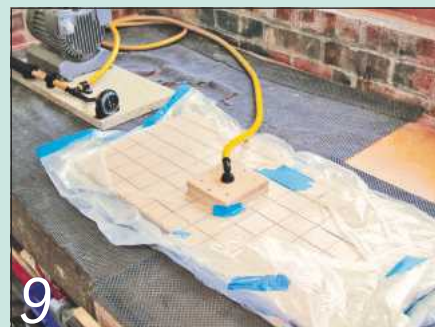
9 Press the veneered tabletop assemblies between two flat cauls. I used a veneer press
