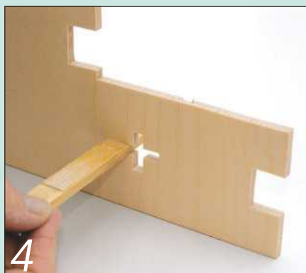
4 Use abrasive paper stuck to an offcut to sand inside all the internal cuts
