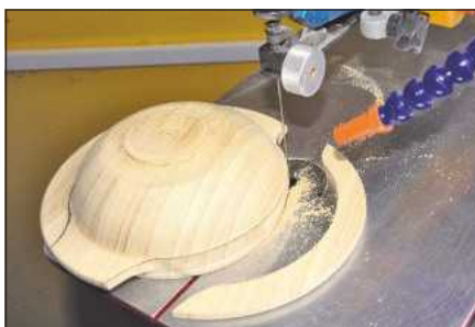
6 Mark the handle positions on the rim and cut them away on the scrollsaw
