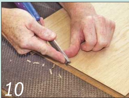
10 Trim the overhanging veneer flush using a sharp chisel or a plane
