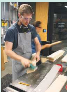
The 60 plywood surface slats are cut to length one by one on the chop saw
