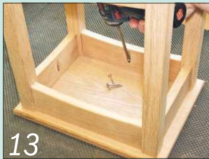
13 Centralise each frame and attach it to its tabletop with pocket-hole screws
