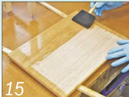
15 Finish the tables with oil, cutting back between coats, and then wax them
