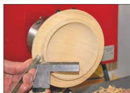
4 Complete the rim, turning down to the pencil line on the outside edge
