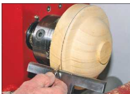
2 Mark the top edge of the rim on the edge of the blank with a pencil
