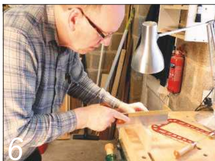
6 A higher bench is an advantage for dovetailing, but a raised centre of gravity affects stability
