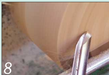
8 ...and also to do the initial shaping of the outside. Keep the tool handle down low
