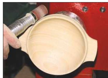
7 I used my Kirjes drum sander on a flexible drive to tidy up the outside edge of the cut
