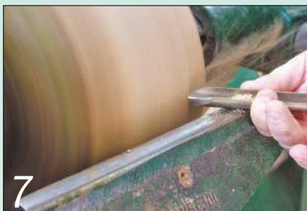
7 Use the same fingernail gouge to bring the blank gradually to round...
