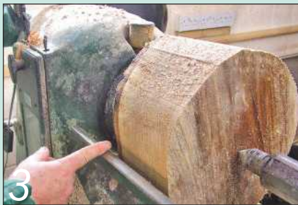
3 Balance the piece on the lathe using your finger on the toolrest as a reference point
