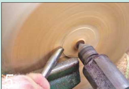
5 ...and to start cutting the chucking spigot to size to match your chuck jaws
