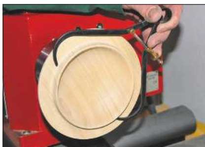
5 Check the outside diameter of the rim with a pair of spring bow callipers
