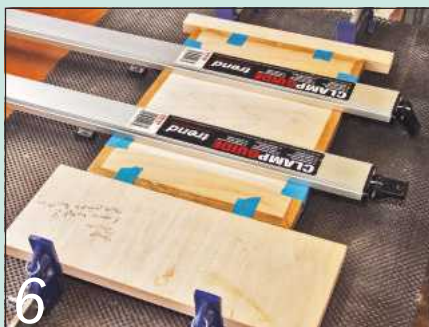
6 Glue and cramp the mitred lengths of oak lipping to the three tabletops
