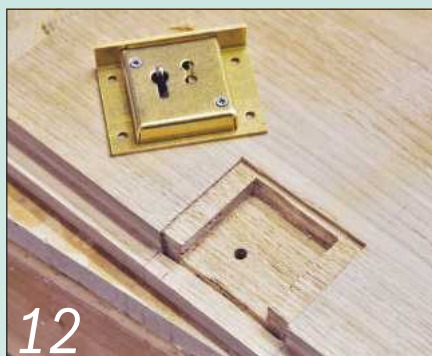
Drill a small hole through the door to mark where the pin protrudes from the lock case
