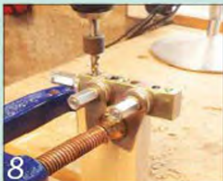
8 I used my Joint Genie to dowel the door and drawer front frames
