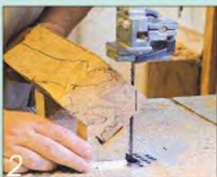
2 A simple homemade sledge like this one saves having to tip the bandsaw table
