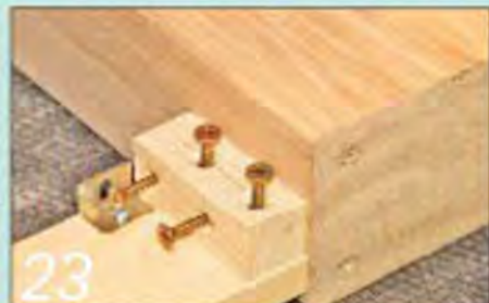
23 Use small glued and screwed blocks to strengthen the lower front rail joints
