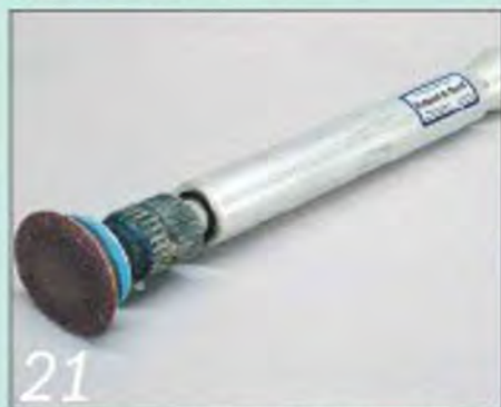
I then used my Extend-a-Sand in a power drill to sand the bottom and the lower side wall
