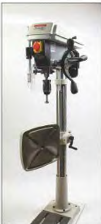
The table can be rotated through 90° to the vertical position...
