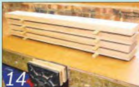
14 Use several pieces planed flat and square to make up the top, shelf and base panels
