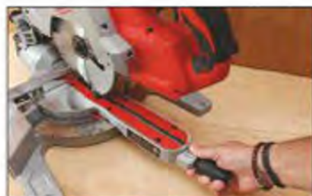
Pushing down on the front handle allows the turntable to rotate. You twist it to lock a position
