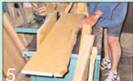
5 The side planks are cut with straight edges to make up the required widths
