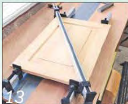
13 Glue up the door frame and panel and check that it's perfectly square
