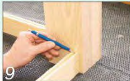
9 Mark out the extent of the stopped grooves required on the legs
