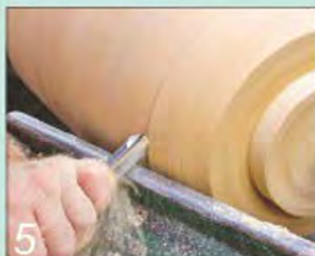
5 Shape the outside next, using the bowl gouge to achieve a shear cut and a smooth finish
