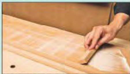
A shooting board for veneers is very useful – simply glue support boards to a baseboard
