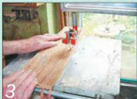
3 Mark the curved front profile on the shelf and remove the waste on the bandsaw
