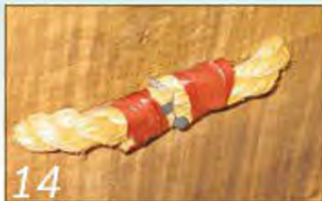
The wire is taped over and a couple of nails driven in to hold each handle in place
