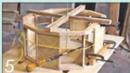
One of the biggest challenges was to devise a way of cramping the structure during the glue-up
