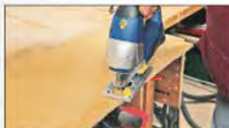
The saw cuts quickly and cleanly when following intricate curves
