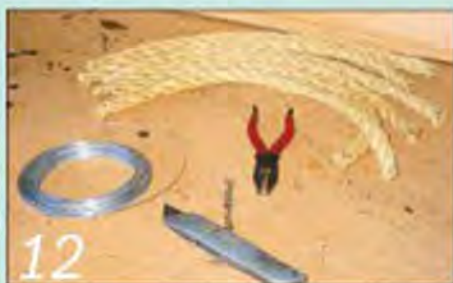
Half a dozen rope handles are wire-bound at their ends, ready for fitting
