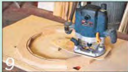
I needed to cut a circle on the inner edge of the door, so I made a compass jig for my router
