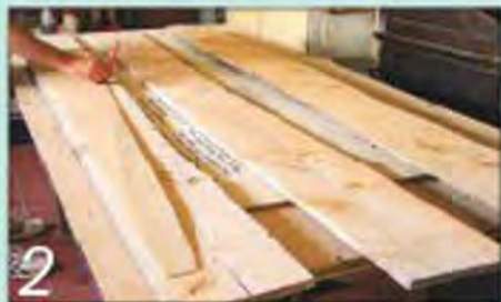
2 I used a ply template to mark out the side shapes for the top and bottom panels
