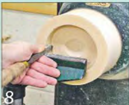
8 Mount some scrap on a faceplate and cut a recess to fit the vase spigot
