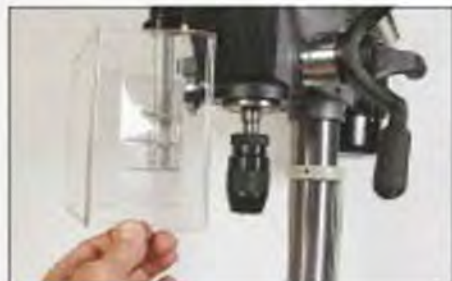
The swelling chuck guard seems over-elaborate, but actually works very well in practice
