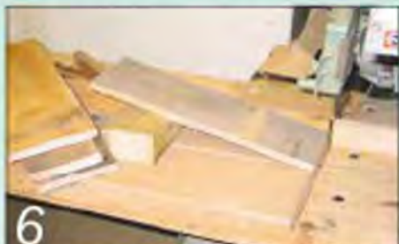
6 The end angles at the shoulder joint on each side can be cut on a cross-cut saw
