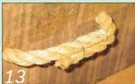
The ends are pushed through their holes, overlapped and joined with twisted wire
