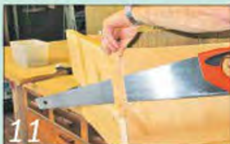
The ends are glued and nailed on, and then trimmed off flush with each side
