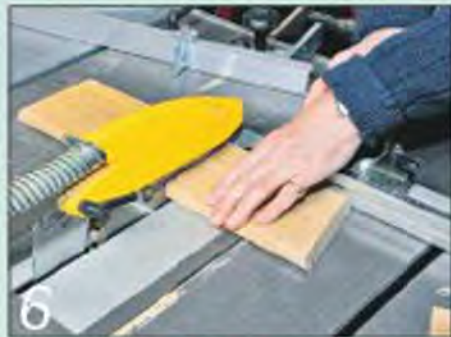
6 Then mark the overall length and cut the other end of each leg square
