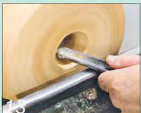
13 If you don't have any hollowing tools, the bowl gouge will work well with this vase shape
