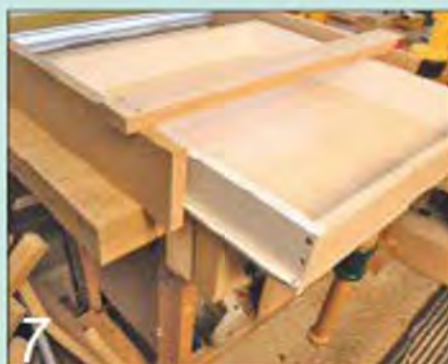
7 The central drawer unit is temporarily tacked together using battens as spacers
