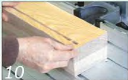
10 Dismantle the parts and rout the stopped grooves along the legs
