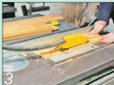
3 ...and rip it down to the final width. I made mine 150mm wide and 500mm long
