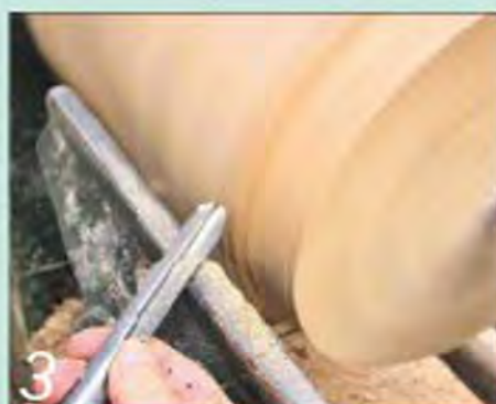
3 I used a fingernail profile bowl gouge to turn the blank to a cylinder
