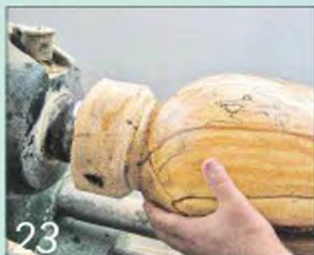
...and weaken the joint so you can prise off the vase carefully by hand
