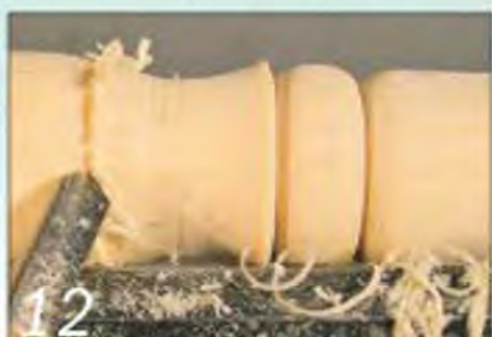
Then twist the handle and start to cut in the opposite direction
