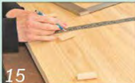
15 Mark the positions of the floating tenons to help align the meeting edges
