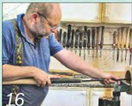
16 Keep the long handle of the tool under your forearm for greater control
