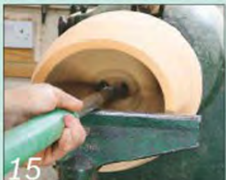
15 I'm using my Big Brother tool here. Note that the cutting tip is rolled slightly anticlockwise
