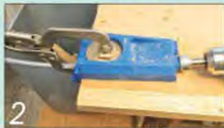
A pocket-hole jig makes quick work of jointing the unit corners
