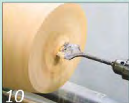
10 Use a large spade bit to drill a starter hole down the centre of the vase
