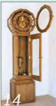
Once the clock face is fitted and the pendulum and weights set in place, the clock is ready to run
