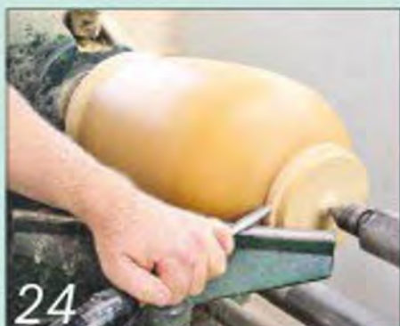
Reverse-chuck the vase onto a domed dolly to remove the chucking spigot
