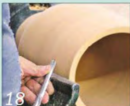
Refine the outside shape using a small spindle gouge, taking light shear cuts
