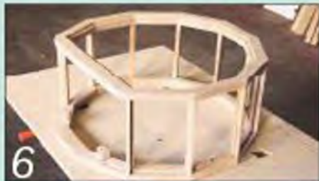
The completed hood assembly is ready to receive the back and the plywood and glass side pieces
