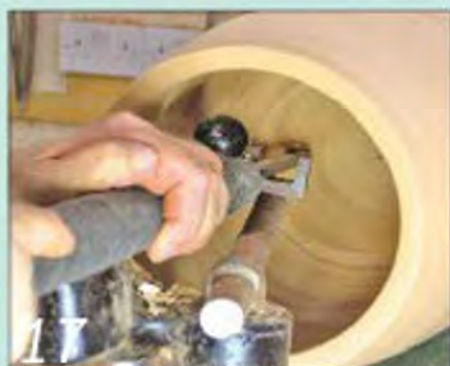
Here I'm using the Rolly Munro tool and my deep hollowing toolrest to finish the job
