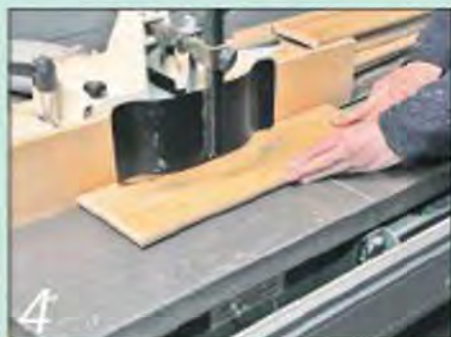
4 Add an edge moulding, profiling the ends first and then tackling the long side edges
