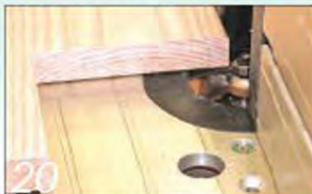
20 Rout a small roundover profile on the exposed panel edges with a 3mm radius cutter
