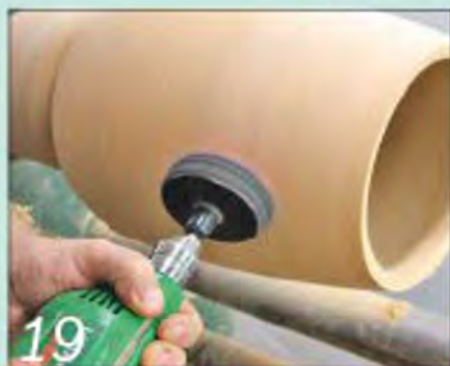
With the hollowing complete, power-sand the outside of the vase first...
