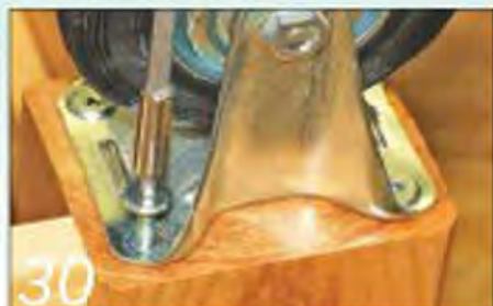
30 Attach the four wheels by tightening down the bolts with a hex driver
