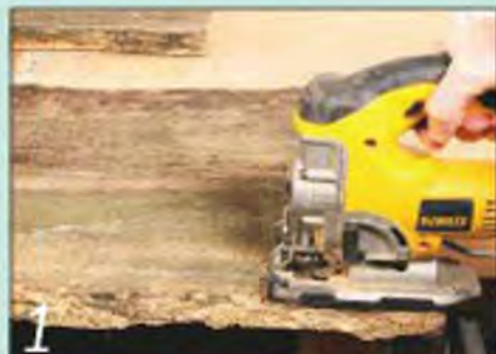
1 Mark a straight line to remove the bark and the sapwood, and cut along it using a jigsaw
