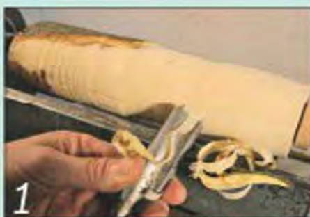
1 Turn the workpiece to a tapered cylinder with the roughing-down gouge
