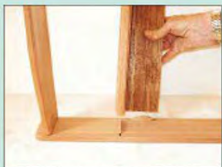
6 Glue up and assemble the various components using biscuits, then cramp the frame square
