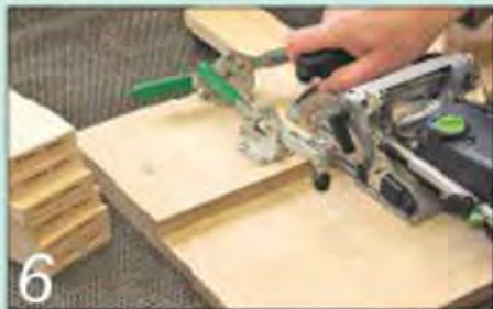
6 Mark out and cut the mortises in the rails for the floating tenons
