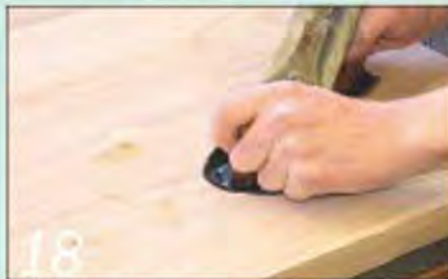
18 When it has, flatten any raised panel joints using a sharp plane
