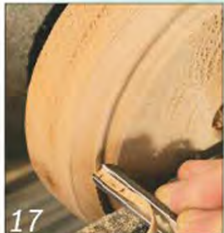
Start rounding off the edge of the base with a bowl gouge by sliding away the waste
