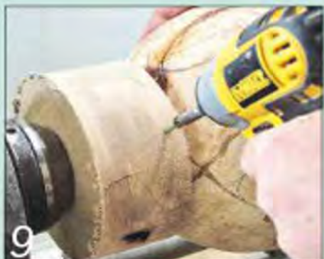
9 Glue the vase spigot into the recess and secure it with a couple of screws
