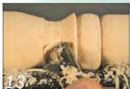
Make sure that the bevel is always flat on the side of the spindle
