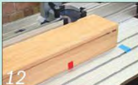
12 Form 8mm wide stopped chamfers along the leg edges using a 45° cutter
