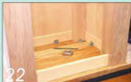
22 ...and also to attach the top panel to the island's top side rails and legs
