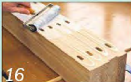
16 Spread the glue evenly on both joint surfaces using a hard roller
