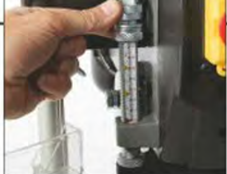
The depth stop is easy to set and gives a good indication of drilling depth
