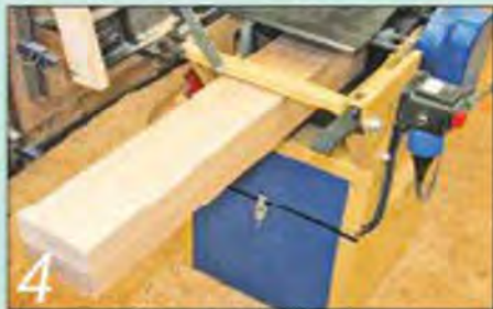
4 Plane, square up and dimension the legs to their finished sizes
