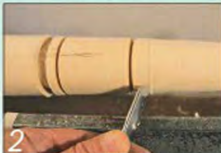
2 Start the V cut on one side of the bead position with the \frac{1}{2} in skew chisel
