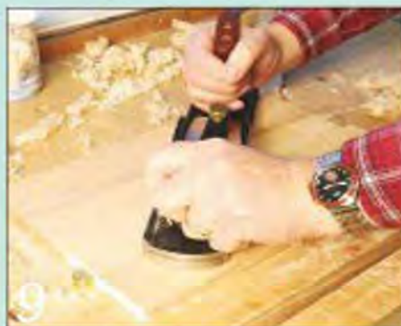
9 After assembling the door panel, I cleaned up the joints with a hand plane...
