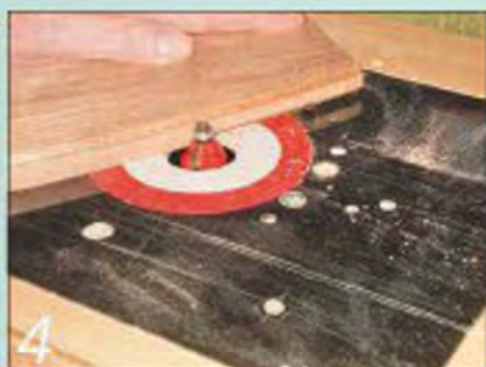
4 Use a small bowl cutter in the router table to profile the front edges of the shelves and sides
