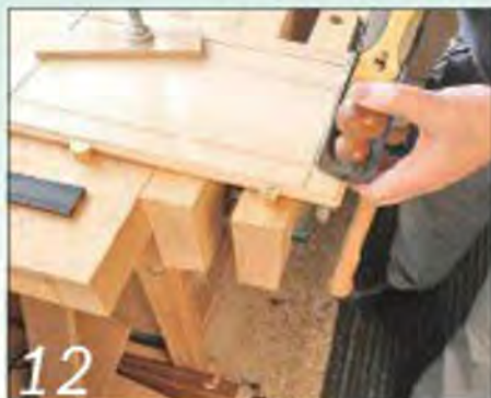
12 Cut the cross-grain chamfers first so any edge breakout will be removed later
