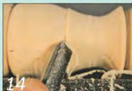
Repeat this process of shallow cuts on each side of the depression
