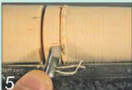
Continue the cuts on one side of the line and then the other in turn
