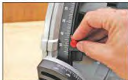
Plunge depths are set on this scale. The cursor rotates to include rail thickness if required
