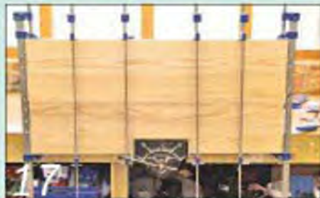
17 Rub-joint the pieces and cramp them all together tightly while the glue dries
