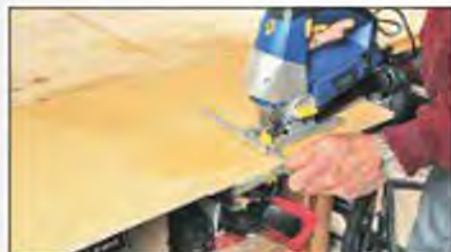
The sturdy side fence guides parallel cuts smoothly and accurately
