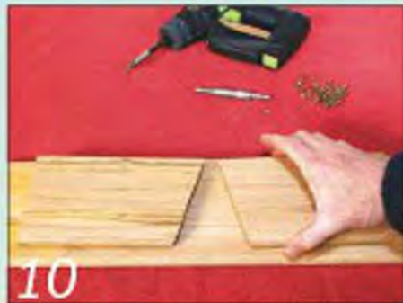
Now fold both legs down and check that they line up. Adjust their positions slightly if necessary
