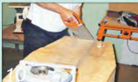
After cutting the end angles, the bottom is trimmed to size with a hand saw
