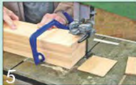
5 Mark and trim the legs to their finished length on the bandsaw
