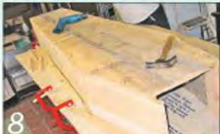
8 With the sides inverted and braced by supports, the bottom can be screwed on
