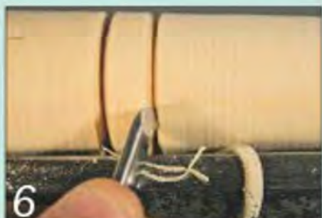
Carry on cutting until the two V cuts reach the required depth
