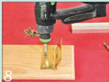
The inside of the hinge leaf is set at 85mm from the end of the seat board. Fix it with a single screw
