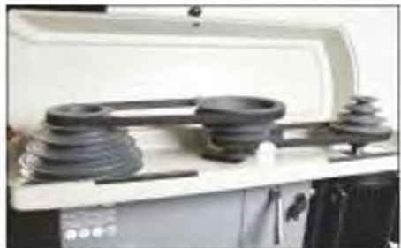
Both machines use the standard three-pulley-and-two-belt drive system
