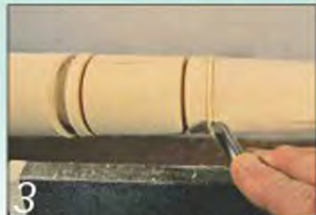
3 Move the tool to the other side and slice down the opposite side of the V cut
