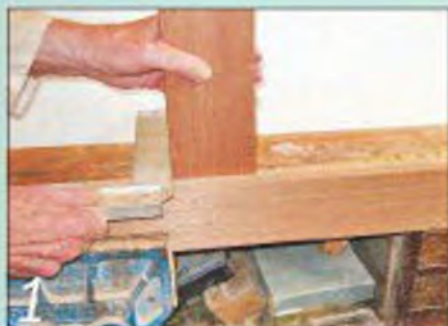
1 Mark the positions of the two shelves and the hidden cross rails on the side pieces
