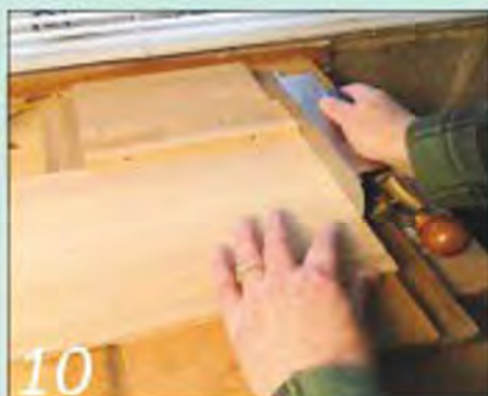
10 ...and shot the panel ends perfectly square on the shooting board
