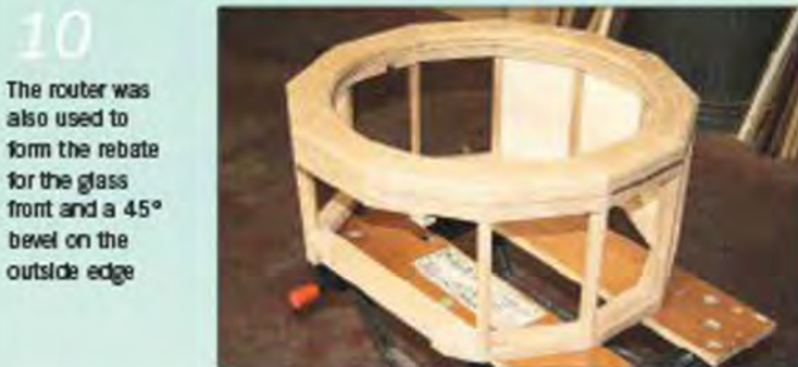
Once assembled, they were then cramped up and kept flat using the same method as step 5
