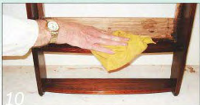
10 Apply the stain, followed by three coats of lacquer, and burnish the surface with a soft cloth
