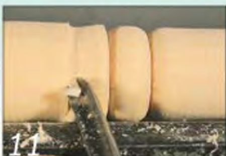
Hold the tool firmly on its side to start the cut and form the pear shape
