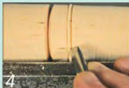
Note that the chisel is cutting only with the point of the tool
