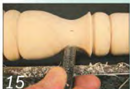
At the base of the hollow section, work with just the point of the tool
