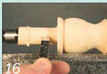
Form the straight dowel at the base of the candlestick stem with a parting cut
