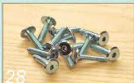
28 I chose 20mm M6 flange-head bolts to secure the wheels to the legs
