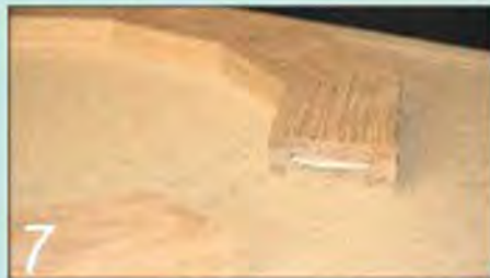
The 12 oak sections forming the hood door were glued together one by one using biscuit joints
