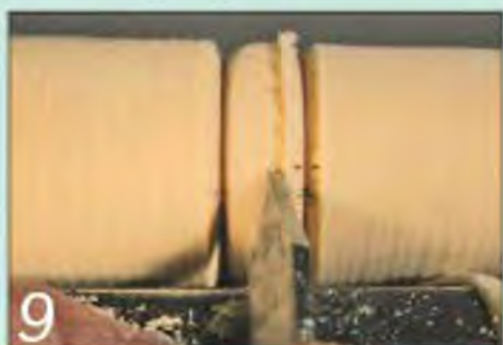
Reverse the tool angle and start cutting the curve in the opposite direction
