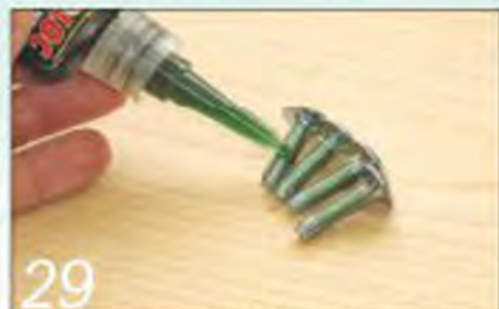
29 Apply thread lock fluid to the bolt threads to prevent them from working loose
