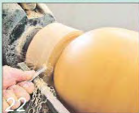
Remove the fixing screws and take gentle cuts to remove some of the scrap block...
