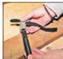
The post simply screws into the head. A shorter post is also available
