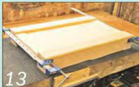
13 Begin the frame assembly by gluing up the two island side sections
