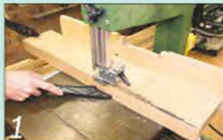
1 Rough-cut the wood for the legs slightly over-length using the bandsaw
