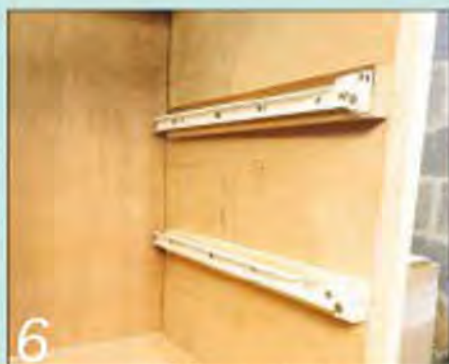
6 The runners need to be packed out on the hinge side to clear the door edge
