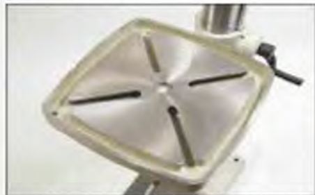
The tables have mounting slots and a coolant gutter around the edge for drilling metal
