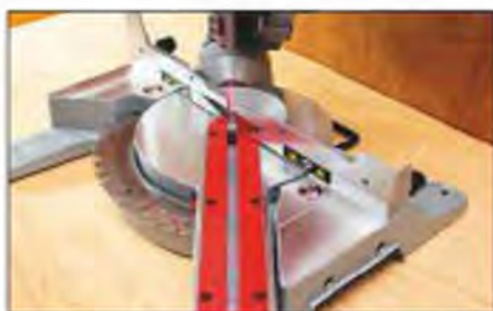
Slits in the lower guard allow the laser beam to spot the work for accurate alignment
