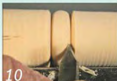
Complete the bead by working down into the depth of the second V cut
