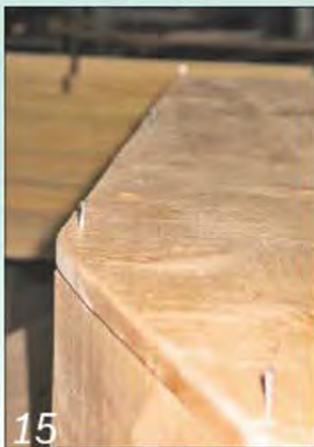
The top is pre-drilled to take the cut nails that will secure it in place
