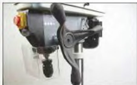
Both these machines both have a sturdy one-piece cast iron feed handle
