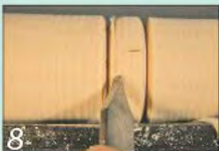
Move the cutting edge to one side with a slow-motion twist of the tool
