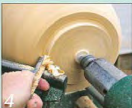
4 Square off the end and form a spigot about 130mm in diameter and 25mm deep
