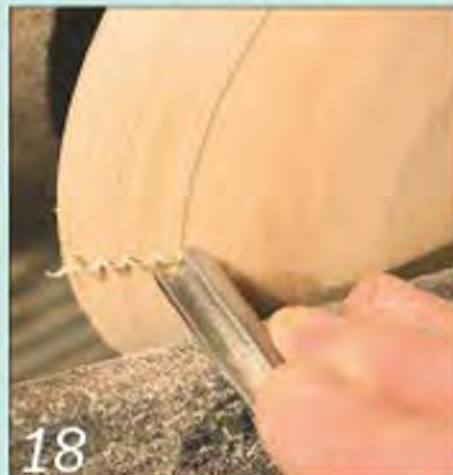
Notice how smoothly the gouge cuts when going away from the centre of the work
