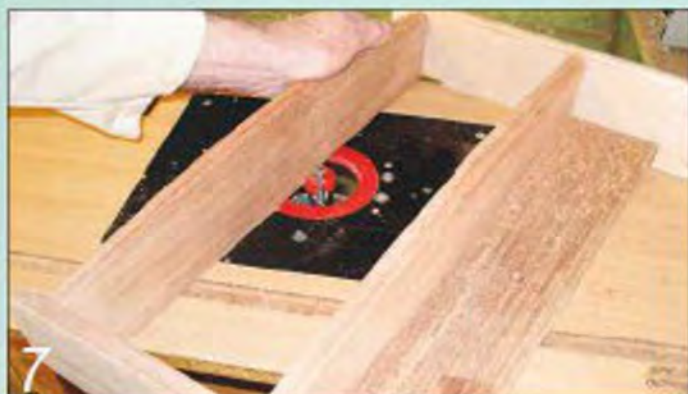
7 Form a shallow rebate round the edges of the lower section to take the plywood back panel
