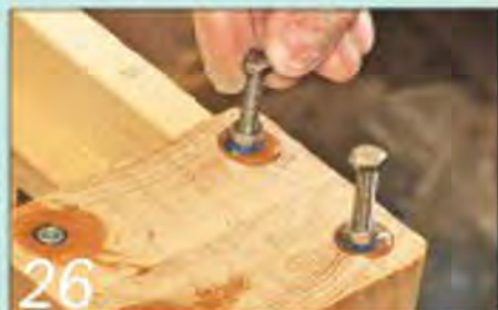
26 Squirt adhesive into the leg holes and insert the threaded sockets using a bolt to hold them
