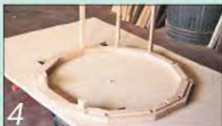
The 12-sided front is made from four sections, each containing three angled side pieces
