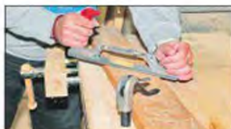
The work could move under pressure unless the leather pad is used
