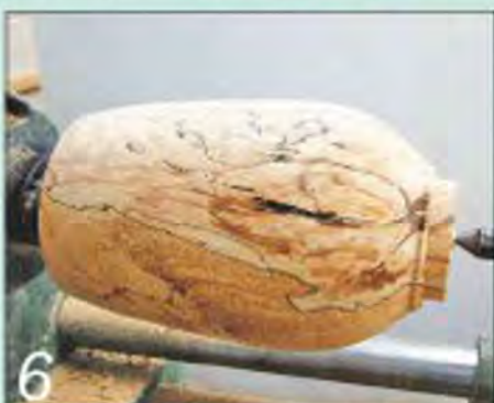
6 Aim for the widest part of the vase to be about a third of the way up from the base
