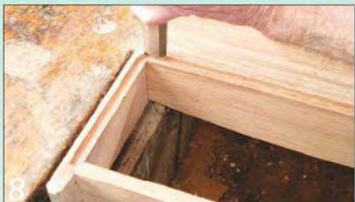
8 Use a sharp chisel to square off the rounded internal corners of the rebate left by the router
