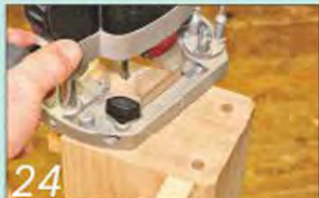
24 I started boring the holes for the threaded sockets using a straight router cutter...
