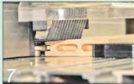
7 Rout the grooves in the rails to take the panels using the table router
