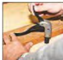
The cam lever swings through from back to front to increase the pressure
