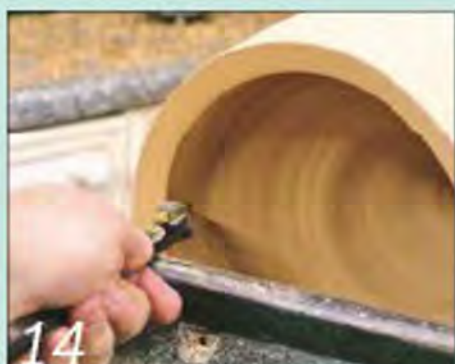
14 When you reach the bottom of the drilled hole, reduce the side wall to its final thickness
