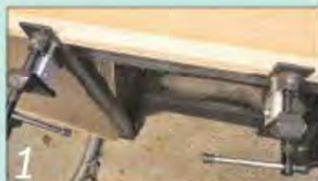
The edging strips were biscuit-jointed and then cramped to the boards
