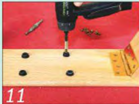
Fit the four rubber bumpers. These protect the legs and seat and allow the stool to be folded quietly
