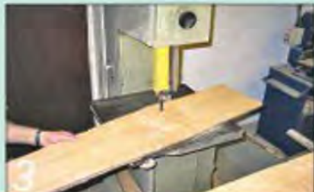
3 The plank shapes are cut on the bandsaw and then planed true afterwards
