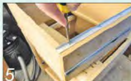
Aluminum angle, available from most DIY stores, makes good file rails
