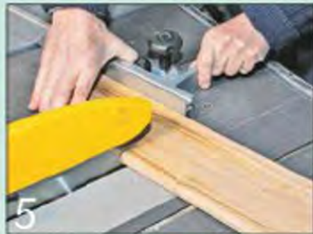
5 Use a table saw or mitre saw with the fence set to 15° to cut the angled ends of the legs
