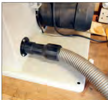
Dust extraction is essential. An ordinary vacuum cleaner will do for a benchtop bandsaw...
