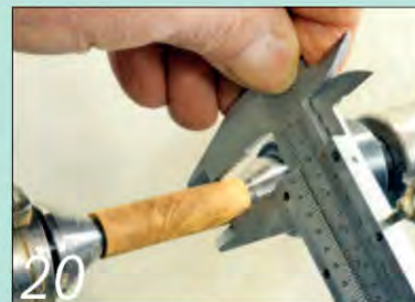
20 Turn it down to size – in his case, to two different diameters
