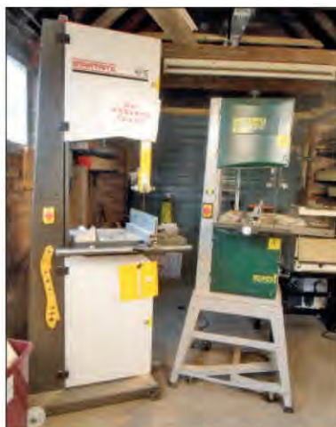
The industrially rated Startrite bandsaw (left) surprisingly has a smaller footprint than the bench-top machine on the right
