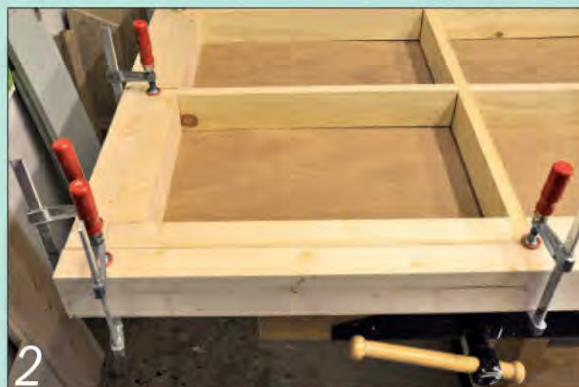
2 The plywood has little compressive strength, so I fitted additional lengths of wood along the front and side edges to withstand clamp pressure
