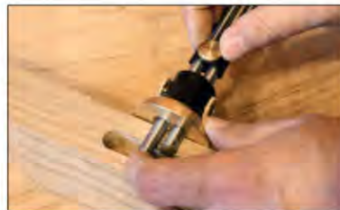
The shaft clamp slips over the two rods and locks them together via a thumbscrew
