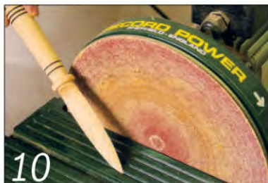
10 The rest of the shaping can be done on a disc sander, then finished by hand
