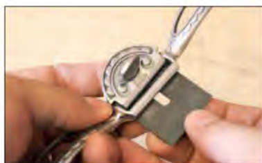
The PM-V11 blade slides into the body easily once it's been honed
