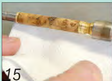
15 With the lathe off, apply the superglue quickly using some kitchen roll
