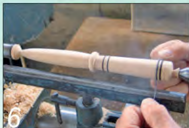
6 Run the lathe and apply a length of wire to burn in some decoration
