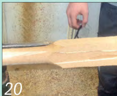
The final section involves turning the splices to the correct taper
