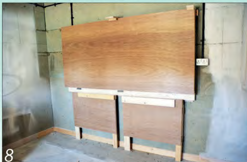
8 The bench takes up little space in the workshop once it's pushed up against the wall
