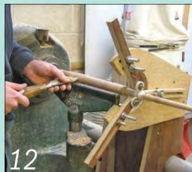
12 Version two of the steady supported the stock all the way round; much better!
