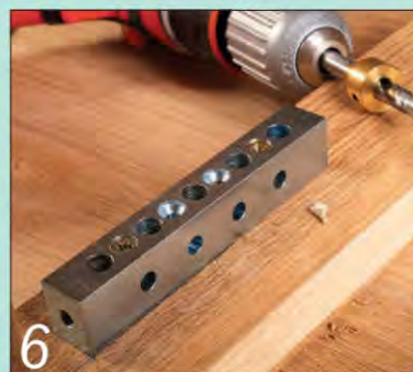
6 I used my Joint Genie for positioning the dowels accurately. Screw it to the cross rail
