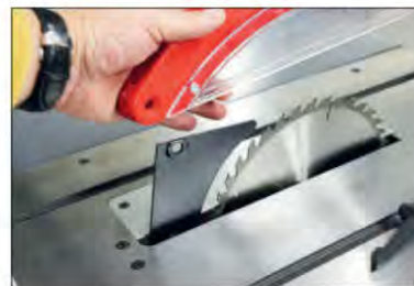
It connects to the decent sized riving knife with a single Bristol lever
