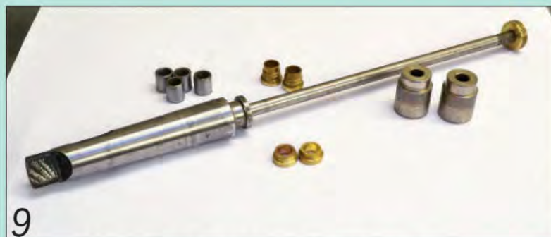
Pen mandrels are available with a variety of bushes to suit different pen kits
