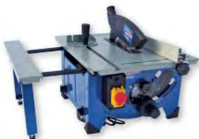
The side extension has adjustable feet that are used to get it level with the table
