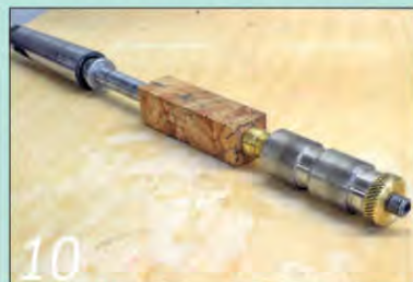
Fit the bushes, the blank and as many spacers as you need onto the mandrel
