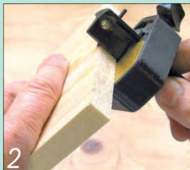
2 Set the gauge to just over the 15mm thickness of the timber
