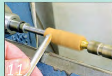
Run the lathe at high speed and turn the blank with a bowl gouge
