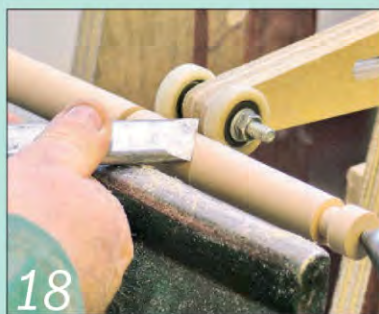
You can use a skew chisel instead to achieve a better finish
