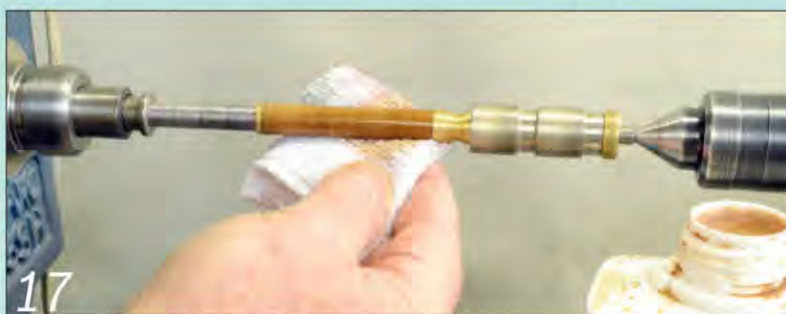
17 Finish the process by polishing the surface with burnishing cream
