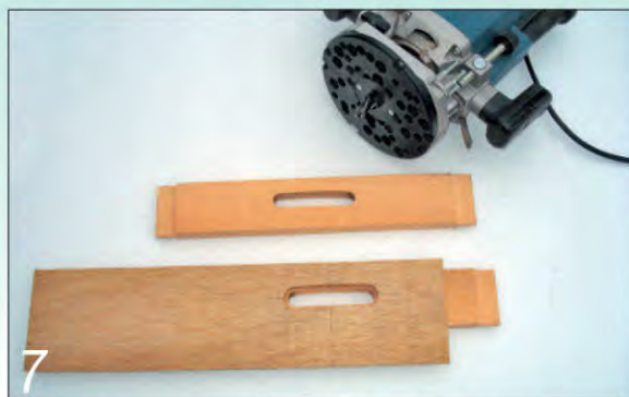
Then use a router and a template to trim the handle holes neatly
