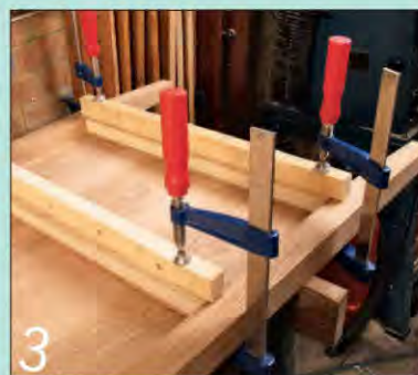
3 The convex cauls spread the clamping force along the whole length of the batten
