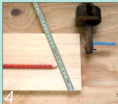
4 Divide the width by five by using a rigid ruler held at an angle across the face of the wood
