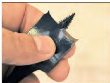
The spurs are positioned slightly inboard of the overall bit diameter
