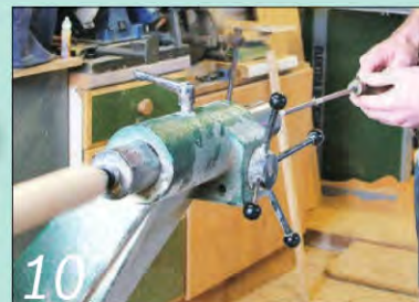
10 Drill the hole using an auger threaded in through the hollow tailstock barrel
