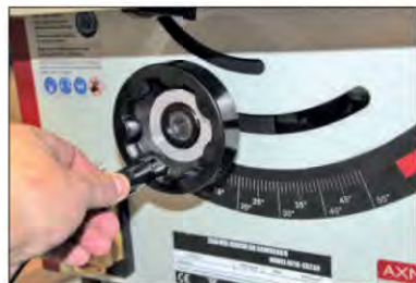
Although the blade tilt scale reads to 50°, the maximum tilt is actually 45°
