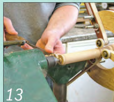
13 Turn the tip end down to a diameter of 10mm using a parting tool...
