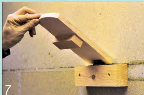
7 The smaller safety catch has a bigger overhang to make it easier to grab and push up when the bench is lowered
