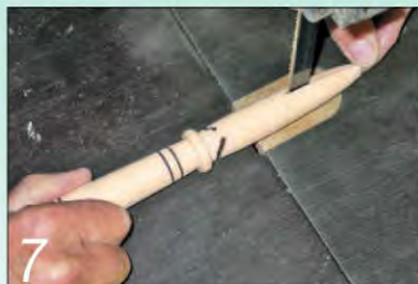
7 Cut off the waste and roughly shape the blade; I used my bandsaw
