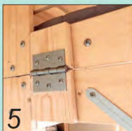
The top bunk hinges are fitted on spacer pads next to the L-posts
