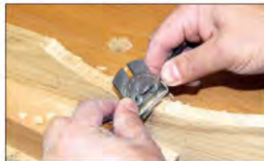
You can use a spokeshave by pushing or pulling it, working with the grain
