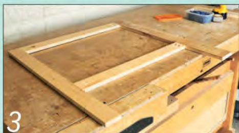
3 The legs are simple A frames, assembled with pocket-hole screws. Once clad with ply on each side they became very rigid
