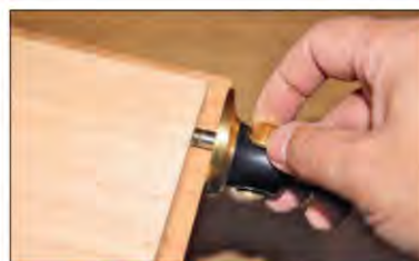
The flush-fitting outer wheel can be used to gauge and transfer rebates
