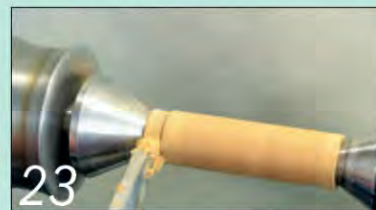
23 Then remove the end section next to the cone carefully using a parting tool
