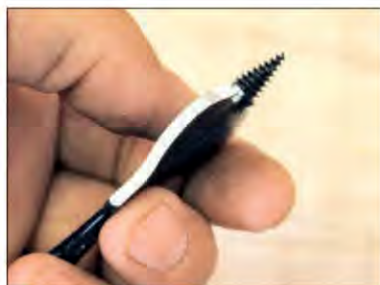
The edges of the bits have a defined wave profile when viewed side on
