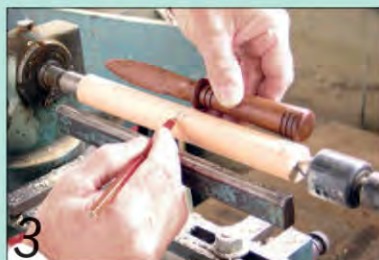
3 Mark the position of the handle, guard and blade, with a bit to spare each end
