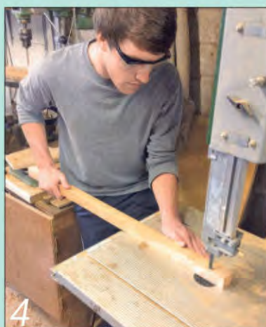
4 Cut the tapers on the bandsaw, working on the waste side of the lines
