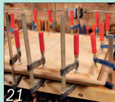
21 A plywood panel gives a neat flat top and strengthens the cornice sub-assembly
