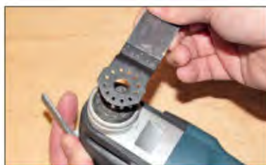
The accessories can be fitted at an angle to suit the work you're tackling
