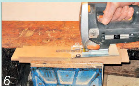
Drill out the handle holes and cut out the waste using a jigsaw
