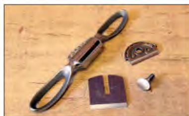
Just four components make up this impressive little spokeshave
