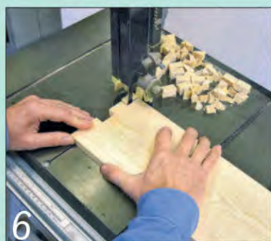
6 These fat finger joints can be formed with care using just the bandsaw
