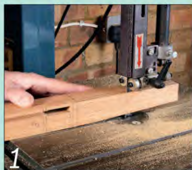
1 Cut the taper on the legs with the bandsaw and clean them up with a plane
