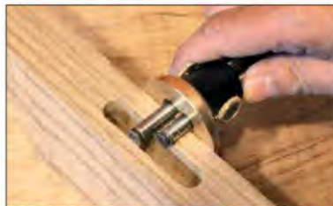
It's particularly well suited to gauging and transferring mortise widths
