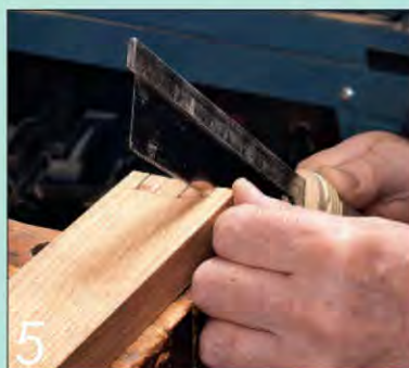
5 Cut the dovetail recesses with hand tools in the traditional way
