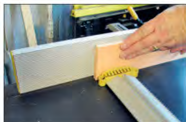
Initial planing involves two distinct functions: the first is overhand planing, using a fence to get a square edge...
