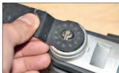
Releasing a lever allows the split pin to open and secure the accessory
