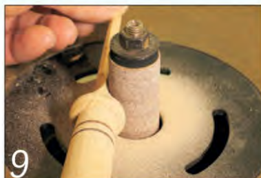
9 Use a bobbin sander to clean up the shape round the base of the blade
