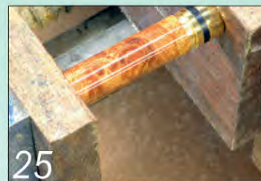
25 A bench vice is ideal for pushing the pieces together to finish the pen
