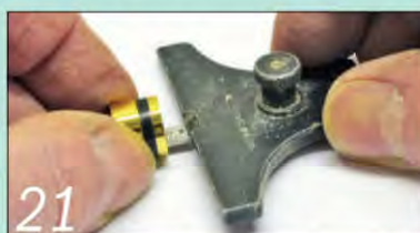
21 I measured the overlap required and reduced it by 0.5mm for safety
