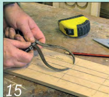
15 Use a scale drawing and callipers to set the correct diameter at 100mm intervals
