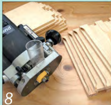
8 Cut the back rebates with the router. The rebate is stopped on the long sides.
