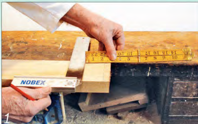
Mark out the joint positions with the legs held together in a vice
