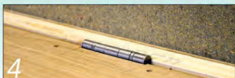
4 The heavy-duty steel hinges project above the workbench, but will be concealed by the sacrificial sheet of mdf
