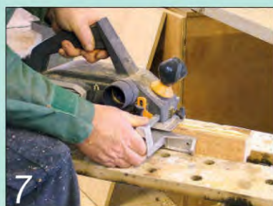
7 Use a power planer to bring the stock back to 35mm square
