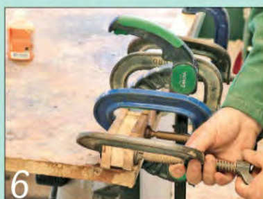
6 Glue and cramp the first two splices to the tapered faces of the butt
