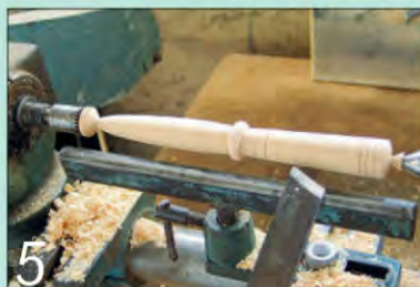
5 Once the blade is shaped, cut some shallow grooves in the handle with a skew chisel
