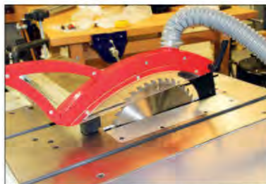
The crown guard is well made with a built-in handle, and is easy to adjust
