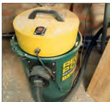
...while this drum-type extractor can be adapted for 32mm vacuum or 100mm extractor hoses
