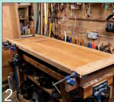
2 Gluing up each side frame took up the whole of my bench top
