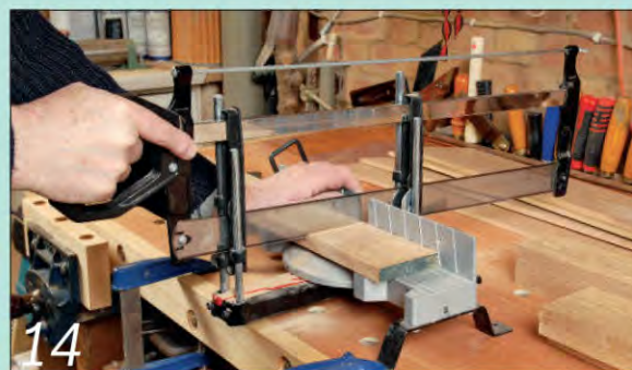
Trim the back panel frame components to length on the mitre saw for accurate results
