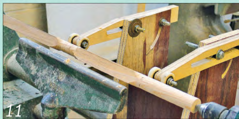
11 My first home-made lathe steady let the stock ride up the wheels
