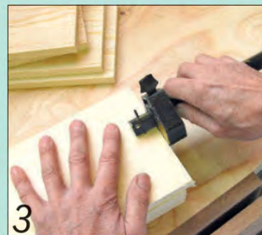
3 Strike a gauge line on each face at both ends of all the components
