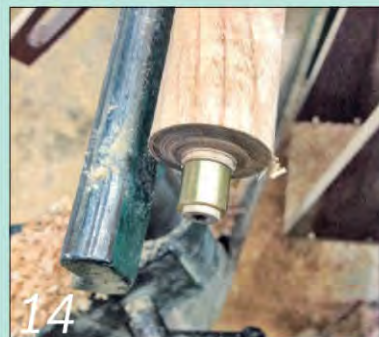
14 ...and test the fit of the brass ferrule. Sand the tip for a better fit
