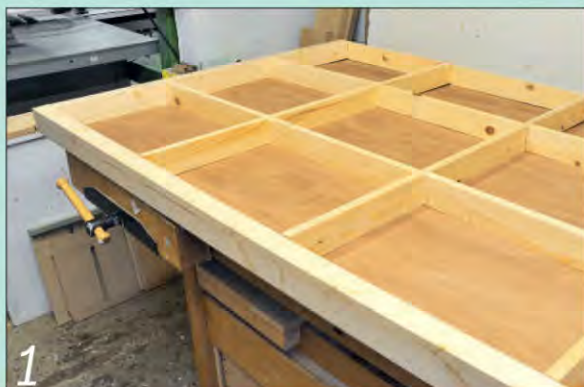
1 I laid one piece of 6mm plywood on the bench and loosely laid out the frame and the internal braces of the torsion box
