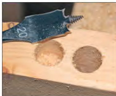
The resulting holes are relatively clean but have minor tearing at the edge
