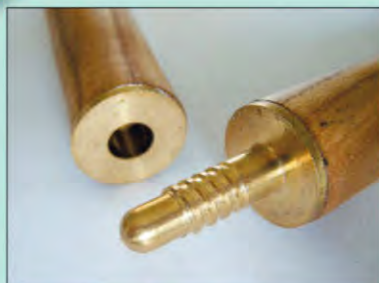
Glue in the two parts of the brass joint with epoxy resin adhesive
