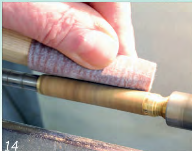
When the glue has dried, turn the bump level with the rest of the blank and sand it smooth
