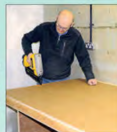
7 The smaller safety catch has a bigger overhang to make it easier to grab and push up when the bench is lowered
