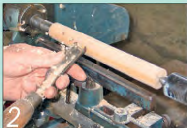
2 Turn it a straight cylinder with a gouge to about the finished size
