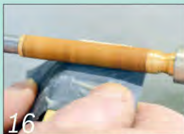
16 Sand it, apply more glue, sand it again and then lubricate it with wax
