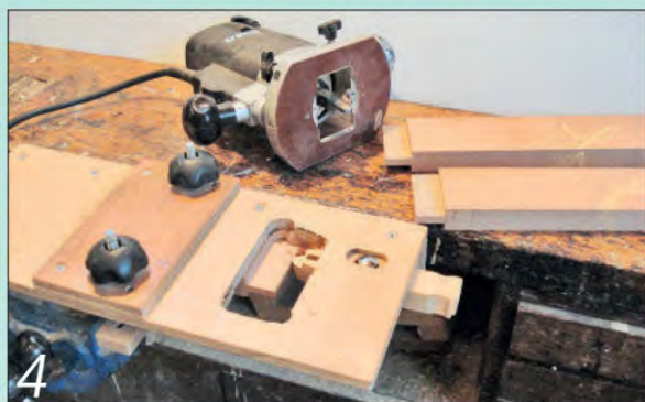
I cut the tenons on the rail ends using a shop-made jig and router
