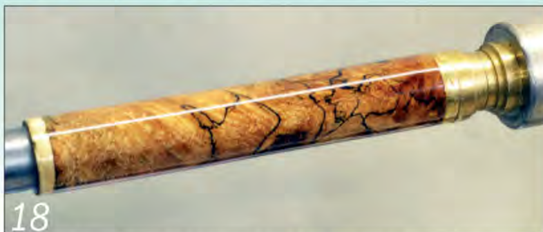
18 The result is a smooth, glossy and hardwearing surface finish to the pen body
