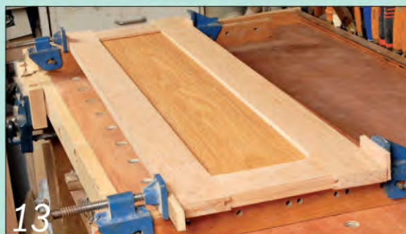
Gluing up the doors is a more manageable operation than assembling the side panels
