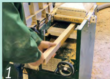
1 Use a planer thicknesser to prepare the two sections of ash stock
