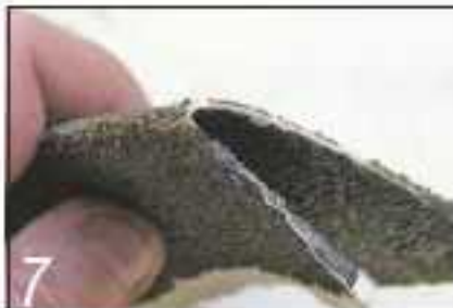
7 Paper-backed abrasive is less flexible and cracks when it's folded
