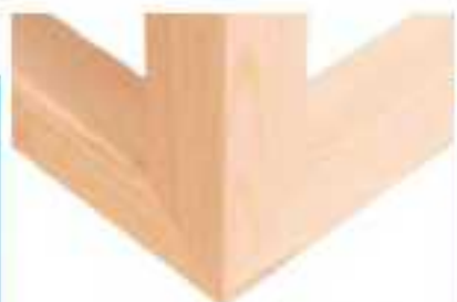
The completed joint shows all the parts fitting closely together as three-dimensional mitres with no end grain visible anywhere
