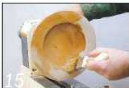
15 Apply a liberal coat of oil with a brush and let it soak in for a while
