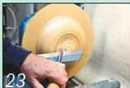
Remove most of the dovetail spigot to leave a slightly raised centre
