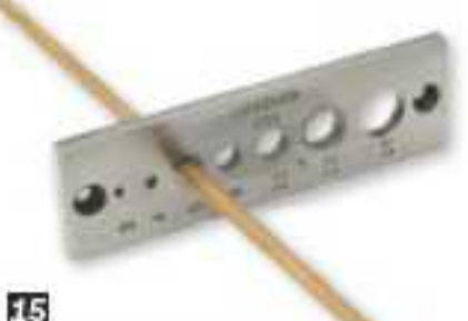
15 If you want to use wooden spacers, cut a length using a dowel plate
