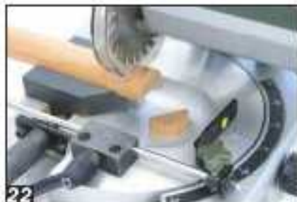
22 Hold the piece on the saw table and cut off a series of 8mm slices
