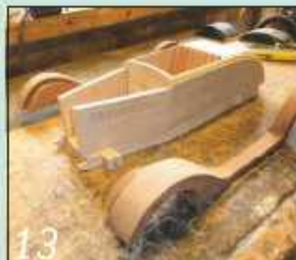
13 Angle the rear edges of the engine side panels and stick them in place
