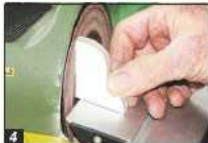
4 Set the disc sander table to 10°. I use a little plywood setting jig for accuracy
