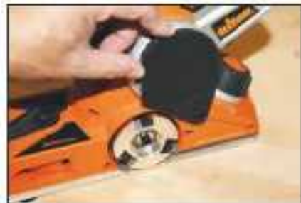
For unlimited rebating this guard lifts away from the side of the planer
