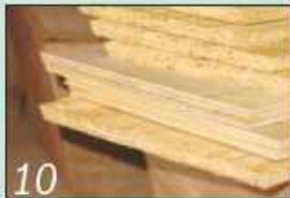
10 Cut base panels to size and plane down the edges at the 75° angle all the way round
