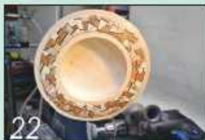
Power-sand the interior of the bowl down to 400 grit, ready for sealing
