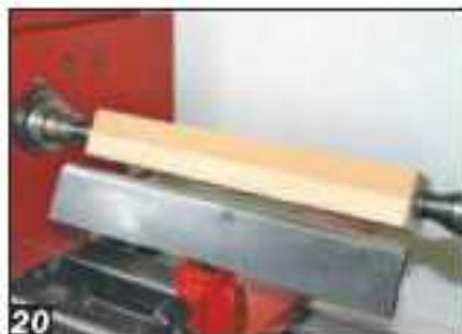
20 Mark centres on the ends of the blank and mount it between centres
