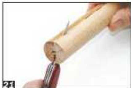
21 Turn the blank to a 33mm diameter cylinder and separate the halves
