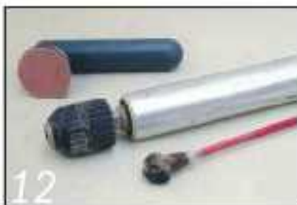
12 There are lots of the aids on the market such as Extend-A-Sand to help internal sanding
