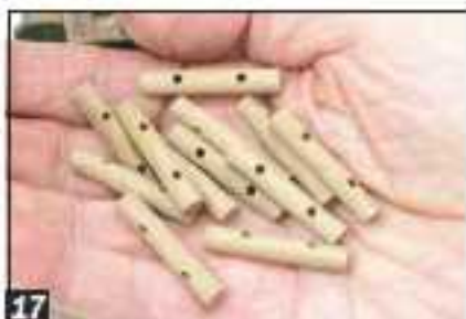
17 The finished spacers - shown here in walnut - are now ready for assembly
