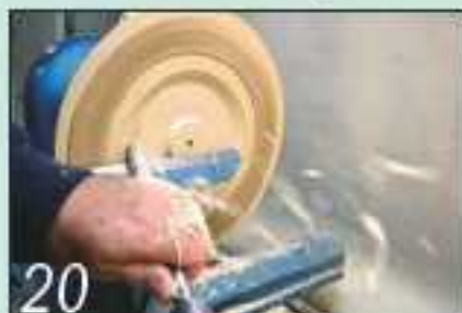
Complete the bowl shape by hollowing out the centre with a bowl gouge
