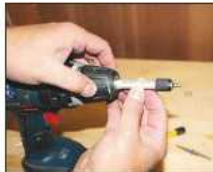
You can use the Xtreme version as a hex screwdriver bit holder
