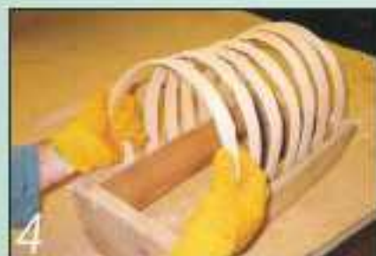
4 I bend the steamed strips freehand and place them in a dummy trug to cool down
