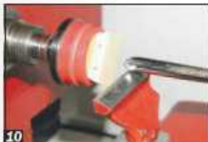
10 Mount the glue chuck in the lathe and turn its top to a gentle curve
