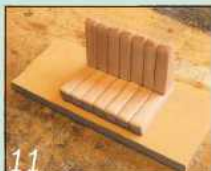
11 Round over the seat and back edges to create a soft curved profile
