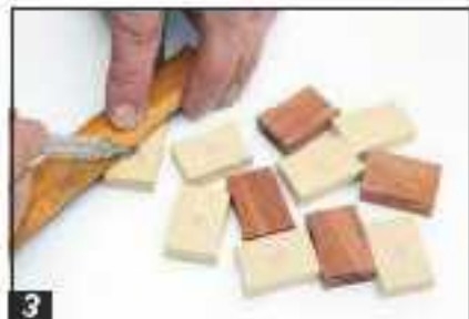
3 Mark the precise centre of each blank and centre-punch a hole there
