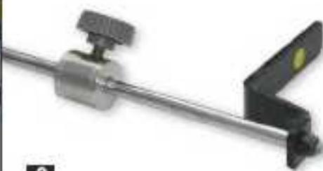
2 I machined this simple stop to fit on the Proxon chop saw's length stop
