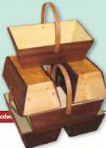
14 Drill pilot holes for the machine screws, then apply glue to secure the handles...
