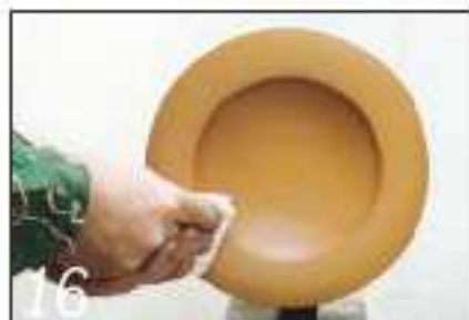
16 Burnish the drying surface with a paper towel. Note the position of the hands
