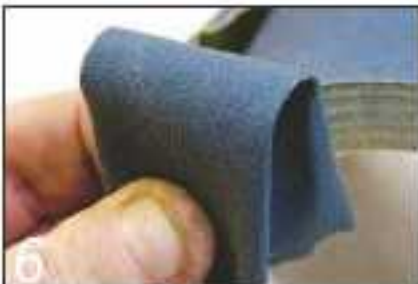
6 Cloth-backed resin-bonded abrasive is the best type to use for turning
