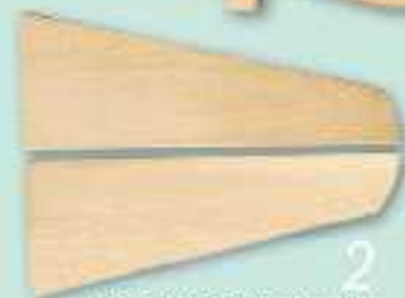
2 The bonnet is in two parts; the join will be concealed by a trim bead
