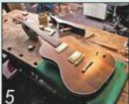
5 Small-scale projects like this electric guitar are equally suitable for this versatile material. However, the density and hardness of Kebony might restrict its use in acoustic instruments to areas like the neck.
