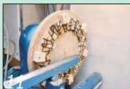
Remove the hardboard disc and cut the inner edge of the band to its marked line
