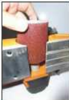
For unlimited rebating this guard lifts away from the side of the planer
