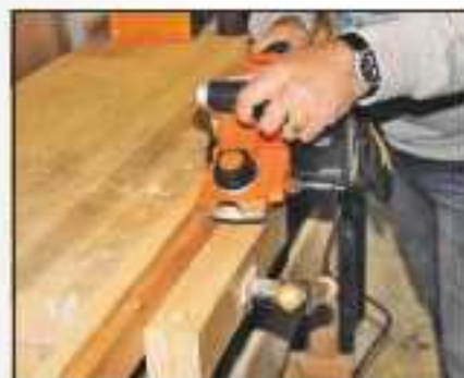
The unlimited rebating function works well for cutting deep rebates...
