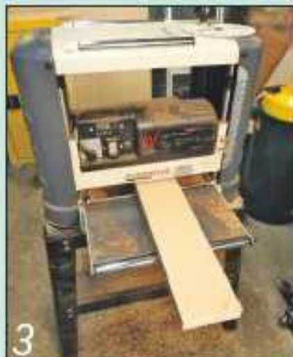
3 The machine shop also gives me space for a dedicated thicknesser, saving a lot of dismantling and re-setting time
