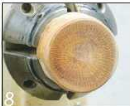
8 These small cracks are caused by over-zealous sanding generating localized overheating
