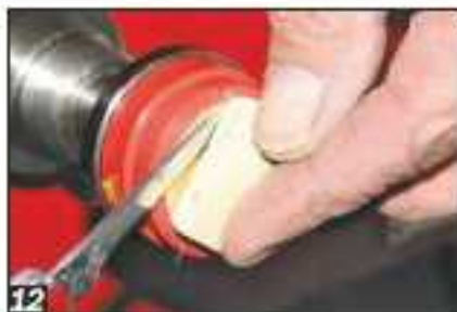
12 Prise the blank off the glue chuck and remove any adhesive residue
