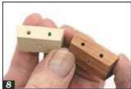
8 Here are two chamfered and drilled segments - one in each of the woods I'm using
