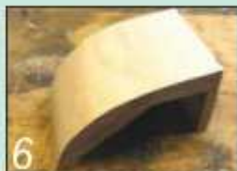
6 The boot is made in sections for economy rather than from a solid block
