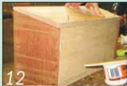
12 Put glue on the edges of the base panel, drop it in, tap it down and pin it in place all round
