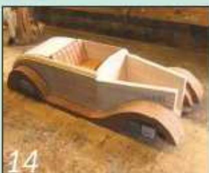
14 Offer up the two running board assemblies and mark their positions on the bodywork
