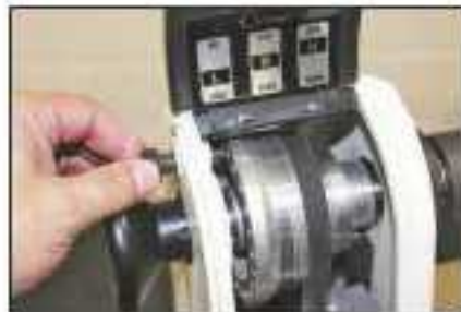
The easily accessible top pulley has a 24-position indexing function with a stop pin
