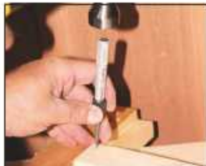
The counterbored tip grips the pin and performs as a good punch should
