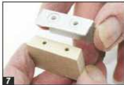
7 This simple drilling guide is made from a short piece of aluminium angle
