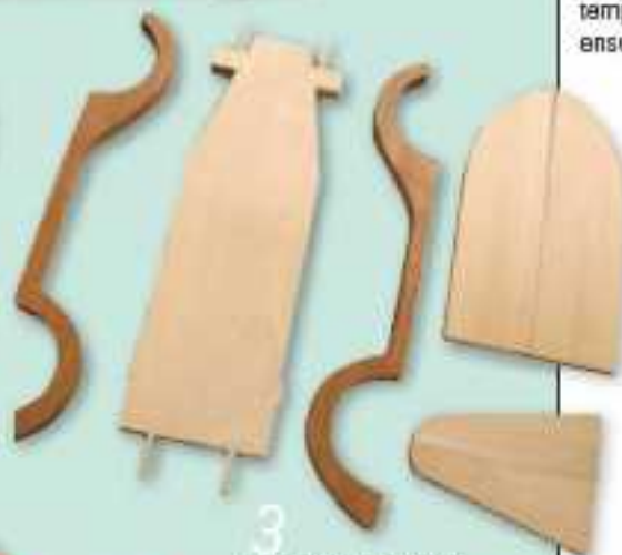
2 The bonnet is in two parts; the join will be concealed by a trim bead
