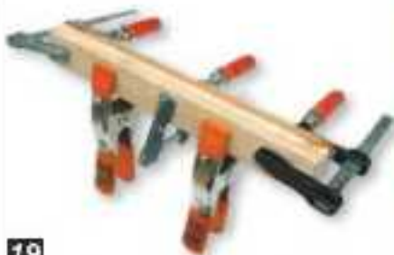
19 Glue and cramp the two lengths of wood together with a paper joint between them
