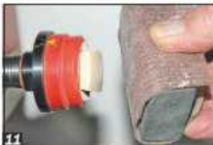
11 Use a pad of abrasive to sand the curved top and its four corners smooth
