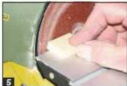
5 Sand a bevel on the four edges of each segment. Keep your fingertips away from the disc!
