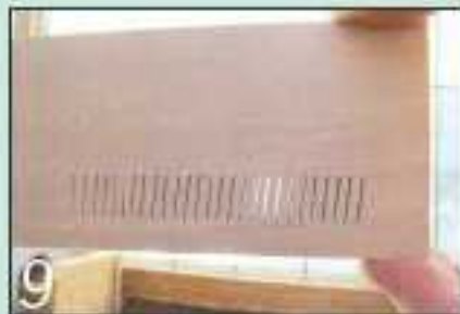
9 Each engine side panel contains 27 carefully scrollsawed cooling vents
