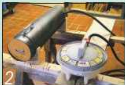
2 My simple steaming rig consists of a sealed tube and an old wallpaper stripper
