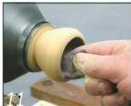
11 Hold the abrasive with a single finger when sanding inside small objects
