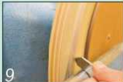
9 Use a 3mm parting tool to cut the outer edge of the band to a true circle
