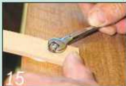
15 ...before fitting a washer to each screw and tightening up the fixing nut
