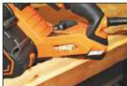
With the bag fitted, the extract chute soon got clogged with chippings
