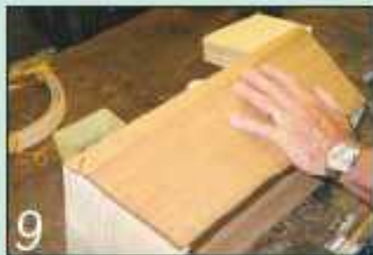
9 Align the second side panel with the ends and drive in the panel pins to secure it
