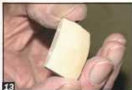
13 Repeat the turning and sanding process to complete the full set of blanks required
