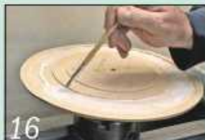
16 Apply PVA glue sparingly with a brush to the band and in the recess
