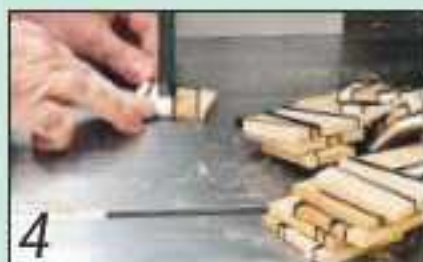
4 Cut the strips into shorter lengths and re-cut them lengthways
