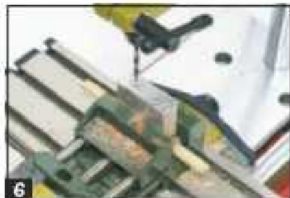
6 Drill two 2.4mm diameter holes through the short end of each segment
