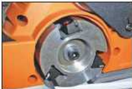
The Triton planer has a unique three-knife cutter block for planing work
