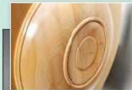
Power-sand the interior of the bowl down to 400 grit, ready for sealing
