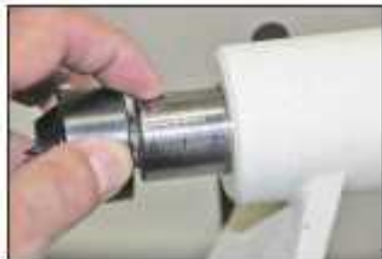
The tailstock is graduated and has 64mm of travel which is easily selected with a flywheel
