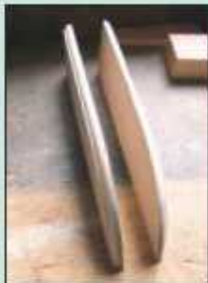
6 The boot is made in sections for economy rather than from a solid block
