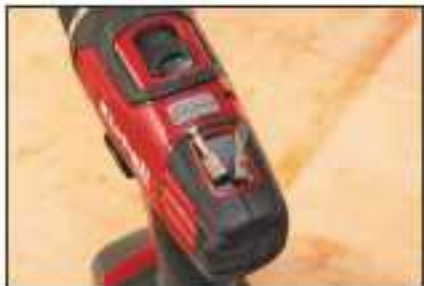
There's a useful magnetic pad on top of the drill for holding bits
