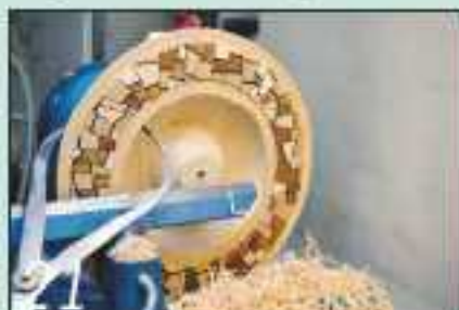
Use callipers to check that the wall thickness is even as you work
