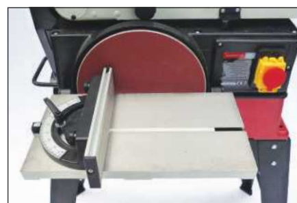
The disc sander table is a generous size. The NVR switch is sited next to it
