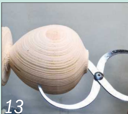
Use double callipers to check the wall thickness regularly as you work
