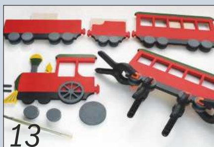
13 Glue the wheels onto the train, with the 3mm thick one to the front and the 6mm one on the back
