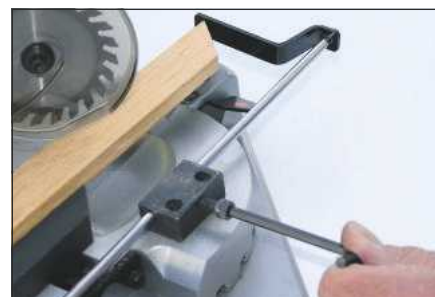
The length stop can only cater for work between 150 and 250mm long
