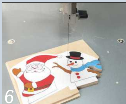
6 Stick the other patterns to a two-layer stack of 3mm ply (held together with double-sided tape) and cut them out
