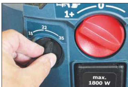
Set this three-position dial to match the hose diameter and ensure correct airflow
