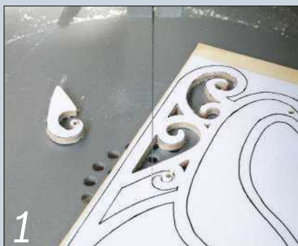
1 With the paper pattern attached to 3mm ply, cut out all the internal sections within the sleigh first
