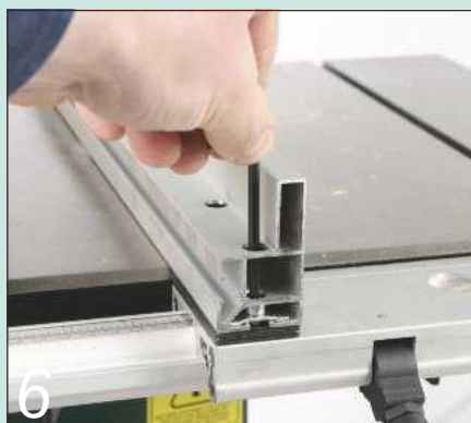
6 Slacken off the fence's locking bolts so you can adjust it for any misalignment
