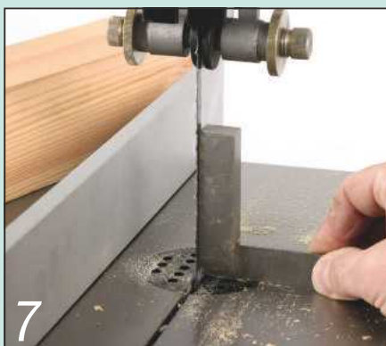
7 Check that the table is dead square to the blade using an engineer's square
