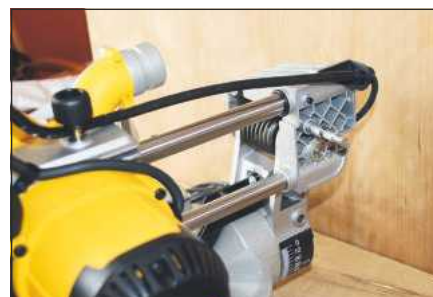
The internal forward-facing bars mean there are no rear projection problems
