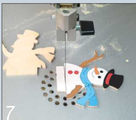
7 Separate the two 3mm thick layers and cut the tab off the layer with the pattern
