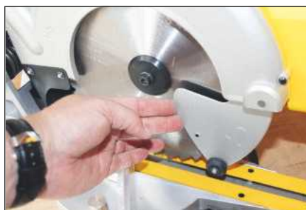
The guarding on the 250mm diameter blade is all metal and very robust
