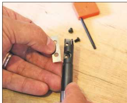
The twin-edged blade slides into a slot in the shank of the cutter...
