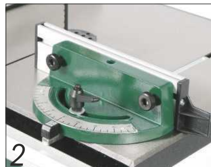
A mitre guide isn't essential, but a substantial one like this does make the job easier
