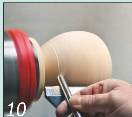
Shape the outside down towards its final thickness with a bowl gouge
