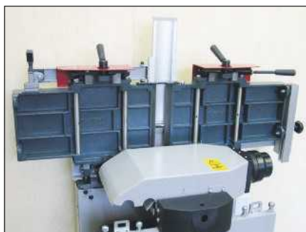
The extractor hood and guard covers the cutter block in thickening mode
