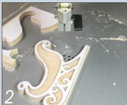
2 Stick this layer to two 6mm thick blanks and cut around the sleigh's perimeter. Then separate the three layers
