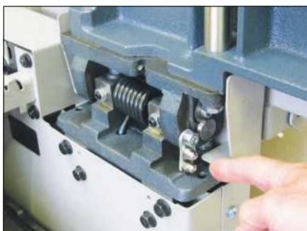
The tables are spring-assisted and lock into place with the minimum of effort
