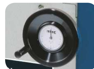
Large handwheel with digital read-out table setting plus 1/10 th mm final dial setting for super-fine finishing cuts.
