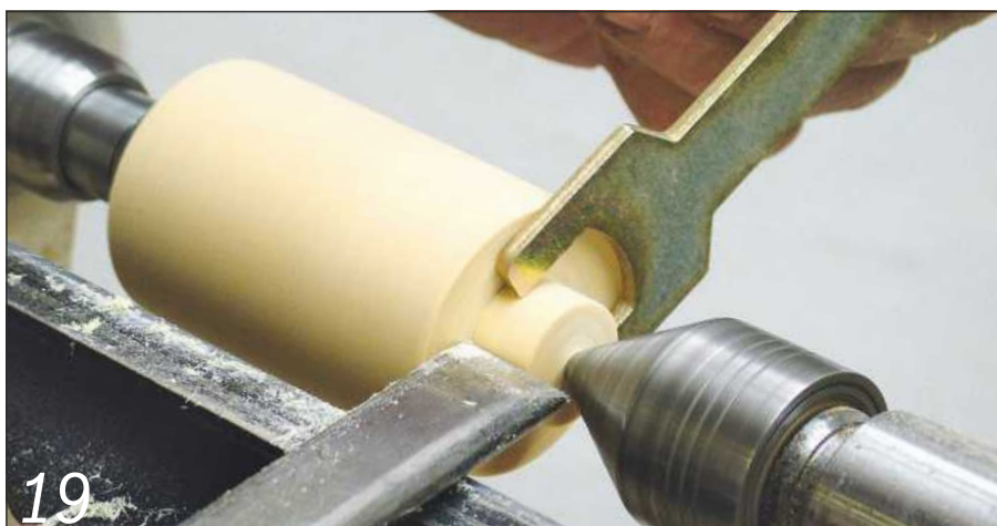
Open-ended spanners can come in handy for checking the diameter of turned tenons
