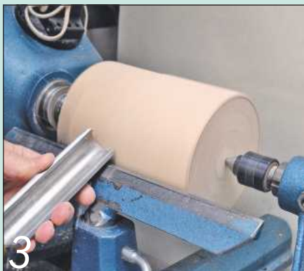
3 Turn it down to a smooth cylinder using a spindle roughing gouge
