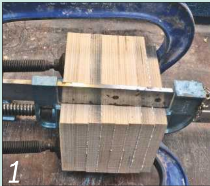
1 Glue the plywood offcuts together, cramp the block securely and leave it to set overnight
