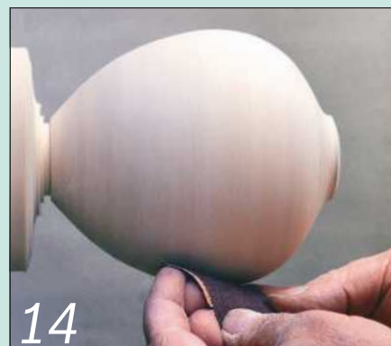
Sand the outside of the hollow form smooth with 80-grit abrasive paper
