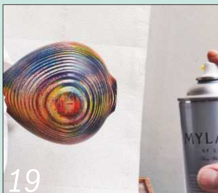
19 Sand and seal the form, then apply several coats of acrylic lacquer
