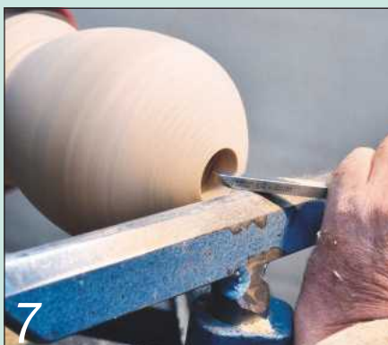
7 Enlarge the hole using a round-nosed scraper; mine is home-made
