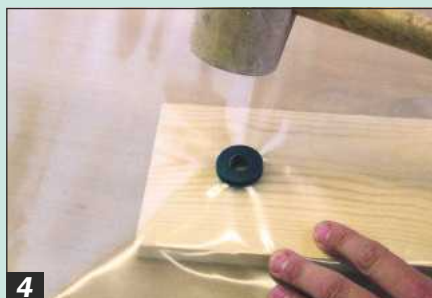
4 Reverse the valve housing and snap the two halves together. A soft hammer might help
