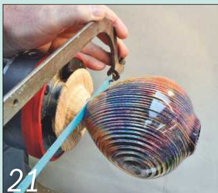
21 Turn the base down to a narrow section and cut it off with a fine-toothed saw
