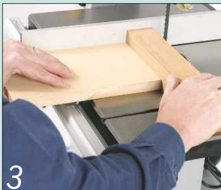
3 If you don't have a mitre guide, use a right-angled piece of thick mdf as a fence
