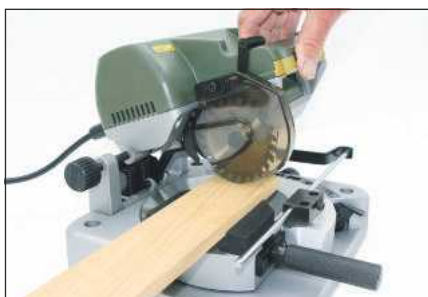
The saw is designed for one-handed operation; keep the other one safely out of the way
