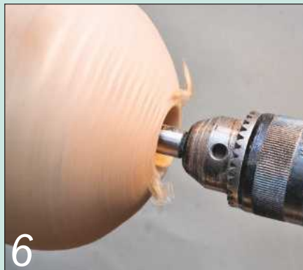
6 Start the hollowing by boring a hole using a large Forstner bit
