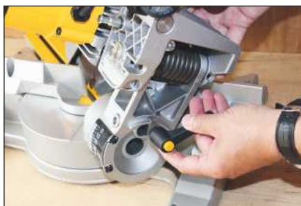
The head is locked with this Bristol lever and can be tilted to 48°
