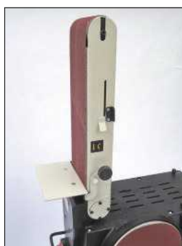
The disc sander table is a generous size. The NVR switch is sited next to it
