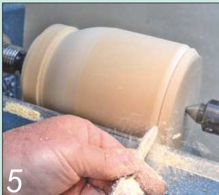
5 Begin shaping the outside of the blank with a small bowl gouge
