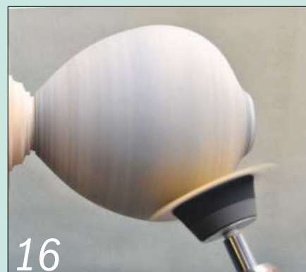
Power-sand the surface with 120-grit paper to remove excess stain
