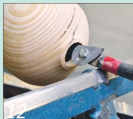
...and this broad-bladed scraper will help to smooth the rest of the interior
