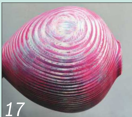
17 Apply red dye next, allow it to dry and power-sand it with 180-grit paper
