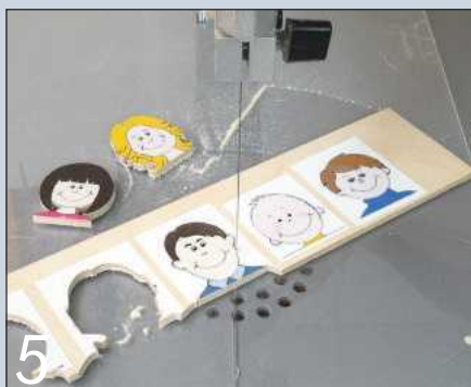
5 Enlarge and photocopy the passenger faces, stick them to a strip of 3mm thick ply and cut carefully round each one
