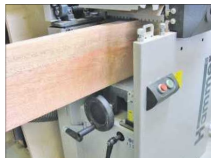
The thickening table is raised and lowered in the customary handle turning way. Note lock
