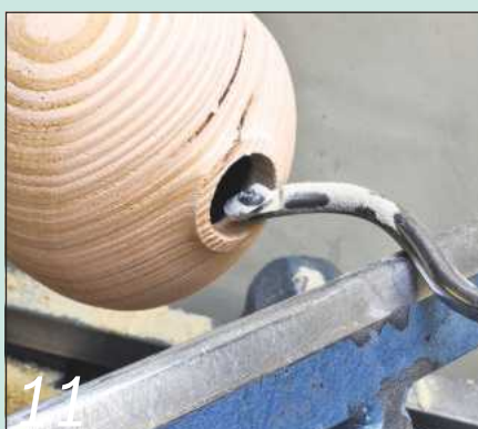
A swan-necked scraper will smooth out the inside of the shoulders...
