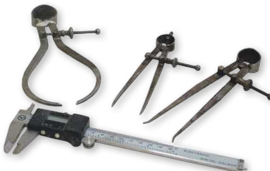
Callipers are useful for measuring wall thicknesses, while dividers can check workpiece diameters
