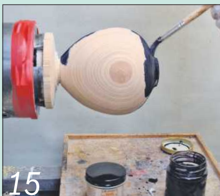
With the lathe stationary, brush on a coat of light-fast black dye
