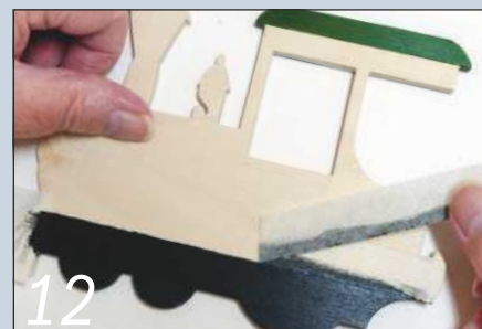
12 Mask off the roof and undercarriage and paint them. Then remove the masking tape and paint the central areas red
