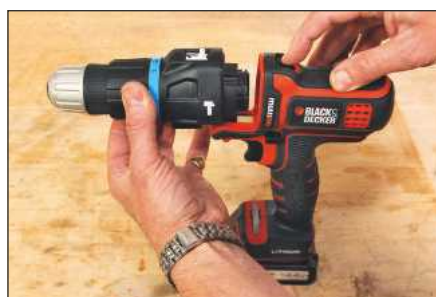
Press the button on the top to release and replace the accessories
