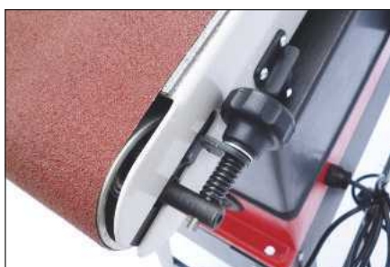
The front roller on the belt sander is adjustable for tracking purposes
