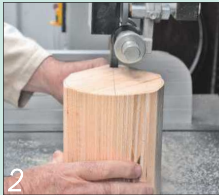
2 Reduce the blank to a rough cylinder by trimming it on the bandsaw
