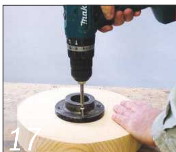
A faceplate is screwed to the workpiece – for example, as a way of holding this bowl blank for its initial shaping
