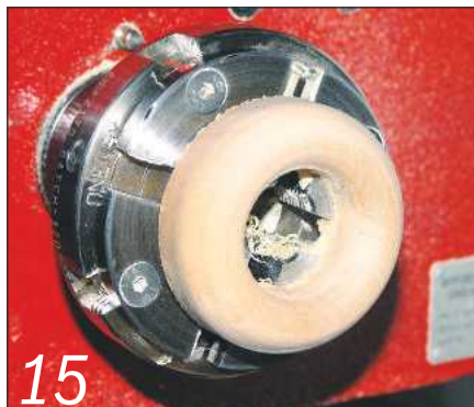
15 ...or can expand into a dovetail recess or other internal opening in the workpiece
