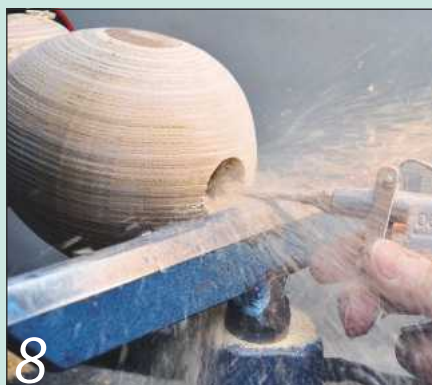
8 Remove the debris regularly; I do it with a puff of compressed air
