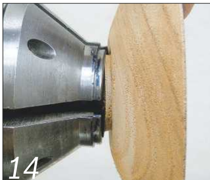
14 Dovetail jaws are the most common, and can clamp down onto a matching spigot...
