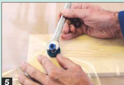
5 Screw the valve itself into place in the housing with a 14mm spanner and connect the hose
