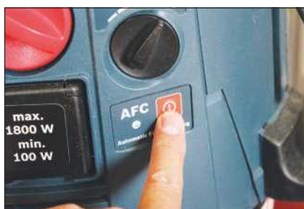
The automatic baffle filter cleaner is engaged with this power button
