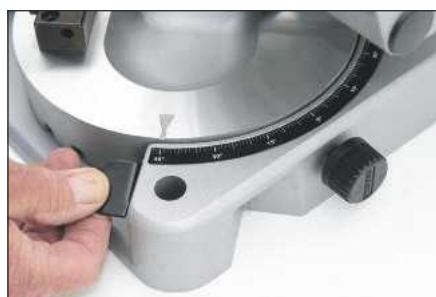
The circular baseplate rotates through 45° to the left or right
