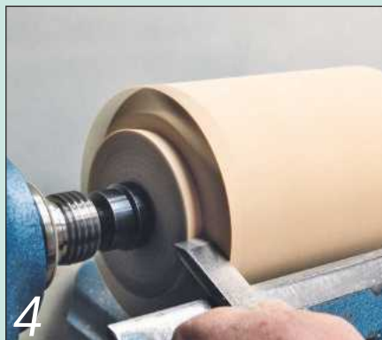
4 Use a skew chisel to cut a dovetail spigot on one end of the blank
