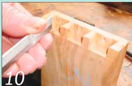
10 Bore out the bulk of the waste and trim to shape with a sharp chisel
