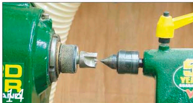
14 When the headstock is returned to its normal position, it's important to check that the spindle lines up accurately with the tailstock
