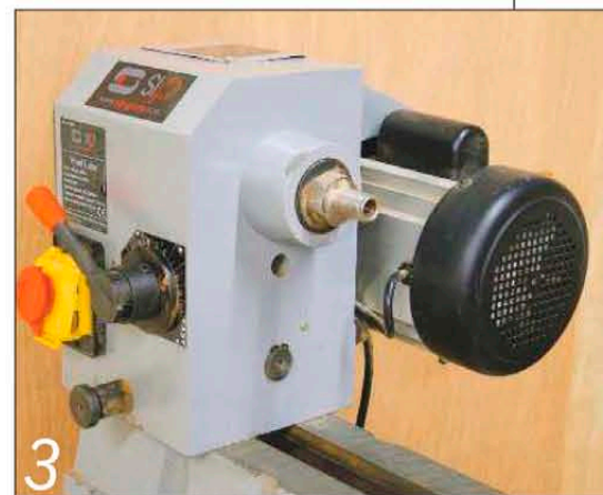
The headstock houses the lathe's spindle, plus on-off and speed-change controls. On some models the headstock can swivel round
