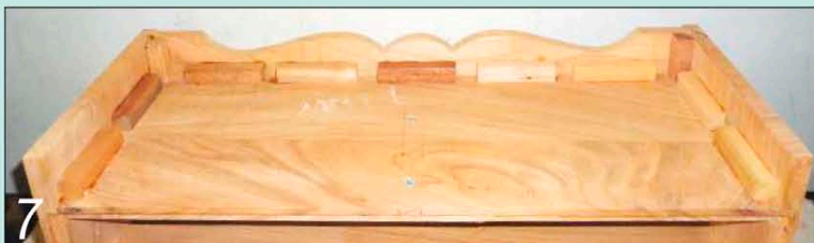
7 Fit the plinth in place and add glue blocks all round the underside
