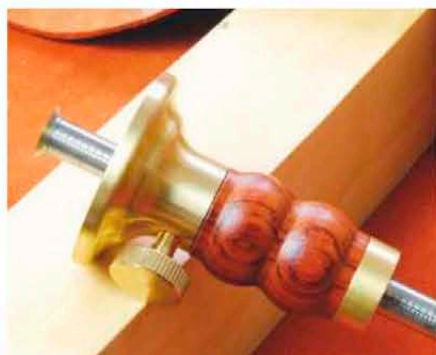
The scale etched on the stainless steel shank is a useful guide to positioning the gauge body
