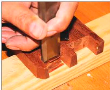
The chisels take a fine edge that's ideal for paring work
