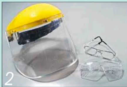
2 Safety gear must include goggles, and preferably a face shield as well
