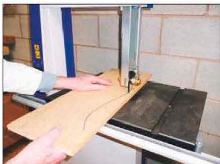
The minimum blade width is 6mm – ideal for cutting shallow curves like these
