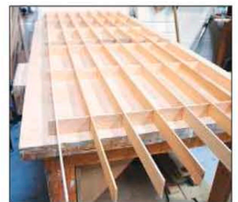
2 A lattice structure was used to create maximum strength with minimal amounts of material
