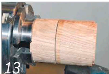
13 The fit should be tight enough for the box body to grip without support
