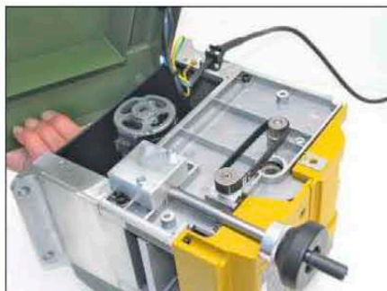
Removing the other cover gives access to the height adjustment system
