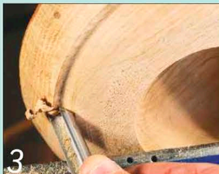
3 Use the gouge in the opposite direction to form the top surface of the scoop's handle
