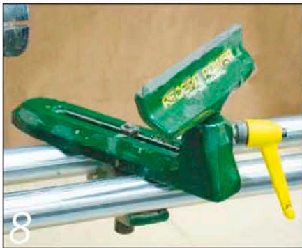
8 The toolrest sits in the toolpost, and can be swivelled and adjusted in height to give a wide range of working configurations
