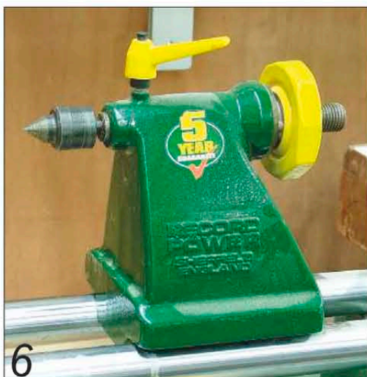
The tailstock is designed to slide along the bed bars, and is held in the required work position with a clamping mechanism
