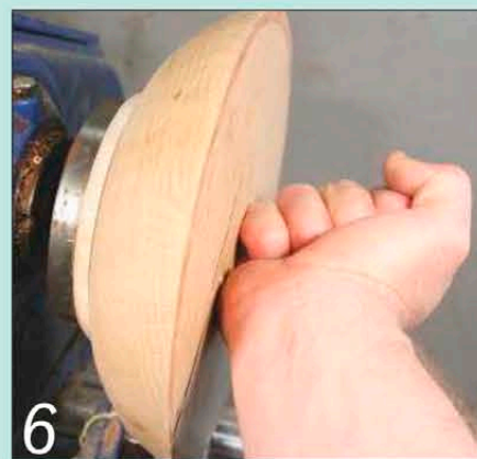
6 Mount the scoop onto the jam chuck by hammering it hard with your hand
