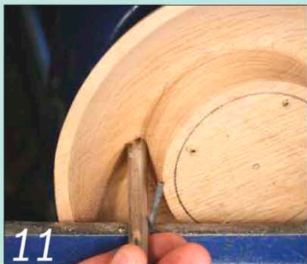
11 Take very fine cuts as you work, with just the point of the tool cutting into the tight angle
