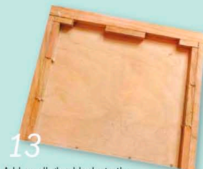
13 Add small glue blocks to the underside of each drawer for extra strength
