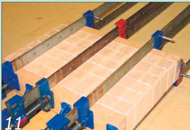
11 Assemble the six strips and the two sides as before and cramp them up
