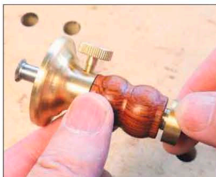
The fine-adjuster is a useful feature; a lock-screw on the collar would make it even more so
