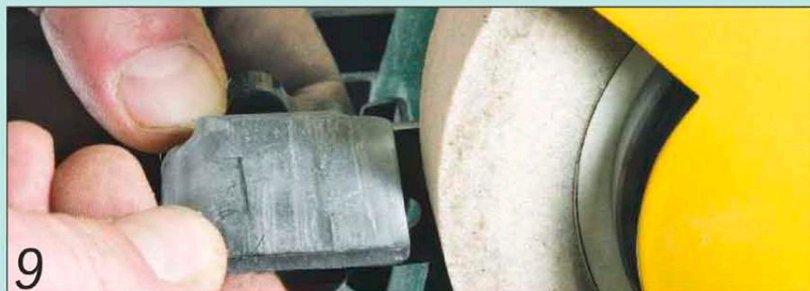
9 Adjust the tool rests and spark arresters after dressing is complete
