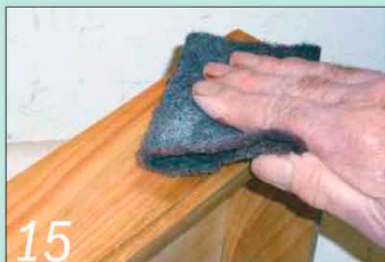
15 Apply three coats of your chosen finish, flattening down lightly between coats
