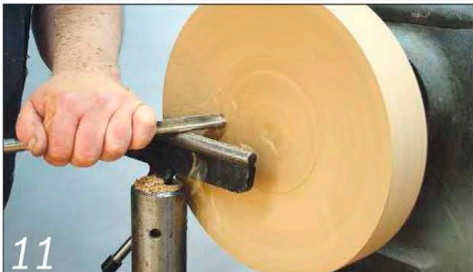
11 In faceplate turning the work is held at the headstock end of the lathe, and the toolrest is positioned across its face or edge
