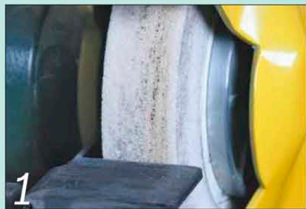
1 A worn and untreated grindstone will have a glazed and ridged surface
