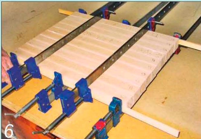
6 Add the two square outer strips and leave the assembly in the cramps
