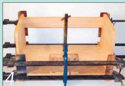
4 Assemble the other components, check that they're square and cramp them up
