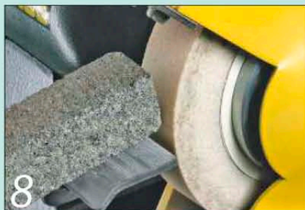
8 Lightly re-dress the surface with the devil stone for a smoother finish
