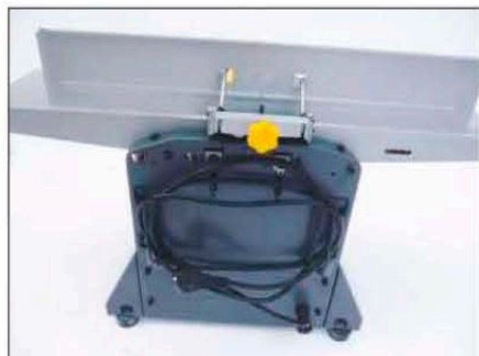
The fence can be tilted for bevel edging (see opposite) but cannot move laterally
