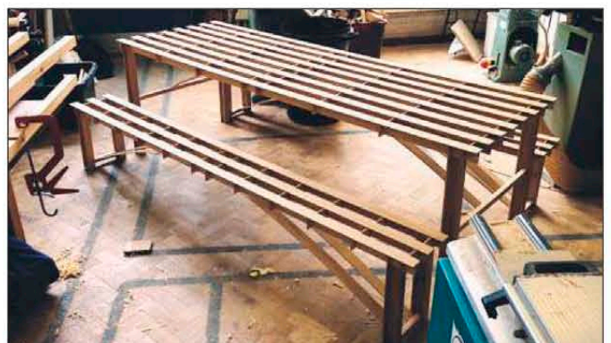
4 Will used the same structural techniques to create two matching benches. The braces make them amazingly rigid
