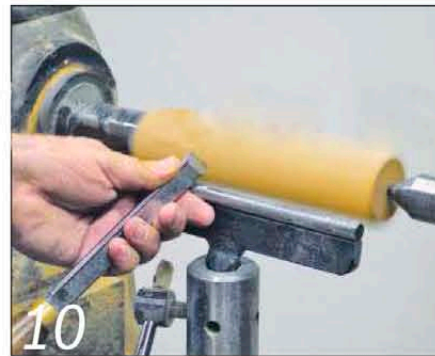
10 In spindle turning, the workpiece is held between centres in the headstock and tailstock, and is turned with the toolrest parallel to the work
