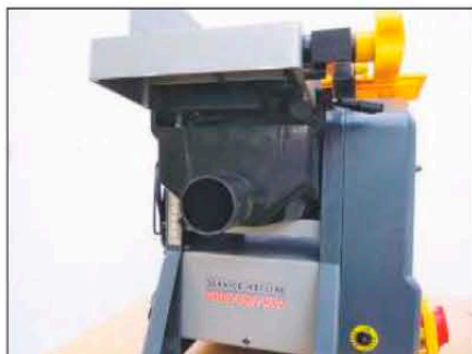
The thicknessing aperture holds the debris hood when surfacing
