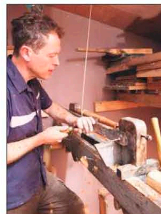
The legs and back spindles are turned on the pole lathe
