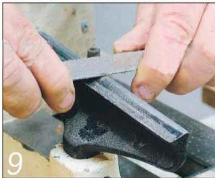
9 It's important to keep the toolrest smooth and free from rust so your turning tools can slide along it easily as you work
