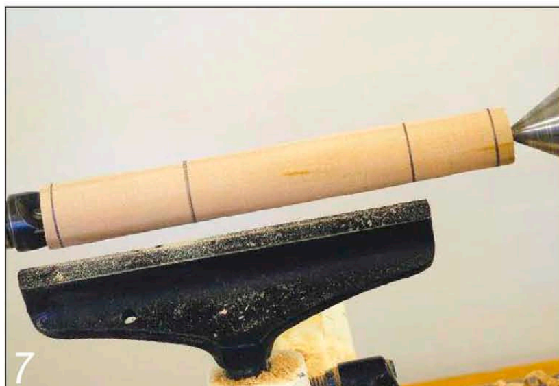
The tailstock houses a revolving centre (far right) which supports the free end of the workpiece and allows it to spin freely
