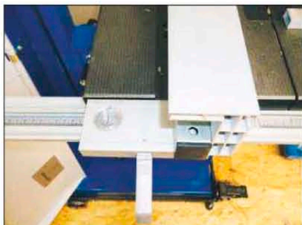
The rip fence anchors very firmly to the calibrated rail by means of a toggle lever
