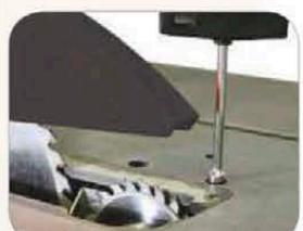
Optional pre-scoring unit with integral motor. Precisa 6.0 VR model only. Cannot be retro-fitted.
