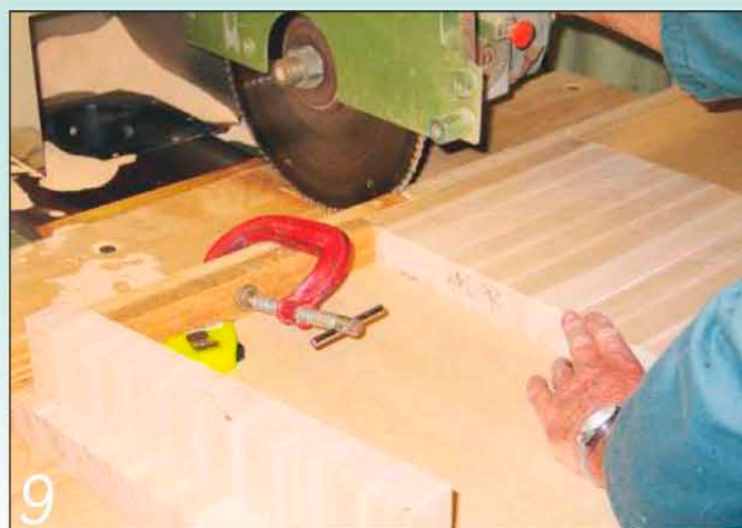
9 ...as you cut the six strips of glued blocks 75mm wide from the large blank
