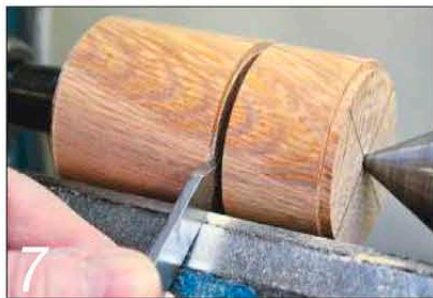
7 Part off the section for the lid, widening the cut to stop the tool binding
