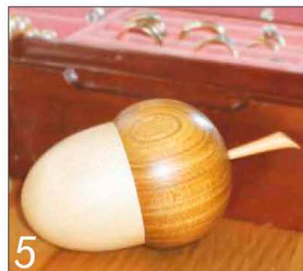
5 Using different timbers for the box and its lid makes life a lot easier
