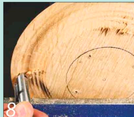
8 Form the underside of what will become the tip of the handle at the disc edge
