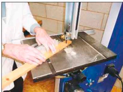
The cross-cut fence runs in grooves at either side of the blade
