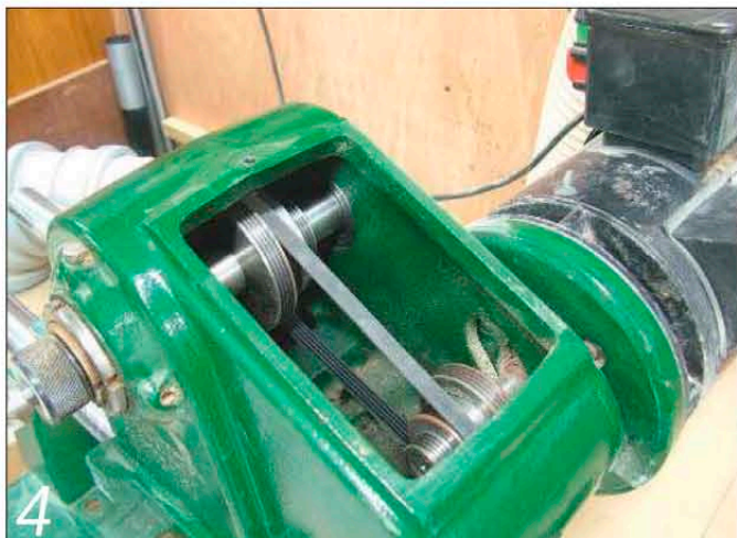
Two sets of pulleys connected by a ribbed drive belt transfer rotation from the motor's drive shaft to the lathe spindle
