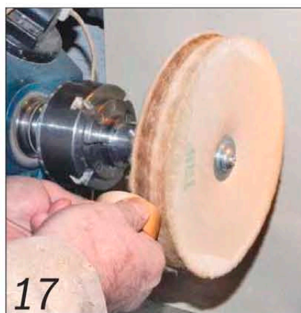
I prefer to polish boxes on a buffing wheel, and generally use the Beall system
