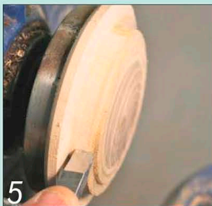
5 You now need to make a jam chuck to hold the scoop on the lathe in reverse
