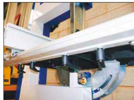
A series of levers hold the rail securely across the front of the table
