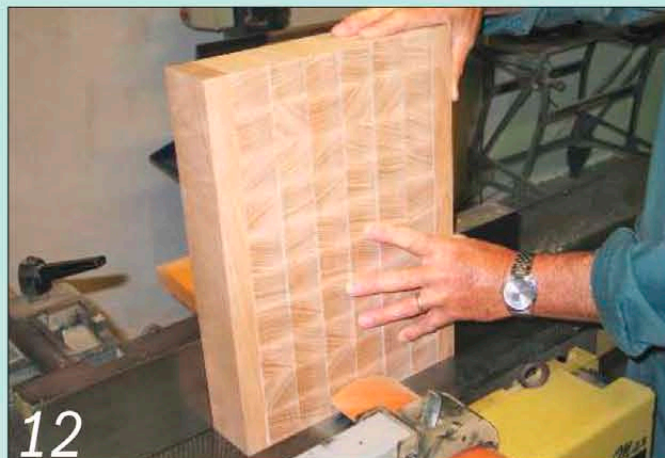
12 When the glue has dried, trim the ends down to size on the planer
