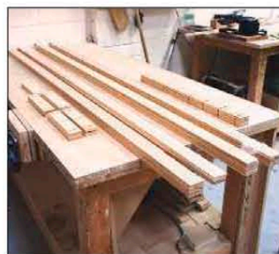
1 All the components were finished to size with a belt sanding machine to keep wastage to a minimum
