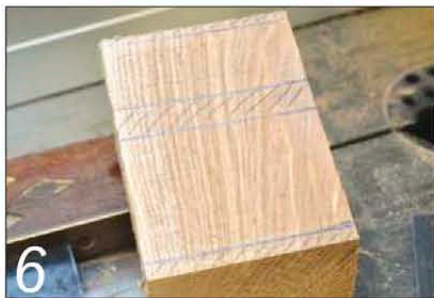
6 Prepare your blank by marking out the various areas that will be lost during the turning
