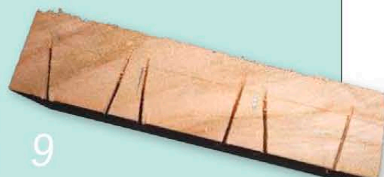
9 Use the dovetail saw to make the initial cuts at each pencil line
