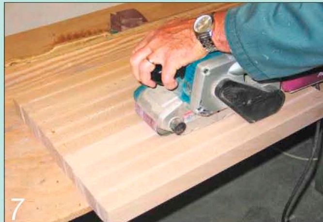
7 Sand the assembled panel to smooth it and remove any excess glue
