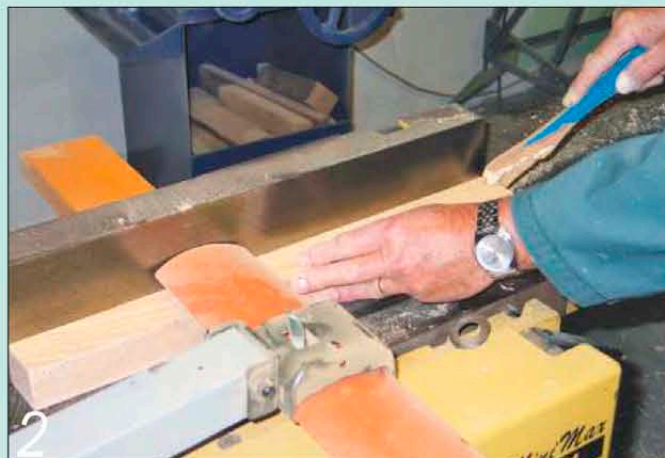
2 Plane the eight centre strips so they measure 42mm in one dimension
