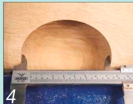
4 Record the diameter of the opening and check that the recess has parallel sides
