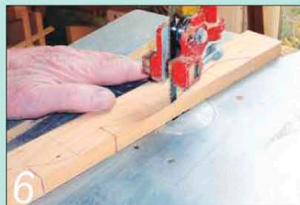
6 Mark the plinth shape with a template and cut it out on the bandsaw
