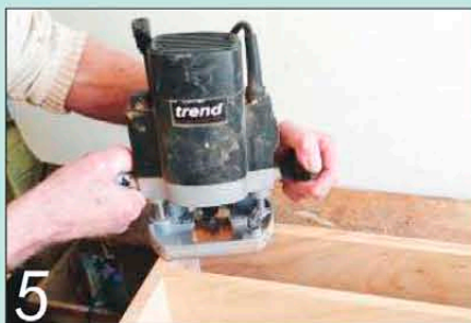
5 Rout the shallow rebate for the plywood back panel and square up the corners
