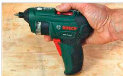
You simply slide the switch forward to load the selected bit in the holder
