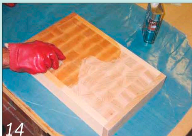
14 Sand off any excess glue and apply the finishing oil of your choice
