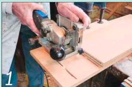
1 The main carcass components are all biscuit-jointed together
