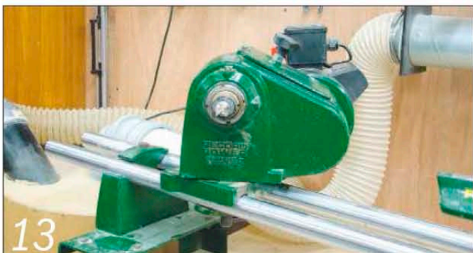
13 Many lathes have a headstock that can swivel on the bed bars, allowing large-diameter pieces to be turned without fouling them
