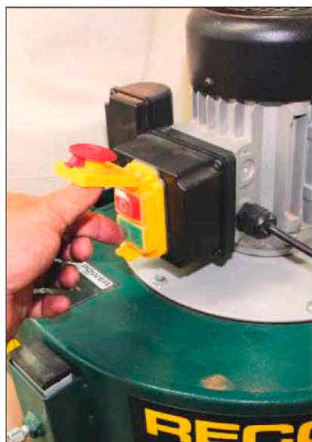
The NVR switch is fixed directly to the motor housing, which can be inverted for a fixed system
