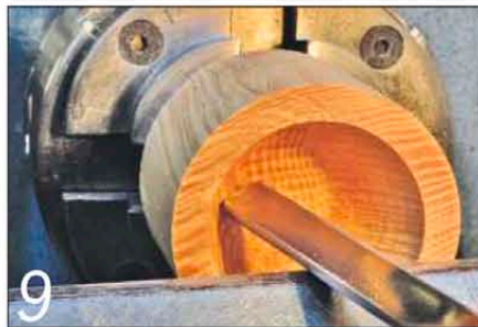
9 Cut from the bottom outwards with the gouge or a round-nosed scraper
