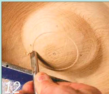
12 Complete the underside of the scoop by rounding off the bowl and sanding it smooth
