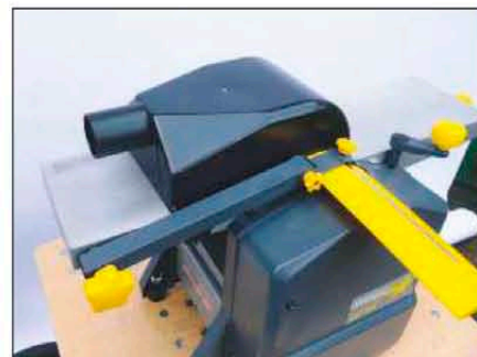
The fence must be removed to fit the hood in place for thicknessing
