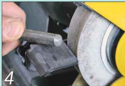
4 The diamond dresser has a tiny diamond set into the end of a metal rod
