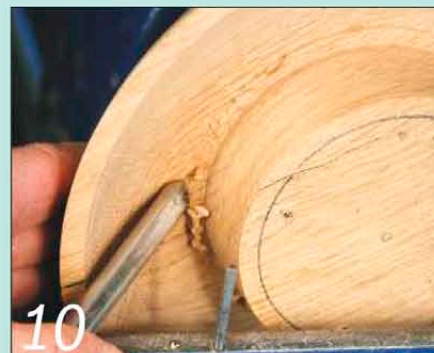
10 Switch to a spindle gouge to finish hollowing the angle where the handle meets the bowl
