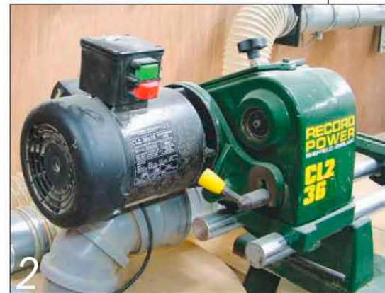
Most lathes have induction motors, with ratings ranging from around 250W for the smallest machines up to 750W on larger models
