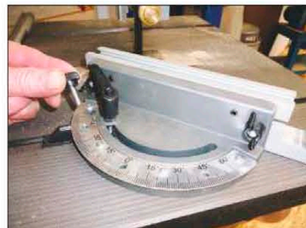
A loose pin locates the cross-cut fence positively at the 90° and 45° positions
