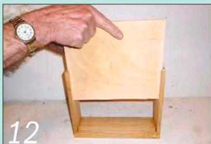
12 Slide the plywood drawer base into place and pin it to the drawer back
