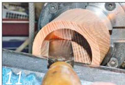
11 Its slightly angled blade is designed to cut the internal corner square
