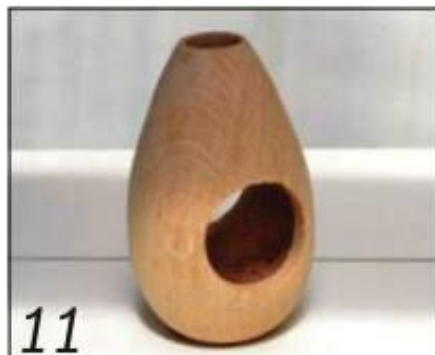
The presence of holes in the side of the work actually makes the hollowing easier
