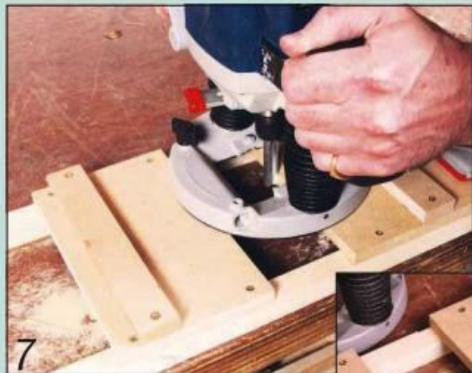
7 Place the router against the back guide bar and trim the front of the first mdf plate
