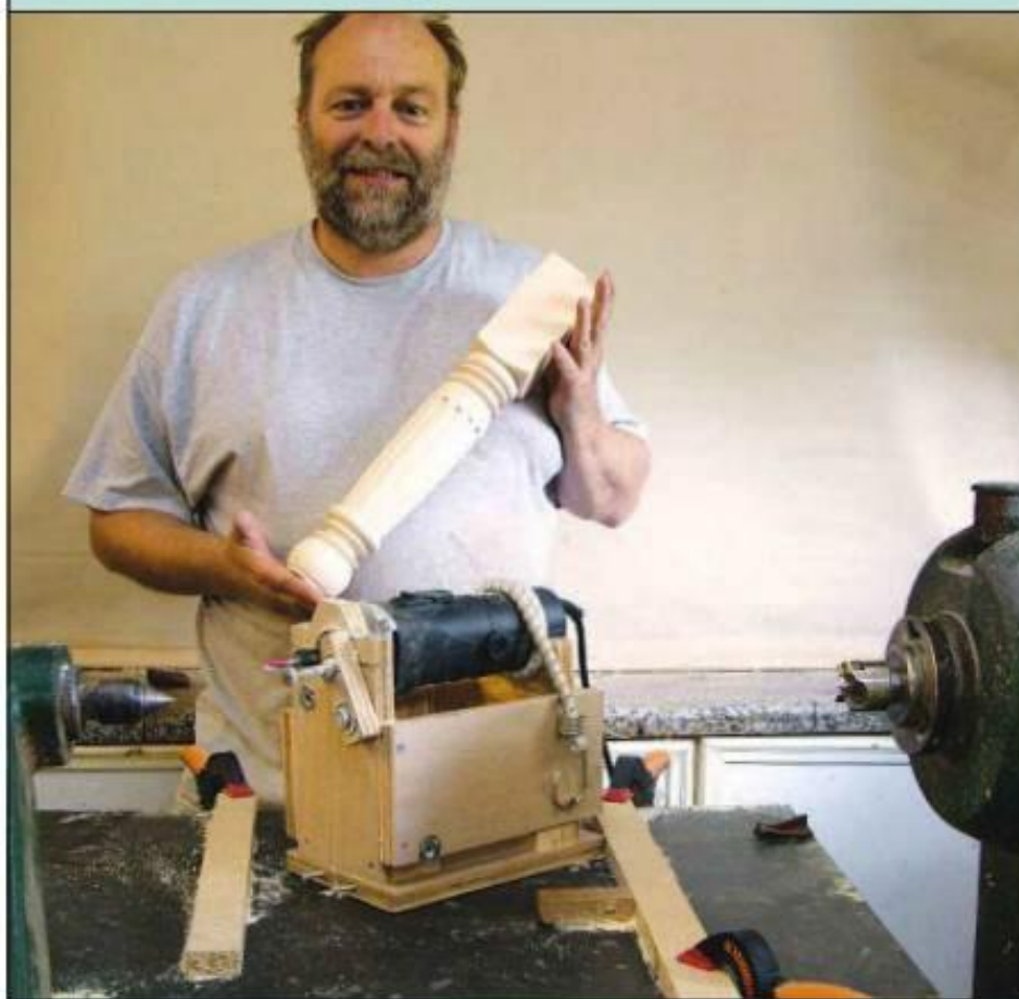
18 Cut the first flute, then move the indexing system on to cut the next. Repeat until they're all done...
