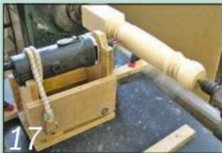
17 The battens cramped to the table limit the sideways travel of the jig
