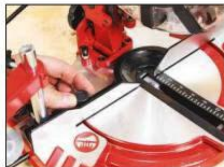
The table is locked in position with a small knob just behind the fence
