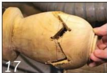
17 One solution is to make a zigzag cut round the piece with a jigsaw after doing some hollowing
