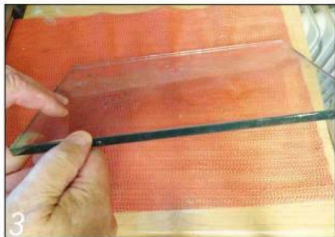
3 A sheet of 10mm thick float glass makes a good backing for the abrasive sheets, but handle it with care... and don't drop it!
