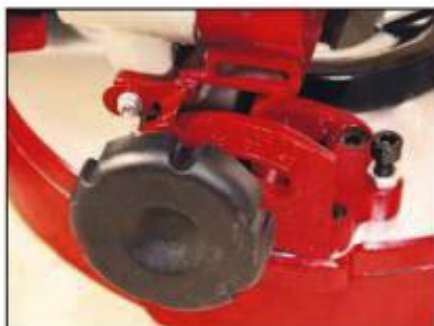
This is a single-bevel mitre saw, so the head tilts 45° to the left only
