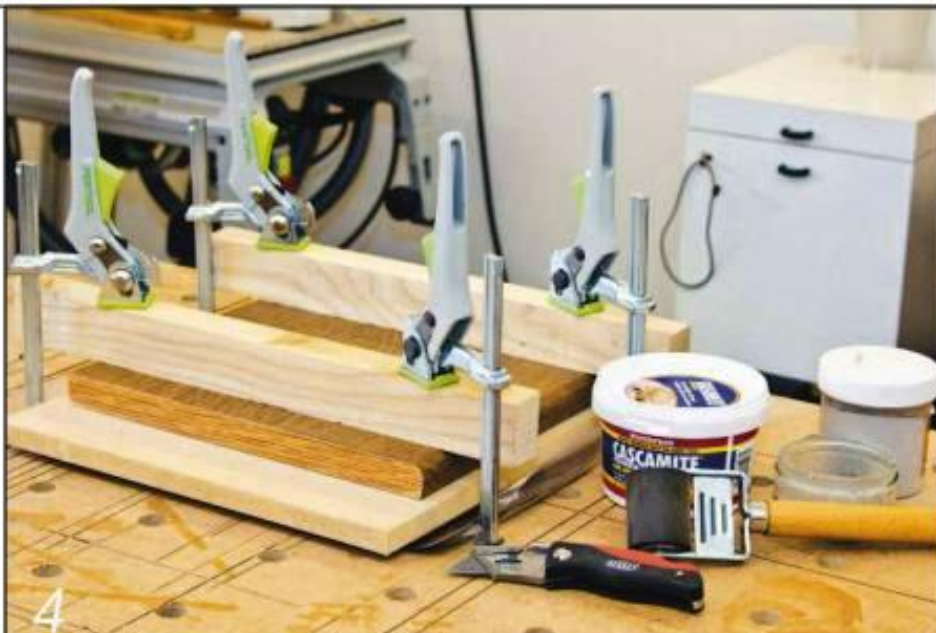
I used wooden cauls and lever cramps to glue the veneer to the mdf
