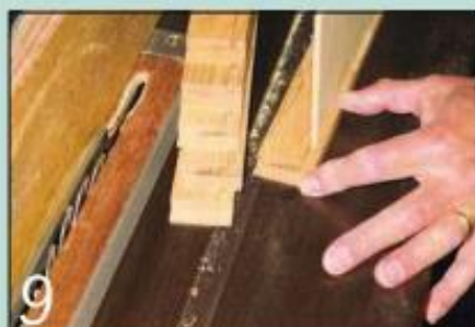
9 The drawer fronts and sides are grooved to accept the mdf base panels
