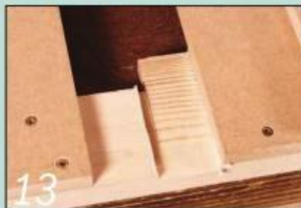
13 Here's one side of the tenon completed. Turn the work over and cut the other one
