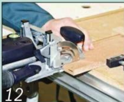
12 Set the jointer fence at 90° and cut the matching mortises in the shelf ends
