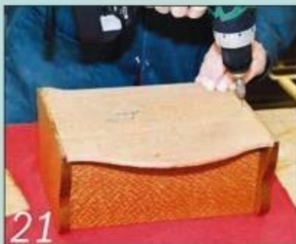
21 Glue and pin the back panels in place. Angled pilot holes help avoid splitting
