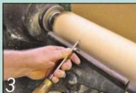
3 Use the long point of the skew chisel to start cutting the pommel, taking alternate V cuts
