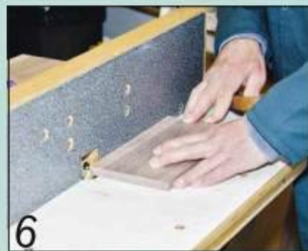
The router table made light work of ogee-moulding the shelf edges
