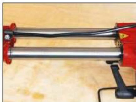
The saw head is supported on a sturdy pair of round hardened steel bars
