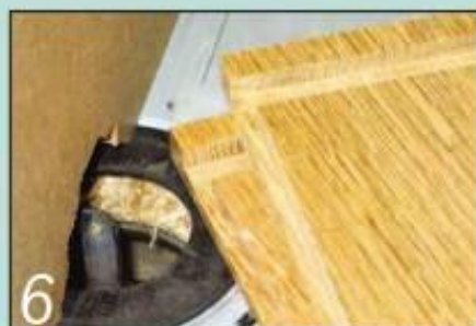
6 Use a straight cutter in the router table to form a rebate for the back panel
