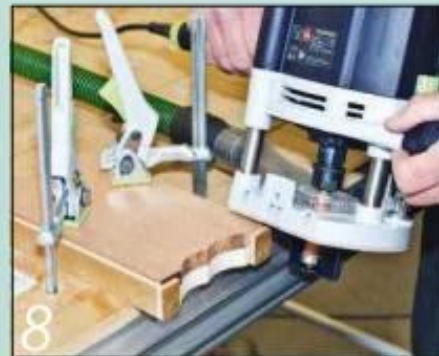
The template in the jig guides the router when finishing off the curves
