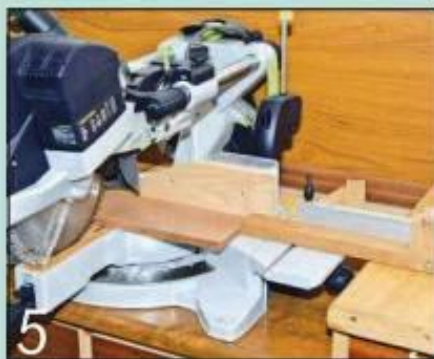
A home-made length stop on my mitre saw makes a series of repeat cuts easy
