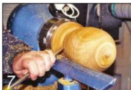
Shape the outside of the form first to act as a guide for hollowing the inside
