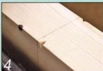
4 This is what you should see after the first two V cuts are completed
