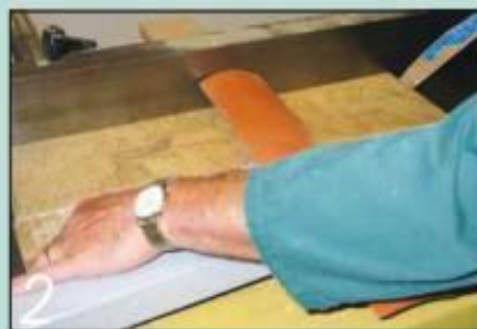
2 Leave the cramped boards to set overnight, then surface-plane each one to its finished size
