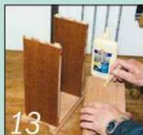
13 Use a lollipop stick to spread adhesive into those narrow 4mm mortises
