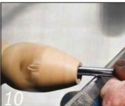
With the lathe running, you can now view the progress of the tool through the side window
