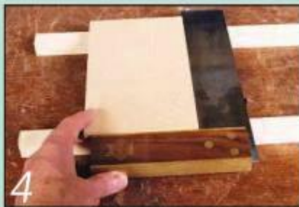
4 Position the first mdf plate and check that it's perfectly square to the rails
