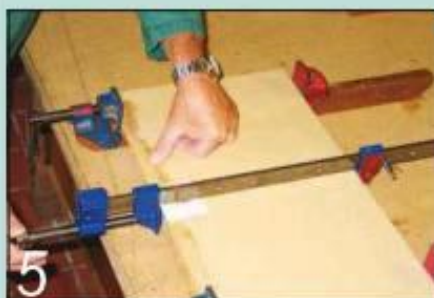
5 A piece of mdf with a solid wood edge strip glued on forms each drawer divider
