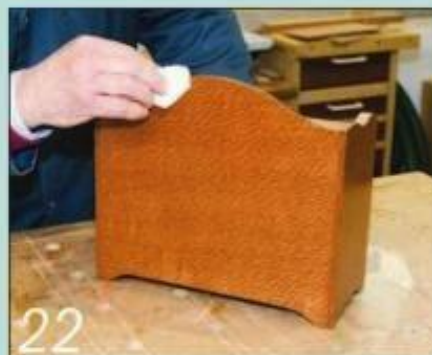
22 Round over the edges of the top panels slightly and apply oil with a soft lint-free cloth
