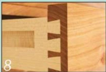
8 The storage drawer has an elm front dovetailed to sycamore sides
