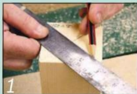
1 Mark the centre of each end of the blank accurately and pop-mark it
