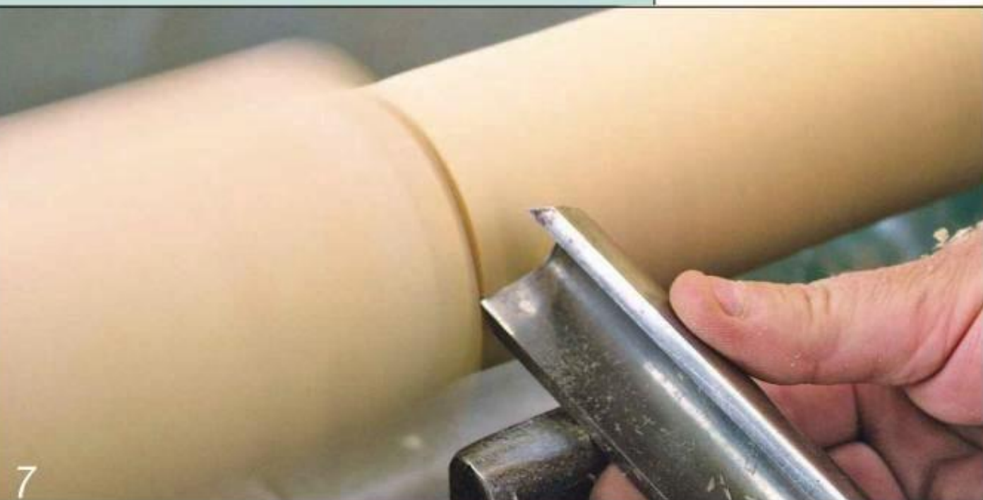
7 Use the roughing gouge on its side as shown here, to avoid making contact with the square section
