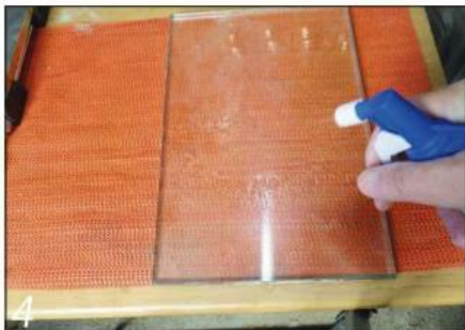
4 A film of water applied to the glass using a plant sprayer will hold the paper still and also provide lubricant
