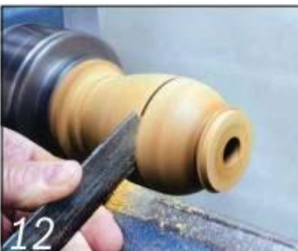
If you fancy cheating, you can use a narrow parting tool to cut the piece in two
