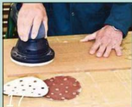
17 I planed and sanded the back for the lacewood bookcase to a thickness of 8mm
