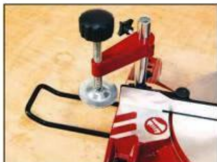
The solid material clamp is fully adjustable and very easy to position as required
