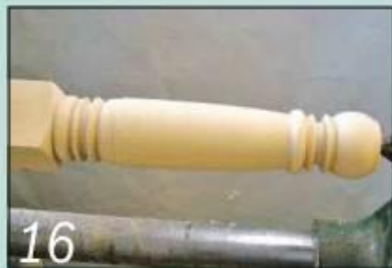
16 The turned leg should now look like this, ready for fluting to start
