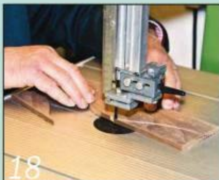
18 Mark the curves along the top of the back panels and cut them on the bandsaw
