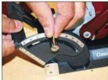
The tilting shoe is indexed to control the depth of the slot. The single locking lever holds the shoe in place.
