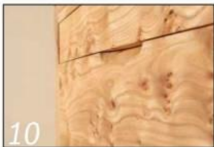
10 The groove under the drawer's front edge is accessed via this D-shaped cut-out
