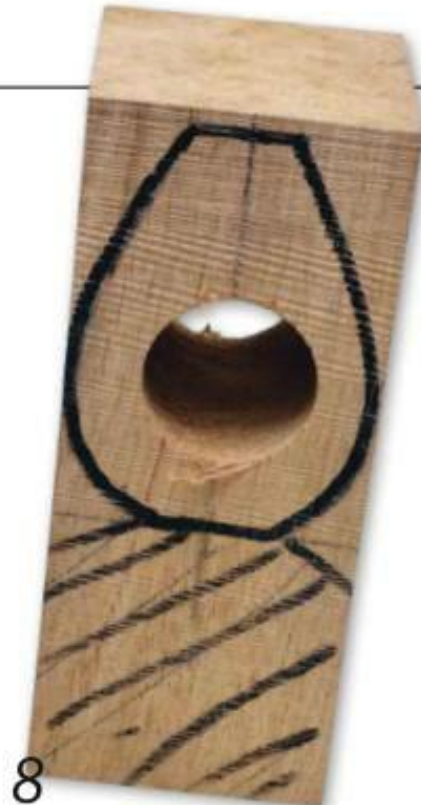
Make the interior visible for practice purposes by drilling a large hole through the blank
