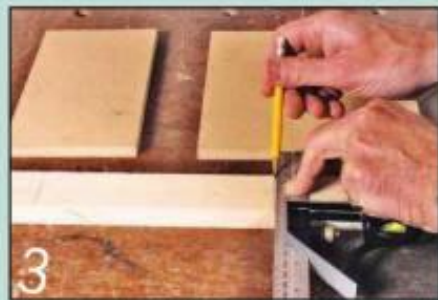
3 Place the rails together and use a square to mark the mdf plate positions on them
