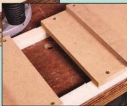
8 Let the cutter bite into the side rails to form an alignment mark for the tenon shoulders
