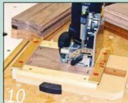
Align the jointer's centre mark with each line in turn and cut the mortises
