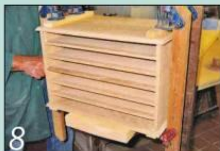
8 Fit the drawer dividers, add the top and bottom and cramp everything up square
