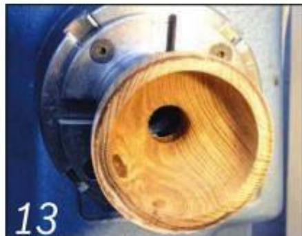
13 It's then a simple matter to hollow the two halves with a bowl gouge...
