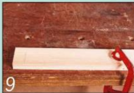
9 Mark the position of the tenon shoulder on the workpiece and clamp it to the bench
