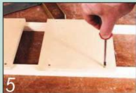
5 Cramp the plates in position, drill clearance holes and screw them to the rails
