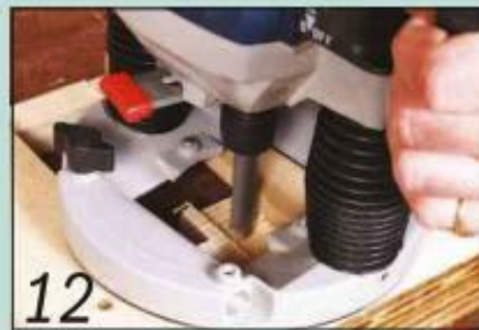
12 Set the cutter depth to match the required tenon shoulder depth and make the first cut
