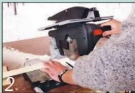
2 Switch to the cross-cut saw to trim off two pieces, each about 600mm long
