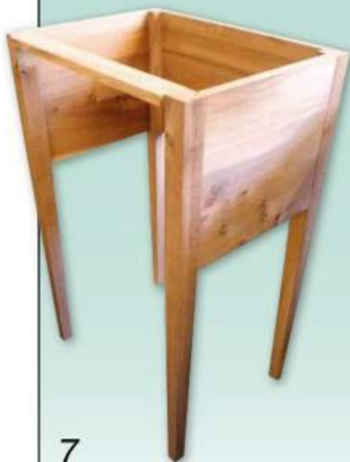
7 Three tenoned-in panels and a dovetailed front rail form the lower cabinet
