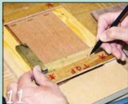
11 Transfer the lines on the jig to a try square blade for marking the shelves
