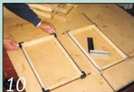
10 I used a couple of frame cramp sets to hold the drawer boxes together
