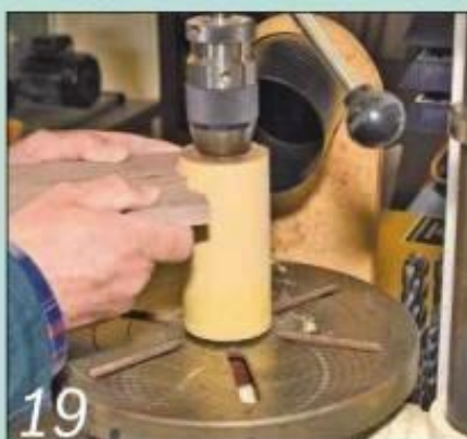
19 Smooth the sawn curves down to the pencil lines using a drum sander
