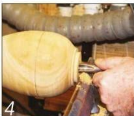
A bowl gouge can be a surprisingly effective hollowing tool. Note the position of the flute
