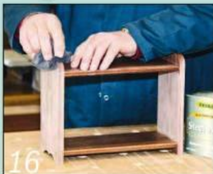
16 Sand the bookcase sides and apply a coat of oil. Keep clear of the rebates
