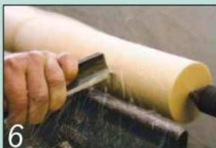
6 Rough down the rest of the blank with a spindle roughing gouge
