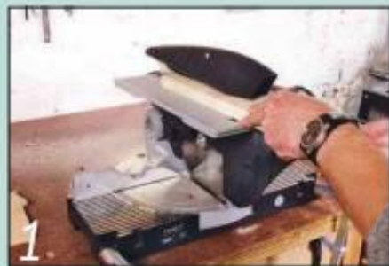
1 Start work by cutting some 20mm square softwood stock on your table saw
