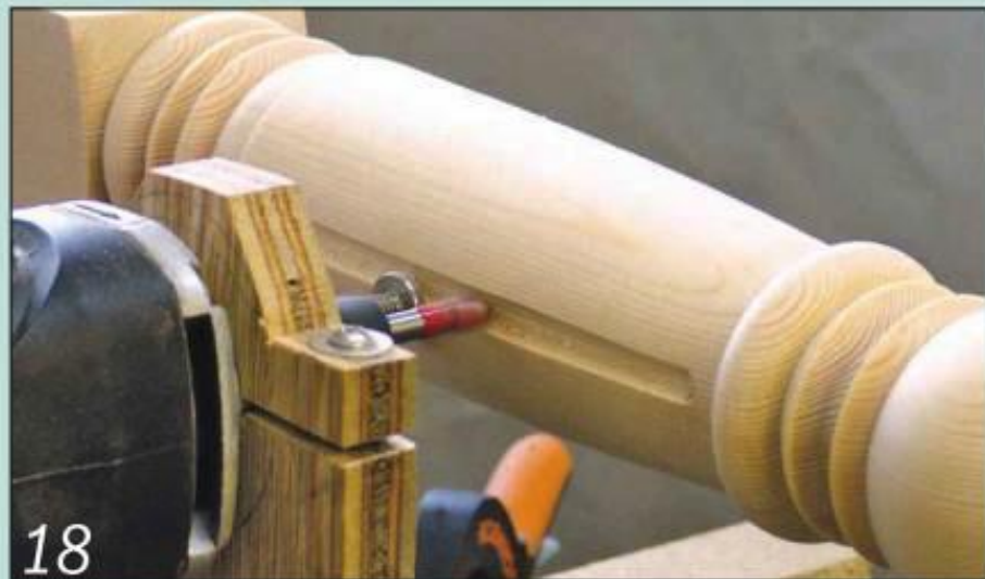
18 Cut the first flute, then move the indexing system on to cut the next. Repeat until they're all done...
