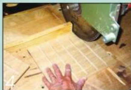
4 Cut the five housings in the side pieces with a crosscut saw (or a router if you prefer)
