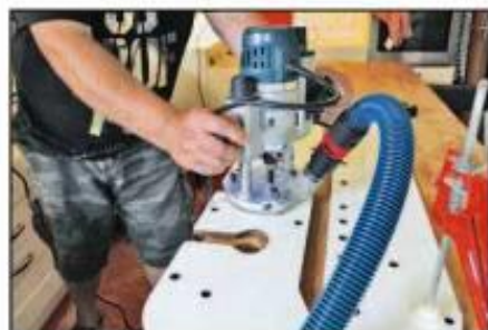
Use the index pins again to position the jig for routing out the connector bolt holes
