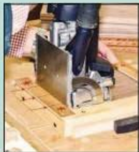
3 The second jig (shown in fig 2) was designed to help position the dominos accurately
