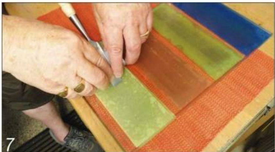
7 3M self-adhesive abrasive film is my choice: a few quick strokes and the chisel's keen to go again
