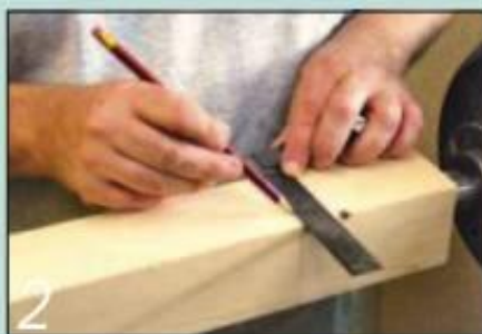
2 Square a line all round, 125mm from one end, to define the pommel
