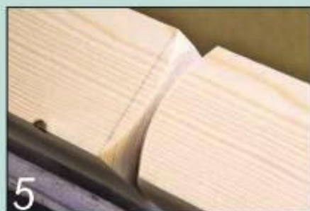
5 Deepen the two cuts and work one side back towards your pencil line
