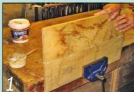
1 Rub the glue into the joint of each main carcass board to create a good bond
