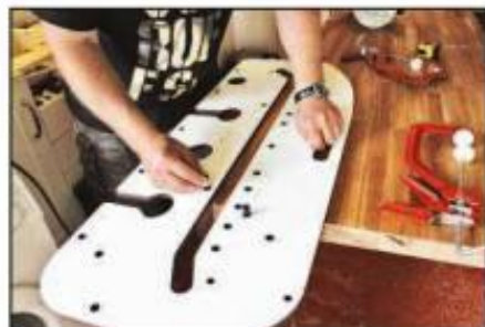
Insert the index pins to suit the cut you're making; then clamp the jig to the worktop
