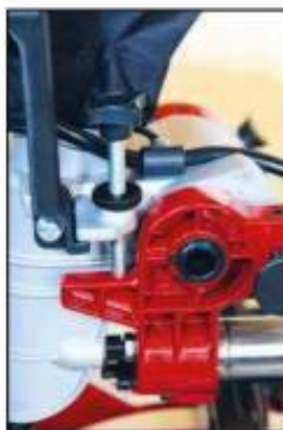
The depth-of-cut adjuster allows partial cutting of housings or tenons
