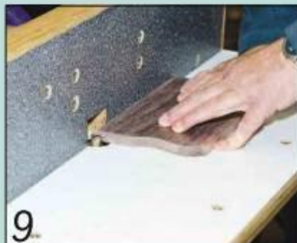
Go back to the router table to cut rebates in the edges of the bookcase sides
