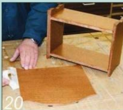
20 Sand the back panels and apply a first coat of oil. Protect the rebates with masking tape
