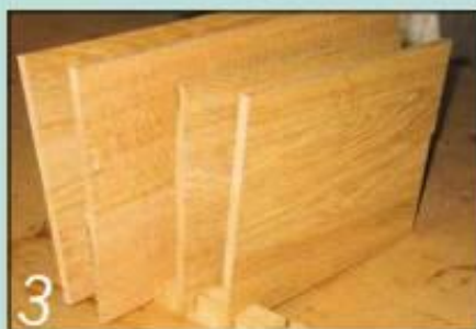
3 Stack the thin boards on edge to stop them picking up moisture and warping
