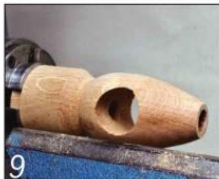
Then shape the exterior of the blank and drill a hole into it so you can start the hollowing
