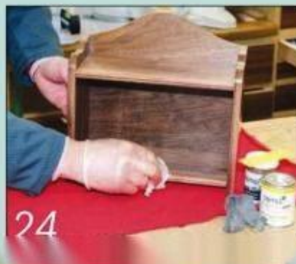
22 Round over the edges of the top panels slightly and apply oil with a soft lint-free cloth
