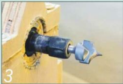
3 Secure the router in its cradle and fit your choice of beading bit
