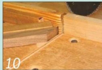
Make sure that the sloping cuts on the four legs are all at the same angle
