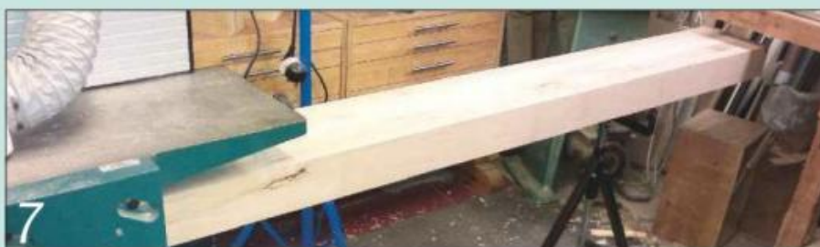
7 Plane each completed top section smooth and then thickness it down to 93mm
