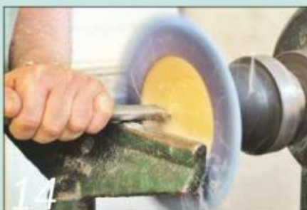
Remount the chuck on the lathe and hollow out the inside with a bowl gouge
