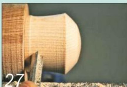
27 Finish shaping it with a small bowl gouge, then sand and finish it as before
