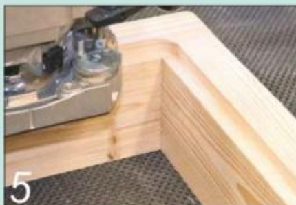
5 Cut a rebate in the internal top edge of the frame to take the base panel
