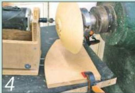
4 Cramp a template to the table for the screws in the jig to follow....
