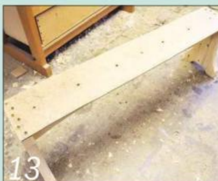
13 I pinned some hardboard to the top of the leg assembly to form a template for the dowels
