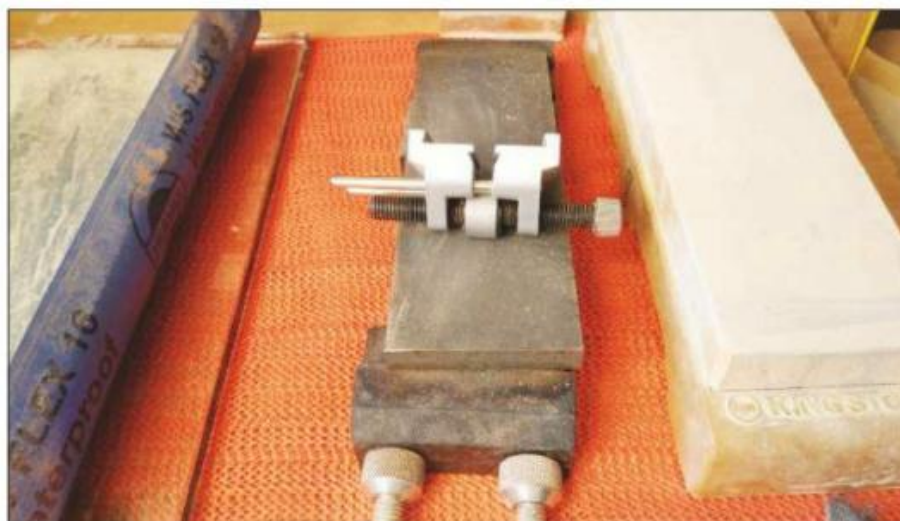
The narrow roller allows me to tweak the angle if I wish, and is great for radiused plane irons
