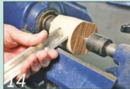
Mount the shorter block between centres and turn it down to a cylinder
