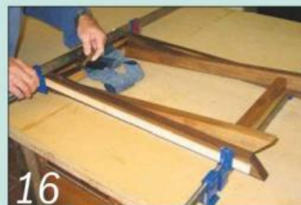
Check that the outer frame is square as you fit the cramps round it
