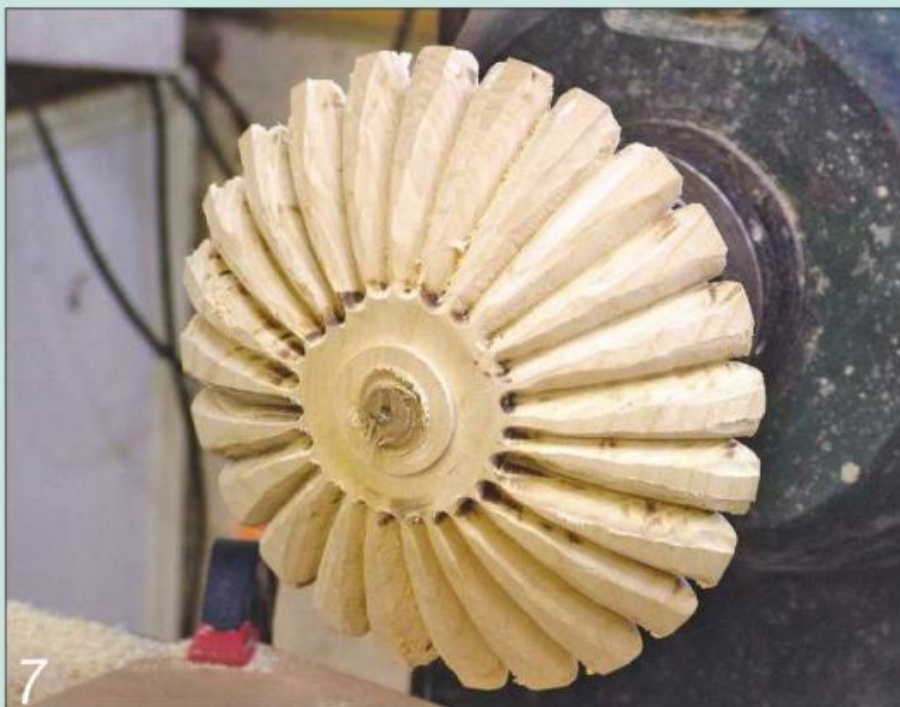
7 This is how the bowl looks after the first pass with the router over all 24 beads
