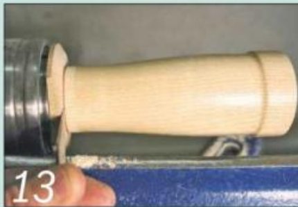
Sand and polish the body, then part it off with an extra-thin parting tool
