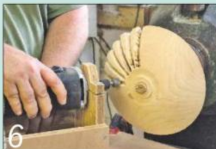
6 Rout the beads in stages, cutting a little deeper with each pass
