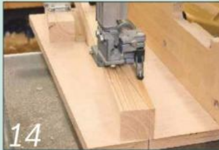
14 Cut 7° chamfers on the A-frame uprights using a simple bandsaw jig
