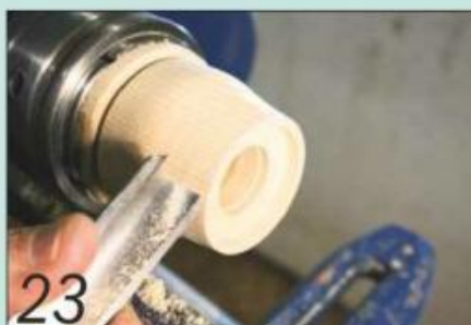
23 Form the approximate shape of the top in situ using a roughing gouge
