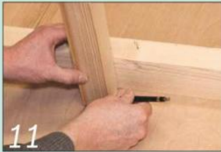
11 Mark the positions of the A-frames on the underside of the base panel
