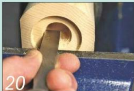
20 Cut the recess to take the head mechanism using a square scraper
