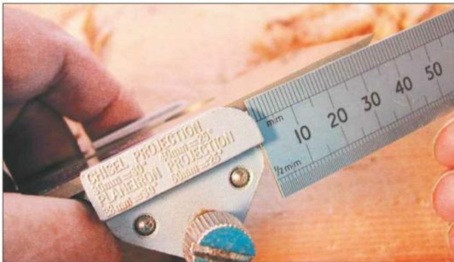
A honing guide ensures a constant bevel; just set the required blade projection with a rule
