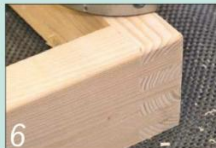
6 Round over all the external edges of the frame with a 6mm radius bit
