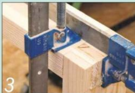
3 Glue and cramp the frame rails together and check that they're square
