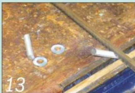
Use a hacksaw to cut the two pivots from 10mm diameter steel rod
