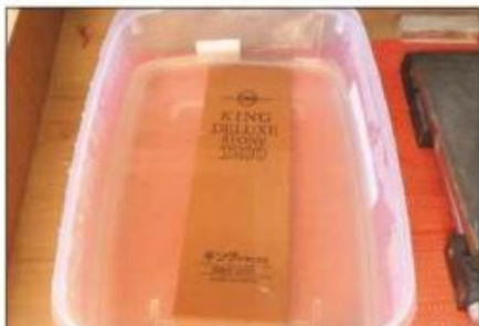
Water stones need to be stored immersed in water. Don't let them freeze in winter
