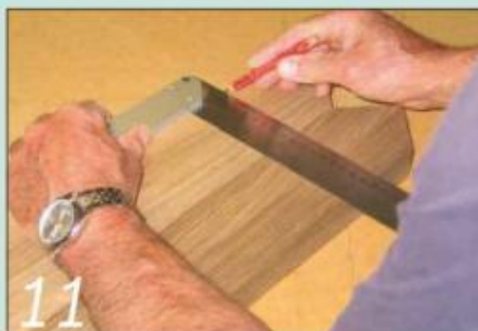
Mark out the mortise positions on all four legs at once for accuracy
