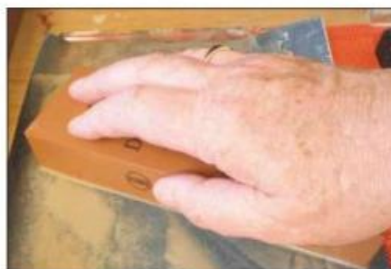
...but the way they shed surface grit during the sharpening process means that they need frequent flattening to stay in shape
