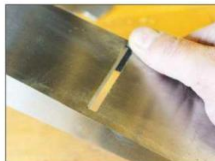
You can open up the mouth to a massive 9mm wide for taking heavy cuts
