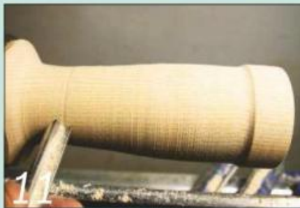
Complete the outer shape using a gouge. Aim for a simple, smooth profile
