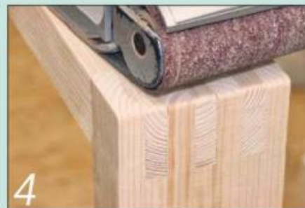
4 Chisel off any glue squeeze-out and plane or sand the joints smooth
