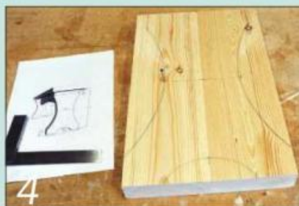
4 After marking out the leg shapes, I flexed a steel straightedge round a nail to create the curves
