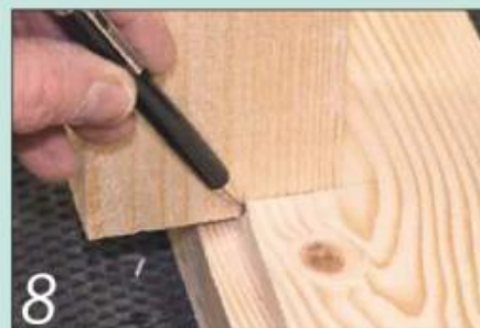
8 Hold the rails in their housings so you can mark the shoulder lines accurately
