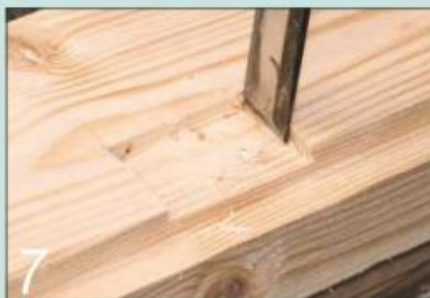
7 Mark and cut the shallow housings for the intermediate rails in the base frame
