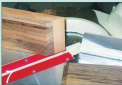
Mitre the four tray sides to length, using a mitre saw if you have one
