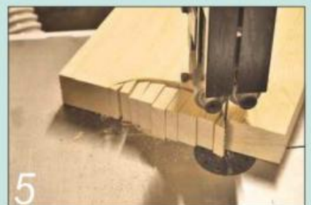
5 When cutting a tight curve on the bandsaw, these parallel cuts allow the waste to drop away
