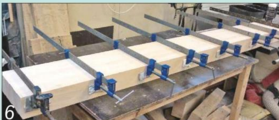
6 Each section of the bench top is made up of laminated and biscuit-jointed strips
