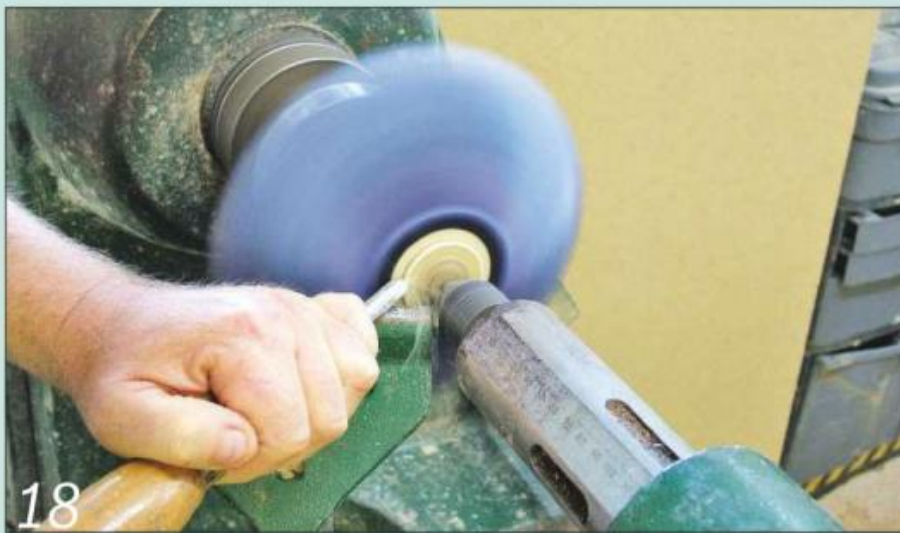
18 Turn away the chucking spigot and sand the bowl base smooth
