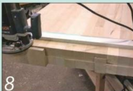
8 The easiest way to trim the top sections to length is with a router and a guide fence
