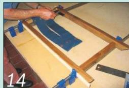
Assemble the inner frame first, after looping the straps over the top rail
