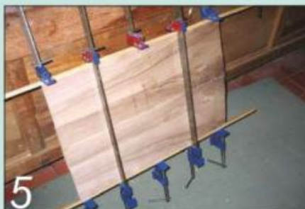
5 Cramp the panel between protective battens and put it aside to dry
