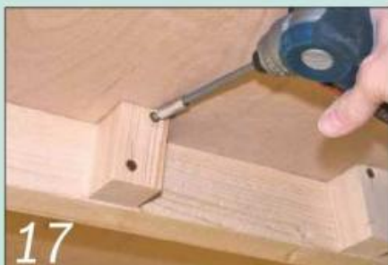
17 Use two screws to secure each A-frame leg to the base frame rails
