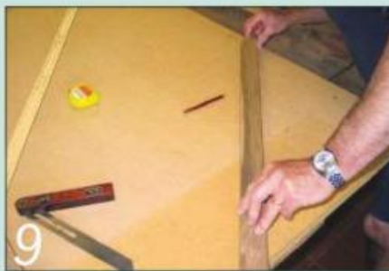
A full-size drawing – a rod – is the best way to mark out the dimensions and angles
