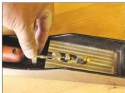
The Norris-style lateral adjustment lever is excellently engineered
