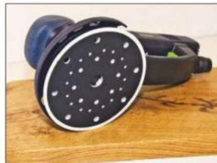
The sanding pad features the Multi-Jetstream pattern of dust collection holes
