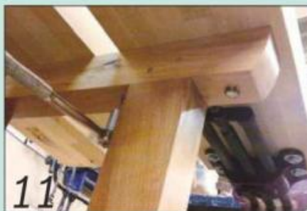
11 Attach the tops using coach screws driven up into them through the trestle top rails
