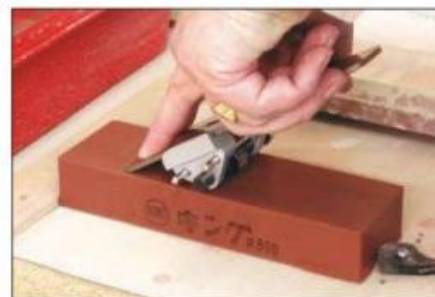
Japanese water stones retain their cutting ability well thanks to their construction...
