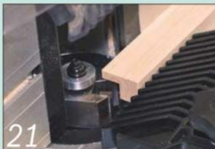
21 Cut a 12mm deep rebate in each length of side trim on the table router
