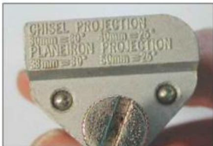
This guide from Axminster has the most-used blade projections marked on the side
