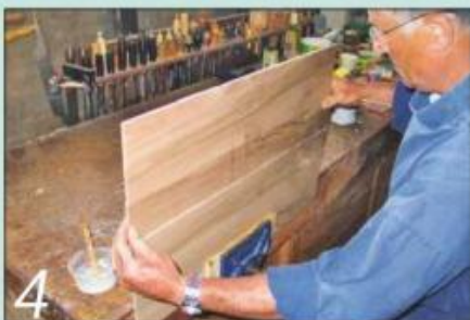
4 Repeat the process to join the second pair of boards to the first pair
