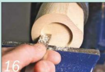
Use a scraper to cut the shallow recess that will fit over the mill's body
