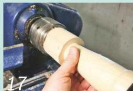
Offer up the mill body to check that it will revolve smoothly inside the recess
