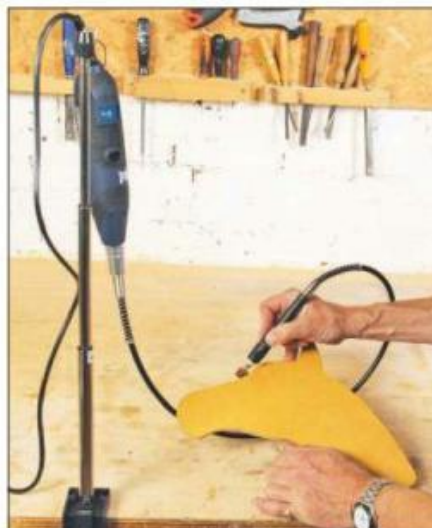
The bench stand and flexible shaft are ideal for doing detailed work
