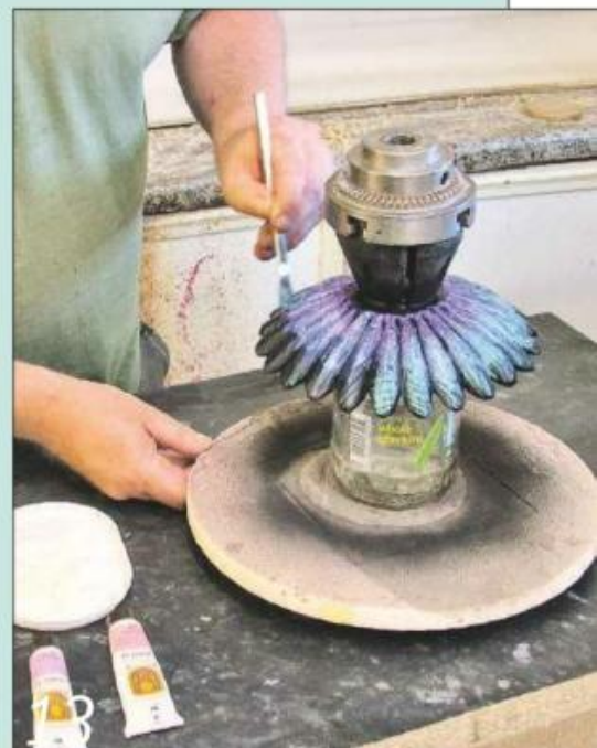
Remove the chuck, put it on a turntable and start to stipple on the paint
