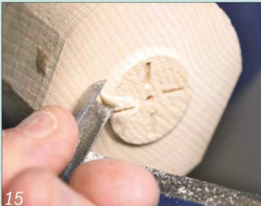
Reverse it in a compression chuck and slice the end flat with a small gouge
