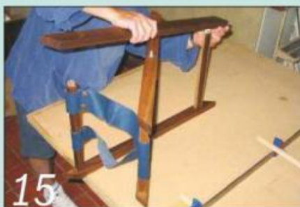
Fit the outer frame components round the inner frame one by one
