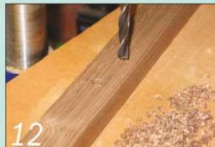
Bore a stopped hole for the pivot in each of the meeting leg faces
