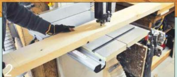
2 I marked the rail's curve with a long straightedge and cut it on the bandsaw
