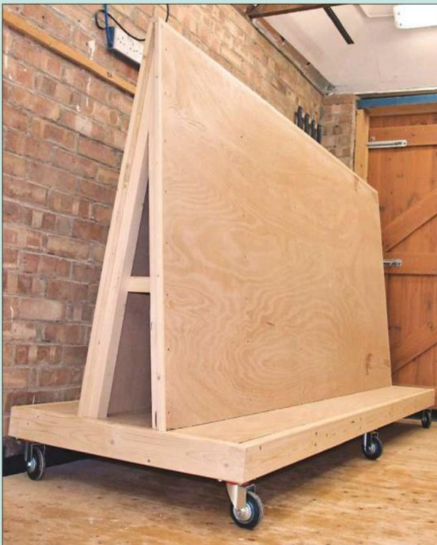
23 Add a softwood trim to protect the top edges of the two sloping panels
