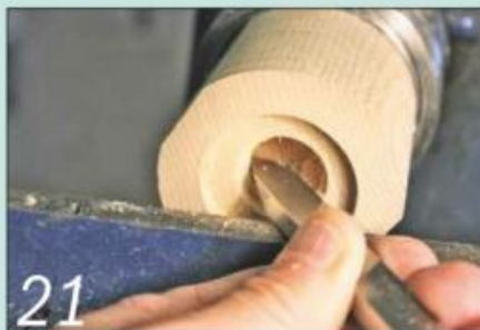
21 Form a sloping under-cut to accept the head mechanism's fixing lugs
