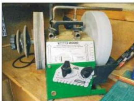
I use my Tormek wet grinder for general grinding, and the leather wheel for stropping carving tools. I still hone chisels and planes by hand
