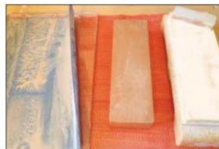
I use a 1200-grit water stone for honing and an 8000-grit one for polishing, plus wet-and-dry paper on float glass to flatten them
