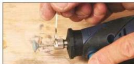
A small spanner is supplied for use when changing collets or bits
