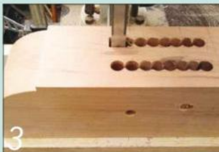
3 Cut the top rails and shoes to shape and drill out most of the mortise waste
