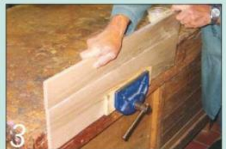
3 Glue and rub-joint the first two pieces of the tray's base panel together
