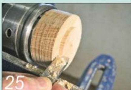
25 To finish the top, form a small jam chuck for it on a piece of waste wood
