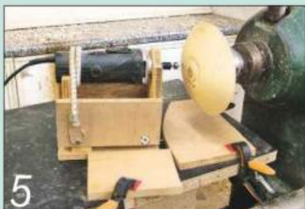
5 ...and add an offcut to act as a stop block that will limit the jig's travel
