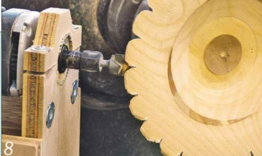
Align the routed bead with the cutter and tighten up the chuck
