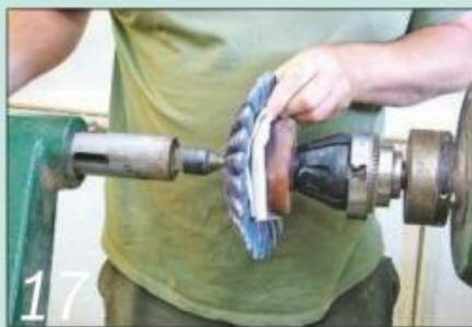
17 Reverse-chuck the bowl onto a wooden dolly lined with a pad of kitchen paper
