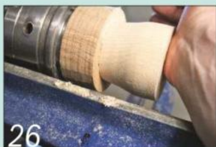
26 Push the top firmly onto the jam chuck and check that it fits securely
