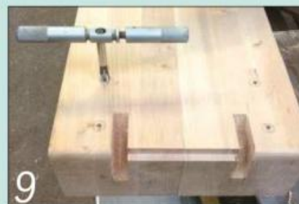
9 I prefer to use engineer's bolts rather than coach screws to attach my vice bodies
