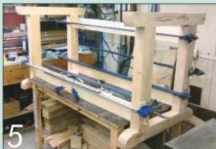
5 Cut the three stretcher rails to length and assemble the complete underframe
