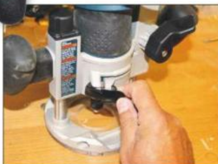
Lock the base to the motor housing with this easy-to-operate toggle
