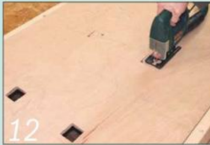
12 Unscrew the base panel and cut out the marked holes using a jigsaw
