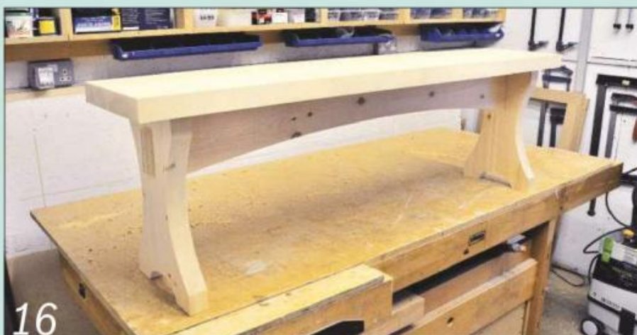
16 Brush more glue onto all the dowels and fit the top to the leg assembly
