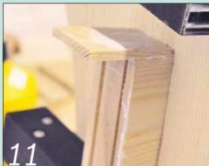
11 After assembling the joint I drove a softwood wedge into the gap at the top to lock it
