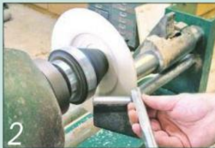
2 It's easier to rout the piece if you shape or flatten the rim at this stage
