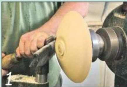
1 After rough-turning the blank, shape the back using a bowl gouge
