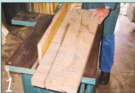
1 Cut out all the defects; the saw guard has been removed here for photographic clarity
