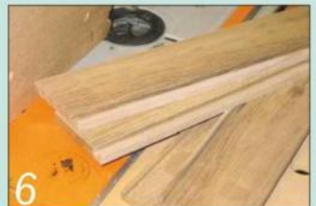
6 Cut the grooves in the tray sides for the base panel on the router table
