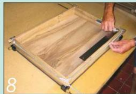
Assemble the sides round the base panel and check that it's square
