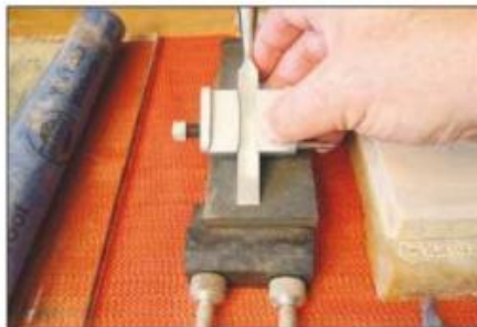
Gripping the tool by the edges keeps the blade square to the stone surface during honing
