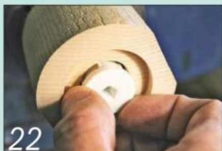
22 Push the mechanism up into the top of the mill until it clicks in place
