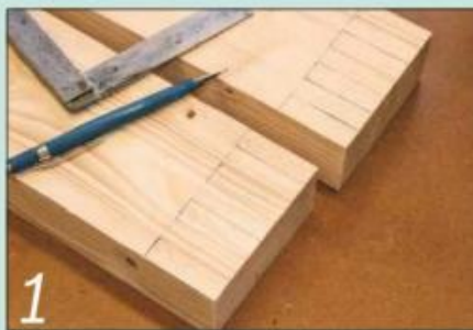
1 Mark all the 14mm wide finger joint positions on the base frame rails
