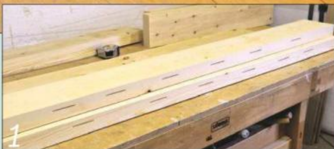
1 I added some size 20 biscuits before joining the halves of the legs and top
