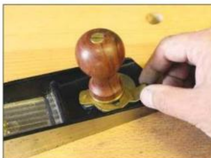
The mouth adjuster looks a little crude, although it works flawlessly
