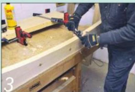
3 The bandsaw blade left a poor finish, which I cleaned up with a sharp spokeshave
