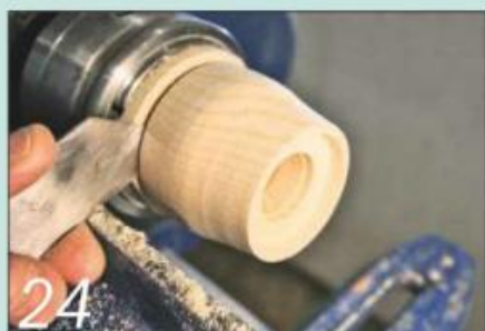
24 When you're happy with its proportions, sever it with your thin parting tool
