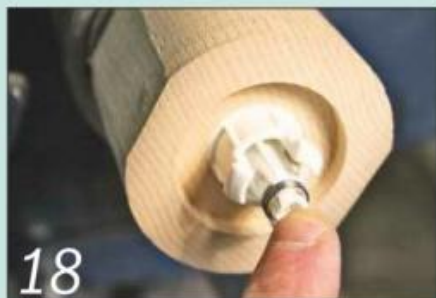
18 Cut a recess for the mechanism's flange in the underside of the head
