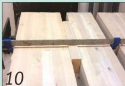
10 Fit spacers between the top sections as you attach them to the underframe
