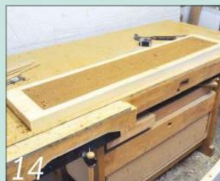
14 I then used it upside down to drill the corresponding holes in the underside of the top
