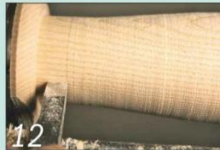
Form a parallel-sided section at the top on which the head will rotate
