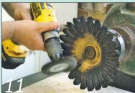
Remove the carbon deposits from the petals with a rotary nylon abrasive brush
