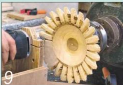
Rout the rim of the bowl in the same manner, moving the index on one space at a time
