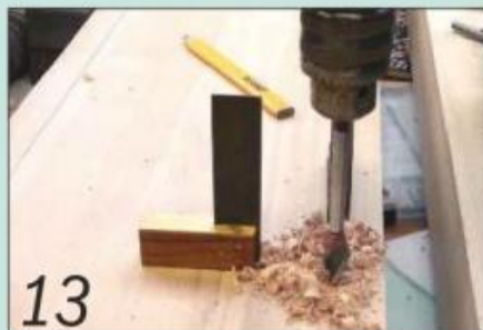
13 Mark lines along the bench top and drill dog holes along them at regular intervals
