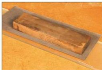
Oilstones are simple, cheap and effective, and can produce reasonable sharpening results
