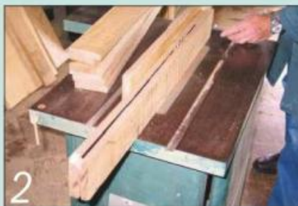
2 Deep-saw the stock to thickness; the wedge in the foreground stops the blade from jamming
