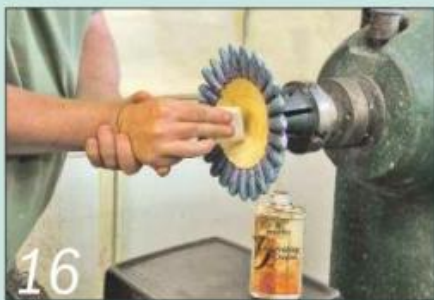
16 Allow the lacquer to dry and then buff it up with burnishing cream
