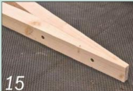
15 Join each pair of chamfered faces together with four screws – two from each side
