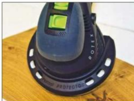
The circular black edge protector allows sanding right up to vertical surfaces
