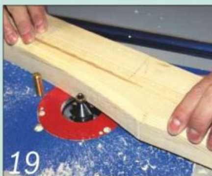
Add chamfers to the curves using a lead-in pin on the router table, or a hand-held router
