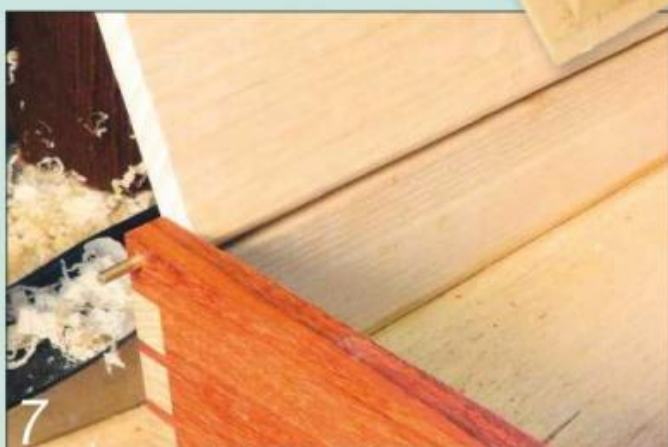
7 Use temporary over-long brass rods to hold the lid while you test its fit
