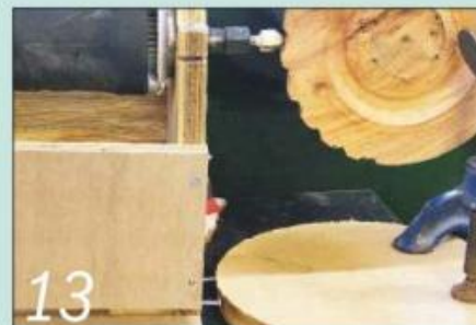
Cramp a template to the baseplate and run the two screw heads against it
