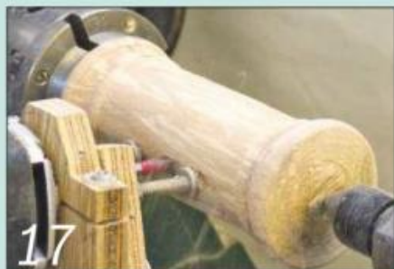
17 The completed cradle runs along the centre of the workpiece...
