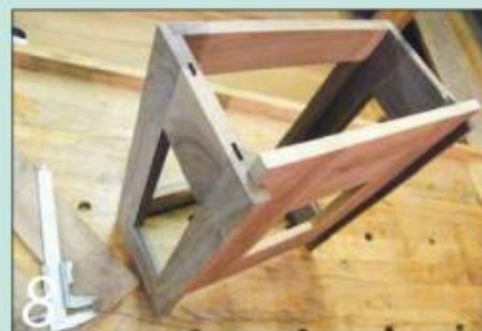
8 The dial mask slides into grooves cut in the inner face of the side frames
