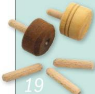
19 Fix the blank to the chuck with hot-melt glue and turn it to shape
