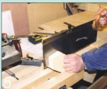
5 I cut all the tenon cheeks by hand with my big Pax rip-filed tenon saw
