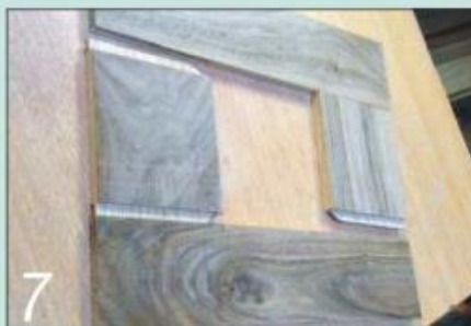
7 Assemble the veneered dial mask using shallow tongue-and-groove joints
