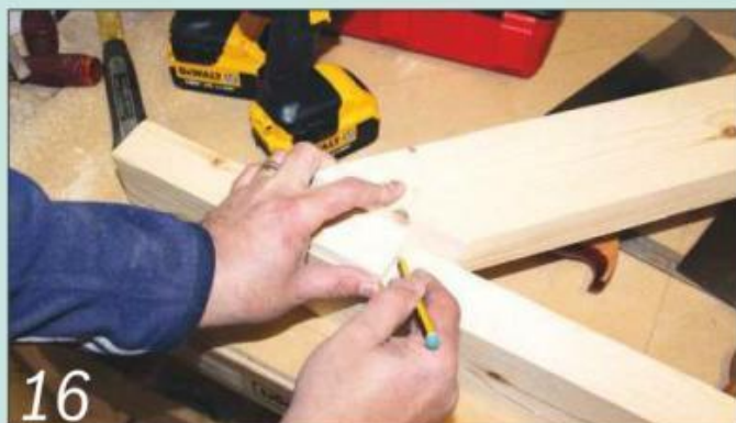
Cut the angled tenons on the brace and use them to mark the mortises
