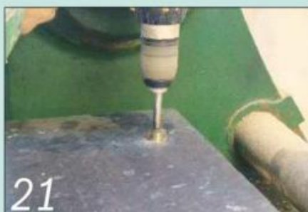
21 Drill a hole for a T-nut in the baseplate to secure the pivot point
