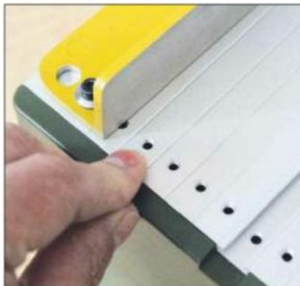
A series of holes allows the fence to be repositioned for cutting grooves
