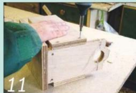
Make up the rest of the cradle from 18mm plywood, glued and screwed together
