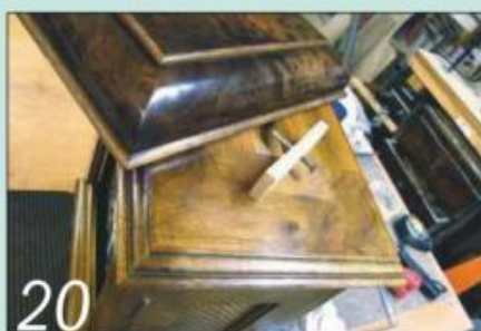
20 Attach the bell top to the case using two small wooden toggles and a couple of long screws
