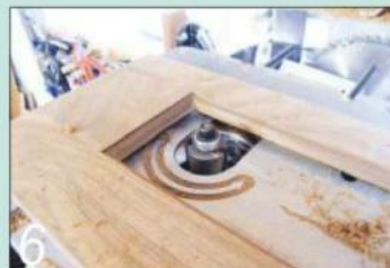
6 Cut a recess on the inside of each side frame to receive the brass fretwork
