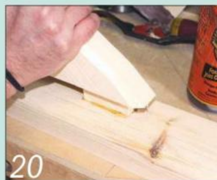
Glue the brace tenons into their mortises and secure each one with a single screw
