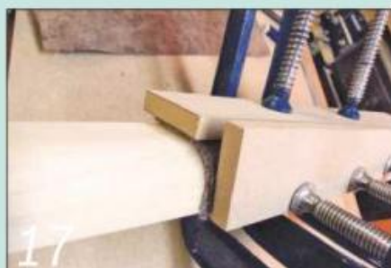
17 Make the bell top sections by gluing veneer to a quadrant-shaped softwood moulding
