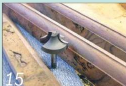
15 Veneer the timber for the bottom moulding and then form the edge profile
