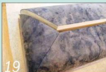
19 Cut the four bell top sections with mitred ends as shown and glue them together
