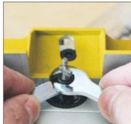
Two small spanners (supplied) are needed to fit and swap the cutters
