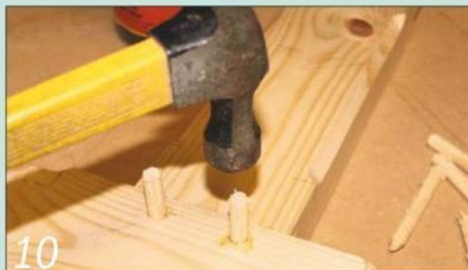
10 Hammer in the dowels to draw the tenons tightly into their mortises
