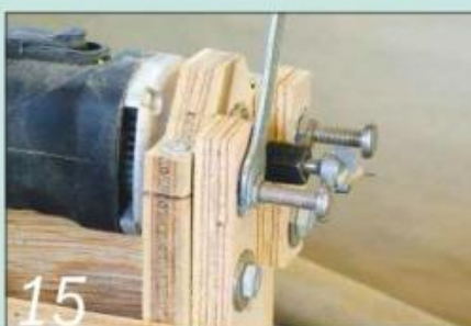
15 Mount plywood strips containing follower bolts to the front face of the cradle
