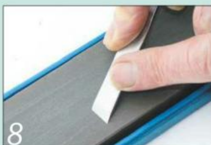
8 Keep your miniature tools sharp using a diamond or ceramic stone
