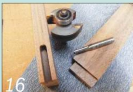
16 The rear door is a simple frame assembled with mortise-and-tenon joints
