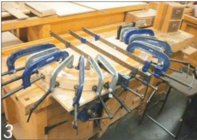
3 I cramped the laminate strips that form the curved bottom rail round a former made up from three layers of 18mm thick mdf
