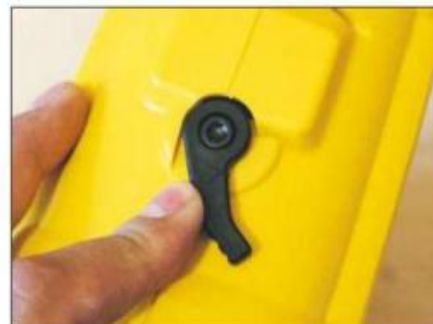
If the firing pin jams because of a misfire, this lever resets it
