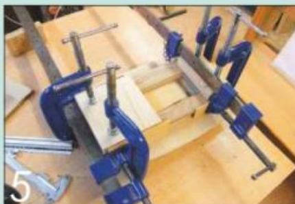
5 Assemble the side frames, check them for square and cramp them up
