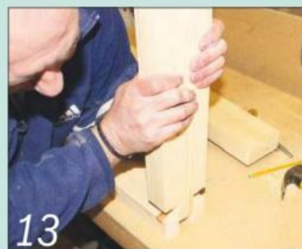
13 Test-fit the joint; the two components should go together tightly for maximum strength
