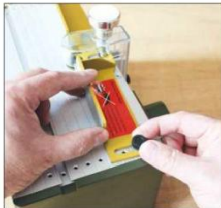
The fence is fixed at one end and can be pivoted on the infeed side
