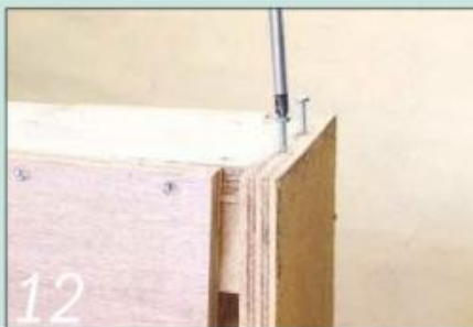
Drive two roundhead screws part-way into the bottom edge of the cradle base
