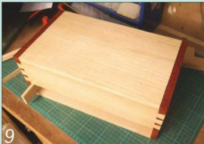
9 Cut the drawer components to size and test the fit of their side pieces
