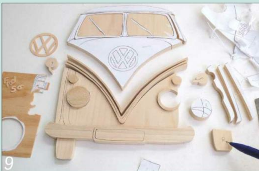
9 Peel off the paper patterns and label mirror-image parts such as the wheels with an L or an R
