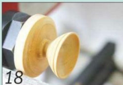
18 Make small dowelled glue chucks for turning bowls, platters and vases
