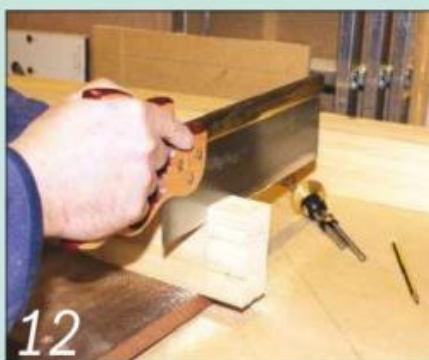
12 The gallows bracket components are joined together with a simple corner bridle joint
