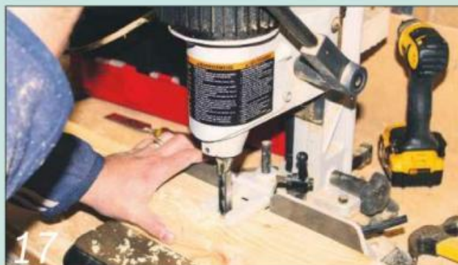
Cut the through mortises, flipping the work end over end for a clean cut
