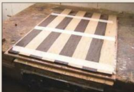
1 Tape the veneer strips together, stick them to the first baseboard and cut them at right angles
