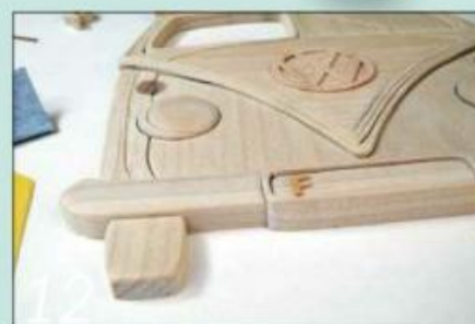
12 Hand-sand all the parts to give them a more rounded and finished look
