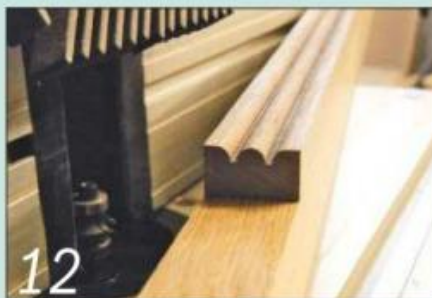
12 Use a sunk bead cutter to form a bead in the centre of the walnut strip
