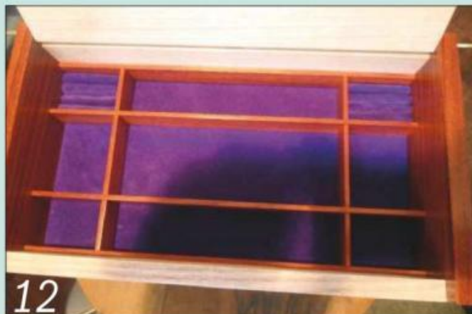
12 Fit the suede in the fixed compartment and add the liners and dividers
