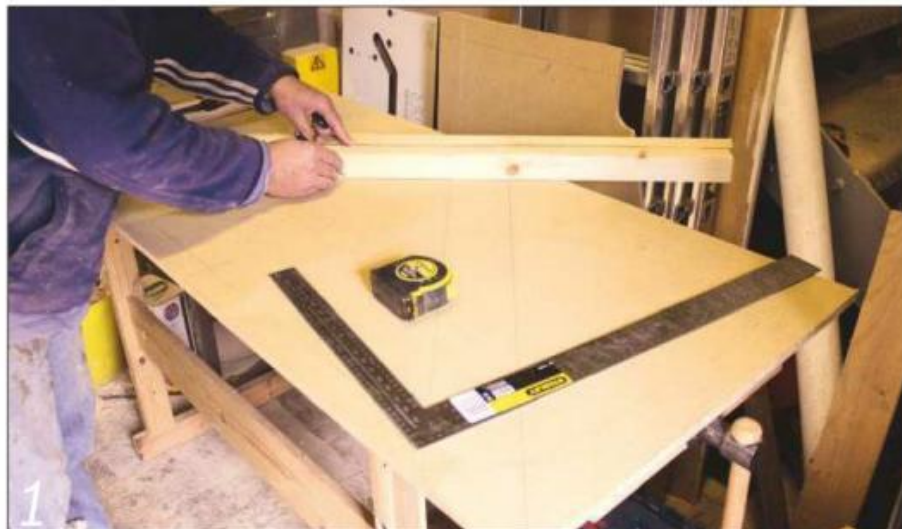
A setting-out rod is an essential aid to easy and accurate working
