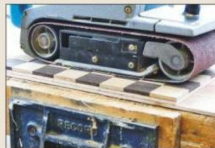
2 Glue these strips to the second baseboard and sand the face and edges
