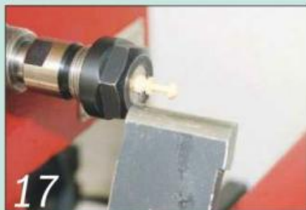
17 Form knobs and finials on a short length of wood held in the collet
