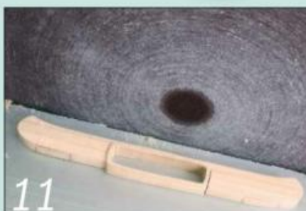
11 Reduce the thickness of the bumper on the disc sander so the number-plate surround projects
