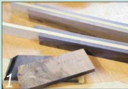
1 Feed the wood through the thicknesser on either side of a carrier strip of mdf
