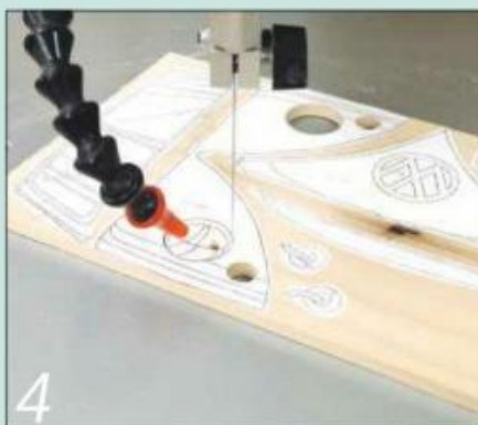
Cut out and remove the headlights and sidelights from the 6mm thick wood
