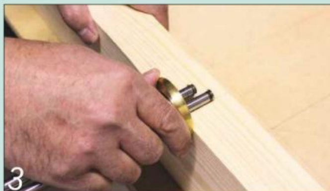
3 Draw in the tenon lines and outline the mortises with a sharp gauge
