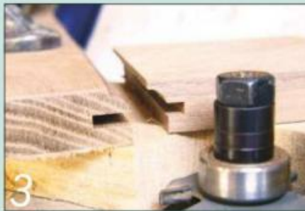
3 The result resembles a profile-and-scribe joint, but without the tongue
