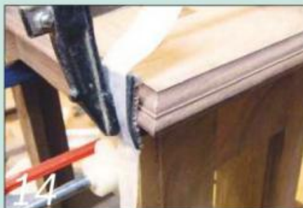
14 Cut the moulding to length, mitre its ends and glue it round the top panel
