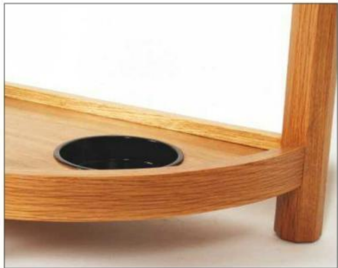
4 The curved rail needed planing and sanding down to its finished width. I trued up one edge with a plane before machining the other one parallel
