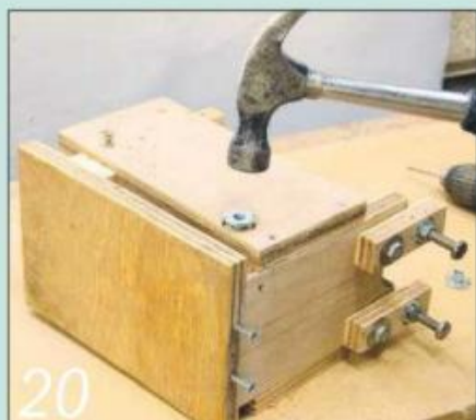
20 Use T-nuts driven into holes in the sides of the cradle to bolt the outrigger on
