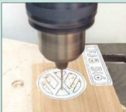
Use a twist drill bit in a pillar drill to make the blade entry holes for all the internal cut-outs
