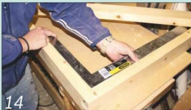
14 Glue and screw the corner joint and check that it's perfectly square
