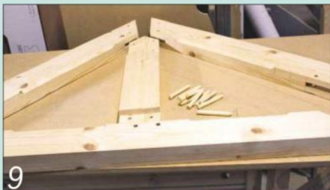
9 The truss is now ready for assembly. Note the complex bridle joint at the top
