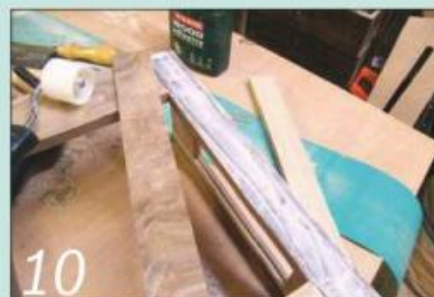
10 Cut some walnut veneer and glue it to the rear frame to hide the joints
