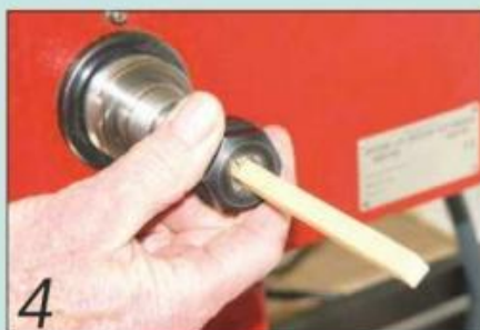
4 Finger-tightening the nose-cone nut is sufficient to secure the blank
