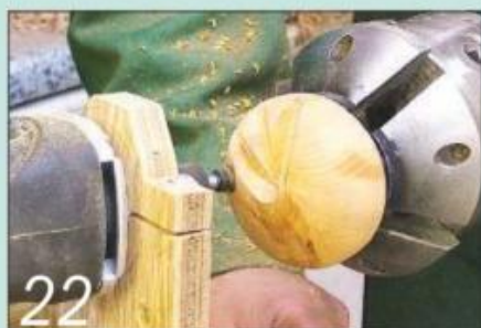
22 The router cuts elegant grooves in the work as the cradle rotates
