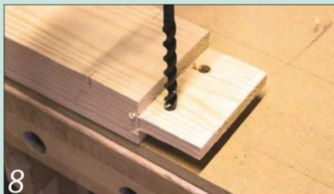
8 Mark the hole positions on the tenons, then drill them closer to the shoulder
