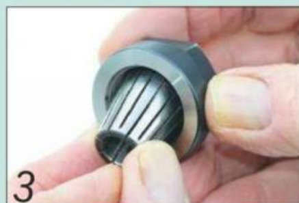
3 The nose cone nut is only 35mm in diameter, so doesn't get in the way when turning
