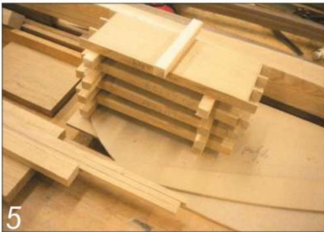
5 I prepared the key box components using a dovetail saw, a coping saw and a chisel, plus a small router to remove most of the dovetail waste
