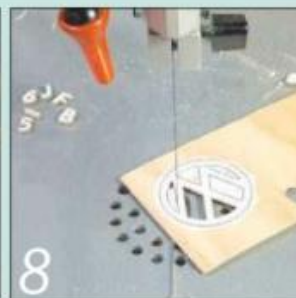
8 Cut out the thinnest parts such as the VW badge and the letters and numerals from 2mm wood
