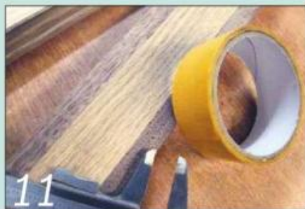
11 Stick the walnut strip to the edge of the bearer using double-sided tape
