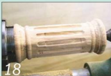
18 ...to create a series of parallel flutes as the blank is rotated on the lathe
