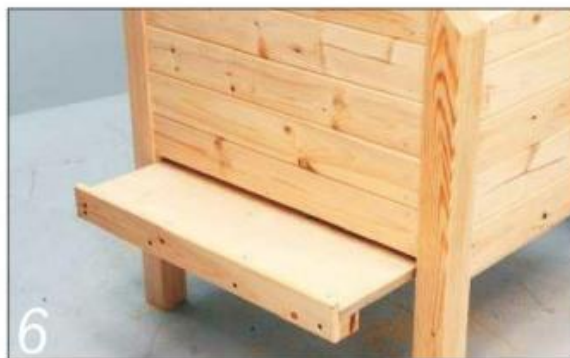
6 A piece of the cladding attached to a packing block at the back end of the tray acts as a sturdy handle and completes this part of the job
