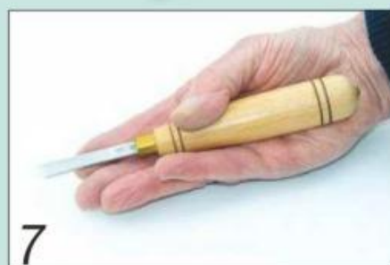
7 I prefer a skew chisel with a rectangular cross-section as it's more rigid
