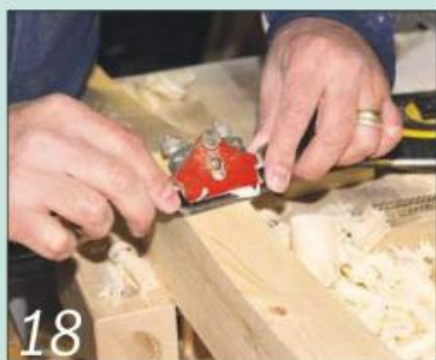
Form the shallow curves on the bandsaw and smooth them with a spokeshave
