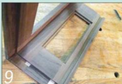
9 Make up the rear frame and test its fit. Note the rebates for the floor panel
