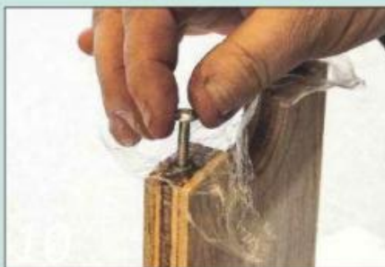
Use clingfilm to keep the glue from contaminating the nut's thread
