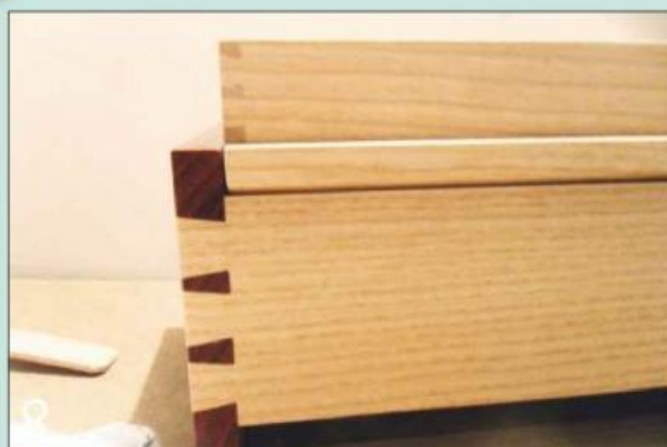
8 The tray dovetails are cut in the same orientation as those on the carcass
