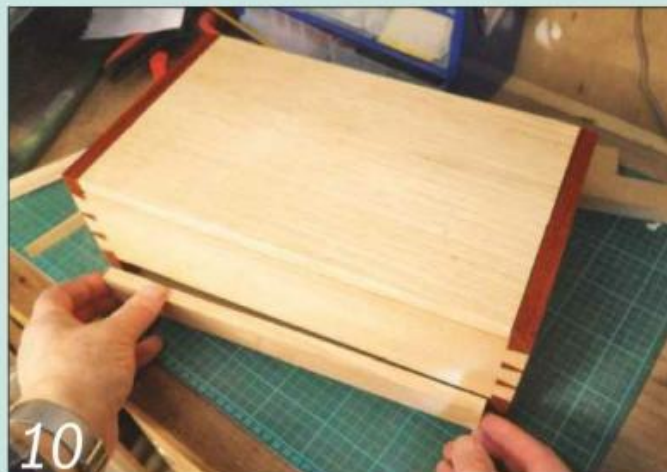
10 Re-thickness the drawer front to 10mm and aim for a good sliding fit
