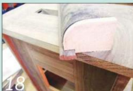
18 Machine a slim walnut lipping and glue it into a rebate cut in the quadrant
