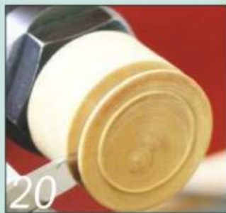
20 When you've finished turning, use a parting tool to release the work and remove any glue residue
