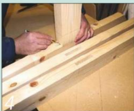
4 Cut the rafter mortises first, then use them to mark the cross-beam tenons
