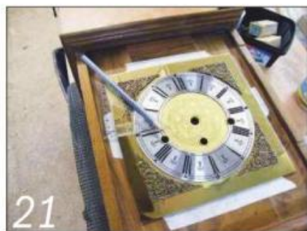
21 Mount the face on the dial mask. Then fit the movement and the other hardware
