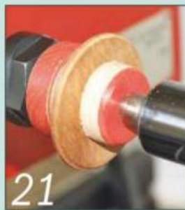
21 Use pressure pads to sandwich items such as tabletops for turning
