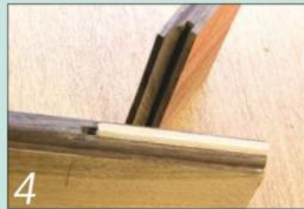
4 Sand a plywood tongue down in thickness to fit snugly in the slots
