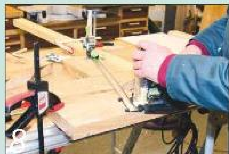
Fit the trammel bar to the jigsaw and make the curved cuts on each leg
