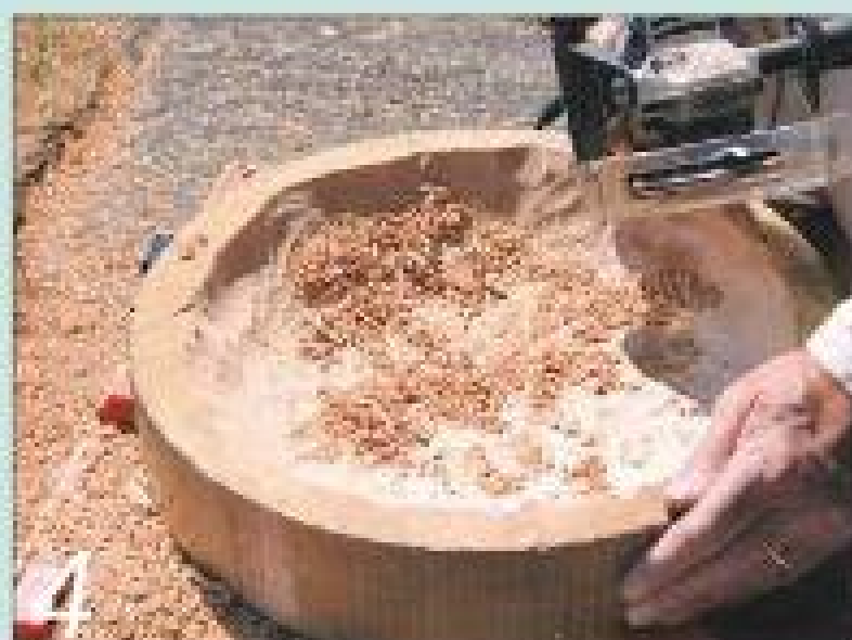
4 The cuts gradually go deeper and deeper, but still leave a good margin all round
