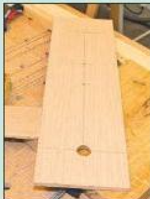
The guidebush in the router trammel forms the perfect holder for a pencil
