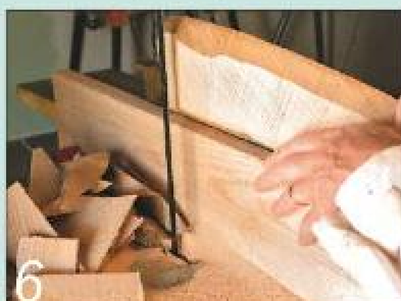
6 A series of angled cuts made on the bandsaw quickly removes waste from underneath
