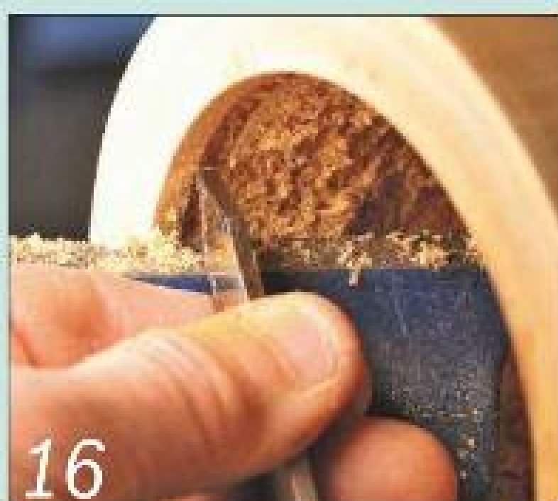
16 Cut a groove to hold the container's loose base panel using a parting tool
