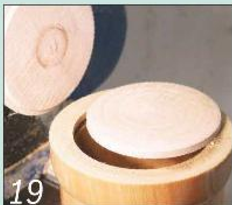
19 Push the disc into the bottom of the container and position it within its groove
