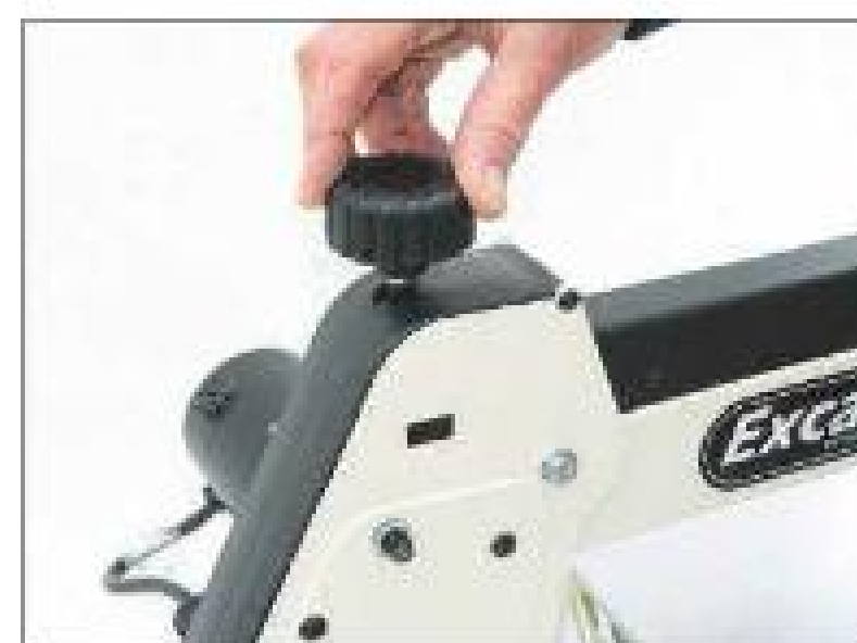
A large tension setting knob is positioned at the top rear of the machine
