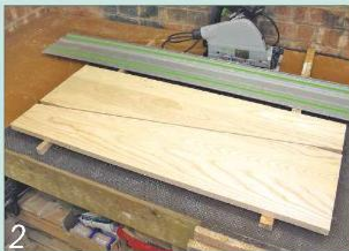
I used a circular saw and guide rail to cut the angled side panels to size
