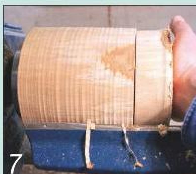
Mount the severed lid on a jam chuck formed in the end of the base section
