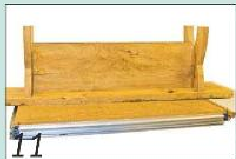
Position the frame board and legs on the top and mark the clearances
