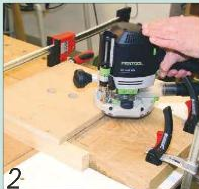
2 The router runs against the ends of the jig to cut the ends of the channel
