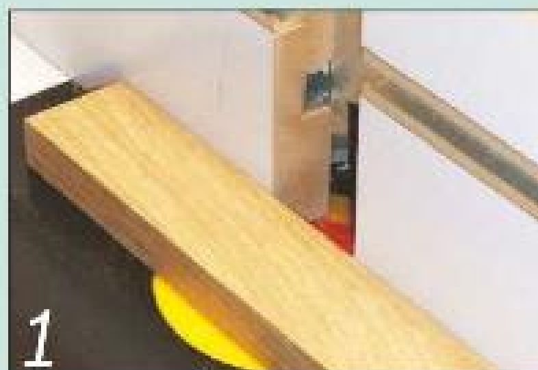
1 I got cleaner rebates by passing the workpiece face down over the router cutter.
