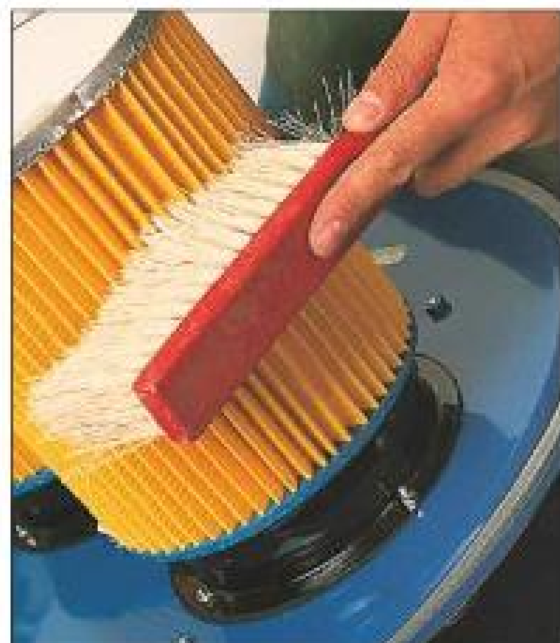
5 You have to keep paper filters clean to ensure that they remain efficient
