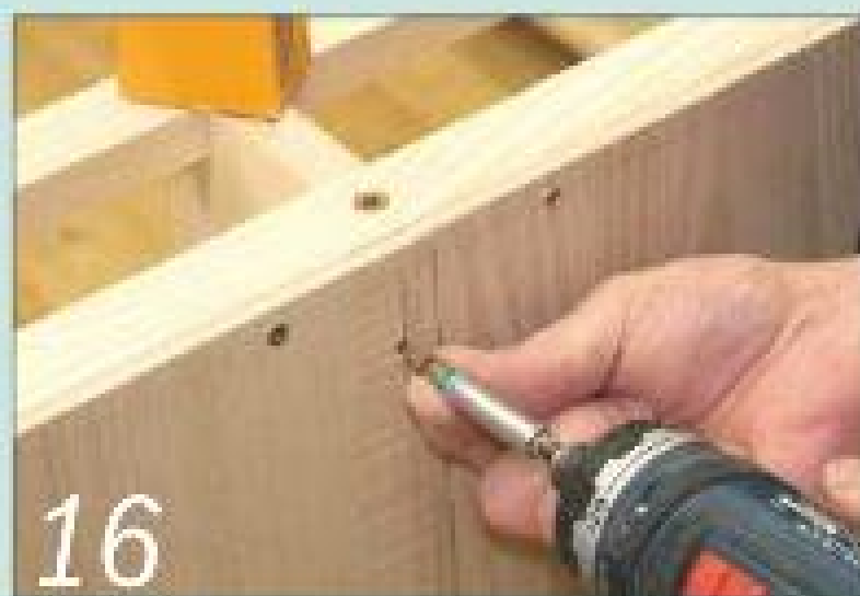
16 Butt join the back panels behind the supports and screw them in place
