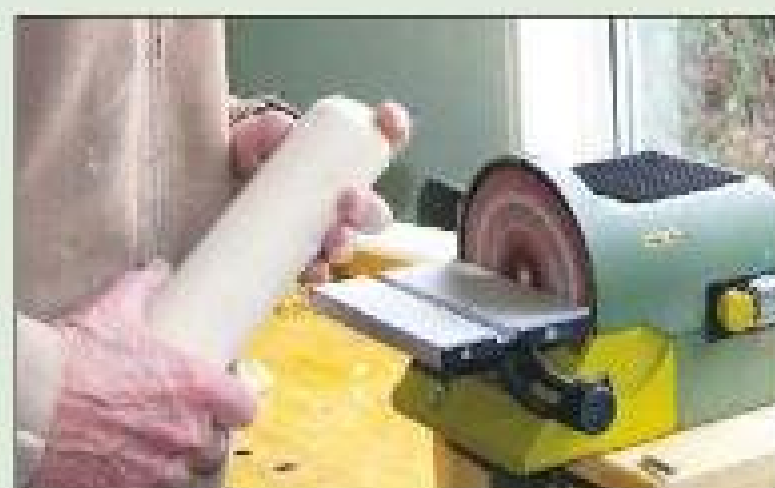
9 Sand off the saw marks and finish the pin with a final hand sanding
