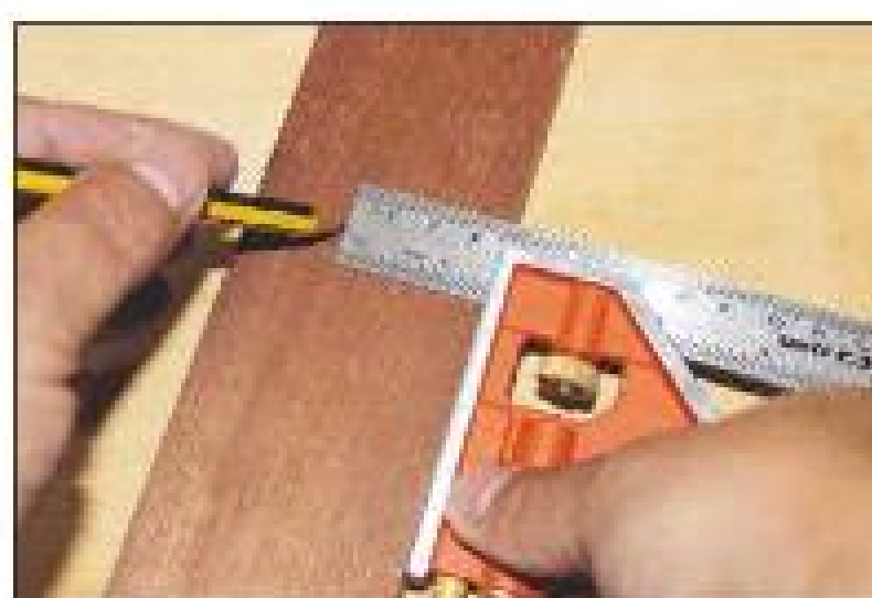
It's equally controllable and perfectly accurate for striking parallel lines
