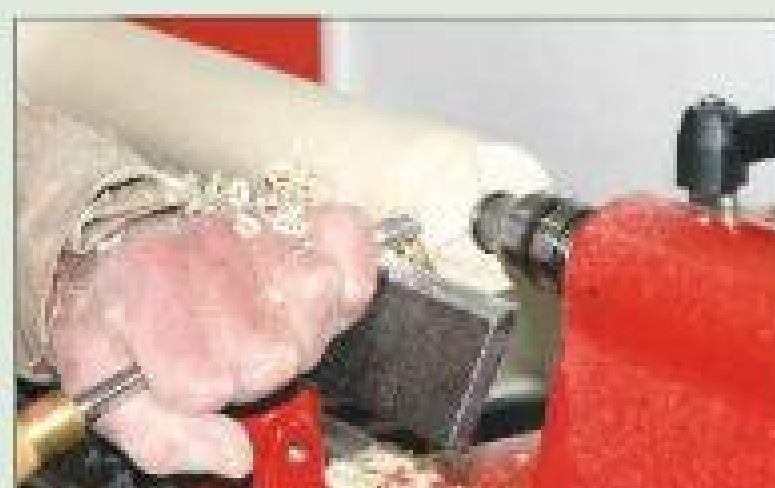
7 Then shape each end to a smooth, round curve with a spindle gouge
