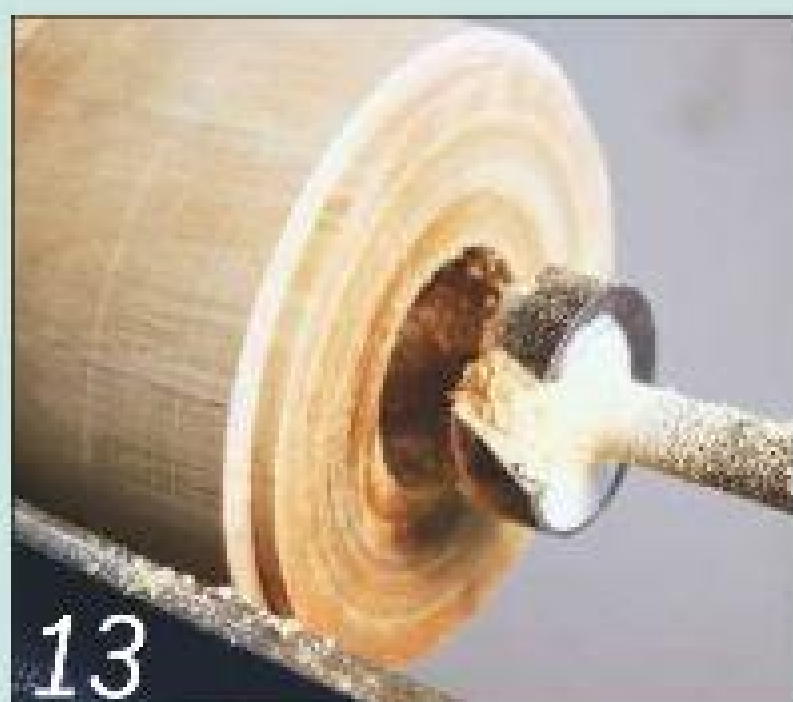
13 Bore a pilot hole in the base using a saw-toothed centre bit in the tailstock
