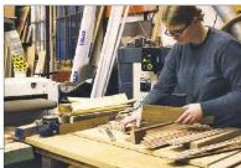
Laminating timber is the prelude to creating a patterned turning blank
