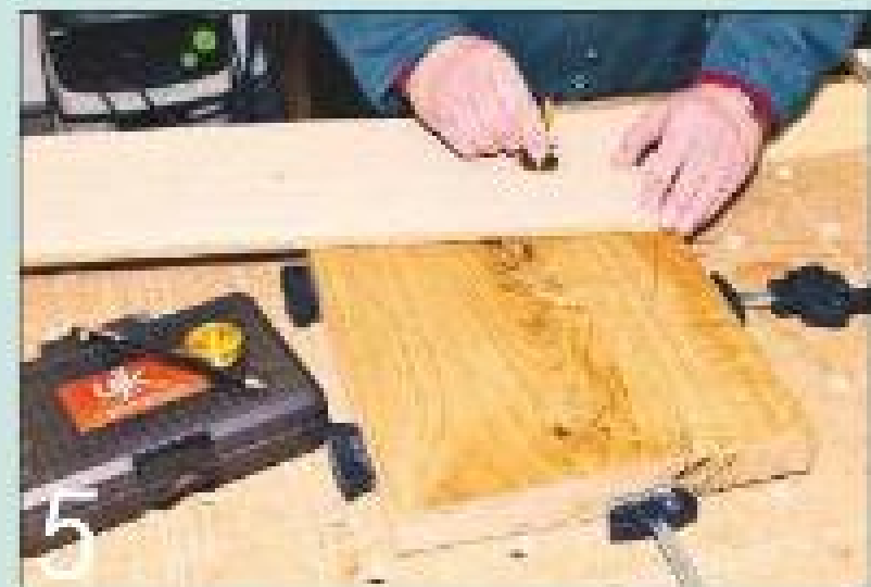
The guidebush in the router trammel forms the perfect holder for a pencil
