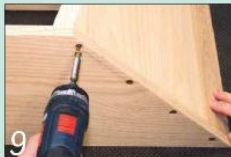
9 Begin the assembly by screwing the base to the inner side panel
