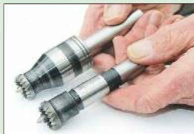
1 Mount the blank between centres; these Steb centres are ideal for this
