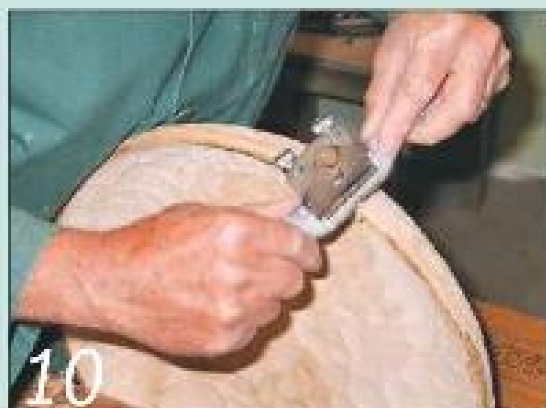
Finish off the rim to less than 12mm thick with a sharp spokeshave
