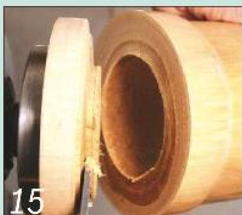
15 To complete the hollowing-out process, part the base off below the plinth
