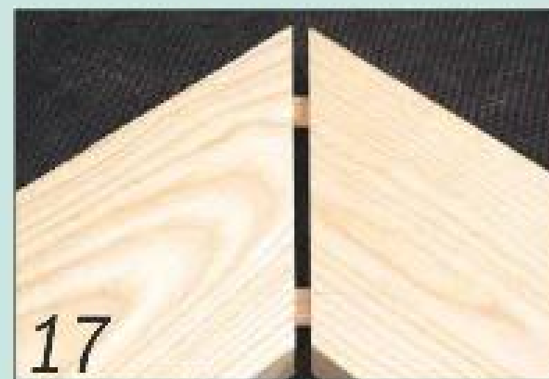
17 Add two floating tenons to reinforce the mitre joint between the top sections
