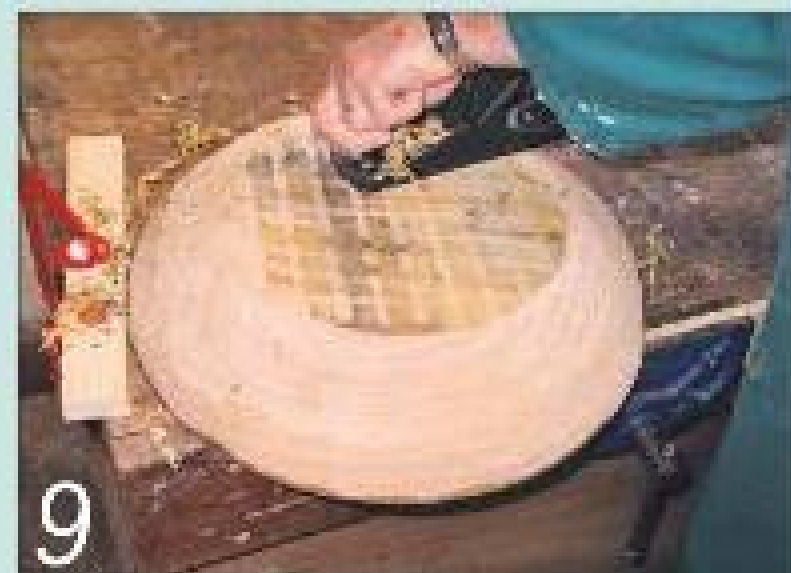
The rough-sawn base of the bowl can be trimmed flat with a sharp plane
