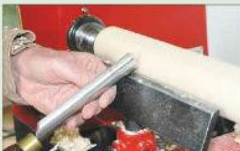
2 Start to turn the blank to round using a spindle roughing gouge
