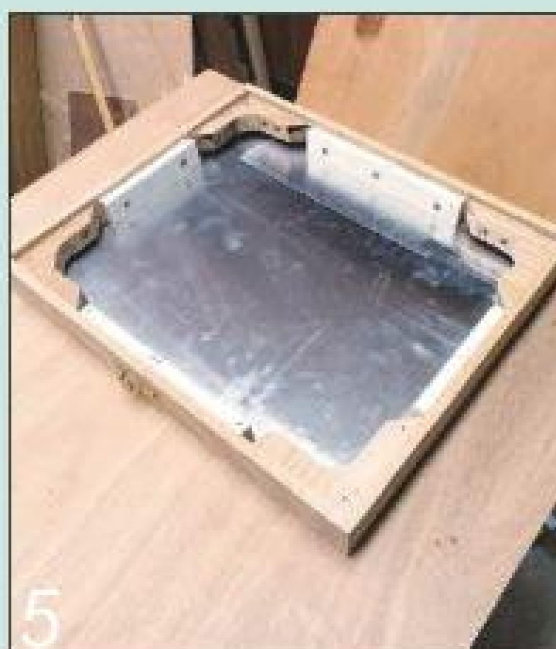
5 ...and were then screwed into the frame corners. Note the reinforcing beads between them.
