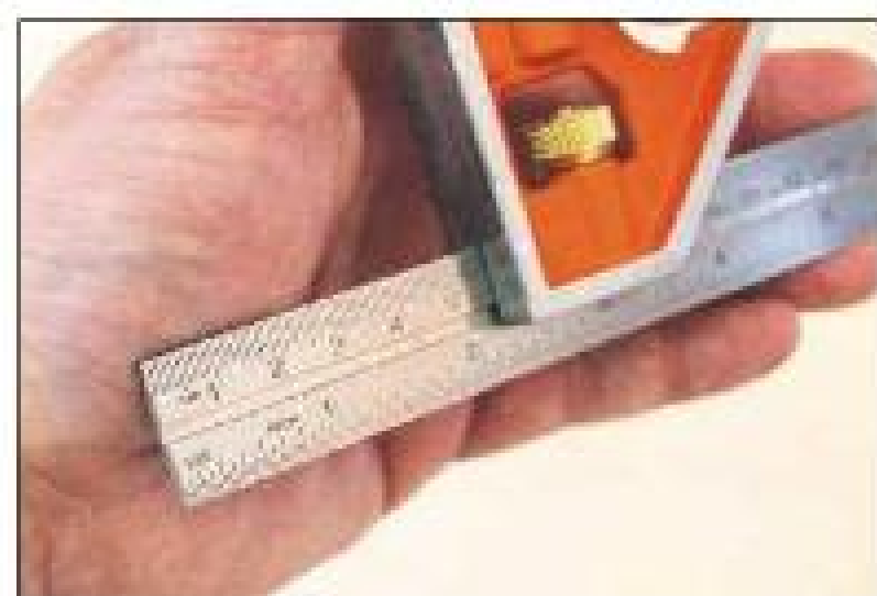
The steel blade is deeply etched with metric and imperial measurements
