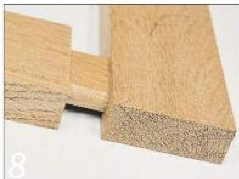
8 I used a relatively oversized tenon 12mm thick for maximum strength
