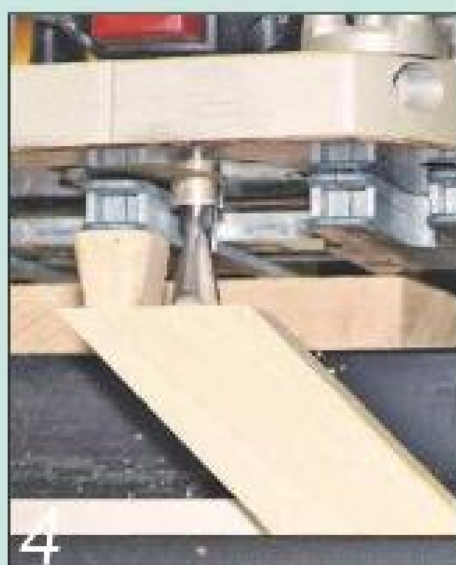
Prepare the rails and cut the angled tails on them using a dovetail jig
