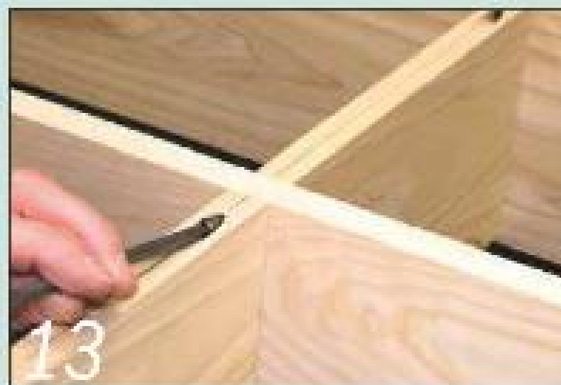
13 The others are fixed through the shelf above and at the top rear edge
