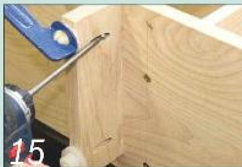
15 The bookcase feet are simple rectangles attached with pocket-hole screws
