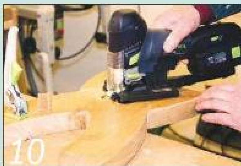
...and remove the centre section with freehand cuts using the jigsaw
