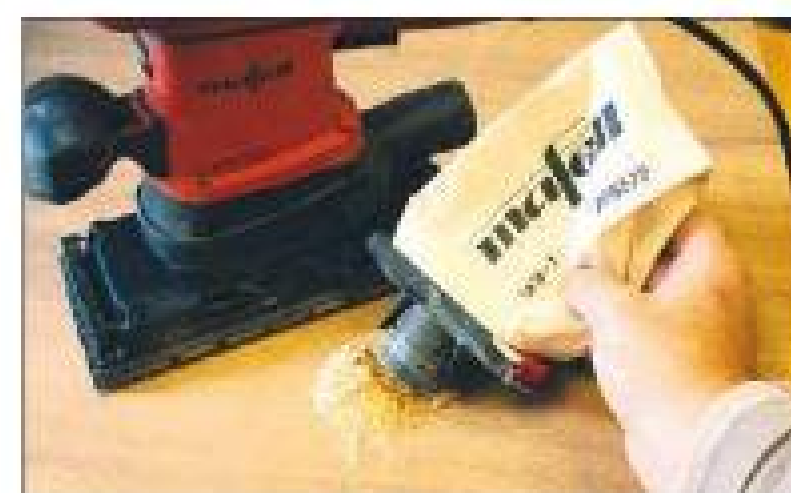
1 The best on-board dust collectors can collect a lot of the waste
