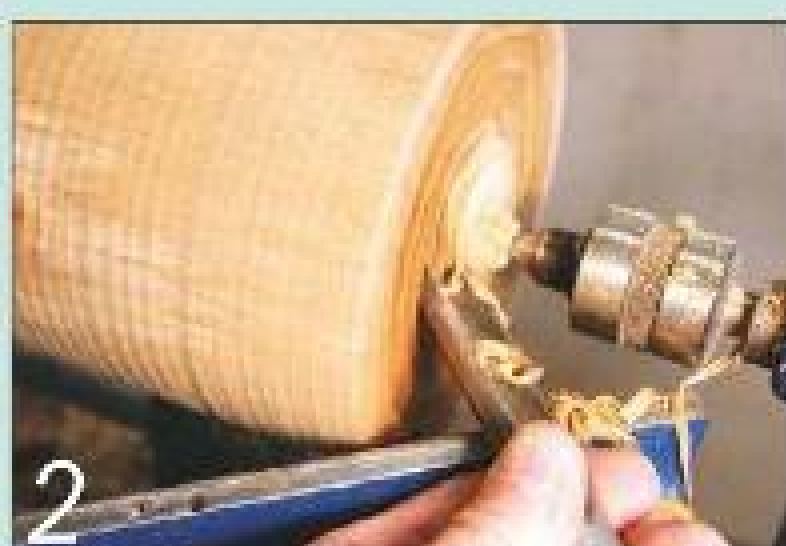
2 Set the toolrest at a 45° angle and slice the end square with a bowl gouge
