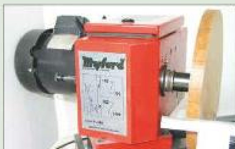
2 Swing the lathe head round and fix the faceplate to the headstock spindle
