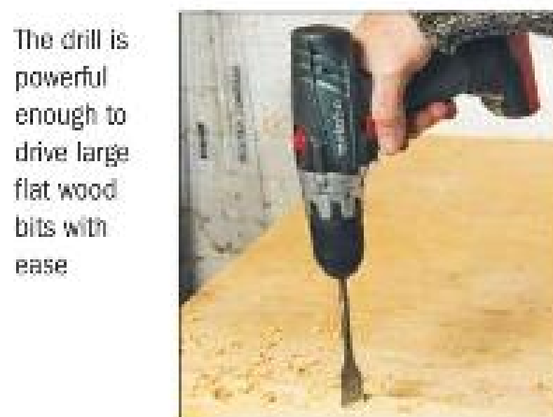
The 10mm capacity keyless chuck screws directly onto the bit-holder
