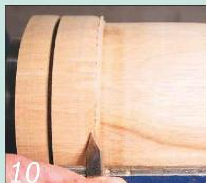
Cut in with a parting tool and then roll the tool on its side to form a bead
