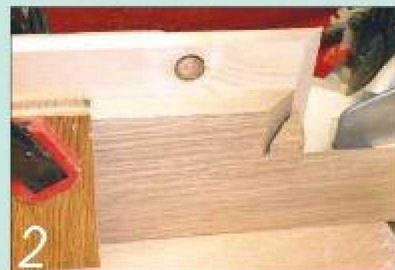
2 I cramped the frame rails one above the other to ensure that I cut the mitres accurately.
