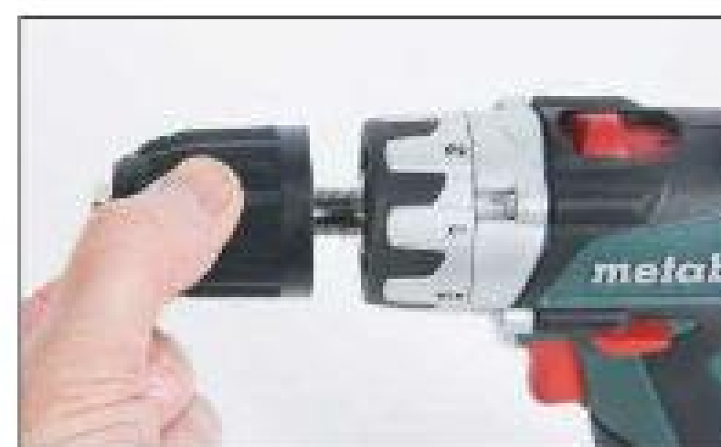
The 10mm capacity keyless chuck screws directly onto the bit-holder
