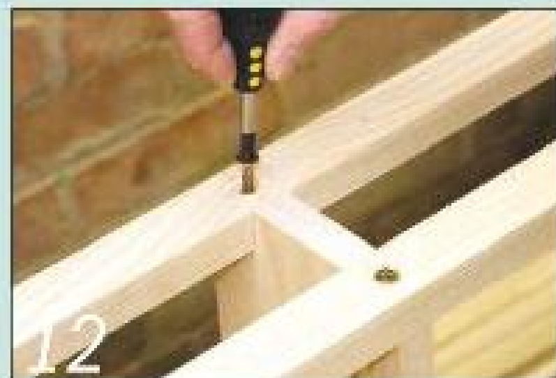
12 The upper notched supports are screwed into the rails, top and bottom
