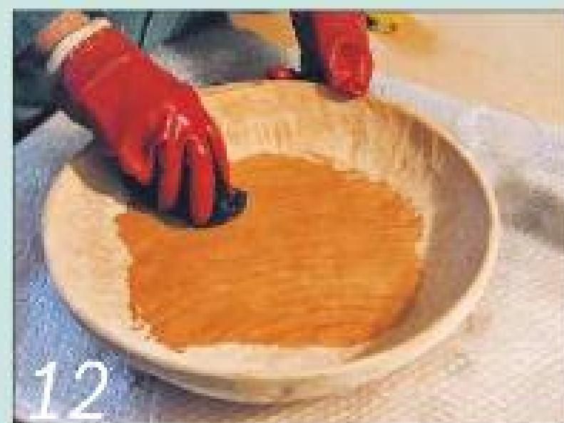
Dilute the first coat of tung oil and follow it up with a couple more full-strength coats
