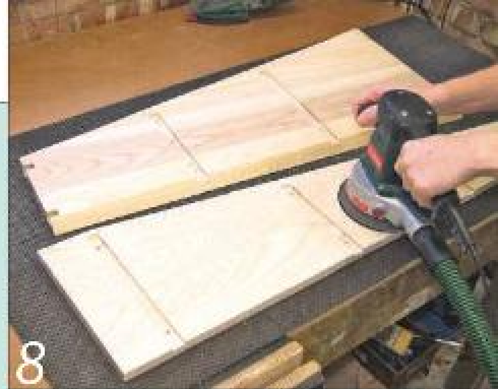
8 With all the sockets and housings cut, sand each side panel smooth
