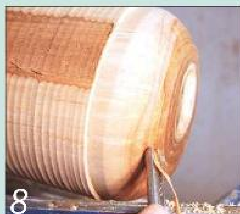
Use a slicing cut with the bowl gouge to form the dome shape of the lid
