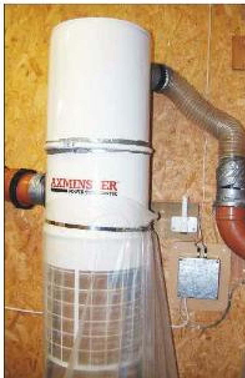
1 Wall-mounted systems simply dump the waste into a plastic sack
