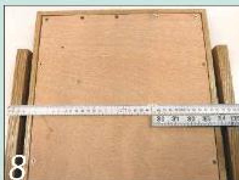
8 Measure the overall width and transfer this measurement to the base panel.
