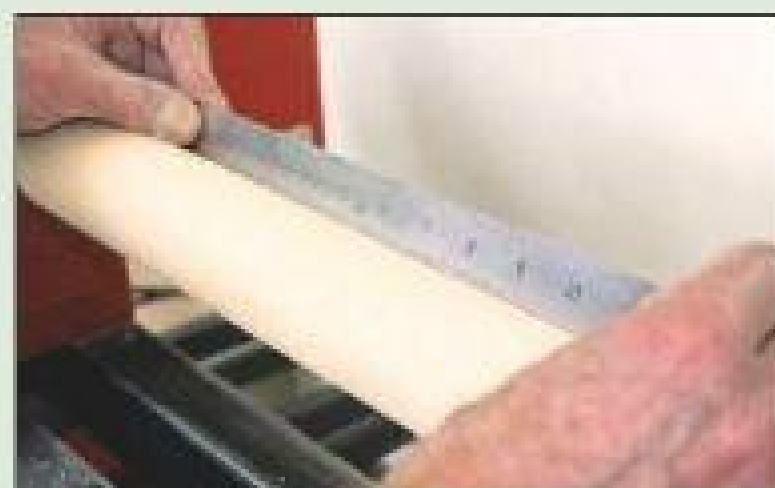
5 Hold a steel ruler against the cylinder to check for any discrepancies
