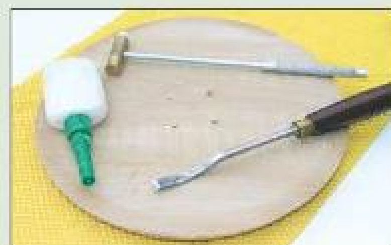
9 Unscrew the faceplate and fill the screw holes with small glued-in dowels
