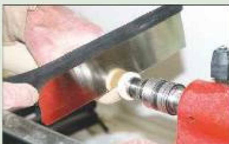
8 When you have just 10mm of wood left, cut through it with a saw
