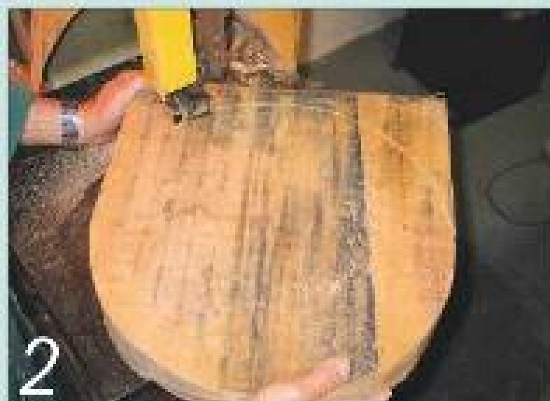
2 After cutting a chunk off, I scribed out a large circle and cut it out on the bandsaw
