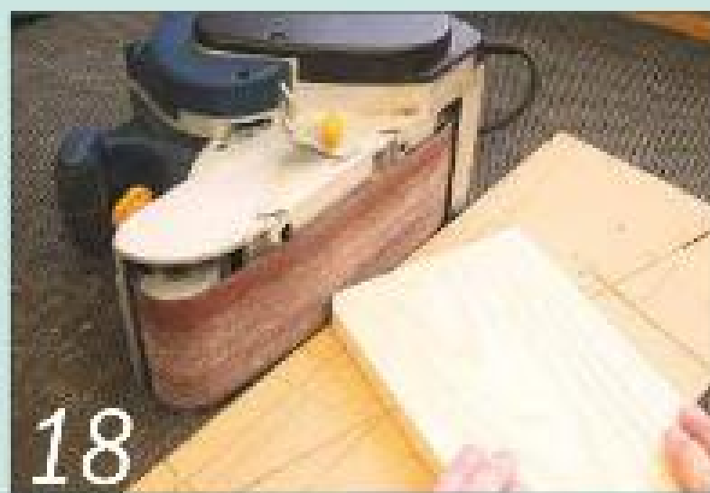
18 Round off the external corners of the top sections on the belt sander
