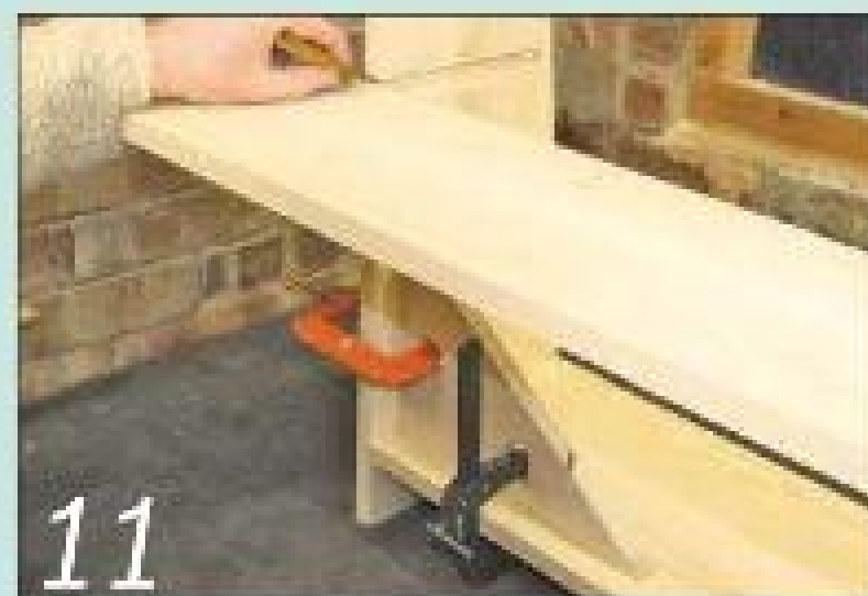
11 Mark the length of each shelf directly from the rear of the carcass
