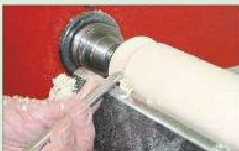
6 Measure 10mm in at each end and make a V-cut at each mark
