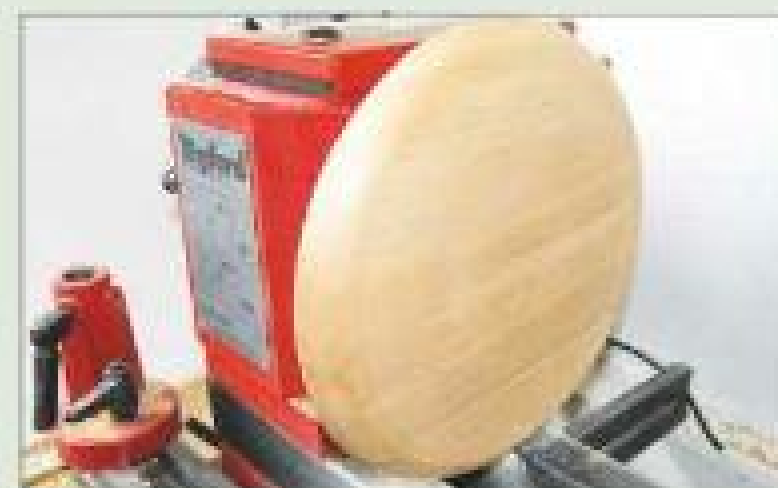
7 Turn a gentle curved chamfer, running down to the edge of the blank
