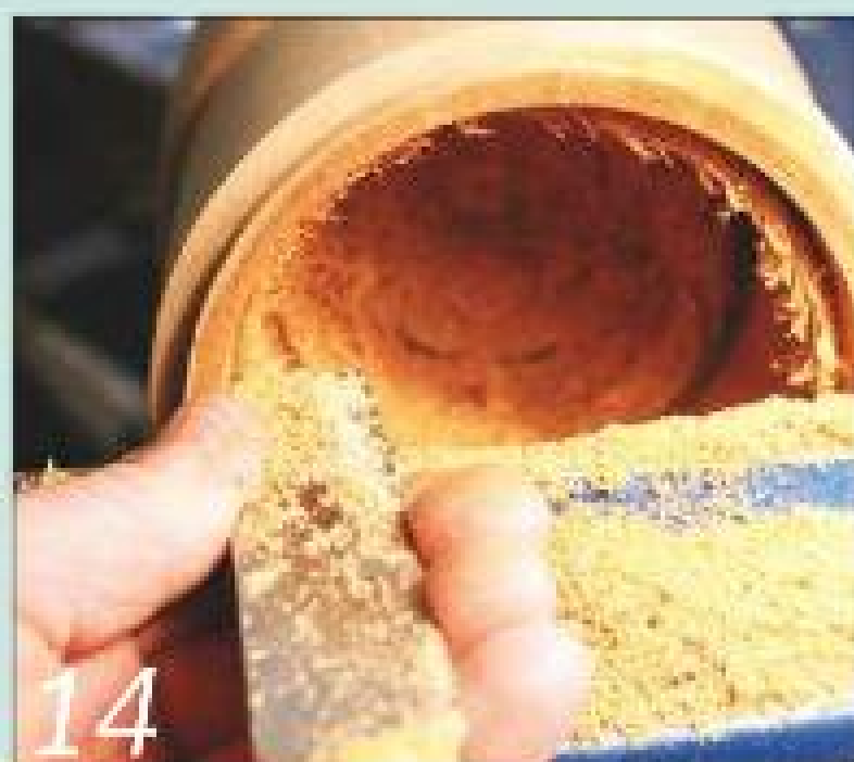
14 Gradually widen the inside of the base to its full size with a square scraper
