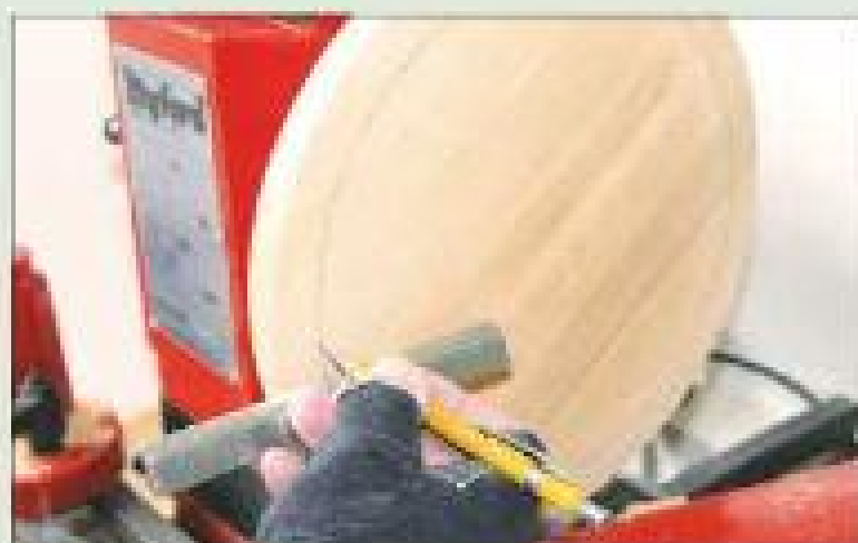
6 Draw a pencil line 20mm in from the edge to mark the rim area
