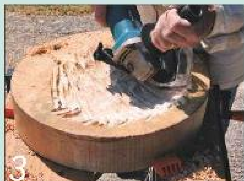
3 Make the first few cuts well in from the edge until you get the hang of it
