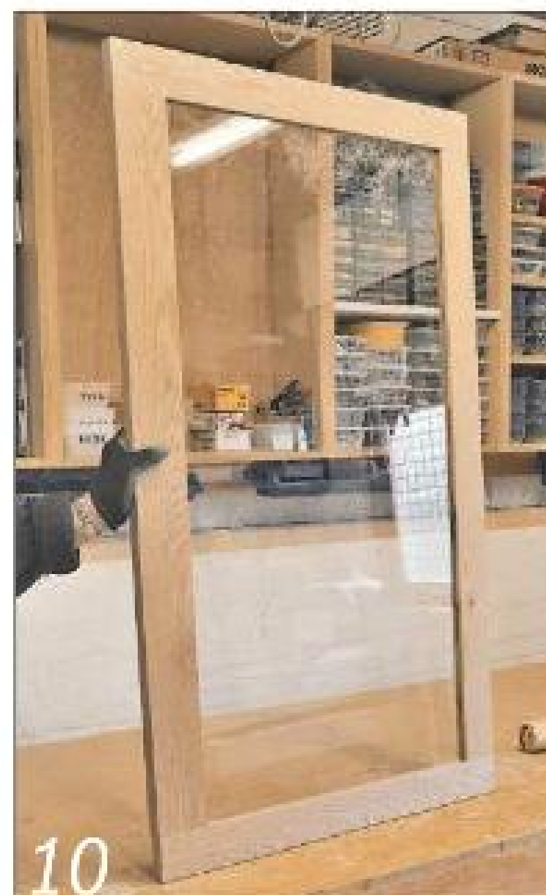
10 A dry fit made sure that the polycarbonate sheet could move freely within the frame
