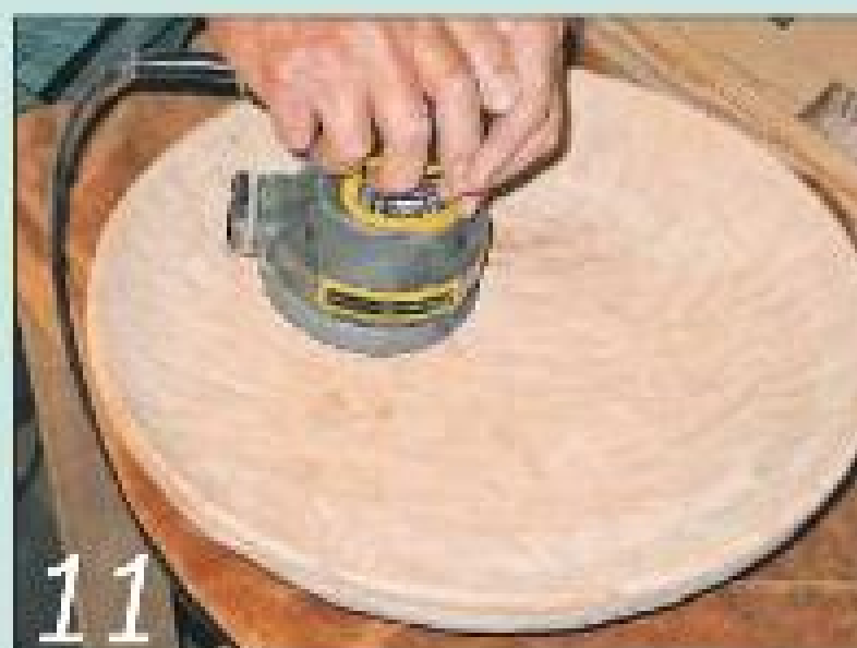
Sand off the rough ridges, but leave the chiselled effect visible on the surface
