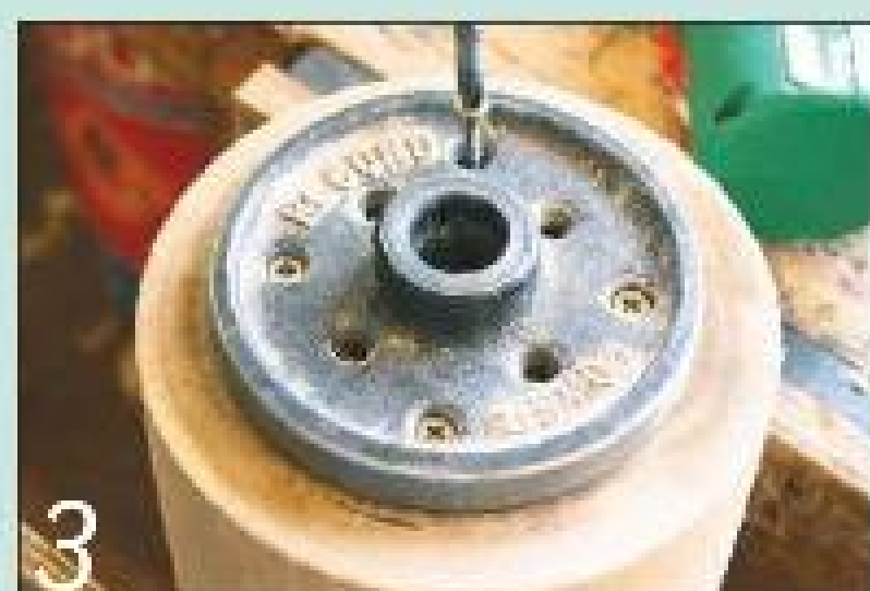
3 Screw a faceplate to one end of the blank using four 25mm long Spax screws
