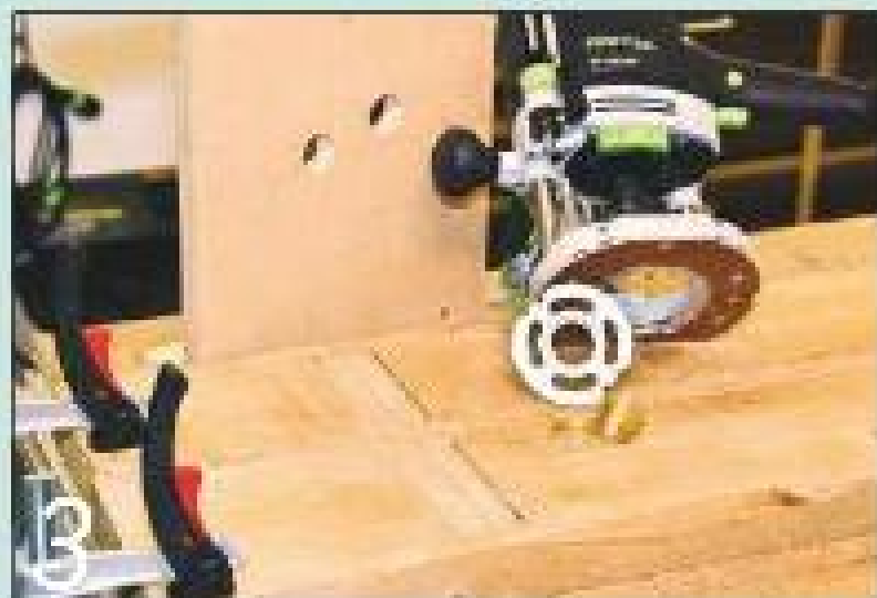
The completed channel in the underside of the bench top looks like this
