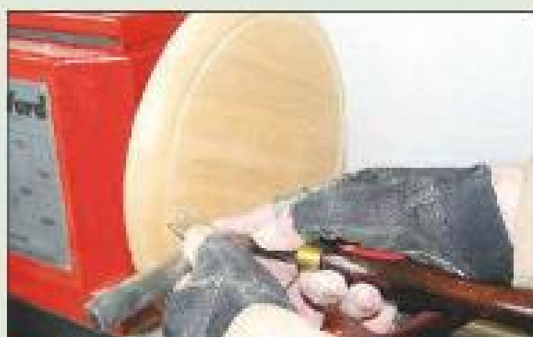
8 Change to a 4mm parting tool and cut a crumb groove 4mm deep
