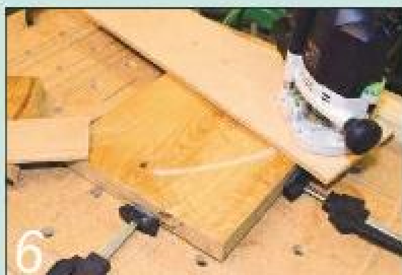
Insert the router in the guidebush and cut the grooves. Note the end stop at the left-hand side
