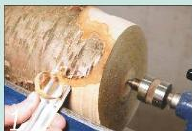
1 Turn the rough section of log down to a cylinder using a freshly-sharpened roughing gouge
