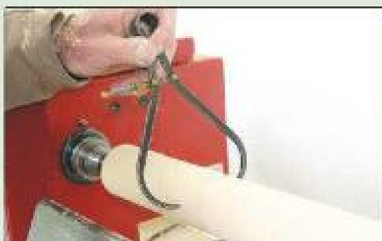
4 Use callipers (with the lathe turned off) to check the diameter as you work
