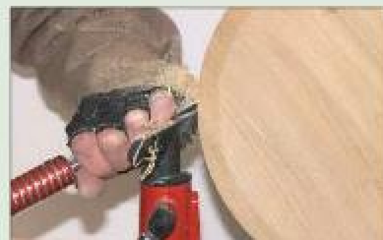
3 Use a sharp bowl gouge to turn the edge of the blank to a true circle
