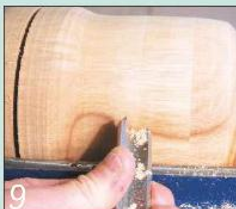
Finish the outside of the box by taking a series of fine parallel cuts
