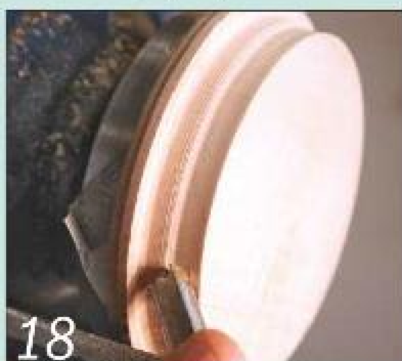
18 Slice the edge of the base disc to the correct diameter and part it off
