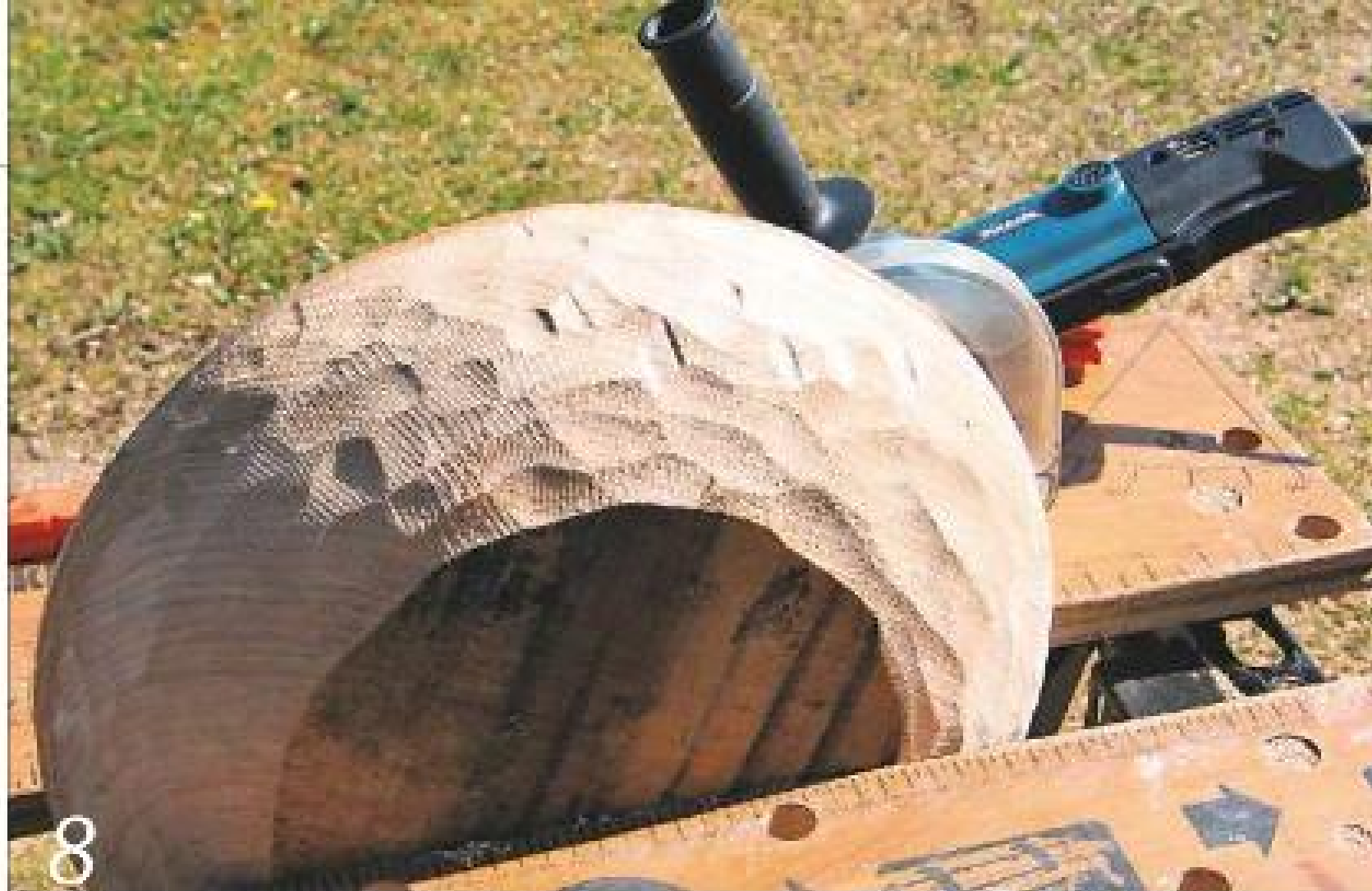
To finish the lower profile, the bowl needs mounting on its edge in the Workmate
