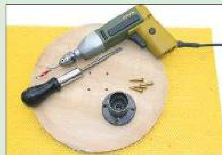
1 Drill pilot holes for the faceplate screws on the underside of the blank
