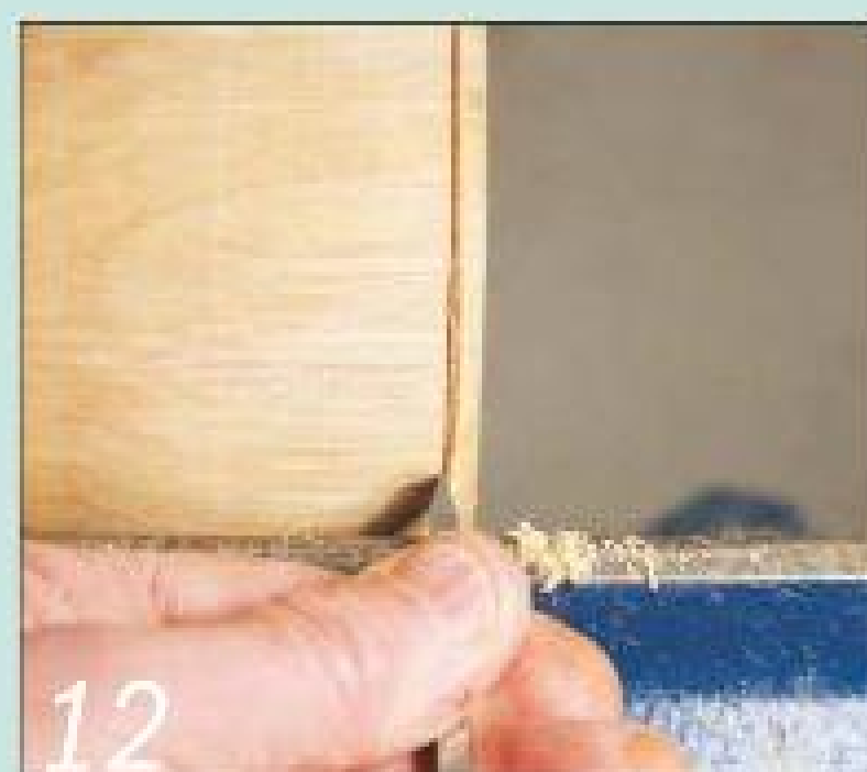
Remove the lid from the chuck and cut a chamfer at the top edge of the base
