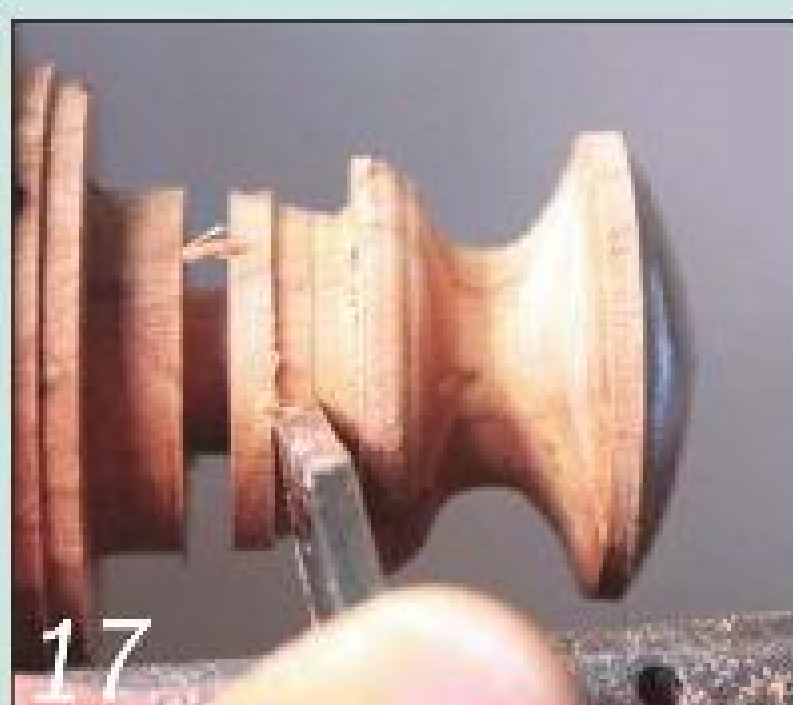
17 Turn a small blank to the knob shape, then form a narrow spigot on one end
