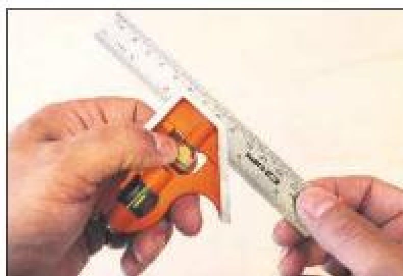
The solid aluminium stock is locked securely in place with a brass knob
