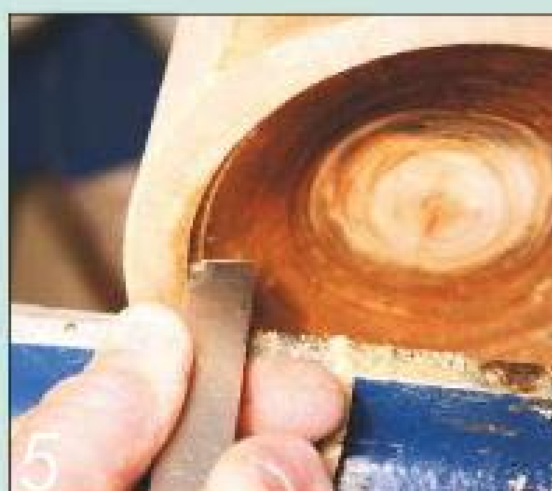
Use a square scraper to form a rebate on the inside edge of the lid
