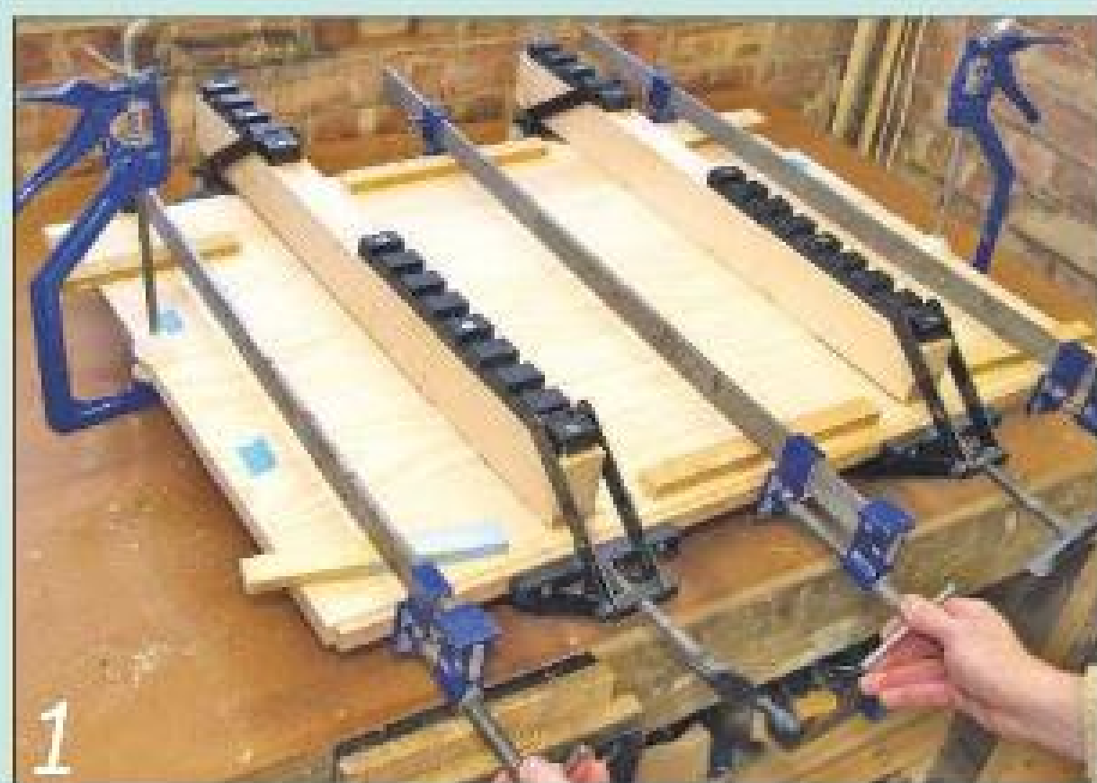
Prepare the ash boards, then glue and cramp them together into panels
