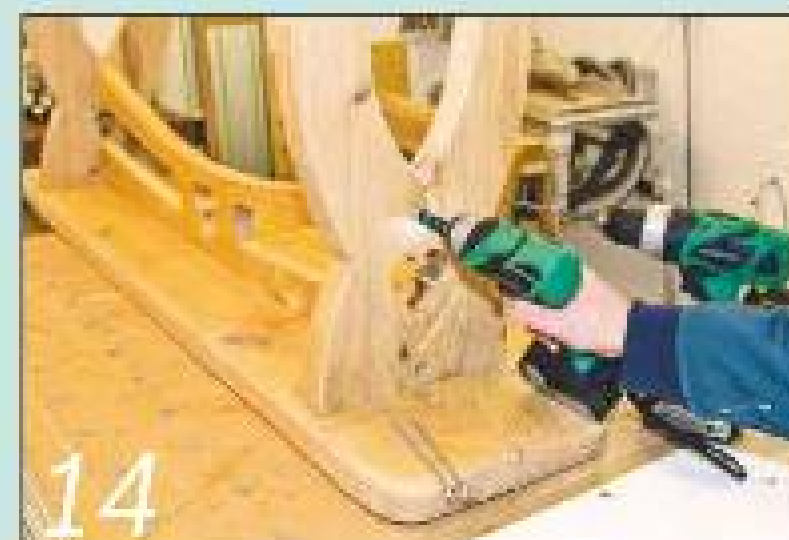
14 Screw the legs to the frame board first, then attach the top to the frame and legs
