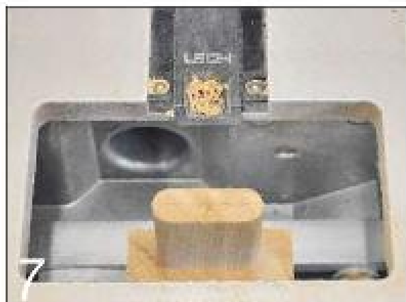
7 The FMT jig produces a very clean tenon which should be a perfect fit
