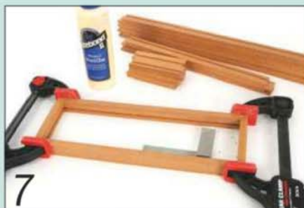
7 Glue and cramp up one side of each frame and check that it's square
