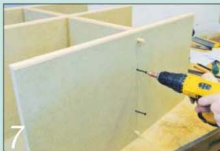
7 Every other joint can be screwed, which speeds up the assembly process dramatically
