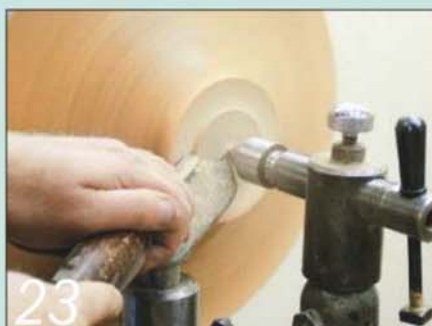
23 Finish the job by reverse-chucking the piece and turning away the spigot
