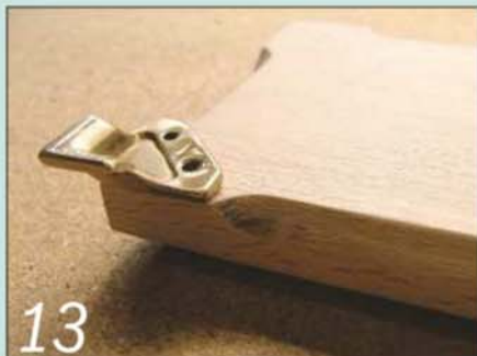
13 Mark the positions of the feet on the base and cut a stopped chamfer between them
