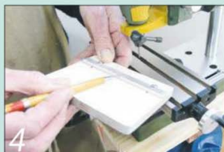
My routing table has a notch 8mm wide in its aluminium angle fence
