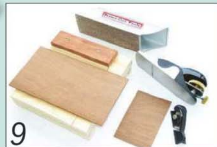
9 True up the edges using a sanding block or a small block or edge plane
