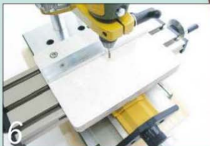
6 The router table can be moved precisely in either direction to position the cutter
