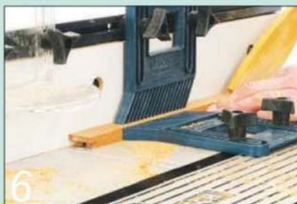
6 Run a groove down one face of each of the frame members to take the glass
