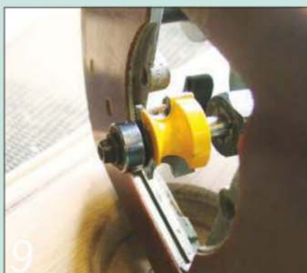
9 Fit an edge beading cutter in your router and set it to cut in from each face
