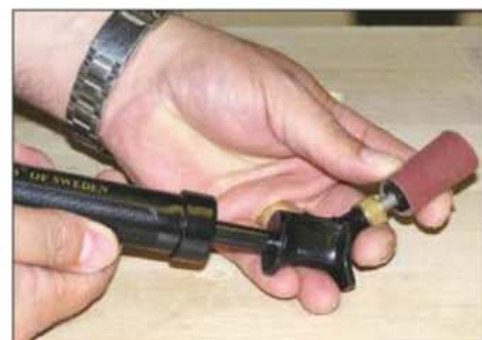
1 Small pneumatic drums can be inflated to different pressures to suit the work
