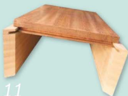
For an integral lid, the panel floats in interlocking grooves
