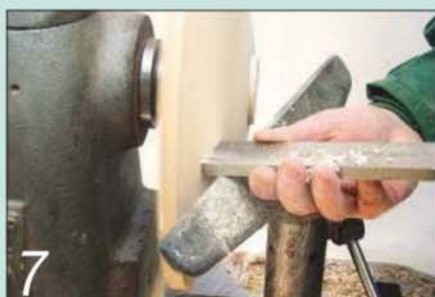
7 Alternatively you can smooth the surface with a square-ended scraper
