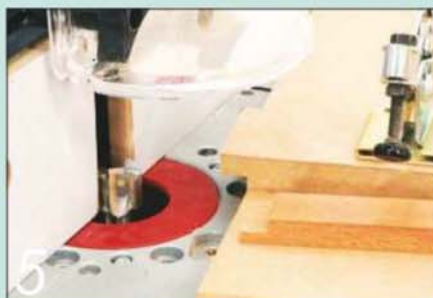
5 The cut goes through into the jig's sacrificial strip to minimise the risk of breakout
