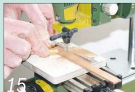
15 Cut a strip for each set of drawer sides and rout a rebate along the bottom edge
