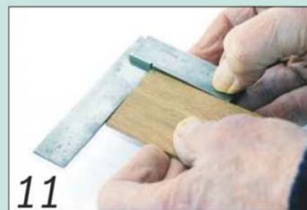
11 A small engineer's square is useful for checking that right angles are true
