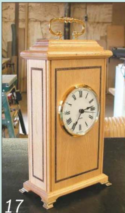
17 Apply the finish, fit the battery, set the clock and push the insert into its recess
