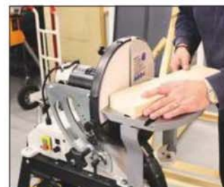
4 This Axminster sander has a unique pivoting motor and static fence
