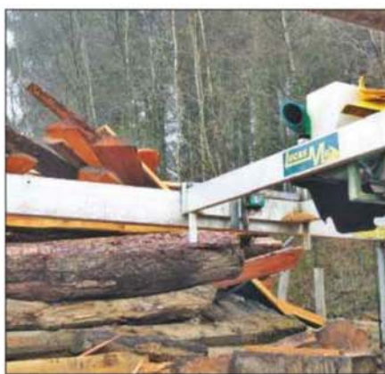
The logs are ripped down using the coarsest saw blade I've ever seen; it has only five teeth!
