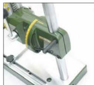
The head can be rotated or moved up and down, locked by a T-bar
