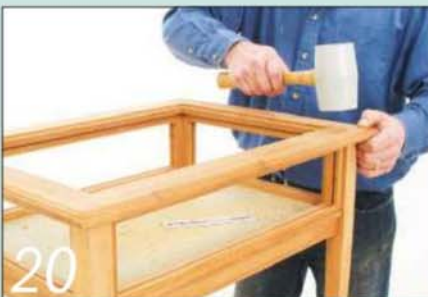
20 Centre the top frame on the table and tap each corner with a soft mallet to mark the underside
