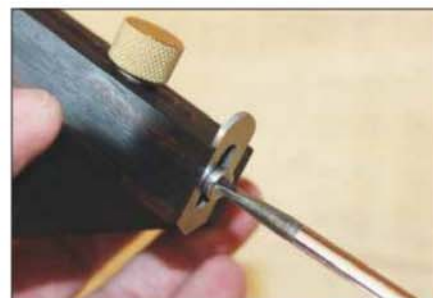
The blade can be adjusted for depth of cut using a screwdriver
