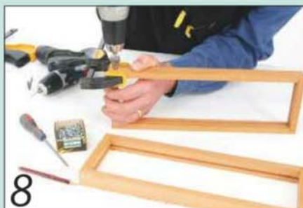
8 Drill and countersink a hole in each top corner so you can fit the rail later
