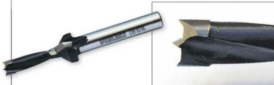
The DB1016 cutter makes a countersink and counterbore for a 5mm (No 10) screw
