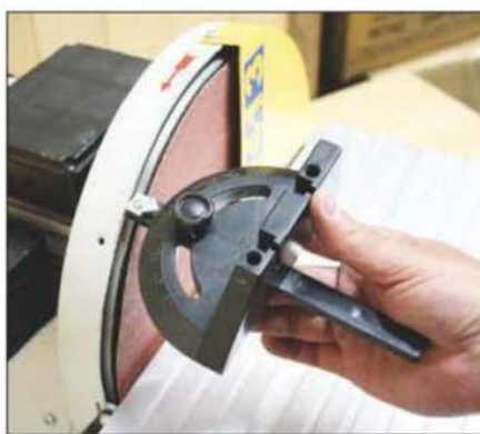
4 Accessories such as mitre fences on budget models are often of inferior quality
