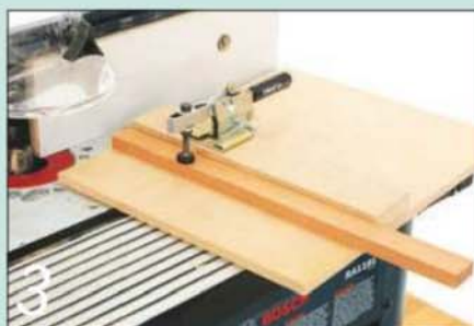
3 Make up a simple sliding jig with a toggle clamp to cut the rebates
