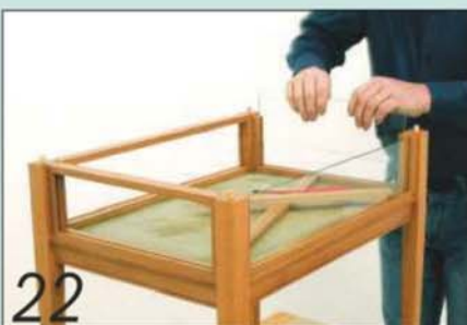
22 Unscrew the top rail of each side frame and drop in the glass pane
