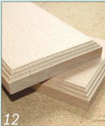
12 The top and base sections are the same size, and have an ogee edge moulding
