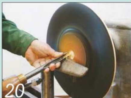
20 Turn away the hollow centre part of the platter in the normal way
