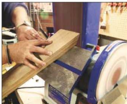
8 Some models allow the disc fence to fit to the belt for extra diversity
