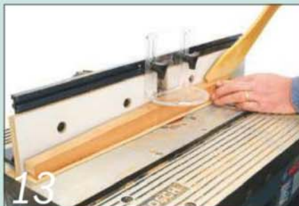
13 Move the template to the adjacent face of the leg and cut the second taper
