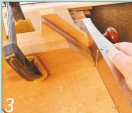
3 Mitre the linings and shoot them to length using the bird-house jig
