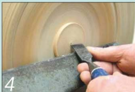
4 Pop-mark the centre of the spigot with the point of the skew
