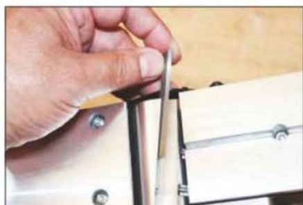
The curvature of the blade allows for the skewed fit to the block
