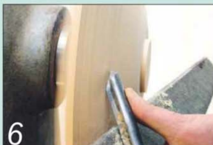
6 Shear-cut the outside of the platter to get a good surface finish
