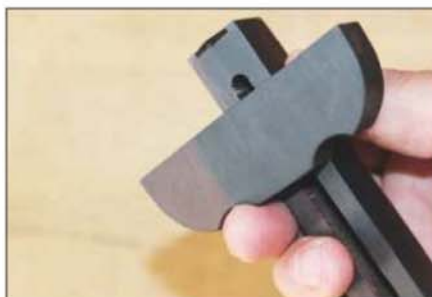
Small scallops behind the stock provide natural resting points for the fingers
