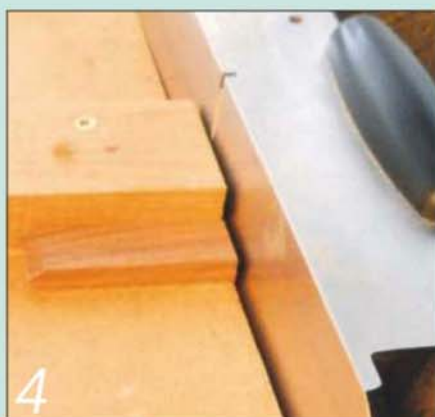
4 Cut the longer linings in half and shoot them together until the divider is a snug fit
