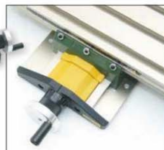
One division on the calibration scale is equal to a table travel of 0.05mm
