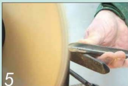
5 True up the edge of the blank using just the tip of the bowl gouge
