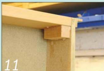
11 To reinforce the plinth I glued a couple of beech blocks to the inside corners
