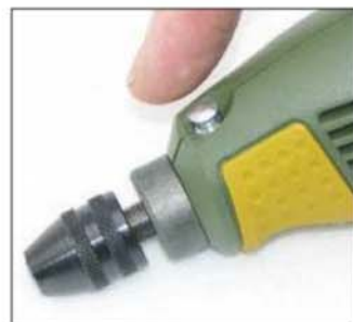
Pressing this button locks the spindle so the chuck can be tightened and released
