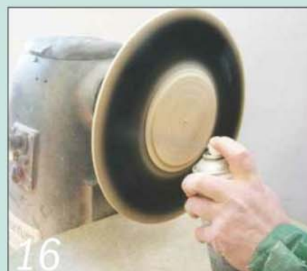
16 Set the lathe speed to 50rpm and spray the rim with ebonising lacquer
