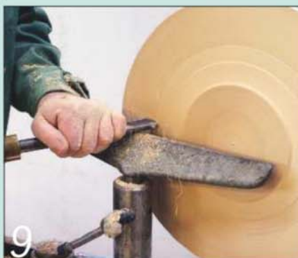
9 Turn the platter round and flatten the rim with the fingernail bowl gouge
