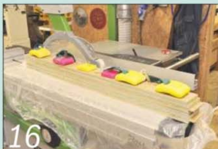
16 The cornice was made up from rub-jointed offcuts weighted down while the glue dried
