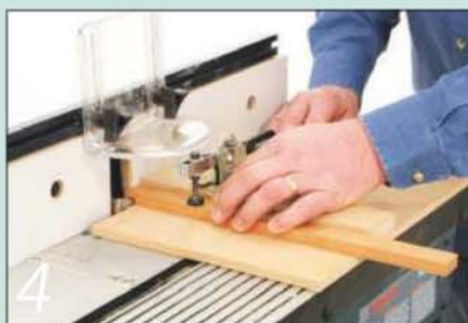
4 Adjust the projection of the straight cutter to form the rebate you want
