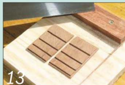
13 Then saw the piece in half to produce two perfectly-matched sides
