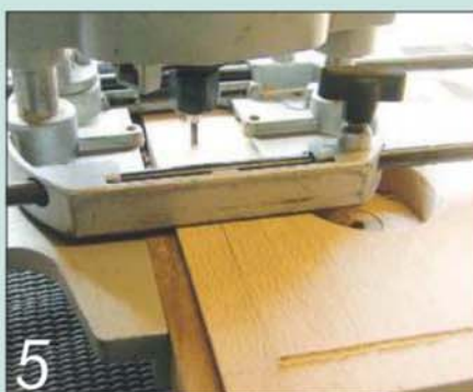
5 Rout grooves on the face and sides of the clock body to accept inlay stringing
