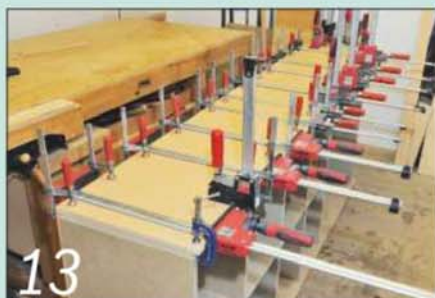
13 I needed nearly all my cramps to fix the outer skin in place to the side panels
