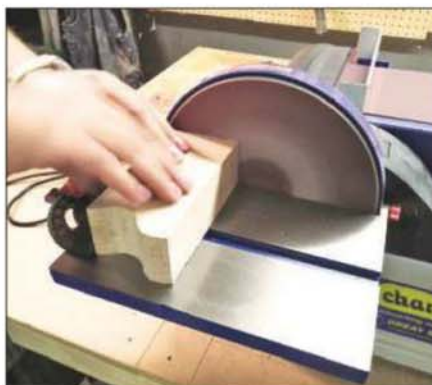
6 Safe practice means the work is normally held to the left (downward-moving) side of the disc
