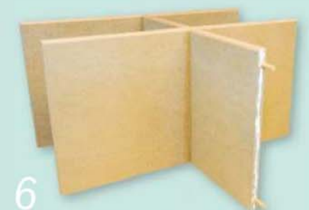
6 The dowels are long enough to connect both of the dividers through the shelf
