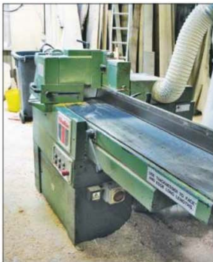
All facing and edging takes place on this rock-solid Wadkin planer...
