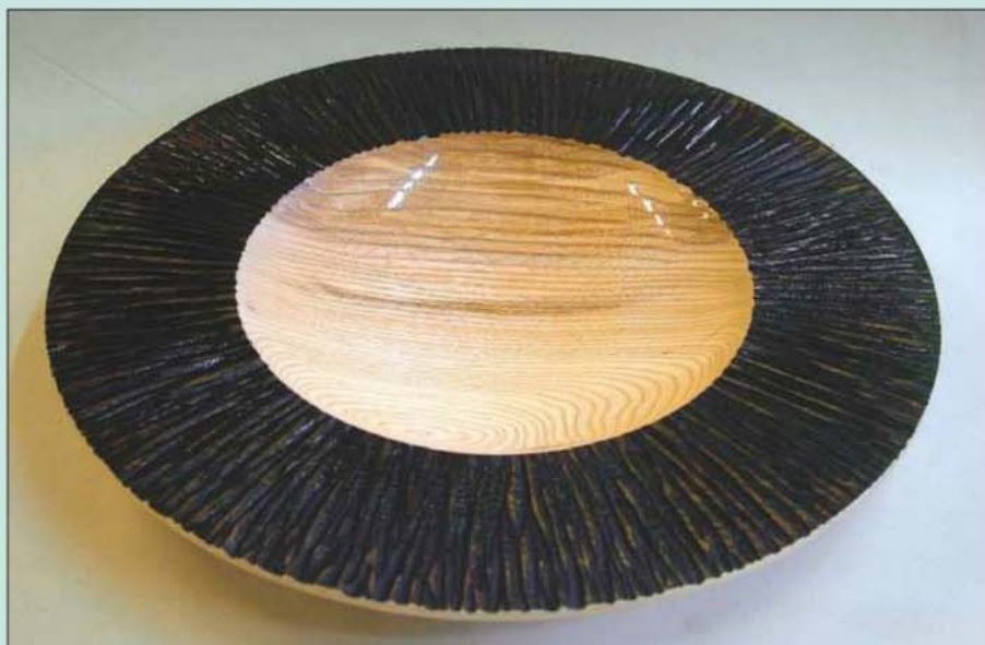
22 I finished the piece by spraying it with Chestnut acrylic gloss lacquer
