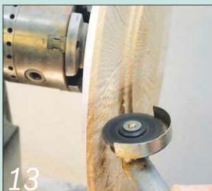
13 Continue making further radial cuts all the way round the rim of the platter
