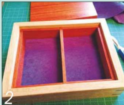
2 Another way is to fit dividers and form a recess for the lid at the same time
