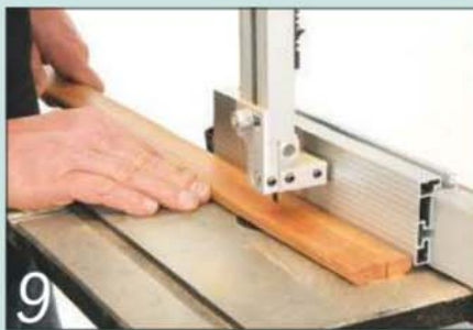
9 Round over both edges of some wide stock, then cut it down the middle on the bandsaw
