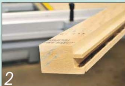
2 It's always best to machine a small moulding from larger stock and then cut it down to the size you need
