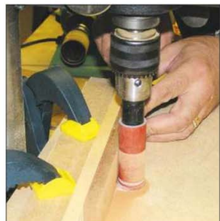
6 Cramp a back fence on a pillar drill table to carry out uniform thicknessing
