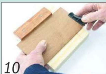
10 The Veritas miniature edge plane shown here slides along a straight edge with ease
