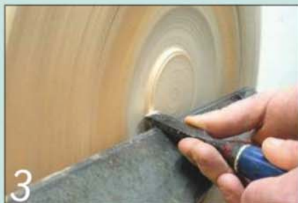
3 Then cut the chucking spigot in the centre of the base with a small skew
