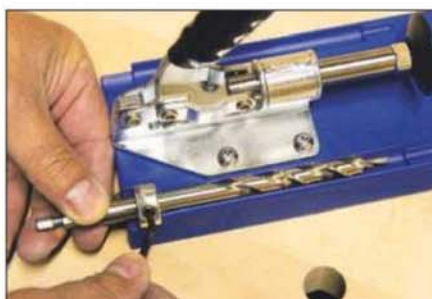
The neat drill setting guide makes it very quick to alter the screw depth
