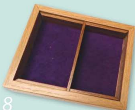
The box is now ready for the widthwise linings to be inserted
