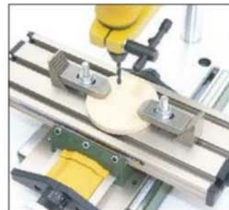
Work can also be held directly using the straps and blocks supplied
