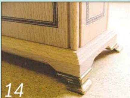
14 Screw the four feet in position and glue or screw the base to the clock body
