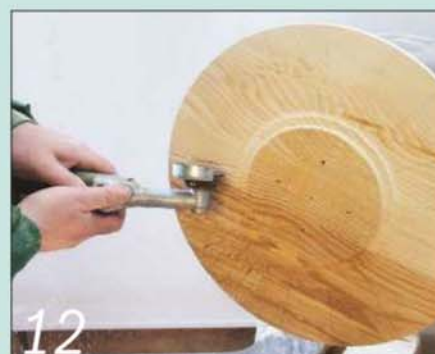
12 Make light cuts with the lathe stationary, working out towards the edge
