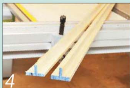
4 I made these mouldings overlong so they could be trimmed to length once they were glued in place
