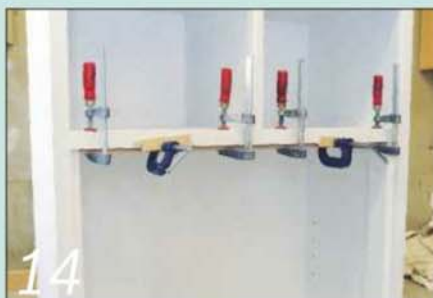
14 This strip of beech sits flush with the back edge of the frame and acts as a door stop
