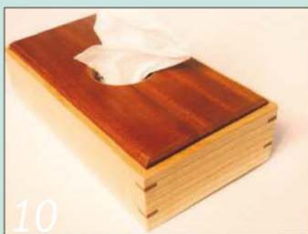
A tissue-box cover needs no separate lid. The hole is made with a Forstner bit and router
