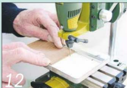
12 Slide the side panel against the fence to cut the grooves and rebates
