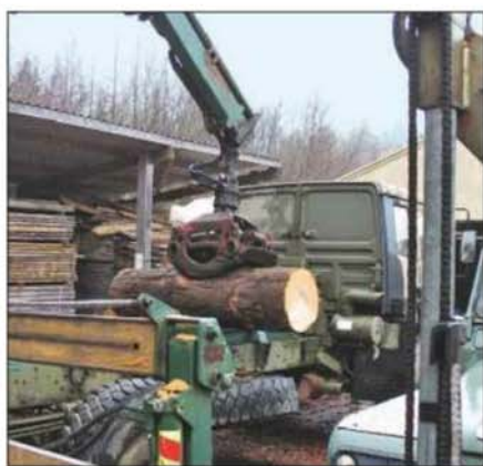
Felled timbers are hoisted into the frame of the Lucas mobile saw mill
