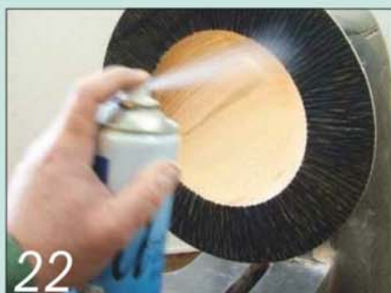
22 I finished the piece by spraying it with Chestnut acrylic gloss lacquer
