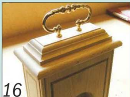
16 Fit the handle to the top blocks and attach the completed assembly to the clock body
