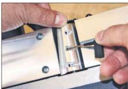
An on-board wrench is used when you need to replace the blade
