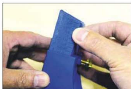
The tool post is set to suit the timber thickness read against the scale
