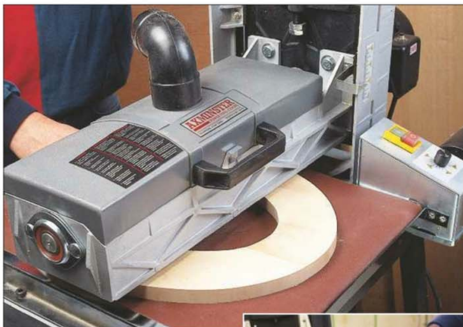
1 A drum sander works like a thicknesser on flat frames and panels
