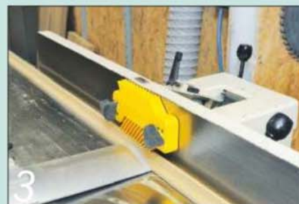
3 This Magswitch featherboard kept an even pressure on the moulding as I fed it across the planer
