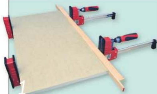
1 I used a long batten to apply even pressure when gluing the lipping strips onto the mdf panels
