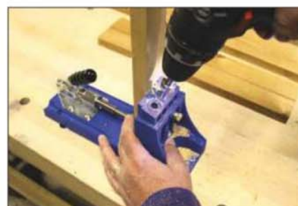
You can hold the jig by hand, or screw it to the bench or a backing board
