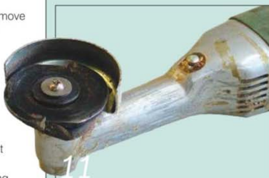
11 I tackled the carving with my mini Arbortech cutter in a Proxxon angle grinder
