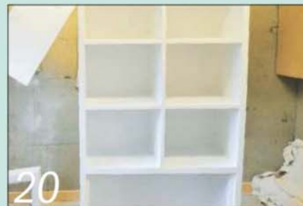
20 Spraying into open boxes is always a bit of a challenge. I reduce the spray to a fine point
