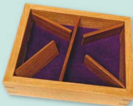
6 Loosely arrange the lengthwise linings and the divider in the box
