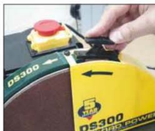
1 The right-hand side of the disc is often shrouded for safe practice
