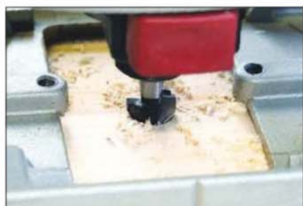
The cutter bodies have a black Teflon coating to reduce resin and chip build-up
