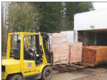
Finished blocks are manoeuvred out of the way so the last load of rough blanks can be removed from the kiln
