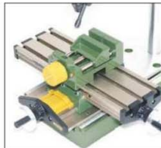
The machine vice can be fixed to the compound table to hold work
