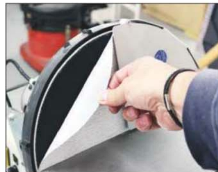
Velcro-backed disc abrasives are easy to swap as well as being long-lasting
