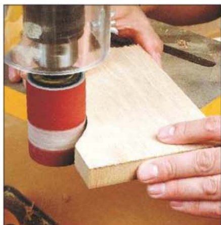
4 Alternatively the table can be moved to the side for freehand sanding
