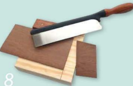
8 Cut a piece of 2.5mm thick wood to make the sides of the carcass
