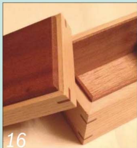
16 Mitred linings project to form a rebate that will lock the lid in position
