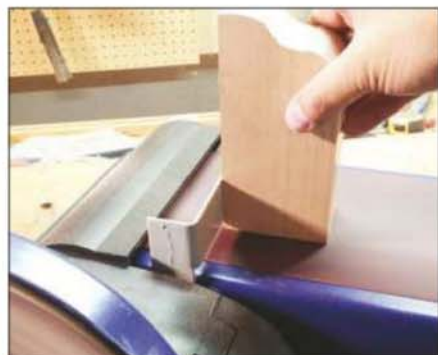
7 The belt sander normally has a simple metal backstop to restrain work safely
