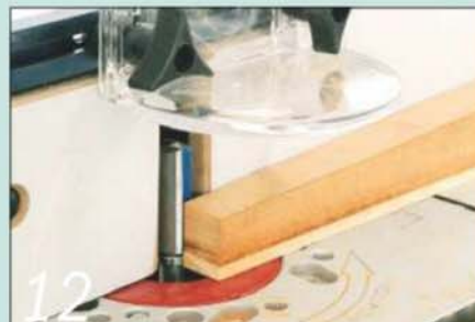
12 Stick the template to the leg and use a trimming cutter to clean it up
