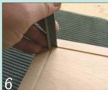
6 Square the rounded corners of the inlay grooves with a sharp corner chisel
