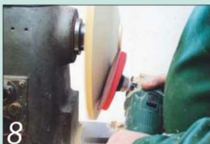
8 Sand the back of the platter down to 600 grit using a power sander
