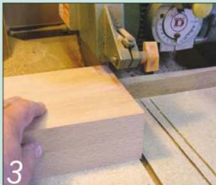
3 Cut the ends of the block square to a finished length of 250mm on the radial arm saw
