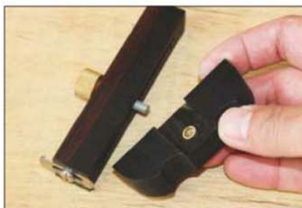
Brass inserts ensure secure connections between the parts and a long life
