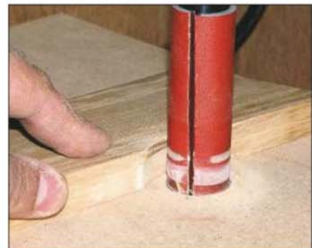
3 A pillar drill needs a table that allows the drum to pass up and down through it
