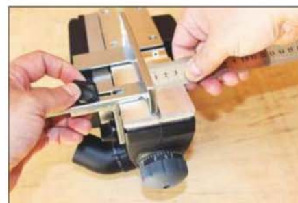
A rebating fence is supplied as standard but there's no depth stop
