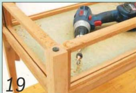
19 Drill a 10mm hole in the top of each leg and drop in a dowel marker pin
