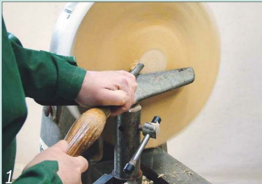
1 Start the job by using a fingernail bowl gouge to flatten off the base
