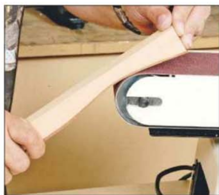
3 Internal curves can be shaped over the rounded end of the belt
