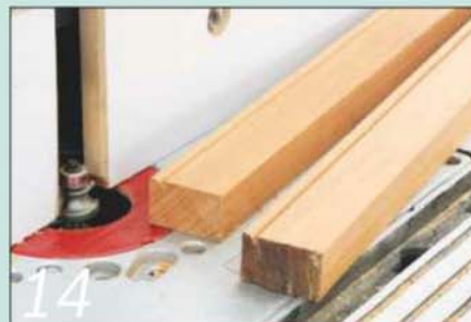
14 Cut the lower rails to length and add a decorative bead along one face
