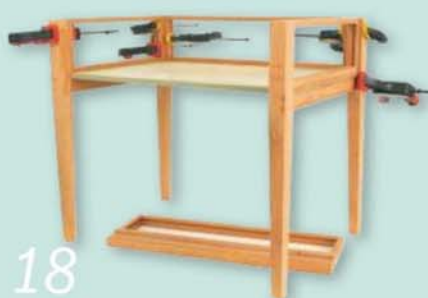
18 Build up the table by gluing and cramping the frames and legs in place
