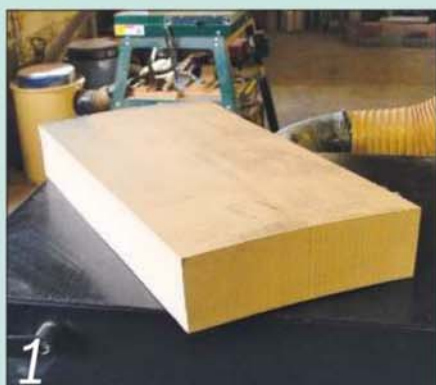
Check that the block for the body of the clock is free from obvious defects
