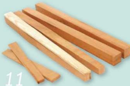
11 Use a template to mark the taper on each leg and cut it on the bandsaw
