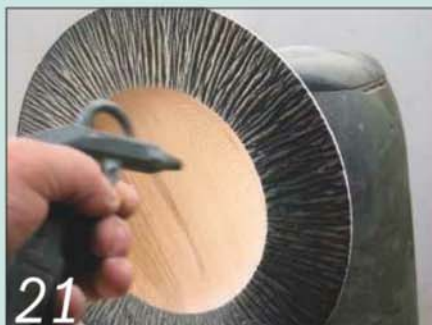
21 Remove the sanding dust with a blast of compressed air or a soft-bristled brush
