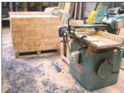
The Dominion cross-cut table is the blocks' last machining stage
