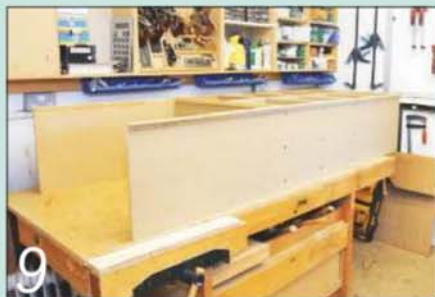
9 The two long lipped side panels can now be attached to the shelf assembly
