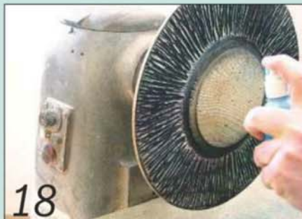
18 Spray the rim with coloured spirit-based stains in a random pattern
