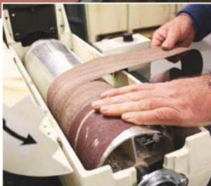
2 Abrasives are economical – a strip simply wound onto the drum
