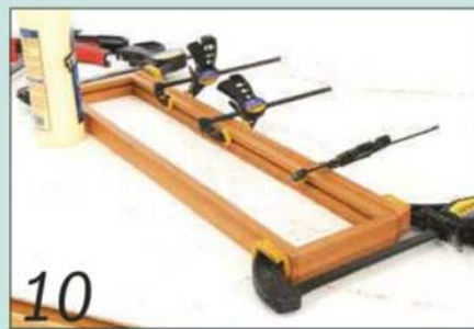
10 Glue a length of beading in place to the bottom edge of each frame
