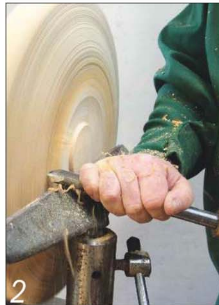
2 Shape the outside of the platter using a bevel-supported push cut
