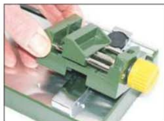
The groove on the underside fits over the drill stand's parallel fence
