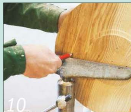
10 Make radial reference marks around the rim to act as a guide for the carving
