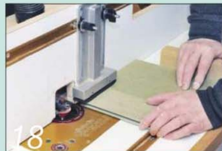
18 Keep the rail perpendicular to the fence when cutting the short rail joints for the doors
