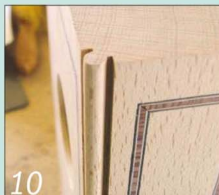
10 By taking this double cut, neat corner beads are formed on the clock body
