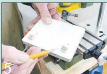
Two T-bolts supplied with the KT 70 table hold the router table in place
