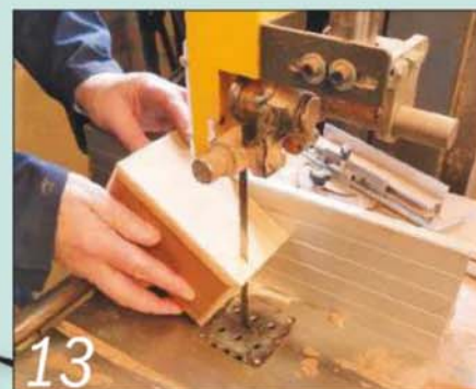
Carefully feed the complete box at a decreasing angle into the bandsaw
