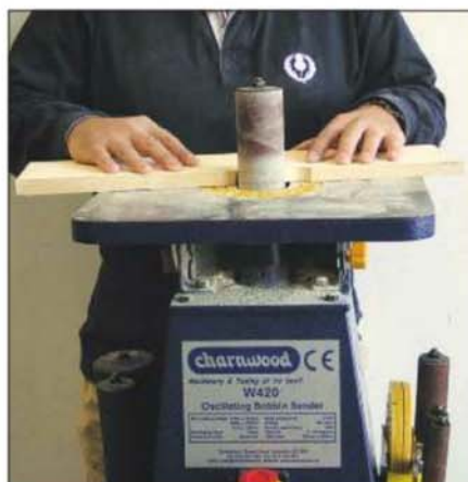
5 An oscillating sander has interchangeable bobbins and is very fast and efficient
