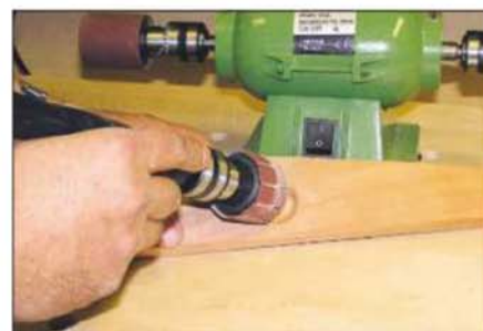
2 A flexible shaft and shaped sanding pad are useful for fine detail work
