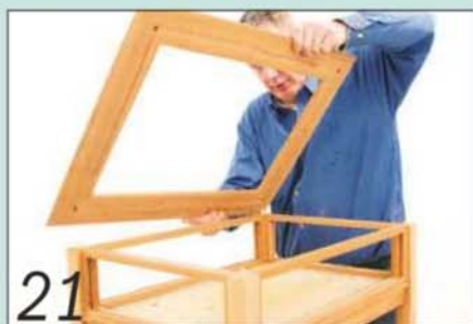
21 Drill matching holes for the dowels in the underside of the top frame and test its fit
