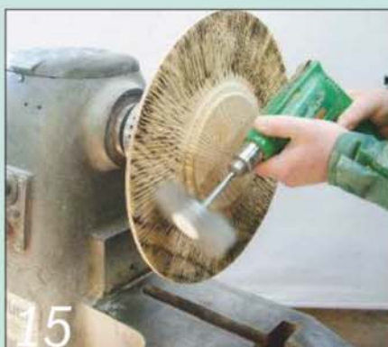
15 Then use a nylon rotary abrasive brush to clean up the whole surface
