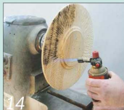
14 Use a blowtorch to burn away any stray wisps of wood left in the grooves
