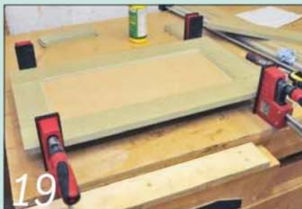
19 The doors need to be assembled and cramped up on a completely flat surface
