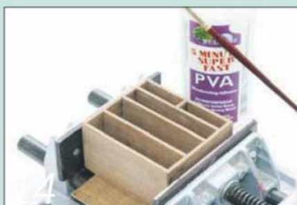
14 Cut the five horizontal pieces and the short divider to size and assemble the carcass
