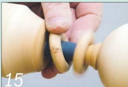
15 Attach some abrasive to the stem to sand the inside of the ring
