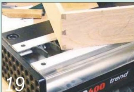
19 A dovetail jig makes quick work of jointing the four drawer sides
