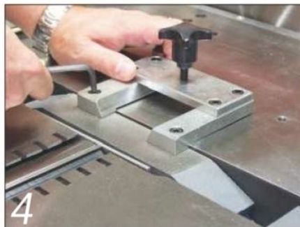
Having to bolt on brackets for fences can be a nuisance when re-setting
