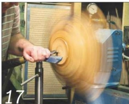
17 Even large and irregular pieces can be held securely on a vacuum chuck
