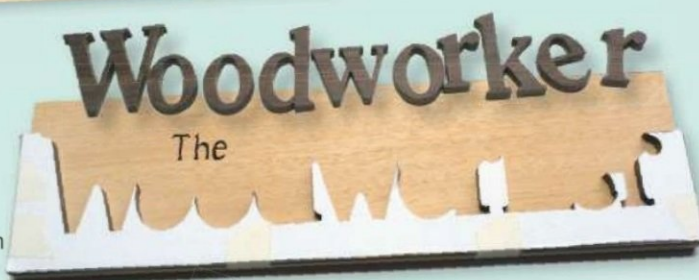
When the glue is dry, mark and trim off the top to the required height
