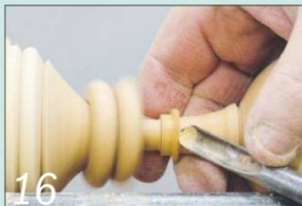
16 Support the stem with the fingers of one hand while shaping it
