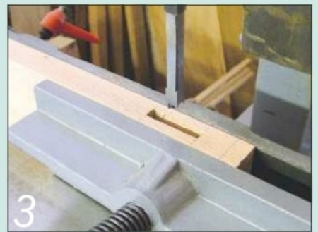
3 All the mortises in the long frame rails were cut using a hollow chisel mortiser
