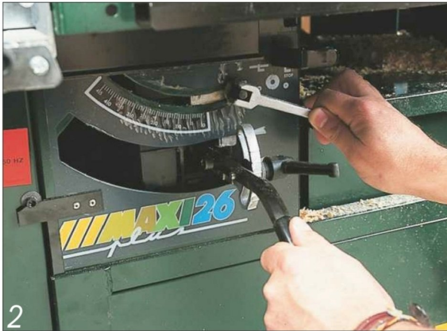
Budget machines have quirky adjustments such as a lift-up saw blade
