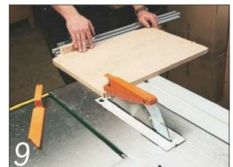
9 The sliding carriage on the table saw can be a small on-board type...
