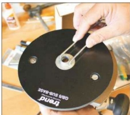
You may need a sub-base to accept the elliptical guide bush
