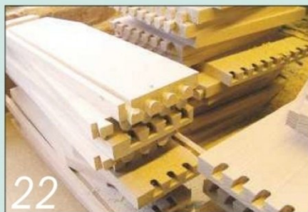
22 With all the drawer components joined, I rounded over the tops of the backs...
