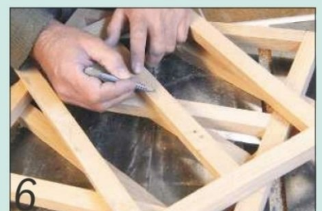
6 Make a trial assembly of the panel frames and mark each face side
