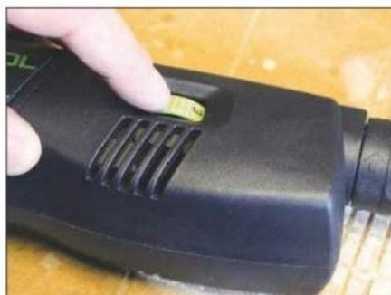
The variable speed dial has an auto setting that adjusts speed under load
