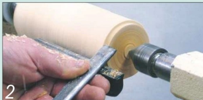
2 Cut a chucking spigot on the end that will become the goblet base
