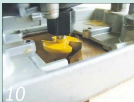
To finish the frames, I ran a small chamfer all round their inside edges with my router
