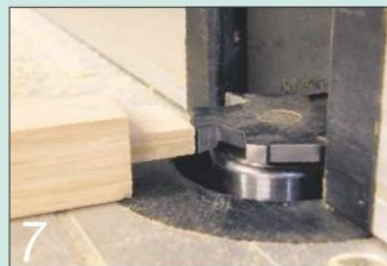
7 Align the cutter with the tenon and machine the 6mm wide grooves
