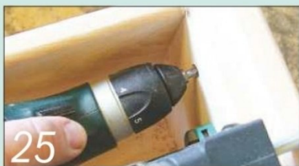
25 The false fronts concealing the drawer runners were screwed on from inside the boxes
