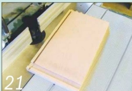
21 ...and a slotting cutter in my router table to make the grooves for the bases
