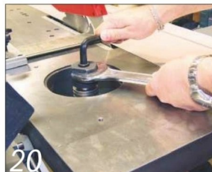
Spindle swaps vary, but a two tool set-up as shown here is commonplace
