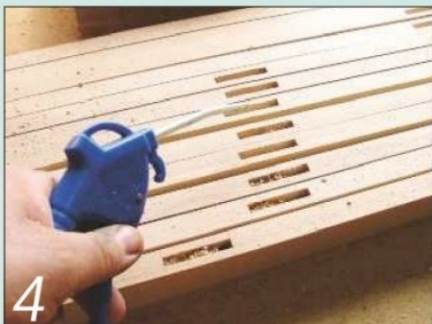
4 I used a gun connected to my air line to clear all the debris from the mortise holes
