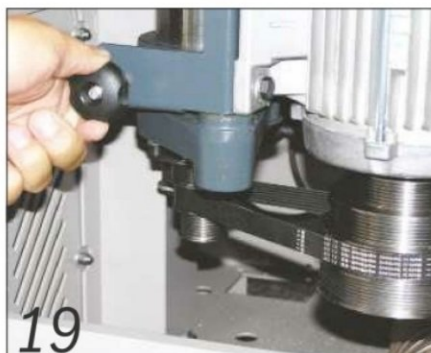
The spindle motor may need a manual belt swap for speed changes; all have replaceable cutters
