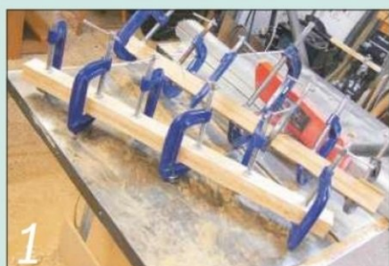
1 Laminate narrow boards if required to make up the width of the legs
