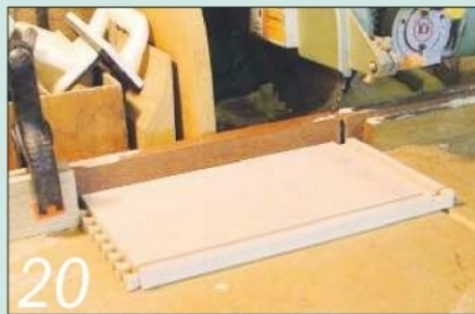
20 I used my radial arm saw to cut housings in the drawer sides for the backs...
