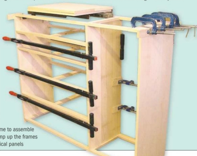
I secured all the glued mortise-and-tenon joints using a headless pinner
