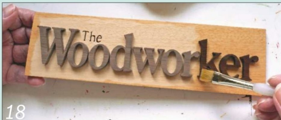
Apply two coats of a clear liquid polish, buffing it up between coats
