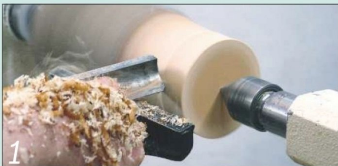
1 Mount the blank between centres and rough it down to a cylinder
