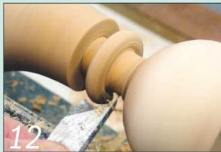
12 Swing the handle to the right to cut the right-hand side of the ring
