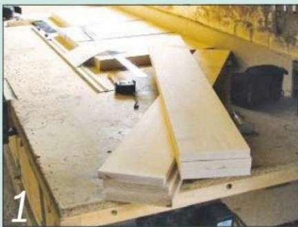
1 I started the job by cutting the carcass components from thickened stock
