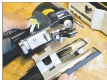
Slide this lever and the base easily disengages to allow other bases to be fitted
