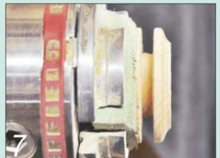
7 After finishing turning the detail, I sanded it to a fine finish before parting it to thickness
