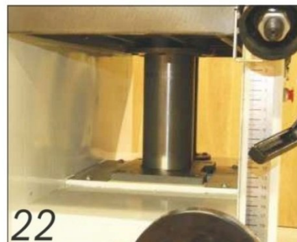
A central ram to set the thickening dimension is normally seen as the better option
