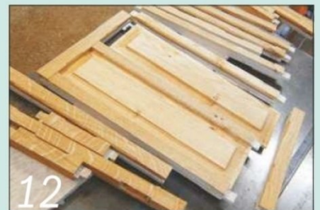
Apply a finish to all the components before gluing the parts together
