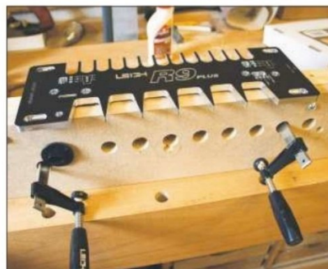
The right-hand clamp is moved along to suit the width of the workpiece
