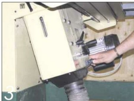
You may have to lift the whole saw-head assembly to make bevel cuts
