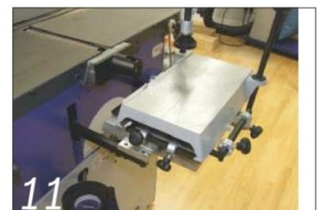
11 A horizontal mortising table is normally an optional accessory on a combi...
