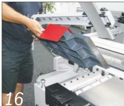
...or it may use a lift-up bed system. This model operates inboard
