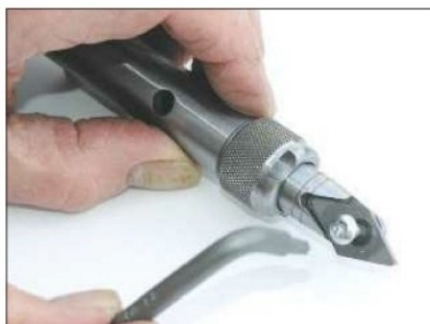
The cutter is attached securely to the head with a T20 Torx screw
