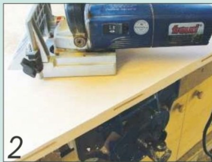
2 The boards for the top, sides and divider were all assembled with biscuit joints
