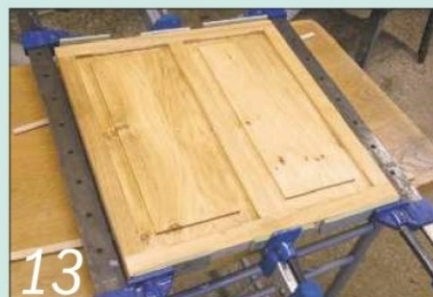
Assemble and cramp up each panel, and check that it's square
