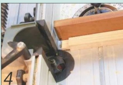
4 Use the sliding mitre fence on the router table to cut all the tenons
