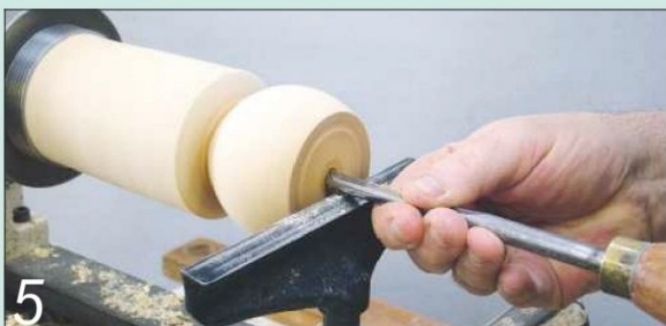
5 Use the same gouge held horizontally to start drilling the hole...
