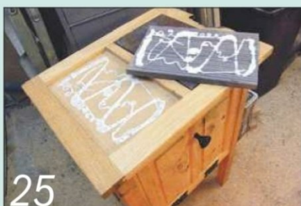
25 Use quick-setting adhesive to fix the two slate panels to the MDF base board
