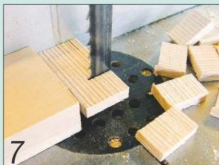
I removed the waste from the haunched tenons with a single bandsaw cut
