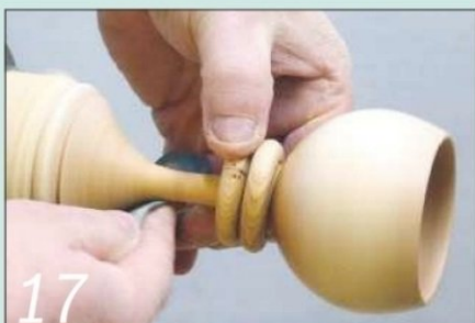
17 Hold the rings out of the way while you finish sanding the stem
