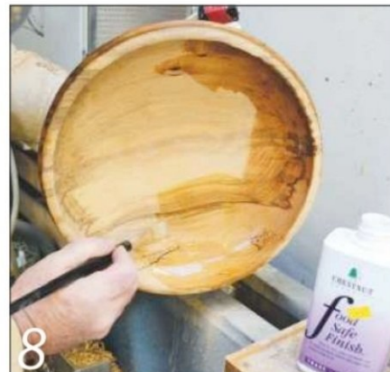
Leave a generous coat of finishing oil to soak in before removing the excess with a dry cloth
