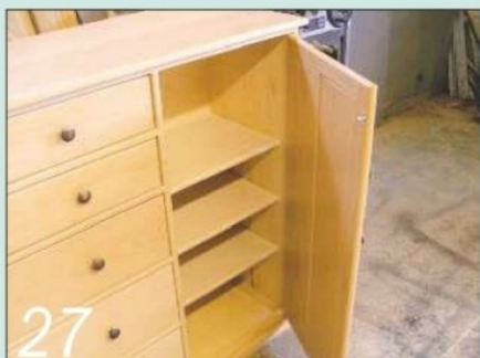
27 Finally, three shelves were fitted in the cupboard on shelf support pegs
