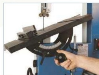
Single handed table adjustment
