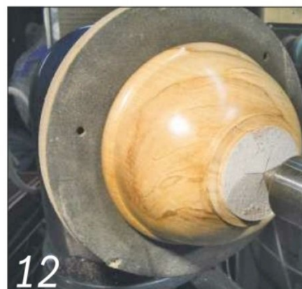
Friction between the bowl and the mat is enough to drive the bowl round
