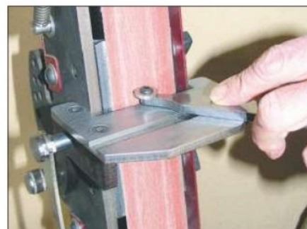
The HSS cutters can be sharpened; a special jig is available to hold the cutter securely
