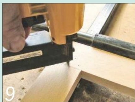
I secured all the glued mortise-and-tenon joints using a headless pinner
