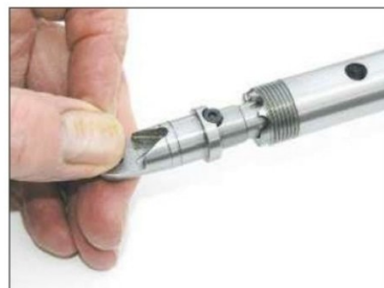
The head can be rotated in the shaft to offer one of three cutting positions
