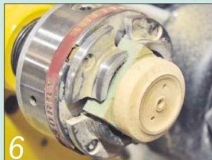
6 I turned the beech blank to size and added the front detail before drilling the mounting holes
