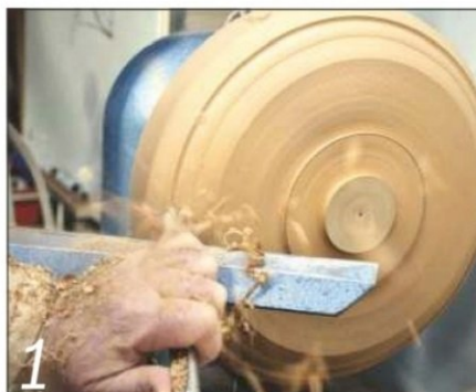
1 Shape the underside first, cutting outwards from the centre towards the rim
