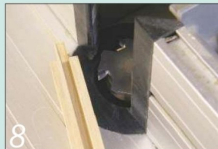
8 Make sure you cut the grooves on the correct face of each component
