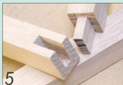
5 Precision cutting should result in a well-fitting mortise and tenon
