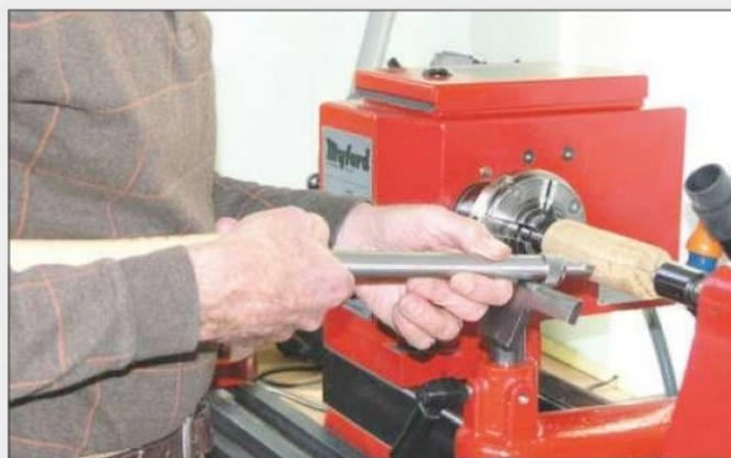
The long ash handle can be tucked under the armpit for greater control
