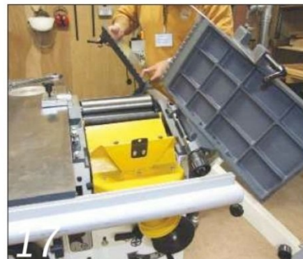
This gullwing model needs more working room and also limits access
