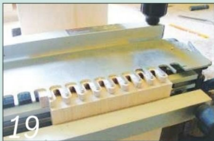
19 My Bosch dovetail jig made light work of cutting dovetails in the drawer sides
