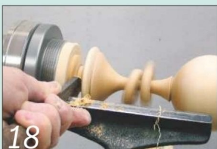
18 Part off the goblet with a parting tool, undercutting the base slightly
