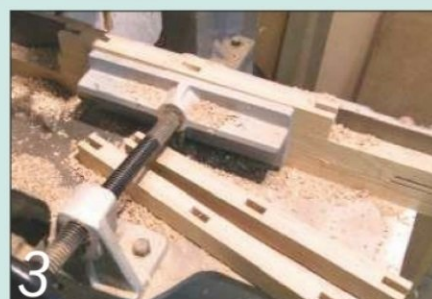
3 A mortising machine makes light work of the many joints to be cut
