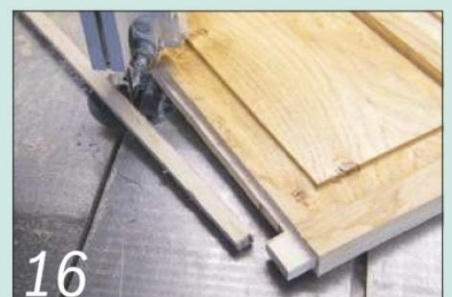
Saw away the excess between the tenons to leave a 6mm tongue
