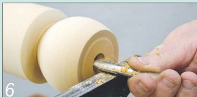
6 ...and then start the hollowing out, pivoting the tool on the toolrest
