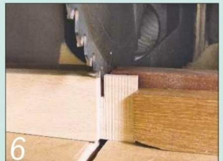
6 I created a haunch on each tenon by cutting down one third of the tenon width
