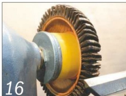
16 A vacuum chuck allows the tailstock to be removed once the work has been centred
