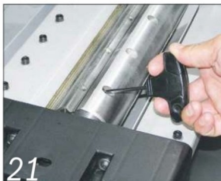
Many planer blocks have multiple knives that need traditional set up methods
