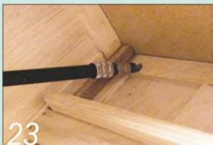
23 Attach the top with screws driven up at an angle through the side rails
