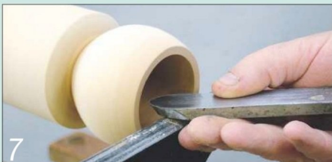
7 Use a round-nosed scraper to clean up the inside surface of the bowl
