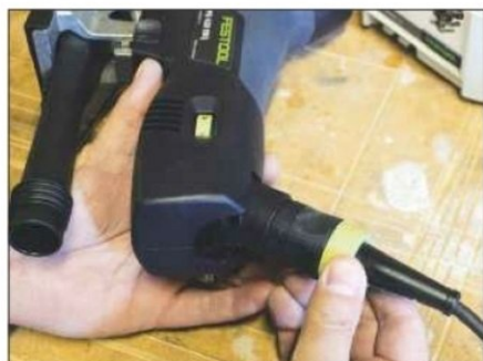
The plug-in flex fits into a pivoting socket to keep the saw free of restrictions
