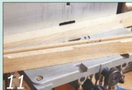
Take care when cutting the chamfers to stop them at the pencil marks
