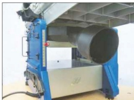
The debris outlet is positioned below the table when surface planing
