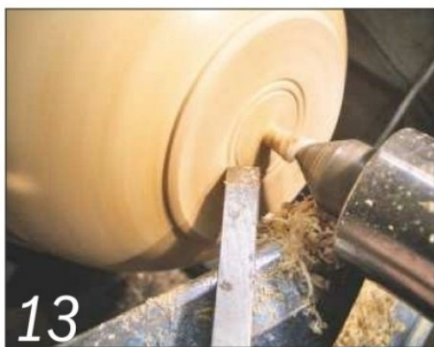
13 Leave a small central portion in place so you can maintain the tailstock pressure
