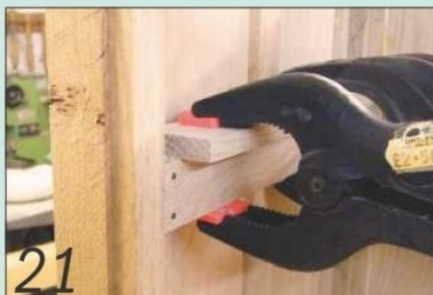
21 The drawer runner is clamped to support strips that are simply pinned in place
