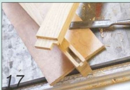
17 Haunched mortises and tenons make strong joints on the top frame
