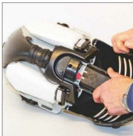
The battery slides into its compartment at the back of the unit
