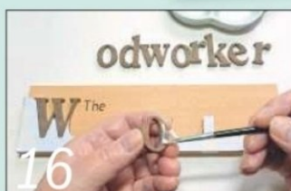
16 Brush glue onto each letter in turn and place it on the template
