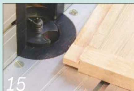
Cut a rebate to form a tongue along the edge of the side and rear panels
