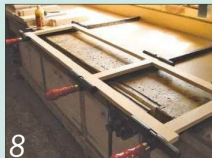
Each of the six frames was then glued, assembled and cramped up square
