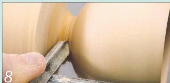
8 Now refine the bowl and the top of the stem with the spindle gouge
