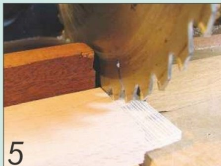
5 The tenons were all cut using a repetitive stop set up on the radial arm saw
