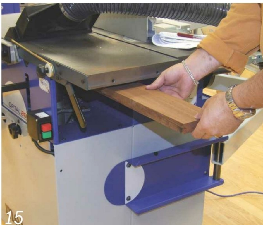
15 The thickness function can be a fixed-bed option, as on this machine...
