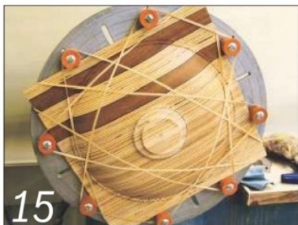
15 Make sure the bowl is held securely by wrapping rubber bands round it
