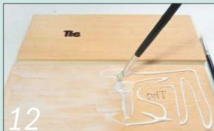
12 Apply an even coat of PVA glue to the underside of the middle section
