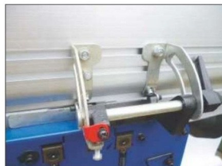
The sturdy fence support allows it to tilt to a maximum of 45°
