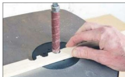
The smallest spindle sanding sleeve is ideal for sanding tight curves
