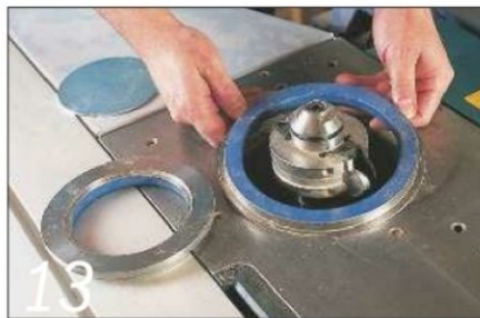
13 The spindle well on this model has clever reversible rings for curved work
