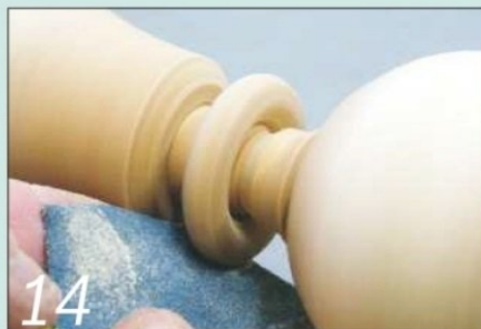
14 Sand as much of the ring as you can before separating it from the stem
