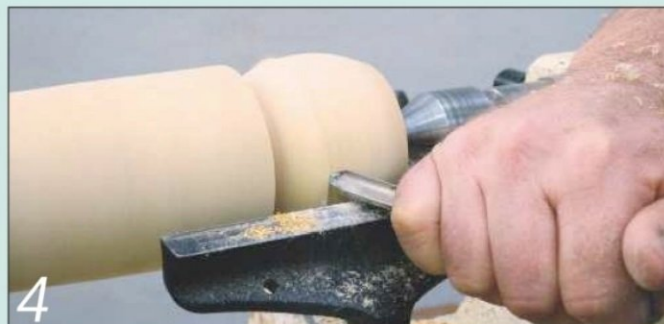
4 Start shaping the bowl part of the goblet with a small spindle gouge
