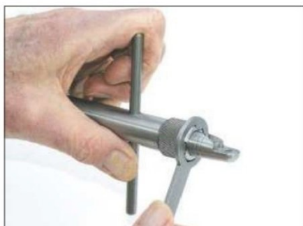
A special spanner locks the nose nut. The tommy bar stops the shaft from rotating
