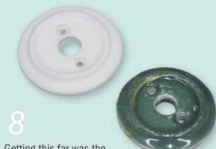
8 Getting this far was the easy bit; the ceramic backplate, which I had to match for colour, is on the right
