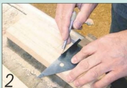
2 Use a square to mark out the locations of all the mortises on the legs
