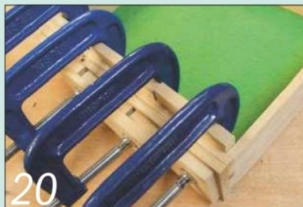
20 The oversize false drawer front is glued and clamped to the drawer box
