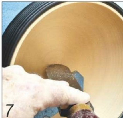
A large scraper will remove any surface ridges and bumps left behind by the gouge
