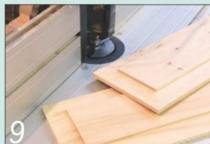
9 Remember to reduce the speed of the router for a cutter of this diameter
