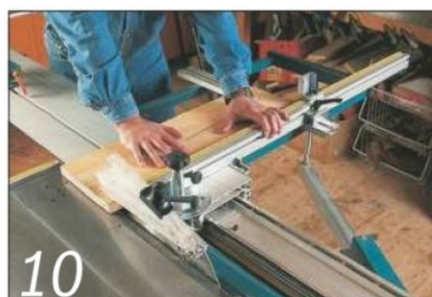
10 ...or a bigger outrigger, ideal for sheet conversion as well as trimming
