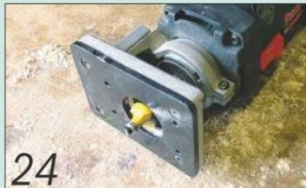
24 I softened all the square drawer edges with a roundover cutter in my laminate trimmer
