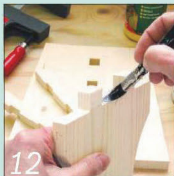
Apply PVA glue to the components with a small brush to ensure even coverage
