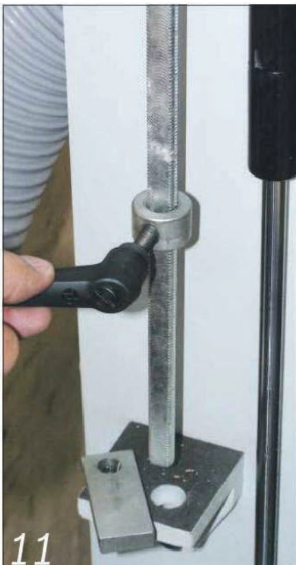
11 ...as are similar settings for cutting haunches and blind mortises
