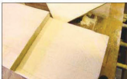
The finish from the saw is clean enough to assemble for joinery work without sanding
