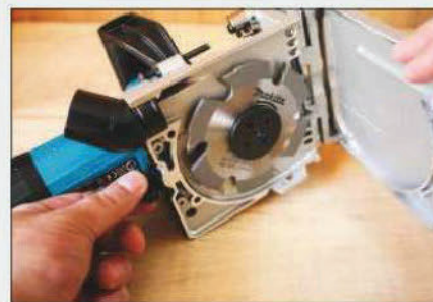
Cutter access is simple, and a pin spanner is supplied for changing blades
