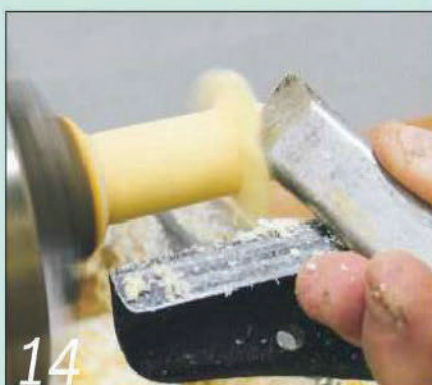
14 Use the small point of the skew chisel to make the first row of petals
