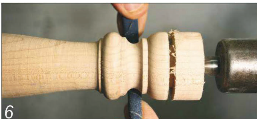
6 Roll the abrasive into a tube to sand small coves
