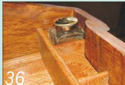
36 I fitted two glass inkwells in the front corners to hide the column fixing screws
