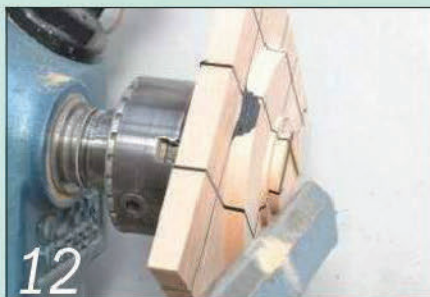
12 Mount the blank in the chuck and set out the dimensions of the piece
