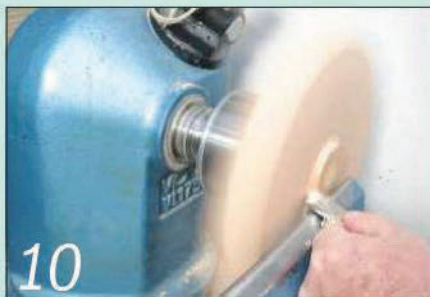
10 Use a skew chisel to form a dovetail shape that will fit your chuck jaws
