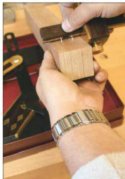
The long pins give loads of roll room for mortises and scratch marking
