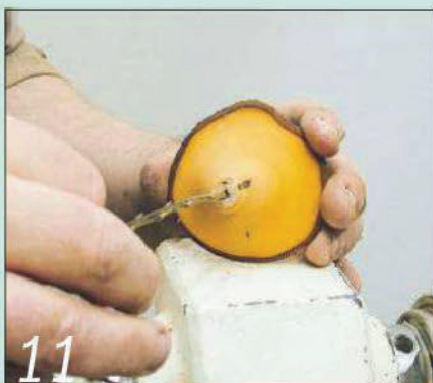
11 Drill a small stopped hole in the turned detail you created in step 7 and glue in the stem
