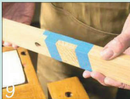
Mark out the tee-halving joint near the middle of the main frame
