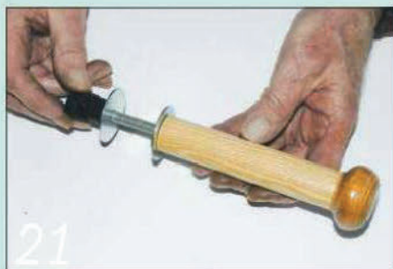
21 Glue the bolt into the handle, fit the end cap and add the washers and knob
