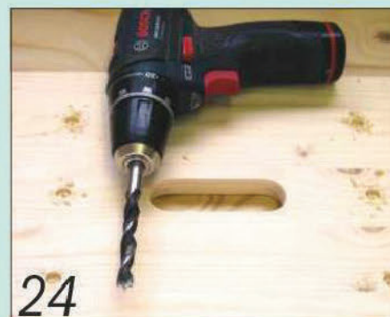
24 Mark the screw positions on the line and drill shallow plug-sized holes
