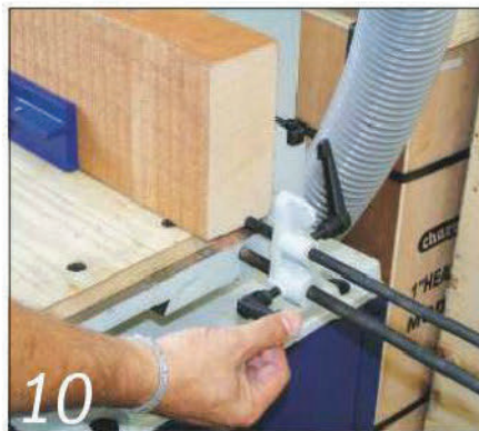
10 Stops for setting mortise positions and lengths are a useful option...
