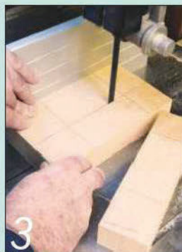
3 Cut the first set of strips on the bandsaw to create four strips of unequal width
