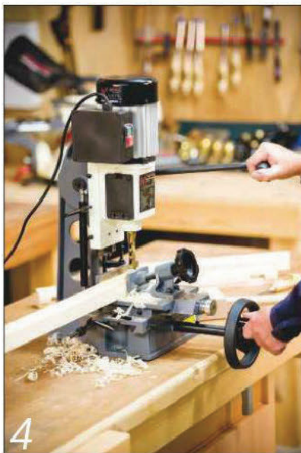
The standard hollow-chisel mortiser is the one we're all more familiar with
