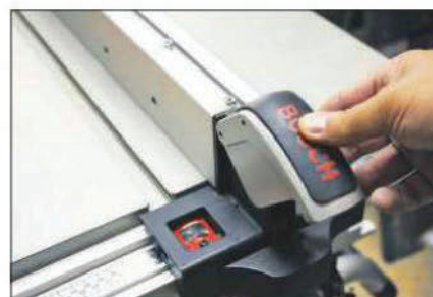
The paddle lock on the fence is positive and locks rigidly in place
