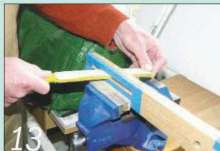
Clean up the inner faces of the slot with abrasive paper stuck to a former
