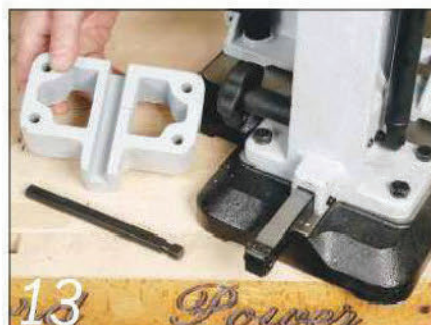
13 Some benchtop models have riser blocks to allow deeper stock to be cut
