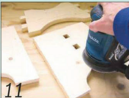
Clean up all base components by hand or with a sander before gluing anything up
