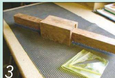
3 Timber for front column needed packing out ready for turning to shape
