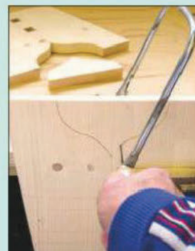
Sketch out a shape for the leg cutouts and cut them with a coping saw
