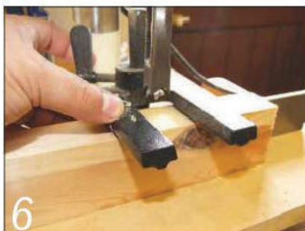
The simplest hollow-chisel mortisers have a basic fork to hold down the work
