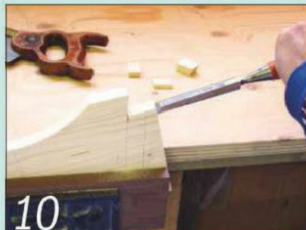
Cut the tenons on the ends of the connecting rail with a saw and then a sharp chisel
