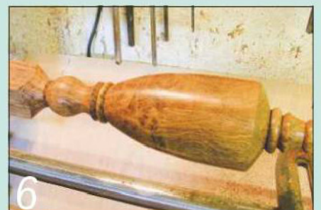
6 Burnishing the column with the shavings gave it a stunning surface sheen
