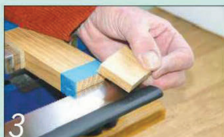
3 Make the second cut with the grain to complete the joint
