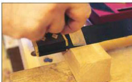
The wide blade of the try square sits rock solid on the stock
