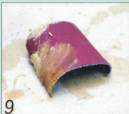
9 Wet wood quickly clogs the abrasive, but a process I call wet sanding is the answer
