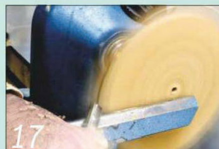
17 Try to maintain an even depth of cut as you work towards the centre
