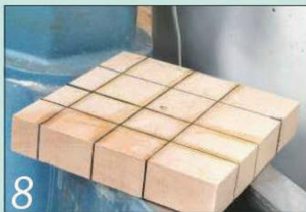
8 Find the blank's centre and drill an 8mm diameter hole to take the screw chuck
