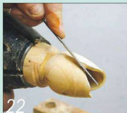
22 Refine the detail of the petal carving with small needle files
