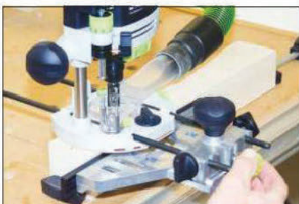
The side fence can be adjusted to 0.1 mm using this green adjuster knob
