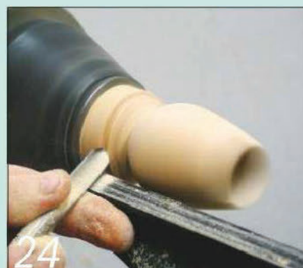
24 Finish shaping the outside with a stem mount as before; then part it off
