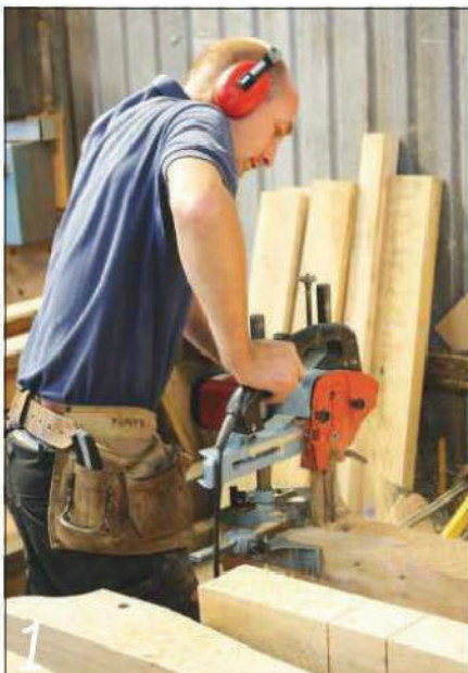
A portable chain mortiser is the ideal choice for cutting big mortises and tenons
