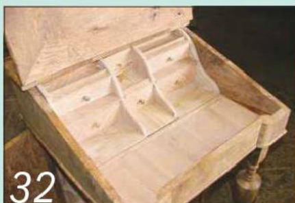
32 This set of five small storage drawers fits snugly inside the top box...
