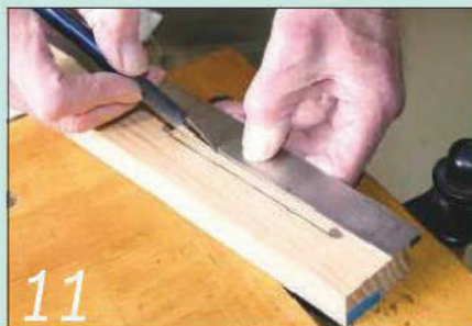
Mark the position of the frame slot and drill a hole at each end
