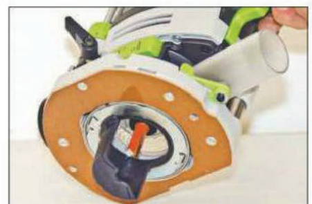
The chip deflector can be rotated as required to facilitate the collection of chippings
