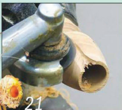
21 Carve the petal shapes; I used a mini Arbortech cutter in my small angle grinder
