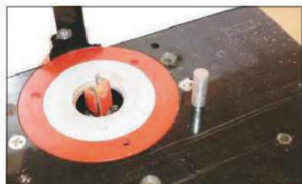
The lead-in pin can be fitted in either of two locations to suit the work
