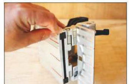
These two rubber buttons help prevent slippage as the cutter engages
