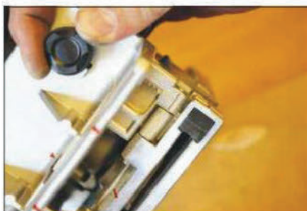
Adjustment of the slide-on shoe is with a single rack and pinion
