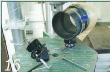
16 You can remove the cramp and rely on the magnet to hold the support on the table
