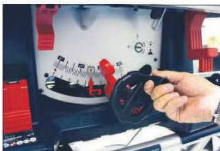
Only one central wheel is needed for making blade adjustments
