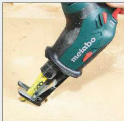
The saw can also plunge-cut using the saw's foot as shown here
