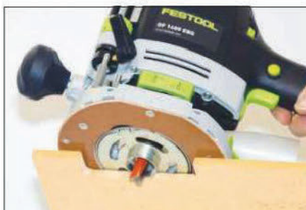
The 30mm copying ring clips in and is released without the need for tools
