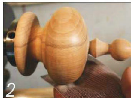
2 600-grit Abranet is particularly good at removing scratches from dense-grained wood
