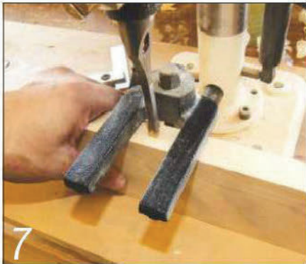
7 However, you have to hold the work against the fence and move it along by hand
