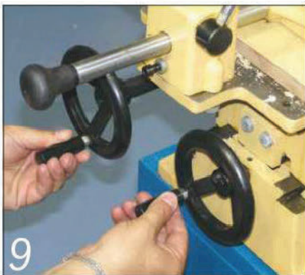
9 Wheel adjusters are essential if you want to work quickly and efficiently
