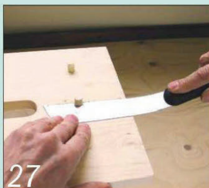
27 When the glue has set, trim all the plugs flush with a flexible saw...
