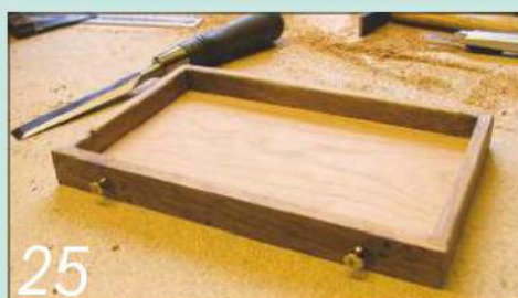
This small secret drawer was designed to be concealed within the foot plate
