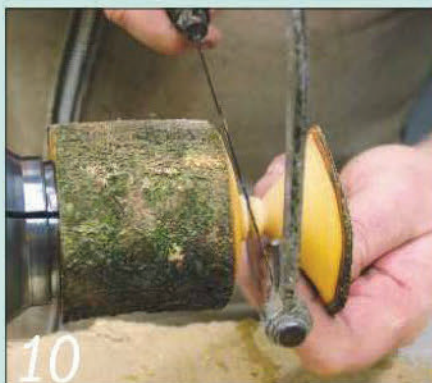
10 Stop the lathe and cut the flower off with a spindle gouge or a fine-toothed saw
