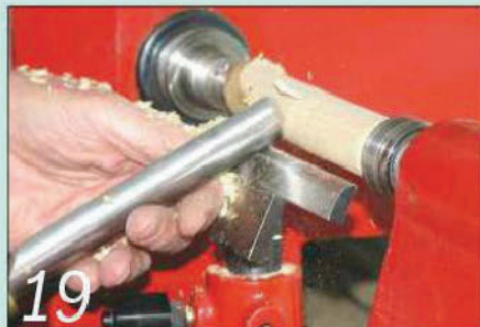
19 Mount the blank for the tensioning handle and turn it to round
