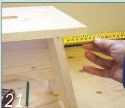
21 Centre the seat on the base and check that the overhang is the same at each end
