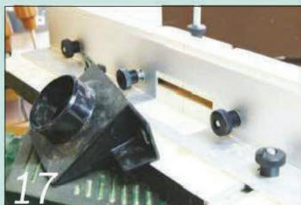
17 The table outlet is held in place by the fence locking screws, so is easily removed
