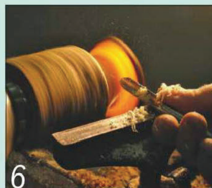
6 A bright work light shining through the wood helps you to judge an even wall thickness
