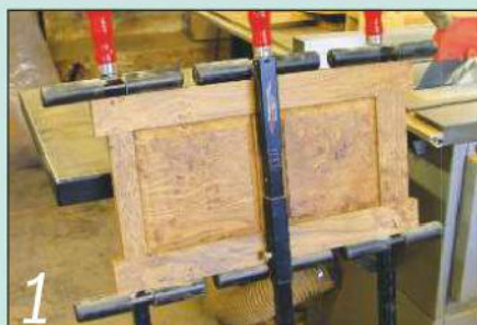
1 I assembled and cramped up the two-panelled door for the cupboard...
