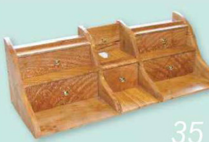
35 The complete unit features two slim pen trays on the top and a false centre panel
