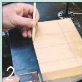
2 Mark out sixteen irregularly-shaped squares on the blank with a pencil
