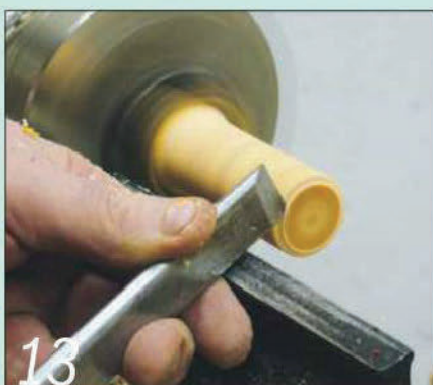
13 Square the end of the branch off sliver by sliver with a fine slicing cut
