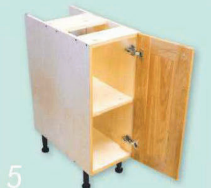
5 We made the carcasses for the base units from 18mm birch ply which was edge-banded with 2mm oak strip to match the cabinet doors
