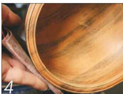
4 Keep your fingers trailing in the direction of the rotation to prevent snagging
