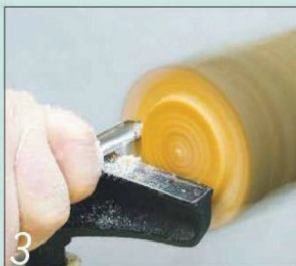
3 This cut is made slightly against the grain, but it helps to keep the bark on
