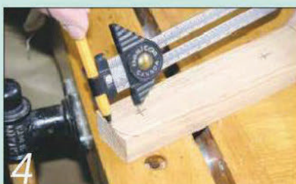
4 Draw a curve on one end of each upright with a pencil and compass
