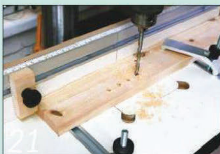
21 Its fence, cramps and stops make jobs such as repetition drilling simple
