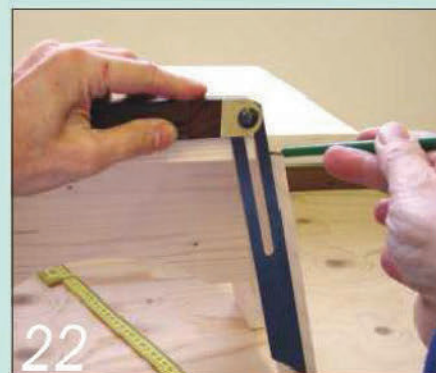
22 Use the sliding bevel to transfer the centre line of the legs to the seat
