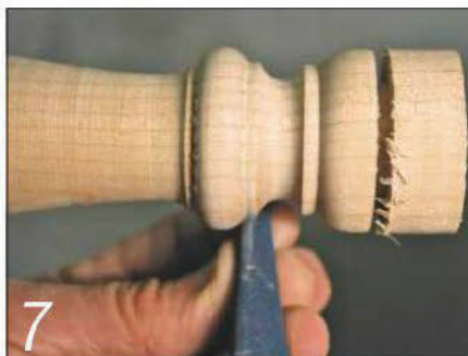
7 Fold the abrasive round a small scrap of wood to sand the fillets cleanly
