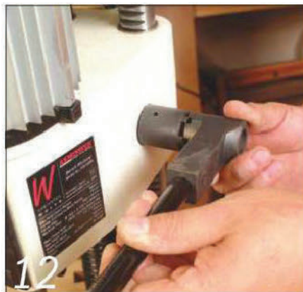
12 Adjustable plunge arms allow you to select the best leverage position
