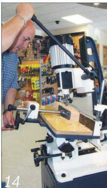
14 This particular machine has a tilting table for cutting compound mortises
