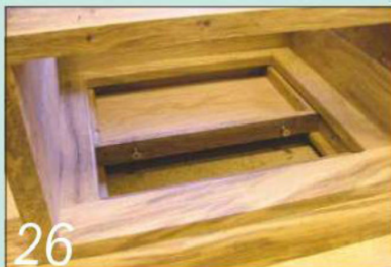
26 Removing the bottom drawer reveals where the secret drawer is fitted
