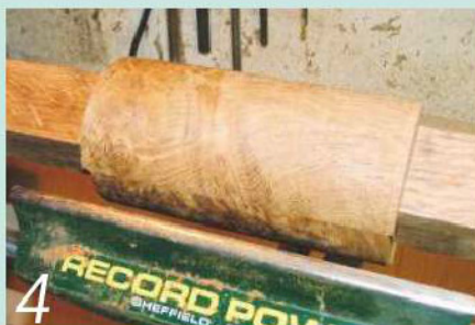
4 I started by turning the larger centre section of the column to a cylinder...
