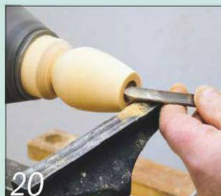
20 Then drill a hole down the centre of the flower and start to hollow it out
