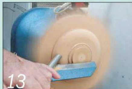
13 Shape the underside of the bowl in a curve using a 13mm bowl gouge
