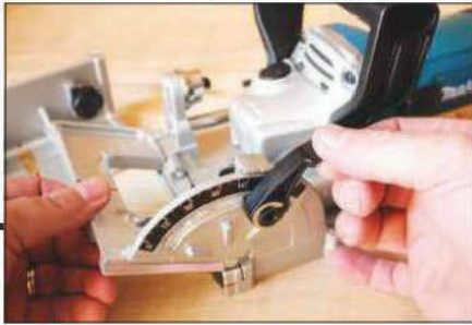
The tilting fence locks positively with a single lever
