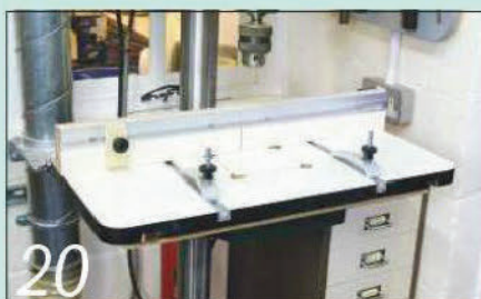
20 The new drill press table is easy to position on the false table below
