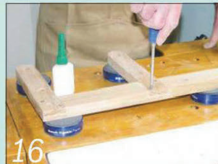
Glue and screw the uprights to the main frame via the clearance holes you drilled earlier
