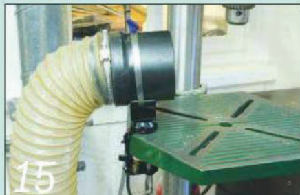
15 The support cramp can be attached to the table and will hold the hose horizontally or vertically
