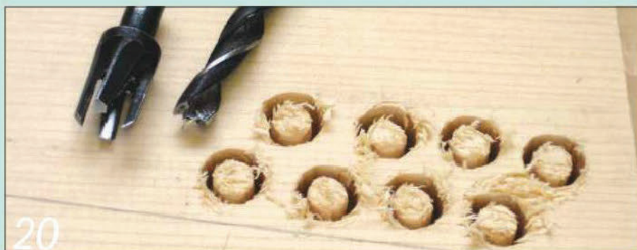
20 Use a dedicated plug cutter to produce a batch of cross-grained plugs
