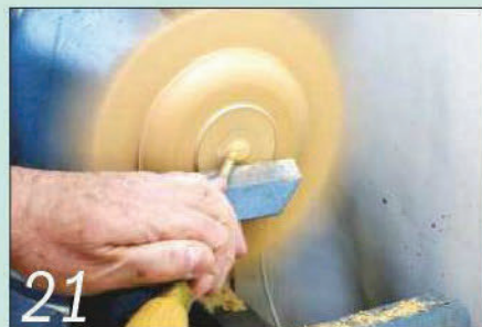
21 Remove the spigot and tidy the foot, leaving its centre slightly concave
