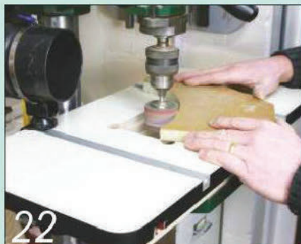
22 The removable centre insert allows quick conversion to a bobbin sander
