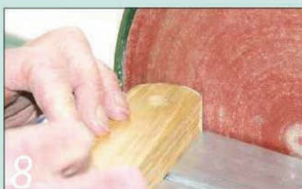
8 Shape the curve and then sand it smooth using a disc sander
