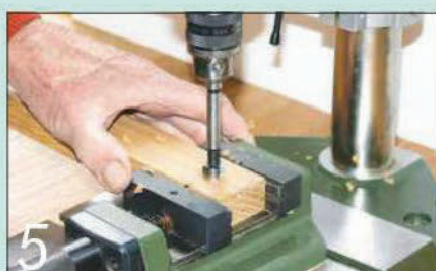
5 Mark the dowel positions and part-drill a 16mm hole at each point
