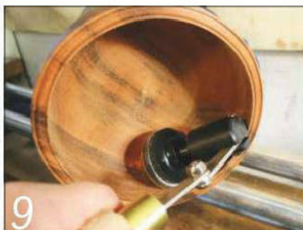
9 Use an angled sanding disc on an arbor. The rotating workpiece drives the head round
