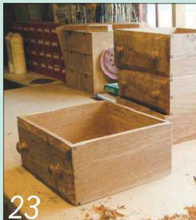
The drawer boxes needed a light planing to ensure a good fit in the carcass
