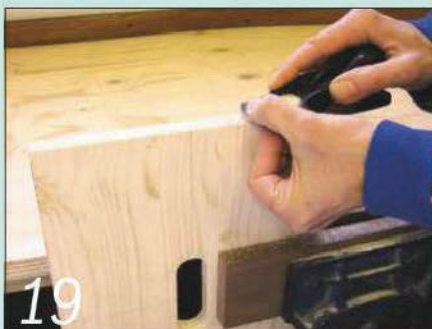
19 Use a sharp block plane to trim the sawn endgrain at each end of the seat
