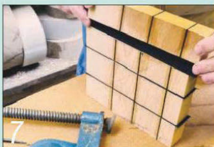
7 Glue and cramp up the strips, making sure that the veneer lines all align
