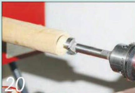
20 Drill a 20mm diameter hole 20mm deep in the end, then continue the hole 8mm in diameter
