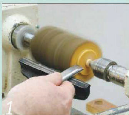
1 Use the tip of the skew chisel to cut a spigot on one end to fit your chuck
