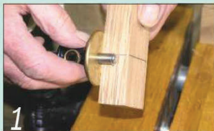
1 Mark out a simple halving joint on one end of each upright
