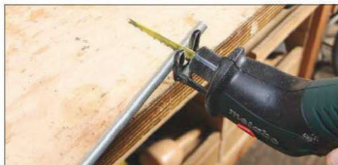
A range of different blades is available for cutting metal and plastics
