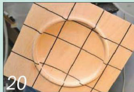
20 Sand the interior of the bowl down to 400 grit, then tackle the corners
