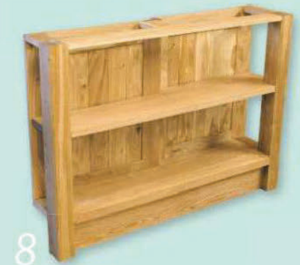
8 We had to step the back of the bookcase unit to take up the difference in the cabinet lengths, but the discrepancy is hardly noticeable
