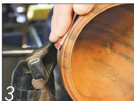
3 Position a vacuum extractor nozzle close to the dust source
