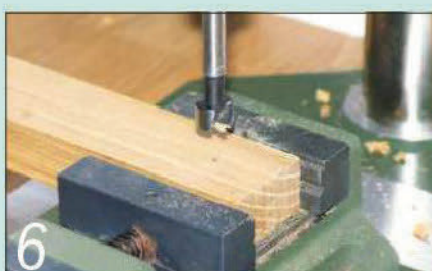
6 Turn the wood over, locate the drill in the pierced hole and finish it off
