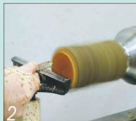
2 Remount the blank and square off the end with a spindle gouge, taking care with the entry cut
