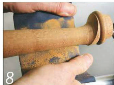
8 Stretch a sheet of abrasive beneath the work to sand tapered spindles
