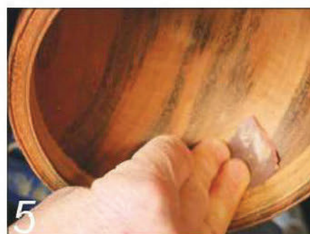
5 Use a smaller square of abrasive to sand the inside curve of the bowl
