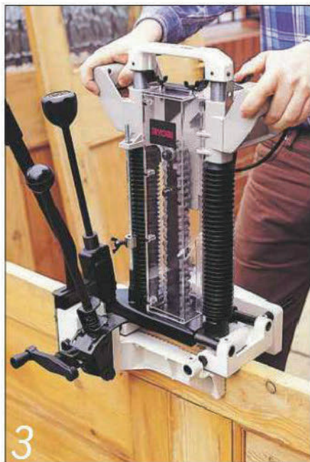
The machine is invaluable for cutting lock mortises on doors and the like
