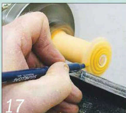
17 Gently brush the rotating petals with a felt-tipped pen to add some colour
