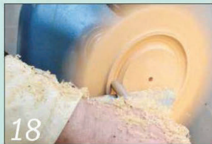
18 Hollow out the centre of the bowl, aiming to leave a raised rim about 8mm wide
