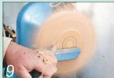
9 Cut in from the corners towards the centre to leave a spigot 5mm deep
