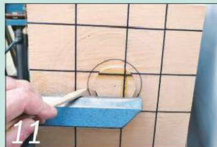
11 Mark out the bowl's foot, which is usually significantly bigger than the spigot
