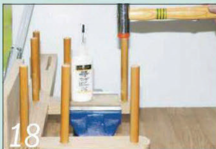
18 Apply glue to the end of each dowel and tap it into its fixing hole
