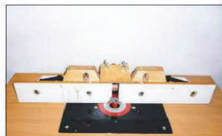
The insert plate must fit flush with the table surface, as mine does
