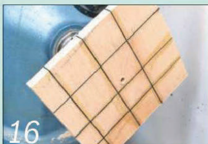
16 Reverse the piece in the chuck jaws and check that it turns true
