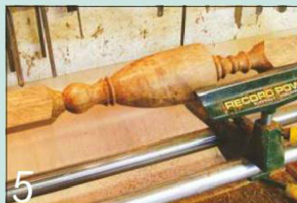
5 ...and then turned it and the rest of the column to the required profile
