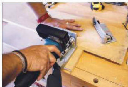
Registration made directly from the base is very accurate
