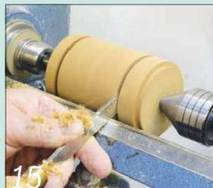
15 Use a narrow parting tool to cut in on the waste side of the marks
