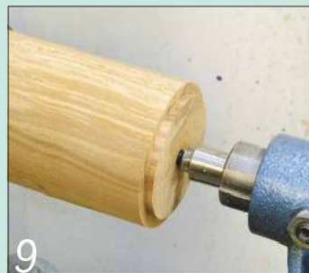
9 I drilled as far as I could reach, then finished the job by drilling from the other end
