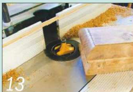
13 I then used a large ovolo cutter in the router to round over its top edges
