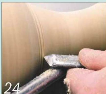
24 ...but cutting a series of beads over the joint area helps to disguise it
