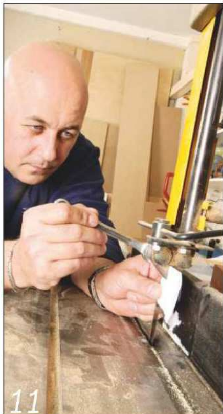
11 Nip block guides up just enough to engage without the blade twisting
