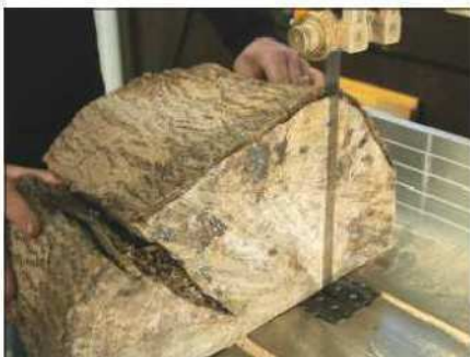
The blade can cope with wood of almost any thickness, as shown here
