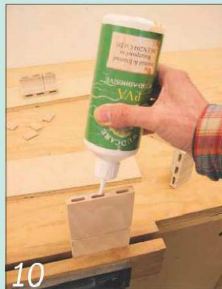
10 With all the case components prepared, it's time for the glue-up to begin
