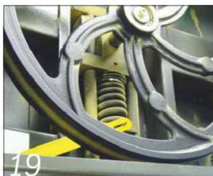
The tensioning spring is also often beefed up considerably on better saws
