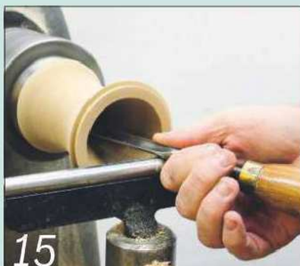
15 Hollow out the neck to about two thirds of its length with a spindle gouge
