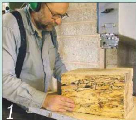
1 Square up your blank and take the corners off on the bandsaw
