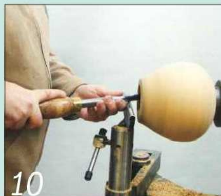
10 This upright stance is far more comfortable than a stooping one
