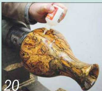
20 ...apply some thinned sanding sealer. You can run thin superglue into very soft areas
