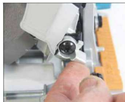
You can release this revolving stopper to get an extra 5° of tilt
