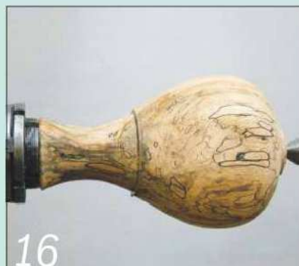
16 Glue the two pieces together, making sure that the grain lines up
