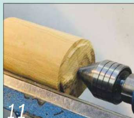
11 Remount the piece between centres located in the ends of the hole
