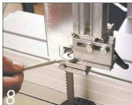
Setting the side guides can be a fiddly job to carry out on some bandsaws
