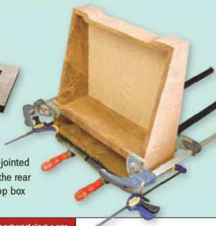
13 I then used a large ovolo cutter in the router to round over its top edges
