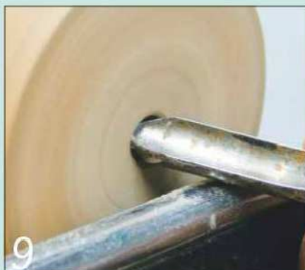
9 Start hollowing by pivoting the tool sideways on the tool rest
