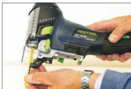
The new blade is inserted into the holder and then twisted to secure it
