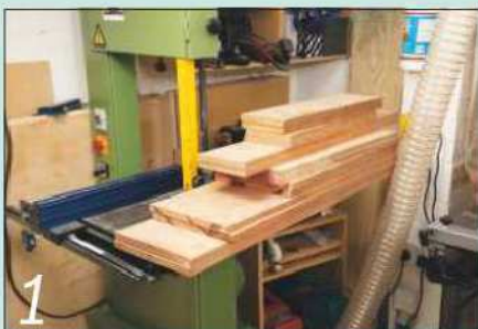
1 My first job was to rip the 50mm thick cherry stock down in width on the bandsaw
