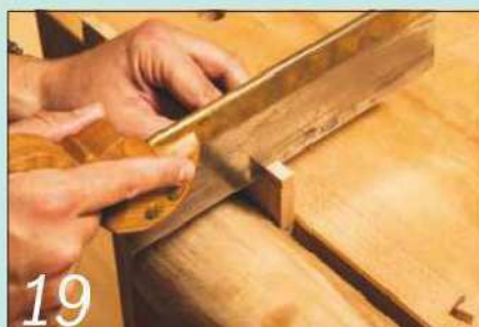
19 Use a sharp tenon saw to cut away the stopped part of the joint
