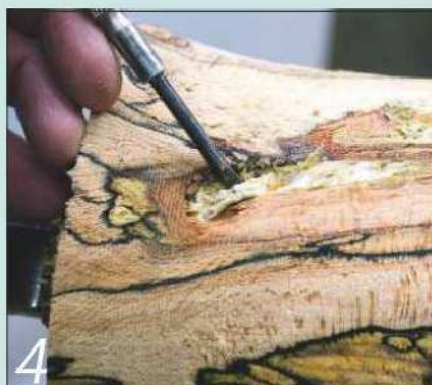
4 This soft area must be turned away, causing a change of design
