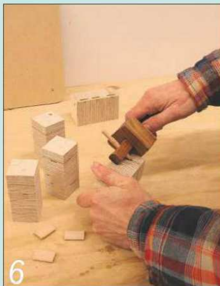
6 Marking out the domino positions on the corner blocks. A test block is in the background
