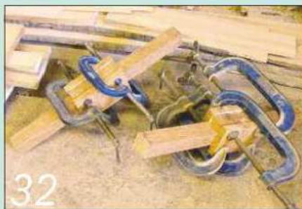
32 I fattened up the blanks for the turned columns by gluing and cramping offcuts to their centres
