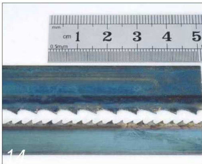
14 Skip-tooth blades (top) are missing every other teeth, creating a wider gullet that clears waste more quickly than a standard set
