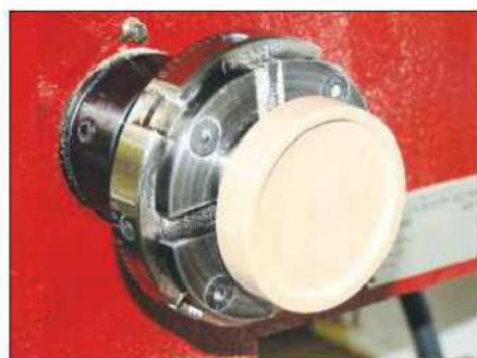
7 Sand the wood by hand on the lathe to get a really smooth finish
