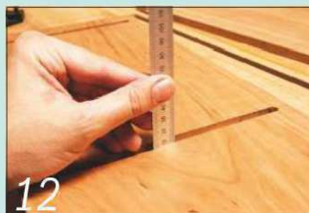
Rout the housing and check the depth; I allow an extra 1mm for the glue
