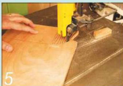
...since the waste pieces break away one by one as the bandsaw blade makes the cut
