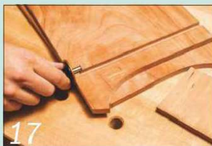
17 Use a marking gauge to measure the inset of the stopped housings...
