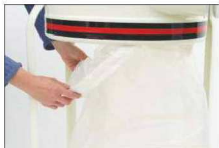
The waste bag is held in place with a bendy plastic ring inside the housing
