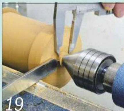
19 Turn the 15mm diameter end stubs and use callipers to get the size correct
