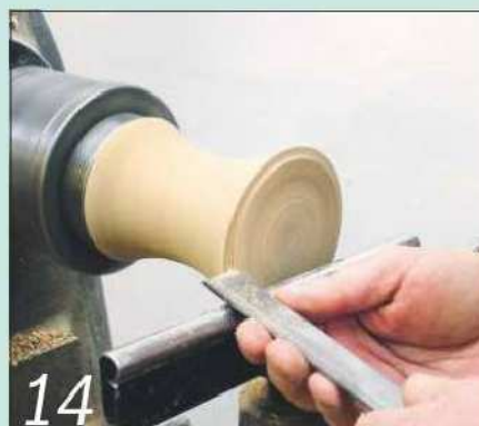
14 Remount the neck section and cut a matching spigot on its end
