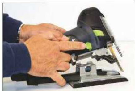
The saw is released from the soleplate by sliding this lever forward
