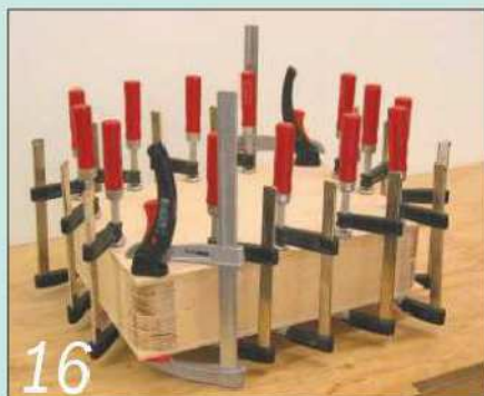
16 The top and the bottom plywood panels can now be glued on and cramped securely
