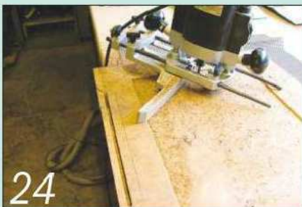
24 ...and removed the straight centre section between them with a series of router cuts
