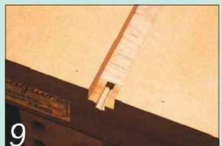
9 All you need to make this simple housing jig are a few board offcuts and some cramps
