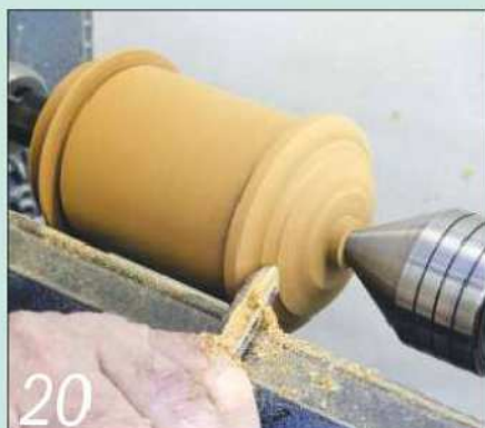
20 Use a small bowl gouge or a spindle gouge to shape the domed end
