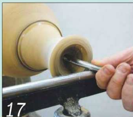
17 Reverse the piece and complete the hollowing of the vase's neck
