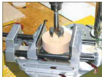
3 Drill a 5mm deep hole with a saw-toothed Forstner bit in the centre of each blank, at a diameter to suit the chuck jaws you're going to use
