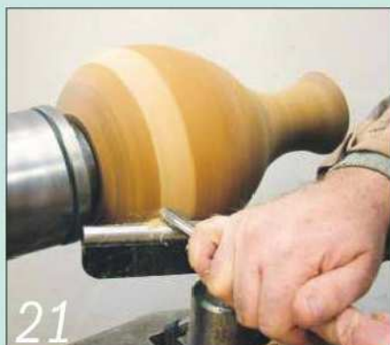
21 When the sealer is dry, take a fine finishing cut with a very sharp gouge
