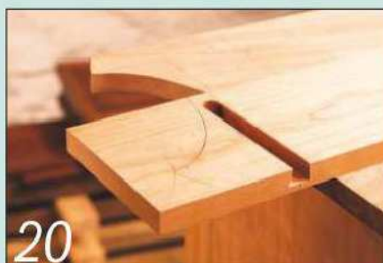
20 Transfer the curved profile from the bookshelf sides to the sides of the smaller unit
