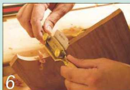
I used a sharp spokeshave to clean up the straight sections on each unit side...
