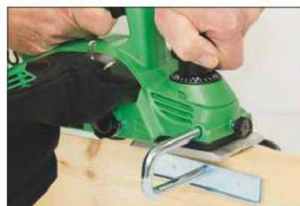
The edge guide is a useful extra support during normal surface planing
