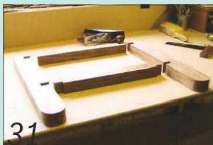
31 After checking the fit of the joints, the foot plate frame was assembled and set aside to dry
