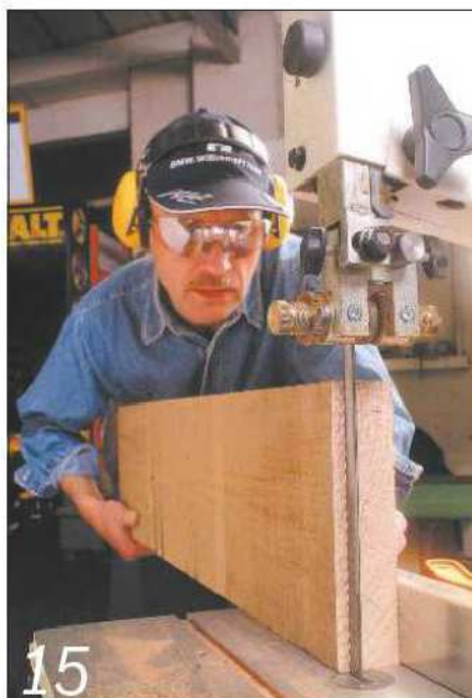
The bandsaw's big advantage over the table saw is its ability to rip deep timber
