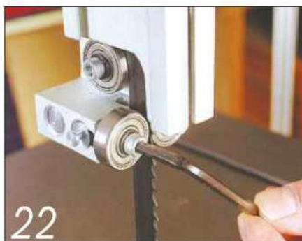
22 You usually need a tool such as an Allen key to adjust side-on roller bearings
