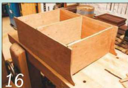
16 Check that all the dovetail housings fit well, and ease any that are tight
