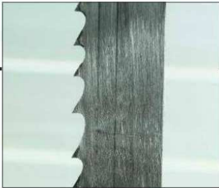
The weld on the blade is perfect, so it runs without surging or bumping
