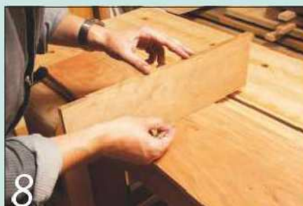
8 Mark out all the shelf positions with care, using a thicknessed shelf held on edge
