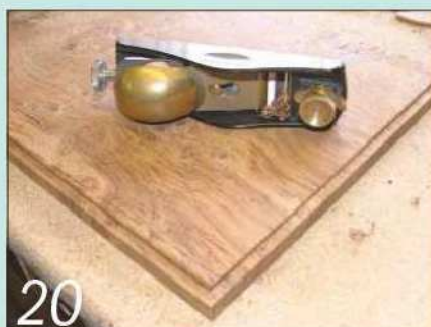
I formed a tongue on each edge of the panel and added a shallow bevel...
