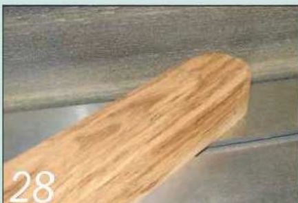
28 I rounded off the front end of each side rail on my oscillating belt sander
