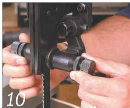
Disc guides should be set a paper's thickness clear of the blade
