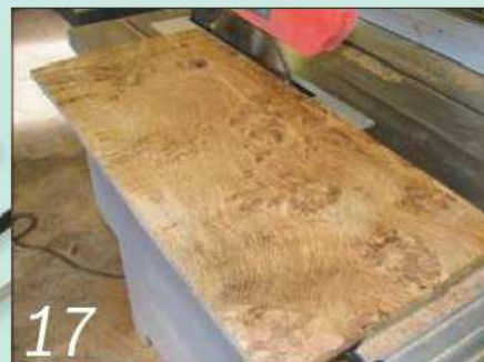
17 I chose a particularly well-figured piece of burr oak for the centre of the lifting flap
