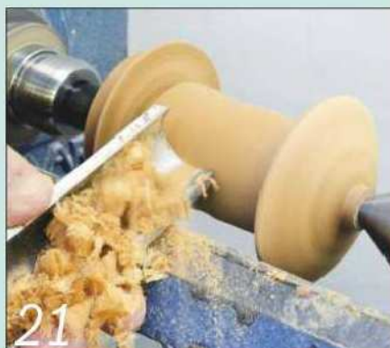
21 You can now remove most of the waste from the central spindle area...
