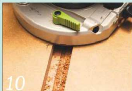
Start routing with a straight bit; the pencil marks on the jig indicate where to stop the cut
