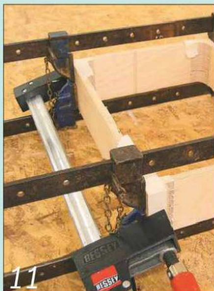
11 Note that the external corners are left square at this stage to make cramping easier
