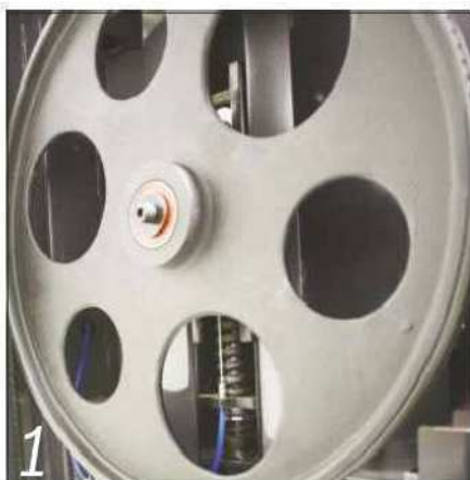
1 The diameter of the wheels determines the bandsaw's throat capacity
