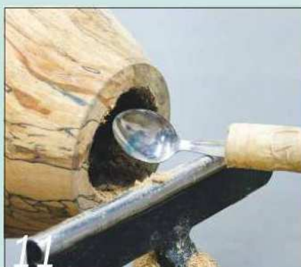
11 An old teaspoon taped to a dowel is useful for removing shavings
