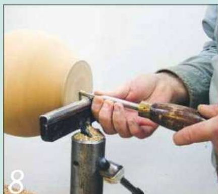
8 Drill a hole with a narrow spindle gouge to the required depth
