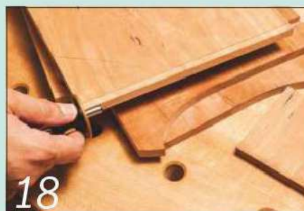
18 ...and transfer the measurement to the front of each shelf dovetail
