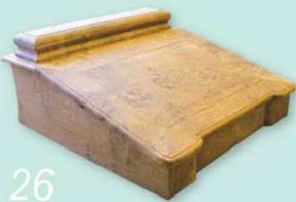
26 The top box could now be dry-assembled and any necessary adjustments made
