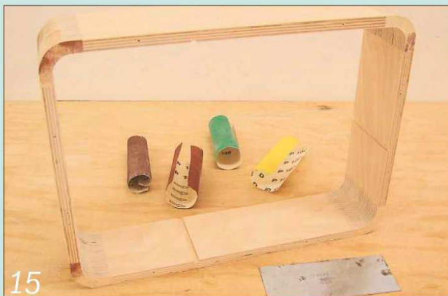
15 This is now the time to clean up the internal corners of the box – a job easier to do at this stage than later
