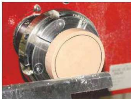
5 Mount the first blank, turn it to round and face it off. Then draw a circle to give a 5mm wide rim around the edge
