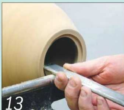
13 Cut a square step on the rim of the vase body with a skew chisel
