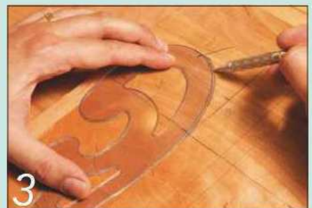
3 I used a French curve and a simple grid to mark out the curved profile on the uprights
