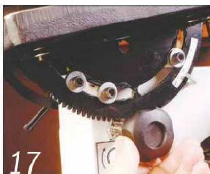
Rack-and-pinion adjustments make bevel setting an easy task
