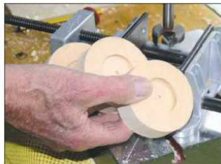
4 Prepare a selection of blanks, ready for mounting on your chuck
