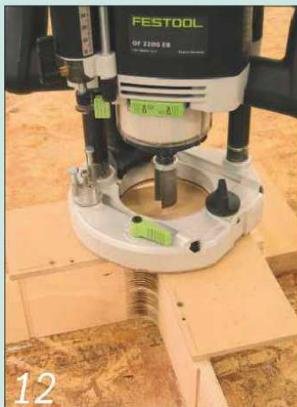
12 The internal corner template allowed me to trim the internal curves; note the cutter burn
