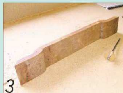
3 The front of the top box has a recessed centre, formed from three overlapping parts
