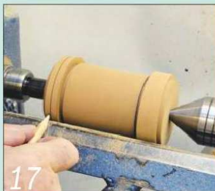
17 Mark out the mid-position of the pulley vee groove with a pencil
