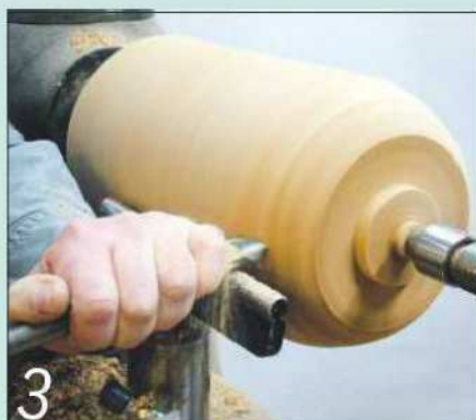
3 Start shaping the outside of the piece at the tailstock end
