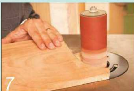
7 ...and a bobbin sander on the curved sections to shape them precisely to the marked line
