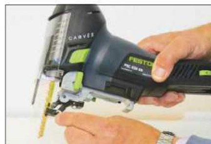
The blade guide screw is adjusted to nip the blade and then slackened
