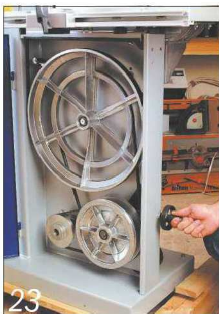
23 Altering the belt on the lower wheel changes the speed ratio
