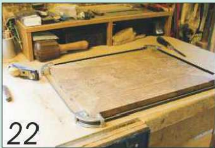
22 After assembling the frame and its panel, I secured the joints with a strap cramp
