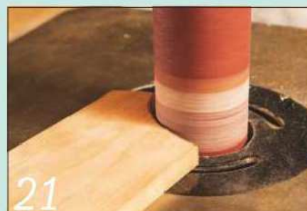
21 Cut the curve on the bandsaw and smooth it on the bobbin sander as before
