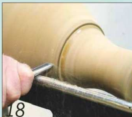
18 Blend the base and neck sections together with the spindle gouge
