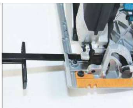
Clever sprung cam levers hold the side fence securely in place
