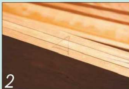
2 After grain-matching the various components, I pyramid-marked all their edges
