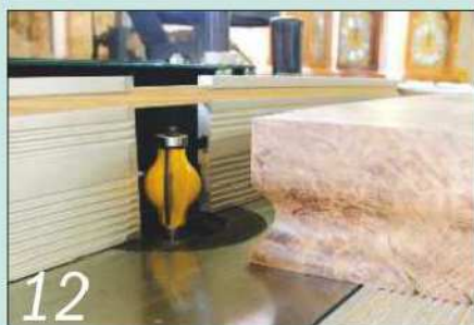
12 I made this curved cut round the base of the gallery top block with a handrail cutter
