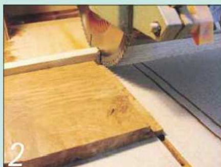
2 I started work on the top box, cutting rebates to join the back corners
