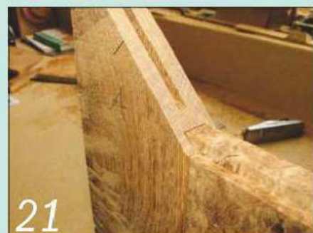
...before cutting grooves in the four frame members to accept the panel tongues
