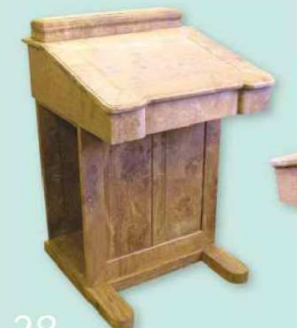
38 The top, the carcase and the foot plate are screwed together to check the fit
