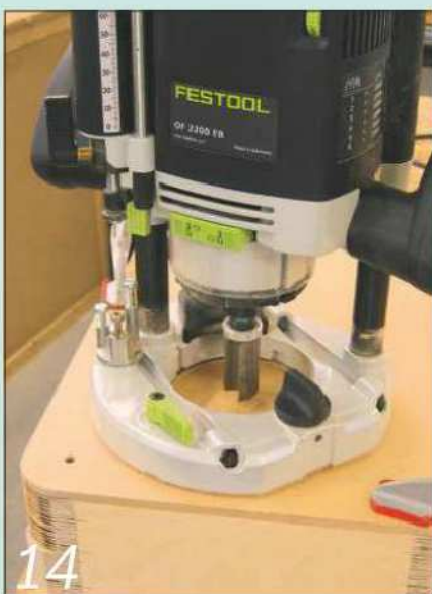
14 I then trimmed them precisely using the external curve template and profile cutter
