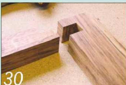
30 ...and a half-lap joint links the side rails to the ends of the rear rail
