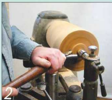
2 Turn to a cylinder and cut a spigot on both ends to fit your chuck
