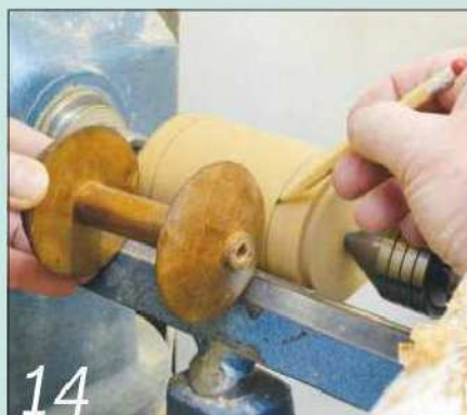
14 Mark the major features directly onto the work from the original
