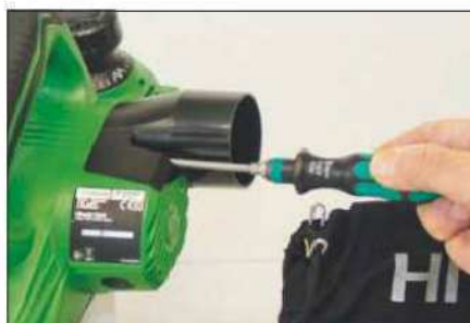
Just one screw secures the optional dust port adapter to the planer body
