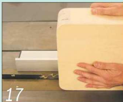
17 After trimming the top and bottom edges, cut the box carefully in two on the table saw
