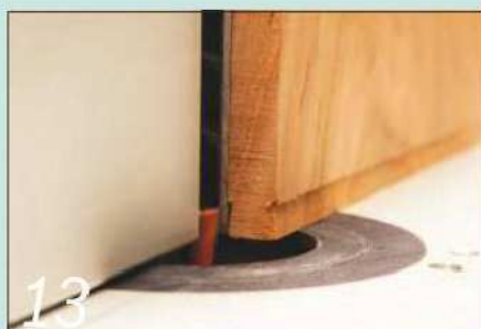
13 Machine the dovetail on the router table, working from both sides of the shelf
