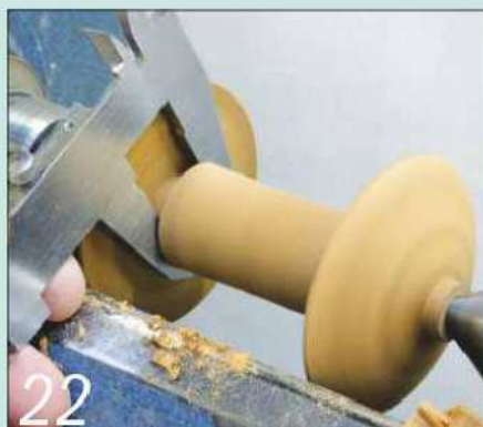
22 ...before sizing its final diameter accurately with the callipers and then finishing it off
