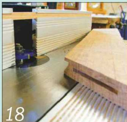
The frame has mitred corners, into which I routed slots to take biscuits
