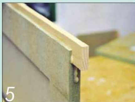
5 A solid wood fillet glued into a groove in the edge of an mdf door makes a secure fixing for the hinge screws
