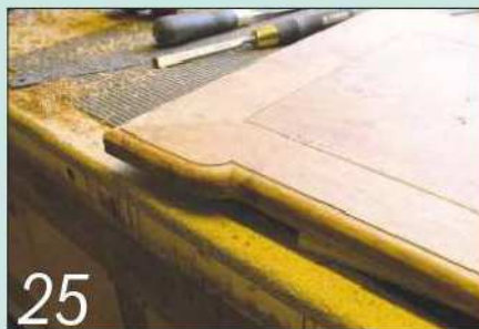
25 After cutting the flap to its final size, I moulded its front and side edges with an ovolo cutter
