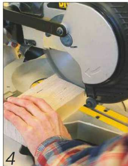
4 The four corner blocks are quickly cut to size
