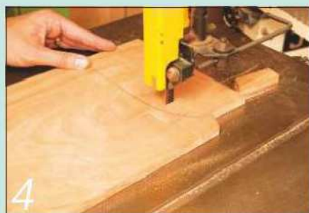
A series of parallel relief cuts make it easier for the blade to follow the curved line later...
