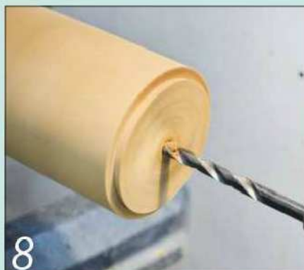
8 Hold one dovetail spigot in a four-jaw chuck while you start to drill the hole
