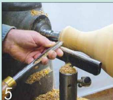
5 Complete the rough shape on the outside using a spindle gouge
