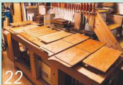
22 Coat all the interior surfaces of the units with quick-drying sanding sealer
