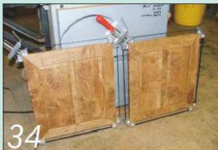
34 The front and rear panelled frames were made with twin fielded panels...
