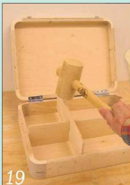
19 Fit the hinges and tap the two compartment dividers into their grooves
