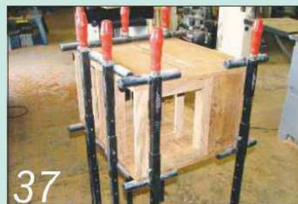
37 The main carcase is assembled, cramped up and set aside while the glue dries
