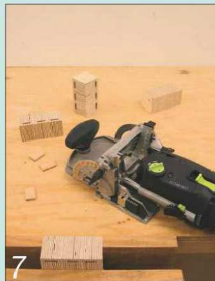
7 The Festool Domino makes a quick job of cutting the slots in each corner block
