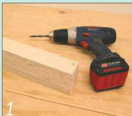
1 The stack of plywood is held in place with short lengths of 6mm dowel through opposite corners
