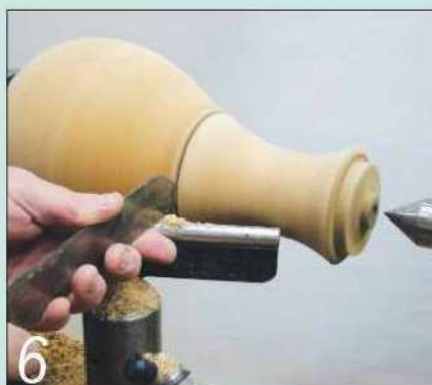
6 Use a narrow parting tool to part off the neck with a thin cut
