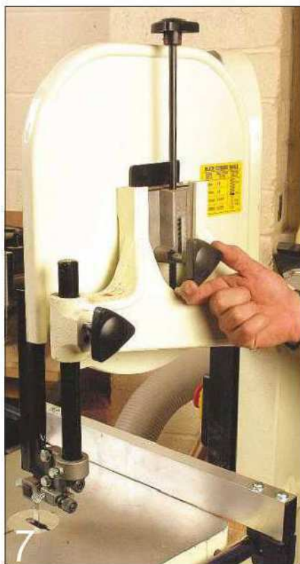
The top wheel is rotated as the tracking is adjusted to align the blade
