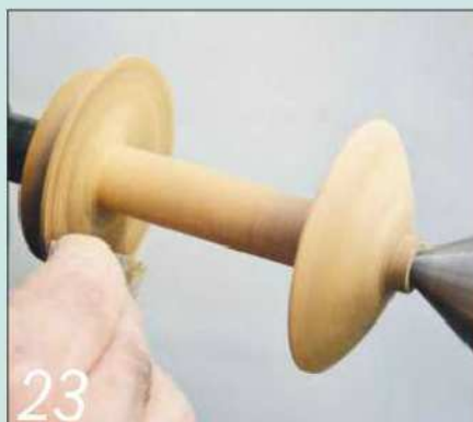
23 Sand the bobbin smooth all over to ensure threads don't snag on it in use
