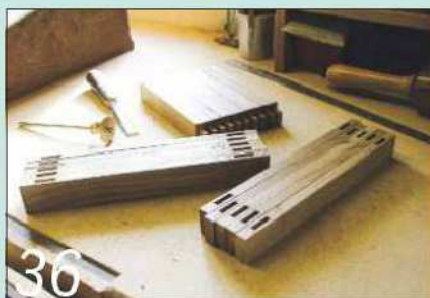
36 The five frames that link the panelled frames have mortise-and-tenon joints
