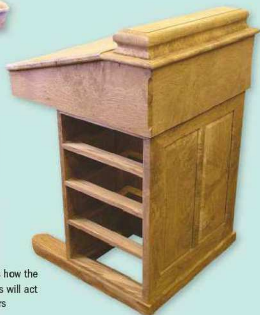
38 The top, the carcase and the foot plate are screwed together to check the fit
