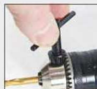
The keyed 10mm (in) chuck is small by today's standards
