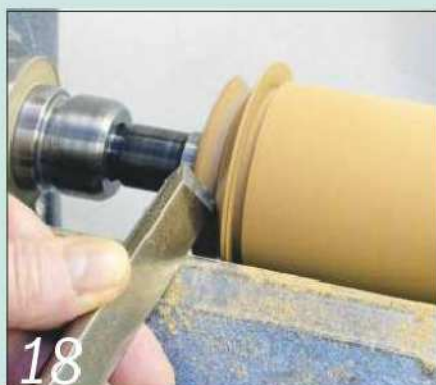
18 Cut the sloping sides of the vee with the long point of the skew chisel
