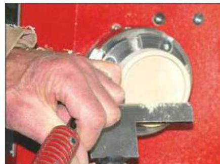
6 Remove the centre with a gouge to produce a shallow recess for the 'jam'. Use a 4mm parting/beading tool to square up the inner edge
