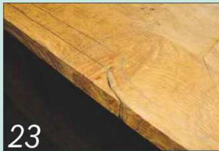
23 I made the curved cuts into the leading edge of the flap with a jigsaw...
