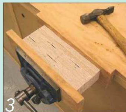
3 ...that there'll be no slippage. The stack is then cramped securely while the glue cures
