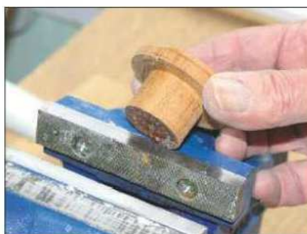
8 Hold the jig in a vice by the lower spigot and push the tart onto the upper spigot. A sheet of tissue paper will help to ensure a tight fit
