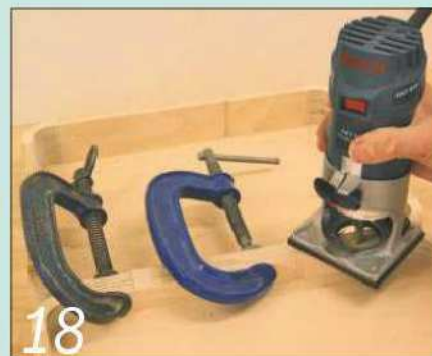
18 Clamp box and lid together and rout out the hinge recesses on both parts at once
