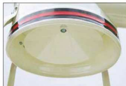
The cyclonic cone fitted to the extractor housing helps to prevent clogging
