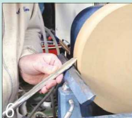
6 Use light cuts taken with the 13mm bowl gouge to true up the blank
