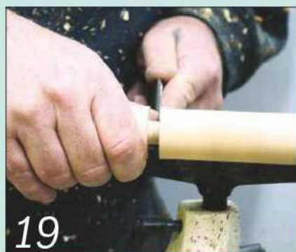
19 Separate the two ends from the body using a narrow parting tool
