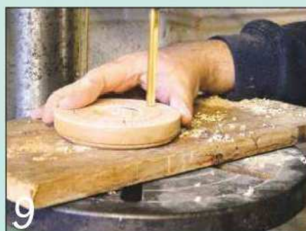
9 Drill an 8mm diameter hole 8mm deep at the three marked spindle locations
