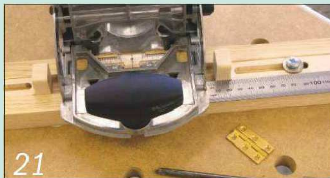
21 When cutting a lot of wider mortises, a home-made jig may speed things up
