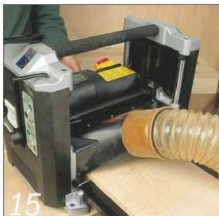
15 Width capacities are usually better than on an entry-level combination planer
