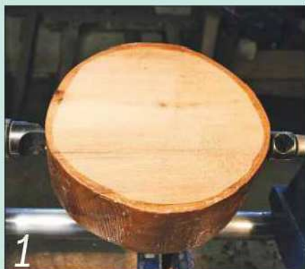
1 Locate the disc centres and mount it on the lathe using the hollow cone centre
