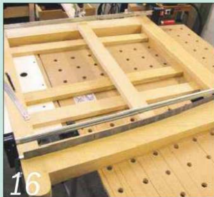
16 Mark the curved underside of the top rail using a steel rule held on edge
