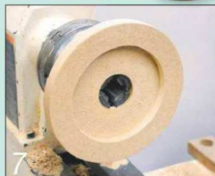
7 Make a jam chuck, mount the workpiece in the recess and clean up the other face
