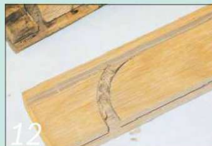
12 I then drilled away most of the waste with a slim Forstner bit...
