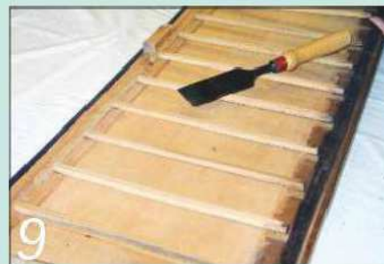
9 I marked all the original drawer runner positions before prising them off
