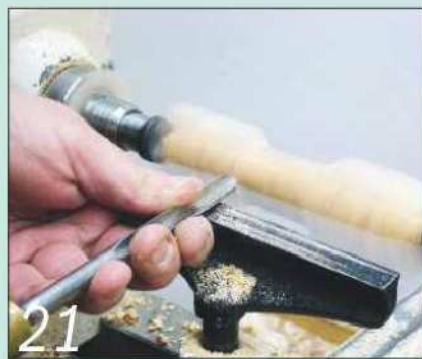
21 Plug the ends, mount the piece on the second set of centres and cut a cove in the middle
