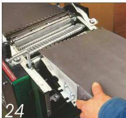
24 On most entry-level floor-standing machines, you have to remove the infeed table to access the thicknesser
