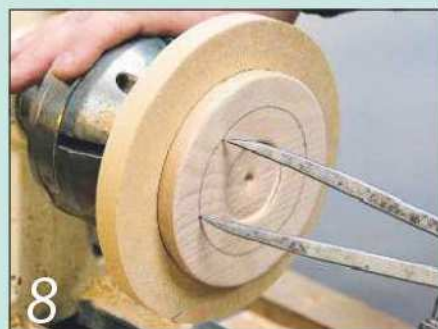
8 Draw a circle to locate the spindles and use compasses to mark their positions
