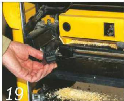
19 The portable versions often have magnetic setting gauges to help as space can be restricted
