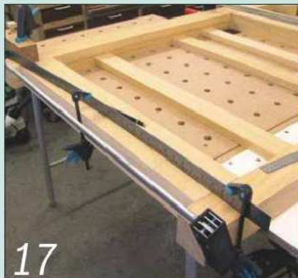
17 Repeat the process on the bottom rail, cramping the curved rule in place
