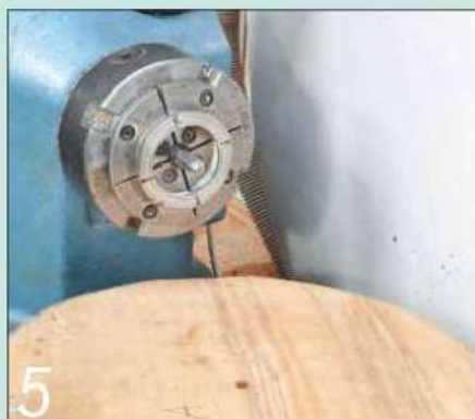
5 The various bowl blanks will be held securely on this screw chuck
