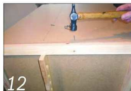
12 Cut the back panel to size and pin it to the rear legs and rails
