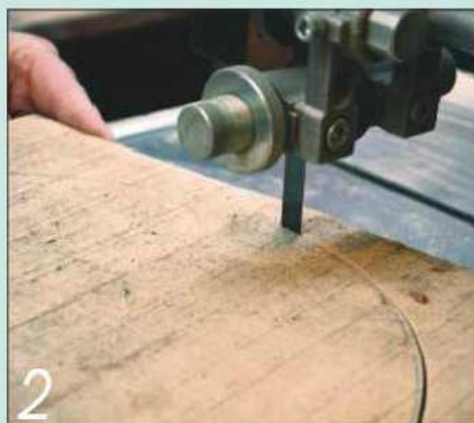
2 Cut out the individual circles closely to size on the bandsaw
