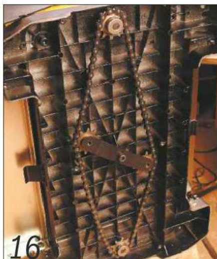
16 The drive gear for the bed can vary from a heavy-duty chain and sprocket...
