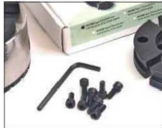
The jaws come with a flimsy Allen key; I'd prefer a T-handled version
