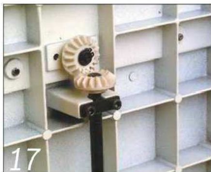
17 ...to simple but not very durable plastic cogged gearing on a cheaper model
