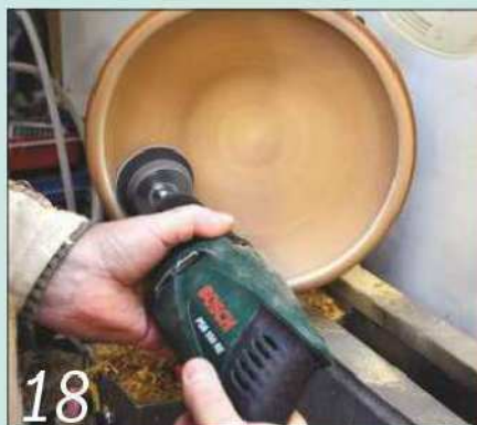
18 Power-sand the interior, working from 120 grit down to 240 or further
