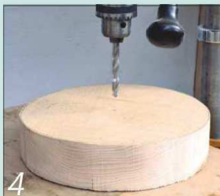
4 Drill an 8mm hole about 20mm deep in the centre of each blank
