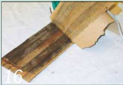
However, a hot iron soon softened the old glue, allowing me to peel the hessian off
