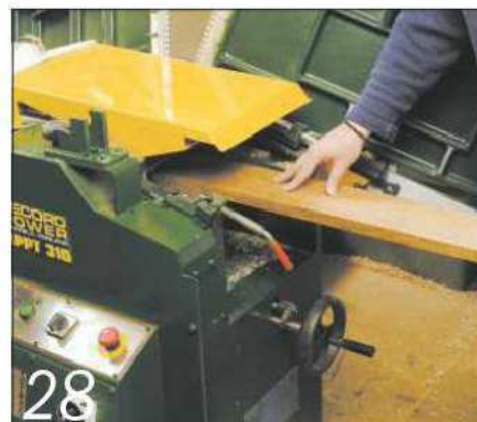
28 Dust control is important with these machines, and integral hoods also serve the purpose of covering the cutter block safely
