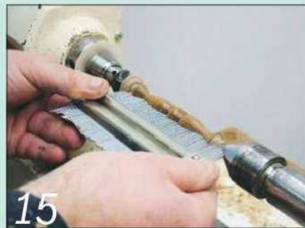
15 Offer up the profile gauge to take a copy of the first spindle's shape
