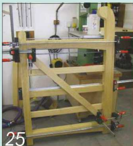
25 I used several small cramps to act as bearing points for the larger cramps
