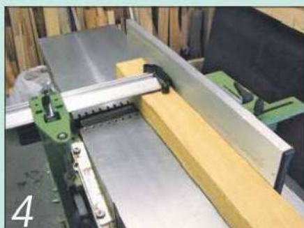
4 After this rough sawing, the stock was surface-planed ready for thickening
