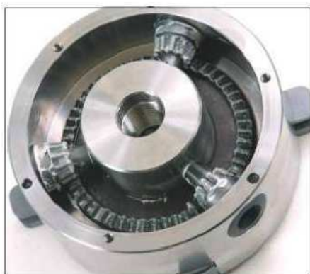
A heavy-duty scroll and three pinions open and close the chuck jaws with a silky smooth action
