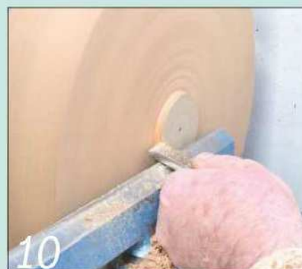
Then you can use a skew chisel to form the dovetail profile on the spigot
