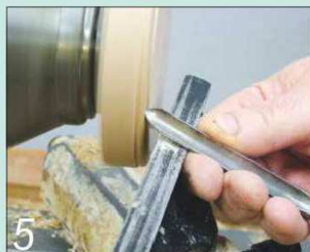
5 Turn a decorative edge to the plate using a spindle gouge...
