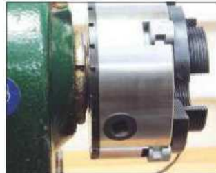
The chuck's flat back may tighten up onto the headstock casting
