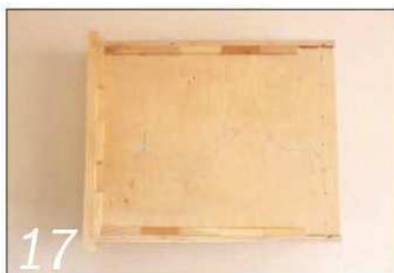
Fit the drawer bottom and add plenty of glue blocks on the underside
