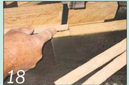
...and then set up a stop on the bandsaw so I could cut their small end rebates
