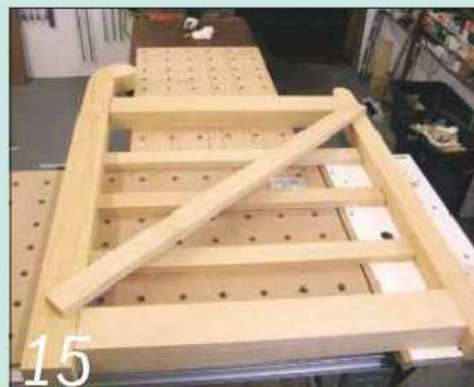
Test the layout so you can mark accurate joint centre lines on all the stock
