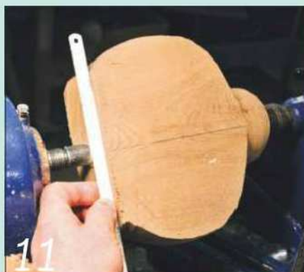
11 Use a straightedge to check that the base is uniformly flat
