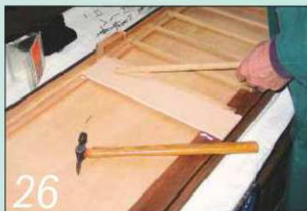
I refitted the old drawer runners to the repaired side panel using a spacer
