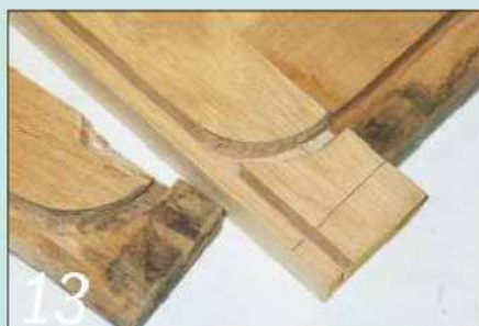
13 ...and finished the job off by hand with a couple of sharp gouges
