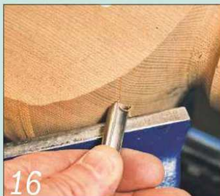
16 Use a sharpened bowl gouge to perform fine finishing cuts around the body
