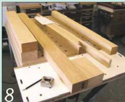
After final planing and thicknessing, all the components were cut to length
