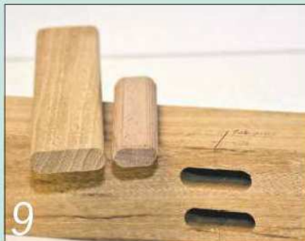
A home-made domino (on the left) is over twice the size of a Festool standard domino
