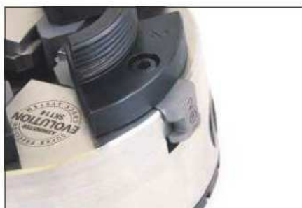
The outer end of each accessory slide is machined to a rounded profile
