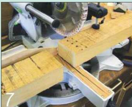
Mark the cut ends to identify them, as they may not end up square after being dimensioned
