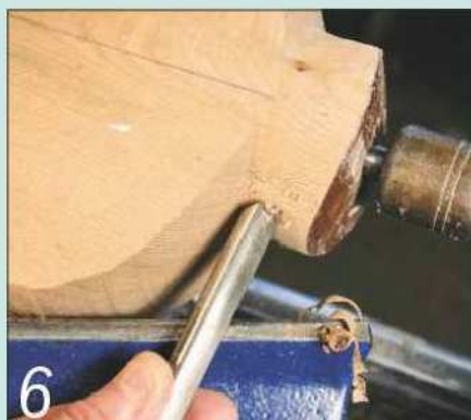
6 When you reach the neck, use the gouge to turn it roughly to shape
