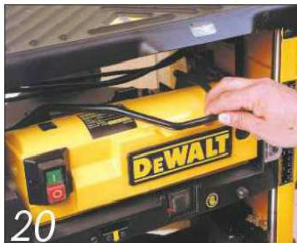
20 Better portable models have a headlock to prevent excessive chatter as the stock feeds through...
