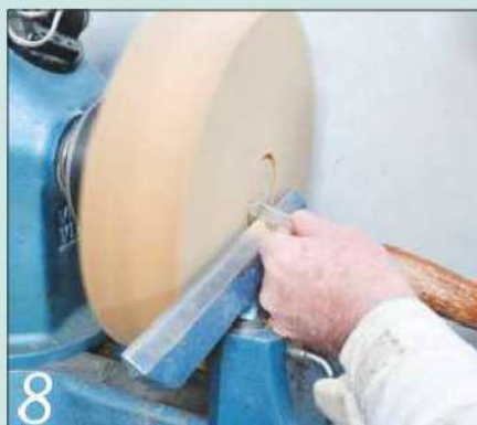
8 Cut in to start forming the spigot which will later be held in the chuck
