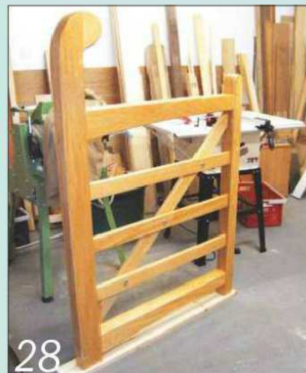
28 I gave the gate two generous coats of Osmo clear outdoor UV protection oil
