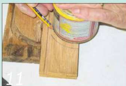
11 I used some conveniently-sized paint tins to draw the corner curves
