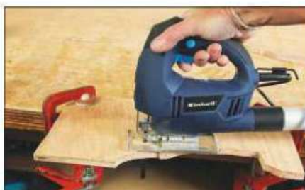
The cutting speed is relatively slow without the benefit of orbital action
