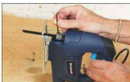
A hex key is used to change the blade and to adjust the baseplate angle
