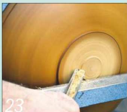
23 Cut away the spigot carefully and clean up the surface using the bowl gouge
