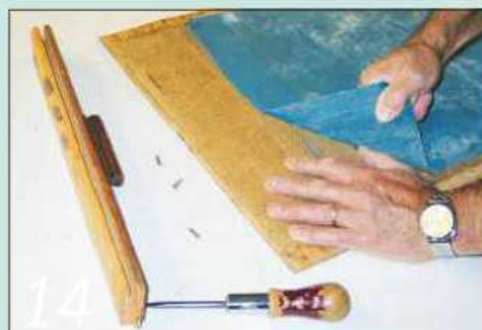
14 I removed the tambour handle bar and tore off the old blue canvas
