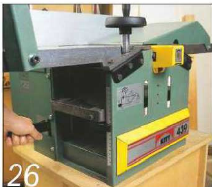
26 The Kity 439 retains the over/under format so there's no bed or fence removal here. Planing and thicknessing capacities are both 200mm
