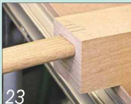
23 This joint shows the centre lines for cutting the left- and rightmost mortise slots
