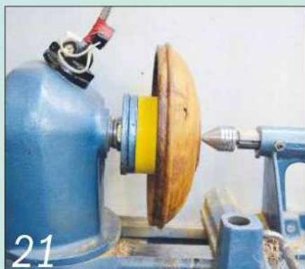
21 Use the tailstock centre to re-centre the bowl on the vacuum chuck
