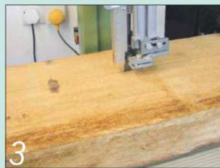
3 As I no longer have a table saw, I planned to re-saw the stock on my bandsaw
