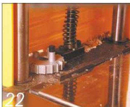
22 The turret post is also superb for making repeat cuts to standard stock sizes
