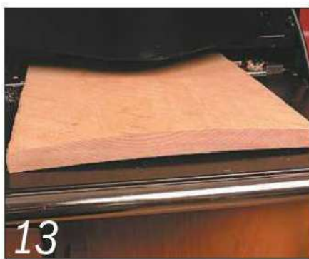
13 Putting stock through without a flat reference face will give poor results
