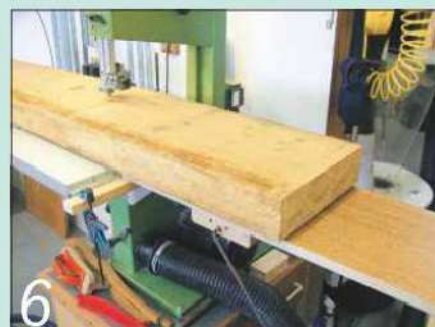
6 My small bandsaw can handle large workpieces, thanks to the addition of an outfeed table
