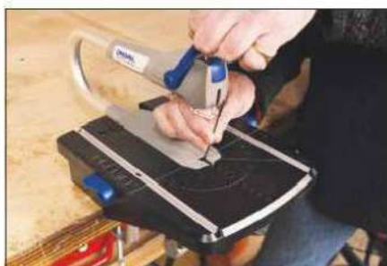
A single lever tensions the blade once it's been hooked onto its clips
