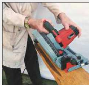
A single knob locks the bevel ripping angle very positively
