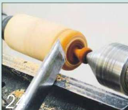
24 Make a slicing cut with a skew chisel to clean up both ends of the piece
