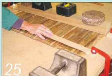
The two lengths of webbing were glued to the slats and weighted down
