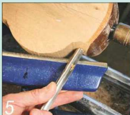
5 Work round towards the neck, keeping the tool bevel in line with the work surface
