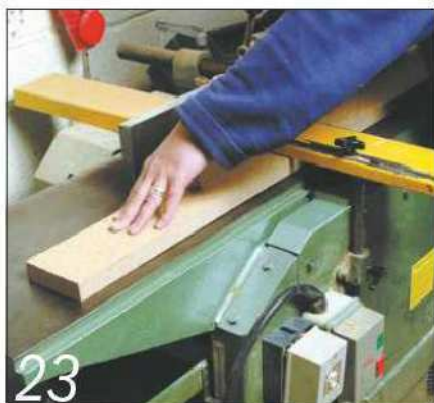
23 Rock-solid and an industry standard, the classic over/under style machine was a workhorse in many workshops
