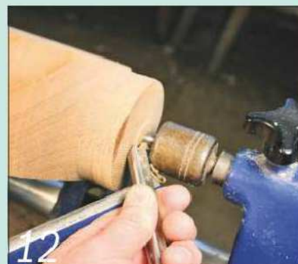
12 Move the toolrest and slice the top of the neck smooth with a small gouge
