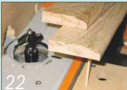
Some lengths of lamb's tongue moulding were soon machined to form the new skirting
