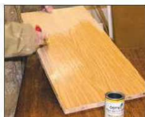
Apply PolyX-Oil sparingly along the grain by brush, roller or cloth
