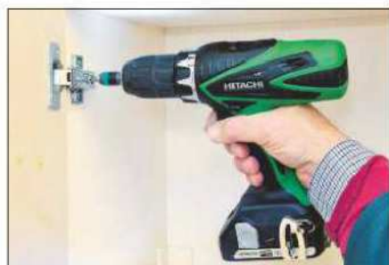
This machine has no worklight, which may be a drawback in dark corners
