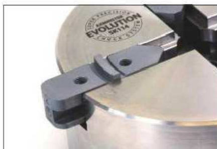
The accessory slides are machined to sit 0.5mm above the chuck body
