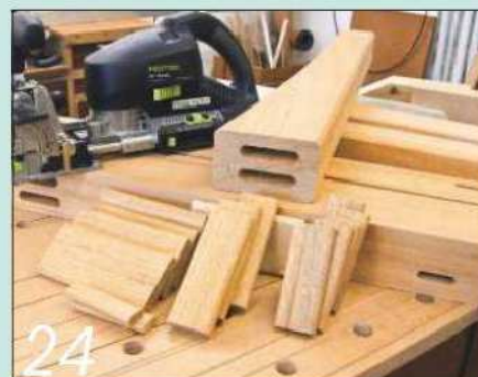
24 With all the components ready for assembly, I put the chamfer details on all the rails
