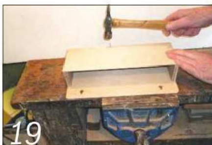
Make up the demountable door storage box from some plywood and mdf offcuts
