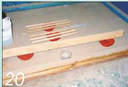
I placed the new slats and the frame piece in my ammonia fuming chamber to darken them
