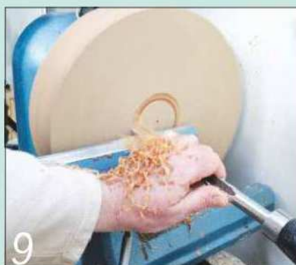
Remove some of the waste surrounding the spigot with a 13mm bowl gouge
