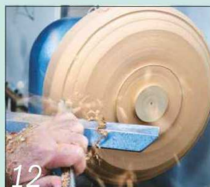
Start to shape the underside working from this corner using the bowl gouge
