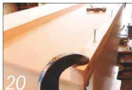
Screw the top in place on the bench base and add the rear lipping strip
