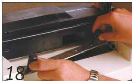
18 Portable thicknessers can have the option of disposable knives or resharpenable ones
