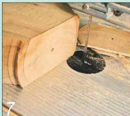
7 Cut the bottom section away on the bandsaw to provide a flat base
