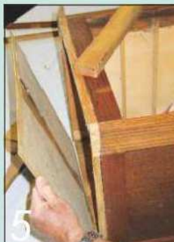
...that the thin veneered top was held on with just some small pins
