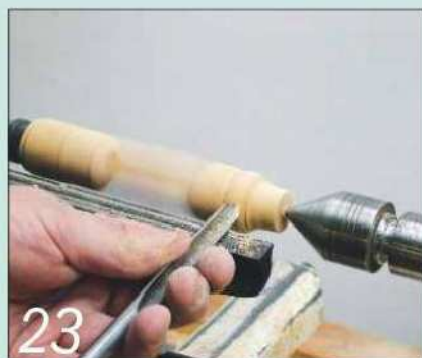
23 Remount the piece on its true centres and turn a bead to disguise each of the plug joints
