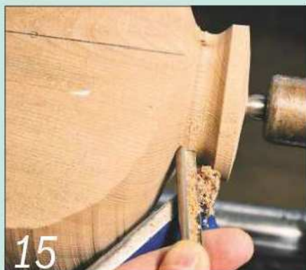
15 Work in the opposite direction to complete the shape of the shoulder
