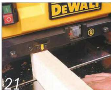
21 ...and an indicator to check how much will be removed in a single pass before feeding it in
