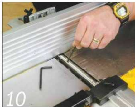
10 The simple wedge block knife retention is commonplace on most jointers
