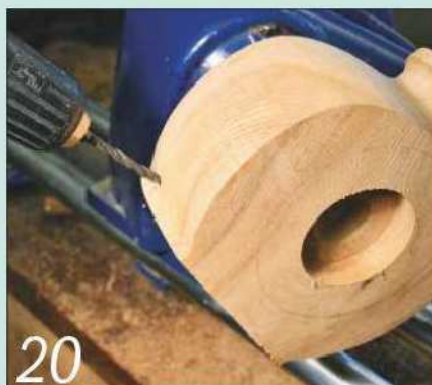
20 Drill a hole through the side of the lamp into the central recess to admit the flex
