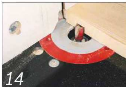
14 Cut the trenches to form the drawer box joints on the router table
