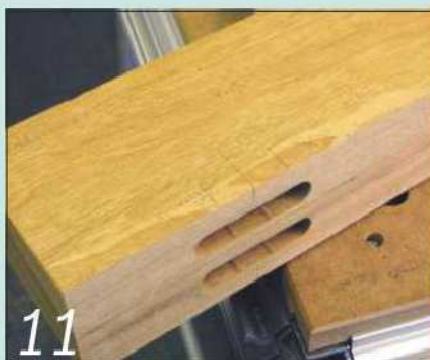
Follow the guide lines for the left and right domino cuts to make an extra-wide mortise
