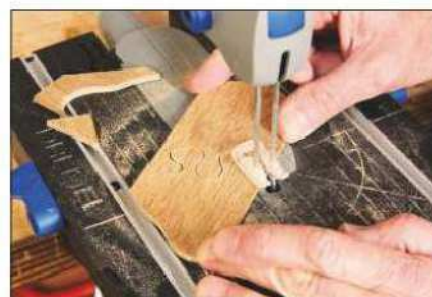
The skinny blade will follow the most intricate curved cuts with ease
