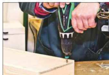
You can control the speed precisely by using the proportional on/off trigger
