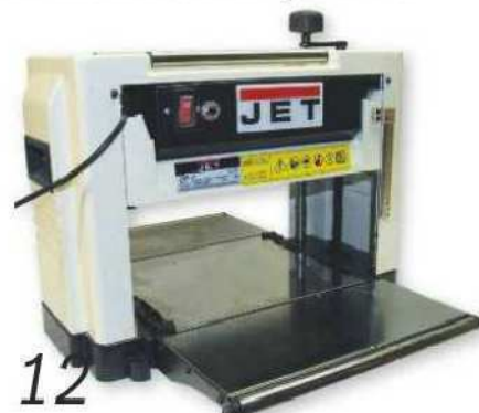
12 Portability and a small footprint are huge advantages in a bench-top thicknesser
