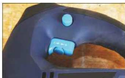
The trigger houses a small wheel that sets the maximum cutting speed
