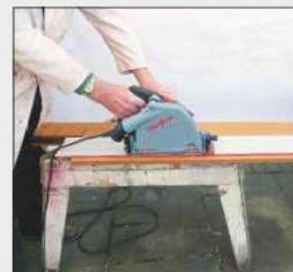
The 1.6m rigid guide rail makes light work of cutting up boards
