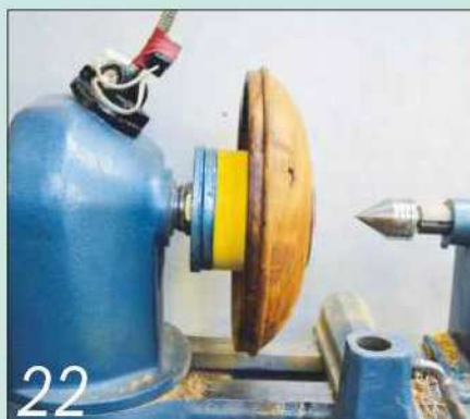
22 Remove the tailstock. The bowl is held on the vacuum chuck as if by magic!
