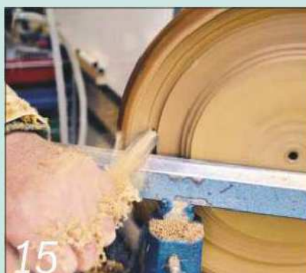
Hollow the bowl by locating the gouge in the groove and cutting inwards
