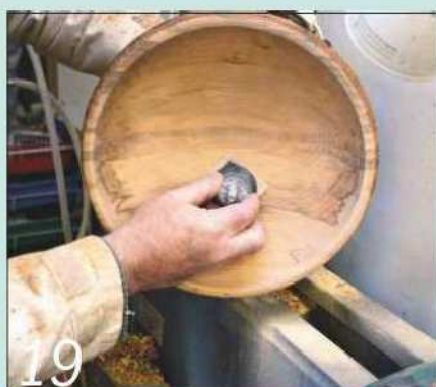
19 Turn off the lathe and hand-sand the surface with the grain after each grit change
