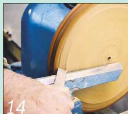
Reverse the bowl and form a starter groove with the skew chisel
