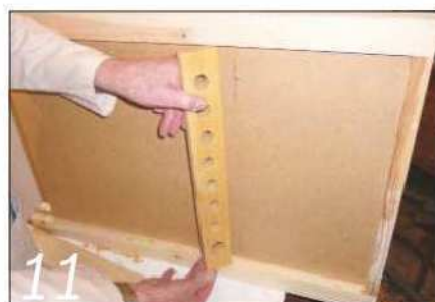
11 Fit the tool storage shelves to the end frames with glue and screws
