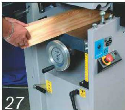
27 Go up to professional level and dial gauges are common, allowing repeat fractional cuts to be set up and made with ease
