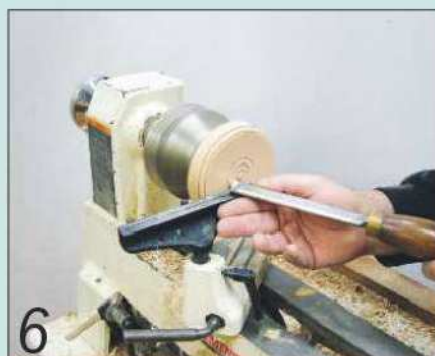
6 ...and cut some decorative beads on the top of the plate with a skew chisel
