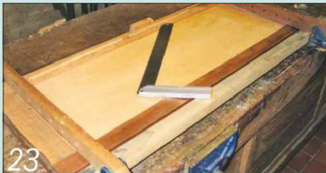
I placed the new slats and the frame piece in my ammonia fuming chamber to darken them
