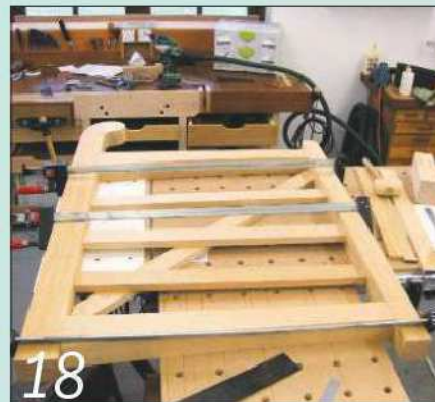
18 Cramp up the gate, place it over the cross brace and mark the angled cutting lines on it
