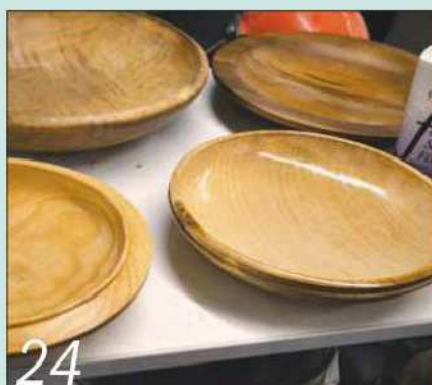
24 Apply three coats of the finish, letting the bowls dry between coats
