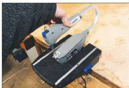
The body of the saw slides into the slot in the table and clips in place
