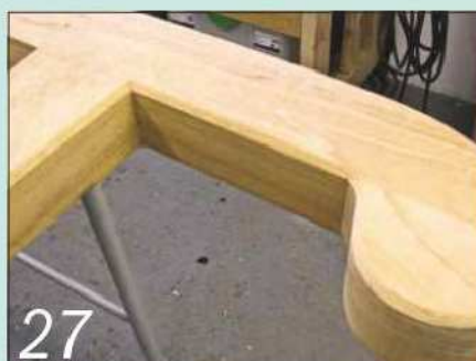
27 With the gate assembled, I tidied up the chamfer details with a chisel
