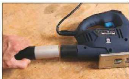
The adapter supplied makes it easy to attach a dust extraction hose
