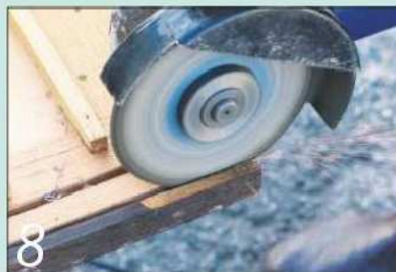
8 Nails reinforced many joints, but my angle grinder soon cut through them
