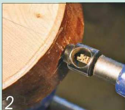
2 Feed the lamp auger through the hole in the tailstock and start boring
