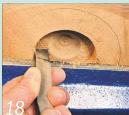
18 Hollow out the recess for the clock body, finishing it with a square scraper
