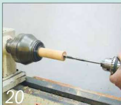
20 Mount the main body in your chuck and drill a 14mm diameter hole through it
