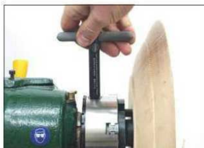
There's no problem using the key behind large-diameter work
