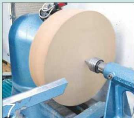
7 Mark the centre of the blank clearly with the revolving tailstock centre
