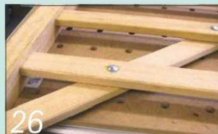
26 I fitted M12 x 60mm coach bolts to secure the brace to the intermediate rails
