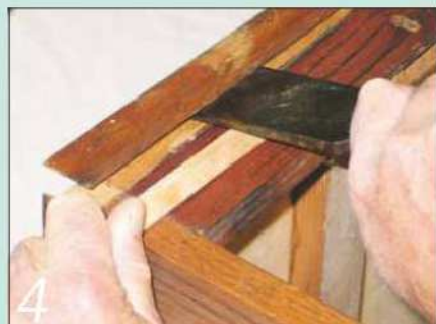
The decorative beading around the top was split. I prised it off with care to reveal...
