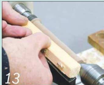
13 Then use the scratch stick to mark the positions of the various details
