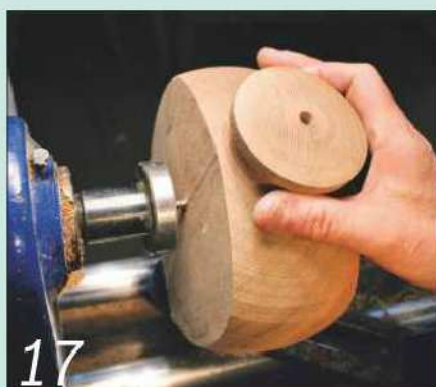
17 Remove the work and mount it back on the lathe using a screw chuck
