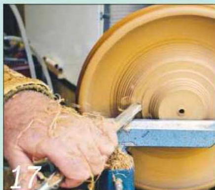
17 Continue hollowing out the bowl until the whole central waste area is removed
