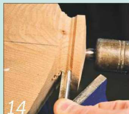
14 Slice in with the gouge to form one side of the neck's concave radius
