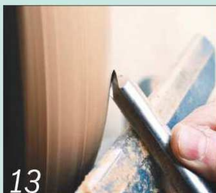
Use the lower wing of the gouge to shear-scrape the bowl surface
