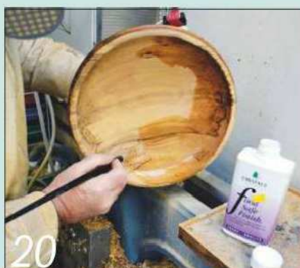
20 Use a clean, uncontaminated brush to apply the food-safe finish
