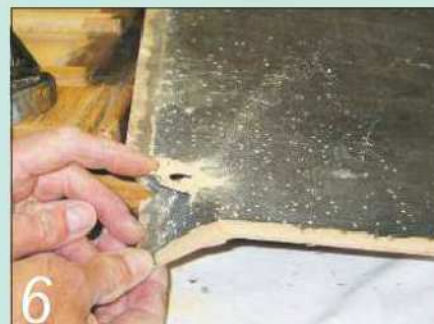
The plywood back panel had provided a feast for generations of woodworm
