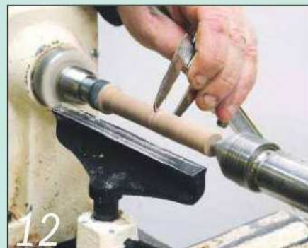
12 Turn the first spindle to a 16mm diameter cylinder and check its size with callipers
