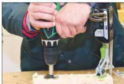
The drill even coped with driving my rather dull 50mm diameter Forstner bit
