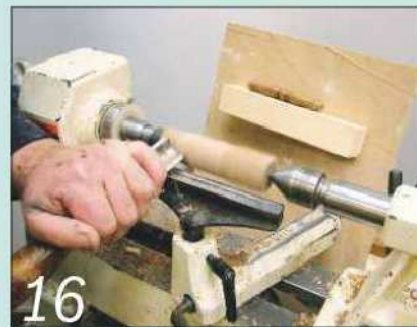
16 Keep the first spindle handy for comparison while you're turning the others
