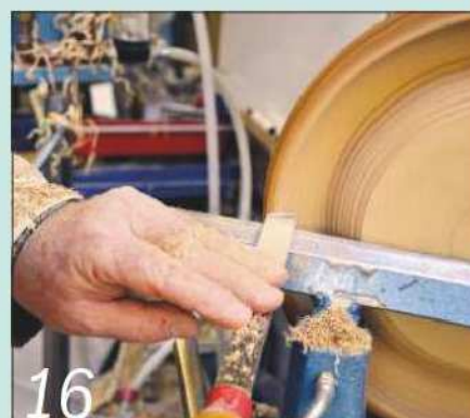
Finish the rim to a pleasing curve before hollowing out the bowl any further
