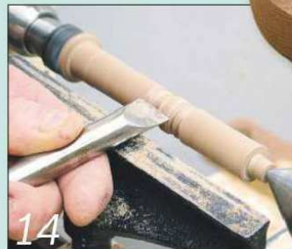
14 I used a skew chisel and spindle gouge to create the spindle profile
