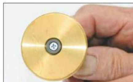
The wheel cutter can be retracted into the gauge face when not in use
