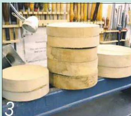
3 After a bit of a bandsaw marathon the stack of blanks is ready for turning
