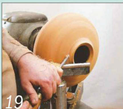
19 With the inside completed, finish the outside with a small spindle gouge...
