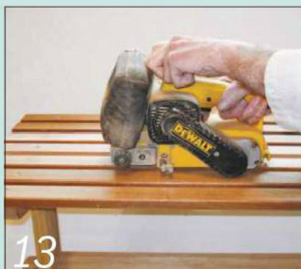
13 Use fine abrasive in a belt sander to give the top a final smoothing
