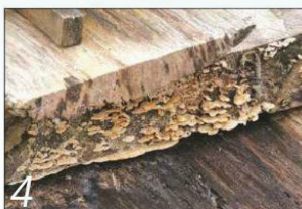
4 Others prefer to attack sawn timber while it's being seasoned
