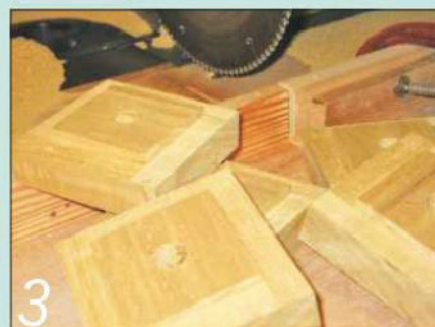
3 I had to relieve the edges of the blanks so I could feed them past the router cutter
