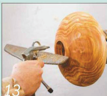
13 Remove the shavings frequently so they don't bind on the tool; I use a blast of compressed air
