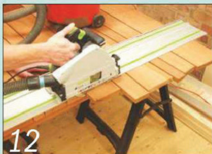
12 Cut the assembled table top to size. I used a circular saw and guide rail system
