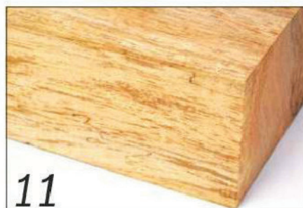
The initial infection affects only the wood's colour, not its strength
