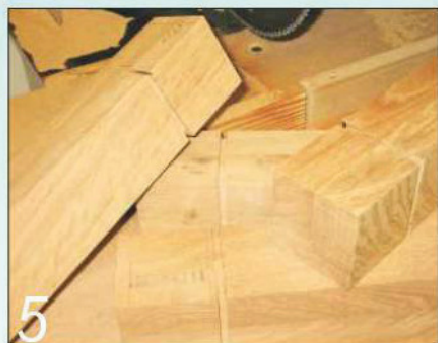
5 Cut a groove on the two outside faces of each leg for the decorative bead
