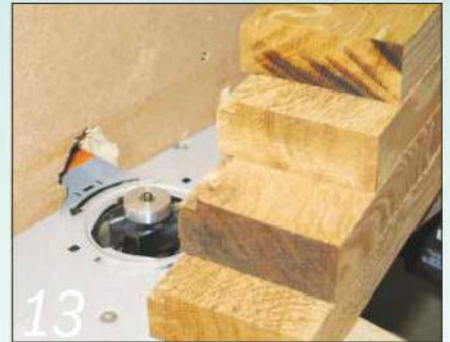
13 Cut the top frame components to length and form a rebate in one edge
