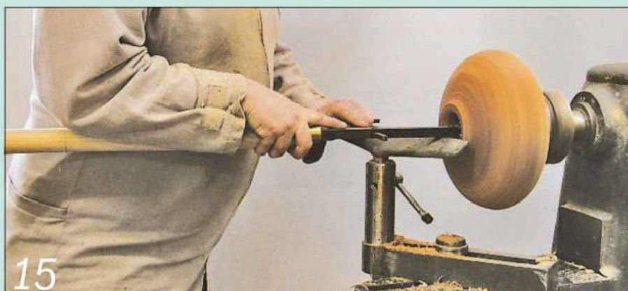
15 In this stance the pivotal force on the tool is absorbed by my forearm and shoulder
