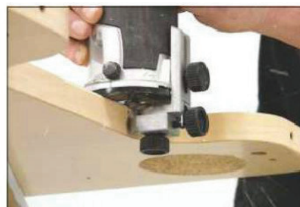
7 The bearing trimmer guide allows you to work against curved edges
