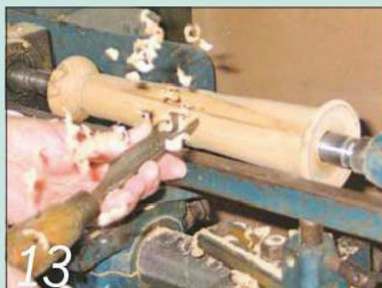
13 Trim the top section to length and start tackling the rest of the shaping
