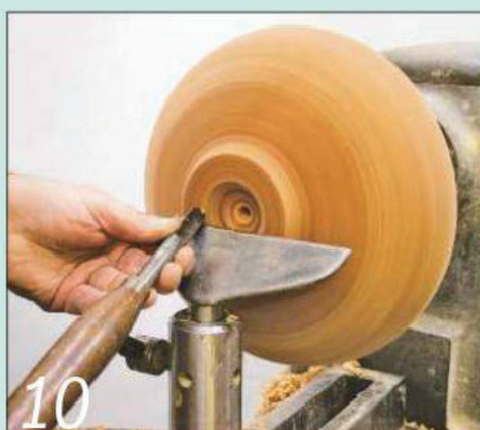
10 Use the bowl gouge to start hollowing, as if you're turning a bowl
