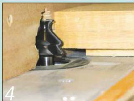
You can see how the relief cut allows the workpiece to pass over the cutter
