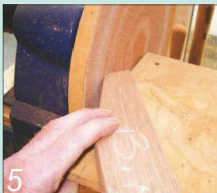
5 Form gently rounded corners on the feet and rails using the disc sander
