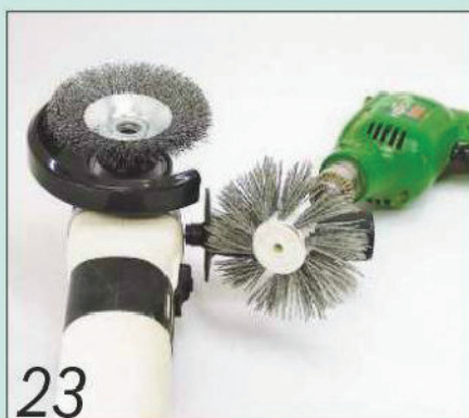
23 Try texturing the piece with a rotary wire brush, followed by a nylon one, if you can't sandblast it
