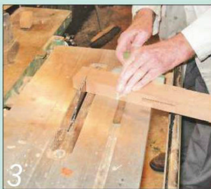
3 Trim the waste at an angle; note that the saw guard has been removed here for clarity
