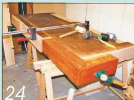
24 The front face was held in place by a clamp before being screwed in place
