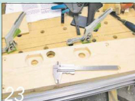
23 The template worked well after I had removed the bulk of the waste with a large Forstner bit
