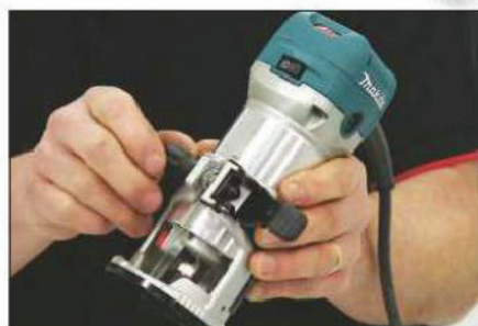
2 This precise rack-and-pinion adjuster sets the depth of cut in seconds
