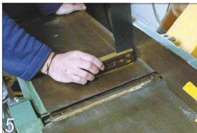
5 On the planer thicknessener, a quick check with a square takes seconds and can save hours of wasted work
