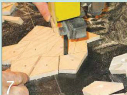
7 Drill and countersink the fixing holes, then cut out all the feet on the bandsaw
