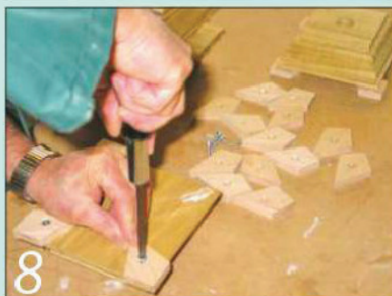
8 A dab of adhesive and a single screw fixes each foot in place to the base block
