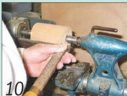
10 Mount each blank, turn it to a cylinder and square off the face of the socket end
