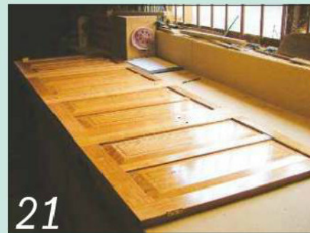
21 The resulting high-gloss finish needed de-nibbing and waxing to soften the glassy look
