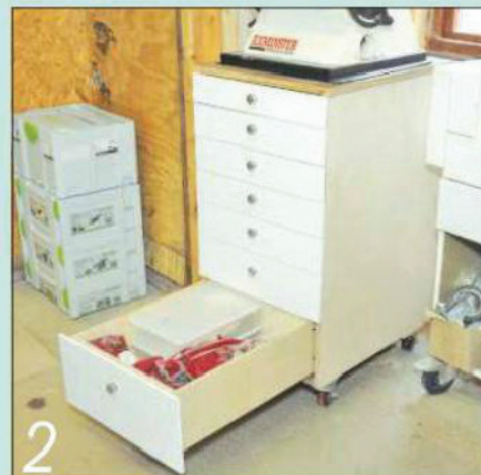
2 These simple drawers are mounted on full extension under-mounted drawer runners. These will carry up to 30kg and give total access to the drawer contents
