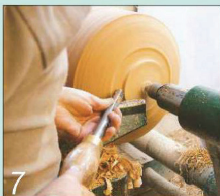
7 Cut the chucking spigot to a diameter that will suit the capacity of your jaws
