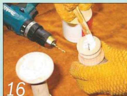
16 Use pliers to turn the screw into a pilot hole drilled in one column...
