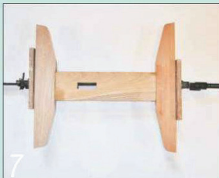
7 Cramp up each assembled leg frame to ensure tight, square joints
