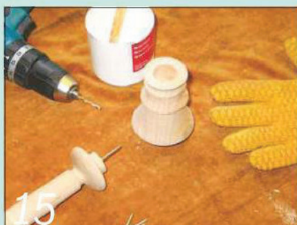
15 A double-ended screw plus a squirt of glue is the best way to join the two columns together
