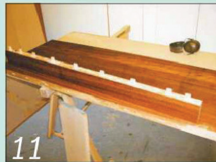
11 An 85mm wide strip of the bench top is re-attached along the front edge with dominos
