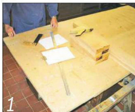
1 Drawing a full-size top view of the table is a useful technique to adopt
