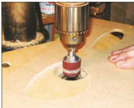
A false table fitted to a bench drill allows highly controlled sanding
