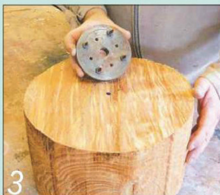
3 This is my adapted faceplate with four equally-spaced spikes screwed to it
