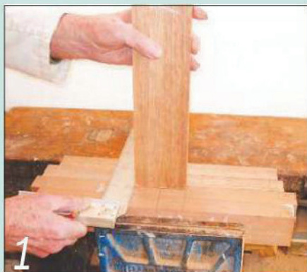
1 Mark out the positions of the mortises on the feet and top rails
