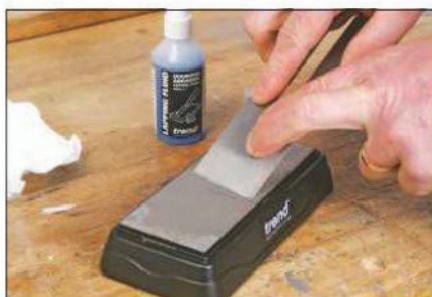
Always use a dedicated honing fluid to maximise cutting efficiency
