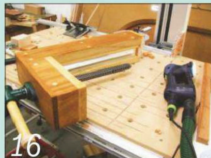
16 The tail vice body is about to be waxed after sanding, ready for installation in the bench top
