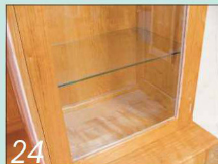
24 The final job was to glaze the doors and to fit the glass shelves on adjustable pegs
