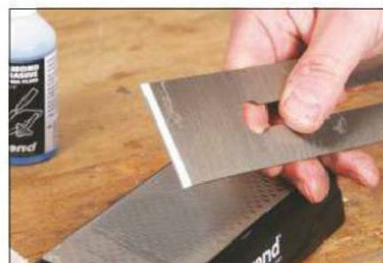
Just a few strokes on the stone were required to produce a super sharp micro bevel
