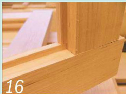
16 The result is a clean rebated corner in the door frame, ready to accept the glass
