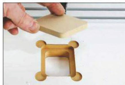
The small sacrificial mdf panels can be removed and replaced as necessary
