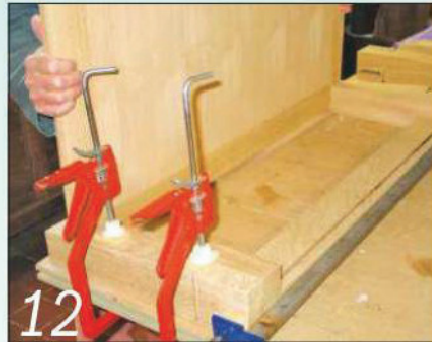
12 Test the fit of the shelf corners in the leg slots, and ease them if necessary
