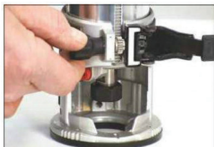
5 With the trimmer base fitted, depth adjustment is still quick and easy
