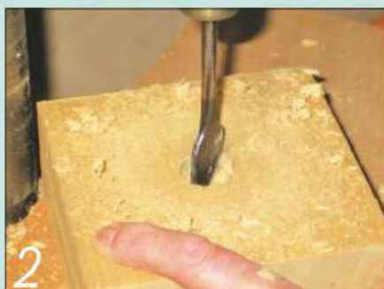
2 Bore a 25mm diameter hole in the centre of each block using a pillar drill
