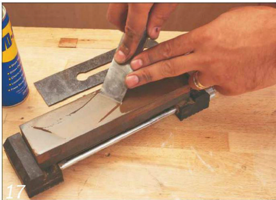
...but freehand honing is faster and every bit as accurate once you've mastered the technique
