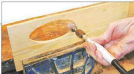
A flexible drive shaft fitted in a drill is a useful alternative method of working
