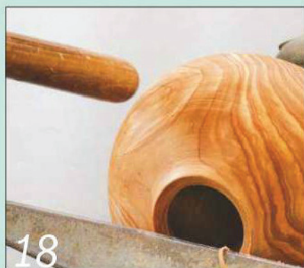
18 Tapping the vessel gives a good audible indication of the wall thickness
