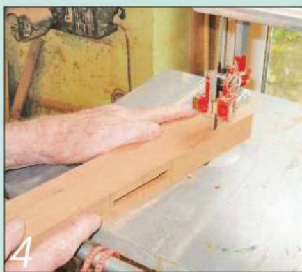
4 A bandsaw is the ideal way of forming the sloping cuts on the feet and rails
