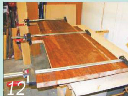
12 The three iroko fillets that will define the tool well area are also domino-jointed to the back edge
