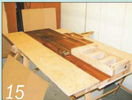
15 The tail vice sub-frame is screwed in place and the plywood bases of the tool wells are added
