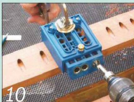
10 Use a proprietary pocket-hole jig to drill the screw holes in the rails
