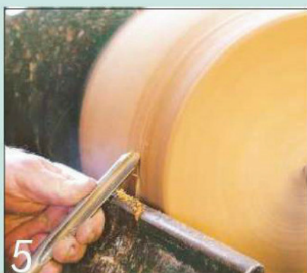
5 Start by truing up the side of the blank with a 1/2 inch fingernail bowl gouge
