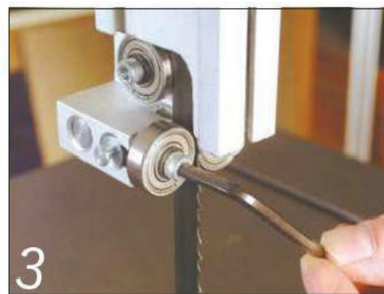
3 The roller bearings on this bandsaw can touch the blade and rotate with it
