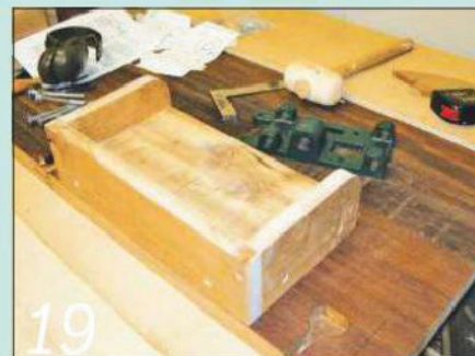
19 The main vice sub-frame shows the centre line used for lining up the assembly
