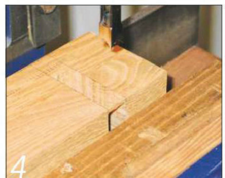
4 Cut the slots for the shelf in the same way while the legs are still square
