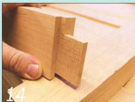
14 The result is a clean and crisp offset shouldered tenon that will...
