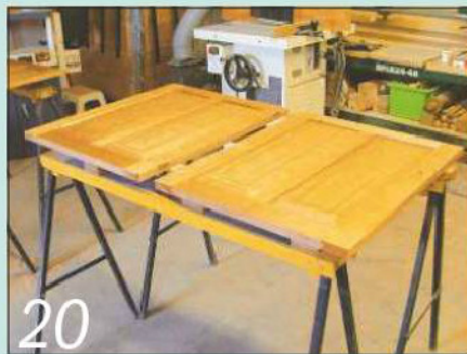
20 Remove the doors so they can be sprayed with a couple of coats of pre-catalysed lacquer
