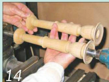
14 Use the first turned column as a pattern to check that the others match its profile
