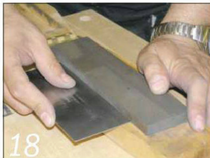
After filing the scraper edge, polish it on the edge of a stone
