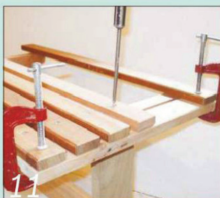
11 Fit the outer slats first, then cramp a batten beneath them to help align the ends of the rest
