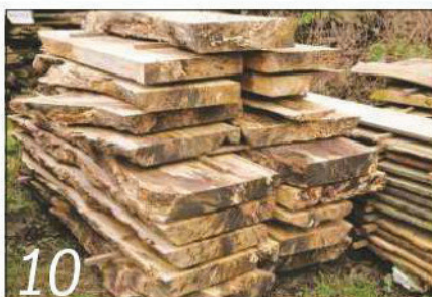
Converted wood is also at risk if it's kept in adverse drying conditions
