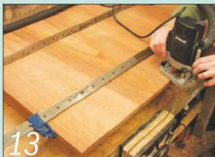
13 Release the slats, cramp them together and use a router to round over the slat edges
