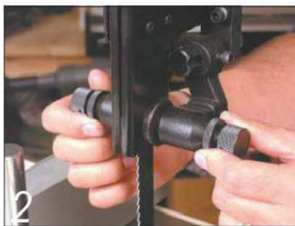
2 Likewise the side guides can differ. The cast discs on this bandsaw should be kept fractionally away from the blade
