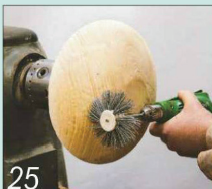
25 Once bleaching is complete, finish off with the nylon abrasive brush to flatten the raised grain
