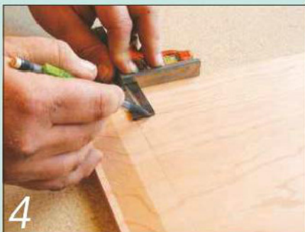
4 Mark the position of the inlay on the various raised panels with a fine pencil line
