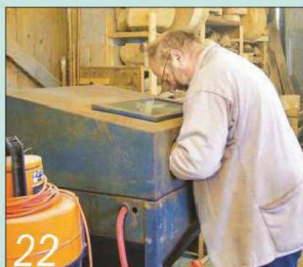
22 I can view the workpiece through the window on top of the cabinet as I manipulate it
