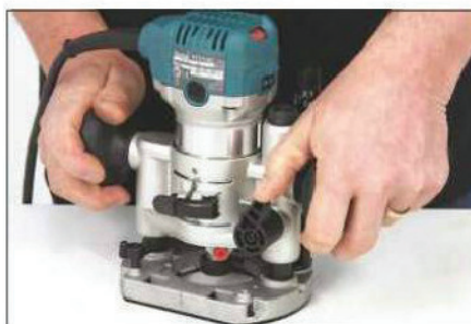
12 The plunge lock is a bit on the short side and can be awkward to reach
