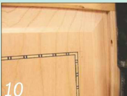
10 Glue the inlay strips into their grooves and finish them flush with a cabinet scraper
