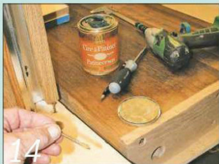
14 The maple faces are screwed in place. I put wax on the screw threads to help create a tight joint
