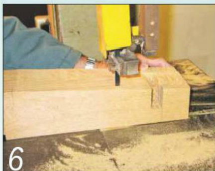
6 Cut the taper on the bandsaw, working just outside the marked line
