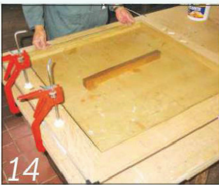
14 Mitre the corners, dry-assemble the frame and check that the glass fits
