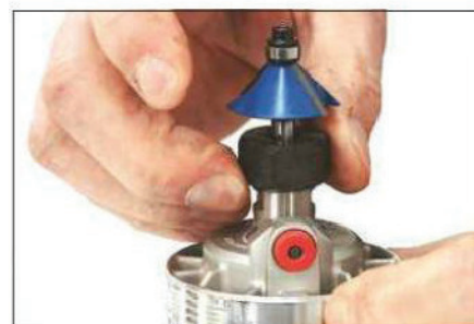
4 The integral spindle lock means you need only one spanner for the job
