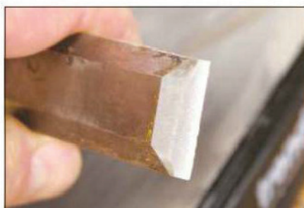
...but the nick disappeared after only a few seconds on the coarse stone
