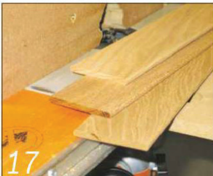
17 Machine both edges of an offcut to make the beading, then cut it to width
