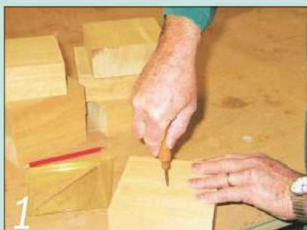
1 Start at the bottom by finding and marking the centre of each base block
