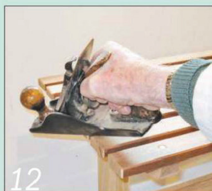
12 Trim the ends of the slats to the same angle with a sharp smoothing plane
