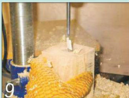
9 Centre-bore a 25mm diameter hole in the lower section of each column on the pillar drill
