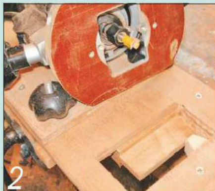
2 I use this simple router jig to cut all the tenons accurately to size
