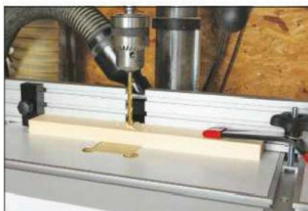
The fence incorporates a large length stop and a dust extraction hood
