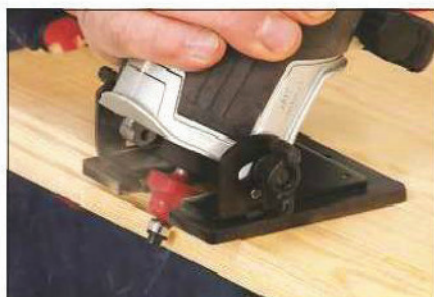
14 The clever tilting base opens up a whole new world of unusual edge profiles
