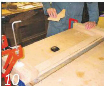
10 Dry-assemble one end of the table and cut a template for the shelf corner
