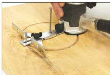
8 The straight guide can also be used as a trammel for cutting small circles
