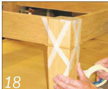
18 Glue the leg beads into their grooves and secure them with masking tape
