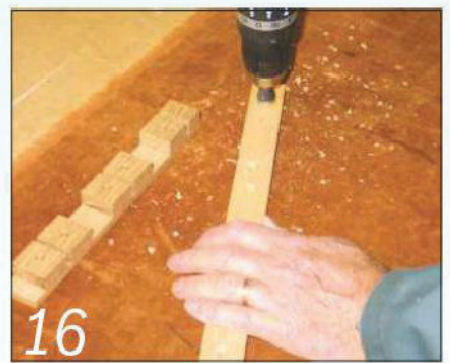
16 Shape and drill the buttons in a strip before cutting them off to length
