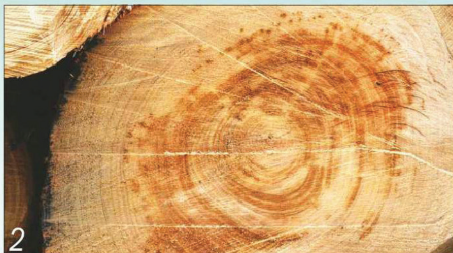
2 The earliest stage of rot infestation usually causes some form of staining
