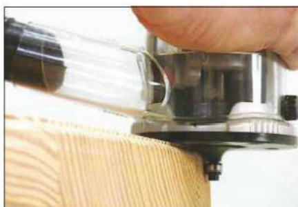
6 The dust extract spout is not brilliant at collecting dust from below the base
