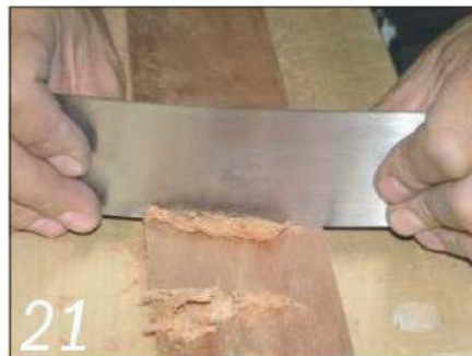
Get it right and you should be taking light shavings, just like a fine-set plane
