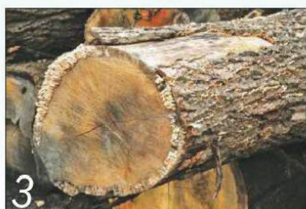
3 Some wood-destroying fungi colonise logs only after they have been felled
