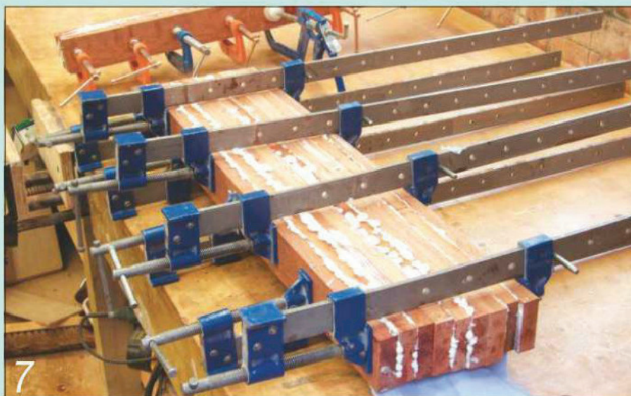
7 I made the legs by laminating together three pieces of thinner stock
