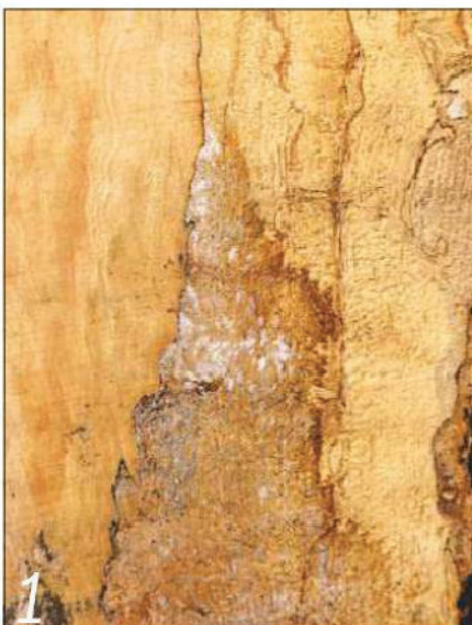
1 Moulds affect only the surface, while stains penetrate more deeply
