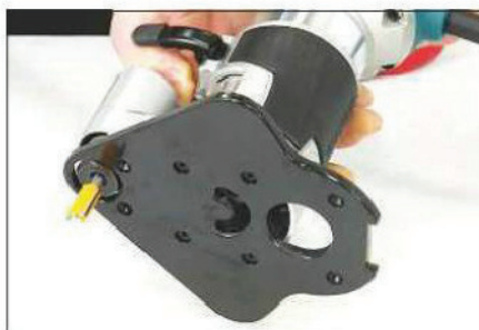
15 The offset base allows the cutter to be fitted very close to the edge...
