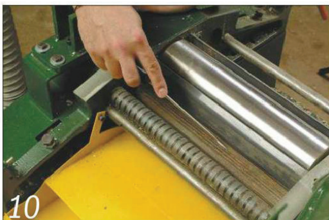
10 General maintenance of all your cutting machinery should involve locating and cleaning off resin build-ups
