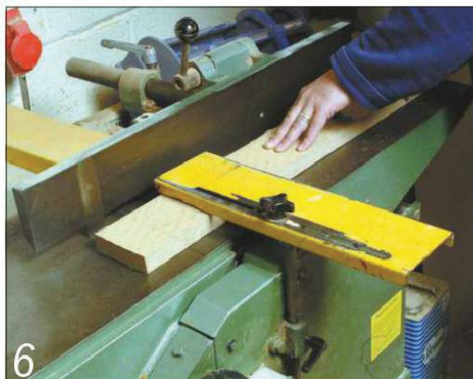
6 Ensuring that the bridge guard is correctly set for face and edge planing helps to keep things safe
