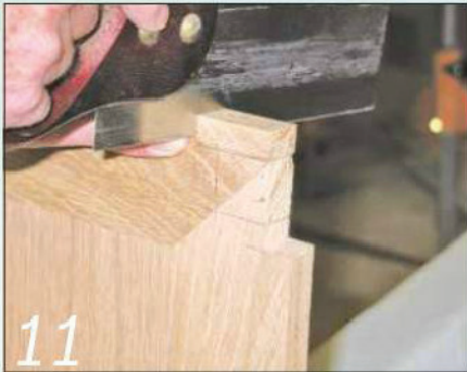
11 Use the template to mark out the shelf corner profiles and cut them with care
