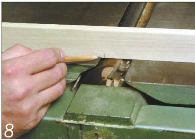
8 A couple of marks on a batten will act as a setting gauge for knife swaps, as explained in the text
