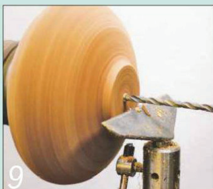
9 Use a twist drill held to bore into the top of the vessel to the correct depth
