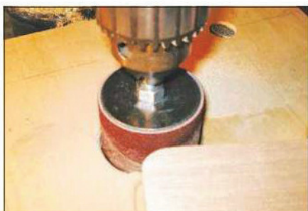
The drum can be raised and lowered through the opening so its entire surface is used
