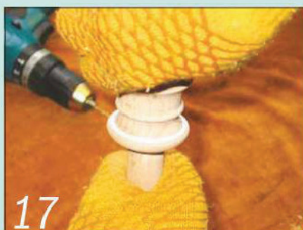
17 ...and screw the two columns together tightly. Easy-grip gloves are a big help here!
