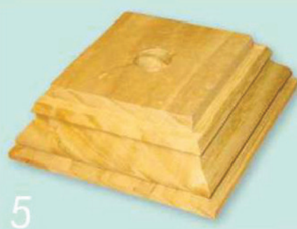
The four moulding cuts were completed with the minimum of breakout on the arrises
