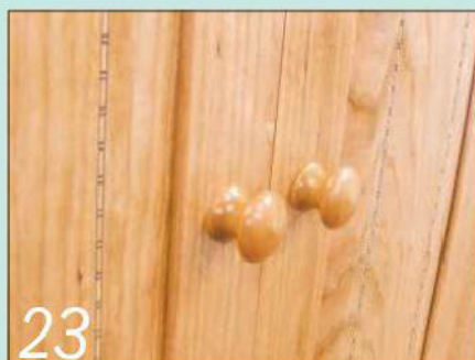
23 I turned a set of eight matching knobs and dowel-jointed them to the cabinet doors
