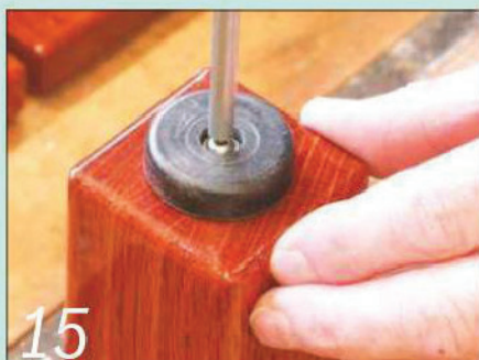
15 Attach a rubber foot to the bottom of each leg for extra protection against damp and rot
