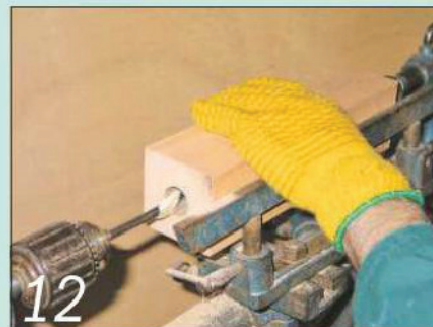
12 Mount the longer sections on the lathe to bore the hole for the candle
