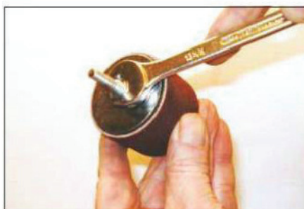
The sleeves are gripped by tightening a nut on the shank of the drum with a small spanner
