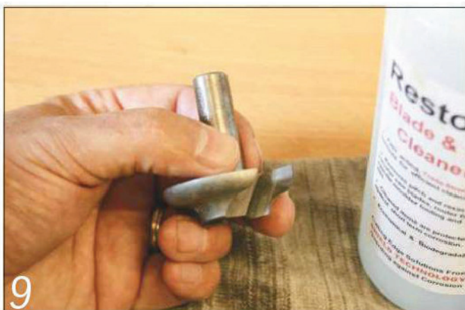
9 Resin build-up on router cutters, planer knives and saw blades should be removed regularly with a dedicated cleaner
