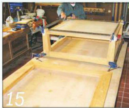
15 Assemble the sub-frame upside down. The top frame is in the foreground
