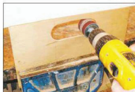
The drums can be used freehand for all sorts of internal sanding jobs
