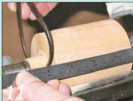
11 Turn the spigot and check its size before starting the rest of the shaping
