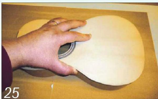
25 Sand the bottom linings flush with the ribs and the neck and tail blocks
