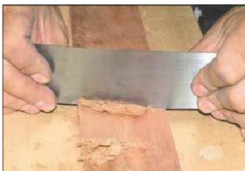
1 The success of a scraper depends on blade curvature as well as the cutting angle
