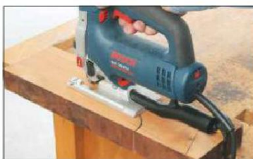
2 A jigsaw with a sharp blade should cut through thick hardwood with reasonable accuracy. Cut just clear of the line to allow for cleaning up
