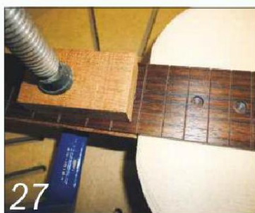
27 Accurately align the twelfth fret slot with the perimeter of the instrument's body
