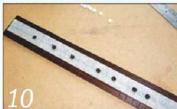
10 Drill blind holes for the dots, using a pillar drill fitted with a depth stop
