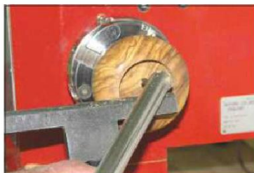
4 Reverse the body onto an expanding chuck and start hollowing it out
