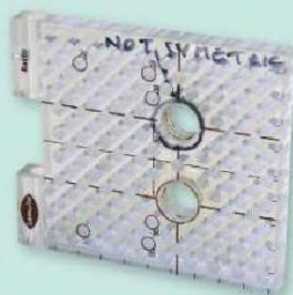
5 I discovered the hard way that one of the bush mounting holes is not symmetrical to the pin holes
