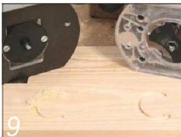
Dust extraction is much improved using the modified guide bush (right)
