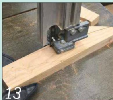
13 Remove the template and rough-cut the supports a little larger than their final size
