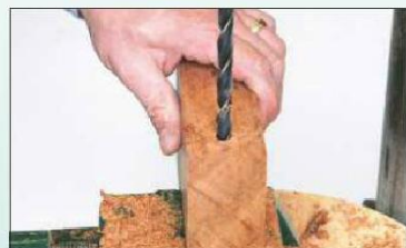
7 The hole for the axle in the front wheel support is much shorter, and I managed to drill it using a long 10mm bit. Back the drill out regularly to clear the waste; otherwise it gets pushed off-line
