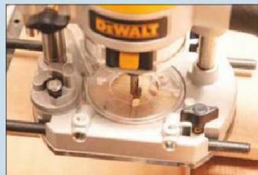
4 The left T-bolt that attaches the fence goes through a routed slot
