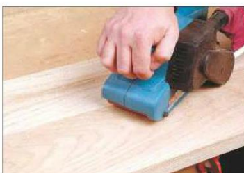
2 Skewing a belt sander gives faster stock removal when cleaning up jointed work
