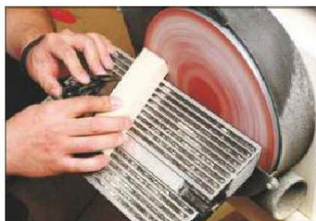
8 ...while the disc and its work table allows precise finishing of components such as mitres
