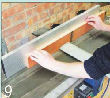
9 Plane the two supports flat and square one edge, then cut them to length
