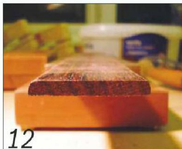
12 To improve player comfort, round over the top corner on each side of the fingerboard
