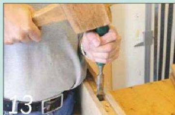
13 Mark out the position of the muntin and cut its mortises and tenons in the door rails
