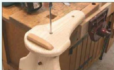
28 I rounded over all the edges to save weight. The seat and rear axle support are screwed to the central strut; plugs fill the counterbores
