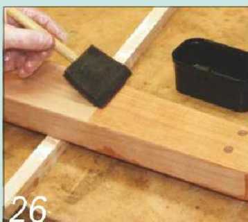
26 Apply the finish to the shelf and the supports. I used three coats of hardwax oil
