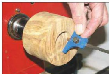
2 Hollow out the recess to a depth of 10mm and check the measurement
