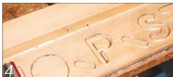
4 Cramp the template to the workpiece with its top edge butted against a thin timber batten
