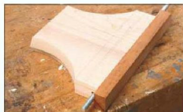
6 I decided to cap this slot with a piece of contrasting timber, working on the principle that if you can't conceal it, make a feature of it!
