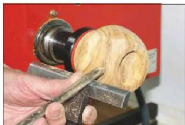
3 Shape the outside of the pincushion body using a small bowl gouge
