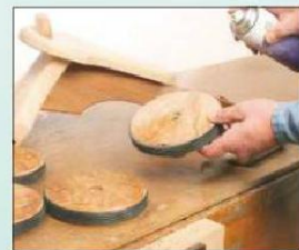
33 Apply several thin coats, then reassemble the trike. Glue the top half of the steering pin into the handlebars and re-fit the wheels
