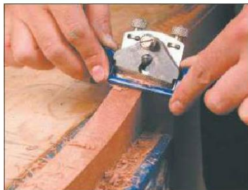
3 Set finely, the spokeshave works fantastically well for cleaning up curved work
