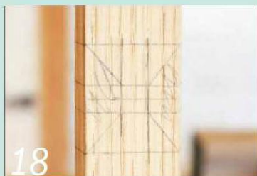
18 After marking the cross-halving joint on the glazing bead, I decided to make some trial cuts
