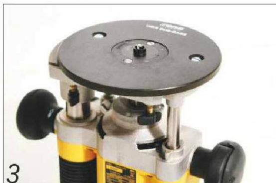
3 If your router has a non-Trend base configuration, you might need the Trend circular sub-base
