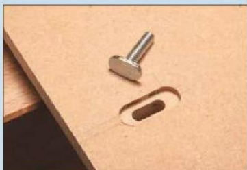
5 The routed and counter-bored slot for the T-bolt allows adjustment of the lateral guide rail
