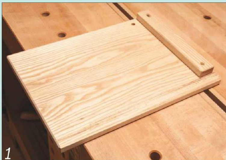
1 The traditional design of bench hook can be used either way up as the cleats are identical
