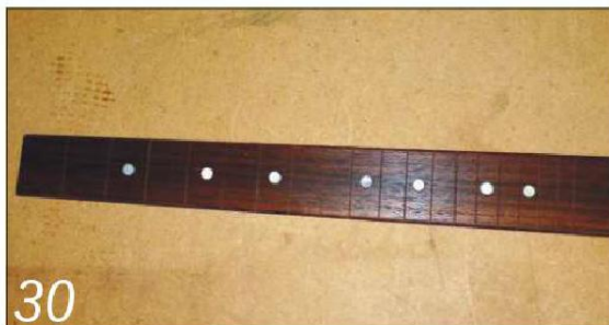
30 Sand the dots flush with the surface of the fingerboard, working down to 400 grit
