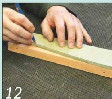
12 Pin the mantel support template to each blank in turn and draw round it
