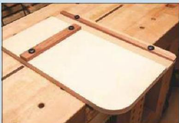
3 I used four thumbscrews to attach the fence and the lateral support to the baseboard
