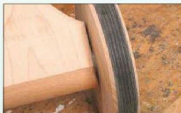
29 Fit a nylon washer between each wheel and the axle support to maintain a small gap and reduce friction between the two components
