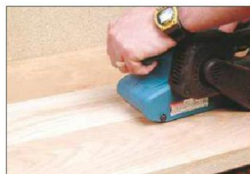
3 The sander should then be straightened up to remove any cross-grain scratching
