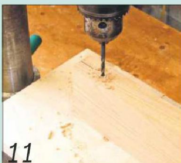
11 Prevent the drill bit from drifting by drilling the holes from opposite sides
