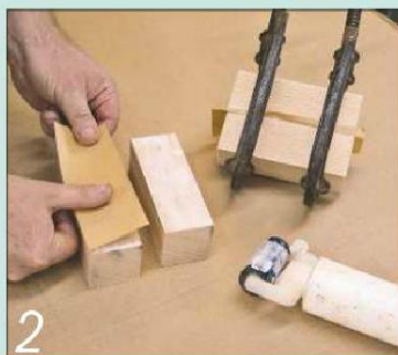
2 Glue and cramp the components together in pairs using paper joints
