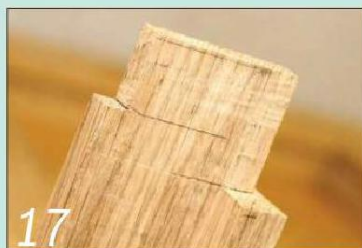
17 I used a fine Japanese saw to cut the tenons on the ends of the glazing bars
