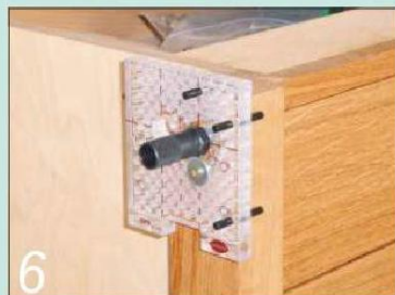
6 For the first hole I fitted three pins to locate the jig, and then screwed it in place to ensure that the drill didn't move the jig as it began to cut
