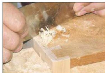
2 A sharp scraper will cope equally well with end grain and wild or interlocked areas
