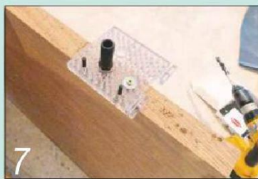
7 The remaining holes still had to be drilled following pencil lines, but at least I could guarantee that they were all equidistant from the edge
