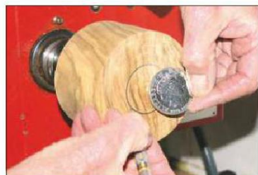
1 Turn the blank to a cylinder, face it off and mark the recess for the coin
