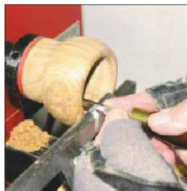
9 Reposition the toolrest and cut through the inside edge of the recess with a parting tool
