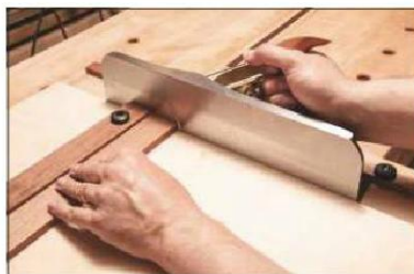
The skewed iron removes the finest wood shavings with surgical precision
