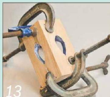
13 Glue the four pieces back together, taking care to keep glue away from the interior
