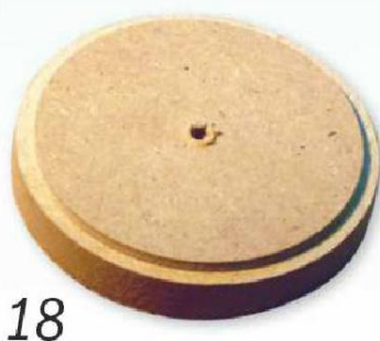
Turn an mdf clamping caul to fit in the soundhole and use it to secure the soundboard to the solera
