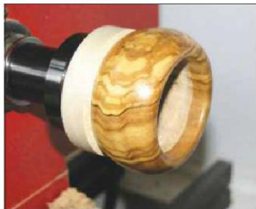
13 Make a jam chuck to hold the ring so you can apply the finish; I used friction polish
