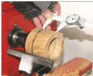
6 Mark a pencil line all round the blank, 40mm from the front face
