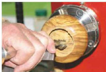
5 Cut back the interior to a gentle curve underneath the rim of the bowl
