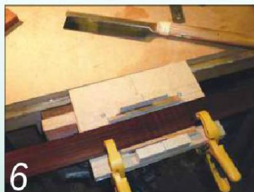
6 The fingerboard must be firmly clamped into the jig. If it moves, it will be ruined
