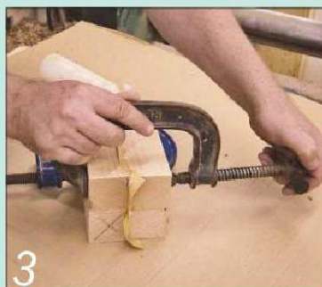
3 Clean up the glue joints and stick the two pairs of blocks together with more paper joints
