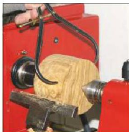
3 Turn the blank to a diameter of 85mm and check the size with callipers
