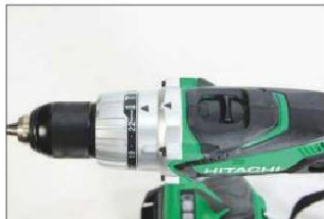
The 22-position torque control and gearbox selector are located on the top of the body
