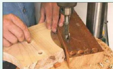
9 The rear axle support and central strut are simply screwed together, so again I made a feature of this by counterboring the holes and fitting contrasting plugs cut from some scrap material
