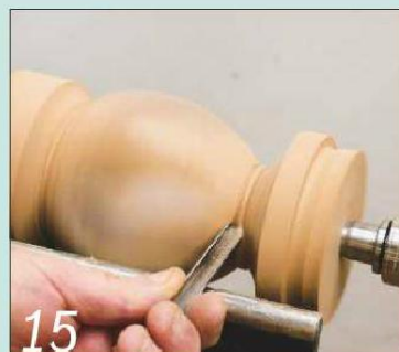
15 I cut a bead for decoration where the foot and the main body meet...
