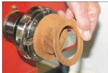
5 Turn a ring for the top of the drum, and a base with a centre spigot
