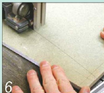
6 Rough-cut the two templates to size on the bandsaw, working close to the marked lines
