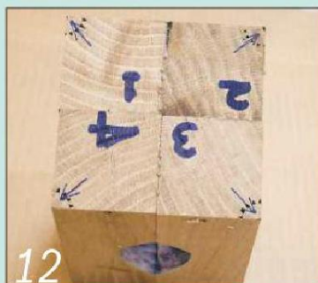
12 Separate the four blocks and rearrange them with the arrows pointing outwards
