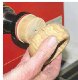
11 Turn a plug insert on the stub of the blank and test its fit inside the ring
