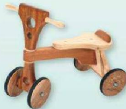
31 All that remains is to give all the surfaces a final sanding and to make sure there are no remaining sharp edges
