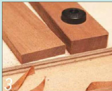
3 Its now clean-cut end is the outcome of being shot with a sharp plane
