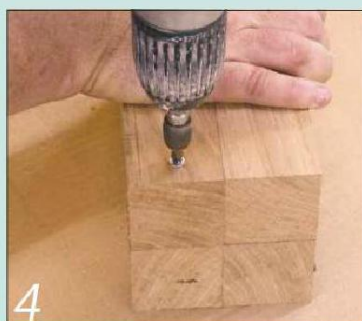
4 You can use screws and over-long blocks as an alternative to using paper joints
