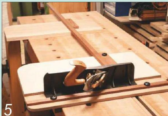
5 The workpiece rests across shooting board and bench hook simultaneously
