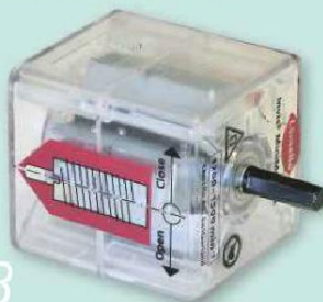
3 The MiniMag has a revolving magnet which turns the threaded stud. It needs to run at 1200 to 1500 rpm, not at the 120rpm given on page 347 of the Axminster catalogue!
