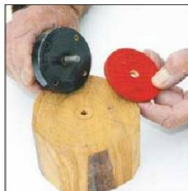
1 I use a 6mm thick plywood spacer with my screwchuck to protect it
