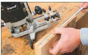
5 For the rear wheel support I didn't think I could drill the very long hole for the back axle accurately enough, so I routed a slot deep enough to take the piece of 10mm studding for the axle
