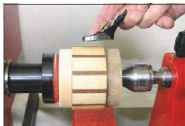
4 Use a small plane and abrasive paper to finish the strips flush with the drum
