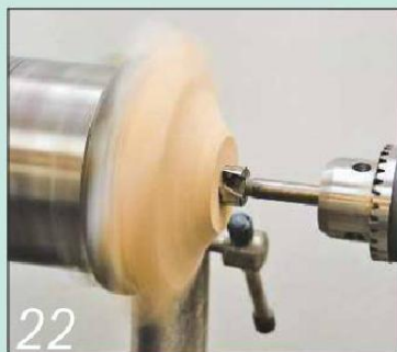
22 Reverse the top onto a jam chuck and drill a hole to accept the spigot on the body
