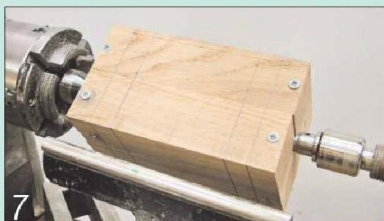
7 Mount the blank between centres and mark the inner section that won't be turned. The outer pair of lines show where the fixing screws are
