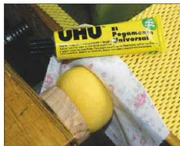
12 Make up the cushion, stick it to the plug insert and clamp it lightly
