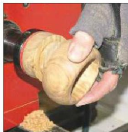
10 The ring will separate from the waste wood when the two cuts meet. Be ready to catch it!
