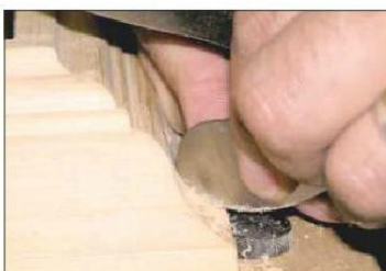
3 Gooseneck and other shaped scrapers earn their keep for cleaning up mouldings
