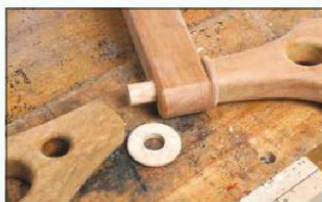
27 The steering components and the central strut didn't meet perfectly, so I turned a couple of large wooden washers in contrasting timber
