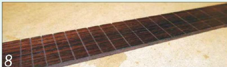
8 You should end up with a series of parallel slots, all precisely 1mm deep
