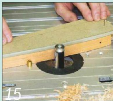
15 ...and trim it accurately to shape along its long edge. Don't trim the corners yet
