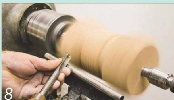
8 Use a spindle gouge to cut the shape in between the inner pair of lines. I'm cutting an eccentric cove
