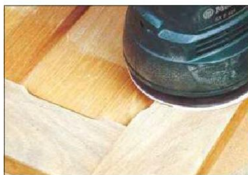
6 The random orbit sander can tackle large flat areas and smaller clean-up tasks
