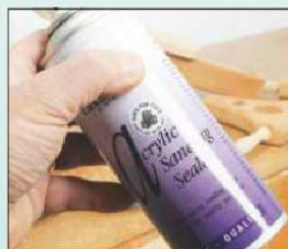
32 I used an acrylic spray lacquer over a sanding sealer. This finish complies with the EN71 European standard for toy safety
