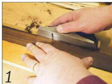
1 Plane one side of the thickened fingerboard blank true and square with a sharp plane
