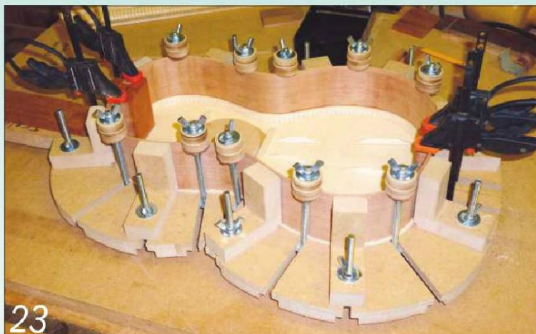
23 Use long cramps to hold the ribs tightly against the soundboard. Leave the assembly to set overnight
