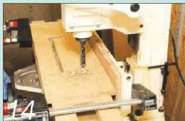
14 I cut the letterbox opening at this stage, using the mortiser and then a bearing-guided router bit
