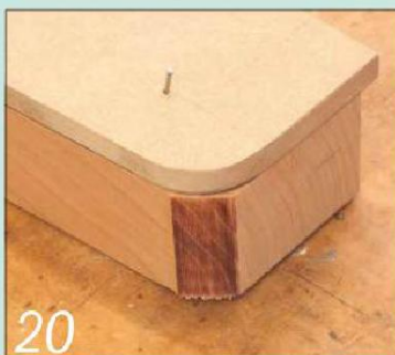
20 As before, leave the end-grain corners and shape them using the belt sander
