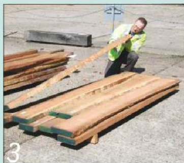
3 Select a suitable piece of 50mm thick cherry from the timber yard's stock for the mantelshef
