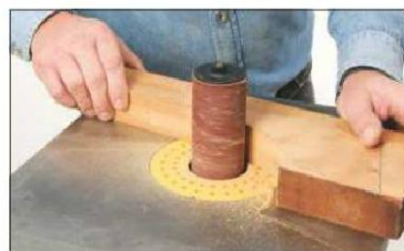
3 Take your time to sand the strut back gently to the marked line using the bobbin sander. Try to maintain the smooth flowing curve
