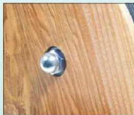
30 Cap nuts and washers provide a secure fixing for the wheels. Fix them with a touch of epoxy glue when you've applied the finish
