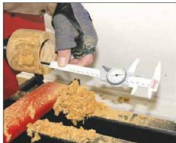
5 Check that the drilled-out recess is the right size by using a depth gauge
