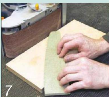
7 Then use the belt sander to finish the curved edges back to the marked line
