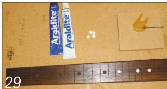
29 Stick the dots in place in their blind holes with epoxy resin adhesive
