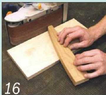
16 To avoid cutter snatch, sand the rough-cut corners to shape on the belt sander
