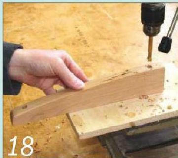
18 Drill counterbores big enough to accept the heads of the fixing screws
