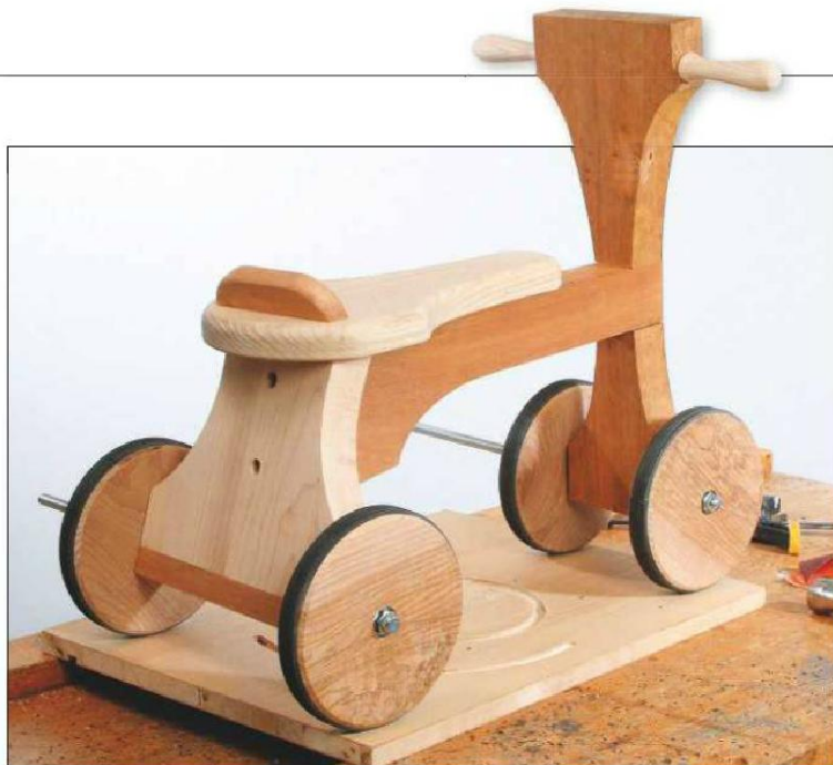
25 A trial assembly showed that everything worked. However, the trike was rather on the heavy side, both in appearance and in weight, and needed to be made lighter in some way
