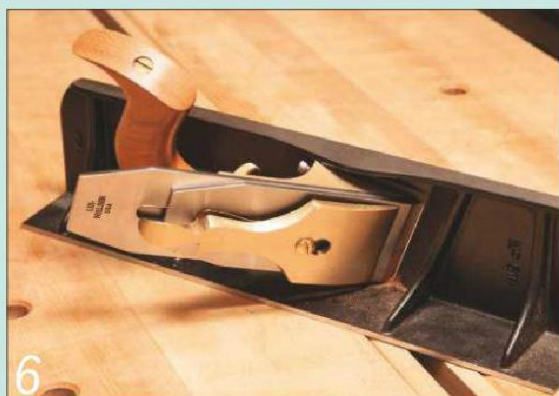
6 The shooting board can't be reversed for use with a Lie-Nielsen No.51 plane
