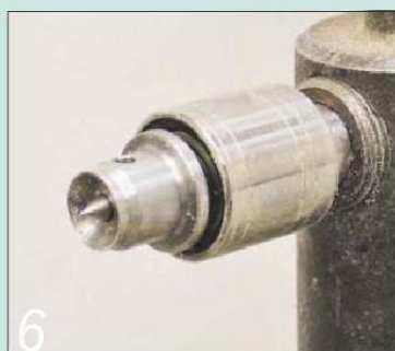
6 With paper joints, use a cup centre rather than a revolving centre to avoid forcing the joints apart
