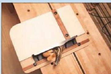
1 The shooting board has a running rebate and a lateral guide rail for the plane
