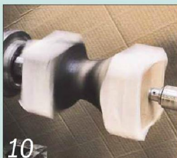
10 Mask off the parts you don't want to paint and spray on ebonising lacquer
