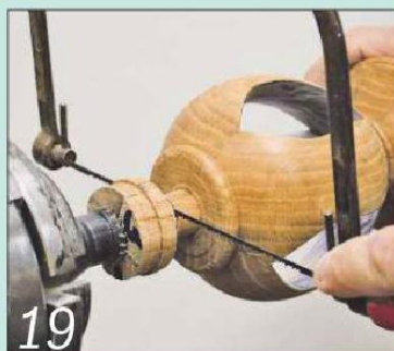
19 Cut off the waste from the top spigot and set the candlestick body aside
