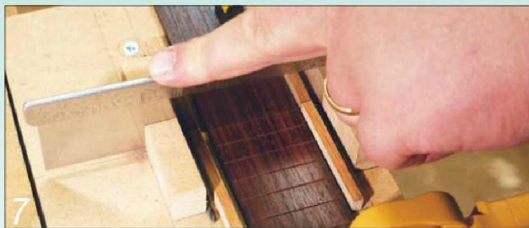
7 I use a Japanese pull-saw with minimal pressure to cut the fret slots
