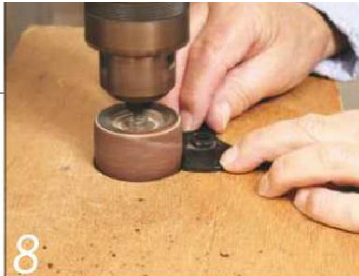
Sand away both sides of the flange to allow the dust to pass through the gaps
