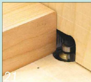
21 Round over the shaped edges of the shelf using the router table
