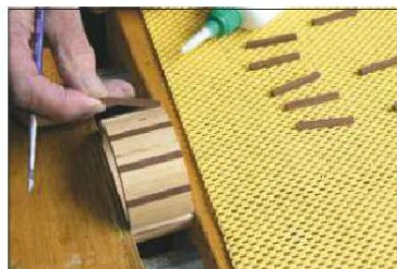
3 Hold the fluted drum in a vice and glue in the 4 x 4mm inlay strips
