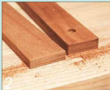
2 This rough-cut end has just been sawn by hand using a bench hook
