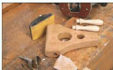
26 I achieved this by drilling large holes through the front axle support and the handlebar assembly and then rounding over the edges
