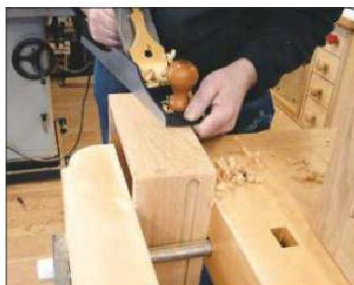
1 A traditional handplane will do the majority of cleaning up where necessary...
