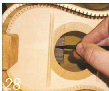
28 Scribe the curve of the soundhole on the back of the fingerboard, ready to be cut along the line
