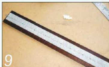
9 Stick masking tape to the fingerboard and mark the centre line; then centre-punch the dot positions
