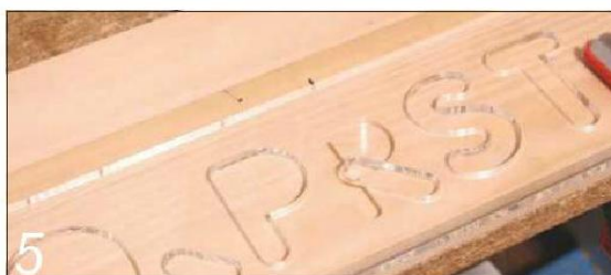
5 O and P are turned into Q and R with the diagonal tails on the template
