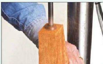
8 Use the pillar drill again to make the 22mm hole for the steering pin in the front wheel support and the handlebar sections. The latter was drilled at an angle of about 5° so it leans back slightly on the finished trike
