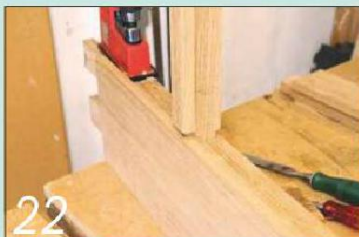
22 I could then check that the assembled bars fitted correctly within the door's frame
