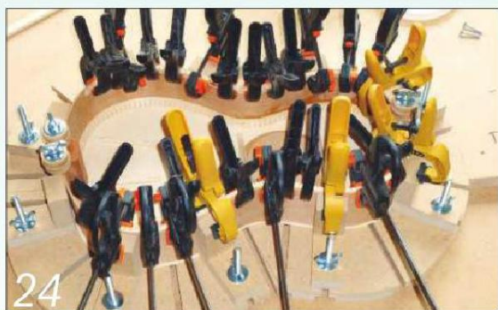
24 Remove the neck. Prepare and fit the bottom linings that will hold the back on
