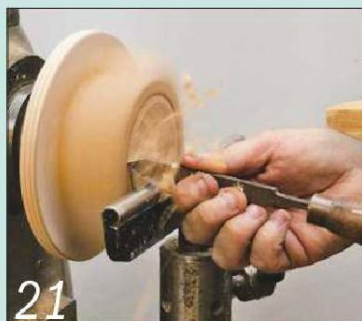
21 Remove the tailstock support and turn a recess in the top for the candle
