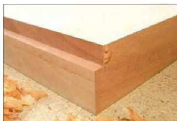
End-grain rebates are cut cleanly with the minimum of breakout.
