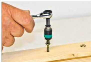
The bit holder collar can be held with your free hand to help steady the screwdriving operation
