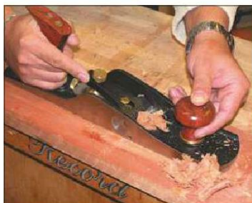
2 ...but for wild and interlocked grain, a low-angle bevel-up plane gives better results
