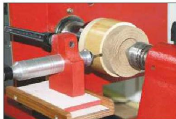
1 Turn a hollow drum, plug its ends and set up the fluting jig in the tool rest holder alongside it
