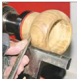
8 Reduce the diameter of the blank next to the headstock and shape the curved section
