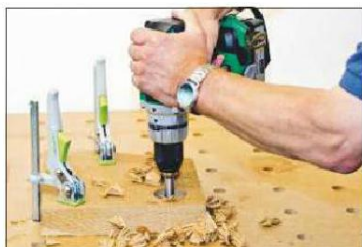
The huge torque means that two hands are needed with this big Forstner bit
