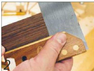
2 Cut one end square to the planed side to form the edge of the nut housing
