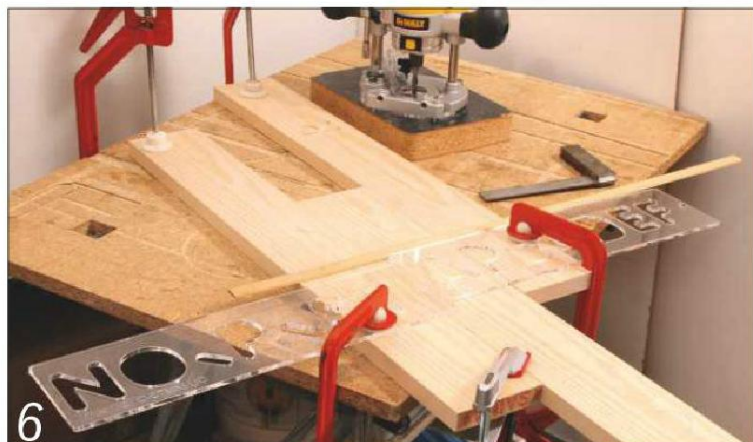
6 This simple bench set-up makes it easy to produce a vertically cut sign on the centre board
