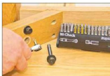
A No 3 Pozidriv bit is ideal for tightening up the fixing bolts on this kitchen table
