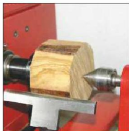
2 Mount the chuck in the headstock and bring up the tailstock for support
