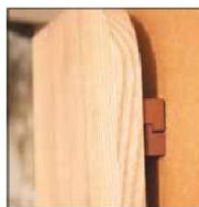
Matching cleats allow both aids to hang vertically on the wall or bench end for storage
