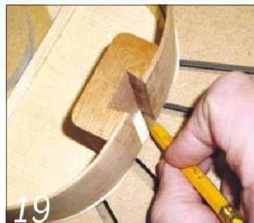
Place the body on the soundboard and mark the position of the dovetail socket on it
