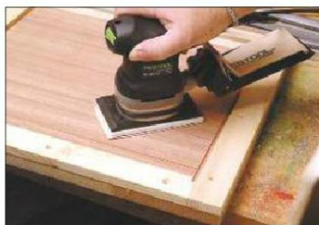
5 Standard orbital sanders are perfect fine finish sanders for flat, square surfaces
