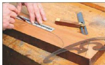
1 I started with the central strut component, setting out a curve that maintains the strength but minimises the weight as much as possible
