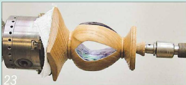
23 Stick the top and body together, using tailstock pressure as a cramp while the glue sets
