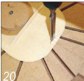
Cut out the waste area with a sharp chisel so you can remove and refit the neck later
