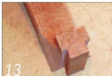
13 Cut the dovetail pin on the end of the neck marginally oversize...
