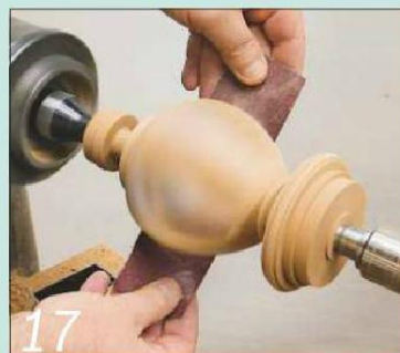
17 Sand and polish the outside. I do this with a long strip of abrasive paper
