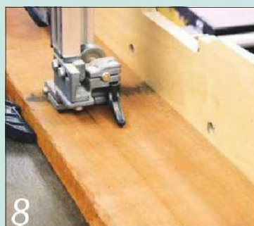
8 Rip the mantel support blanks to their approximate width on the bandsaw
