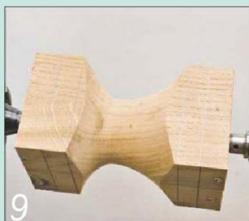
9 Leave the rest of the blank square, then sand the cove smooth
