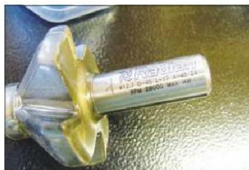
Each cutter shank carries the K mark and vital operating information
