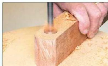
4 The 22mm hole for the steering pin must be drilled dead square, so use a drill press and keep clearing the bit to prevent it binding
