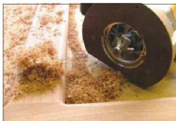
The roundover cutters create smoothly flowing edges on a frame
