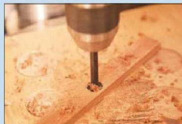
6 Counter-bore holes for the thumbscrew collars to keep them as low as possible on the rails
