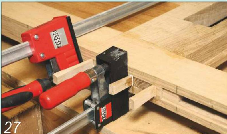
27 Leave all the wedges proud until the glue has cured; then trim off the excess
