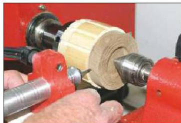
2 Use the lathe's indexing system to cut 12 equally-spaced grooves around the drum
