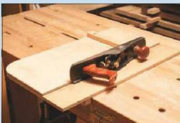
7 I designed this version of my shooting board for a Veritas low-angle jack plane
