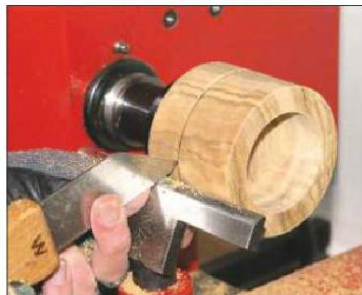
7 Use a thin parting tool to make a cut at this point to a depth of 20mm
