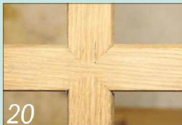
20 The second effort was better but still not perfect. Poor marking-out was at fault this time
