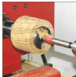
4 Fit a chuck and Forstner bit in the tailstock and drill out the recess to a depth of 35mm
