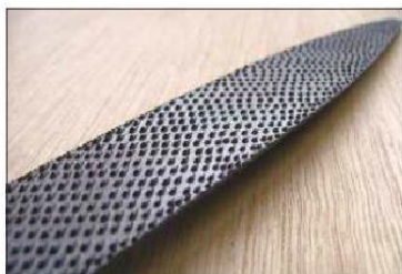
Unlike machine-made rasps, the stitching extends right to the edges of the blade
