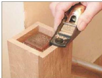
2 Block planes are also useful for cleaning up end grain and working on narrow stock
