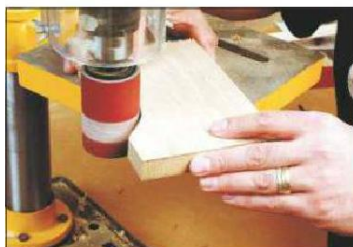
9 A sanding drum fitted in a drill press is a low-cost alternative to a bobbin sander
