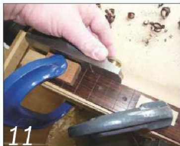
11 Plane each edge of the fingerboard down to a knife-line to form a gradual tapered shape
