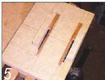
5 I use a tailor-made mitre box for cutting fret slots, with twist drills as depth stops
