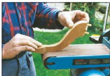
7 The belt on a static belt and disc sander is the perfect choice for cleaning up curves...
