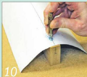
10 Use the paper rubbings to mark the fixing hole positions on the support blanks
