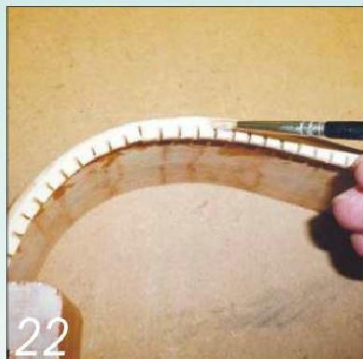
22 Apply glue to the top linings and the top edge of the ribs; keep it well away from the dovetail
