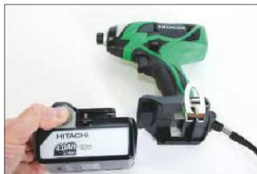
The 4.0Ah batteries use the new Hitachi standard slide-in fitting
