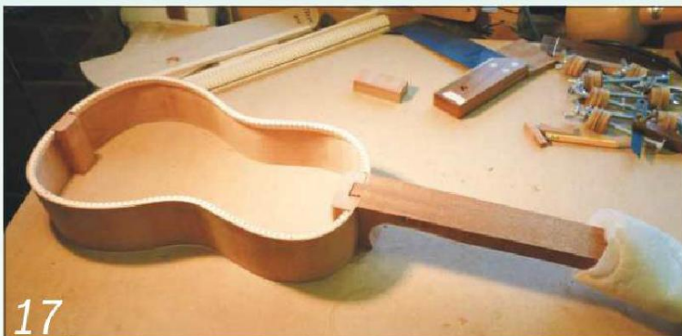
Shave the pin carefully until it's a tight sliding fit in the neck block
