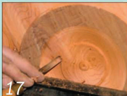
17 Then slowly remove the centre area to form the recessed inner hollow
