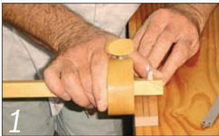
1 Scribe the outline of the two blade recesses on the wood with a sharp cutting gauge
