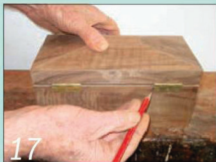
17 Place the hinged lid on the base and mark the hinge leaf positions on it
