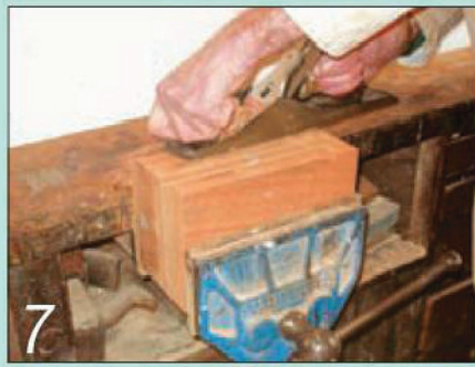
7 Once the box is out of the cramps, plane off the excess to the sides and ends by hand
