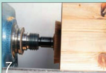
7 Form a dovetail spigot to fit the chuck using a gouge and skew chisel
