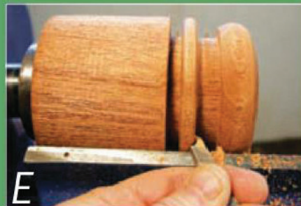
The second scraper is used to cut the other side
