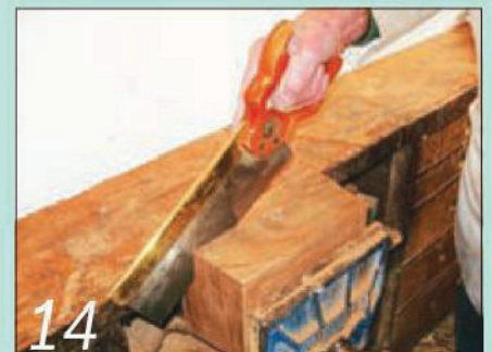
14 Mark the cutting line and use a tenon saw to separate the lid from the lower part
