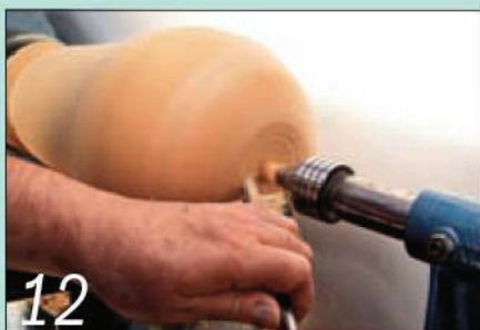
12 Use a small bowl gouge to form the shallow recess in the fat end
