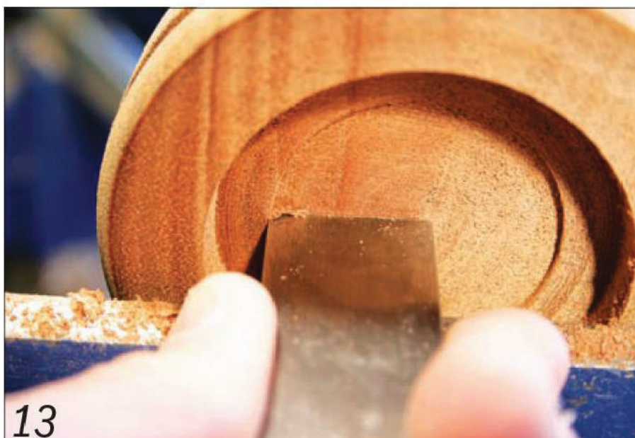
13 Move the scraper laterally across the box floor, cutting a millimetre at a time
