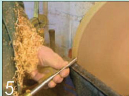
5 Start by truing up the edge of the blank with a freshly sharpened bowl gouge
