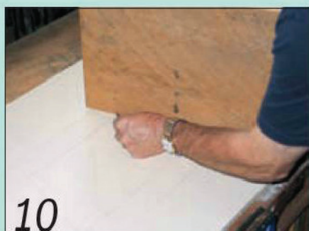
10 A full-size drawing allows you to take dimensions straight off it onto the components
