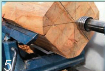
5 The banjo now slipped further under the block so I could remove more wood
