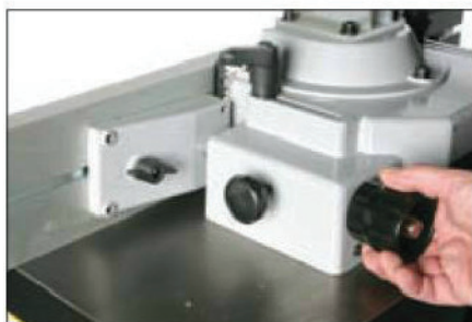
The two components of the fence are independently adjustable
