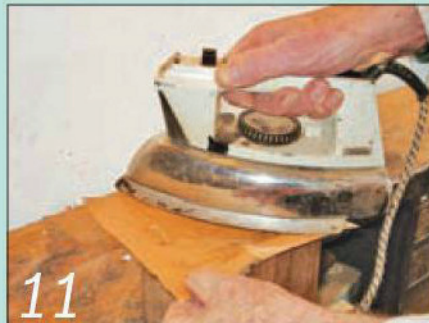
11 Position the veneer, protect it with brown paper and iron over it to bond it in place
