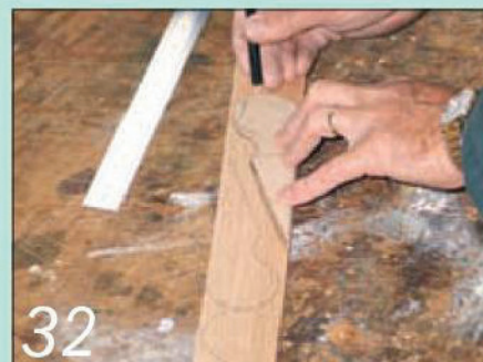
32 Make a template for the wedges and mark them out on some 25mm thick oak scrap
