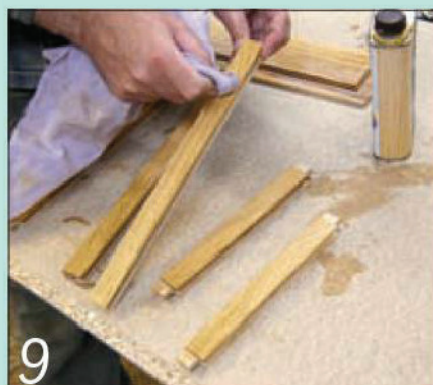
9 Apply a suitable finish before gluing the side panels together
