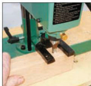
Small mortises can be cut very quickly, even in dense hardwoods
