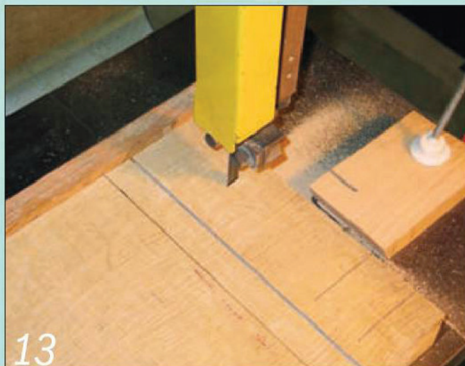
13 Cut the cheeks of the twin tenons part of the way on the bandsaw
