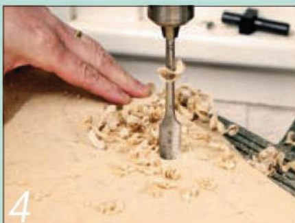
4 Drill the holes with a flat wood bit; a cheap one will probably drill slightly over-size
