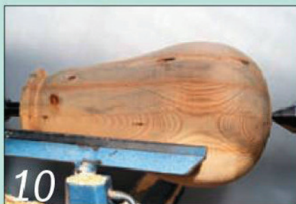
10 As you work towards the narrow end, stop short of the spigot
