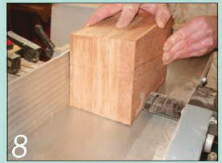
8 Form the taper to the sides on the surface planer. Tackle the ends first
