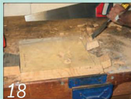
...and use a wide chisel to trim away the waste to the line on the other cheek
