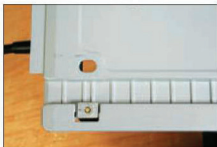
The fine adjusters under the baseplate ensure a good fit on the guide rail
