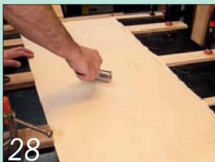
28 Align the 28 tambours, cramp them down on the bench and glue the canvas to their backs
