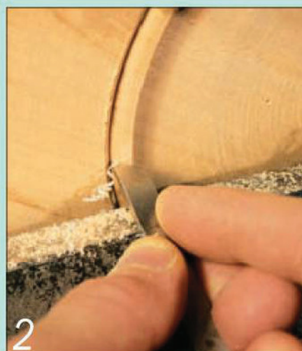
2 This skew chisel is being used on its side to form a bead round a tile recess
