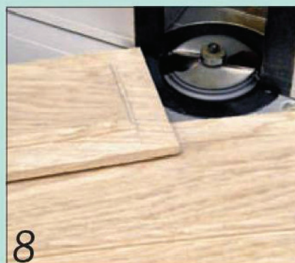
8 Select a panel cutter and field the panels so they'll fit in the grooves
