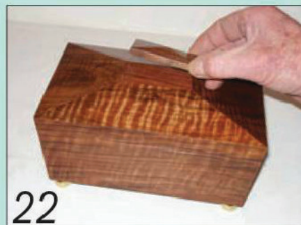
22 ...before positioning the solid walnut capping piece on the top of the lid
