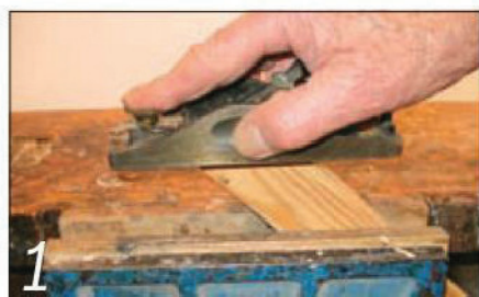
1 A block plane is ideal for end-grain jobs such as trimming mitres
