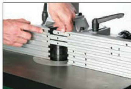
These slot-in fingers link the fence halves and close up any gaps around the cutter block
