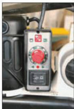
The control panel governs feed speed and direction of travel
