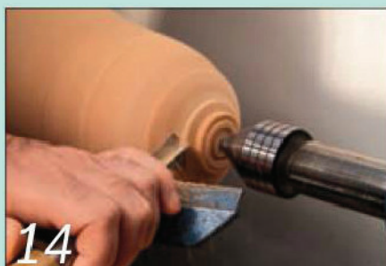
14 Remount the pear and continue shaping the thin end as far as possible
