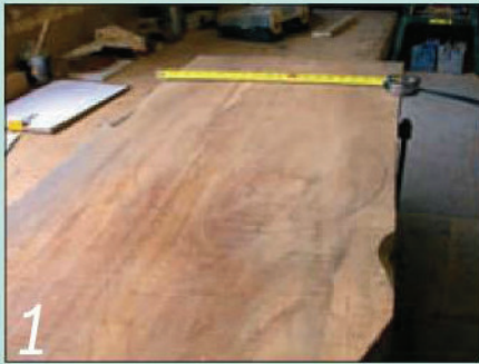
1 First steps; marking out a series of 350mm diameter circles on the yew board
