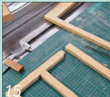
15 The door assembly mimics that of the rear frame, with a central muntin
