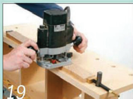
19 A Wonder Pup and a fixed dog act as a tail vice for holding longer workpieces
