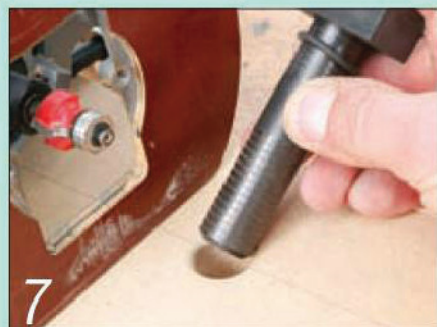
7 This will provide a neat lead-in that makes locating the dogs quicker and easier
