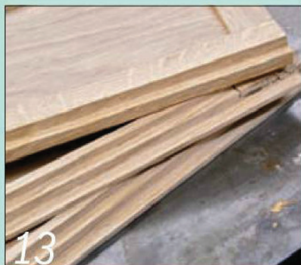
13 Cut rebates so you can join the four sides of the cabinet together
