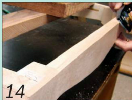
14 When you've assembled the plinth, plane an edge chamfer all round to fit the base unit
