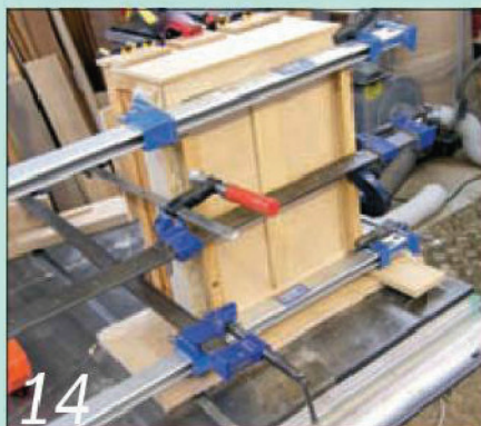
14 Fit the top and base panels to keep everything square, cramp up and leave to dry
