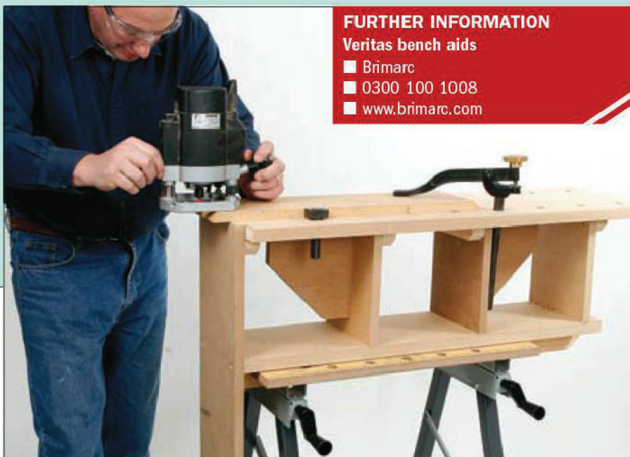
17 Two fixed dogs and an adjustable Wonder Pup are ideal for holding round work
