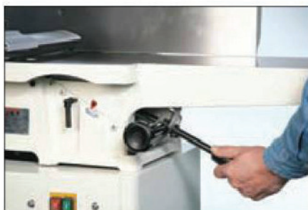
Depth-of-cut adjustment is by means of a lever you move and then rotate
