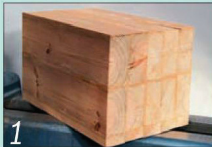
1 Use a good quality PVA adhesive to glue the pieces of softwood together
