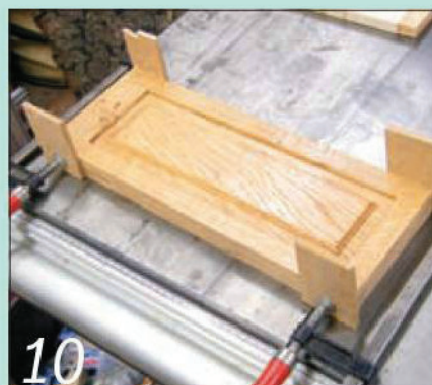
10 Glue and cramp the frames together and compare diagonals to check they're square
