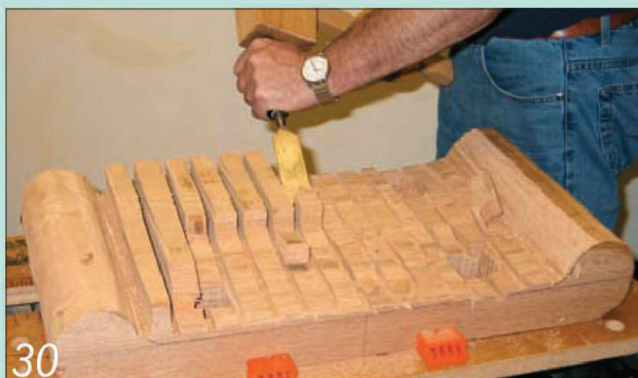
30 Create relief cuts with the chainsaw and chop out the waste with a wide chisel and mallet
