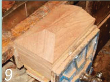
9 Form the slopes to the end of the top entirely by hand planing
