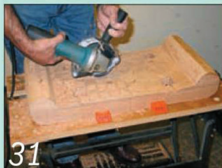
31 I used an Arbortech attachment in my disc cutter to give the seats a rustic finish
