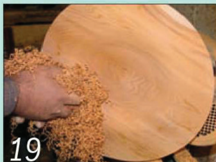
19 Sand the face as you did for the underside, then burnish it with yew shavings
