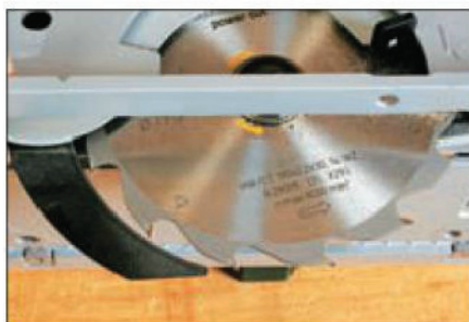
The riving knife supplied with this saw is essential for ripping solid wood
