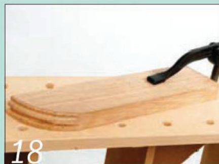
18 A hold-down and a fixed dog (out of sight) anchor flat workpieces in place
