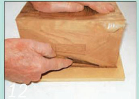
12 Remove excess veneer from all the edges with a sharp knife or scalpel
