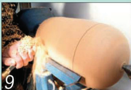
9 The spindle roughing gouge removes waste wood fairly quickly
