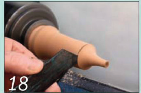
18 Part it off close to the widest point using a narrow parting tool
