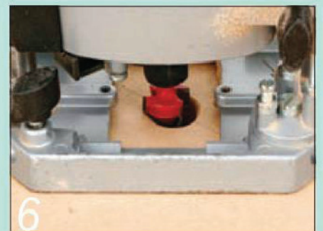
6 ...so run round each one with a small bearing-guided radius or chamfer bit
