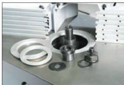
A series of inserts allows you to step down the 200mm table opening
