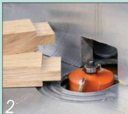
2 Use a bearing-guided rebate cutter to make accurate tenons
