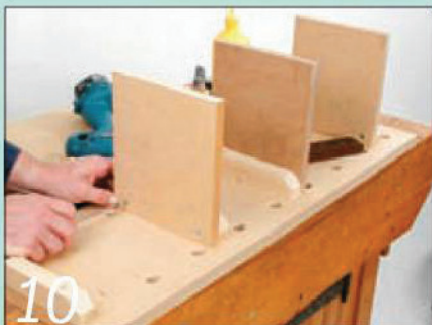
10 Then glue and screw the uprights to the battens, not the other way round
