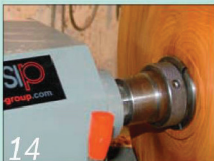
14 ...and mount the chuck on the lathe, ready for the platter's face to be turned
