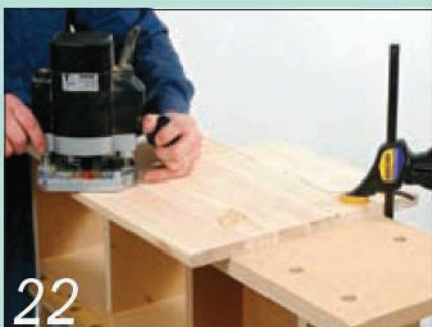
22 ...that allows you to use cramps to secure workpieces you can't hold in any other way
