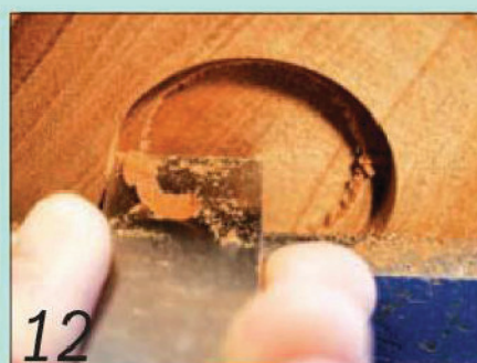
12 To hollow out a recess, move the tool straight into the face of the work
