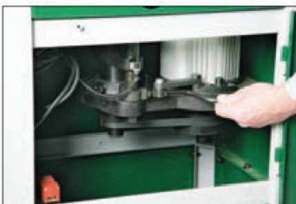
The motor is cleverly hinge-mounted to facilitate easy speed changes
