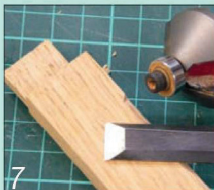
7 Use a sharp chisel to trim the ends of the bevels to a neat 45° angle
