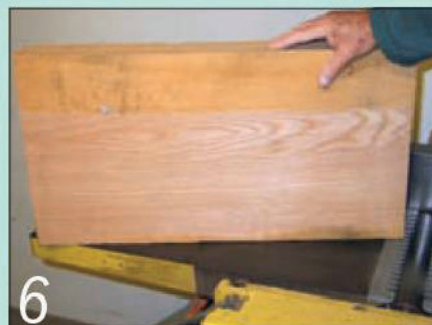
6 Here you can see how the planing is gradually removing the cupping from the lower surface
