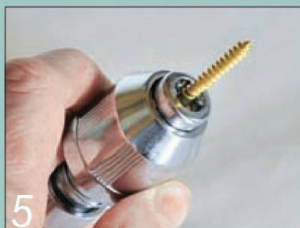
5 Once engaged, the screw is held securely until you retract the sliding collar
