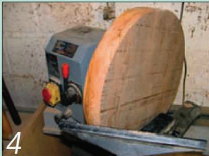
4 The blank is mounted and the tool rest adjusted; let the turning commence!
