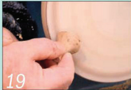
19 Shape the top of the trumpet at an angle on a slow sanding disc
