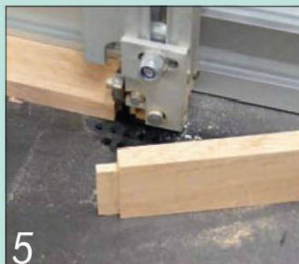
5 Set the position of the fence on the bandsaw to form the tenon shoulders
