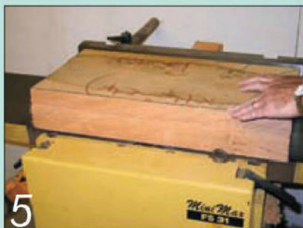
5 The seat material was badly cupped and needed surfacing on the underside to give a flat work face
