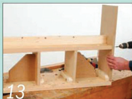
13 Screw the base panel to the batten, then attach the base to the rest of the assembly
