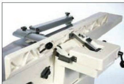
The massive cast iron fence is superbly machined and very easy to adjust
