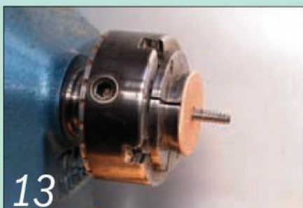
13 Fit the chuck screw with a protective disc of thin plywood
