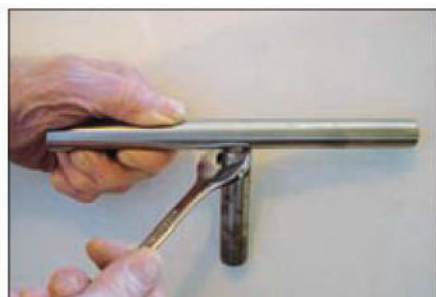
You can tighten the connection between stem and crossbar with a spanner
