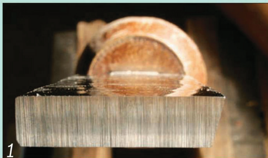
1 Grind away the side of a straight scraper so it doesn't bind in the recess
