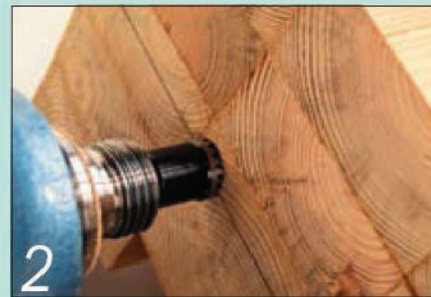
2 A Stebcentre is much safer to use than other drives if you get an accidental dig-in
