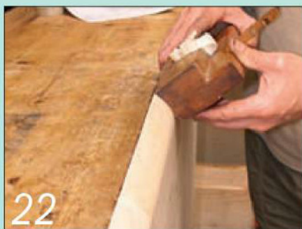
22 The false side panels need a similar but convex curve – a job for my concave moulding plane
