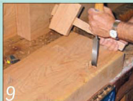
9 ...then switch to a chunky mallet-powered mortise chisel to square up the holes
