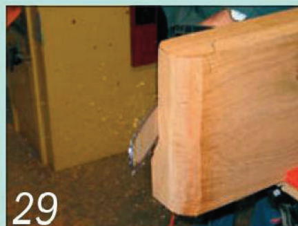
29 Chop off the bulk of the waste from each end of the seats with the chainsaw
