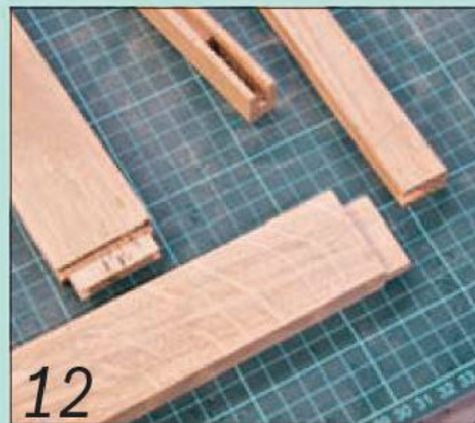
12 The muntin in the rear panel fits into mortises in the top and bottom rails
