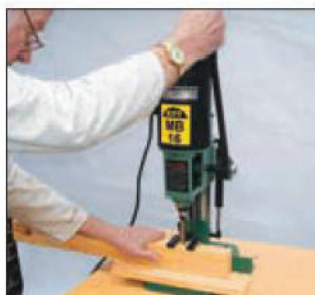
The workpiece is moved along by hand as successive cuts are made
