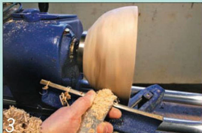
3 Hold the scraper flat on the tool rest and draw the edge along the surface
