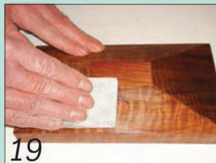
19 I finished my box with pre-catalysed lacquer, rubbed down between coats
