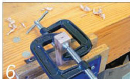
6 Clamp the halves together and use the blade to clean any squeeze-out from the slot
