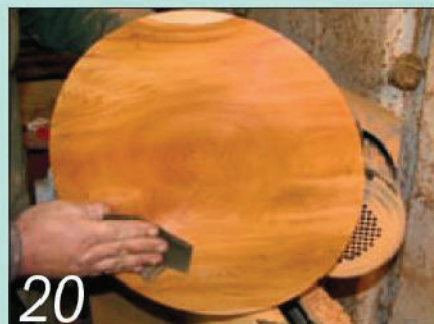
20 Apply two coats of friction polish, cutting back the first coat with abrasive paper
