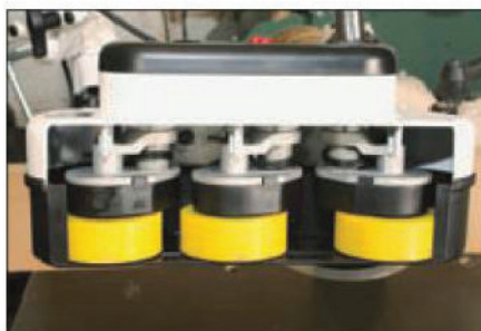
Three plastic rollers drive the workpiece past the machine cutter
