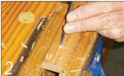
2 Remove the waste from each face to a depth of 0.65mm with a narrow chisel
