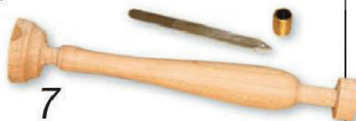
7 Turn the handle to its final shape. Note the projecting ferrule dowel on the right
