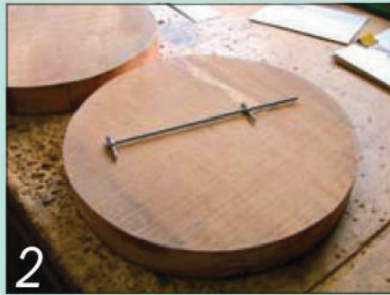
2 I cut several blanks to size on the bandsaw and set the rest aside for the future
