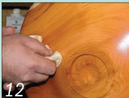
12 When you have an even coat, restart the lathe and polish up the finish
