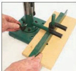
The fence is locked in position where it passes through the column
