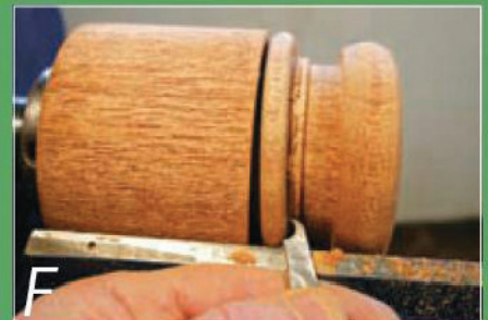
Light cuts are made at each side to free the ring
