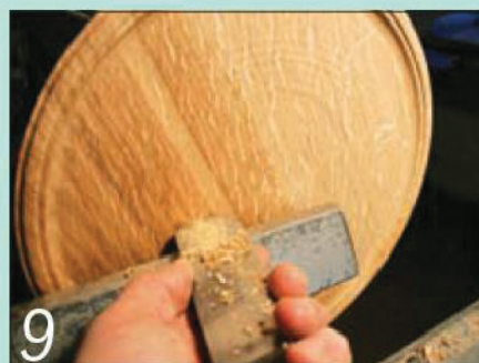
9 Scrapers work best when the grain runs diametrically across the work
