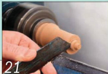
21 Part off a section about 5mm away from the top of the spigot
