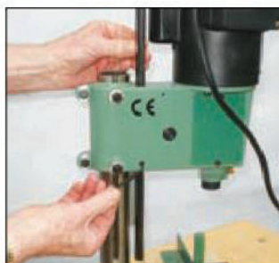
The depth stop controls the lower limit of movement of the head
