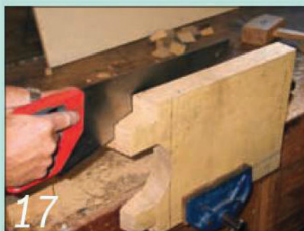
Make the external cut to the marked line on each tenon with a handsaw...
