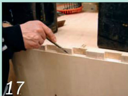
17 The top unit's four panels are assembled using construction dovetails, trimmed with a sharp knife
