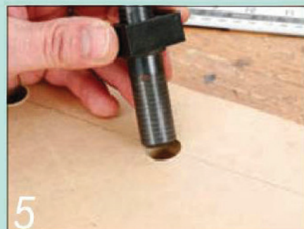
5 It can be a fiddly job engaging the dogs in holes with a square edge profile...
