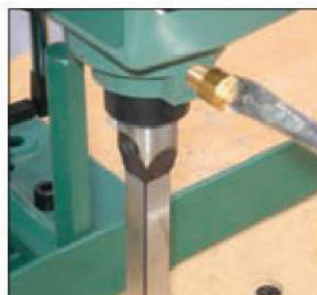
The screw at the front of the head locks the chisel in the chuck
