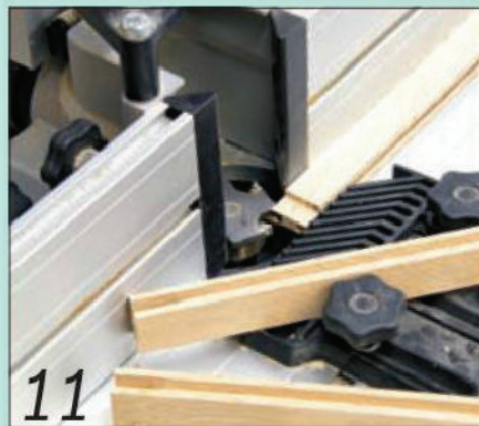
11 Cut the grooves in the back panel frames to suit the MDF panels
