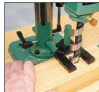
The mortiser can also be used as a drill press for boring holes
