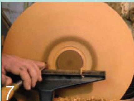
7 Level off the base of the platter, working from the rim towards the centre
