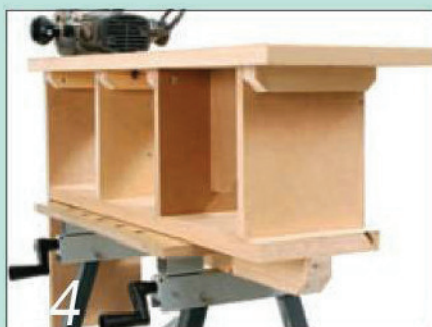
4 The work station should now sit squarely on the bench, securely clamped by its jaws
