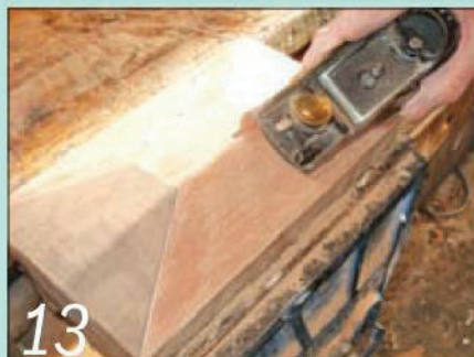
13 Use a sharp block plane to trim the angled veneer edges on the box lid
