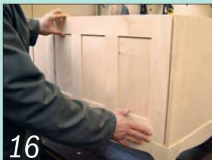
16 The completed panel fits in the rebates cut in the base unit's side panels, and is fixed with screws
