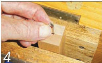
4 Clamp the handle halves together in a vice and check that the blade slides in easily
