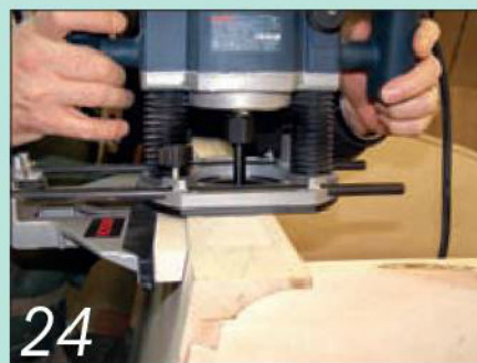
24 Assemble the top unit, then rout a recess 1mm deep in the face of the two false fronts
