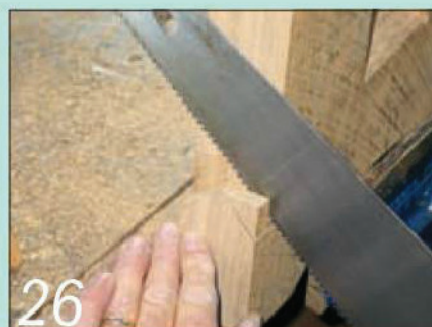
26 Trim the edges of the legs as far as the decoration on the bandsaw, and finish them by hand
