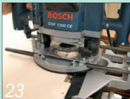
23 Use a router with a fence to create the housings for the false sides in the top and bottom panels
