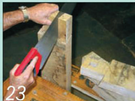
23 Finish cutting the tenon cheeks on the ends of the stretchers with a hand saw
