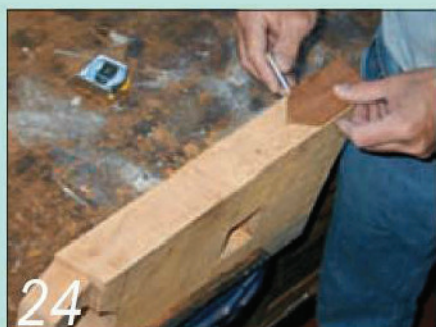
24 Use a small template to mark the extent of the decoration on each edge of the legs
