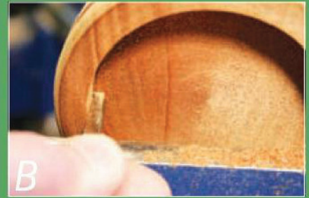
...to undercut the side wall at the base of the recess
