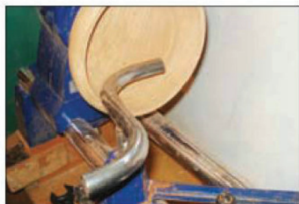
The internal bowl rest provides good support for the tool
