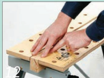
12 Machine the clamping batten so it sits just below the jaws on the portable workbench
