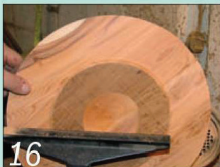
16 Taper the outer part of the blank's face gradually down towards the edges
