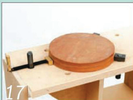
17 Two fixed dogs and an adjustable Wonder Pup are ideal for holding round work
