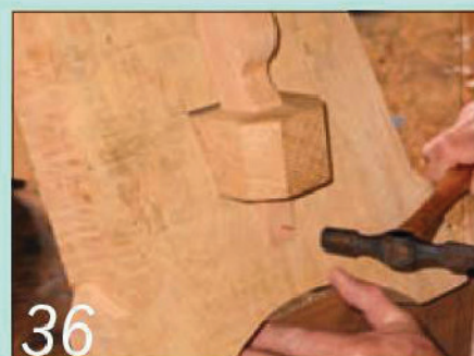
36 Drive a wedge into each stretcher mortise and lock it in place with a copper pin
