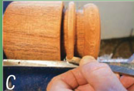
The first ring scraper rounds off the corners
