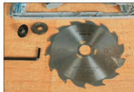
For cutting sheet materials, you'll need to fit a finer blade than the one supplied
