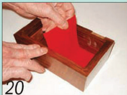
20 Stick pieces of self-adhesive baize into the base of the box and the tray
