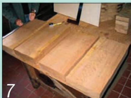
7 Mark the positions of the leg mortises on each seat. Batch marking ensures consistency
