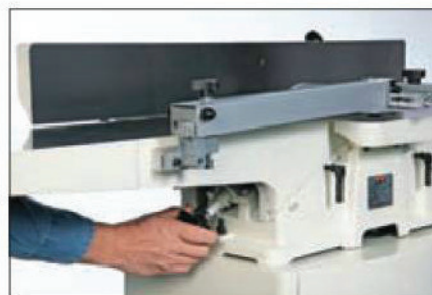
The rear table is also adjustable, which makes setting the knives much easier
