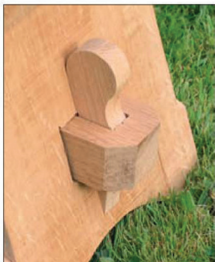
27 Take the bottom angle of the foot from the drawing, and cut all the feet to length
