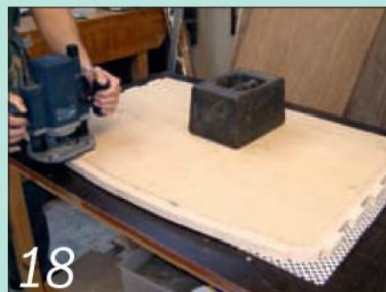
18 Rout the tambour groove in the top and bottom panels using a template and a guide bush
