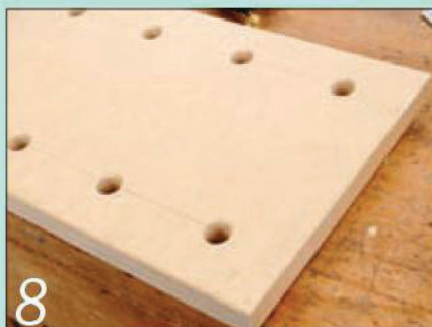
8 While you've got the router out, run it along the edges of both sides of the top
