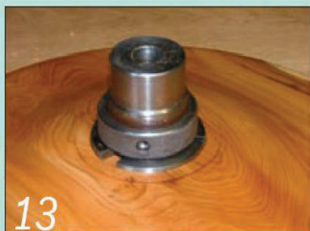
13 Fit the combination chuck into the dovetail recess you prepared earlier...
