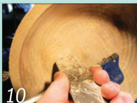
10 Here a round-nose scraper is being used to finish off the floor of a bowl
