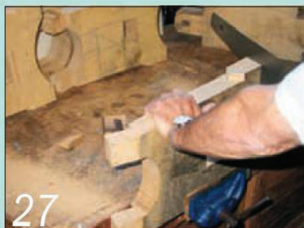
27 Take the bottom angle of the foot from the drawing, and cut all the feet to length
