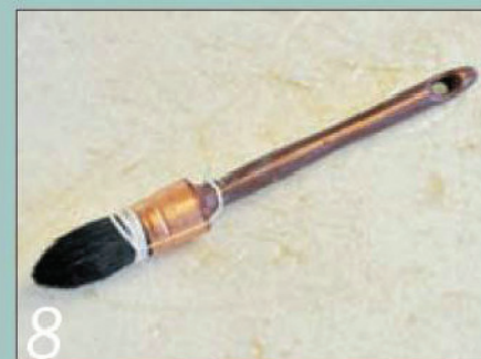
8 Thank heavens for the humble sash brush, the only tool that cuts in well round glass
