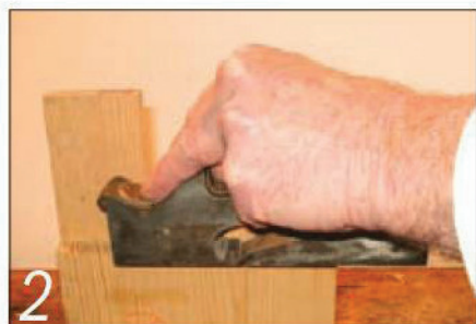
2 A shoulder plane does as its name says; it trims tenon shoulders
