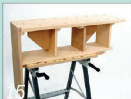
15 Note how the vertical clamping board clears the left-hand end of the bench
