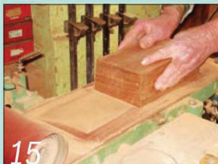
15 Rub sawn edges off the lid and base on abrasive paper to smooth them
