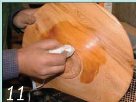
11 Apply a generous coat of friction polish; I prefer to do this with the lathe stationary
