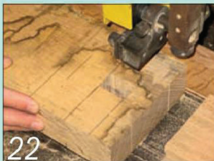
22 Cut a mortise in each end of the stretchers, then part-cut the tenon cheeks on the bandsaw
