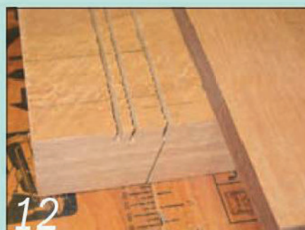
12 Set your circular saw blade at an angle and cut the tenon shoulders on all the legs
