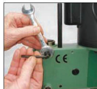
This adjustment limits the possible rotational movement of the head
