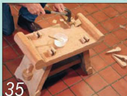
35 Drop the top into place and drive a glued wedge into each expansion slot
