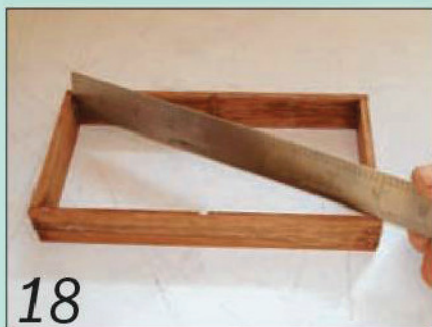
18 The tray is made from 3mm thick stock with dovetailed corners. Note the stopped trenches
