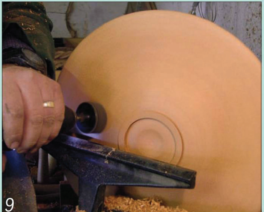
9 Remove any remaining gouge marks by sanding the base of the platter. I used a foam-backed abrasive pad in my cordless drill to follow the contours
