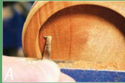
The hook on this side-cutting scraper can be used...
