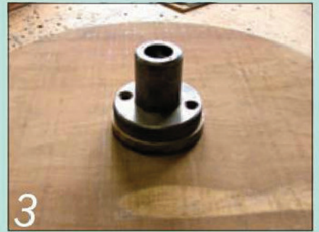
3 I added a plywood washer to my screw chuck so the screws didn't go in too far
