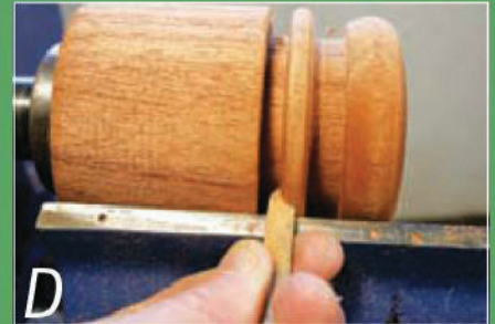
It is then rotated to cut one side of the ring
