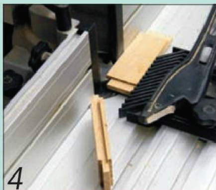
4 Repeat the joint-cutting and grooving process on the short rails
