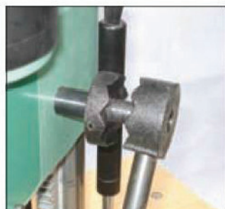
This toothed connector allows the handle position to be altered
