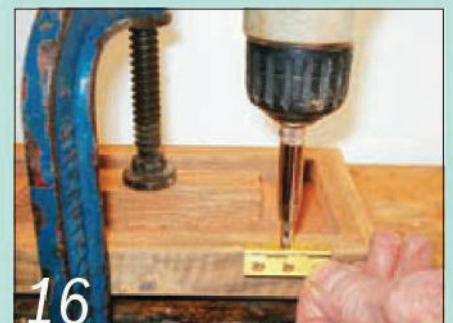
16 Cut the hinge recesses on the lid and attach the hinge. I used a drill guide here
