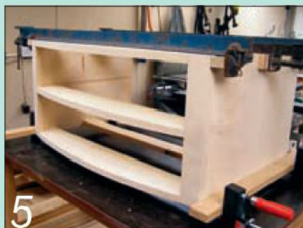
5 Assemble and cramp up the base unit. Note the rebate for the back panel at the rear of the carcass
