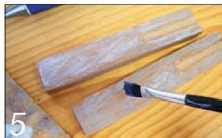
5 Spread PVA glue thinly on the two halves, keeping it clear of the blade recesses
