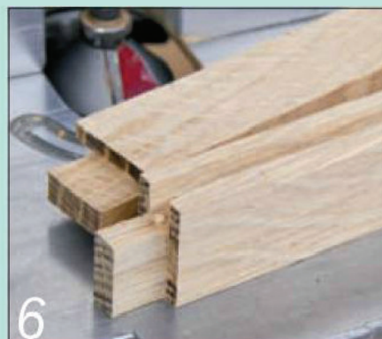
6 Use a bevel cutter to form stopped bevels on the rails and stiles as a decorative feature
