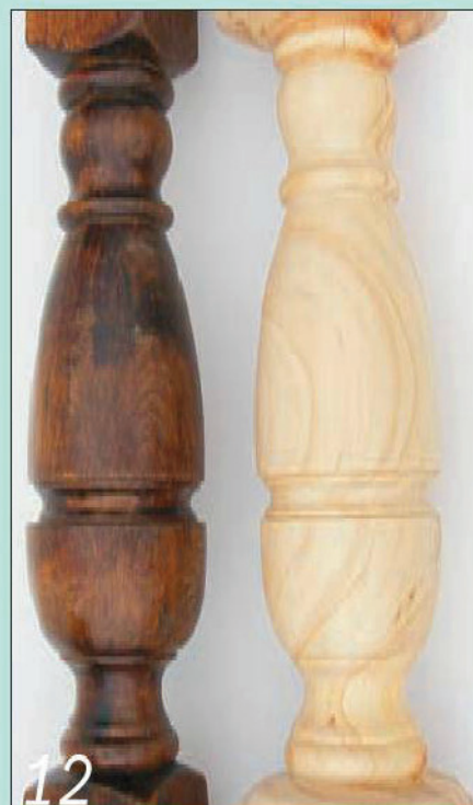
12 The original object (left) and a copy made with the aid of the turning guide
