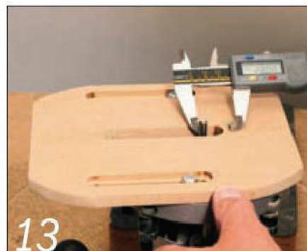
13 Setting the radius with a calliper gauge
