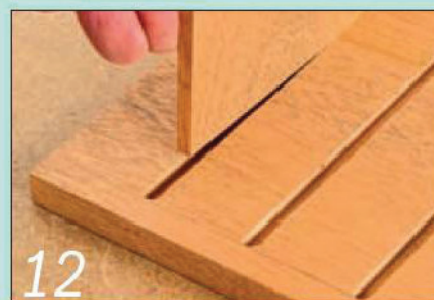
12 Thickness the shelf material down so it's a smooth sliding fit in the grooves
