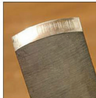
The blade is ground to a 75mm radius
