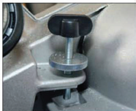
The depth of cut adjuster is a bit fiddly
