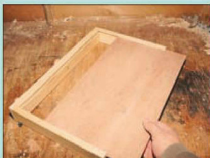
Using a cutter slightly wider than the panel thickness will ensure an easy sliding fit
