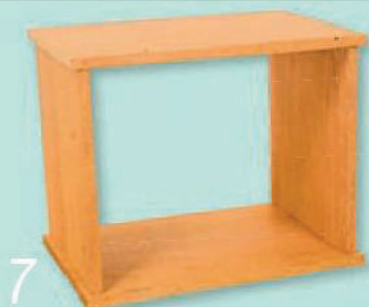
7 Assemble the main carcass dry to test the fit, and do any necessary trimming
