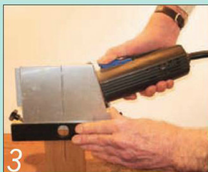
3 I then used my biscuit joiner to cut all the biscuit slots
