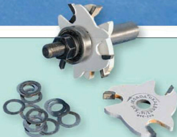
Adjust the width of the slot by arranging various cutters and shims on the arbor
