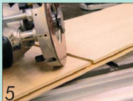
5 I used a slot cutter in a hand-held router to groove the edges of the top...
