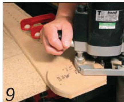
Shaping the end of the jig with the router
