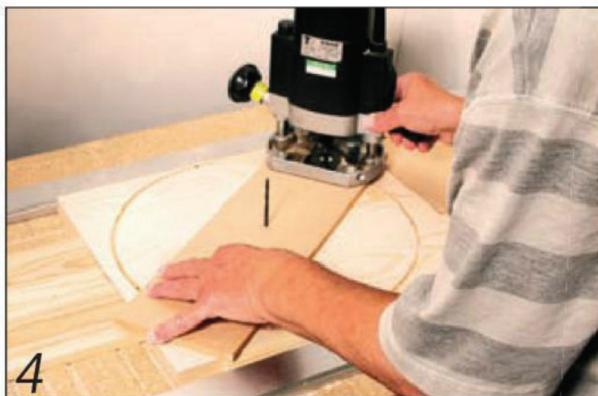
4 Cutting the circle by moving the router anti-clockwise
