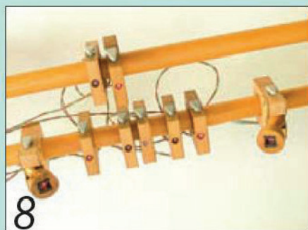
8 An underside view of one possible configuration, with nine laser units on two rails
