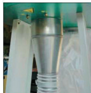
The metal reducing coupling connects 100mm hose
