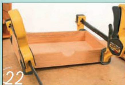
22 Shape the radiused finger pull using a drum sander and assemble the drawer
