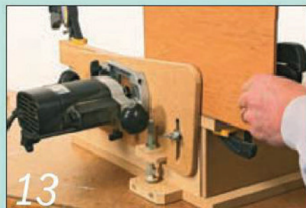
13 Round over the shelf edges using a tall temporary sub-fence as a support
