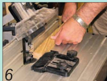
6 ...and installed in the router table to cut the offset tongues
