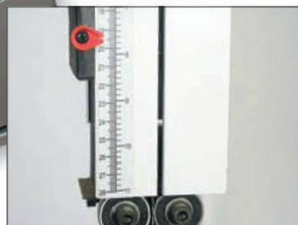
The upper guides are mounted on the blade guard
