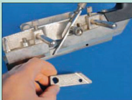
Make sure second-hand planes are complete. This was missing the wide cutter clamping block
