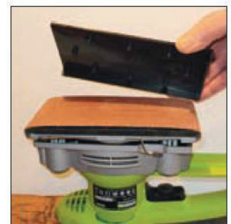
Use the plastic punch to pierce hand-cut abrasive sheets
