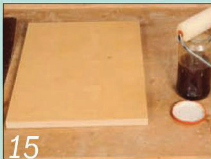
15 Apply contact adhesive to both surfaces using a paint brush or mini paint roller
