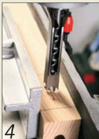
4 Clamp the workpiece and align the auger on the centre line
