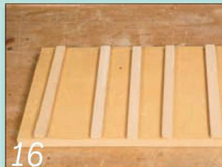
16 Place scrap strips on the base board so the laminate can be positioned accurately
