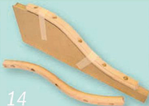
14 Without this purpose-made support, boring these sockets would be impossible
