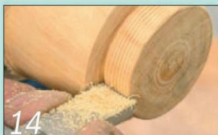
14 Reapply the chaser at the start of the thread to gradually deepen it
