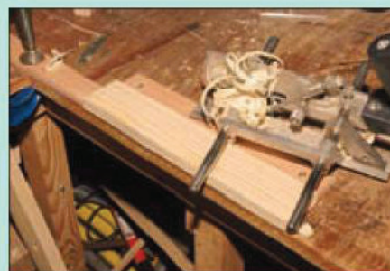
A ploughed groove in the top of a small wall cabinet, ready to accept a captive loose back
