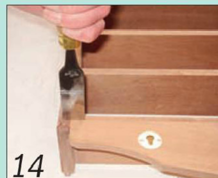
The rebates for the back panel needed their corners squaring up
