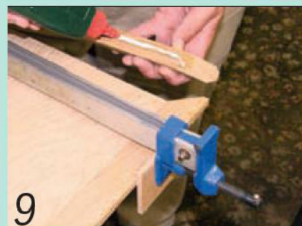
9 The top lippings are carefully glued and cramped in place
