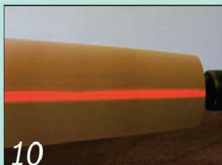
10 The straight, wide laser line on the centre line shows tapered turning completed
