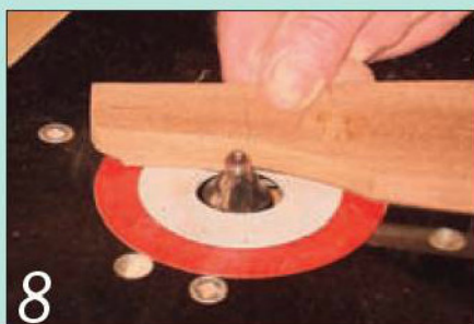
8 Use a 4mm bearing-guided quadrant cutter to detail all the edges
