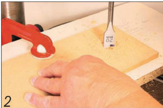
2 Boring the 20mm diameter hole for guide bush
