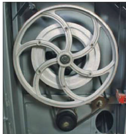
The lower bandwheel with the two-speed pulleys
