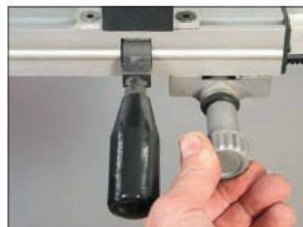
There is a micro-adjuster on the rip fence
