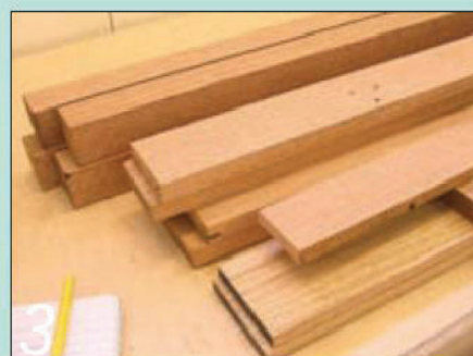
3 Once the parts are squared and thickened, you can cut them all to length
