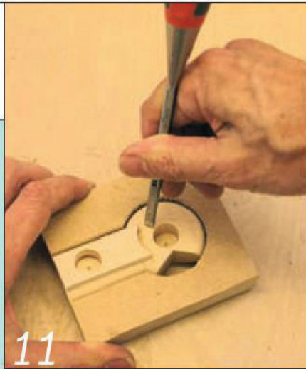
11 A simple holding aid ensures consistency and easy handling of small components
