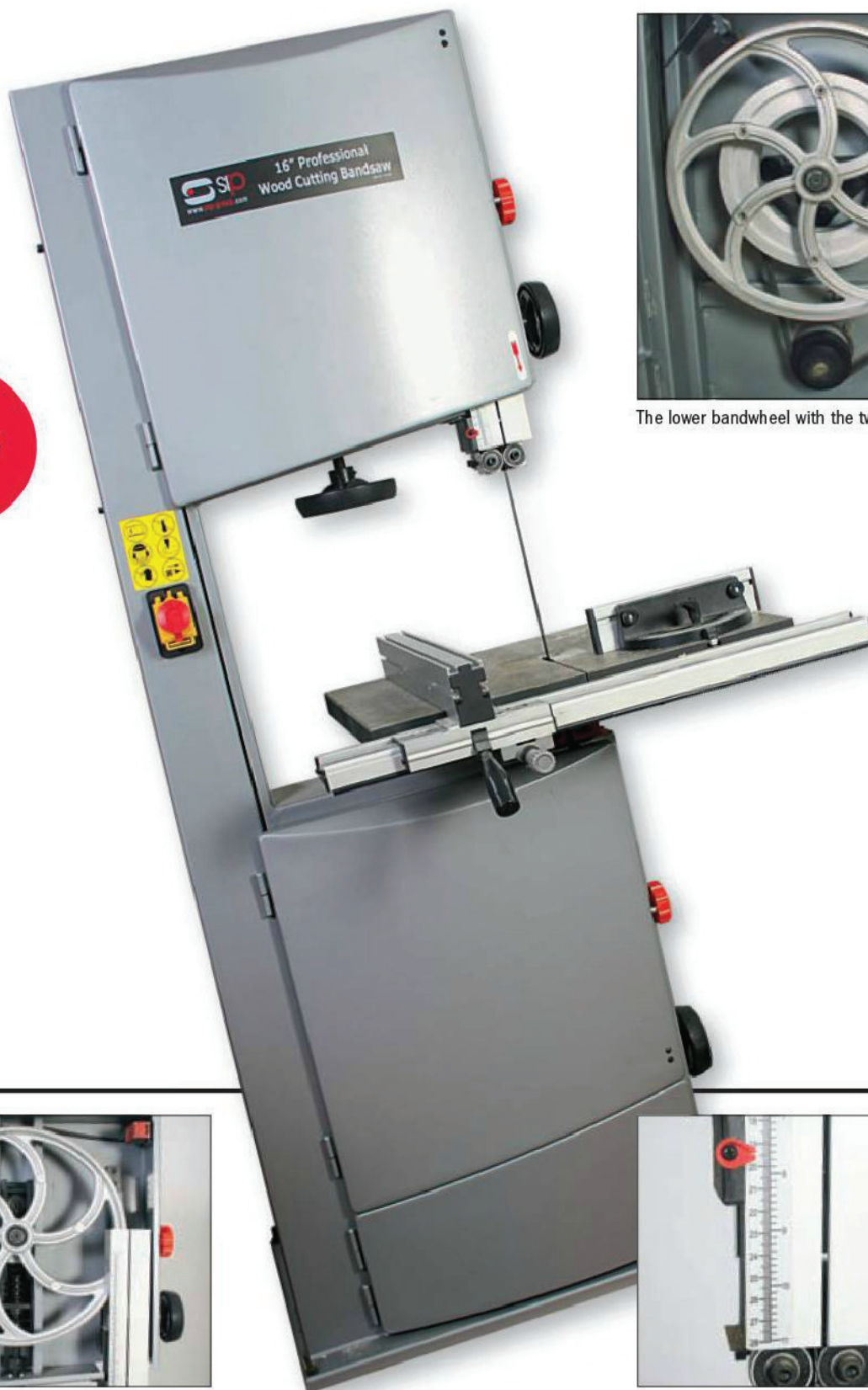
The upper guides are mounted on the blade guard
