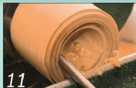
11 Gradually scoop out the interior of the box base with a small bowl gouge
