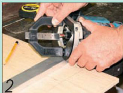
2 Set the same depth of cut for the grooves using a depth gauge
