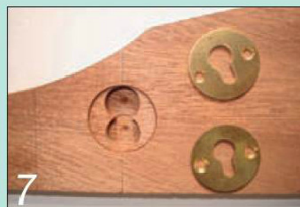
7 Bore large and small holes to accept the hanging plates and screw heads
