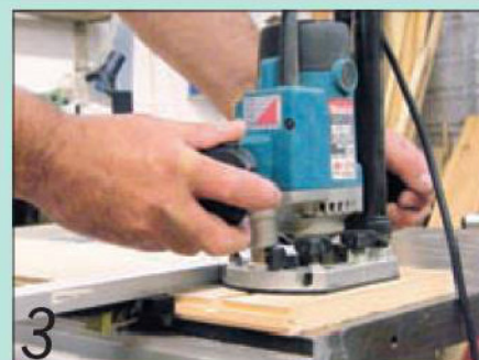
3 Use a straightedge as a guide when cutting the grooves
