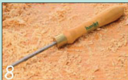
8 Many chasing experts use a point tool for the shaping work on these hard woods
