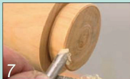
7 Chamfer the leading edge of the spigot to give the thread a clean start
