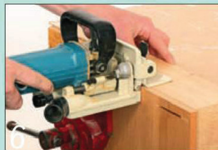
6 Use the fence again to provide the correct offset
