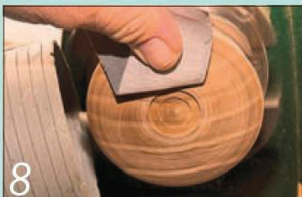
8 Sand the lid smooth, starting with 180 grit and working down to 400 grit
