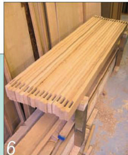
6 Complete all of one manufacturing stage first, as with these through mortises...
