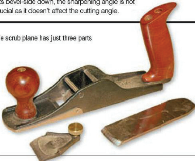
The blade is ground to a 75mm radius
