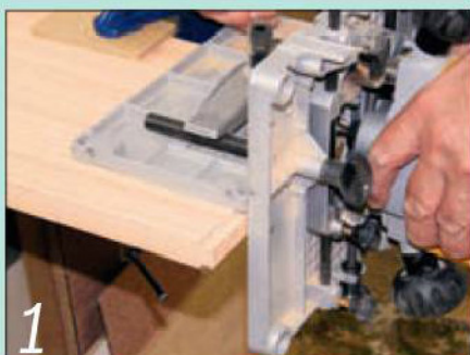
1 Use a small router table hand-held to cut the dovetails on the board ends
