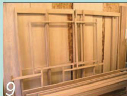
9 All these frame beads have been mitred on the same machine setting
