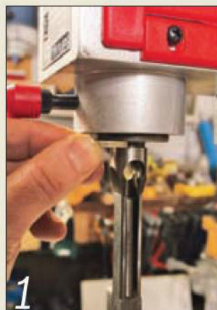
Use a £1 coin to set the chisel/auger clearance
