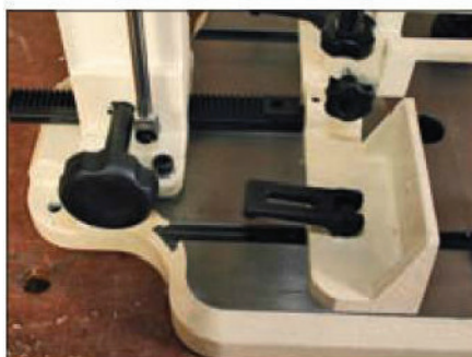
The cam clamps and the fence's rack-and-pinion adjustment
