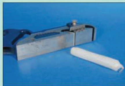
Lubricate the running surfaces with candle wax to reduce friction and make the cut easier to progress
