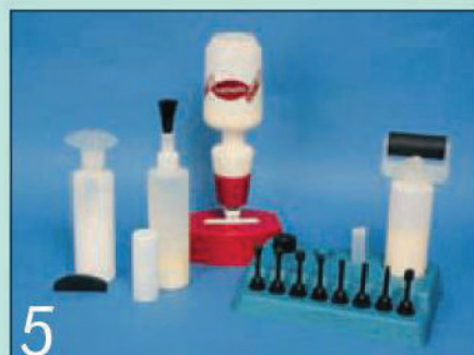
There are lots of applicators for PVA. Most of the screw-on type will fit standard glue bottles
