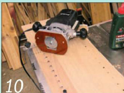
10 The Trend shelf support jig guarantees accurate positioning of holes for the shelf pegs
