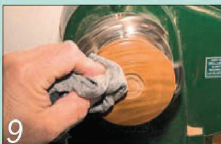
9 Apply a coat of friction polish first, then finish it off with wax polish
