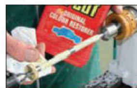
The turned blanks are sanded and buffed
