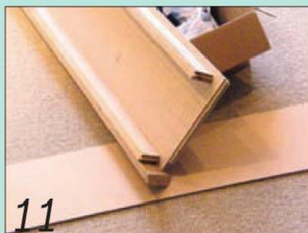
11 Two lengths of softwood give extra support beneath the base
