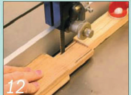
12 Temporary stops can make repeat cutting so much easier – and more accurate
