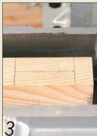
3 Mark up the workpiece as shown, ready for mortising
