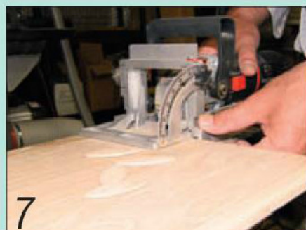
7 Biscuit joints will secure the top panel to the bookcase sides
