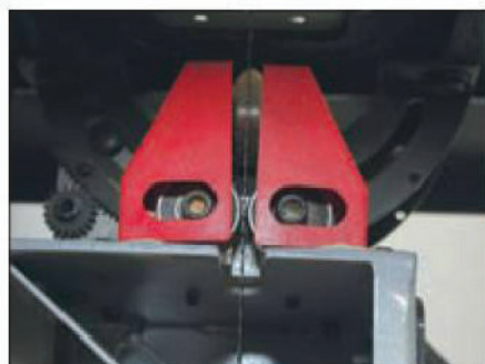
The lower blade guides give excellent blade support
