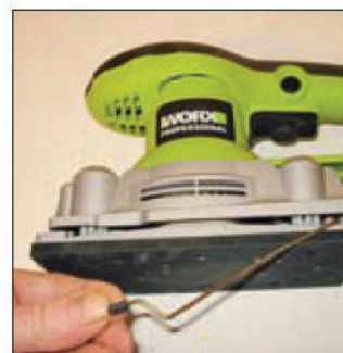
The abrasive sheet is held in place with simple wire clips
