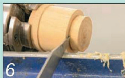
6 Turn a small spigot on the blank with a rebate at its inner end
