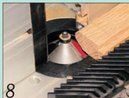
8 I cut a chamfer along the length of the lipping for the top panel
