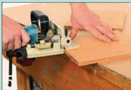
5 Align the biscuit slots using the fence on the jointer
