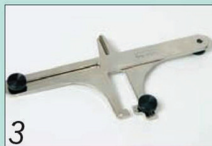
3 A sizing gauge makes matching internal and external threads a lot easier
