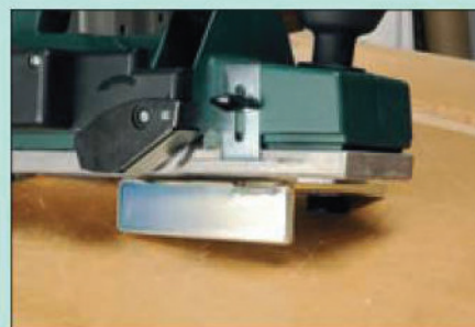
The power planer ready for rebating; remove the material in small bites
