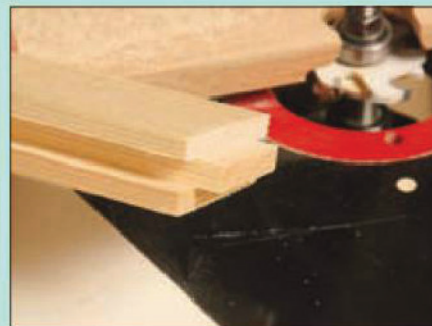
Using a slotting cutter to cut grooves on either side of a muntin
