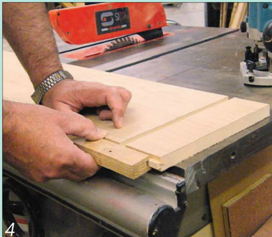
4 Tongue and groove joints are used to locate the oak lippings
