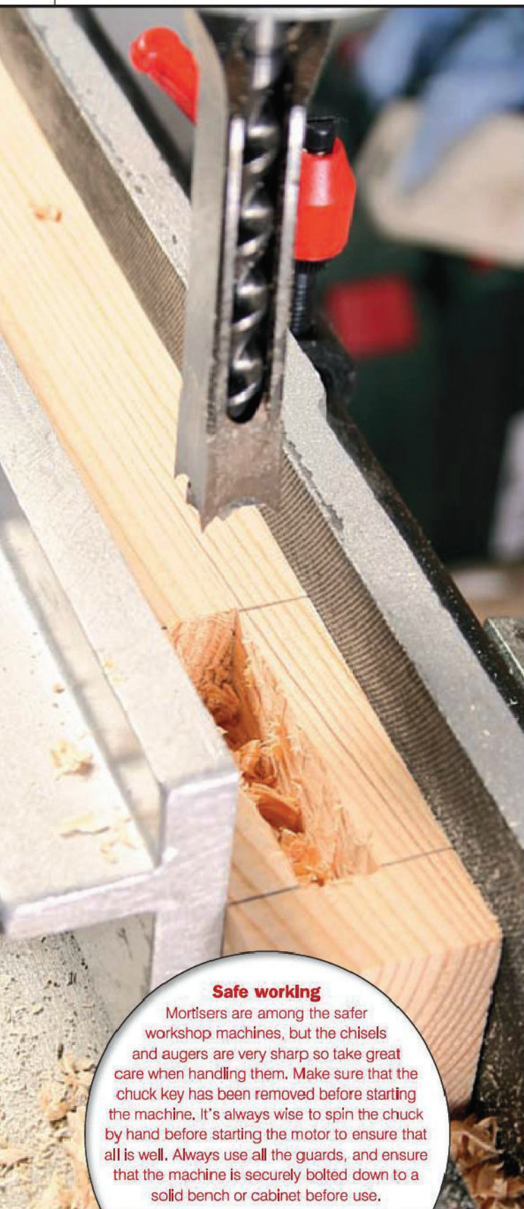
Use a £1 coin to set the chisel/auger clearance
