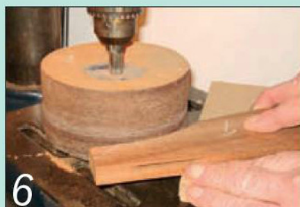
6 ...and finished the shaping with a compass plane and drum sander
