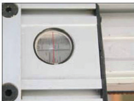
The rip fence setting window is highly accurate
