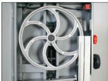
The cast alloy bandwheels have nylon tyres
