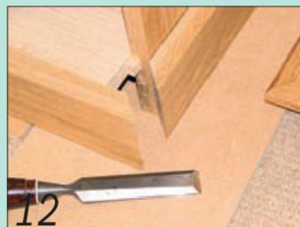
12 Sliding the sides onto the ends of the base as the bookcase is assembled
