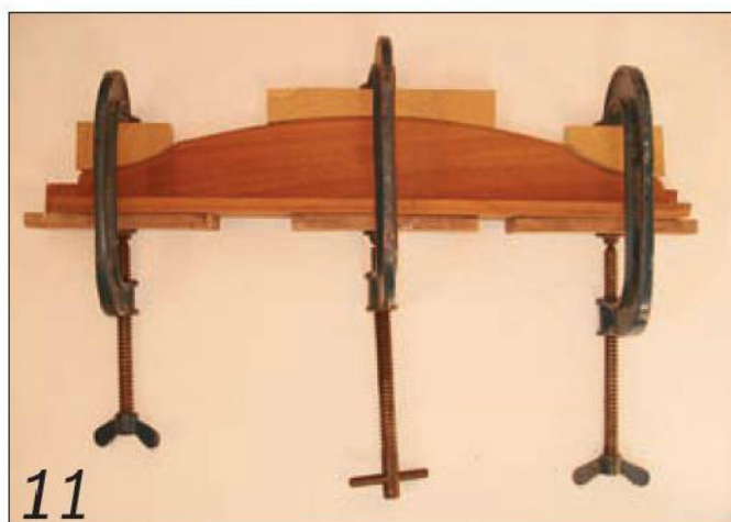
I used shaped packing pieces to cramp each sub-assembly
