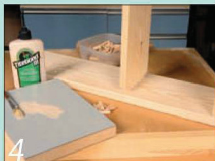
Small amounts of PVA glue can be poured onto a non-porous surface and picked up on a brush
