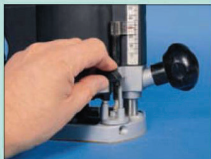
Lock a hand-held router down with the plunge lock and the depth stop
