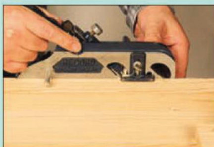
For cutting deeper rebates, the fence bar can be withdrawn into the machined side of the plane
