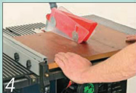
4 Rip the widened boards down to the required widths
