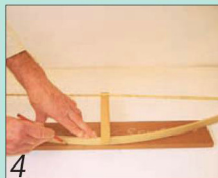
4 A home-made string bow makes smooth curves easy to mark out
