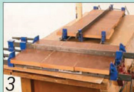
3 Cramp the widened sections and leave them to dry
