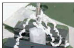
Acrylic resin is easy to cut and drill
