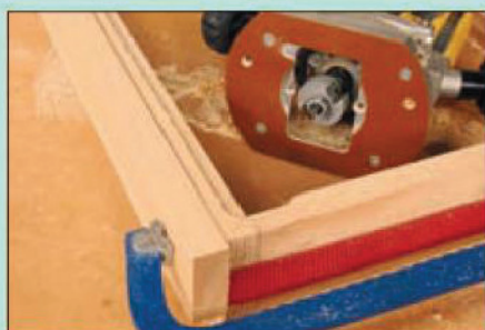
The router is ideal for rebating an assembled carcass...
