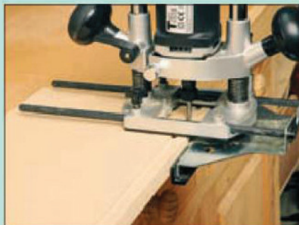
Using a straight cutter to sink a groove in the face of a piece of MDF
