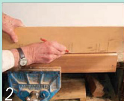
2 I clamped the two end pieces together before marking the shelf positions
