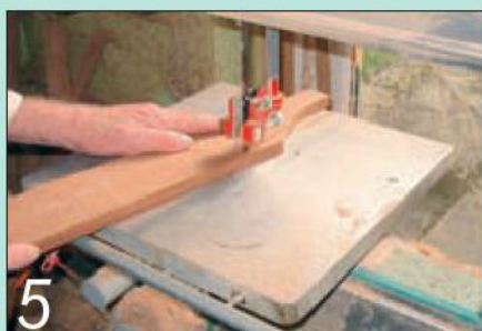
5 I cut the curved top rail roughly to shape on the bandsaw...
