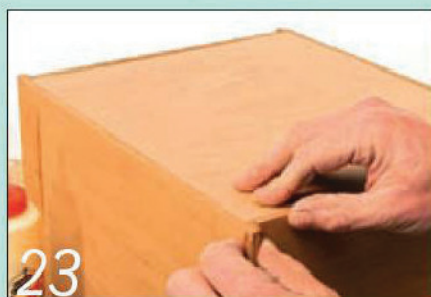
23 Glue the back panel into place in the squared-off rebates. There's no need to pin it
