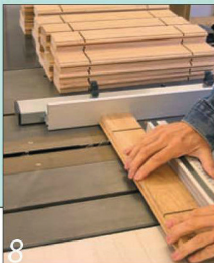
8 Working from the saw fence produces a set of identical tenon shoulders
