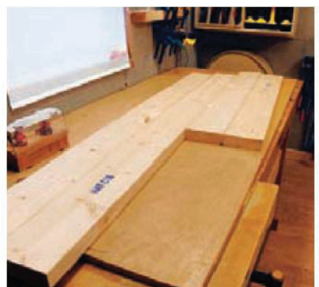
2 The wood I used for the door is inexpensive softwood, supplied ready-planed
