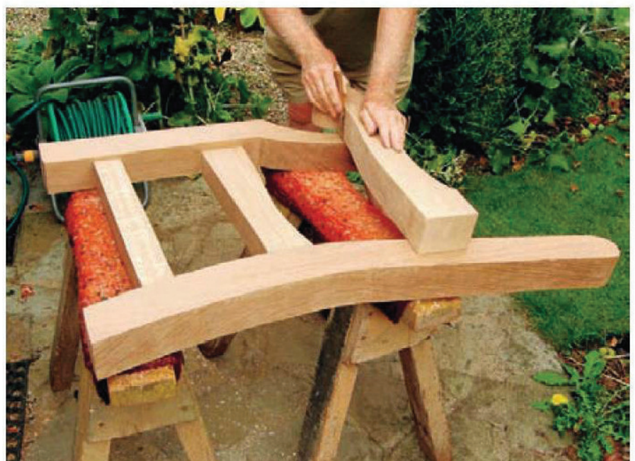
10 Lay each arm across each end frame and mark the shoulders with a marking knife
