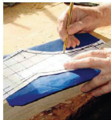
3 Transfer the outlines of the components to the planed timber using a pencil and carbon paper
