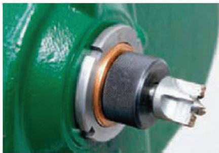
18 A solid spindle needs a centre ejector screwed onto the spindle nose
