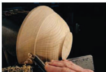
7 Swing the gouge in an arc so the bevel follows the curve
