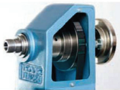
19 A three- or four-step pulley gives a speed range of 400-2000rpm
