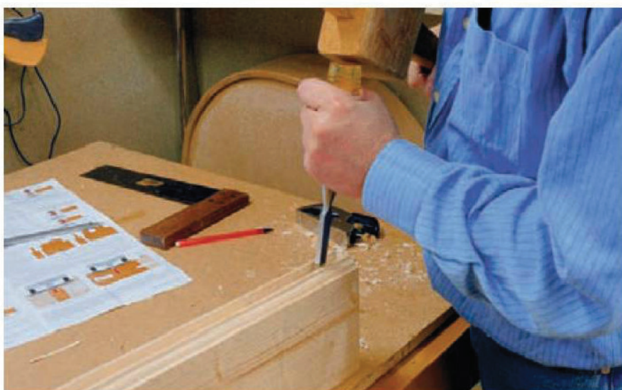
13 I had to resort to drilling and cutting the mortises by hand
