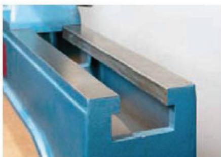
8 More expensive beds are solid castings that are almost a work of art
