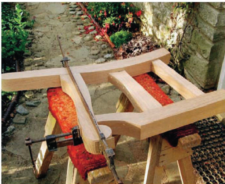
11 Cut the mortise and tenon on each arm, fit it to its end frame and glue and clamp it in place
