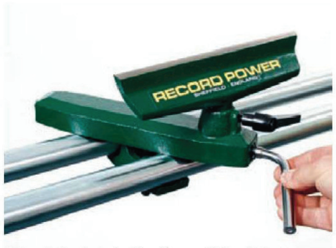
26 A cam lock on the tool rest is easily accessible from the front
