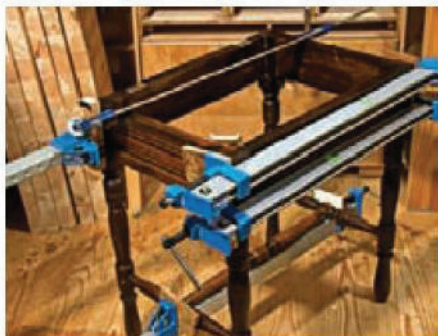
13 With the joints glued, I cramped up the table frame and left it to set...
