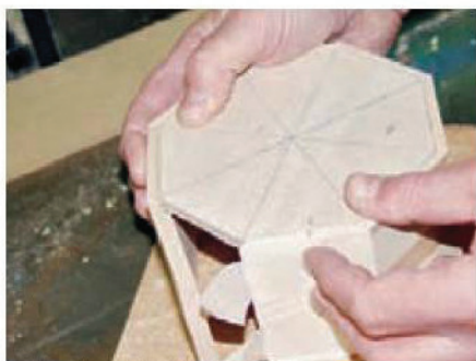
9 Glue the eight sides around the base and lid of the box
