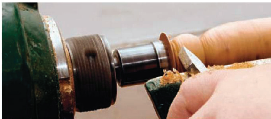
14 Add the turned detail at the other end of the handle
