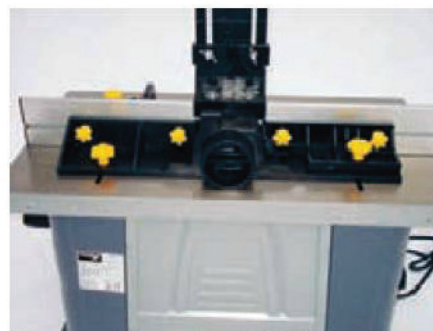
The two-part fence viewed from the rear
