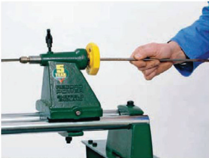
25 ...and should be drilled through to allow for long hole boring
