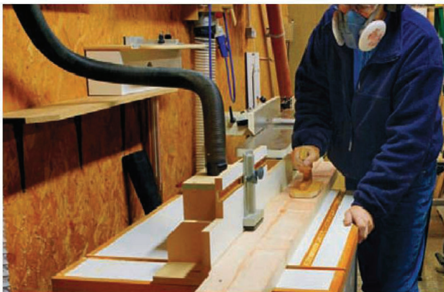
10 With such large pieces of timber, a substantial router table is a must
