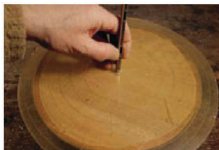
2 Use a simple centring device to find the centre of the bowl blank
