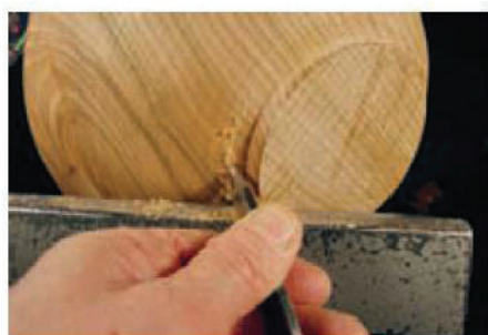
10 Form the shoulder using just the corner of the blade
