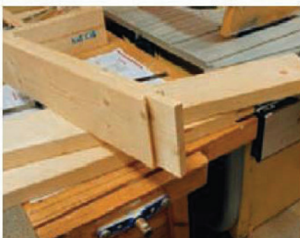
8 The finished result is a very neat 63mm long tenon
