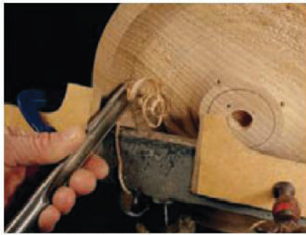
17 Use vertical toolrests to guide the gouge as you shape the bowl
