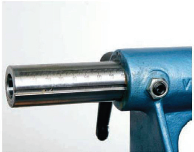
24 The tailstock barrel needs plenty of travel for drilling work...
