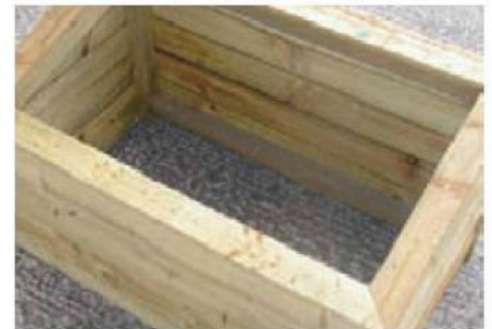
6 Mitre-join the top frame and fit it to the top rails of the frame
