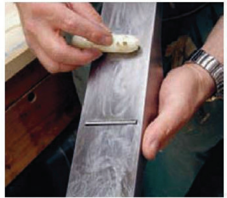
14 Rub candle wax on the plane's sole to reduce friction
