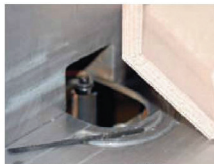
11 Cut a shallow rebate around the perimeter of the box base for some stringing
