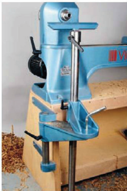
14 You need an additional tool rest for turning big-diameter bowls
