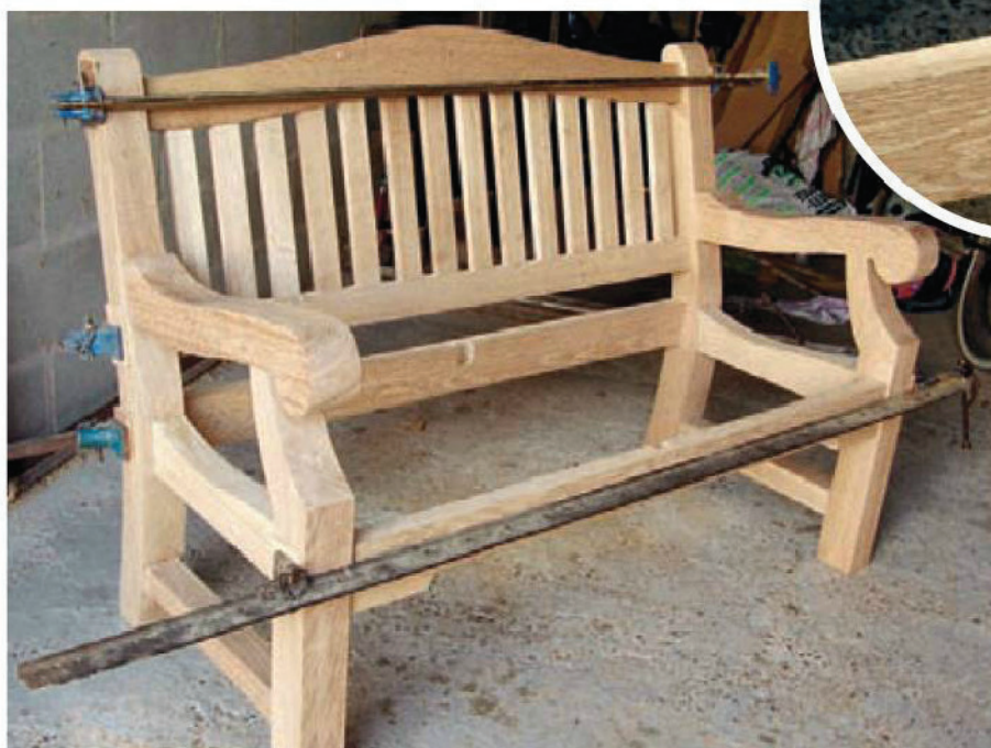
14 Cut notches in the front and rear seat rails for the centre seat support ( inset ), then assemble and clamp up the main carcass
