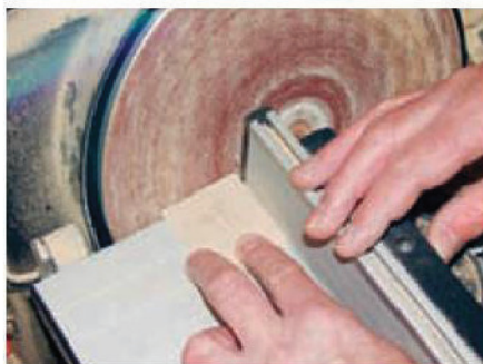
13 Bevel the edges of the lining pieces to fit inside of the box
