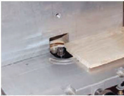
1 Cut a rebate on the timber to match the thickness of the veneered plywood
