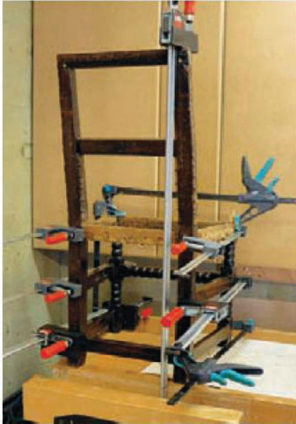
17 I then fitted the front frame to the rails and cramped up the whole assembly
