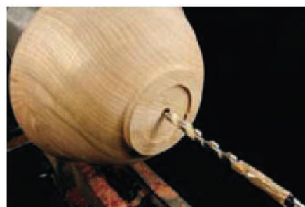
15 Bore the hole for the bolt of the nutcracker mechanism
