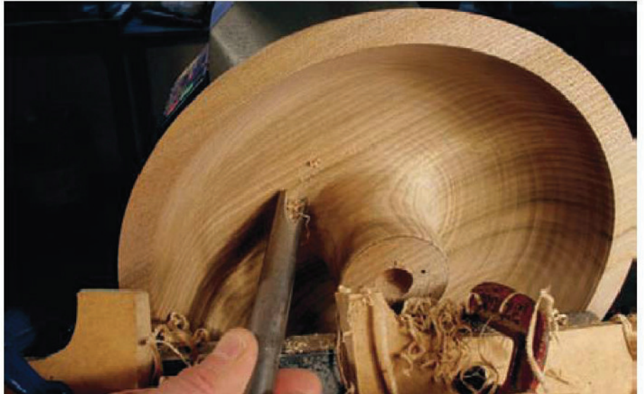
20 Finish the floor of the bowl with the blunt angled gouge
