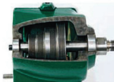
10 The bearings should be good quality heavy-duty ball races
