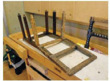
16 Once the frames were set hard, I fitted the side rails to the back
