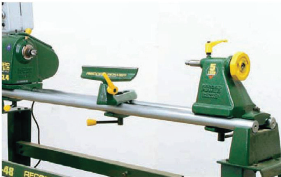
7 The lathe bed is made from heavy metal bars or tubes
