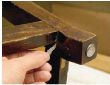
15 A coat of shellac round the joints before gluing makes clean-up easier
