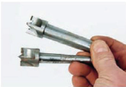
17 Morse tapers are a universal means of installing centres
