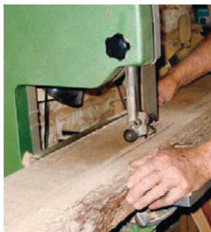
2 Remove the sapwood with a bandsaw before planing and thickening the wood
