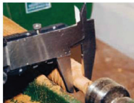
13 Form a spigot on one end and check its diameter with callipers
