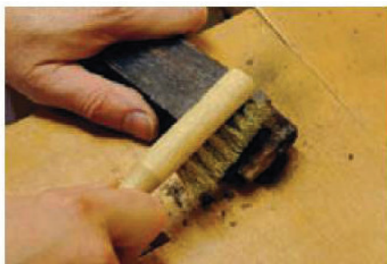
12 ...and cleaned off any remaining old glue with a stiff wire brush
