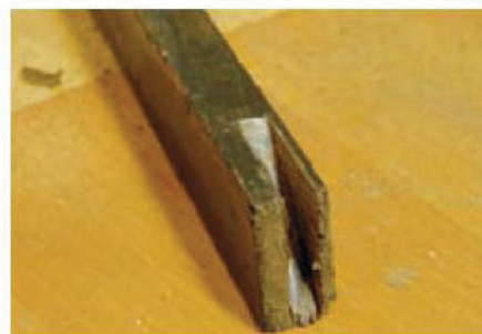
8 I carefully chopped out the waste wood with a sharp chisel...
