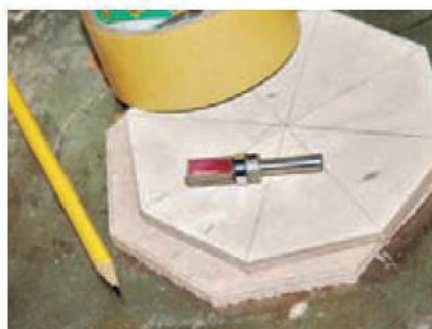
7 Use the base as a template to make the lid
