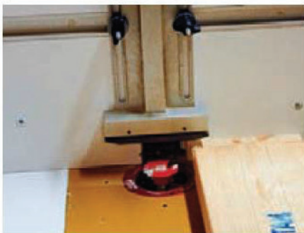
7 The tenon passes over the top of the cutter, so any length can be cut
