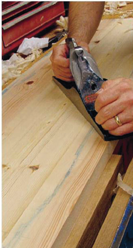
13 Plane off any blue-marked high spots by hand
