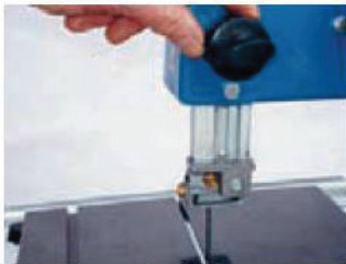
This knob controls the height of the blade guide
