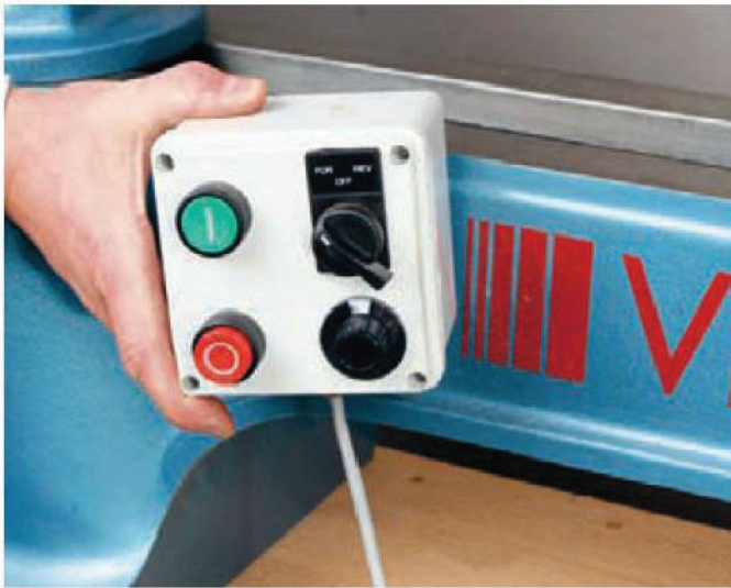
23 A magnetic switchbox can be fixed wherever you're working
