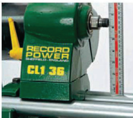
3 ...and a swing of at least 9in between spindle and bed
