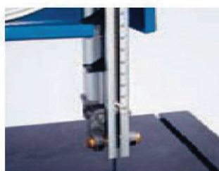
The blade guide and guard are readily adjusted
