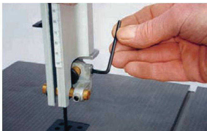
Blade guide adjustments are made with an Allen key
