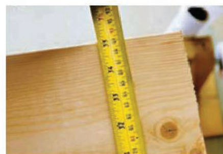
14 Dry assembly revealed that the door was spot on for width
