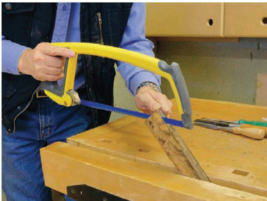
7 I had to cut some joints with a hacksaw to cope with all the deeply embedded upholstery tacks
