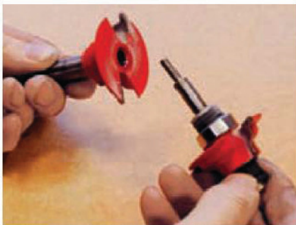
6 ...to leave a flat-topped tenoning cutter
