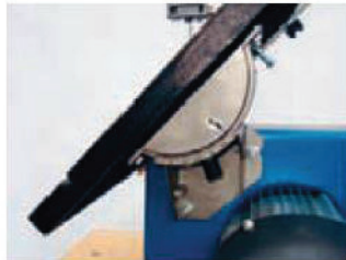
The table will tilt up to to 50° to the right
