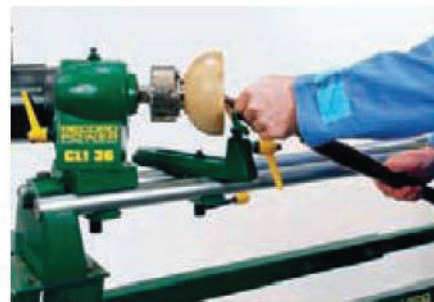
13 Swinging the head off-centre keeps tool handles clear of the bed
