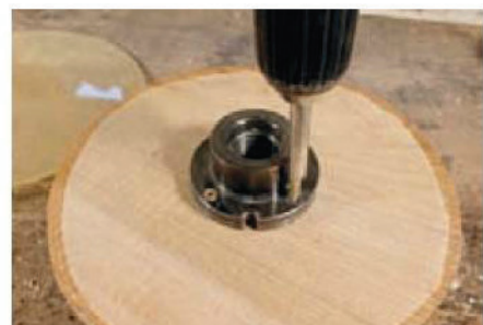
3 Use four size 8 Spax screws to secure the faceplate to the blank
