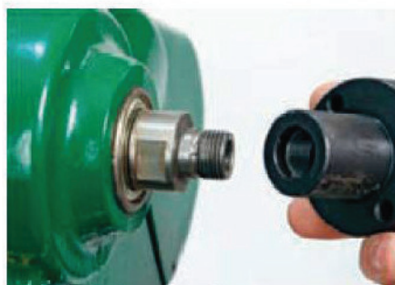
16 A spindle thread size of \frac{1}{4} in x 16 tpi is the industry standard
