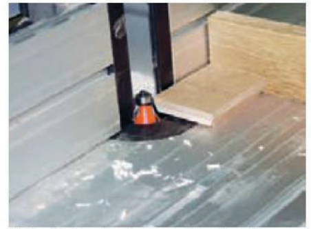
3 Trim the bevels using a router cutter. Note that the finger guard has been raised for clarity
