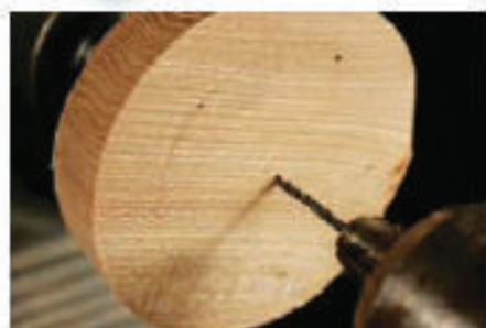
4 Drill a pilot hole for the screw chuck in the centre of each disc
