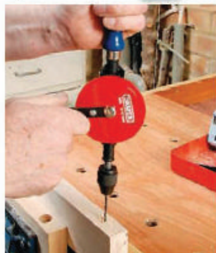
The drill quickly makes small holes
