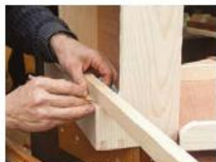
32 Mark one hinge rail to fit the box...
