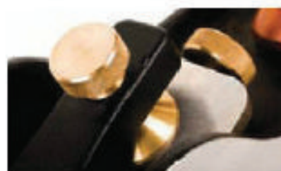
The lever cap knob, lever cap and depth of cut adjuster
