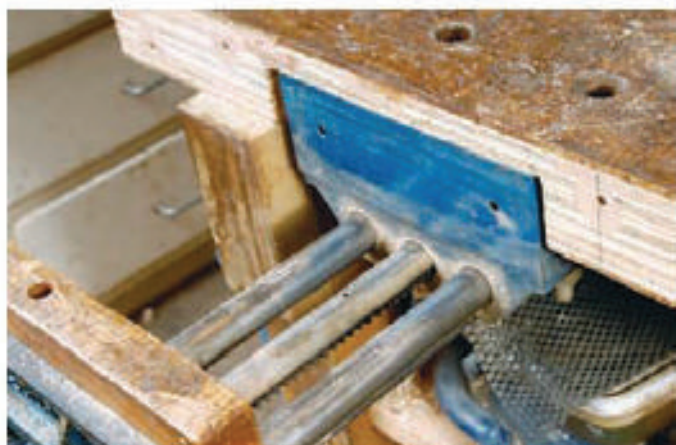
The vices are rebated into the top before fitting the lippings
