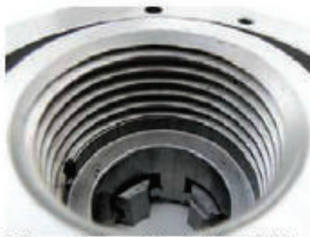
7 The manufacturer of this chuck has failed to allow for the horizontal register or spigot, so it won't fit the lathe it's designed for.
