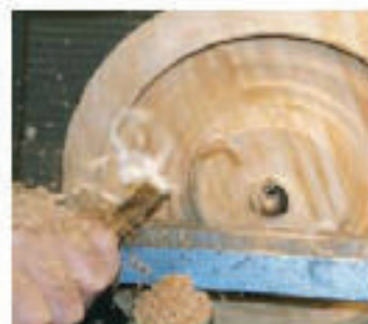
15 Hollow out the remainder of the shape with the bowl gouge
