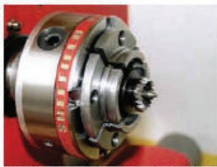
9 A Robert Sorby Steb centre designed to fit into the standard jaws of the Patriot chuck.
