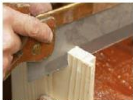
7 Cut down to the shoulder line
