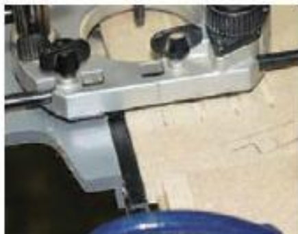
1 Fit a fence to the router to cut the flutes on the front stiles
