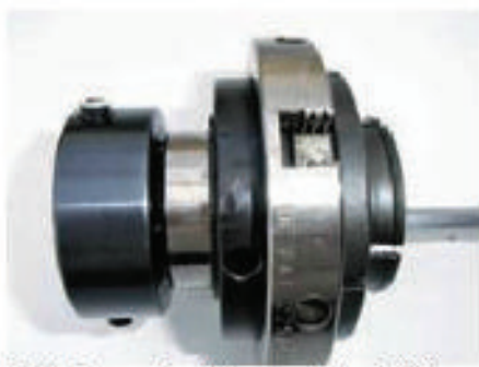
8 This One-way chuck has an adapter to fit the Myford Mystro lathe, so it can be locked into the V slot behind the register. The number on the jaw carrier can be seen.
