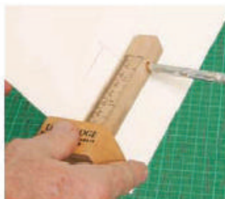
15 Use a modified marking gauge to define the corner of the cut-out
