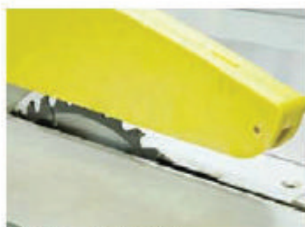
The long crown guard makes sighting the line of cut difficult
