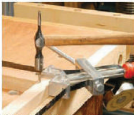
8 With care, you can tap the V nails fully home with a pin hammer
