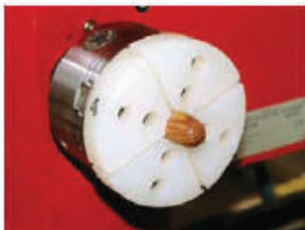
11 Nylon jaw plates can be adapted for a particular job and are extremely useful. Here they are shown holding a thimble.
