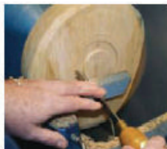
3 Cut a dovetail and spigot on what will become the underside
