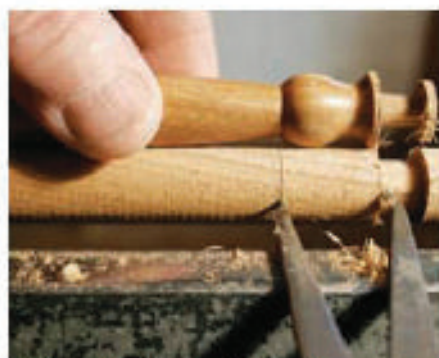
17 Use callipers to transfer dimensions from one column to another
