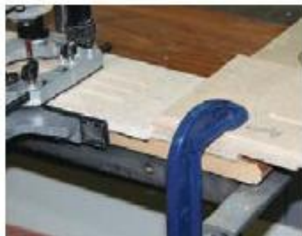
2 Use a suitable step to ensure the flutes are level with each other
