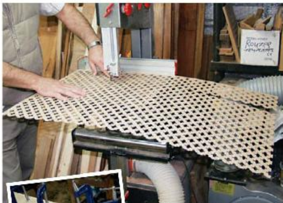
9 Cut the fret panels to size and paint them before you fit them
