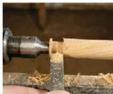
11 Reduce the blank to a cylinder and cut a shoulder at one end
