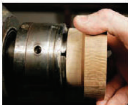
6 Reverse the blank and wind it up tightly on the screw chuck
