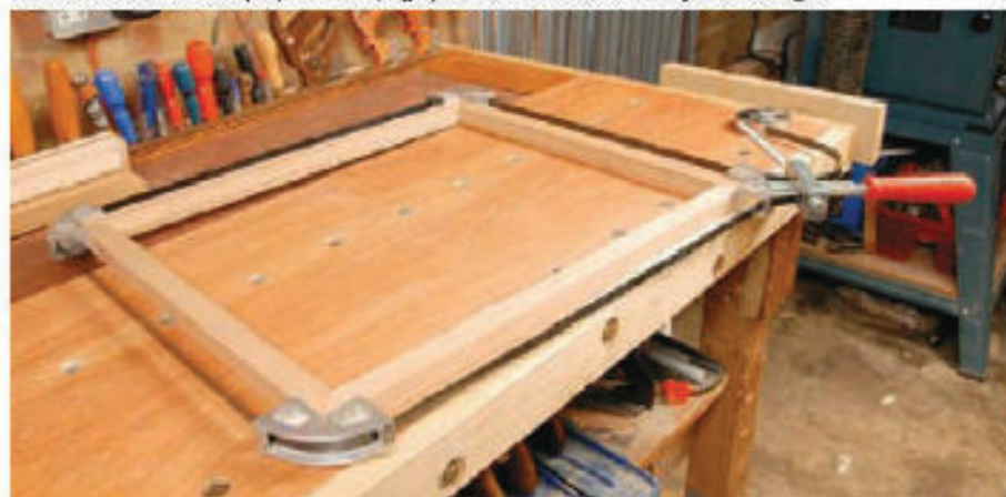
6 Dedicated frame clamps (see detail, right) ensure the corner mitre joints are tight
