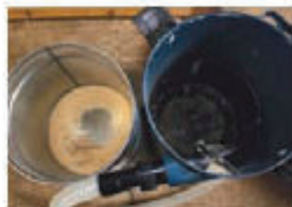
All the dust drops into the Dust Deputy, none in the vacuum
