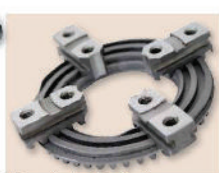
3 The scroll on the front of the disc drives the action of the jaw carriers
