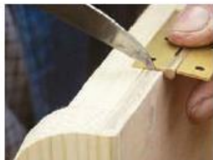
37 Mark both sides of the hinge with a knife
