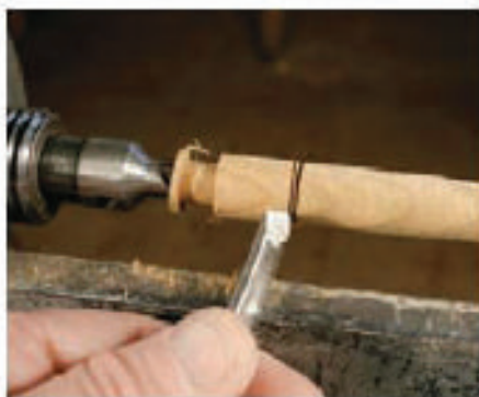
13 Slice a V cut at each end of the column with a skew chisel
