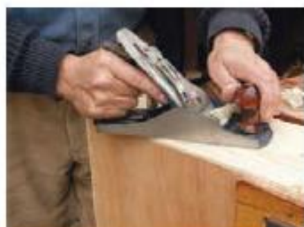
24 Trim all the frame edges with a plane
