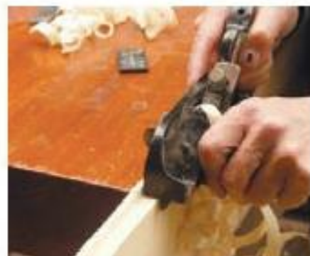
1 Cut the two rebates first...
