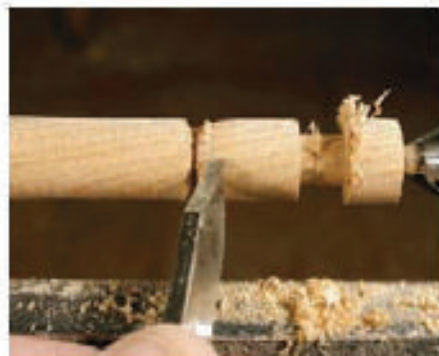
14 Round off the bottom of the tulip shape with a parting tool
