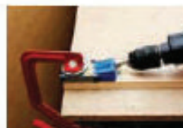
3 Drilling pocket holes in the workpiece
