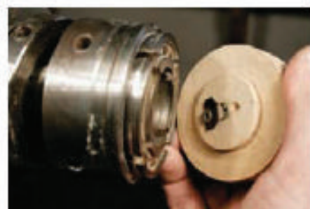
5 The rear of the screw chuck showing the screw locking plate
