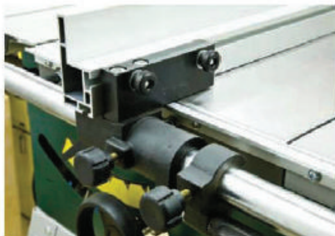
The rip fence assembly is connected to a solid steel rail at the front
