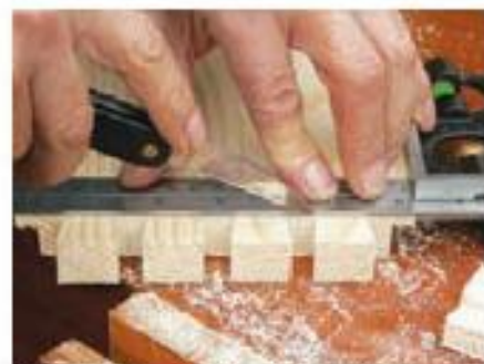
10 Mark the shoulder line for final trimming
