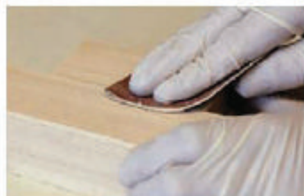
3 Lightly abrading the surfaces you're sticking with 100 grit paper gives a better bond
