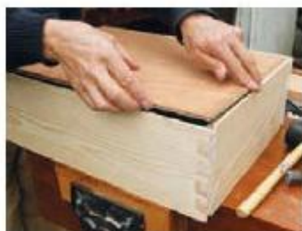
19 Cut the rear skin and test its fit
