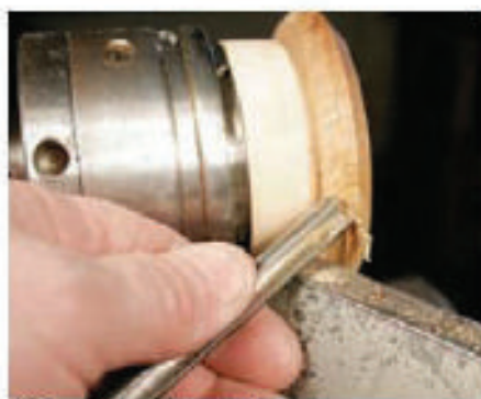
9 Form the top chamfer, then cut the under-chamfer in the same way
