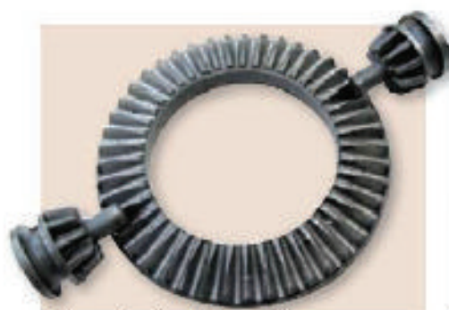
2 The gear teeth on the rear of the disc engage with the two pinions
