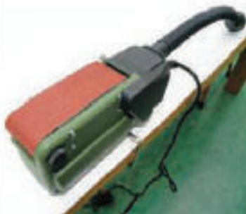
A simple clamp secures the sander to the workbench when required
