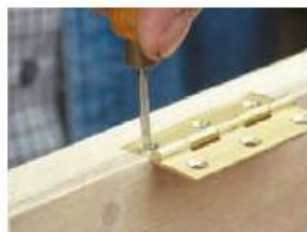
41 Use a bradawl to start the screw holes
