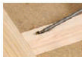
4 Driving screws by hand or with a cordless driver
