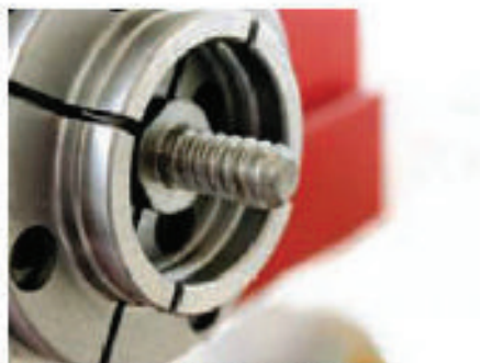
12 A screw insert is usually included as a standard accessory with any chuck.
