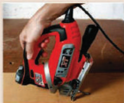
1 Position the tool nose-down with the blade over the waste part of the workpiece. With the blade clear of the workpiece squeeze the trigger and wait for the tool to get up to speed
