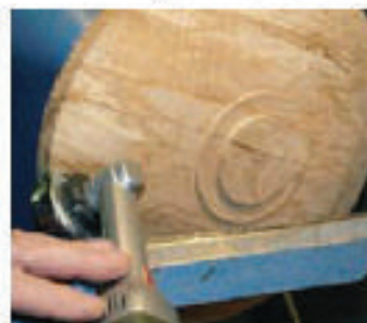
6 The long neck allows you to hold the grinder on the tool rest
