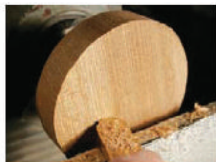
2 Use a round-nosed scraper to flatten off the face of the discs
