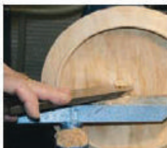
16 Finish the recess with light cuts using a round-nosed scraper
