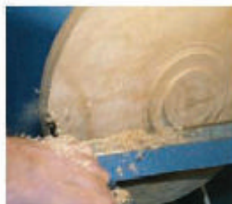
5 ...and repeat the process to clean up the underside of the rim
