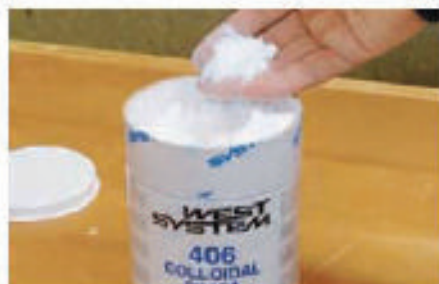
4 Colloidal silica is one of the fillers that can be used with epoxy resin adhesives
