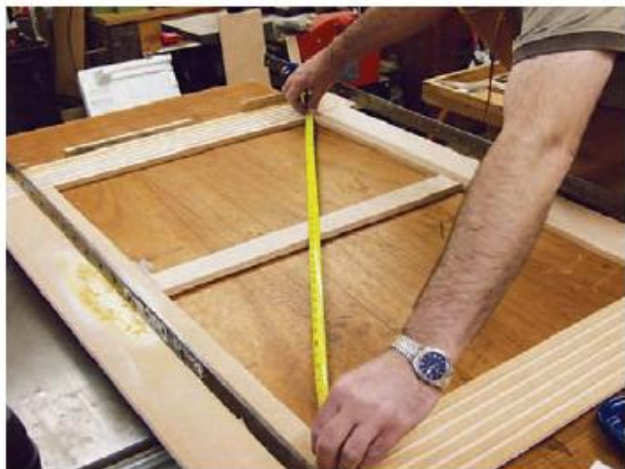
5 Check that the frame is square by comparing the diagonals
