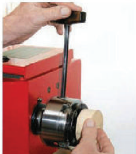
6 A single-key chuck has the advantage that the work can be held with one hand and the key rotated with the other
