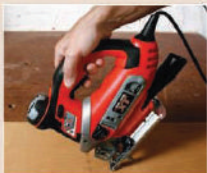
2 Gently tilt the jigsaw back so that the blade begins to cut the surface. Don't press hard; otherwise the blade action may cause the tool to dig in and jump upwards. Let it dictate the speed of the plunge
