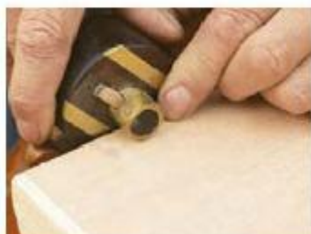
39 Mark the recess depth with a cutting gauge
