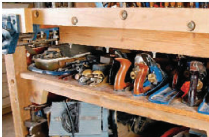
Bolting bracing beams under the top prevents it sagging
