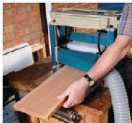
1 The first stage in making your own mouldings is to thickness the stock
