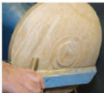
4 Shape the underside to an ogee shape, taking the finest shavings
