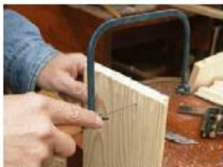
8 Trim out the waste with a coping saw
