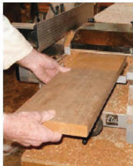
2 Thickness the bottom rail...
