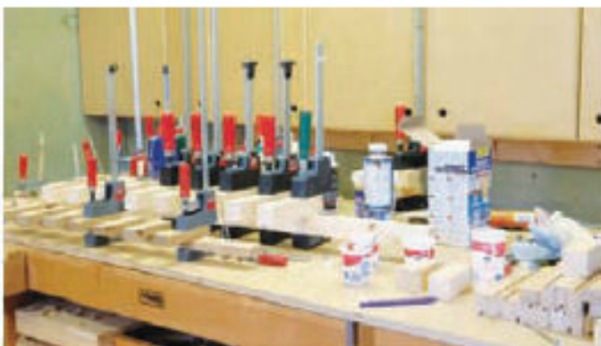
1 I've made a large number of test joints using the different adhesives on test
