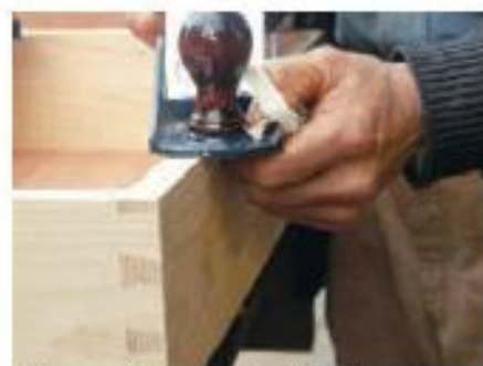
30 Remove the saw marks with a plane
