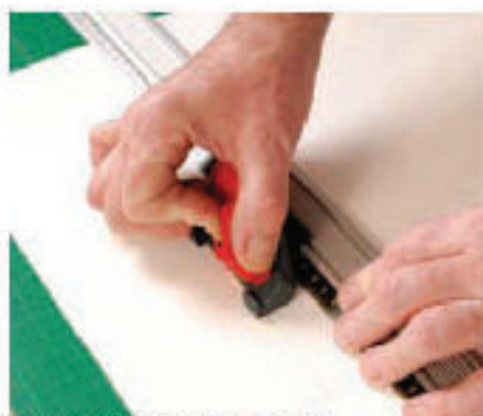
13 Depress the blade and draw it along the line to make the mitre cut
