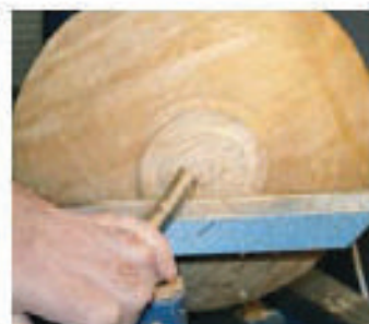
19 Turn the spigot away carefully and sand the foot smooth
