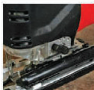
Extraction tube clipped in place
