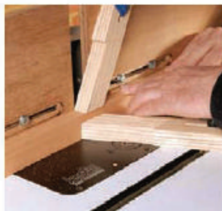
3 Using fingerboards on the router table ensures consistent, accurate results
