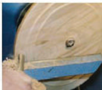
12 Reverse the bowl on a four-jaw chuck, shape the rim and form a bead
