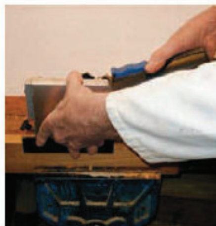
4 Cut the slots with the biscuit jointer
