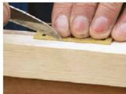
38 Then run the knife along the hinge edge
