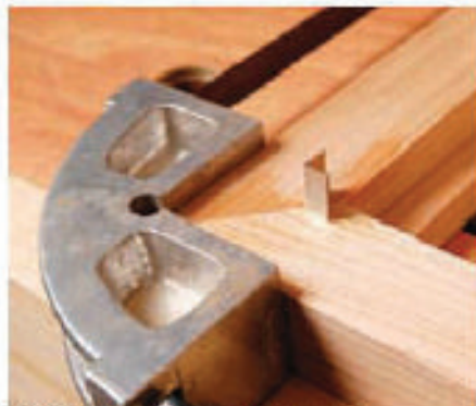
7 A V nail in position over the corner joint, ready to be driven home
