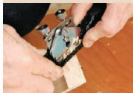
Two screws give good blade adjustment
