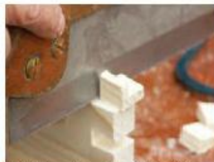
9 Cut off the outer sections with a dovetail saw
