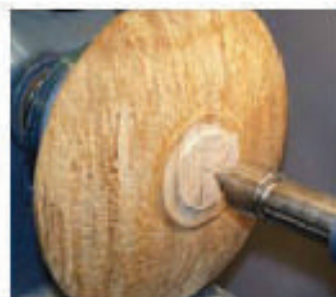
18 Reverse the bowl onto the vacuum chuck and remove the tailstock
