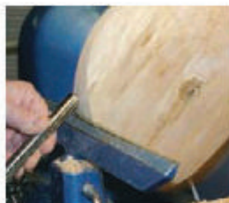
2 Reverse the blank onto the screw chuck and turn it to round
