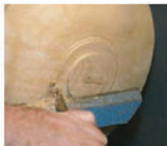
8 Use a narrow parting tool to cut through the texturing near the foot...
