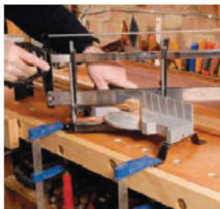
4 Cut the first mitre at one end of each frame component...
