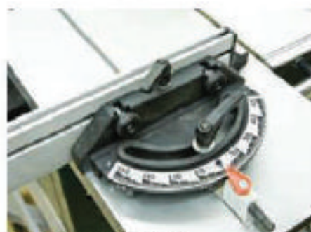
The crosscutting assembly is attached to the sliding beam
