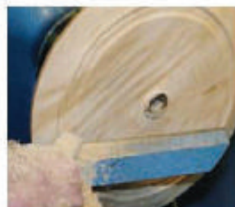
13 Use a skew chisel to form a groove in which to locate the bowl gouge
