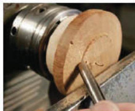
8 Slice across the top surface of the disc with a gauge
