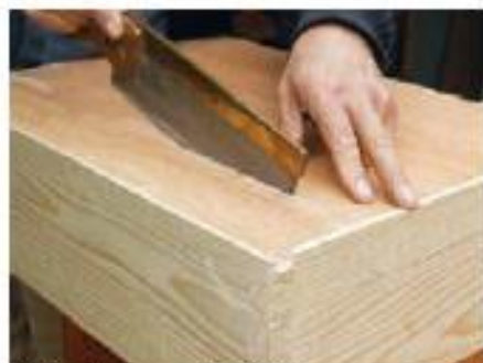
27 Start the separation with a tenon saw
