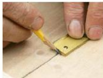
36 Mark the hinge positions on box and lid
