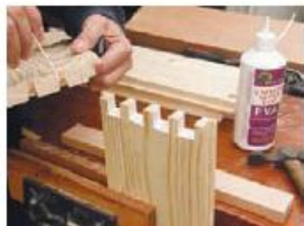
17 Glue up the frame corner by corner
