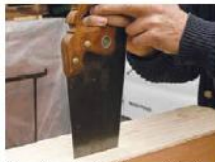
29 ...and complete the cut to separate the lid
