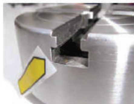
1 The T slots for the jaw centers should be rounded off smoothly
