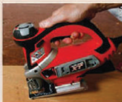
3 As the blade works through the thickness of the material, slowly slide the machine forward a little to increase the clearance on the end of the blade. When the blade breaks through, pull the jigsaw back a fraction and let it settle down onto the workpiece
