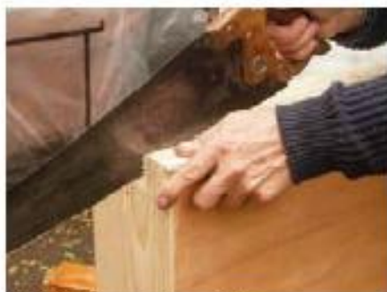
28 Switch to a panel saw at the corners...
