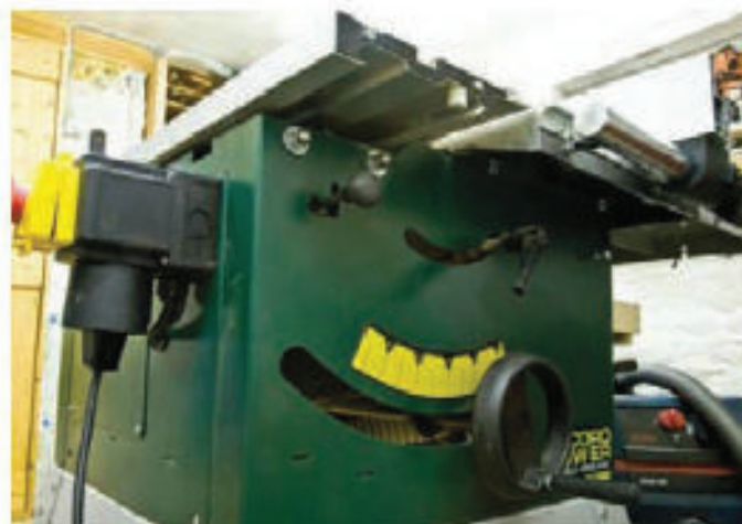
The saw body is of fabricated steel
