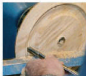
14 Deepen the cut with the gouge to undercut the rim slightly
