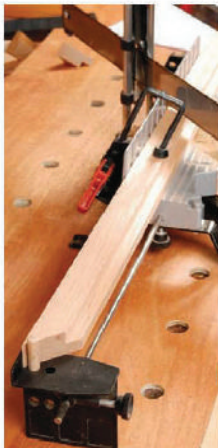
5 ...then use the end stop to give precisely matching lengths
