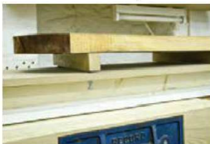
16 Rest a board on the jig and adjust the rails to support it (see panel, right)
