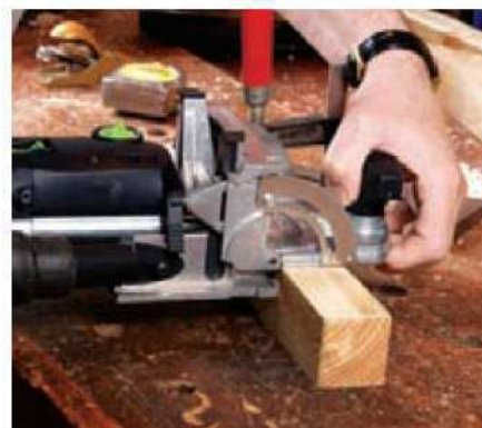
19 It machines slots rather like a biscuit jointer
