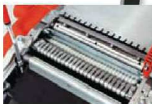
The cutterblock and drive mechanism showing the serrated feed roller and anti-kickback pawls
