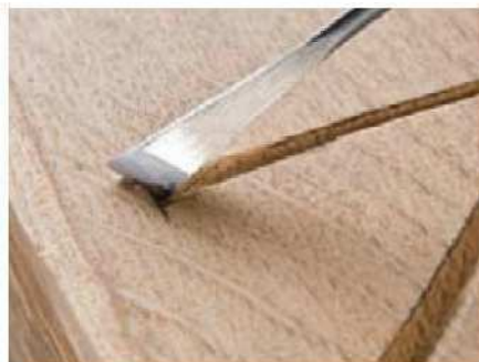
10 A skew chisel is useful for cleaning letters and forming serifs
