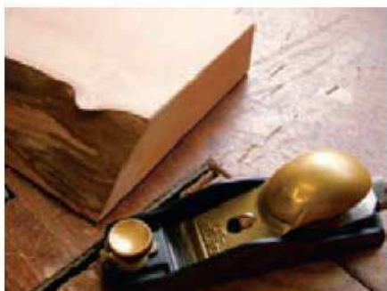
9 I applied delicate chamfers to the top edges with a block plane
