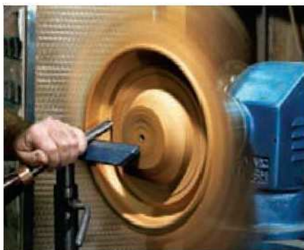
14 Hollow out the bowl interior, but take care to avoid the whirling wings
