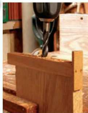
11 A typical jig tailored for just one job, then discarded
