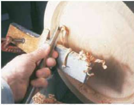
9 Use a bowl gouge to hollow out the underside, then check the depth of the recess
