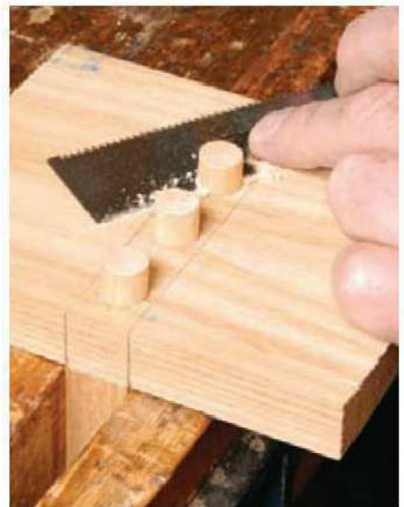
5 Once the glue has set, trim the dowels flush with the surface using a fine saw
