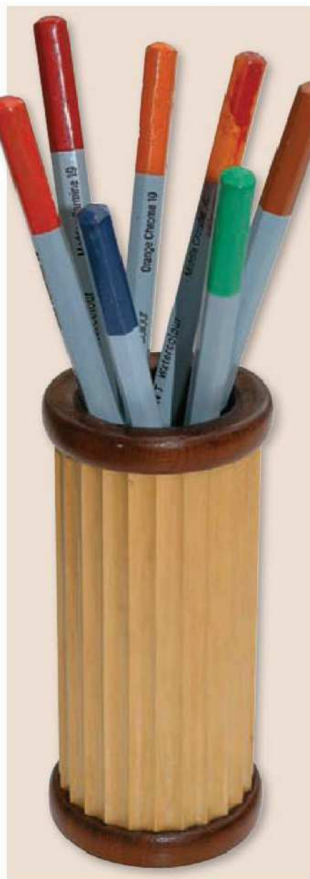
8 The cylinder is hollowed out and a top and bottom are added to make a pencil pot
