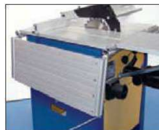
The side extension folds down for easy transport
