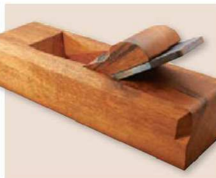
21 Finish the plane by applying two coats of boiled linseed oil, then wax it and buff it up
