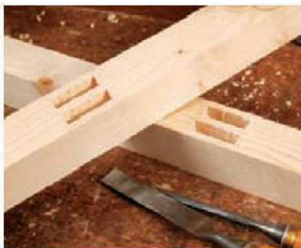
4 The finished double mortises should be clean and crisp
