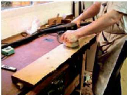
6 My random orbit sander produced a glass-smooth finish on the top
