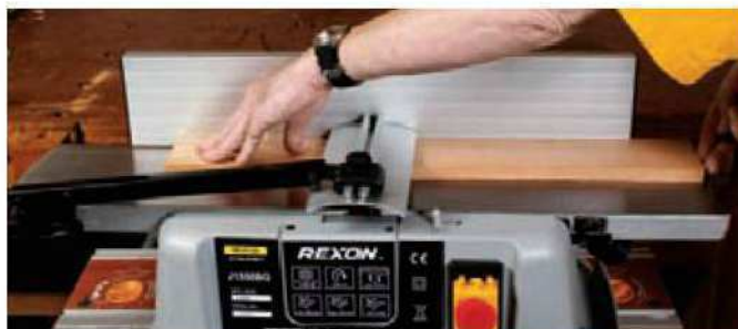
3 Transfer your front hand onto the workpiece on the out-feed table. Hold it down securely to ensure accurate planing. Continue to push the workpiece from the rear, but don't push it down onto the in-feed table
