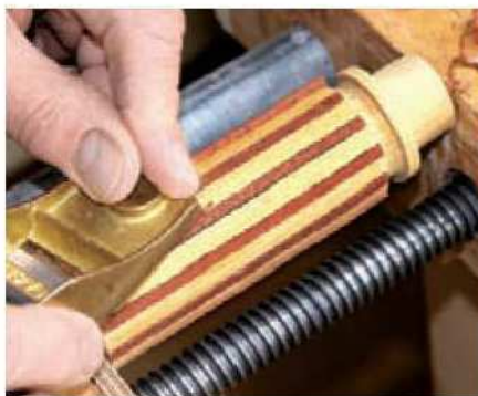
16 Planing off the surplus mahogany flush with the cylinder to create an inlay
