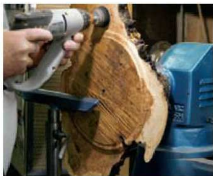
13 Power-sand the top surfaces of the wings before carving them
