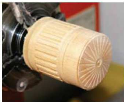
12 You can use the same technique to flute a box on the lid and sides...
