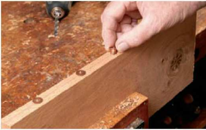
2 Drill one set of holes and insert the dowel centres
