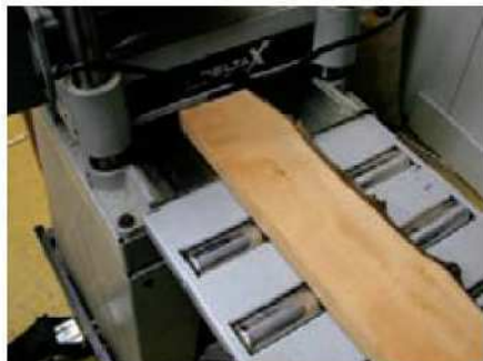
5 I ran the opposite face through the thicknesser to get it flat and parallel
