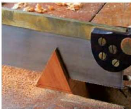
12 Clamp the block in a vice and cut to the waste side of the lines
