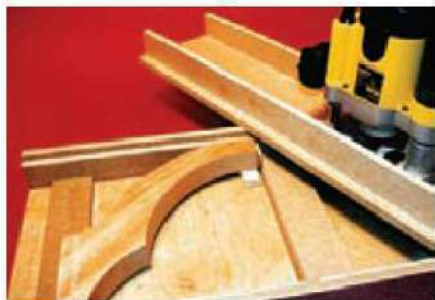
7 Use a simple jig to hold the legs while you taper them with the router
