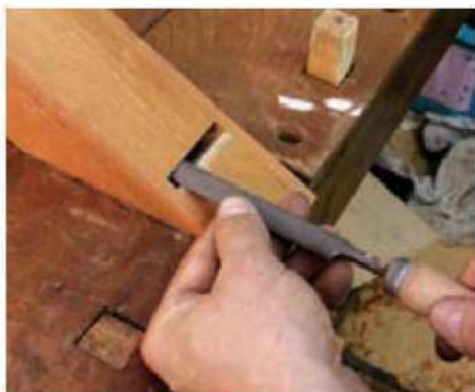
19 File the wear strip until the iron just peeks out of the mouth
