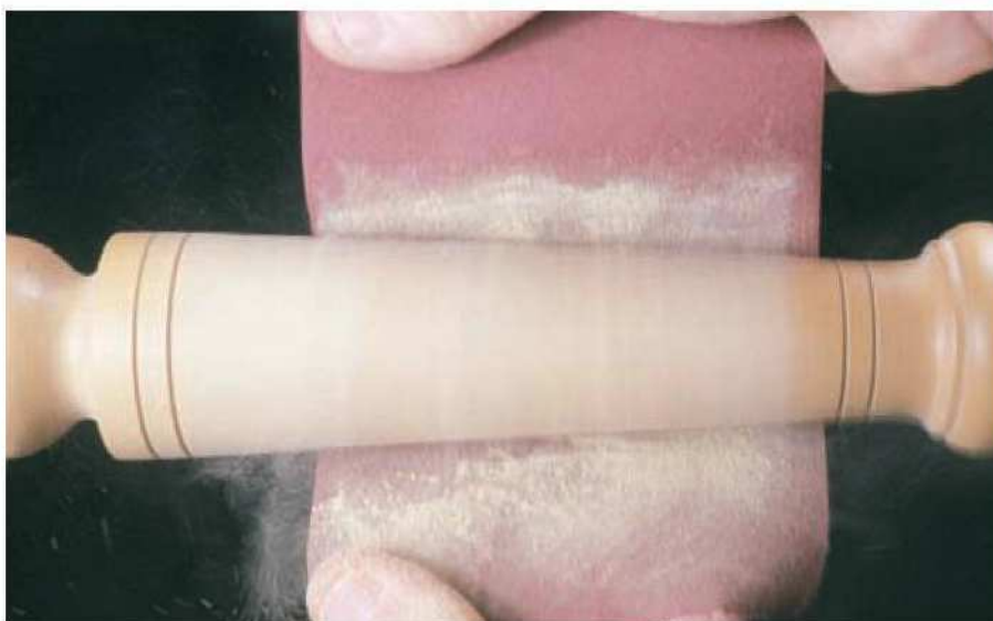
5 Sand a straight taper with a wide strip of abrasive paper
