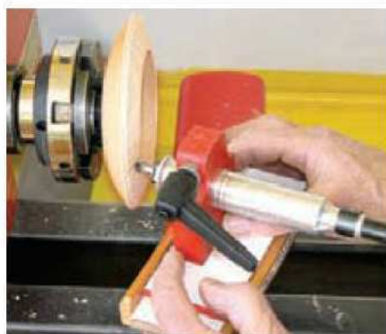
10 Angle the table as required to cut the flutes on the rim of a dish.
