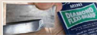
Use a diamond shim to take the roundness out of the bottom of the V
