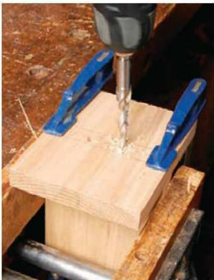
3 I found it easiest to clamp the joint and drill the holes for the central dowels first
