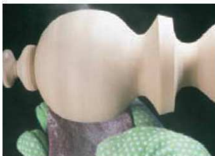
9 Keep your fingers flat against the workpiece when sanding in gloves
