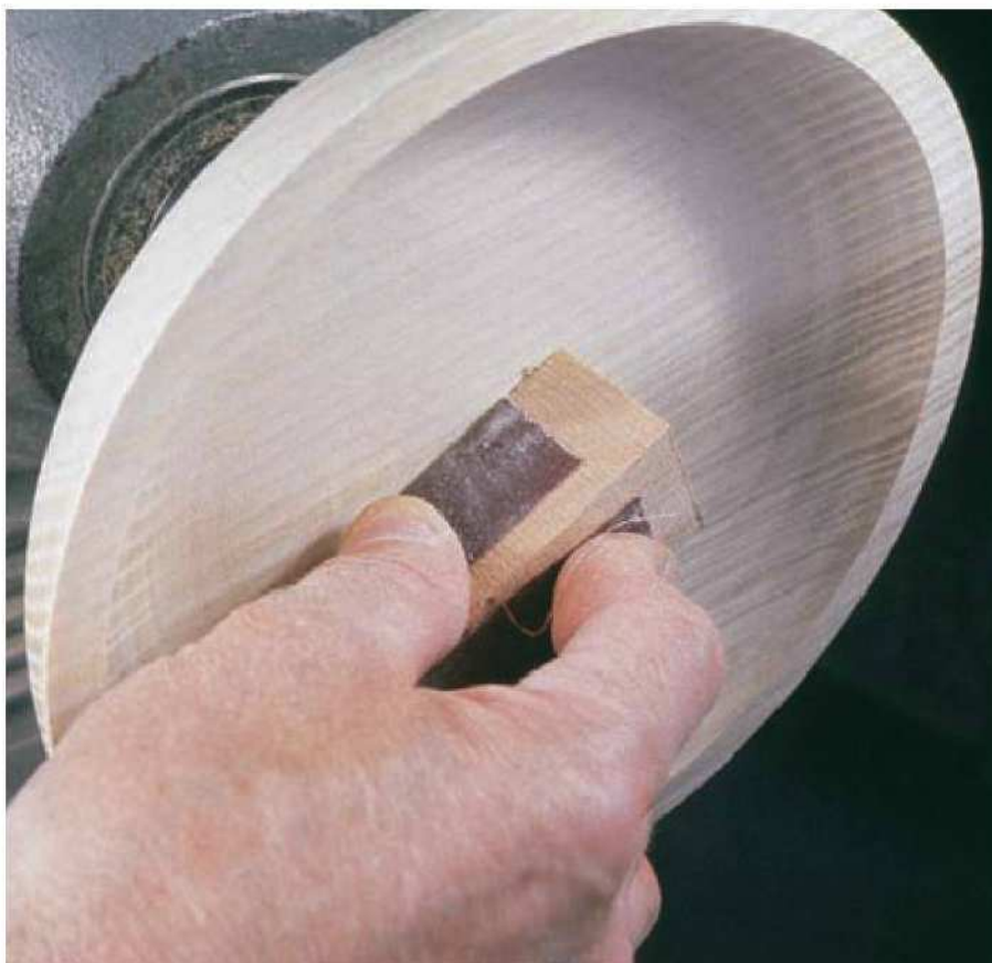
3 Sand the floor of the bowl flat using a small sanding block
