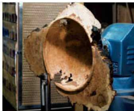
15 Sand down to 400 grit, then seal and polish the interior
