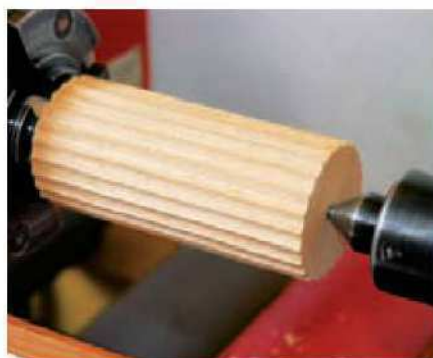
7 After working all the way round the cylinder, the flutes are complete
