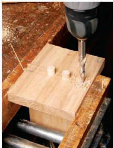
4 After inserting these dowels, I drilled the outer holes and completed the joint
