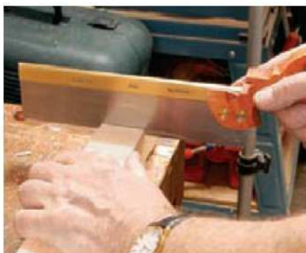
8 Cut the outside shoulders of each tenon with a hand saw
