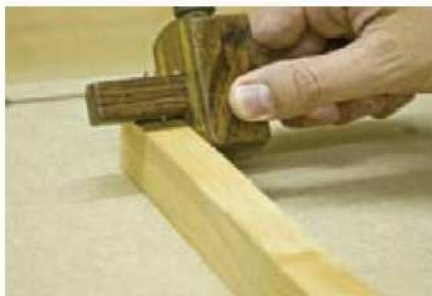
11 Mark the centre line on each rail with a marking gauge
