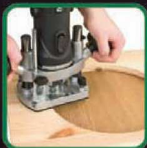
Template routing with a guide bush.
