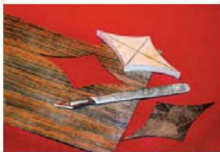
4 Make an accurate MDF template for the rosewood inserts
