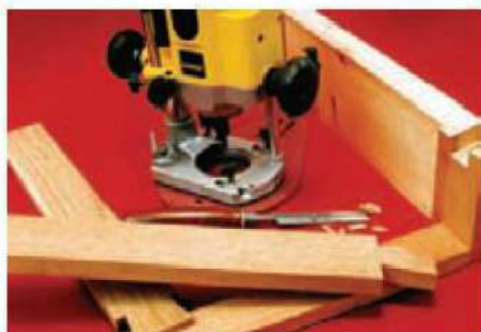
1 Dovetail joints are used to assemble the casework.
