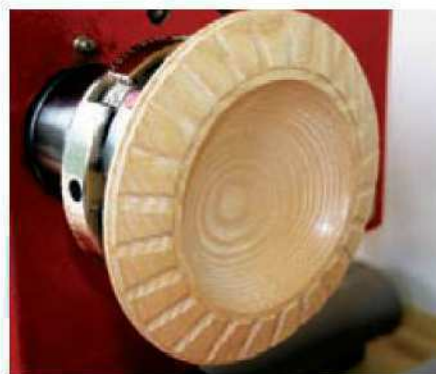
11 The completed dish, ready for its final sanding and finishing
