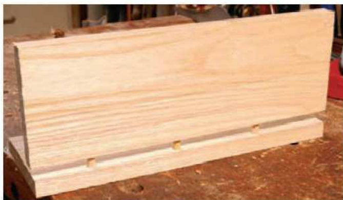
9 This type of jig guarantees accurate hole alignment
