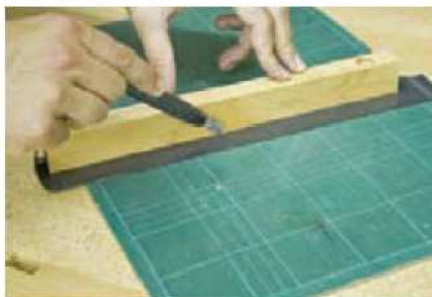
14 Stick grip tape to the opposite face of each rail and trim it flush with a sharp knife
