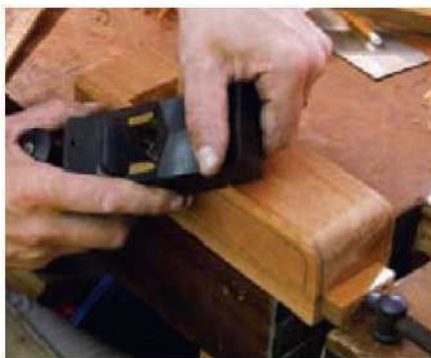
20 Mark out the chamfers on the plane body and trim them with a block plane
