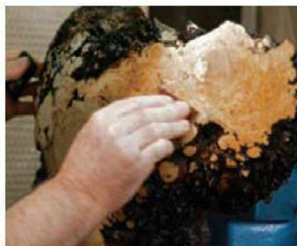
9 Use wet and dry paper dipped in paste wax to smooth the surface
