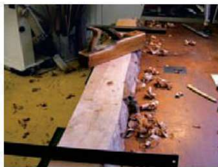
4 I flattened one surface by hand-planing it to remove any wind
