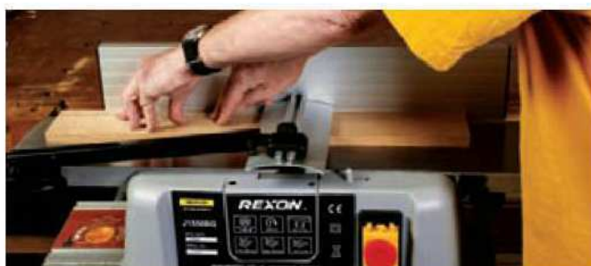
4 Finish with both hands on the out-feed table. Never let your rear hand get too close to the cutterblock
