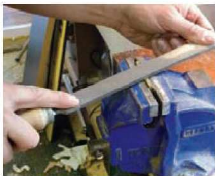
11 Rough-cut a piece of brass to fit the rebate and file it down to size
