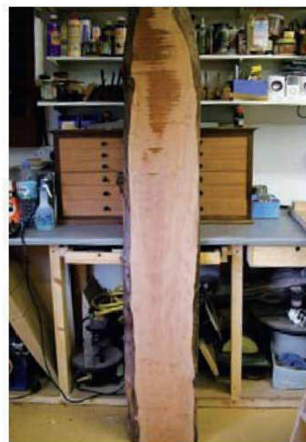
1 I let the plank acclimatise in the workshop for several months to ensure that it was dry
