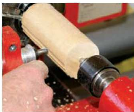
6 Reversing the direction of cut to clean up the flute
