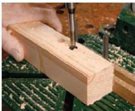
1 Use a Forstner bit in a drill stand to cut the mortises
