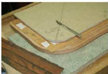
10 Make an MDF template to cut the veneer corners to shape
