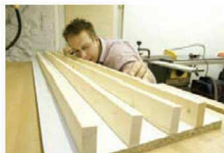
2 Aligning the battens by eye and mark their positions lightly in pencil
