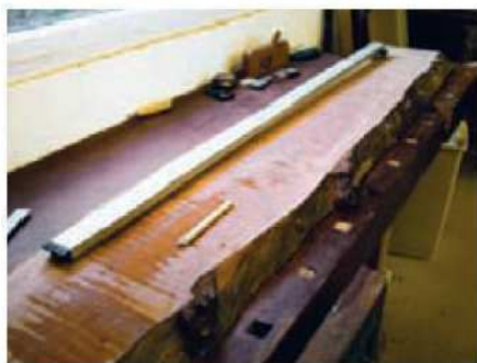
2 A long straightedge made marking out the shelf a simple job
