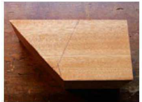
7 Mark the sides to define the throat position
