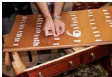
9 Tape the veneer sheets together before laying them on the tabletop
