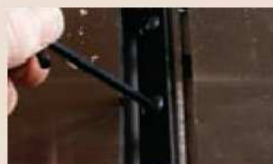
Loosen the knife clamping screws
