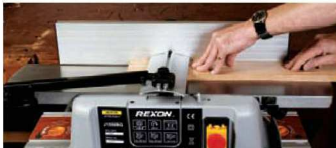
2 Continue to feed the timber through the machine and onto the out-feed table with steady forward hand pressure
