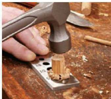
16 Hammer the dowel through the plate and into a dog hole in the workbench
