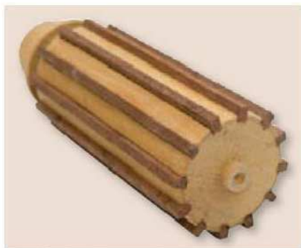
15 Strips of mahogany glued into square grooves cut in a cylinder
