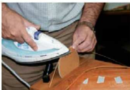
11 Bend the stringing around a curved former with a hot iron
