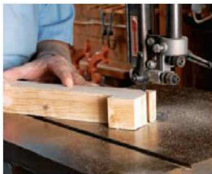
10 Glue on the foot blocks and shape them on the bandsaw
