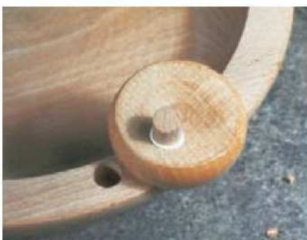
13 Glue the dowels into the feet, then fix them into matching holes drilled in the stool frame
