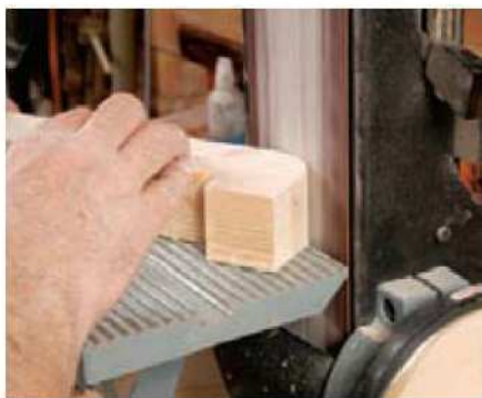
11 Sand the foot blocks and the tops of the uprights to shape
