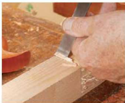
7 Use a chisel to define the edges of the shoulder lines
