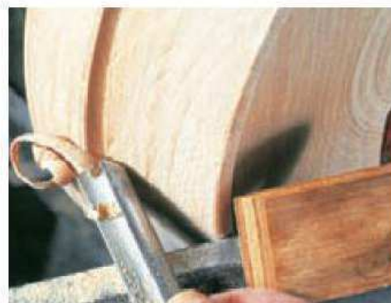
6 Cut a step in the side about 25mm up from the base of the frame
