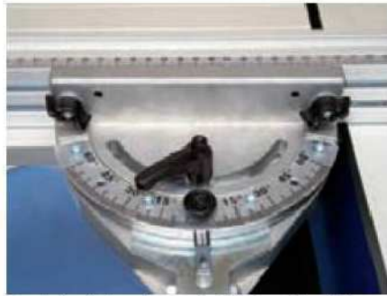
A substantial protractor is fitted on the sliding carriage fence
