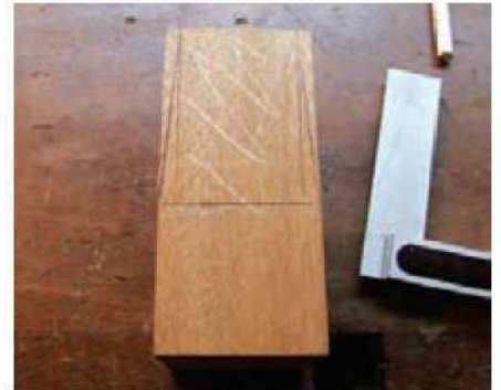
6 Mark the throat position on the top face of the front block
