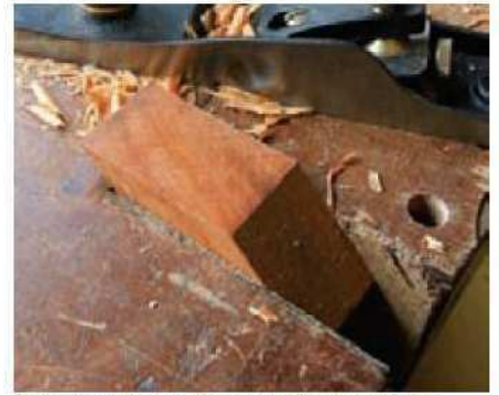
4 Clean up the angled end of the bed with a block plane
