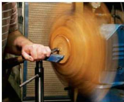
16 Reverse the burr onto a vacuum chuck and remove the spigot
