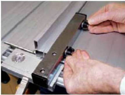
The rip fence adjusts backwards and forwards
