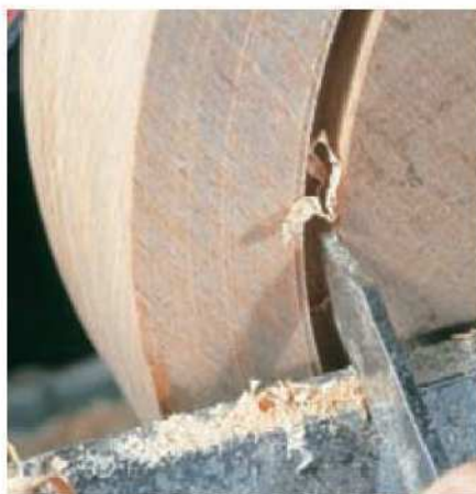
2 Cut the outer perimeter groove with a parting tool and check the depth
