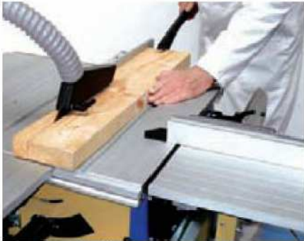
Ripping stock with the crown guard dust extractor in position
