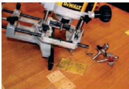
14 Cut the recesses for the table hinges using a router
