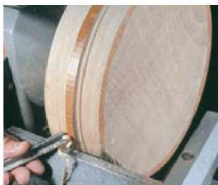
1 True up the rim of the disc with a bowl gouge, slicing in from each edge in turn
