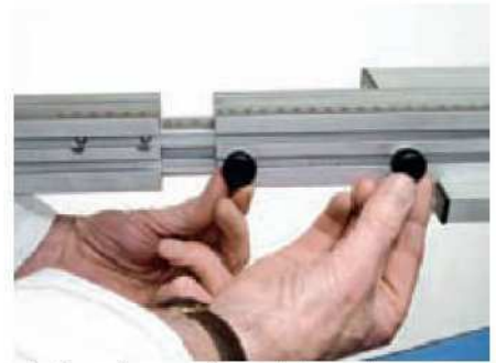
The fence has easy-to-use telescopic extensions
