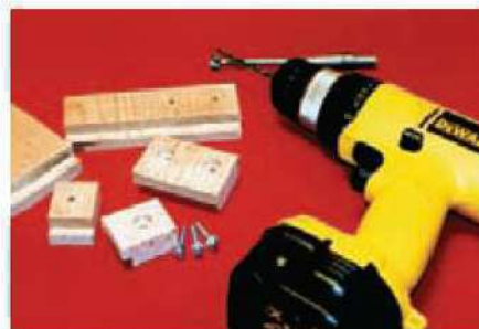
15 Make the buttons used to secure the top from a strip of softwood
