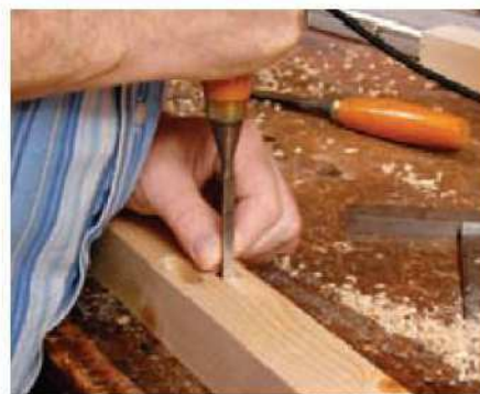
3 Square up the ends of each one with a chisel
