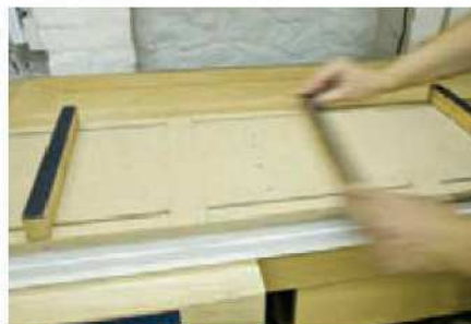
15 Fit the rails onto the bolt tails in the jig and check that they move freely
