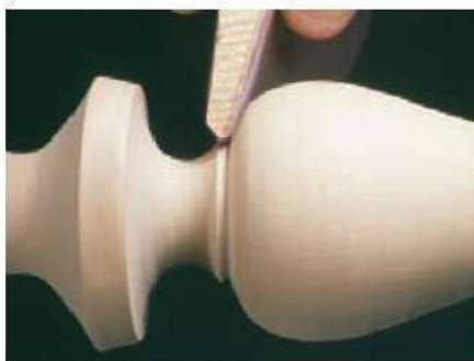
8 Fold the abrasive round a wedge block to sand a small fillet
