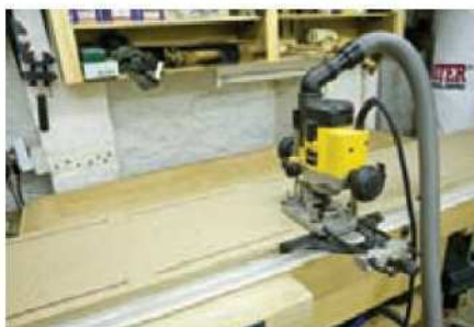
8 Use the router to cut a series of slots in the top board. Note the gaps between the slots
