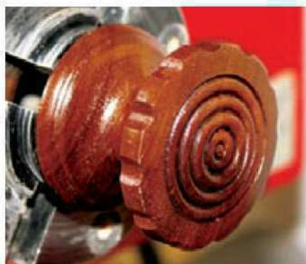
9 Cutting short flutes cut around the rim of a turned knob
