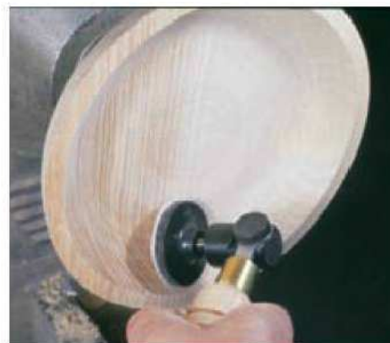
4 Use a free-wheeling sanding disc that matches the bowl's curvature
