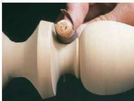
7 Wrap the abrasive cloth round a dowel when sanding a deep curve
