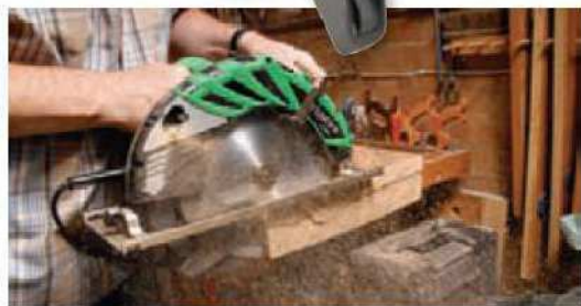
The saw cut an 85mm thick slab of oak with ease
