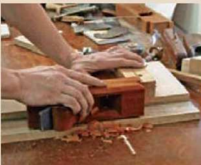
2 Slide the plane forward and through the cut
