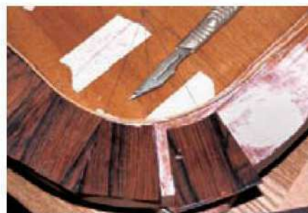
12 Cut the cross banding into small wedges to fit round the curves
