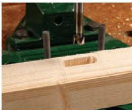
2 Remove the waste to leave a round-ended mortise
