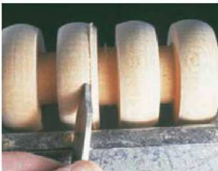
11 Shape the toe of each foot with a rolling and lateral cutting technique
