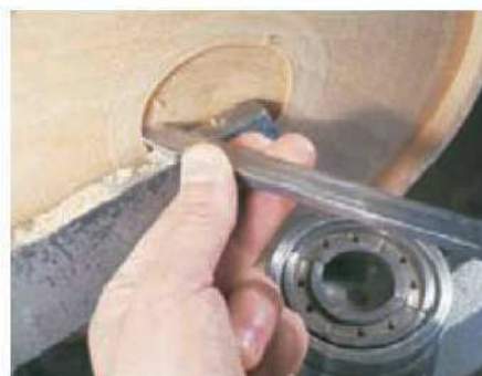
8 Take care to hold the dovetail scraper steady when forming the dovetail
