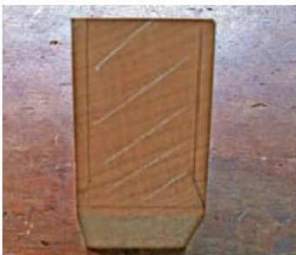
8 Complete the marking up of the abutments for the wedge
