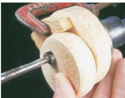
12 Use the lathe as a makeshift drill press to drill the dowel holes in the feet
