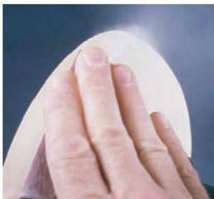
1 Change your abrasive as soon as the cloud of sanding dust disappears
