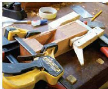
16 Glue and clamp the cheeks and centre blocks together and allow to set
