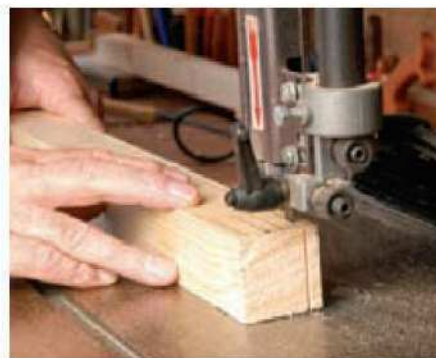
6 You can cut the tenons very quickly on the bandsaw
