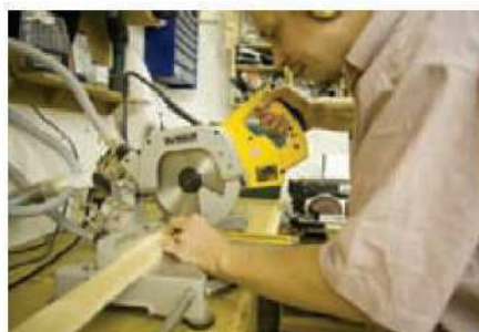
1 Cut the four softwood battens to length from 45 x 19mm stock
