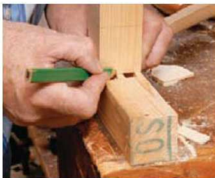
5 Mark the tenon widths directly from the mating mortises
