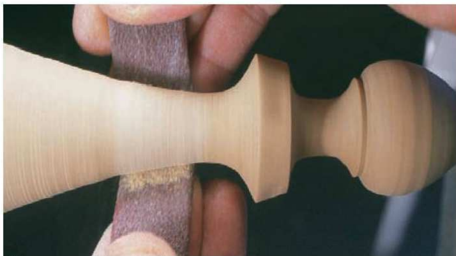
6 Use a narrower strip to sand shallow pear-drop curves
