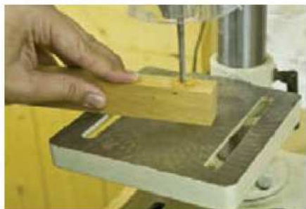
13 Drill a pair of 6mm holes 20mm deep at the marked point in each rail
