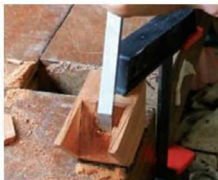
13 Use a chisel and mallet to remove the bulk of the waste wood
