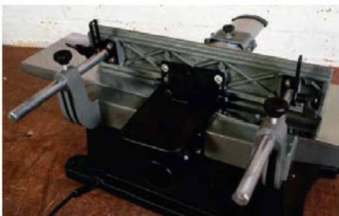
3 The fence support mechanism
