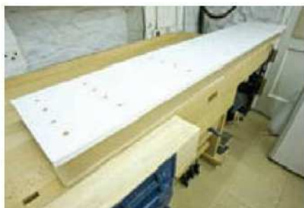
7 The partially assembled jig is now ready for its slots to be cut
