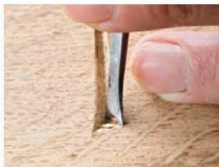
9 I've ground a 6mm no 3 gouge to an exaggerated fishtail, great for forming serifs
