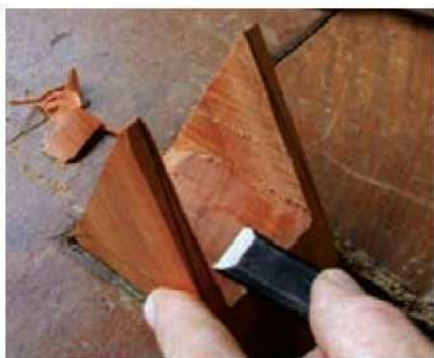
14 Clean up all the surfaces of the throat carefully with a paring chisel
