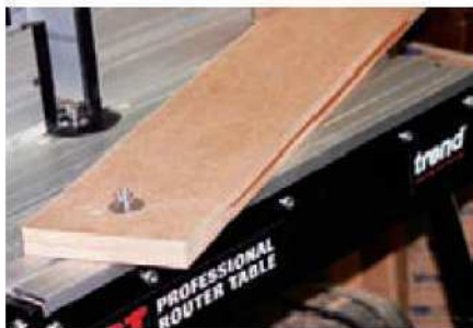
8 A simple MDF jig used to cut the veneers square and straight
