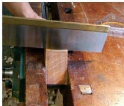
9 Make two saw cuts across the mouth to remove a small rebate
