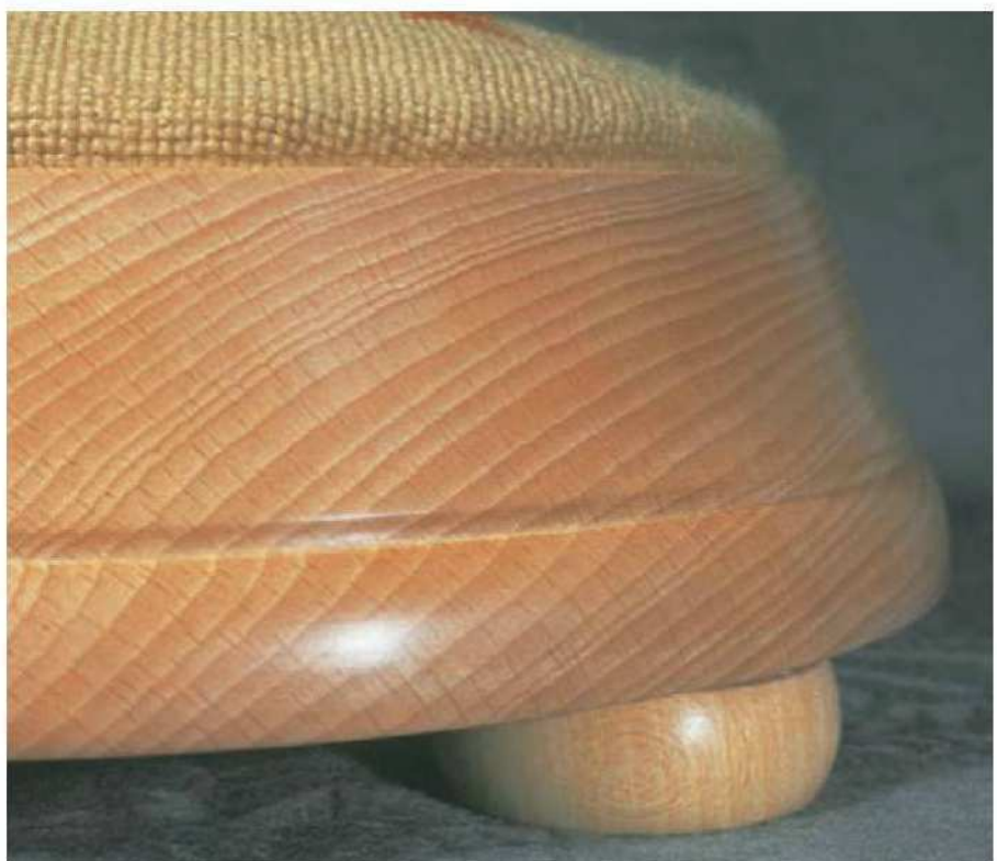
13 Glue the dowels into the feet, then fix them into matching holes drilled in the stool frame
