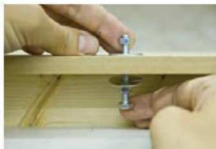
9 Fit an M6 bolt plus its various washers and nuts into each slot
