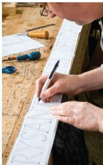
3 Transfer lettering from drawings, or a print out, rather than drawing directly on the timber
