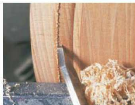
7 Use the same lateral cutting technique to round off the ovolo moulding
