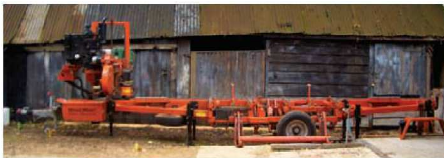
The Wood Mizer wedged in the milling position
