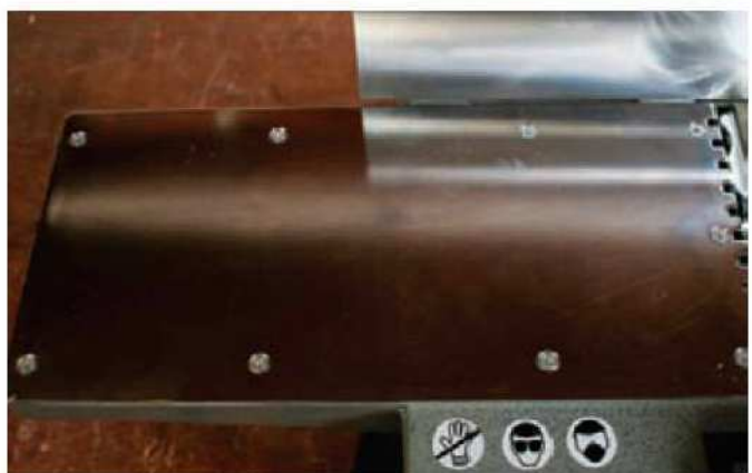
2 The steel-surfaced out-feed table
