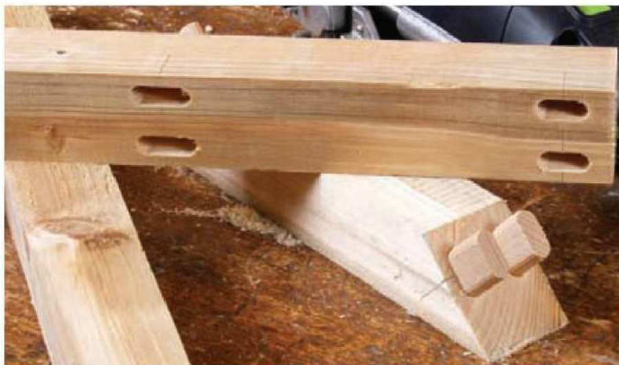
20 The Domino loose tenons make a secure joint
