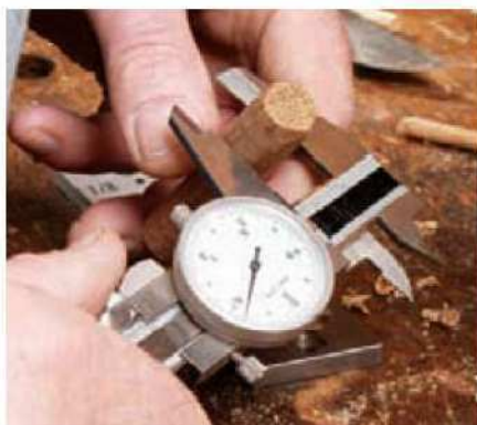
17 Check that the diameter of the dowel is correct before using it
