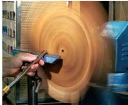
11 Turn the burr the other way round and true up the front surface
