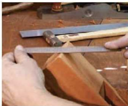
17 Round over the rear edge of the plane body with a rasp and smooth it with a scraper
