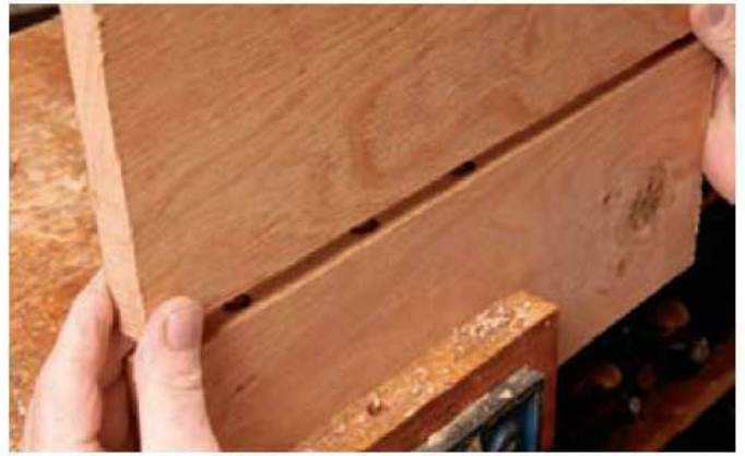
3 Align the second component and press it down to mark the hole positions
