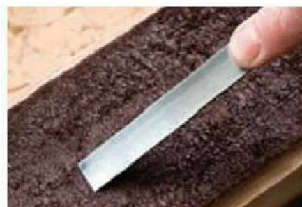
5 Keep your gouges razor sharp with a leather strop
