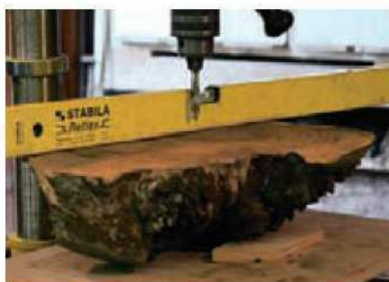
2 Try to get the hole for the chuck perpendicular to the upper surface
