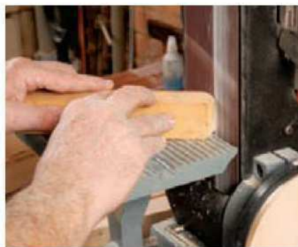
12 Use a rubber cleaning stick to maximise the life of the belt
