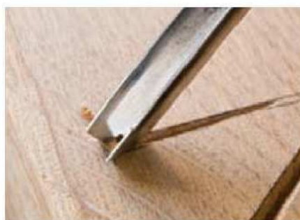
6 The V-tool can be raised at the end of the cut to start forming the serif
