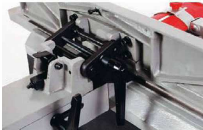
The fence's substantial adjustment mechanism
