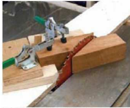
3 Cut the centre block on the table saw using a temporary sled
