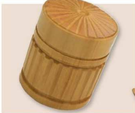
13 ...before adding some turned detail and then parting off the lid
