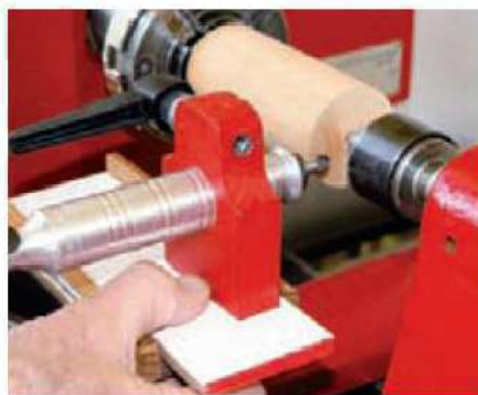
5 Making a fluting cut with the indexing pin set in the first position
