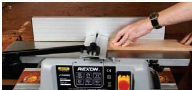
1 Start the machine and feed the timber slowly under the bridge guard and over the cutters
