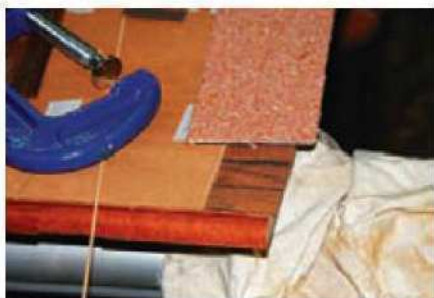
13 Pieces of carpet tile secure the cross banding without damaging it
