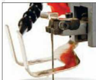
Standard blades with protruding pins are easily fitted
