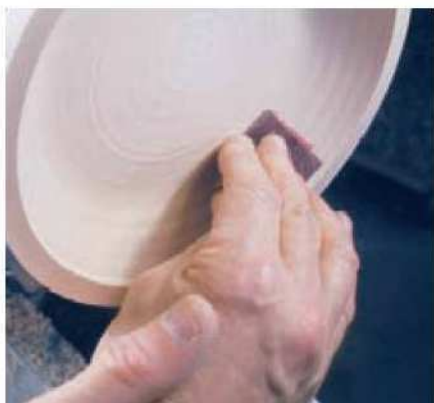
2 Draw the sanding pad up to the rim of the bowl, but not over it
