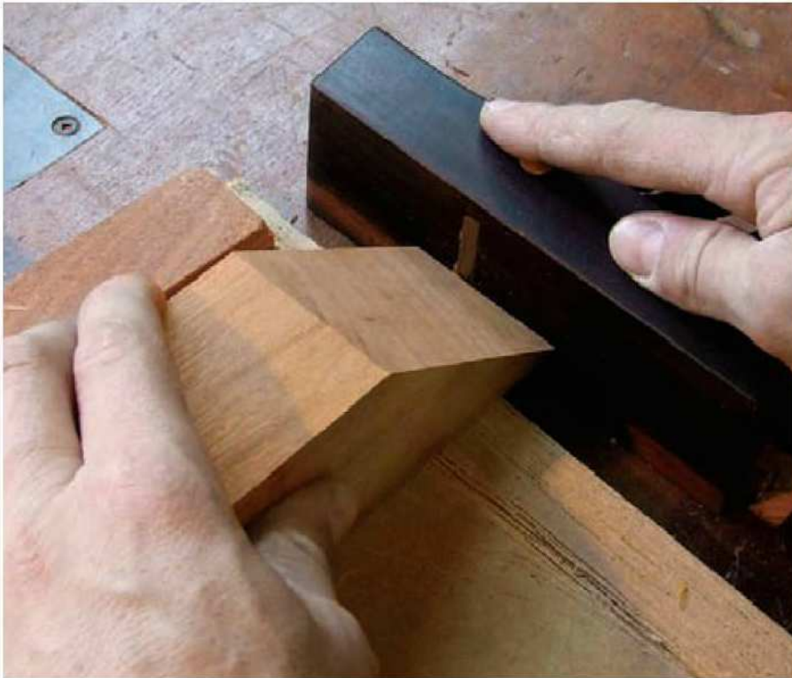
5 Cut a chamfer on the leading edge to stop it from chipping
