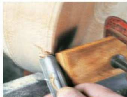
5 Use a plywood fence to support the gouge as you start to shape the sides
