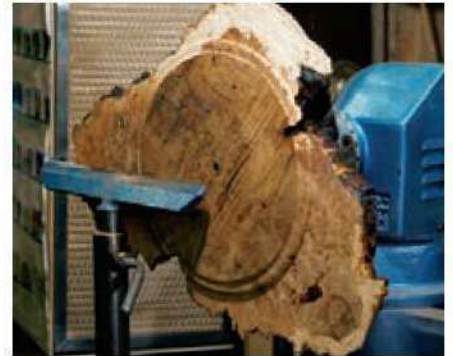
12 Carefully form the rim to mark out the bowl diameter
