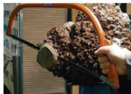
3 Balance the workpiece by removing unwanted lumps or adding weights
