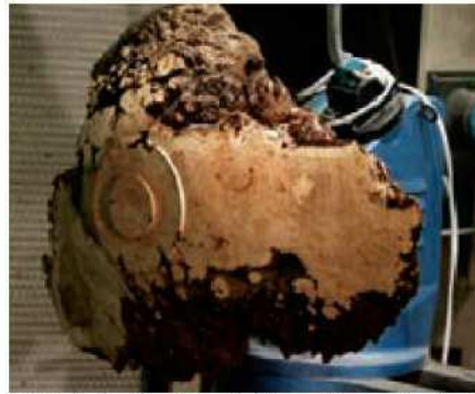
5 Finish shaping the outside and form a foot and spigot on it
