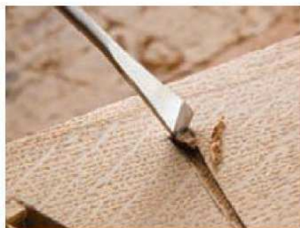
11 The skew chisel is also very good for cutting the end of the serif
