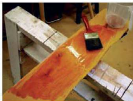
10 Applying three coats of finishing oil was a three-day process
