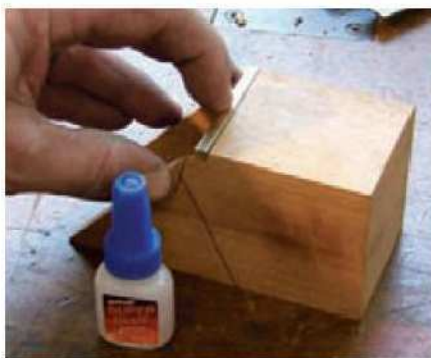
15 Glue the brass wear strip into the rebate in the front block with superglue
