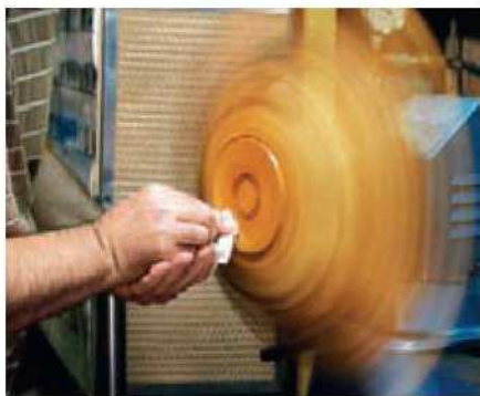
17 Finish shaping the foot, then seal and polish it as before
