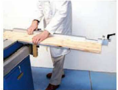
Cross-cutting a large board with the length stop in use
