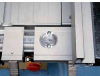
The fence anchor has fine micro-adjustment
