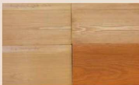
Four finishes on pine (clockwise from top left): English light oak stain; antique pine stain; antique pine varnish; Pine Antiquator
