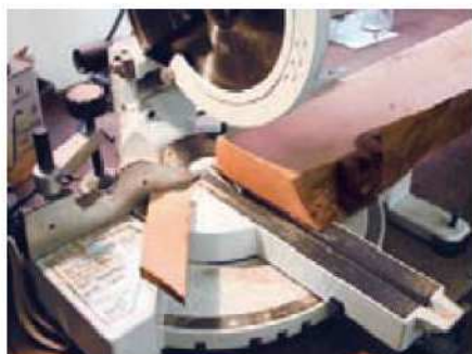
8 Final cutting to length was a straightforward job for the mitre saw
