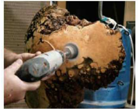
6 Power-sand the exterior of the bowl with the lathe stationary
