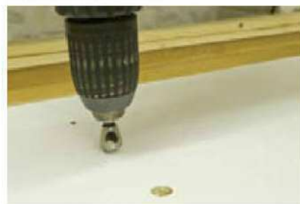
4 Drill through both boards at the same time and countersink the screw holes
