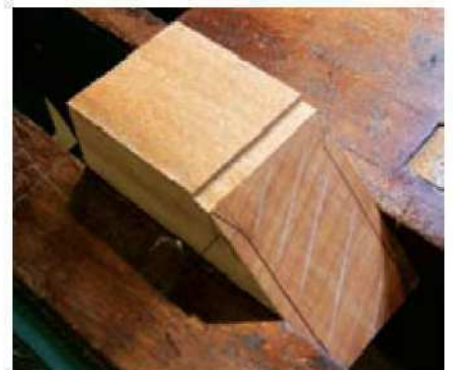
10 Clean up the resulting rebate with a sharp block plane
