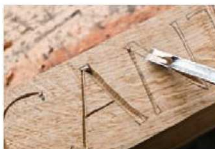
4 A razor sharp V-tool should cut across the grain of most timbers with little tearing
