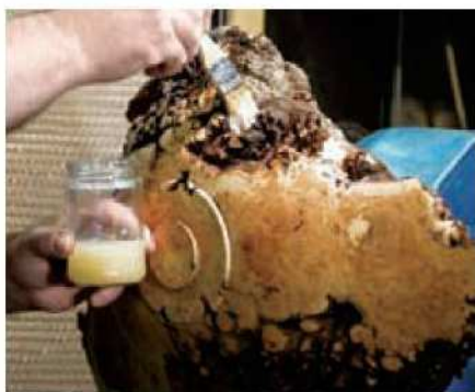
8 Paint on a generous coat of sanding sealer and leave it to dry
