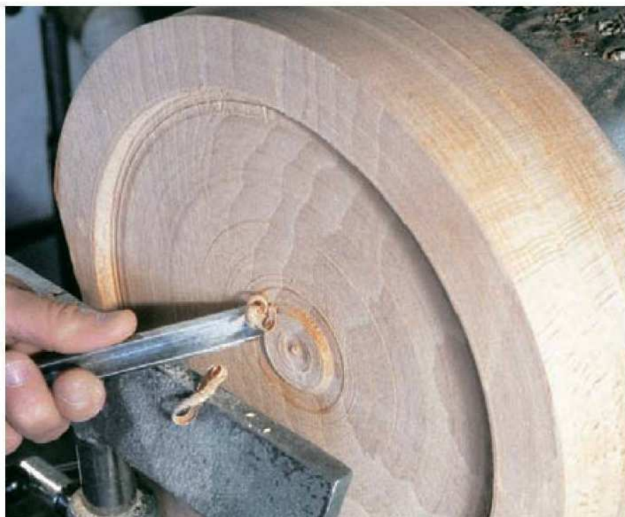
3 Then use the bowl gouge to remove the bulk of the waste from the recess
