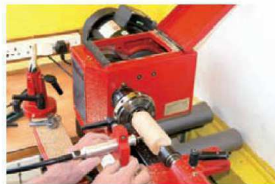
1 The Myford Mystro with the cover hinged back to set the indexing pin
