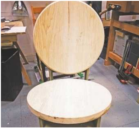
5 An MDF framework tested the seat position's geometry as well as helping to refine seat and back shaping to ensure maximum comfort
