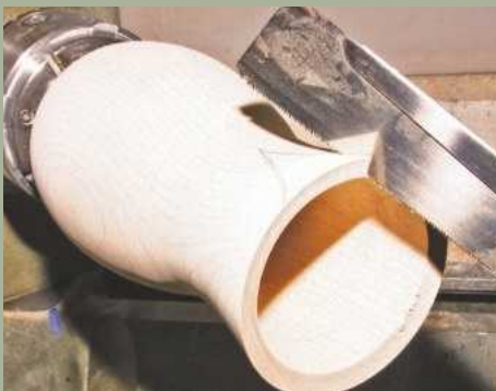
16 Using a fine kerf saw, start to cut away the unwanted area. Once the 'V' is removed, move on to tidying up the split using a file and abrasives
