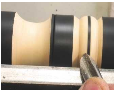
9 Cutting a bead with the gouge is very similar to cutting one with a skew, but due to the bevel angle, this won't give you a narrow cut to the side
