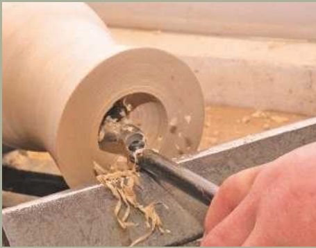
13 Use your chosen hollowing tool to remove the waste material – here I'm using a Rolly Munro mini hollower
