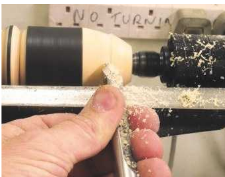
11 As the tool makes its way through the shape, you'll need to lift the handle as the wood gets smaller in diameter; this ensures the bevel is kept in contact with the wood
