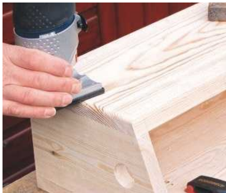
8 To soften edges, rout with a rounding-over or chamfer bit; fill nail holes and sand the box
