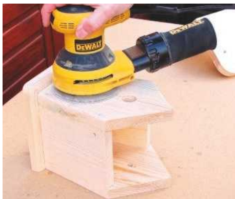
16 Sand the box and roof section, then remove arisises; add internal strips before fixing the roof
