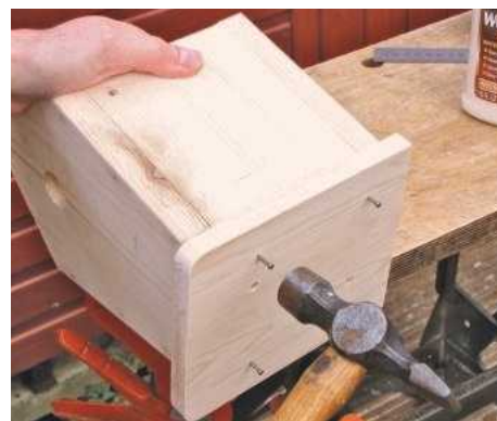
15 Glue and nail the box base in place, checking that the overhang on each side is identical; rear edges should be flush
