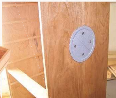
23 ... and drilled the steel back plate so that it could be screwed to the side panels
