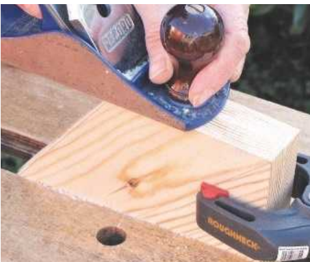
4 Cramp front and back together and trim upper edges with a bench plane, checking for square
