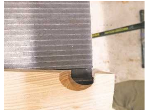
27 After dimensioning the blanks to square, the angled cope joint was cut on the spindle...
