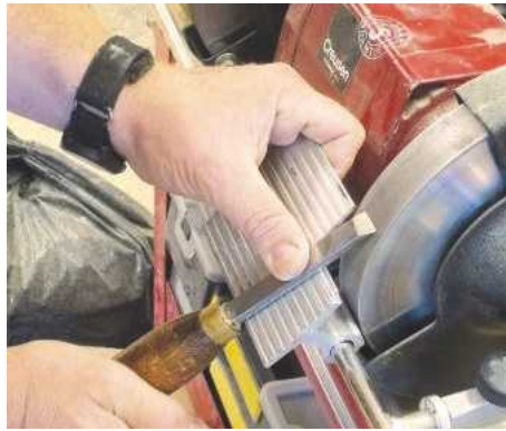
3 If you need to sharpen on a platform, try to get your hands in a position that allows you to slide the tool sideways
