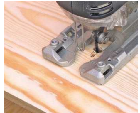
9 Drill holes in the back and saw to form keyhole slots; you'll need 5mm screws for this due to the box's weight
