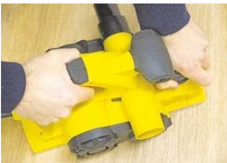
The CON950's handle makes using the adjustment knob more difficult when planing
