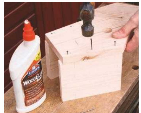
6 Glue and pin the front to the sides, followed by the back; pre-drill nail holes to prevent wood splitting
