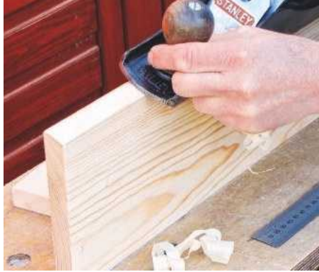
2 Saw front and rear panels to size, then, using a bench plane, bevel the top edge of both pieces to match the ends
