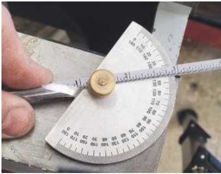
5 A good working angle on the spindle gouge is around 40°. Going to 35° would be better for shaping and 45° is better suited to hollowing
