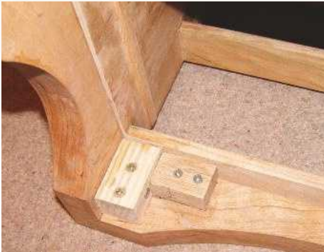
8 The plinth was attached by screwing through the bottom rails into blocks glued to the plinth's inner faces
