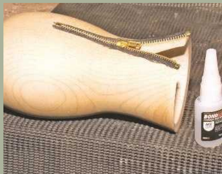
23 Using CA adhesive, glue the zip in place so that it corresponds with the 'V' cut out of the neck
