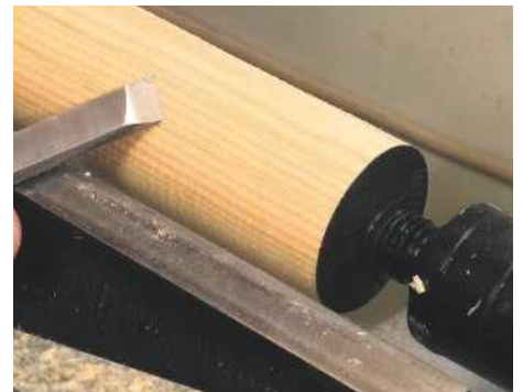
13 The spindle roughing gouge won't leave a great finish, especially on pine. The skew is now presented with its centre cutting and bevel rubbing
