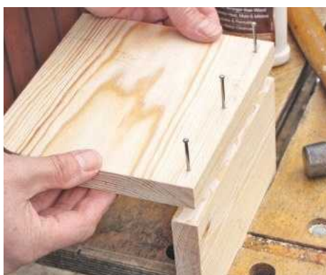
10 Glue and pin roof sections together at 90°; make the joint slightly proud and plane flush when dry
