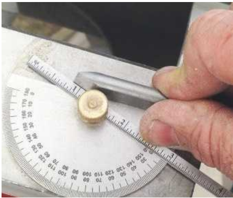
5 The tool is ground to an angle of around 20°; this will allow it to easily slice through the timber's fibres
