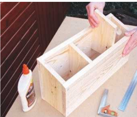
4 Check internal dividers slide into the box; these can be glued and pinned at any stage
