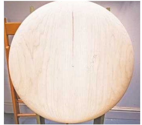
7 The first phase of shaping the 'Luna' chair back following some sanding to remove tool marks
