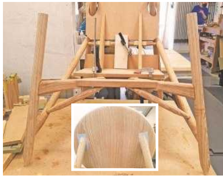
26 After flush cutting with a hand saw, the joint was refined to meet the seat back's curved face, using a sharp block plane and pieces of abrasive
