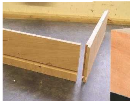
17 The drawers were constructed with simple half lap joints...
