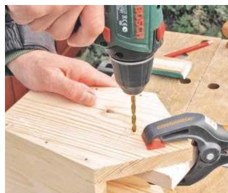
12 Form a keyhole slot for the screw in the back by drilling 10mm and 5mm holes, 10mm apart; join up with a jigsaw
