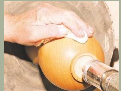
21 Once sanded, apply your choice of finish – I'm using oil but you may prefer to omit this step
