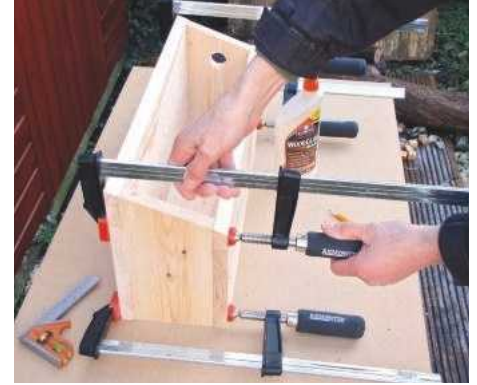
3 Glue front, rear and end sections together and clamp; add nails, pre-drilling the holes to stop splits
