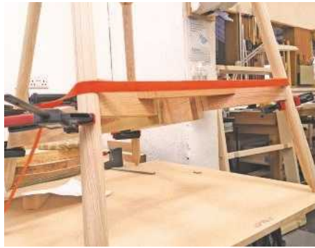
12 Prior to dry fitting, I'd made a lot of progress, from having the legs and rounds all turned to machining and jointing the underseat frame. It was now starting to look a lot more like the drawing
