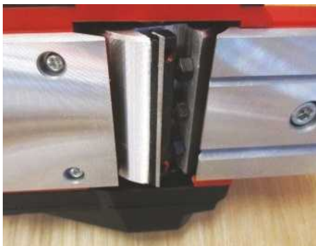
All planes use a similar two-blade drum
