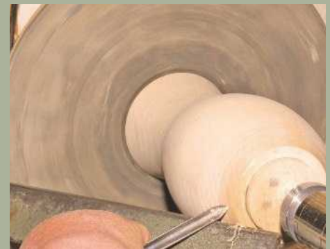
18 Next, mount a large faceplate with sponge backing on the lathe, along with the vase. You can now turn the bottom of the piece so that it blends in
