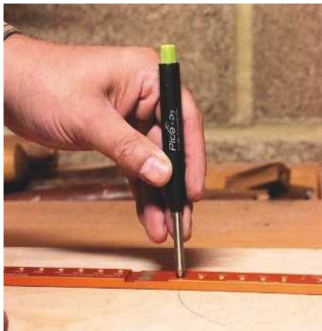
A series of 25mm holes allows bowl blanks to be marked up for cutting
