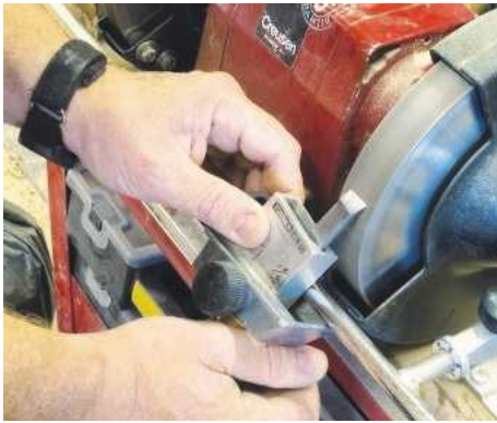
2 My preferred skew is a 13mm version with rolled edge; this stops it sticking on the toolrest. Sharpening it on a jig gives consistent results every time
