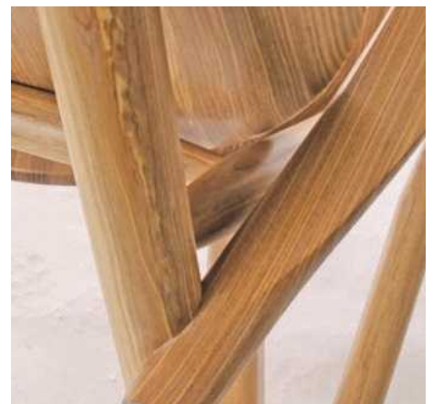
38 My favourite detail on the 'Luna' chair is this collection of joints: two tapered tenons and a coped joint, with the arm's gentle curve creating just enough space for the backrest and side rail
