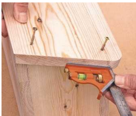
11 Cut the top to size and round front corners; drill and screw to the box, checking the overhang is equal
