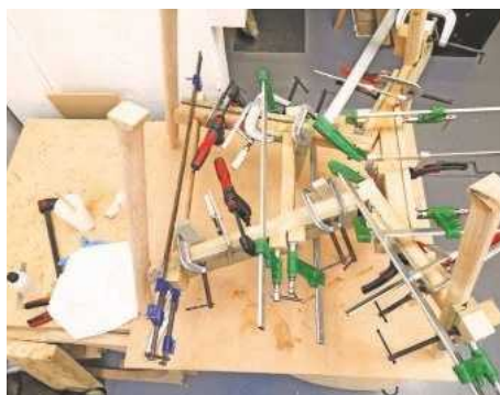
16 The structural heart of the chair, which establishes the geometry and relationship of all components, so getting this perfect was therefore important. If all goes well, it'll look just as good when out of clamp
