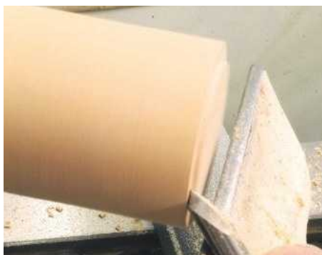
12 The spindle gouge excels at cleaning across end-grain. As you can see, the bevel is positioned according to the cutting angle I want to achieve
