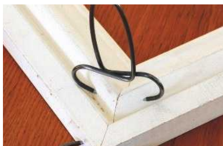
On ornate moulds, additional clamps can be added to the profiles
