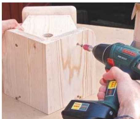
17 Drill roof holes and fix to the box with 40mm screws; the rear edge is flush with the box's reverse
