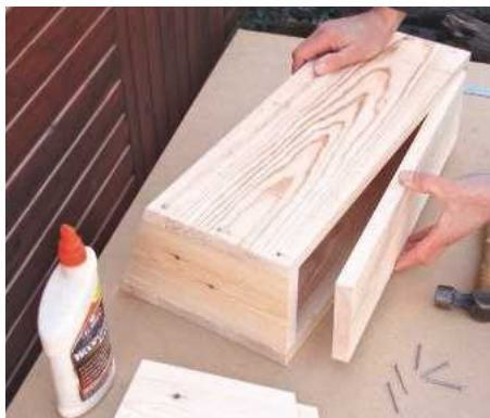
5 Cut the bottom to size for a snug fit inside the box; glue and pin, punching nails below the surface
