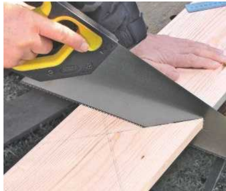
2 Cut front, rear and side pieces to size with a fine-toothed hand saw or mitre saw
