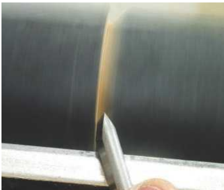
8 The tool is presented with the left-hand bevel at right angles to the work and the longer point downwards. Lift the handle to slice into the wood
