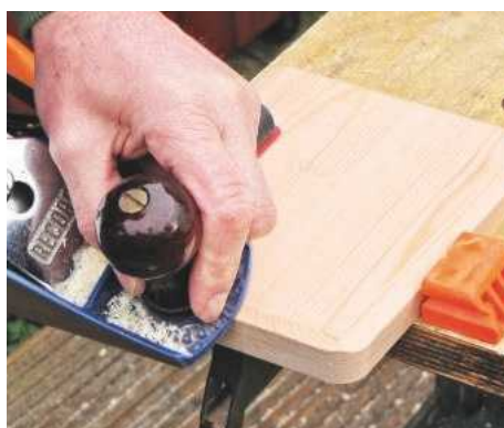
11 The base's upper edges are chamfered at 30°; mark with a gauge and plane to the lines
