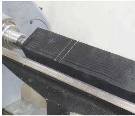
6 I've sprayed a piece of pine black to make it easier to see the cuts made. I've marked the area that'll be cut in from square to round
