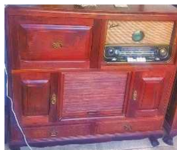
2 The second matching imbuia unit is a radiogram, and behind the left-hand drop-down door, a Garrard 301 record transcription deck slides out on rails to provide access for placing records
