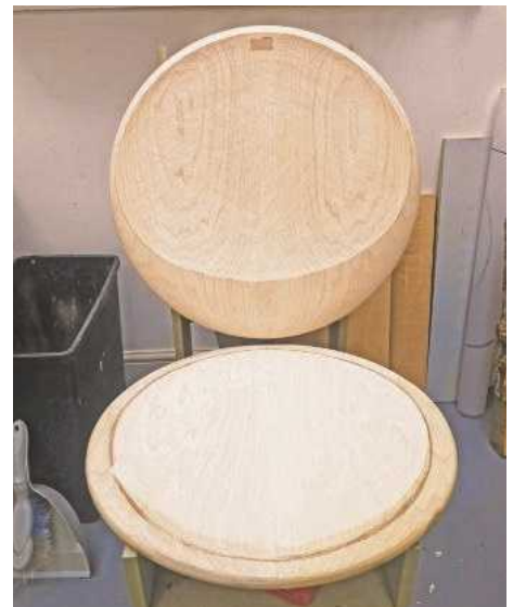
10 Test seat and back begin to take shape following slight deviations from the CAD design
