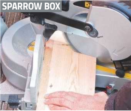
1 Cut the ends and internal dividers to length using a mitre saw; top edges are angled at 70°
