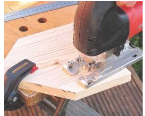
3 Front and back are tapered towards the bottom; mark and cut with a jigsaw, then clean up with a plane
