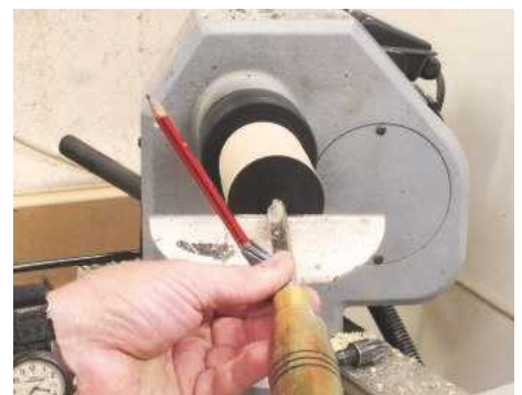
13 Hollowing egg cups, boxes, etc. is best carried out using the spindle gouge. The pencil shows the 11 o'clock position of the tool's flute
