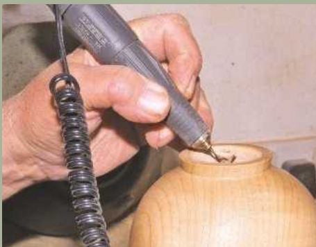
22 Remove the vase from the lathe and using the flex shaft motor as before, carve out the centre pip on the bottom
