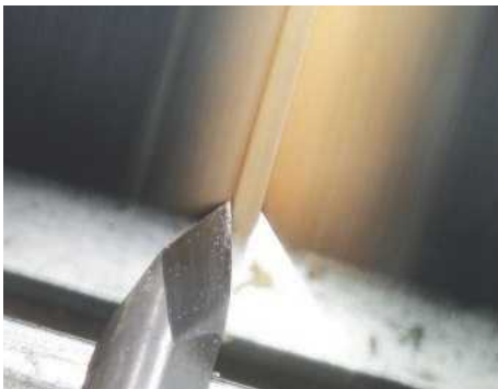
11 If used correctly, you'll only cut using the tool's point. If you start to see dust appear on the skew's bevel, you're very close to having a catch
