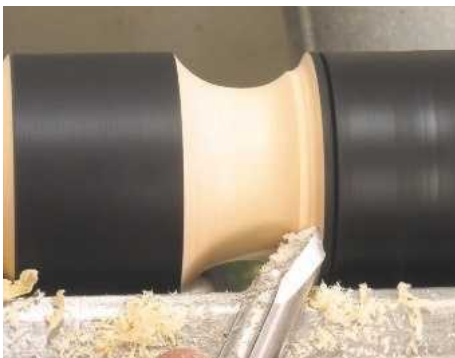
8 You must keep your right hand low throughout the cut; this will allow the bevel to rub. If you're not achieving a good finish, it's often because the tool is held too horizontal
