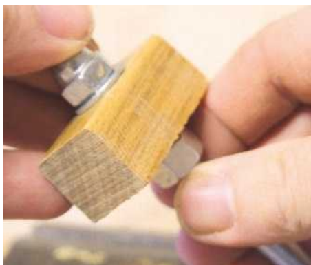
6 The shelves are held by my bolt and block assembly, the dome nut held captive by lots of CA adhesive
