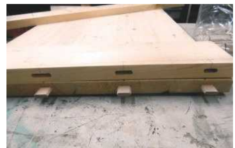
7 Leg mortises cut wider for movement
