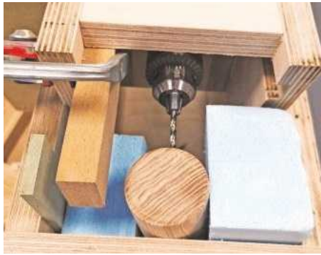
19 The jig was modelled in Fusion 360 and core components machined using the Shaper Origin
