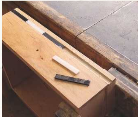
19 The glass sections were glued into routed grooves with builder's epoxy
