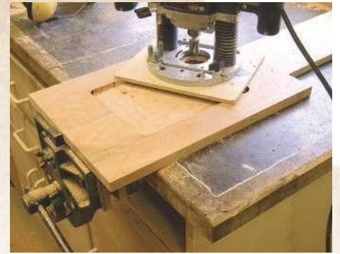
13 The marquetry panel sits in a rebate routed in the top panel; the router's large sub-base prevents it tipping
