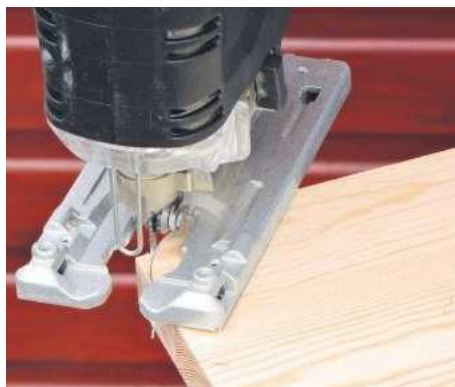
8 Draw around a coin to form curved corners on the roof sections; carefully cut with a jigsaw
