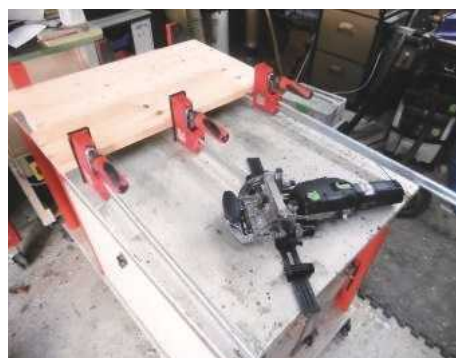
2 Building up the headboard panel
