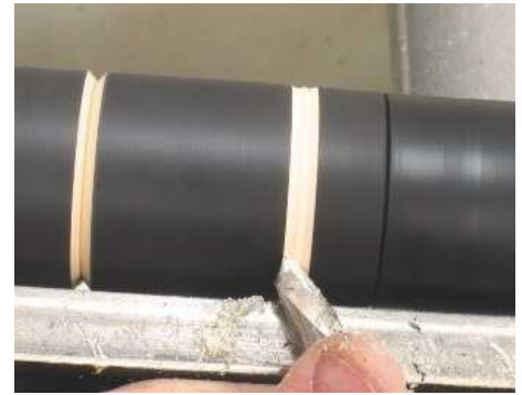
7 Now that the tool is cutting on the other side, only take small amounts of material from each side until the cove gets wider
