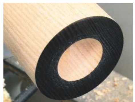
16 If you decrease the depth of cut as you near the finished shape, a pretty good finish can be achieved. The denser the wood, the better the results you can expect to achieve ✂
