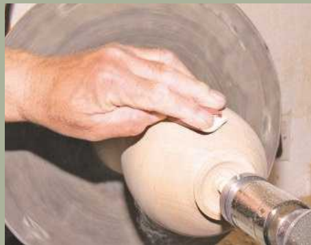
20 Finally, hand sand the vase, starting with 180 grit abrasive and working your way up to 400
