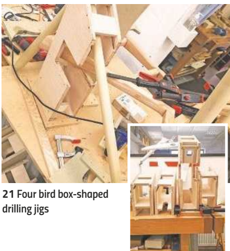
22 Dialling in the mortising process required for the rails
