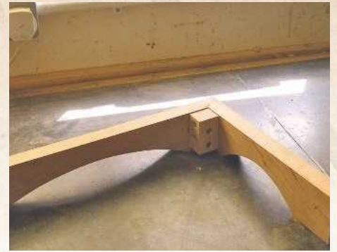
7 The plinth has mitred joints, strengthened with blocks that are glued and screwed into the corners
