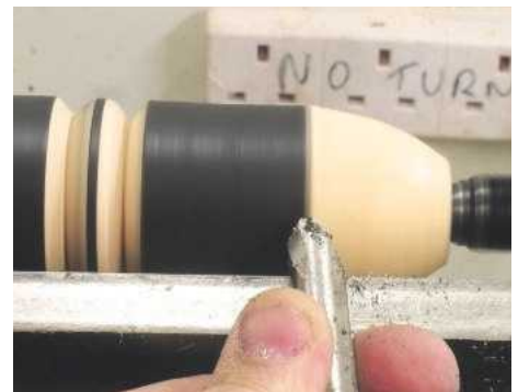
10 To round over the spindle's end, start with the bevel on the wood in a position where the tool will start cutting, with the minimum required movement
