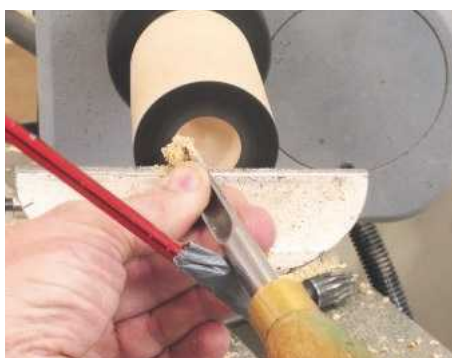
15 As the hole gets deeper, you'll need to close the flute off slightly as you come up the hollowed area's side. The pencil is now telling me it's at 10 o'clock
