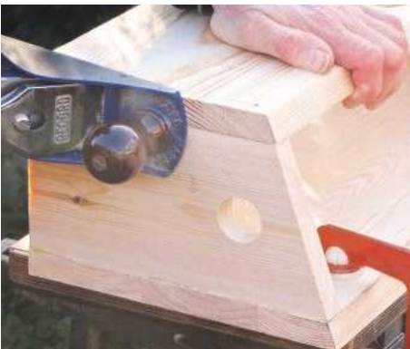
7 When the glue has dried, trim ends flush with a plane; note one entry hole is at the end of the box
