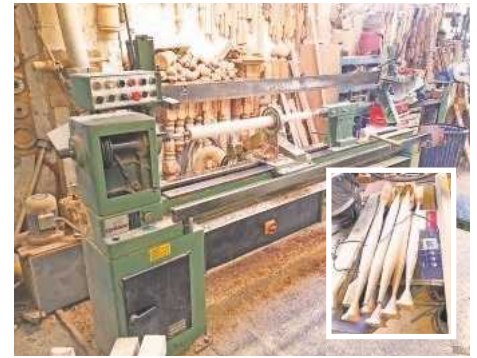
20 All turned components were completed using a copy lathe; a process I decided to outsource to a local joinery workshop
