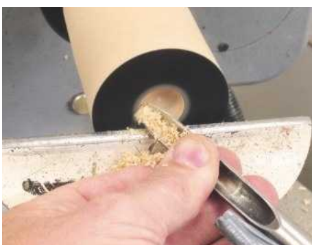
14 Once the gouge has drilled a small hole in the centre, it's pivoted out by moving the handle away from the body
