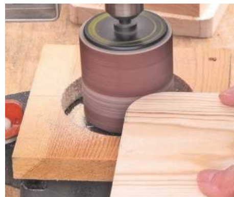
9 Clean up curves with a sanding drum in a drillstand or abrasive block. Repeat for front corners of the base
