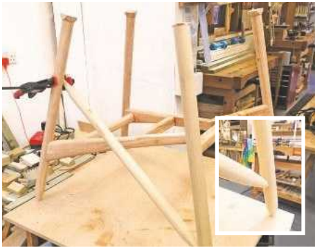
18 Using this method, the geometry and symmetry should be kept identical to the original design and the joints tight and clean
