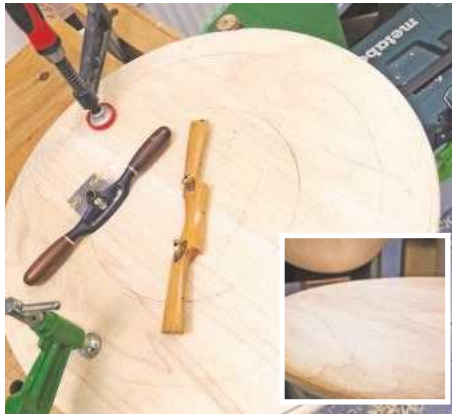
6 I started shaping the back panel and added a roundover to the edges; this gave a reference from which to work when shaping the convex face
