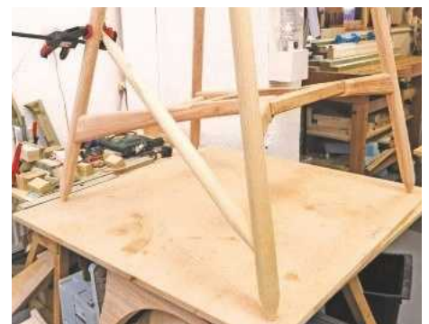
17 Test joint for the angled tapered mortising jig made for the stick jointed rails. Thankfully, it worked perfectly...
