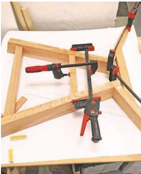
8 Dry fit of the underframe components before final shaping
