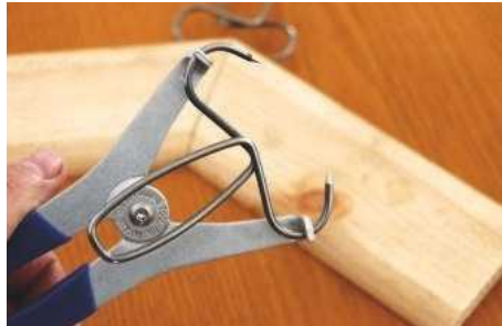
Squeezing the pliers easily opens the spring clamp
