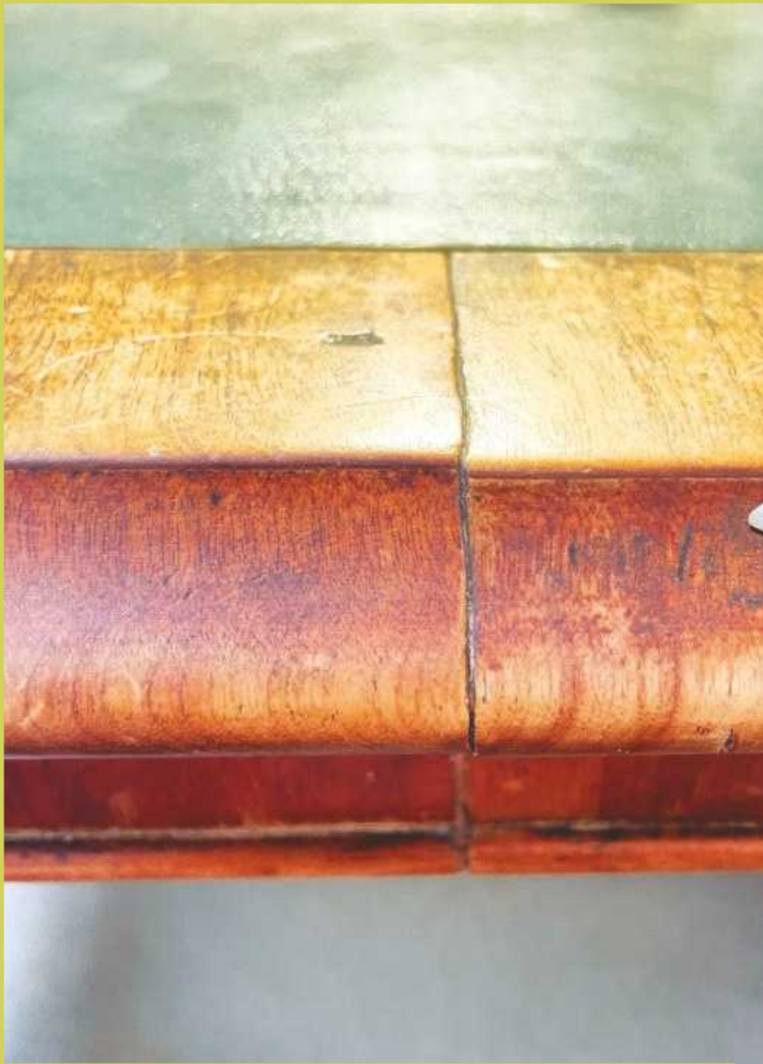
5 Yes, I'll admit it, you can see the join in the walnut cross-banding
