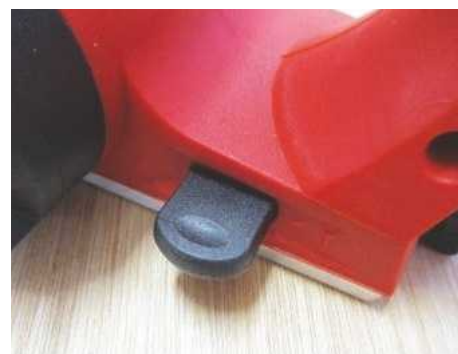
Blade removal spanners are stored in the body
