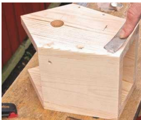
14 Punch all nail holes below the surface and apply exterior filler; drill a couple of drainage holes in the base
