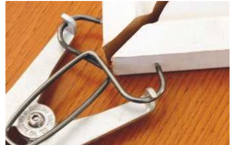
Applying clamp to mitre brings all together tightly...
