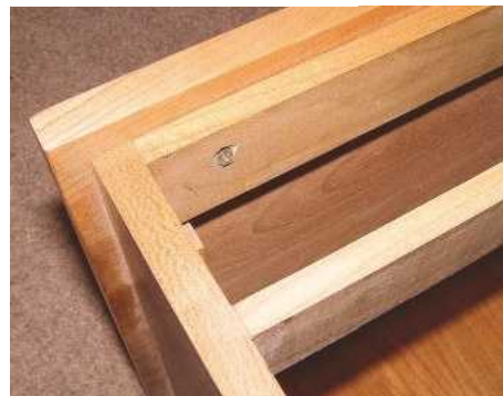
15 The top panel was attached with screws, countersunk so as to clear the drawer back panel
