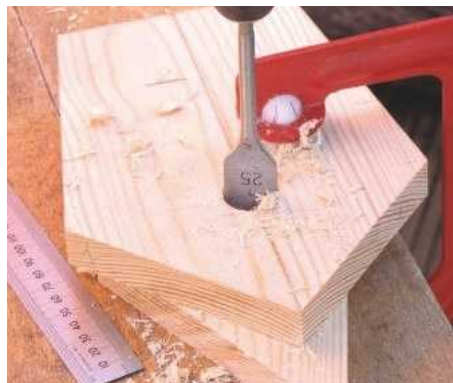
5 The blue tit box entrance hole should be 25mm diameter; mark the centre and drill with a flatbit
