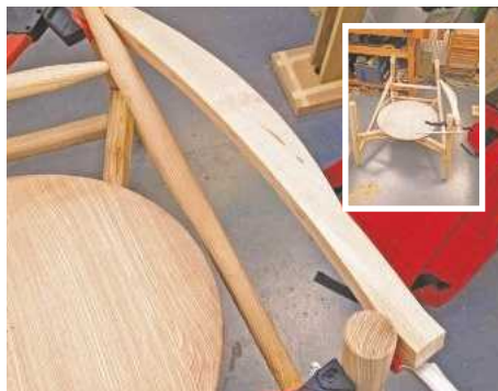
29 This detail was added prior to shaping, which ensured the workpiece could be easily held in the correct position
