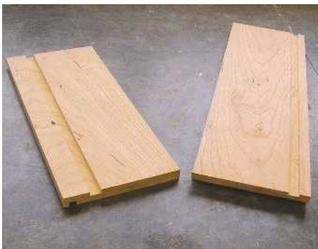
16 The drawer side and front panels were routed for the drawer runners, MDF bottom panels, and glass inlay
