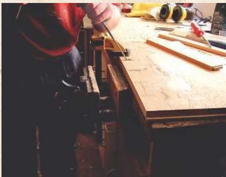
1 Mortising the cabinet sides...
