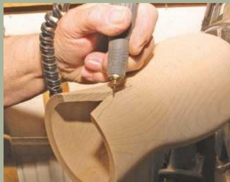
17 Using a flex shaft tool fitted with a dentil drill-type handpiece, refine the area where the zip will be placed
