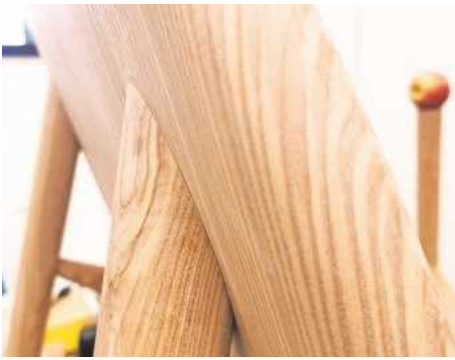
25 Another homemade jig allowed me to flush cut the angle of the back legs, where they met the seat back
