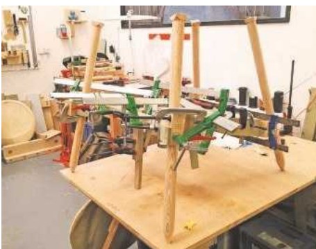
15 It'd been a slow process, but I finally completed the underframe glue-up following further shaping and lots of tweaks and adjustments to the joint
