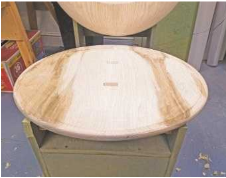
11 After a few sketches, I flipped the seat blank to try out the shape shown here, which resulted in exposing the Dominos. I was much happier with this shape, even though it's a little difficult to see
