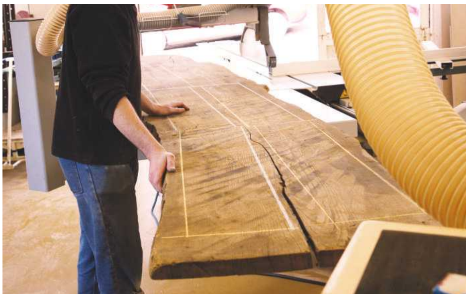
3 Rough marking out with chalk guides a wood machine operator when cutting large, wane-edged planks into slightly oversized component parts
