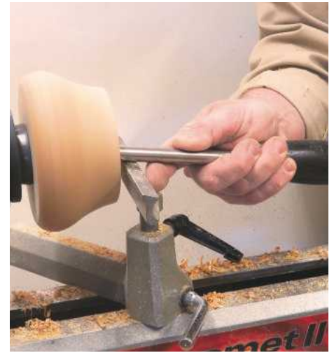
12 An issue with smaller lathes is being able to get the handle of the gouge low enough during the hollowing process – you may have to adapt your technique. I have a set of tools specifically sharpened, which allow me to get around tight curves in shapes
