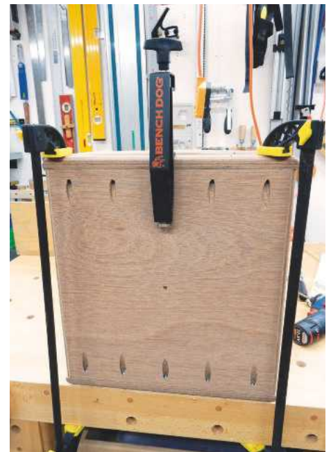
14 Once completed, I glued and pocket-hole screwed the sides to the base
