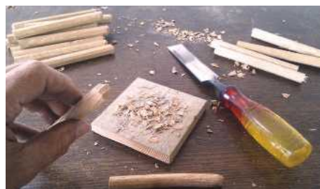
Oak treenails, which are used to pin a wooden structure together. The one in front has been used and pulled out, showing the way forces have permanently deformed the wood
