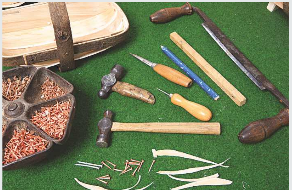
Carl uses simple hand tools to make his traditional garden trugs, including a 200-year old drawknife, seen right
