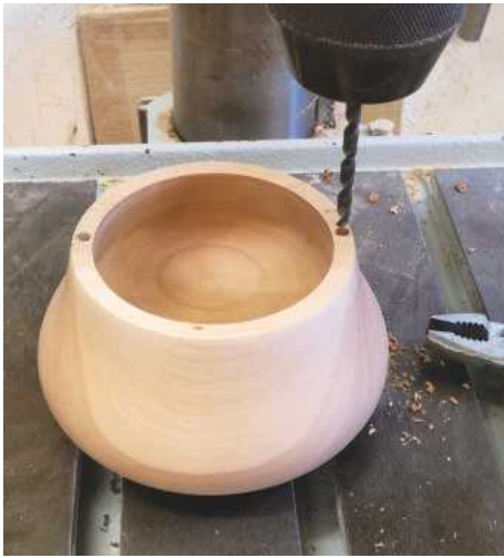
28 Make a cardboard template to mark out the two positions of the magnets and carefully drill down to a depth that's the exact length of the magnets; they'll need to sit perfectly flush with the top surface of the base and lid
