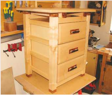
10 Little sanding was required before finishing the piece with Osmo Polyx oil and wax
