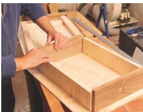
8 Loosely positioning components against one another gives a preview as to how they'll go together and helps to understand how the joints will fit
