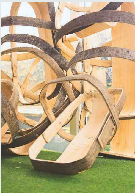
The frame is then ready to accept the willow strips, which are laid on top of one another to form the trug's base
