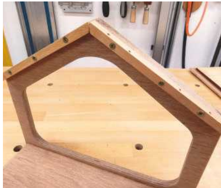
18 To fix the roof panels to the sides, I glued and screwed some beech strips onto the inside edges
