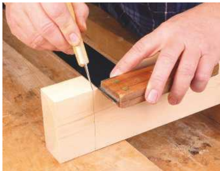
15 To run a series of lines around a piece of wood, place the marking knife in the end of one line and slide the square up against it before marking the next one
