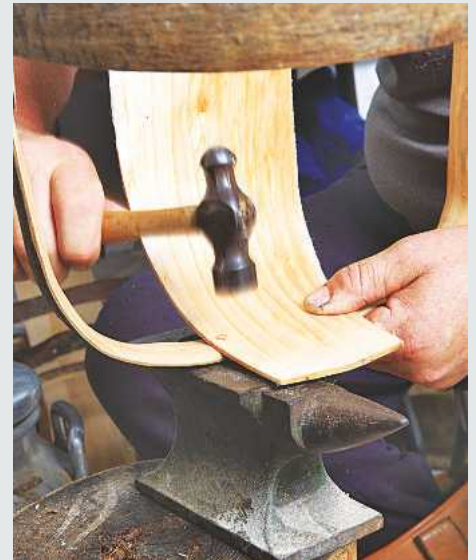
After being soaked, the wands are left to set around a jig for anything up to three weeks, before they're fixed together with copper nails
