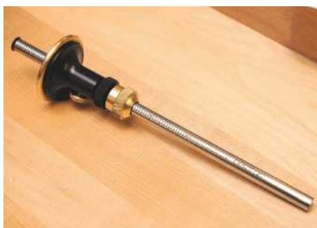
18 Modern all-metal marking gauges have a sharp-edged washer on the end, which makes it easier to produce a clean line than with a pin
