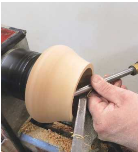
16 Due to the tool's short bevel, in order to start the cut, the handle needs to be in this position. With practice, you can undercut the bowl with a gouge, or if you're struggling, you could take light cuts with a scraper
