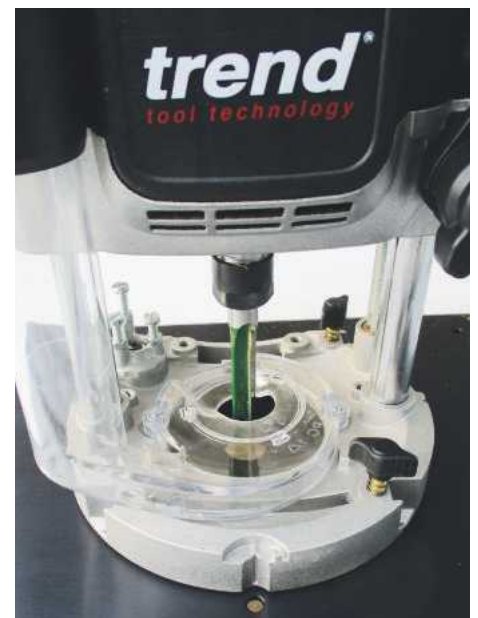
The cyclone dust adaptor fitted in place
