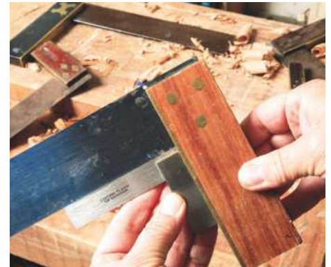
13 Try-squares come in many varieties. The standard type with wooden stock and steel blade should be accurate provided it doesn't get dropped. It's easy to check one square against another
