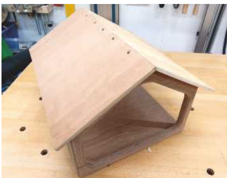
22 Once complete, the roof panel was then ready to receive its rubber covering
