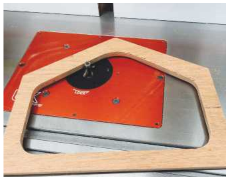
13 I rounded over the outer left, right, bottom and inside edges on each of the side pieces
