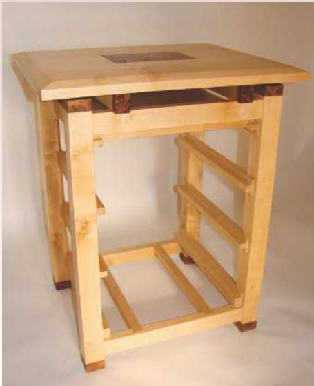
3 The top floats on the frame, which sits on two supports. Also note the cross-rails at the bottom
