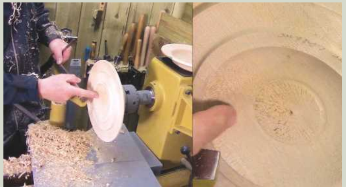
18 When used in pull-cutting mode, however, the Simon Hope carbide tool created the best finish in comparison to others used
