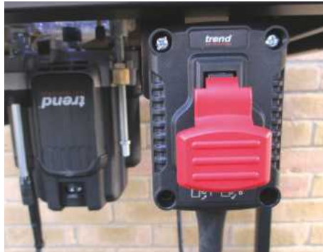
... inside the T14's handle, meaning you don't have to reach underneath the table to operate the router
