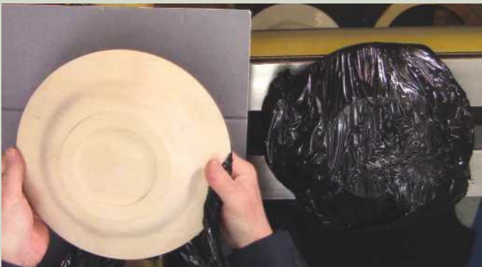
8 The project was completed over two days. To minimise movement, at the end of the first day, I wrapped both plates in pallet wrap – to keep the moisture both in and out. No matter how dry your workshop is, airborne moisture will always be present. Not only can this be lost, however, but also absorbed due to humidity
