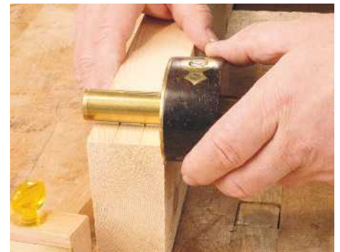
16 Old-fashioned marking gauges with pins require careful handling in order to produce clean lines. The double-pinned variety, known as a mortise gauge, is used for marking positions and widths of sockets
