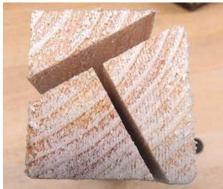
19 Obtaining the necessary 120° top angle for the ridge beam required two passes on the table saw
