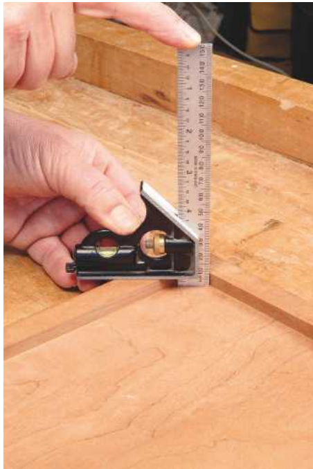
12 A combination square has many uses; here it's working as a depth gauge
