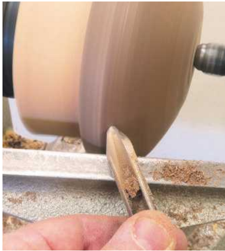
32 To refine the curve on the lid, I swapped to the 13mm signature gouge. You can use a spindle gouge on side-grain as long as the toolrest can be placed close to the work; this minimises the amount of vibration that could occur
