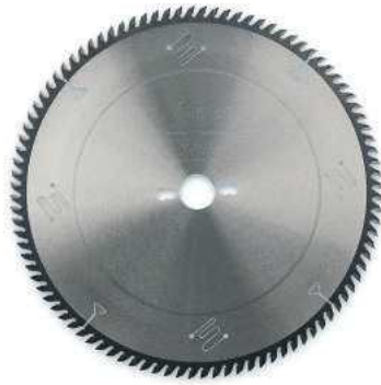
Axcaliber premium TCT saw blade – 315 x 3.2 x 30mm 96T
