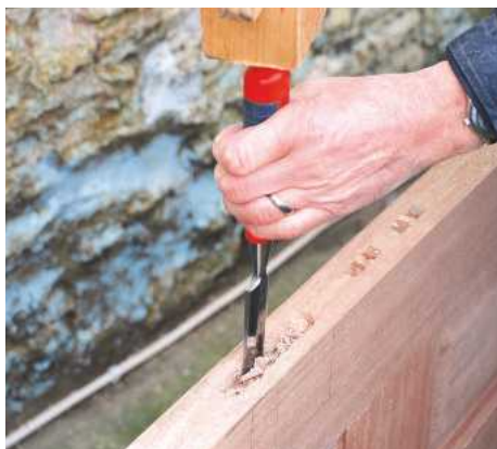
15 Remove waste from the mortise, with the blade just inside the gauged lines. Keep the chisel square and vertical
