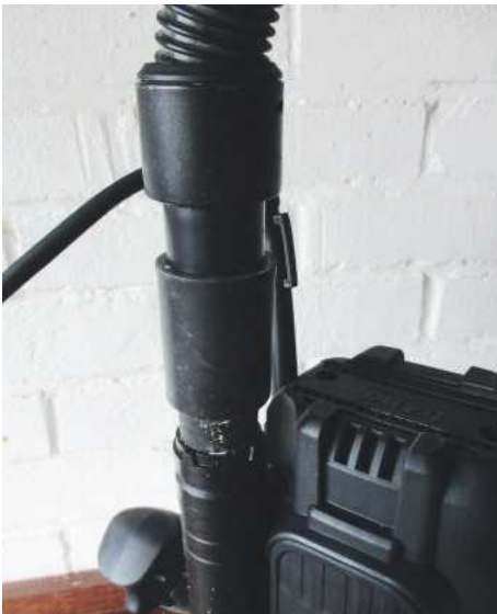
Top-mount cyclone extraction features an enhanced dust adaptor, which prevents hoses from 'snagging'
