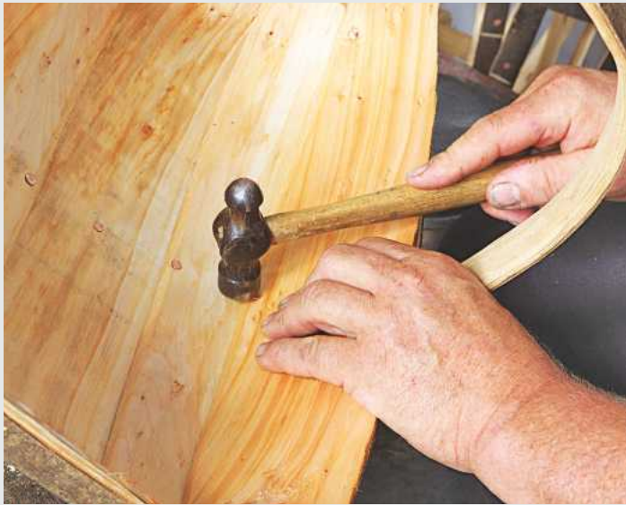
Carl will finally fasten the willow in place, again using copper nails. It's becoming increasingly difficult to find this variety and, although they can be imported, he finds they're of poor quality
