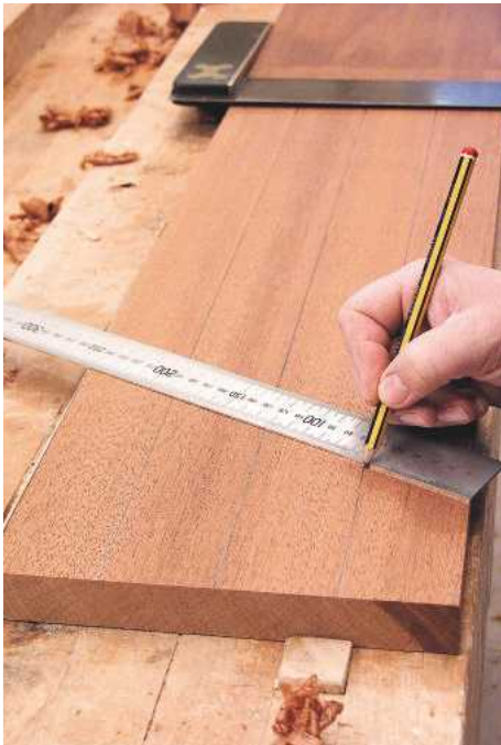
11 Using a steel rule to divide a board into equal widths. By slanting the rule, whole numbers can be used on any width of board, which makes the division much easier
