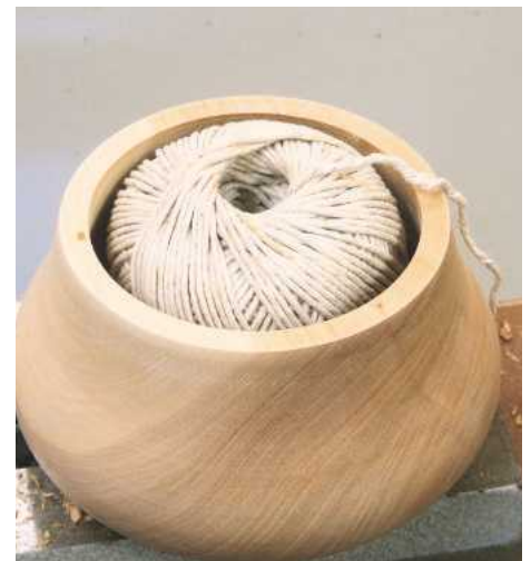
18 It fits in there an absolute treat! Because the ball of string protrudes from the top, I needed to hollow out the underside of the lid to allow for this. Don't remove the spigot until you've turned the lid, in case you need to make any adjustments
