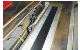
Duct tape applied to underside of throat plate, along its length
