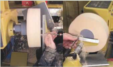
3 Here I'm truing up the sycamore blank using 1) a Record power M2 bowl gouge with swept-back grind and 2) a Crown M42 parting tool
