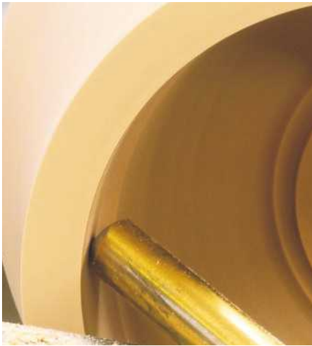
13 This close-up of the bowl interior shows the gouge's required position in order for it to achieve the best cut. The flute of the tool is pointing away from me in the 2 o'clock position and the bevel is in contact with the wood
