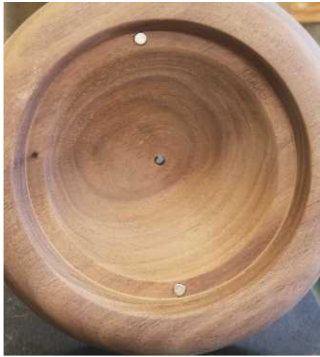
29 The template will allow you to transfer the correct positions of the magnets to the inside of the lid. Repeat the drilling process, then glue the magnets in place using a small amount of good quality epoxy resin
