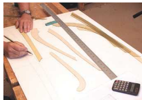
22 Transferring a component design to a full-scale drawing, known as a rod, is particularly helpful when curves and angles are involved
