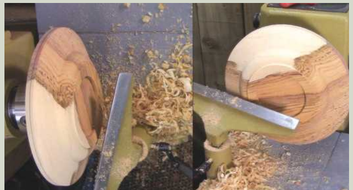
7 The tool produced a good finish on both surfaces, but the wet ash was much easier to work; this was expected due to the material being drier and the fact it was kiln-dried does make a difference. Using this tool, the edge also remained sharper for longer, especially when used on wet material such as this
