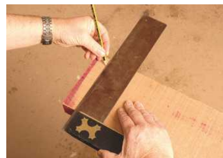
4 A pencil line drawn against a try-square ready to cross-cut a straight end on the board
