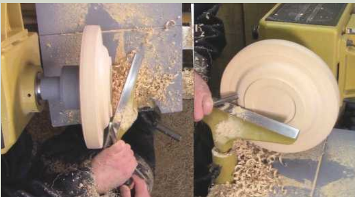
6 Using a Crown M42 parting tool to remove the sycamore ring. I then swapped to the Crown M42 swept-back gouge to produce an ogee shape, used in draw-cutting mode
