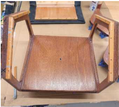
26 The remaining table components and supports were given three coats of outdoor varnish, with a light sanding between each
