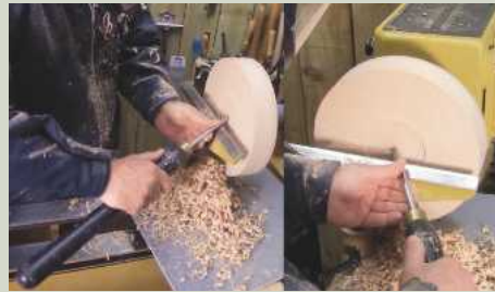
4 Cutting back the 100mm recess using a 10mm traditional-ground Crown Pro PM bowl gouge. I found that cutting from the middle outwards was the best method for laying down fibres, and therefore producing the best cut
