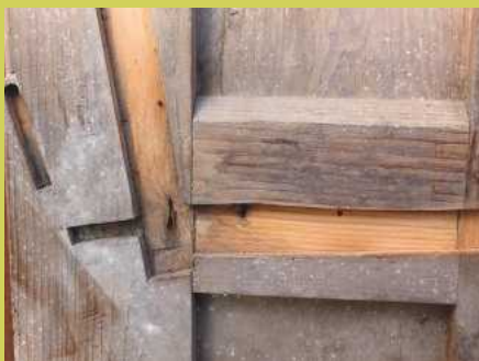
There appeared to be little glue used in the pew's construction
