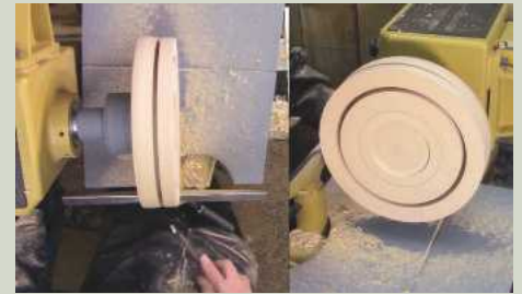
5 Removing a ring of wood, which will be saved for a future project – most likely a circular picture frame. It'll be interesting to note the difference in movement between the dry and wet materials
