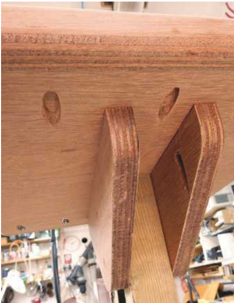
17 I screwed the supports to the table using pocket-hole screws once more, fixing these to the post with two screws on either side
