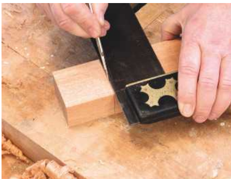
14 Press the square's stock firmly against the edge of the wood while marking against the blade
