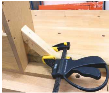
11 To ensure the supports were all correctly aligned on the post, I fixed each in place using a right-angle jig to keep them level with the bottom
