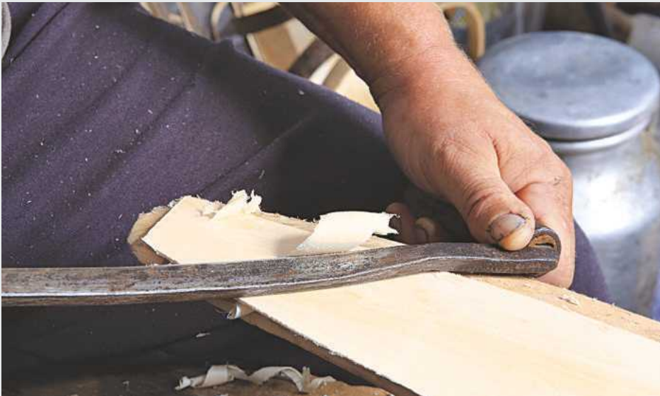
Carl starts a trug build by cleaving the handle and frame from chestnut to produce wands between 32mm and 25mm thick
