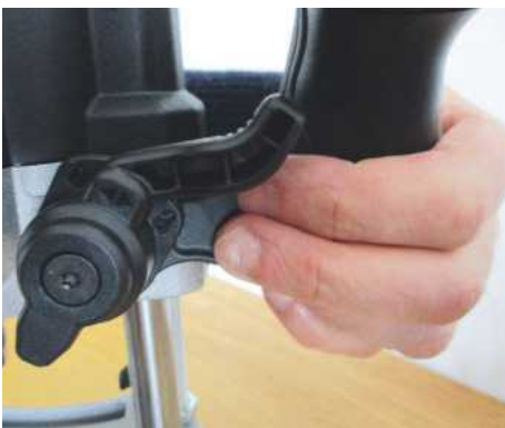
The new auto-lock plunge lever
