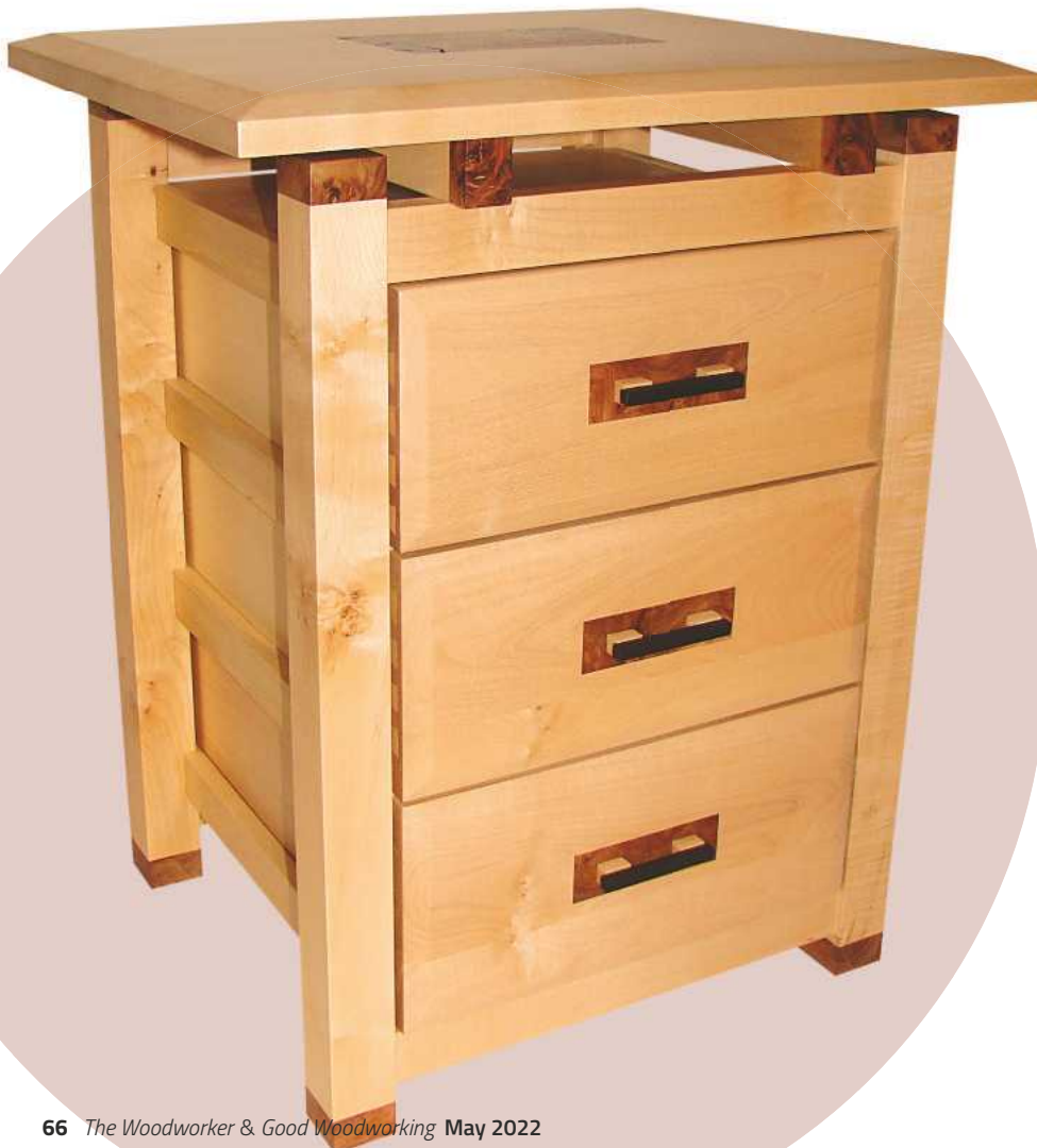
9 In place, you can see the open-structure means that the drawers form the sides
