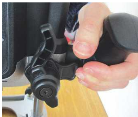
The released plunge lever is out of reach...
