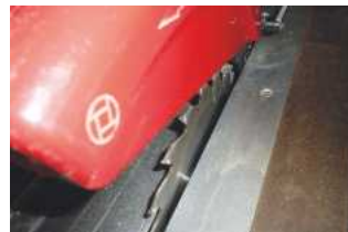
Saw blade with gap between it and the edge of the throat plate where the offcuts easily drop down
