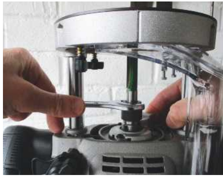
The low profile dust adaptor provides excellent clearance for cutter changing
