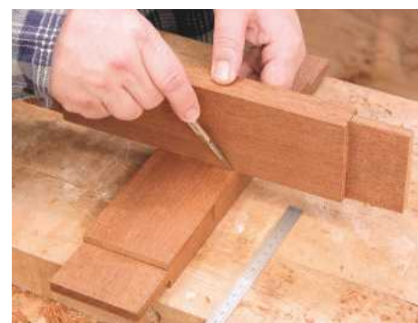
10 Marking directly against both sides of a piece of wood, transfer its thickness accurately onto another piece before cutting a slot
