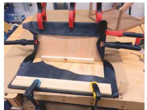
24 Once stretched over the ends, the rubber was clamped in place and left overnight
