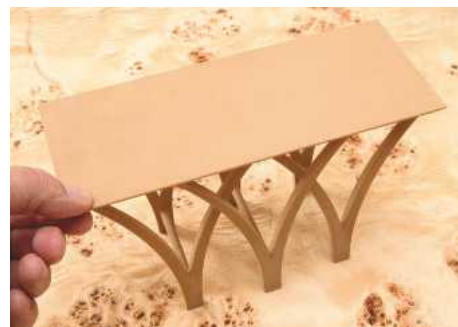
21 If the furniture is going to include unusual shapes, a small model such as this MDF maquette helps everyone visualise the plan
