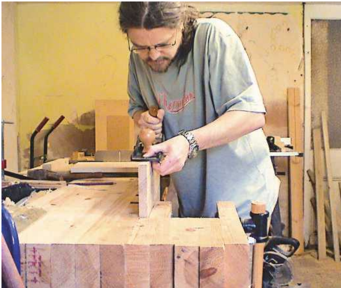
When edging a board, Mike Riley holds the front of the plane body with his left hand, curling his fingers under the sole of the plane to act as a fence
