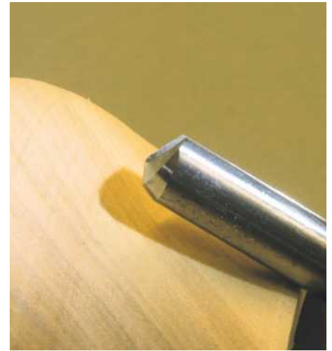
15 I found it difficult to turn the inside of this shape using my normal gouge, so I decided to bring the 60° bowl gouge into play. This tool's extremely upright bevel allows it to be easily controlled in tight spaces
