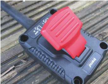
I initially thought the router table safety switch was an additional feature, but it's connected to a port...
