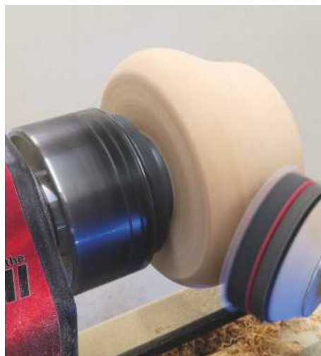
17 The Simon Hope pad is normally a little too big to fit into the curve, but the addition of this soft interface pad allows it to conform to the shape without leaving scratches on the surface
