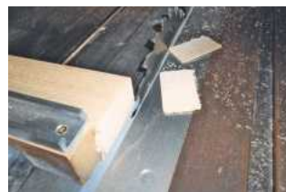
Saw blade with gap between it and the edge of the throat plate where the offcuts easily drop down
