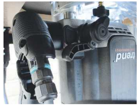
The T14 features a unique router table safety switch
