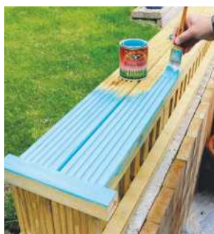
A suitable base coat is first applied – I used a milk paint from General Finishes
