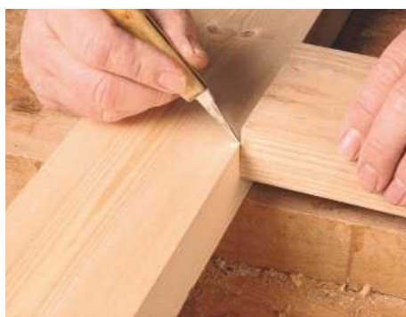
9 For the greatest accuracy, a knife line marked directly against a component to show its position eliminates errors associated with measurements
