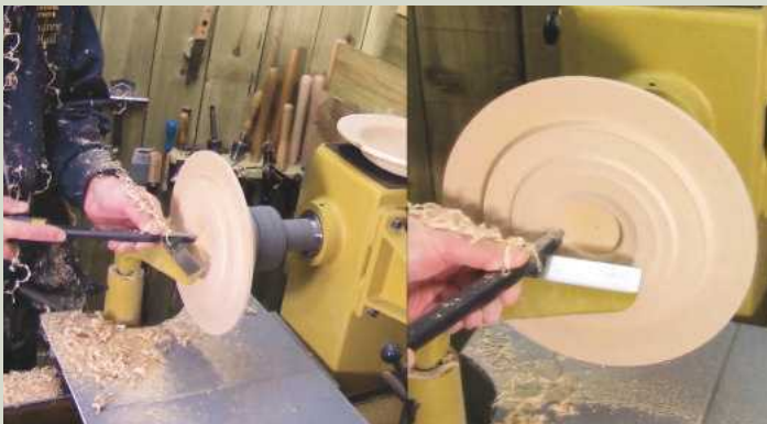
17 An interesting point to note was that all of the carbide tools raised the grain of the dry sycamore during the turning process
