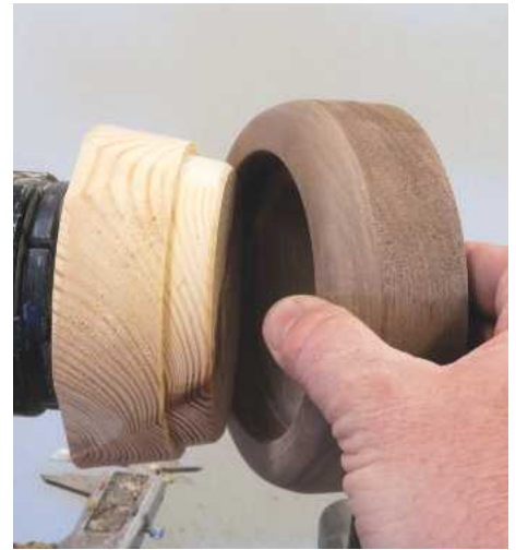
30 The glue chuck now becomes a jam chuck for the lid. Turn a taper on the piece so you can gauge the correct diameter, then remove small amounts until you achieve a snug fit into the chuck
