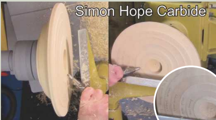
12 I separated the face of the plate into sections, with each one labelled according to the tool used, so that a comparison could be easily made. Both cut in a similar fashion, producing shavings; however, the Jimmy Clewes tool is ground at a set angle whereas the Simon Hope tool is best used at a 45° angle in raking mode
