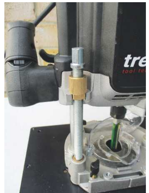
The T14's plunge depth limiter prevents over-cutting
