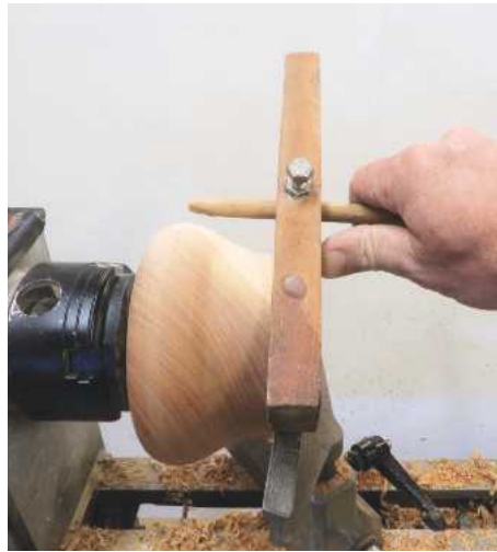
14 You need to aim for an even wall thickness, so achieving the correct depth is therefore important. I use my shop-built depth gauge to measure the base thickness, which ensures I can maintain a consistent 8mm
