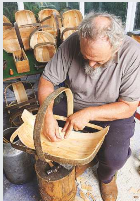
The first strip to go in serves as a sort of keel, over which layers of green willow are built
