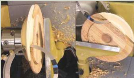
14 I used a pair of figure-of-eight callipers to gauge the rim's wall thickness. The most interesting turning, however, occurred when using various tools to remove the plate's centre
