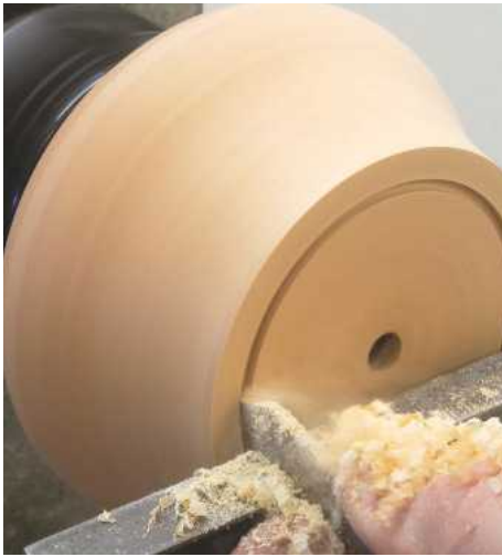
10 The wall thickness depends on two factors: the ball of string needs to fit inside and the wall has to be able to take the size of magnets you choose to use. Make a cut with a 3mm parting tool so you can fix a size to work to
