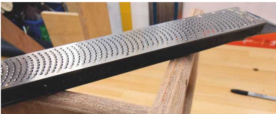
15 As the bottom corners of the sides were still square, I rounded these over using my 40-year-old Surform
