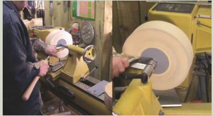
2 Dry sycamore was used for the first plate. When producing videos such as the one shown here, I've now started to spray dry wood with a grey primer to aid visibility, as it allows cuts and tool angles to show up more effectively
