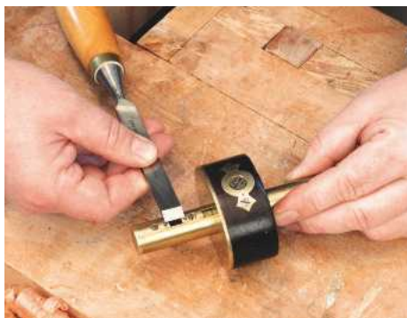
17 Setting a mortise gauge to a single chisel width makes life much easier when it comes to chopping the socket
