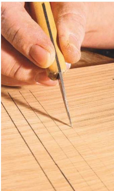
7 A marking knife produces a much finer and more permanent line than a pencil
