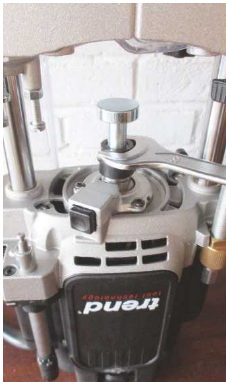
The integrated router rest aids setup
