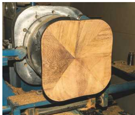
14 I reversed the piece and mounted it on the lathe, ready to cut the top face
