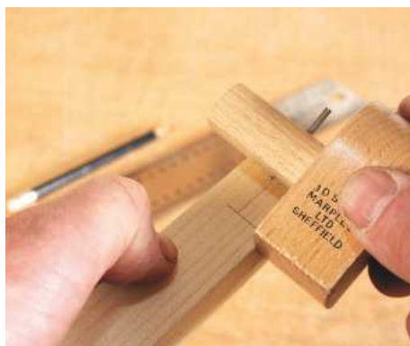
2 Extend the marked line onto the edge of each piece and use a marking gauge to denote the centreline on all edges
