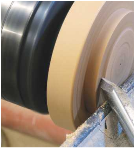
28 The bottom of the lid needs to be cleaned up; the spindle gouge with bevel rubbing will leave a great finish. Avoid starting the cut with the tool tip in the wood as it's likely to skate across the surface
