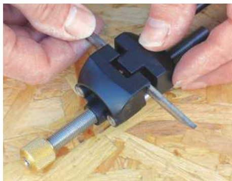
I did detect slight play when clamping a 3mm chisel, even after using the Hex key
