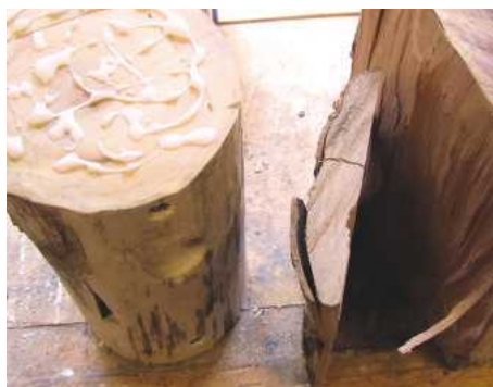
12 One-step roofing. A single split slice – trimmed to size, glued and screwed – should be enough to keep the rain out
