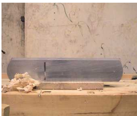
4 Check for twist with your winding sticks. If all's well, the top edges of each stick will be parallel
