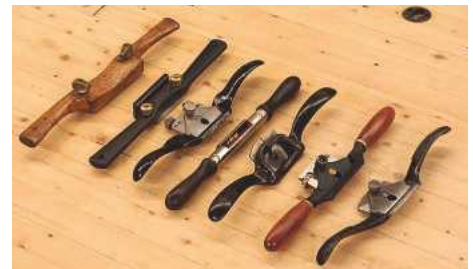
Spokeshaves come in a multitude of versions: wooden body, metal body, round or flat bottom, those with adjustment screws and those without
