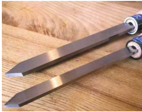
Each of the sets includes a parting tool, albeit in two different sizes
