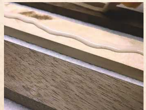
1 To make the side panels, take two strips of walnut and one maple. Glue the flat sides together...
