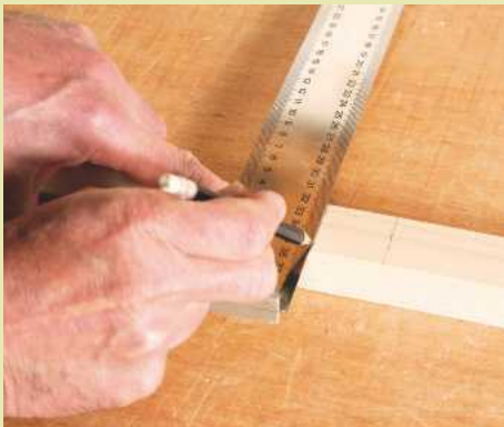
3 Remove the divider carefully so as not to disturb the try square and mark the second line against it to define the joint width
