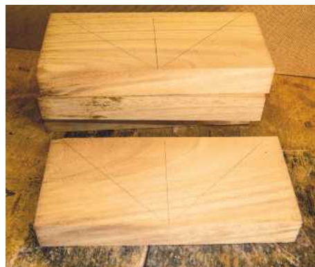
2 Using the hardboard template, I marked the pieces out ready for cutting on the bandsaw
