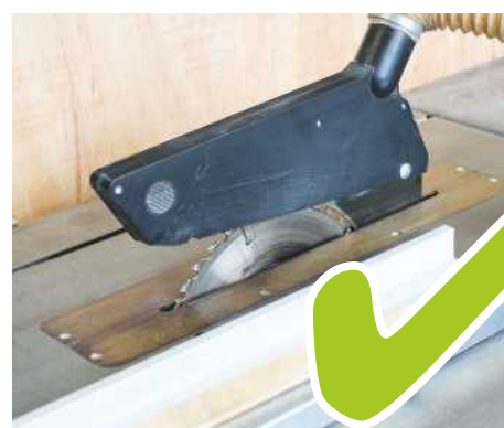
Standard workshop setup, with guard and riving knife in place; note push-stick nearby
