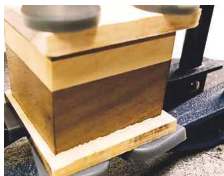
11 The top, sides and bottom are clamped together and the glue allowed to dry
