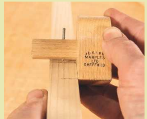
5 Take a marking gauge, set it to exactly half the thickness of the rail, and gauge the joint depth line between the two pencil marks
