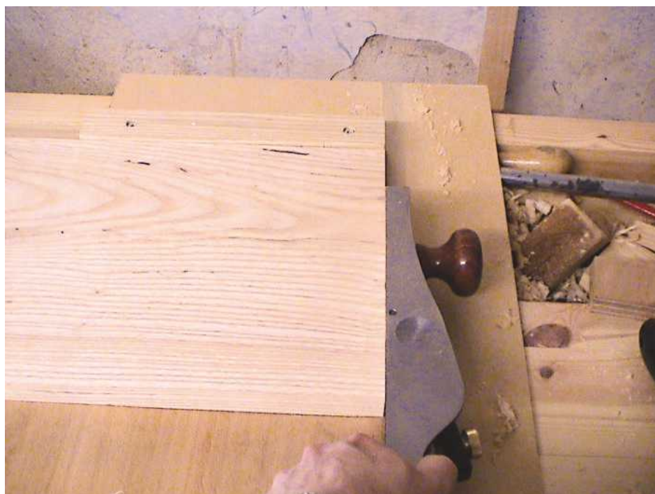
8 A shute, or shooting board, and a fiendishly sharp plane iron...
