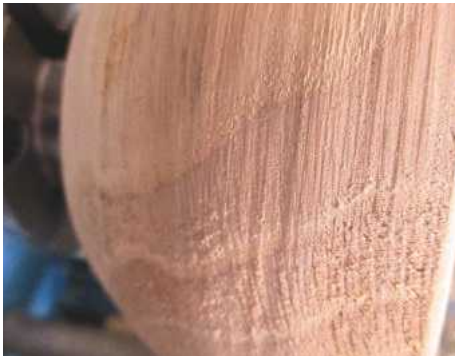
I spent a few seconds turning a bowl before a touch-up grind of the cutting edge was required
