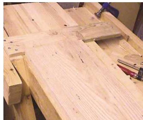
3 With a planing stop, you can rely on the downward force of the plane to hold the board in place
