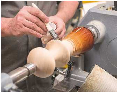
Applying spirit stain to a turned piece while mounted on the lathe
