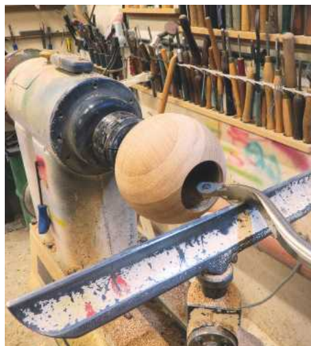
17 The final cuts around the piece are made using the Stewart scraper system from Robert Sorby, which has a small, sharp teardrop-shaped scraper on the end. Be careful here as if the curved part is on the toolrest, it'll twist in your hands
