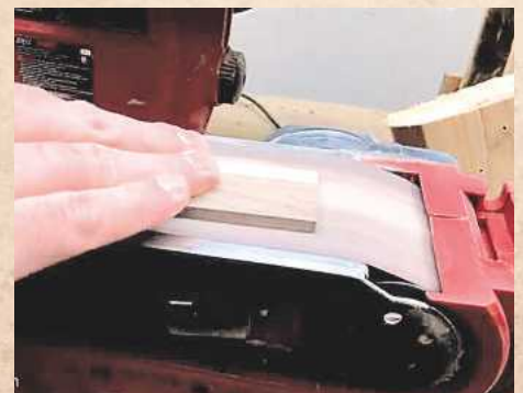
4 Saw marks are smoothed out using a belt sander
