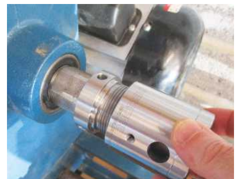
... followed by the chuck, and a grub screw locks everything together
