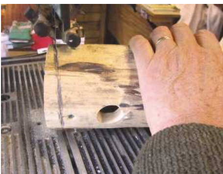
11 Bandsawing a circular piece demands a firm grip, otherwise there's a risk that the blade will spin the wood and squash your fingers
