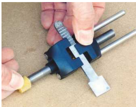
I found it worked effectively with shoulder plane blades, though not surprisingly, spokeshave blades are also too short
