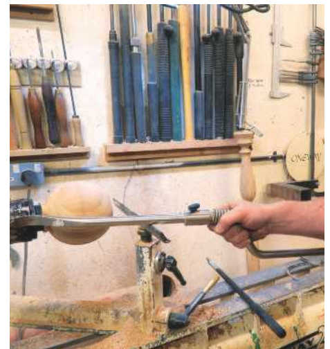
18 The tool has an armbrace attachment, which makes it easy to control. It also has a side handle, but I personally don't recommend this, preferring to look for areas inside the vessel where the tool doesn't twist
