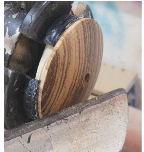
30 I thought a great deal about possible lid shapes and ended up turning a simple dome on the top. Next, drill a shallow 10mm hole to accept the knob, which can then be glued on
