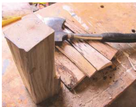
4 Side two, on the right of the photo, split a little short because the wood was slightly rotten near one end, but not enough to weaken the structure
