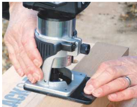
Most of the trim base is shrouded in rubber, creating an excellent hand grip, while the extended sole plate beneath makes it easy to keep the tool steady
