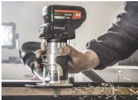
Fixed base keeps the cutter at a set position, which is ideal for repeat cuts including roundovers, chamfers, quirked moulds and trimming laminates
