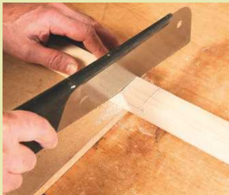
7 Hold the rail on a bench hook and use a tenon or pull saw to cut down to the gauged line, at each side of the joint
