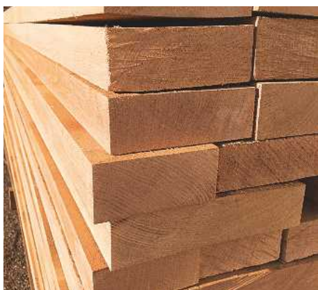
A stack of square-edged sawn lumber
