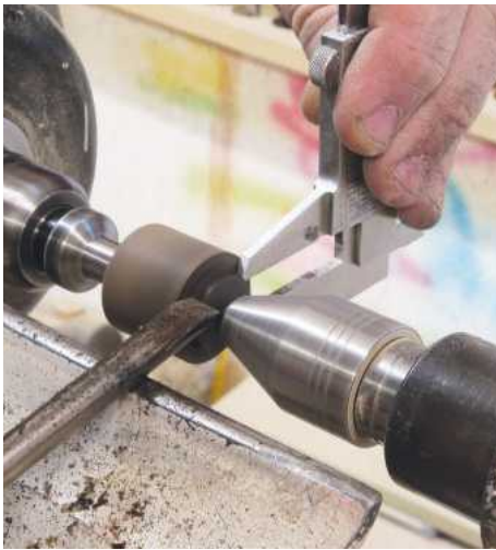
31 Ebony contrasts really well with zebrano, so mount a piece between centres and turn a 10mm spigot to match the hole drilled in the lid
