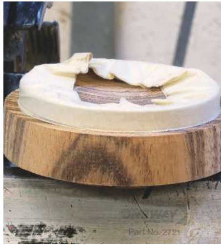
29 Turn the top of the lid by gripping on the spigot you've just made. Using four layers of masking tape will ensure that the chuck jaws don't mark the timber
