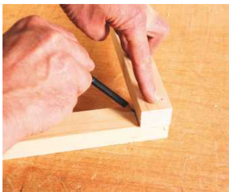
1 Place the two components at 90° to each other using a try square. Either set flush or allow the ends to overlap a little for trimming later. Mark the overlap
