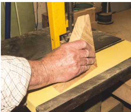
6 To check the sawn faces were truly flat, I marked the face with a soft pencil and lightly sanded them on a flat surface
