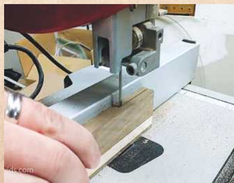
3 Side panels are squared up on the table saw, and resawed to final thickness using a bandsaw
