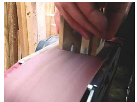
21 ... and finished with a belt sander, ensuring the box exterior is nice and smooth and any sharp edges removed
