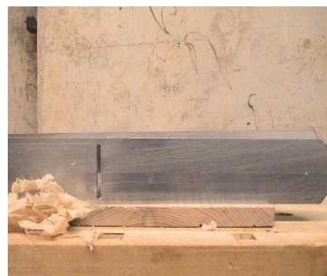
5 Unfortunately, however, it's more likely that the sticks will indicate some amount of twist
