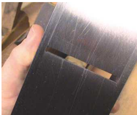
2 Grit or silica embedded in the timber will damage the sole of a plane
