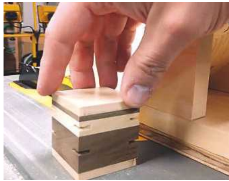
14 When cutting the splines, ensure to remove minimal material – the cuts should only be visible on the outside of the box
