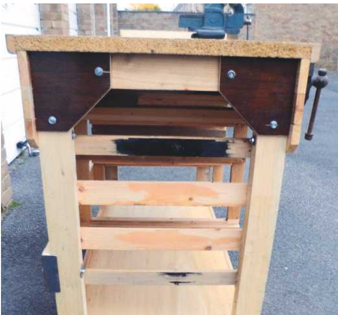
3 The woodworking vice is carried on box-ply, which is itself glued and bolted to the workbench top. Note the coach screws' load is spread over large diameter washers, all of which are recessed below the surface
