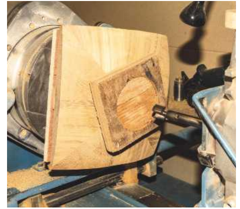
18 To simplify centring, I bored a shallow recess, the diameter matching the faceplate I'd use
