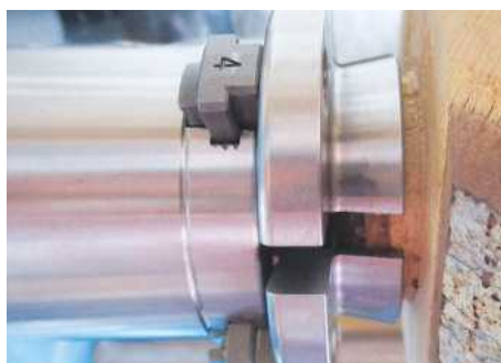
Due to the jaws' compact size, access to the back of the chuck is made possible
