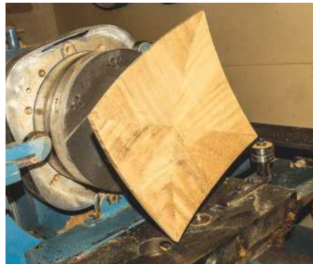
20 The top face part-sanded and the platter ready to be removed for final sanding and finishing
