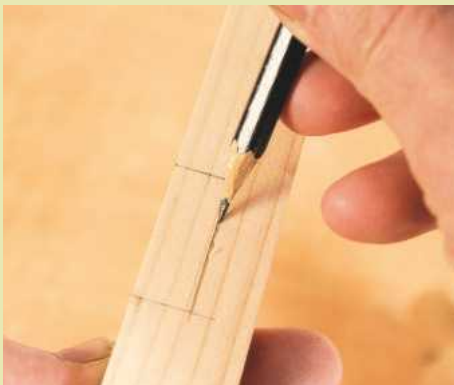
6 Run a sharp pencil along the gauged line to make it more clearly visible
