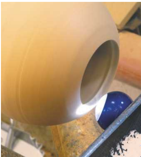
16 A couple of years ago, one of my students gave me a small LED light, which can be easily attached to anything. It's fixed on the toolrest and shines inside the piece I'm working on, but doesn't get in the way of the tool
