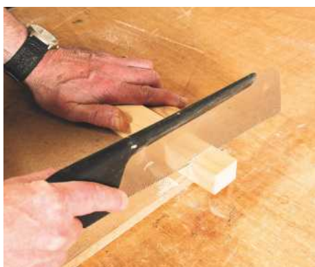
4 Hold each component in turn on a bench hook and use a tenon saw to cut the shoulder
