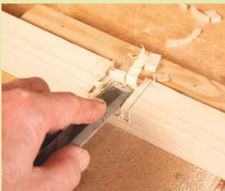
9 Pare away waste wood with a chisel, then mark out and cut a notch on the dividing component, exactly the same as before
