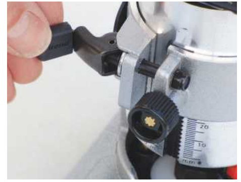
You open out a sturdy, rubber-tipped steel lever, slide the motor in and close it up again
