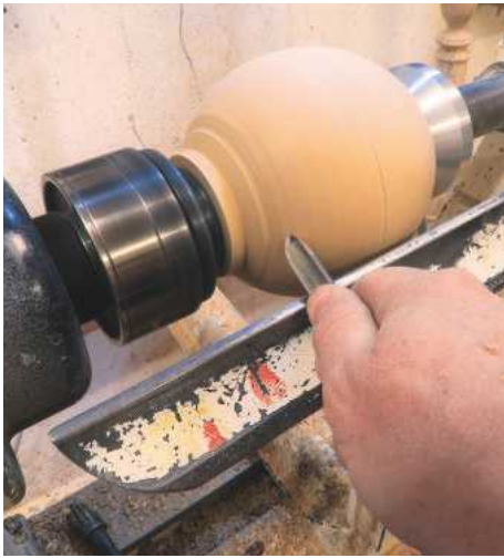
10 The tool is worked this way when coming around the left-hand side of the sphere. The bevel needs to be in contact with the wood as you traverse around
