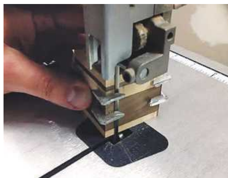
20 Once dry, any protruding, excess material can be cut away using a bandsaw...
