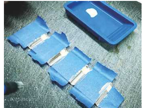
6 Painter's tape is applied to the box exterior, to hold the sides together, and inside to minimise glue clean-up
