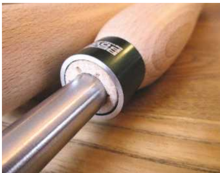
A substantial ferrule adds to the tool's strength and rigidity in use
