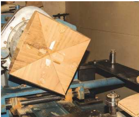
19 I removed the sacrificial wedges that had been used and set up the lathe to cut the top face
