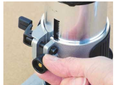
Rack and pinion action gives height adjustment, a cogged wheel on the collar locating on the motor housing's toothed section
