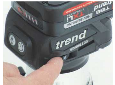
Speed is adjusted via a thumbwheel located on the side of the battery housing
