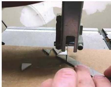
17 Once at the correct thickness, the aluminium is cut into small triangles, which will be used for the box splines
