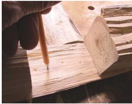
6 Positioning the core ends loosely on one of the sides made it easy to judge where to place an entrance hole for the nest
