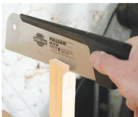
5 Now hold the component vertically in a vice and saw down to the shoulder, removing the waste
