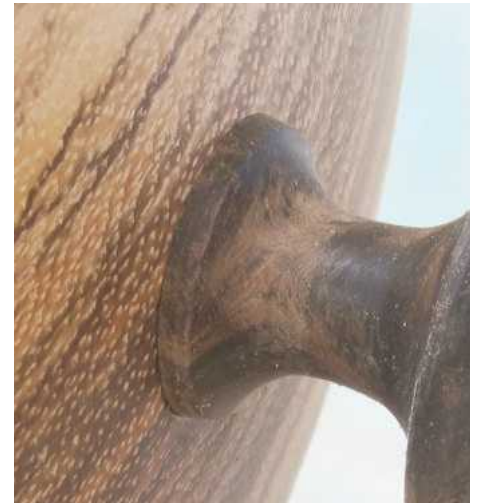
33 The flange on the bottom of the knob has to fit perfectly, so leave a little flat on the zebrano; this needs to be the same diameter as the detail on the ebony stopper's base
