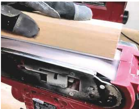
16 When using a belt sander to work down the aluminium bar, ensure to use a piece of scrap wood and wear a pair of thick gloves for protection
