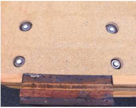
2 End view of workbench showing the fish-plates glued and bolted to improve rigidity
