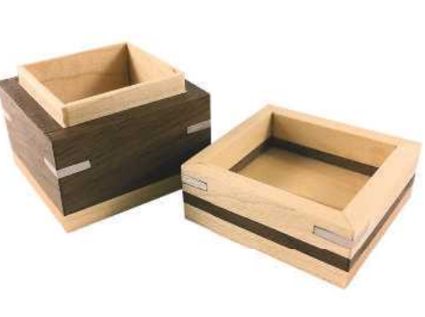
30 The completed walnut and maple box with aluminium spline joints should look something like this
