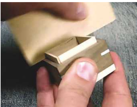
28 In order for the lid to fit correctly, I had to sand small amounts off the liner as it protruded too far. Do this using a sanding block, checking the fit as you go
