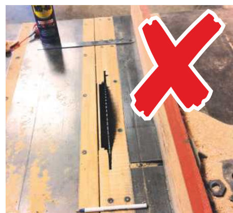
A dangerously modified machine: no guard and the riving knife has also been removed
