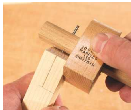
3 Carry the line on across the end of each piece using the same gauge setting
