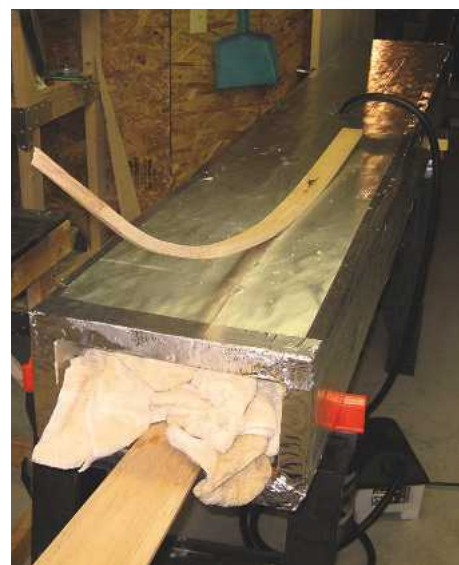
Steam-bending using a homemade steam box
