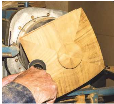
17 Initial power sanding on the bottom face, using a flexible drive fitted with a soft sanding head together with 180 grit abrasive
