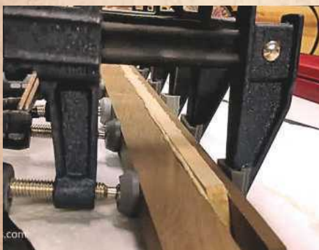
2 ... then clamp up, before putting aside and allowing the glue to dry
