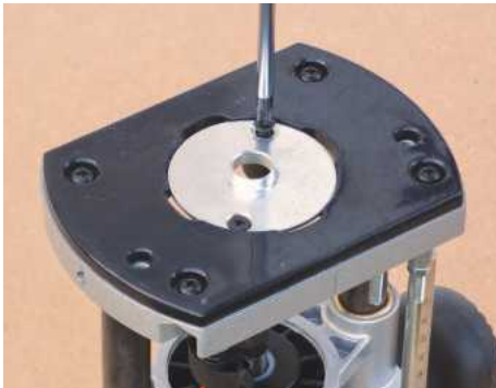
The baseplate follows Trend's time-honoured pattern, with threaded holes for guide bush mounting. A 16mm steel bush fits both bases
