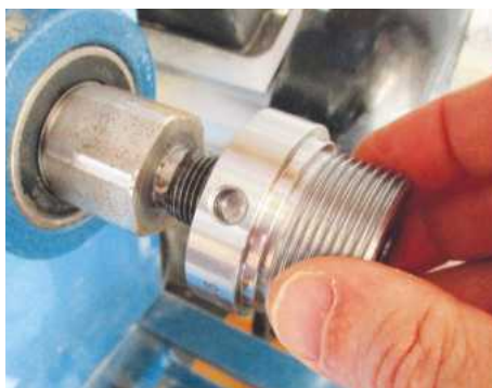
The thread adaptor goes on first...
