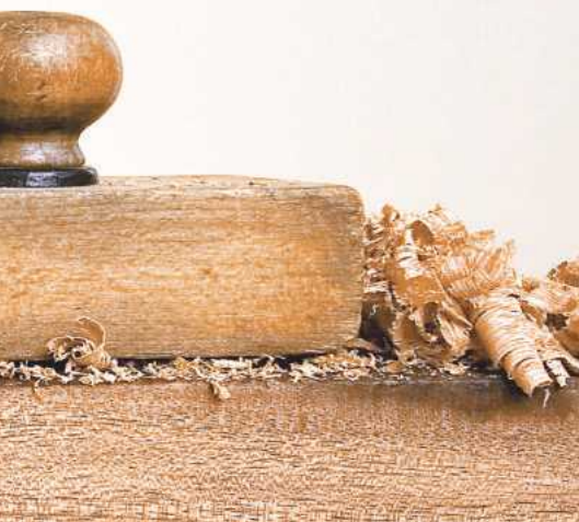
2 Grit or silica embedded in the timber will damage the sole of a plane
