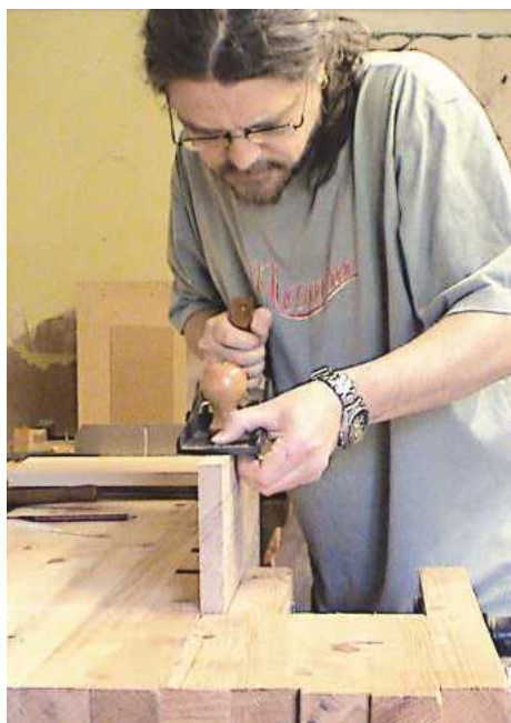
6 Successful edging: I hold the front of the plane body with my left hand, curling my fingers under the sole of the plane, which acts as a fence
