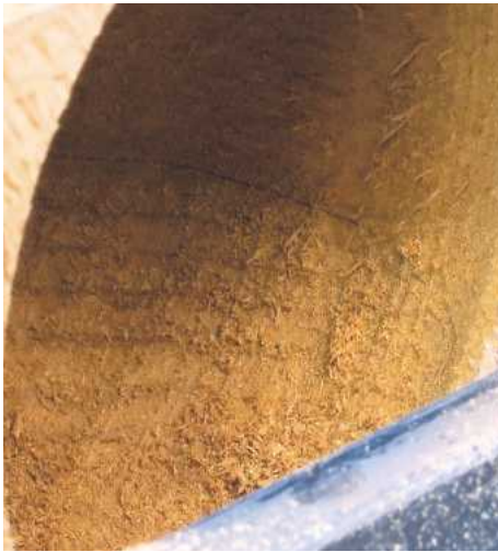
13 The finish left on the dry oak isn't perfect, but does allow timber to be removed very quickly. It's best to clean up the surface with a different tool once you've removed most of the waste
