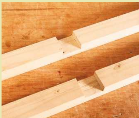
10 Check the fit of completed components, paring more waste away as necessary in order to achieve a perfect fit
