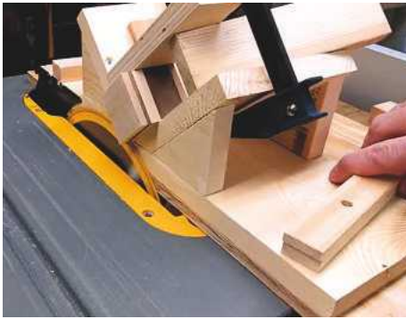
13 My spline-cutting jig holds the box at 45°, allowing cuts to be made through the box corners
