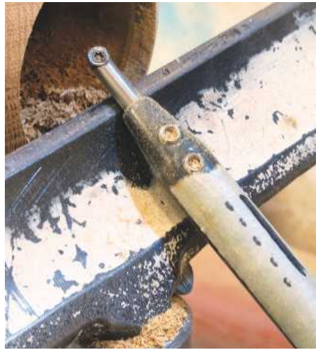
11 The hollowing is carried out using a Simon Hope hollowing tool – the small TCT cutter and big bar is a fantastic combination and facilitates easy cutting. Marks on the top indicate the best position for cutting
