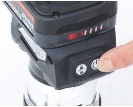
Depressing the first button unlocks and puts the router in standby mode, while the second fires up the motor. Either button can be used to shut it off
