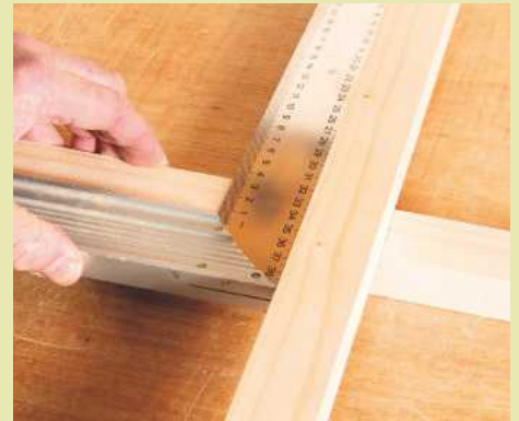
2 Next, lay the divider on the rail with its edge on the marked line, then butt the try square up against it
