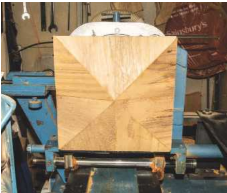
11 The piece set up on the lathe and synchronised with the square cam
