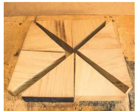
3 After cutting, I was able to match the grain patterns for best effect
