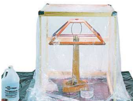
Fuming is a simple and effective chemical stain for wood. Here, a table lamp is placed inside an airtight fuming chamber
