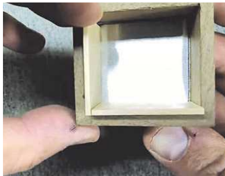
26 Each of the maple liner pieces is glued into position using cyanoacrylate (CA) adhesive
