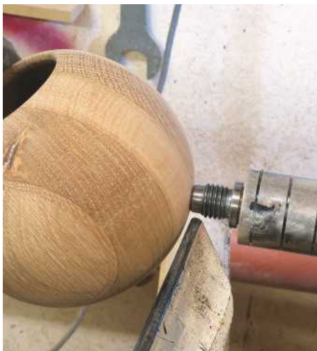
34 The fun part is remounting the salt pig between centres and turning the base so it sits at an angle. If you don't fancy doing it this way, just sand a flat on the underside instead
