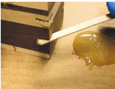
19 Using a basic five-minute epoxy, glue the splines into each of the slots
