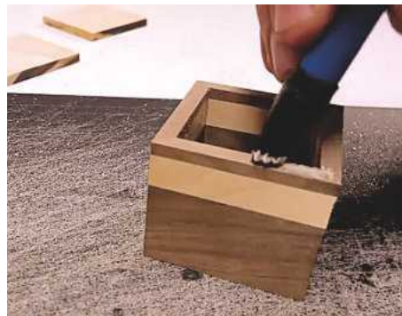
8 Glue is applied to the top panel...
