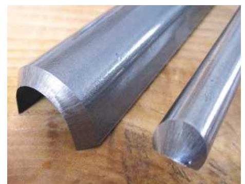
Neatly ground HSS blades ensure the tools keep their cutting edge for longer
