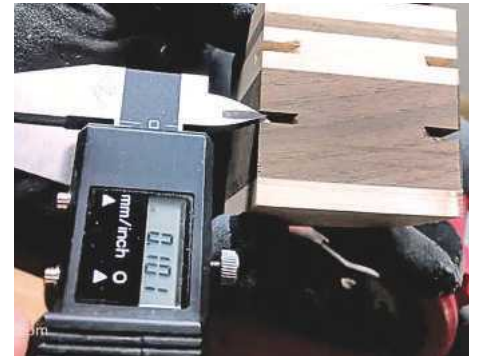
15 After cutting the slots, measure their width using a digital device such as a spline gauge – in my case, the readout was just over 2.5mm
