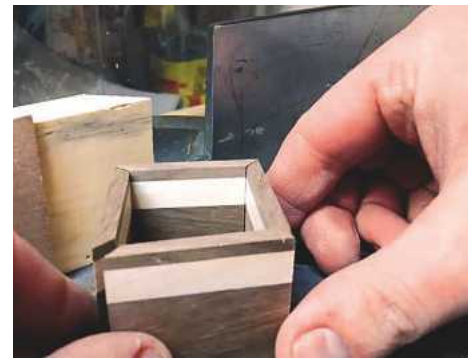
5 Testing the fit after cutting 45° mitres on all four sides
