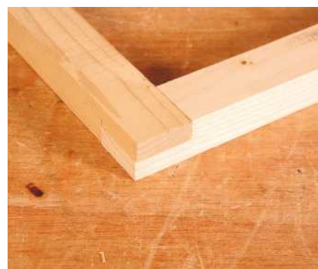
6 Test the fit of the two components, then apply glue, assemble the joint, check that it's square and clamp until the glue sets
