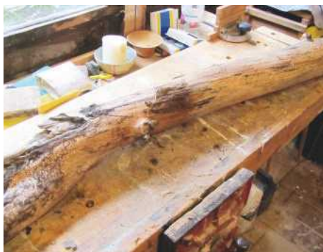
1 The initial log looked unpromising, but the central section was fairly sound, straight-grained, and the ends will brighten the next barbecue
