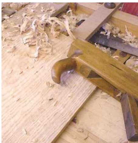
10 Use a scrub plane diagonally across the board to take down almost to the required thickness...
