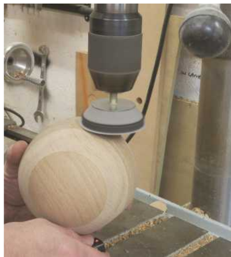
35 The final stage is sanding. Having the sanding pad mounted in a pillar drill is much easier to control than a cordless drill
