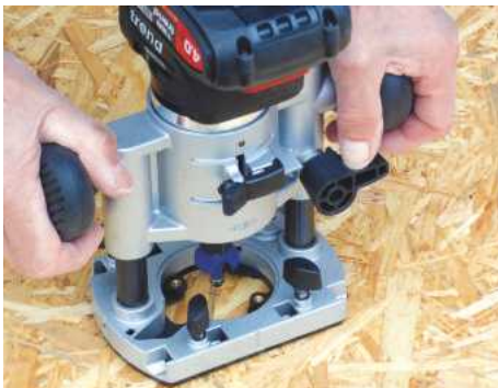
Columns are substantial, with no exposed springs to collect debris, while locking the plunge is via a ubiquitous plastic lever
