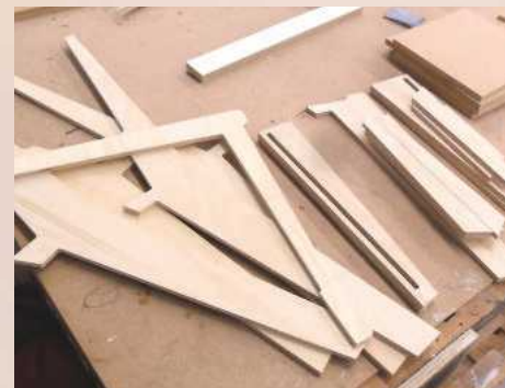
2 After cutting on the CNC machine, the components simply needed cleaning up and sanding in preparation for gluing
