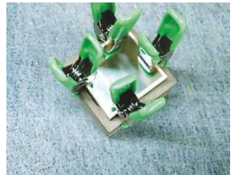
27 Once fitted, the lid is glued, clamped up and left to dry
