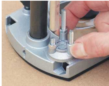
For depth setting there's a three-way turret, with screw adjusters at each position
