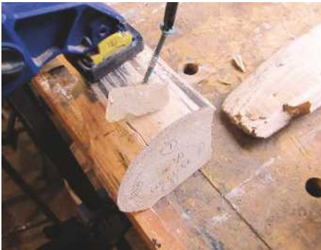
9 A clamp was used to hold a side tight against the core for drilling and screwing. Candle wax rubbed along the thread eases the path for a long screw
