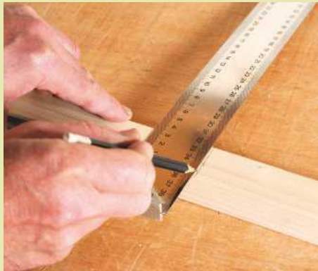
1 On the rail, use a try square to mark the position of one edge of the dividing component
