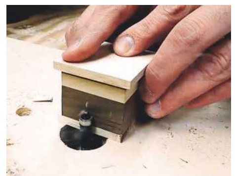
12 Using a flush-trim bit in a router, the top and bottom are squared up and made flush with the sides – PLEASE NOTE GUARD HAS BEEN REMOVED FOR CLARITY
