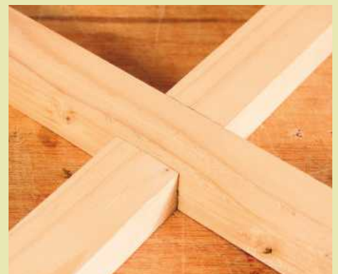
11 Apply glue sparingly to the two notches and assemble the joint. Check that it's square then set aside for the glue to dry
