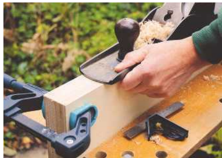
5 Cramp the two jaws together and plane their edges true with a bench plane, checking with a square. Work in from each end towards the centre to avoid splitting the ply
