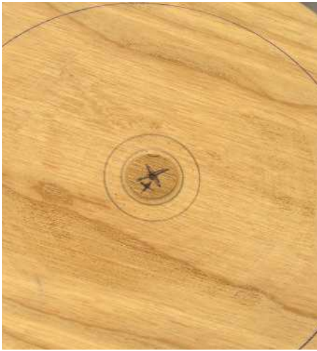
10 I chose to offset the clock slightly – around 5mm will create the desired effect. Mark the diameter of the hole for the clock to ensure it fits in place
