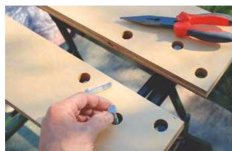
18 Fit the handles, hammering retaining pins through the rods. Add the plastic support blocks and secure both jaws with original bolts
