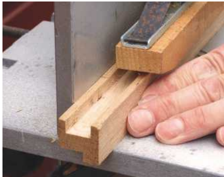
2 Using a straight cutter, rout a groove on the oak's underside, then form the rebate for the glass
