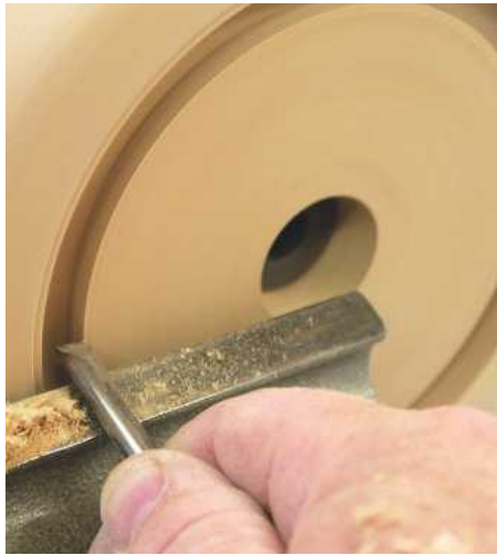
14 To ensure that the tool doesn't bind in the cut, you need to make a cut on the inside. If you tilt the tool over slightly, then the side of the tool will shear cut the timber and improve the finish as a result
