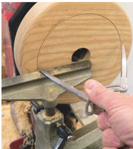
17 After turning the blank around on the pin jaws, the diameter of the hole required must be accurately marked on the other side. If you get this wrong, the holes won't line up and the clock will sit at an angle
