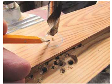
14 The pilot hole gave me the centre for the final keyhole. Drilling from the outside resulted in clean edges. Any tear-out would be hidden by the lock inside
