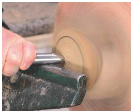
13 Flatten the top surface using a pull cut
