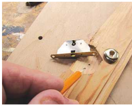
13 Happily the lock's hub – visible in the middle of the keyhole – protruded slightly. Squeezing the lock against the recess served to mark the location for drilling a small pilot hole
