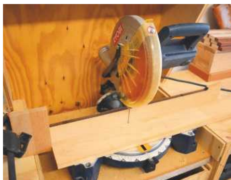
1 Using a powered mitre saw or hand saw and mitre box, cut the 100mm wide strip to length
