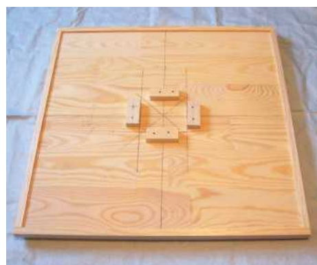
4 Small blocks help to locate the pillar under the top
