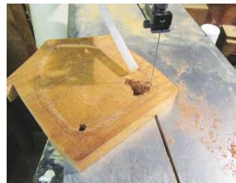
2 A scrollsaw makes short work of cutting a hole that's a little smaller than both the picture and door
