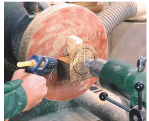
11 Use the tailstock as before to centre the piece, then glue it to the faceplate
