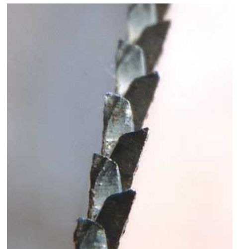
12 Disposable saws are rather coarse for fine furniture making and because of the hardening, their teeth can't be adjusted
