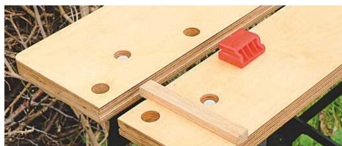
20 Replace the lever springs and check the folding mechanism locks correctly. Add rubber feet and your revitalised Workmate is then ready for action
