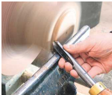
4 ... using the bottom wing of the gouge
