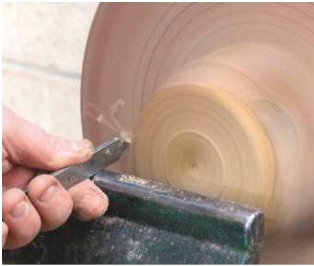
15 Use a parting tool to cut a groove on this mark...
