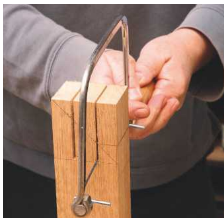
19 Even on simple joints, the coping saw provides a useful way of removing chunks of waste material
