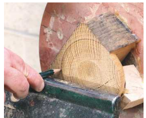
14 Mark the circumference of the outside of the bowl's rim
