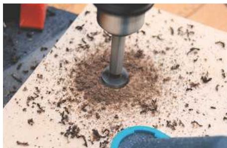
8 Use a 20mm Forstner bit for the bolt and bench dog holes. Cramp the material down and use packing underneath to prevent the ply splitting
