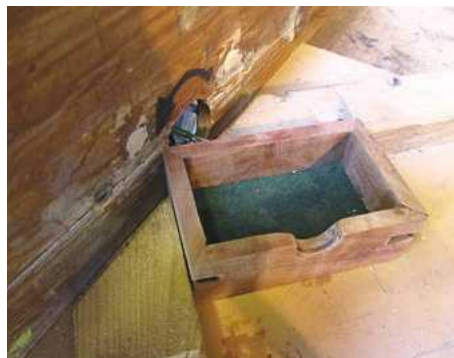
16 The secret drawer – like the main box and an inset tray – had its corners reinforced with dovetail splines cut on my horizontally-mounted router table. The semi-circular notch in the front side allows the drawer to be pulled out with a finger if it gets stuck
