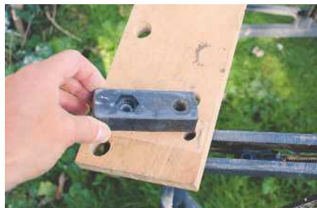
2 Remove the bolts that secure the jaws to the framework. A box spanner is best, although pliers will do. The plastic blocks locate in holes on the underside of the jaws
