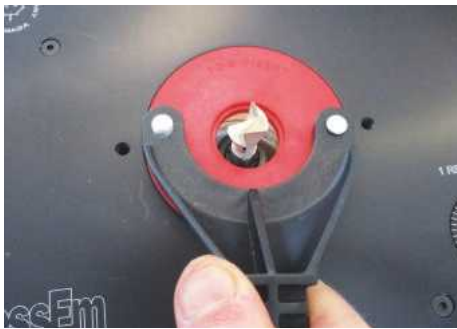
The supplied 'Tab-loc' tool secures the rings in place
