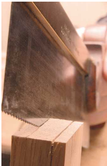
5 When making deep cuts, such as for this joint, the saw blade is continuously guided to stay tight against the waste side of the marked line
