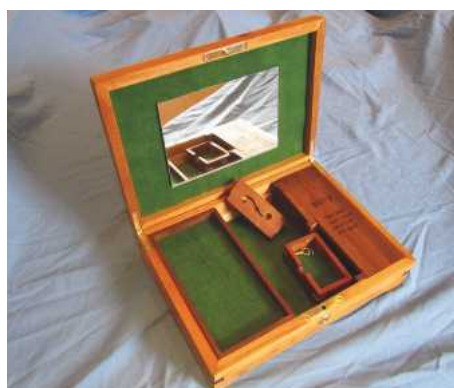
18 The finished box's interior. A shallow tray slides across the top of the teak grid. A glued and pyrographed shelf carries my granddaughter's name and the nursery-rhyme line: 'She shall have music wherever she goes.' The secret drawer is ready to slide into its recess behind a dropped-in wall. I cut a rough hole in the baize of the box's lid so that the mirror – cut by a local glazier for £1 – could be glued directly to the wood with shock-absorbing silicon
