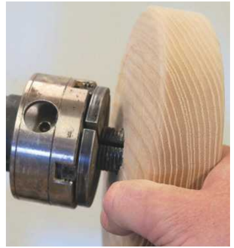
12 Next, mount the blank up on pin jaws. These are an essential part of your woodturning armoury and probably the first additional jaws you should add to your scroll chuck
