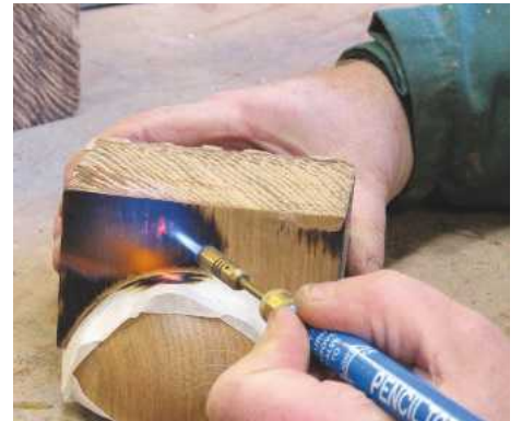
20 Scorch the areas that need texturing using a small gas torch...
