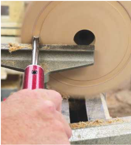
13 The central section needs to be removed and you'll need to ensure that the cut you make is straight. Line up a 10mm skew chisel with the lathe bed, keeping an eye on the speed, as the piece is now running out of true
