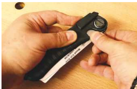
The notch for blade deployment isn't located in the best position
