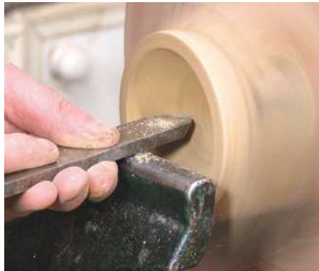
19 Make gentle cuts with a round-nosed scraper to clean up the end-grain
