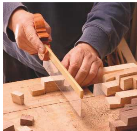
20 Where a large number of similar saw cuts are required, lining them up as a batch saves time and improves accuracy
