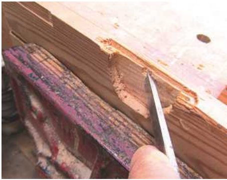
12 Chiselling out the angled recess for the lock wasn't difficult in principle. It did, however, require a lot of adjustment – and several veneer shims – to make sure that the lock engaged fully with the lid and the key could be turned easily
