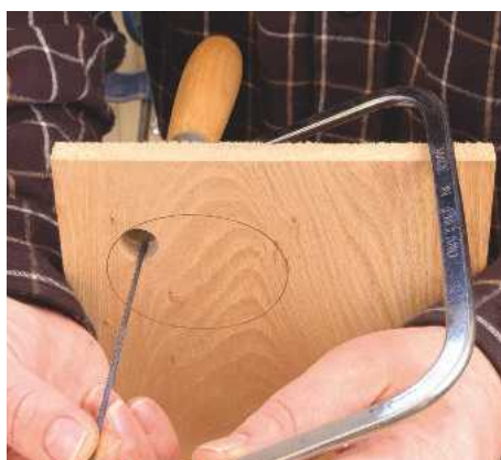
16 The blade can be removed from a frame saw and passed through a drilled hole
