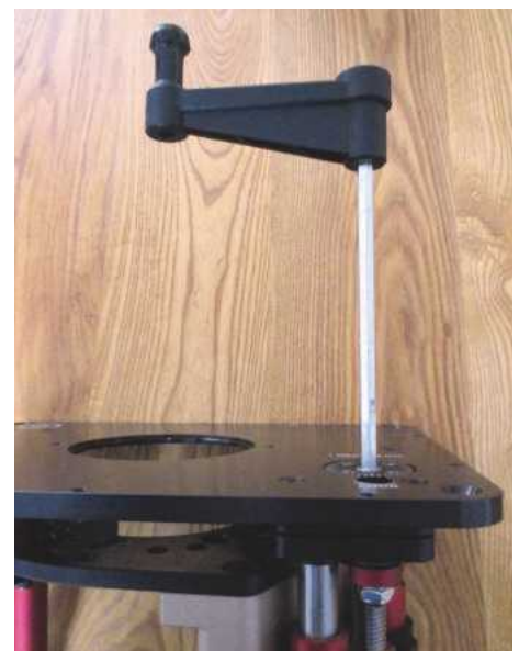
The long handle will clear guards, fences and workpiece
