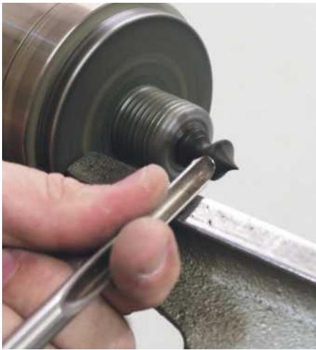
31 Once again, use the pin jaws to hold the 10mm spigot while you turn the top of the finial. You should be able to start sanding the timber at 240 grit, working through 320 and finally 400 to give a smooth surface
