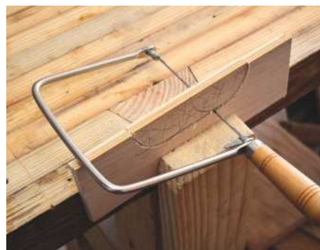
3 ... then use a scrollsaw, coping saw or jigsaw to cut this out
