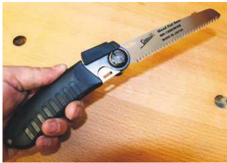
The blades lock out in a straight position...
