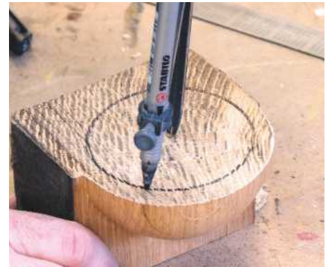
10 Use a pair of compasses to find the centre of the bowl. This involves a bit of trial and error
