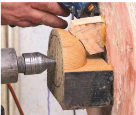
12 Glue in a supporting block under the bowl part
