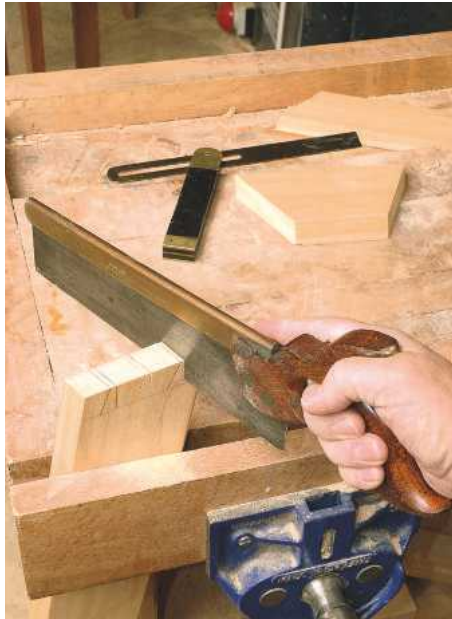
7 With complex joints, it can sometimes be helpful to clamp the wood at an angle to ensure the saw cut remains vertical
