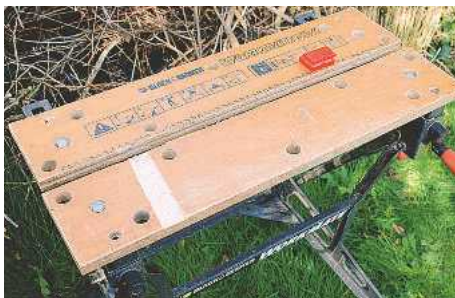
1 There's plenty of life left in this old Workmate yet. The damaged veneered chipboard jaws can be improved by using birch ply, though you'd lose the graduations
