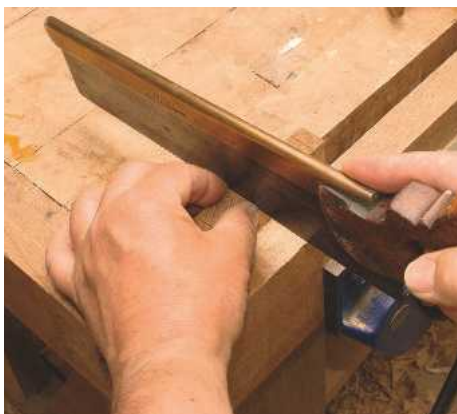
1 The way a saw cut starts is most important – it needs to be clean without any judder, in the right position and at the correct angle
