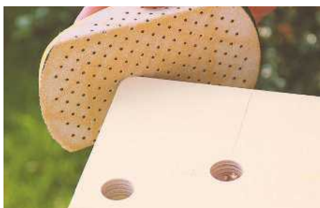
10 Outer corners of jaws can be rounded off for safety. Draw around a suitable coin, then cut with a jigsaw. Finish off with a sanding block
