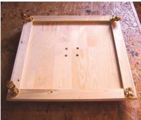
9 The castors in place
