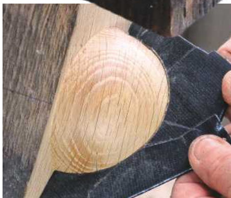
7 ... and keep offering up a template to ensure accuracy
