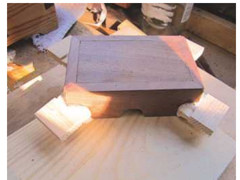
17 Once the glue had dried on the dovetail splines, they were trimmed on a bandsaw, then planed and sanded. Each set of splines and slots was cut with the same router bit set to the same depth. Switching from slots to splines was just a case of lowering the cutter
