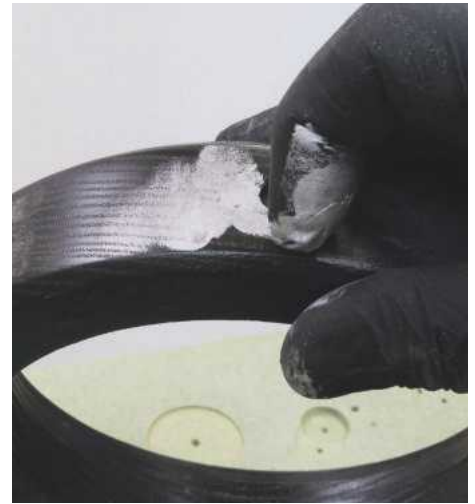
33 Even though I sprayed the ash, the grain was still open and this is ideal for filling with gilt cream. I used silver as it matched that of the clock. Rub it in across the grain, ensuring that all low points are filled up
