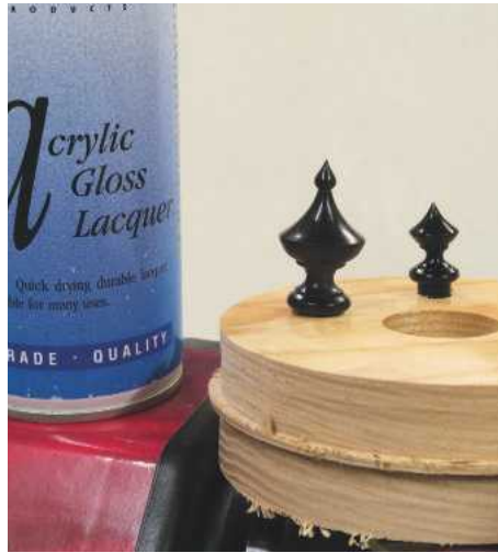
32 I like my ebony to be really shiny and the gloss lacquer gives a great long-lasting finish. Apply a coat then, when dry, cut back with '0000' wire wool before giving it a final spray
