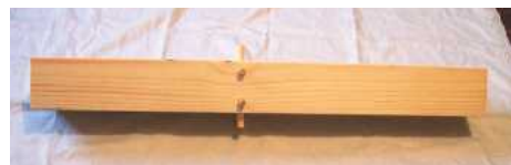
2 The central pillar with middle shelf supports
