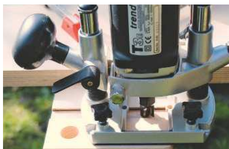
11 When preparing thin timber, it's handy to have a solid stop to plane against. Rout a groove across one or both jaws, cramping a board as a guide
