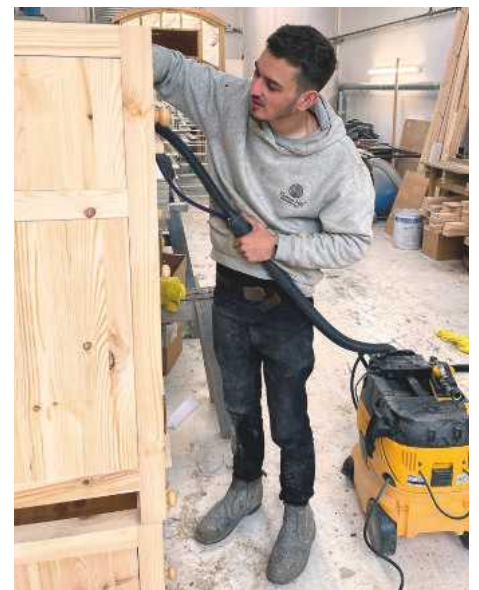
Sanding fixtures and fittings for a new Shepherds' Hut
