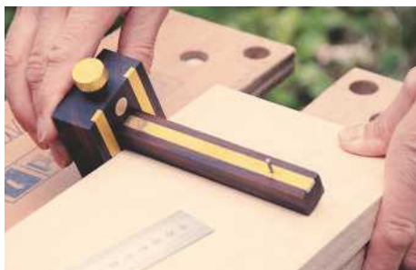
7 Mark out centres for mounting holes. These need to be accurate, otherwise you'll have problems later when attaching the jaws to the steel framework
