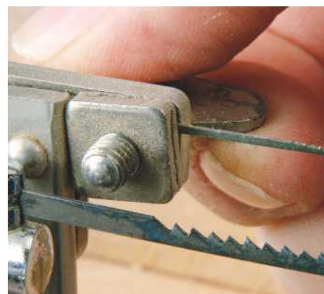
17 The plain ends of a fret saw blade – behind – are clamped into the frame while the pegged ends of a coping saw blade – front – are hooked in place
