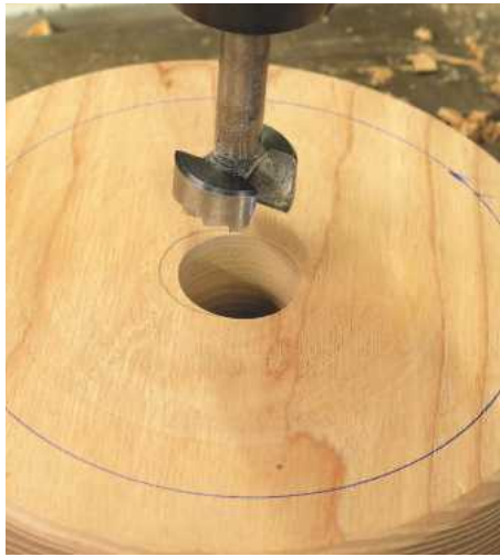
11 The hole needs to be accurately drilled through the piece and the drill press is the tool for the job. 30mm is the correct size to suit my pin jaws
