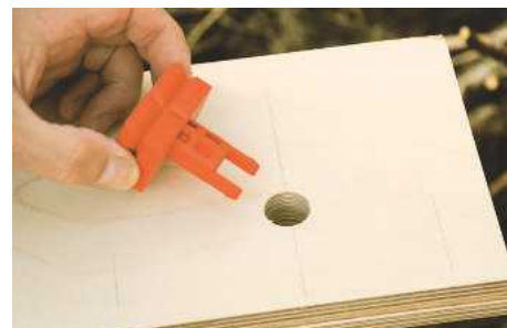
9 Check that bench dogs fit snugly in the holes. If you need to, new ones can be made from close-grained hardwood, turning spigots to fit
