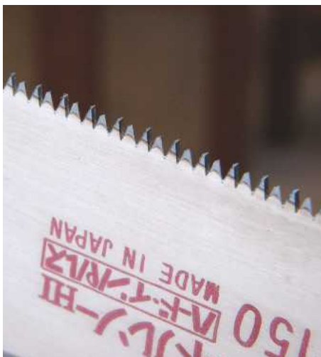
11 The Japanese back saw blade is thin and very suitable for sawing fine joint details
