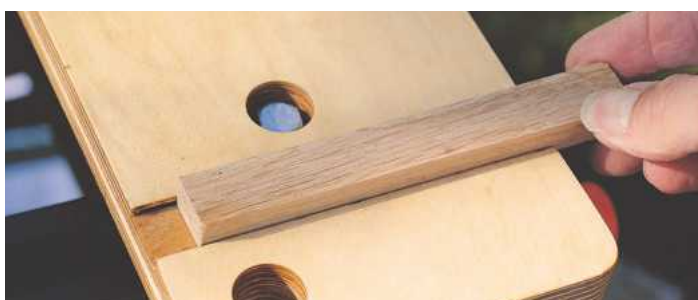
19 Prepare a piece of hardwood for the planing stop. It should be a push fit in the groove and routed to 3mm deep, or, secure with countersunk screws
