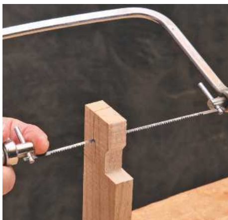
18 Frame saw blades can be guided to follow tight curved or complex joints, such as the one shown here, or on decorating features
