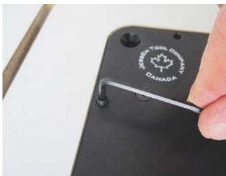
If the plate height needs to be tweaked, it's easy with the 10 height-adjusting socket screws
