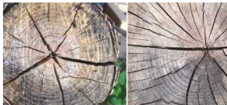
Radial cracks in elm and maple logs
