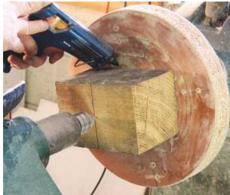
2 Use the tailstock to centre the piece and glue it to a faceplate
