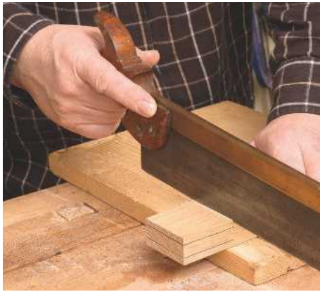
6 Here the wood is held down on a simple guide, known as a bench hook, while making a wide saw cut for the shoulder of a joint
