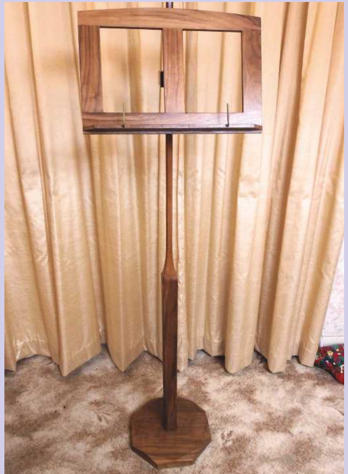
Michael's adjustable music stand in American black walnut, featuring a square lower section which morphs into a slender octagonal upper section
