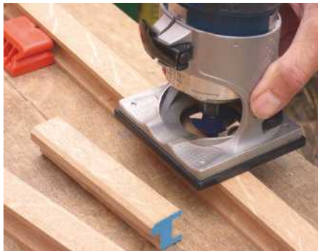
4 Once happy with the profile, rout a decorative chamfer along inner and outer edges of the oak
