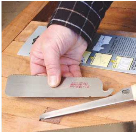
9 Japanese back saws have a different construction to European and American versions. The blade is hooked into a slotted back, which has a wooden handle bound on
