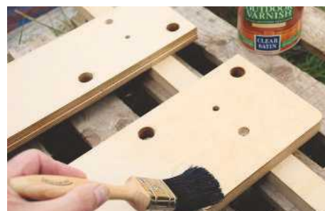
12 Sand both faces of the plywood and remove arisises with a sanding block. Apply two or three coats of a suitable satin varnish to all surfaces
