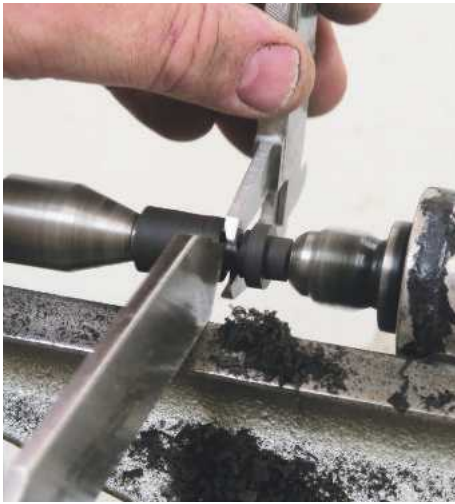
28 Mount the ebony between centres, using drives with very small points as they can split the wood when working on pieces this long. Turn a 10mm spigot on one end to suit the holes in the ring
