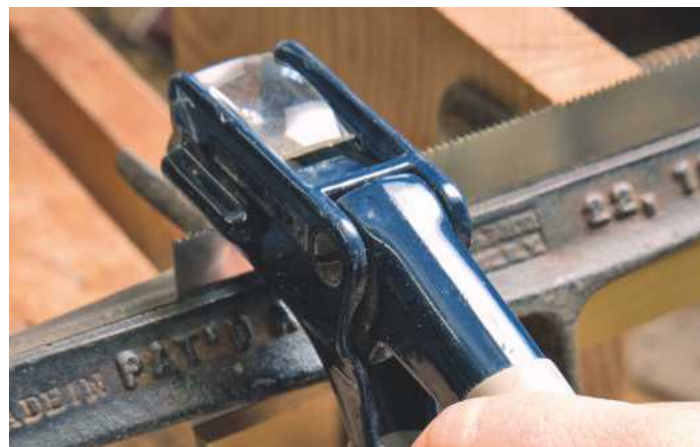
14 The teeth are hardened to keep their sharpness while making them brittle and the blade disposable
