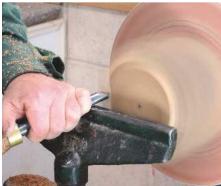
3 Make pull cuts to start shaping the outside...
