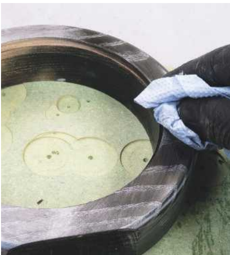
34 Remove the excess by rubbing off with a rag. I used lemon oil to act as the lubricant for this process but finishing or Danish oil will do the same job – you can still add a little more gilt cream if required
