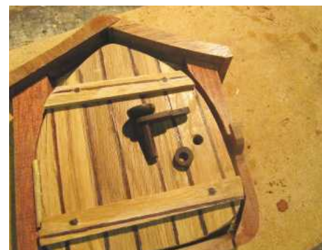
5 A 35mm-long turned wenge spindle fits through three holes – one in the door, the others in a glued-on latch-bar and washer
