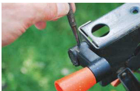
13 Front handles need to be detached so that the threaded rods can be removed before spraying. Use a nail punch on the retaining pins
