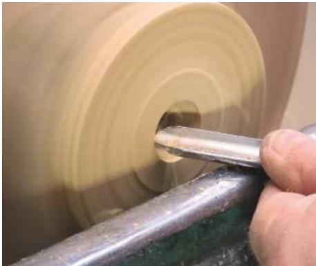
18 ... then hollow from this hole, cutting towards the rim
