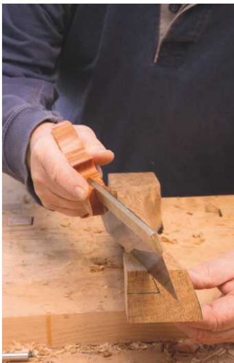
4 By keeping the head centred with one eye above either side of the blade, you can watch to ensure the saw doesn't deviate from a straight line
