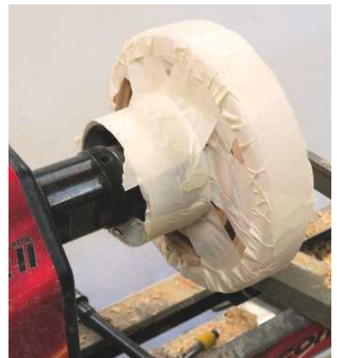
18 It's not easy to just cut through, so you need to prepare for the point when the blank becomes two pieces. Lots of masking tape wrapped around the piece will stop the ring flying off and breaking
