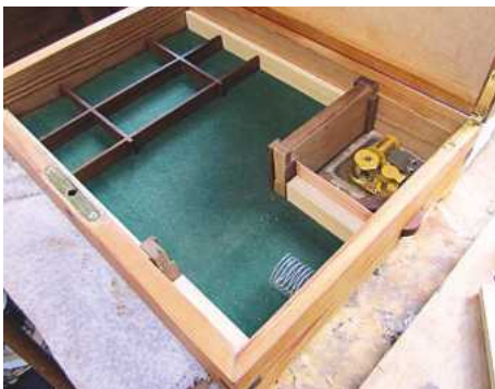
15 The shallow grid, made of teak offcuts, is simply half-jointed, rubbed with teak oil and glued into place. The empty space in the middle of the box allows room for a secret drawer to spring open when a retaining wall is lifted out
