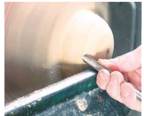
6 Swap to a small spindle gouge for finalising the shape...
