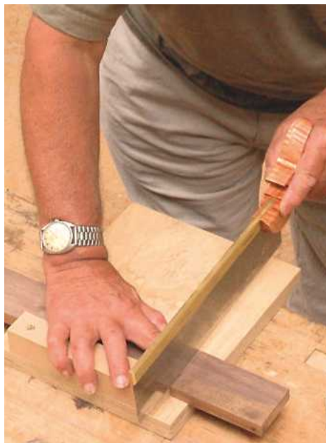
2 Using a bench hook left-handed to guide a wide saw cut. The hook is designed to be used on either side while the saw is held in the left hand; the fingers of the right hand are used to guide the start of the cut
