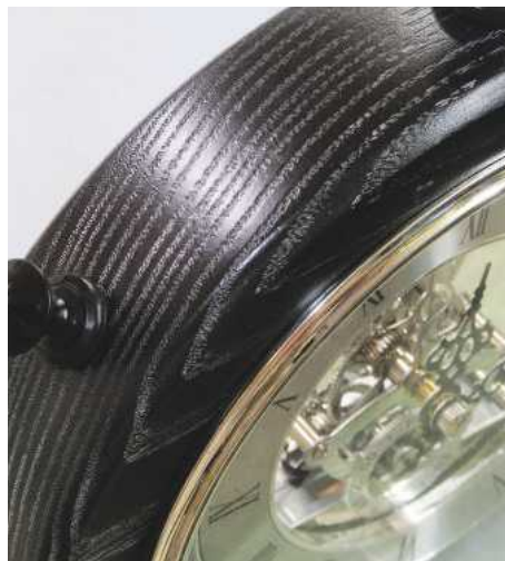
35 The grain should now be completely filled with the silver cream. Check for any torn-out grain or scratches left from sanding as these will also fill up with silver, which can make the final project look messy
