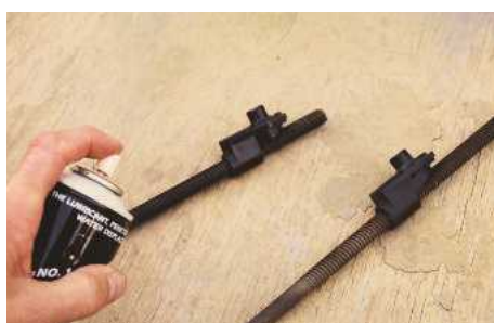
17 Clean the threads and treat with a spray lubricant. Remove masking tape, allow paintwork and varnish to harden, then reassemble the bench
