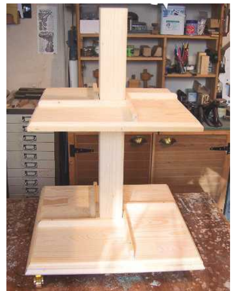
11 A dry assembly to check out alignment
