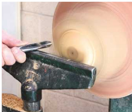
5 A push cut helps to flatten the base
