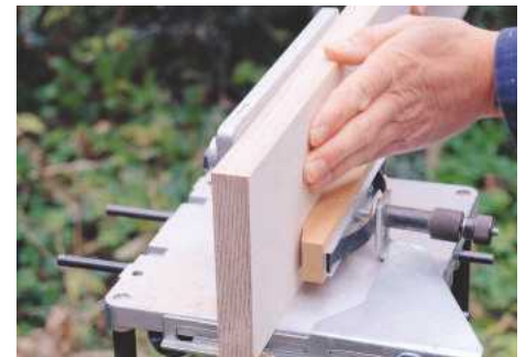
6 Inner edges of both jaws have a 'V' groove running along their length. It's easiest to produce a groove using a router table
