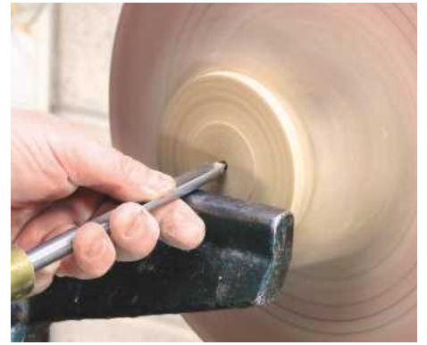
17 Drill a hole in the centre of the bowl with a spindle gouge...
