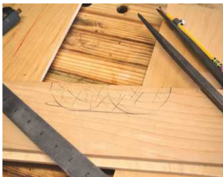
2 Use a pair of compasses and combination square to lay out an appropriate looking curve; this will become the handle...
