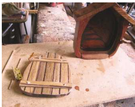
4 Bracing struts add character to the door. They're glued on and pegged with matchstick-sized pieces of oak tapped into drilled holes
