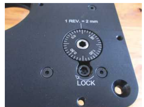
Fine adjustment with a clear gauge and lock
