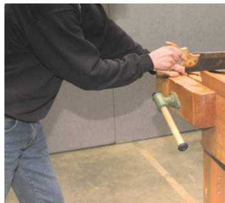
3 Once the cut is under way, the furniture maker stands back from the bench, providing room for the arm to sweep back and forth in a straight line
