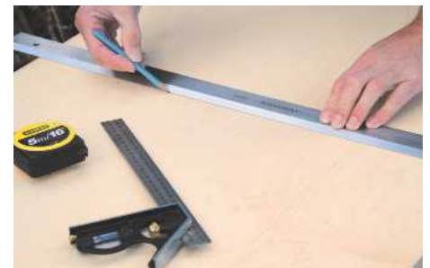
3 Mark out the material for the new jaws. Birch ply is probably the most stable, although MDF is a cheaper alternative. I made the rear jaw 25mm wider than the old one
