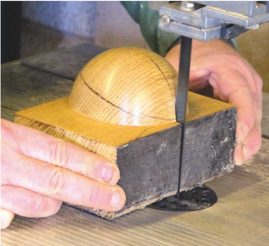
9 Use a bandsaw to cut the piece in half – centre lines drawn earlier will help here
