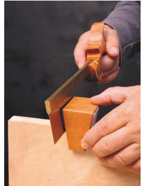
8 A handy magnetic guide can be useful for sawing occasional angled joints
