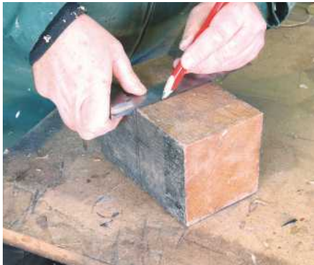
1 Mark a centreline around all four faces and the centre of one face
