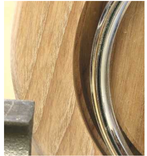
15 The silver ring requires you to cut a small step on one side. You could measure this, but I just kept making small cuts until the ring fitted in snugly. This ring will hide any problems if you end up with the main hole being a little too big
