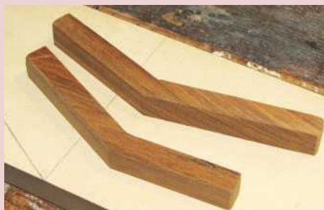
9 150° formers used in assembly of the upper and lower octagons' sides
