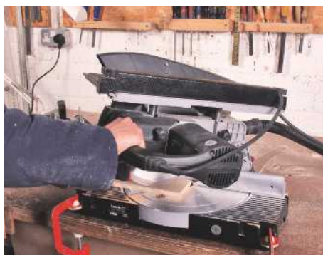
2 Extend the line onto all faces; this will allow you to line up the cut with your saw blade
