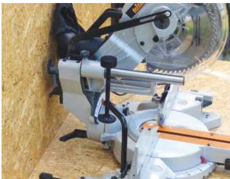
The saw can be positioned so the bar ends are almost touching the wall, which is significant in a small workshop where space is limited
