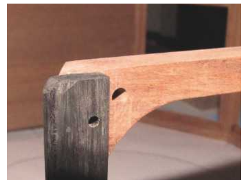
12 Clearance hole for a No.3 screw drilled in beading
