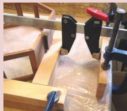
13 Gentle pressure applied to the block closes the joints as the glue dries
