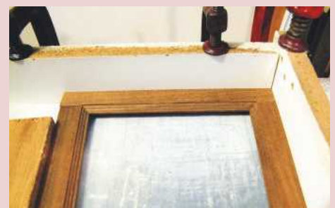
7 Similar right-angled jig used to ensure side frames are square
