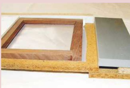
5 Jig to ensure frames that make up the octagon are square and to compress joints while glue sets
