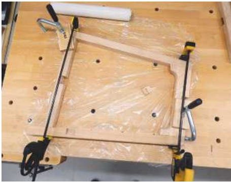
16 Unfortunately, assembly of the first frame wasn't going too well. The top frame on one side wouldn't come together fully, so I gave it a tap with a leather-faced mallet – then heard a pop...
