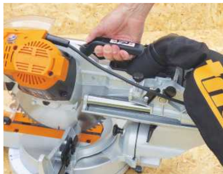
A built-in handle on the upper bar allows you to move the machine around, though at about 20kg it's not exactly lightweight
