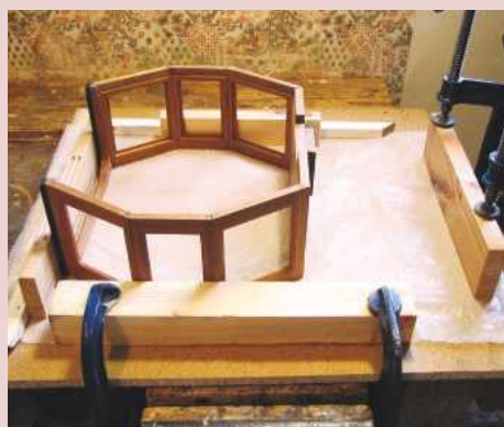
11 Any sideways movement of the octagon is restricted by the guide in the foreground
