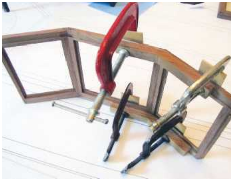
8 Starting to assemble the octagons using a pair of 150° formers to ensure consistency
