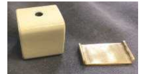
Collars for the pinch sticks use scrap 25mm steel box section
