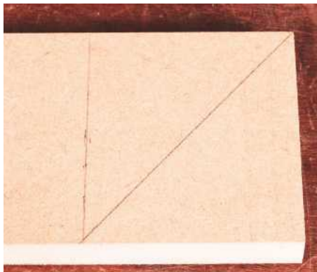
2 Mark the diagonal – this is the mitre angle you need to cut on the first part
