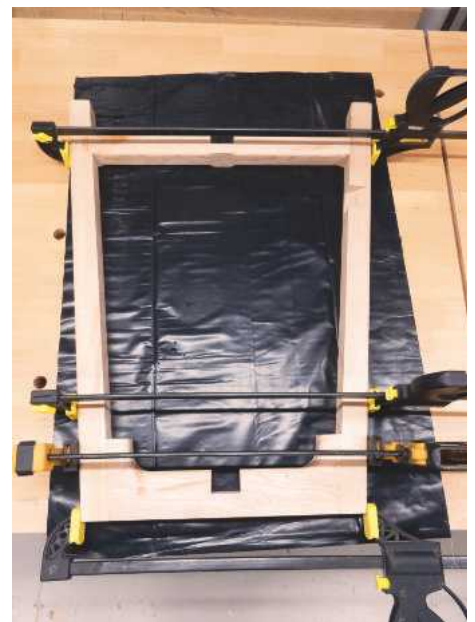
21 The second frame was assembled with just one leg glued – the other needed to be removed to allow the two frames to come together
