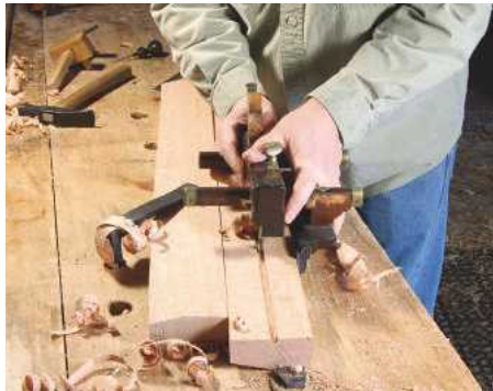
Peter Follansbee ploughing a groove with a plough plane
