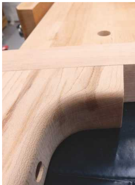
20 When the epoxy had cured, I scraped and sanded until the repair was only just visible. Once finish was applied, however, it was very difficult to detect the repair at all
