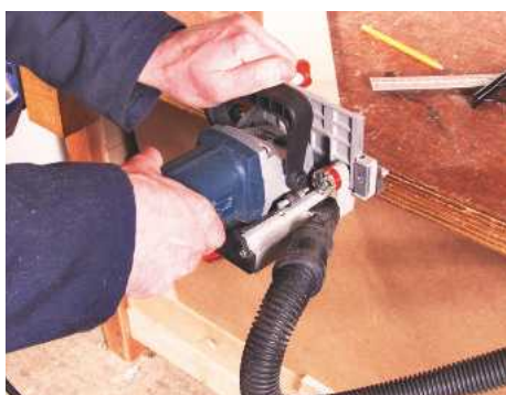
4 Insert a biscuit to strengthen the joint, then mark its position on both parts
