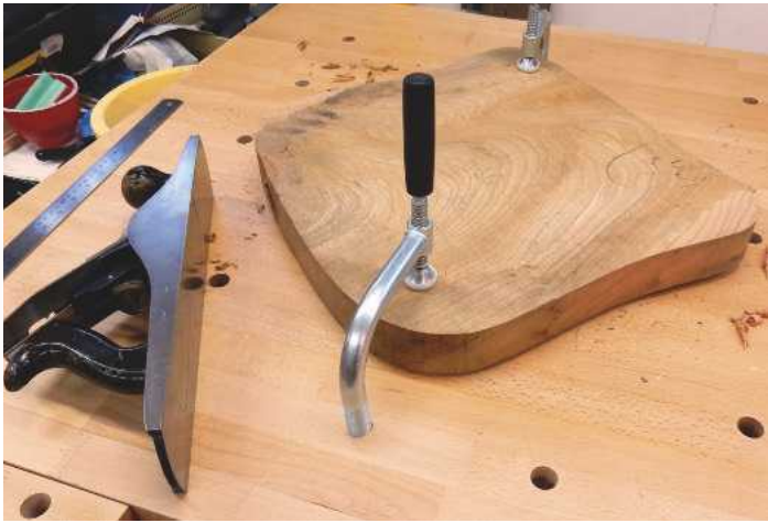
1 The seat blank was far from flat, so using a hand plane, I started by removing some of the high points from what would be the top surface
