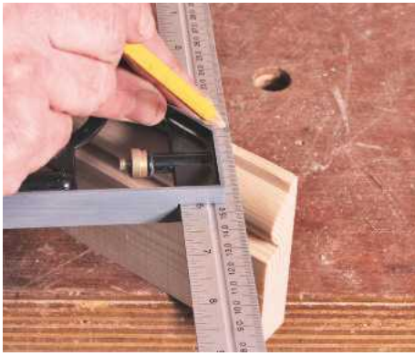
1 Using a mitre square, mark out the 45° cutting angles on the two components
