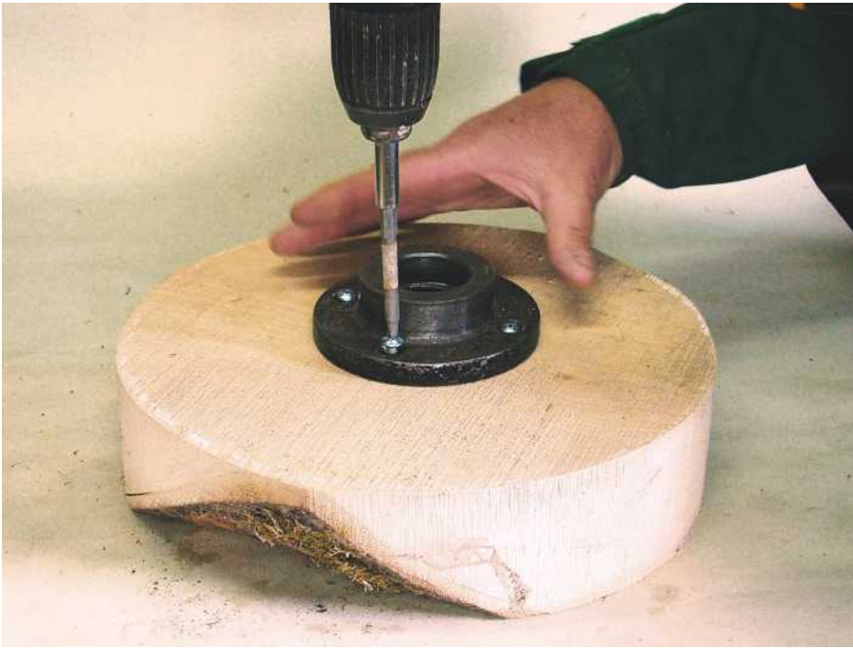
1 Find the centre of the blank and screw a faceplate to it
