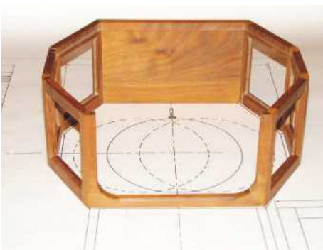
10 Dry assembly of the lower octagonal enclosure...
