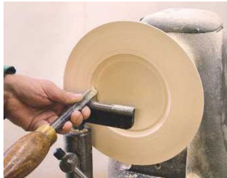
13 Repeat this cut, going a little wider and deeper each time
