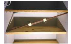
One of the pinch sticks being used to measure a cupboard alcove
