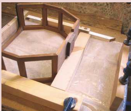
12 A load-spreading block forms the fourth side of the clamping jig
