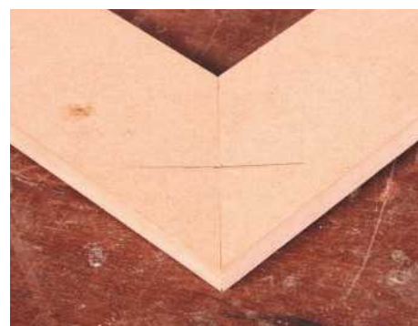
6 Apply glue to the mating surfaces and assemble the external corner joint
