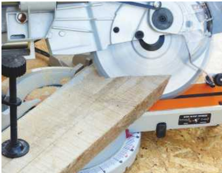
With an 1,800W motor, there's no shortage of power for those deep cuts in heavier timber, which are often necessary for compound bevels
