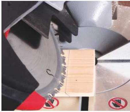
2 Make the cut on both parts. Using a mitre saw is the most accurate method of doing this
