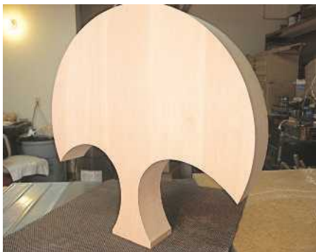
2 After glue-up, I used a bandsaw to cut out the basic shape
