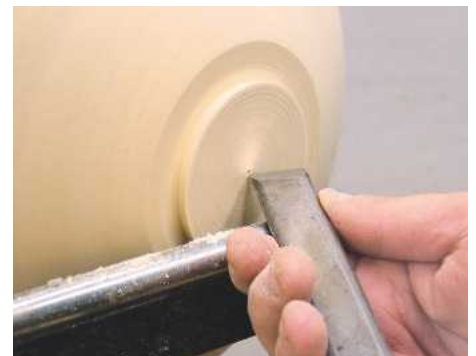
5 Dovetail the spigot and cut a pop mark in the very centre
