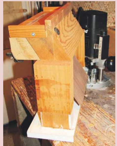
2 Upper octagon top in the 60° jig – note leg extensions on the jig
