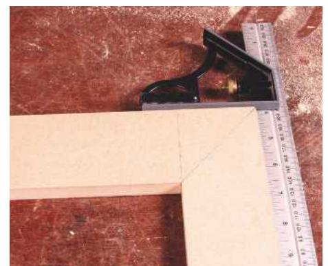
6 Assemble the right-angled joint, after adding a biscuit if additional strength is required
