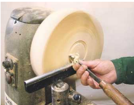
3 Use a parting tool to cut the chucking spigot
