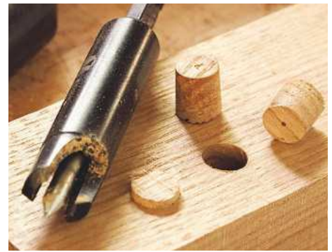
Montana Brand plug cutters: the self-centring bit ensures accurate results with a hand-held drill. The bit is tapered just a little, so plugs fit snugly
