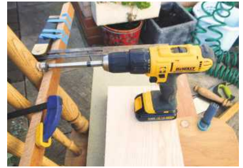
6 Setup for drilling the back uprights
