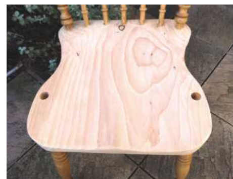
3 Cedar seat after stripping the finish using scrapers
