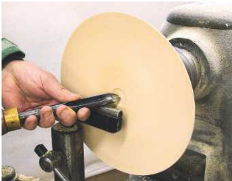
12 ... and swing the handle, moving the cutting edge towards the centre
