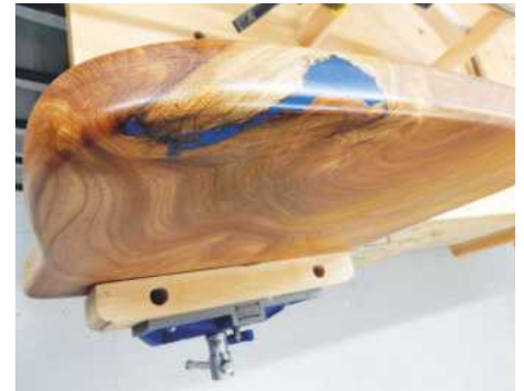
5 I rounded over all the edges with a router and, after more sanding and some buffing, the grain pattern came alive. There were some air bubbles exposed in the resin but as these would be on the underside and therefore hidden, I chose to ignore them
