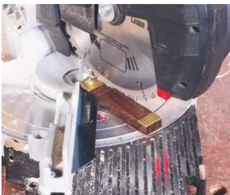
4 Transfer the angle from sliding bevel to mitre saw, then make the cut
