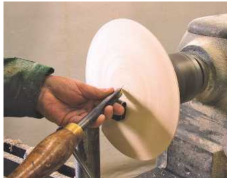
10 Start hollowing with the tool handle well over the bed bars
