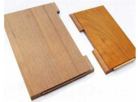
5 Loose tongue in the top of the upper octagon (left) and bottom of the lower octagon (right)
