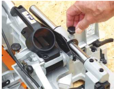
Locked for storage with a thumbscrew, twin offset horizontal bars allow the saw head to travel a maximum distance of 210mm
