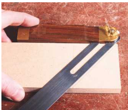
5 Re-set the sliding bevel on the second piece, transfer this angle to the saw, then make the cut
