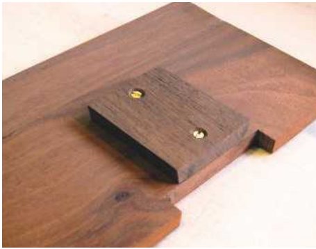
7 Dovetailed tenon fixed to the underside of the lower octagon's base
