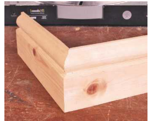
6 Glue the mating surfaces of the components and bring the joint together: perfection!
