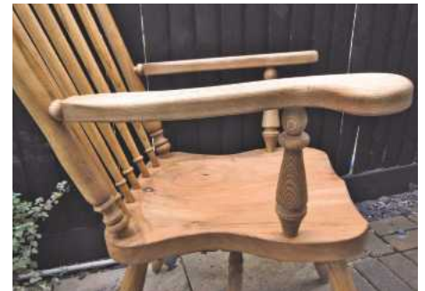
7 The new arm assemblies in place
