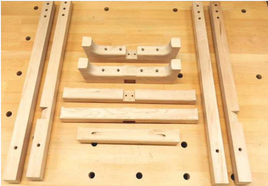
15 The next step was to shape all components using a bandsaw and drum sander, before rounding over most of the edges on a router table
