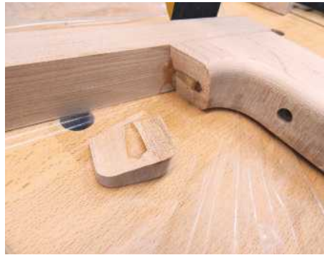
17 Mistake number 3: I'd applied too much epoxy to the dowel holes and the hydraulic action when I tapped with the hammer burst the wood along its grain. At least the joint now came together, though!
