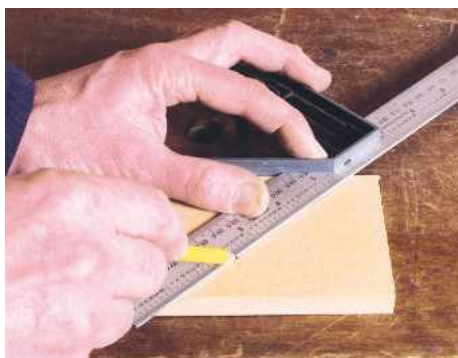
1 Use a mitre square to mark the position of the corner mitre on your workpiece
