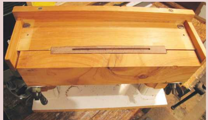
4 Completed 3mm wide x 3mm deep slot
