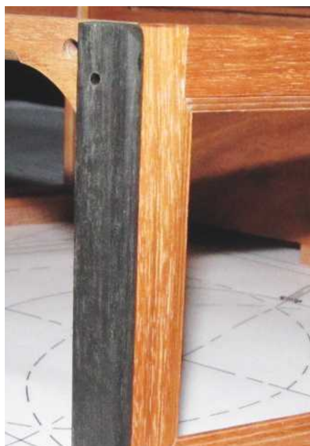
13 Beading with clearance hole drilled to allow screwing to side frame during assembly
