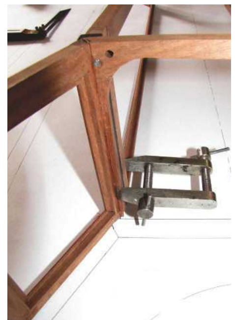
14 Toolmaker's clamp and screw to hold joint when gluing
