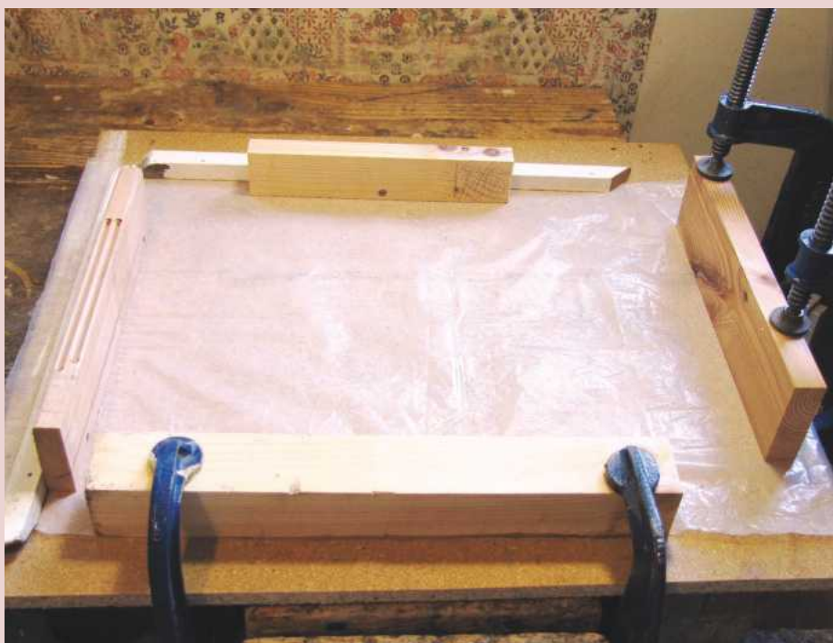
10 A flat board covered in glue-resistant film and a pair of right-angled fences
