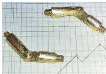
2 Hinges fashioned from the two pin plugs
