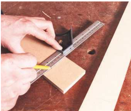
1 Using a try square for accuracy, mark the width of one piece on the end of the other
