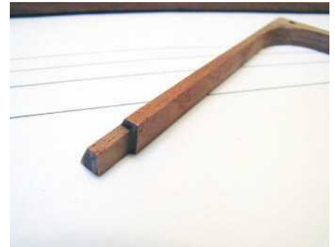
6 2mm deep rebate around the sides of the top frame (lower octagon)
