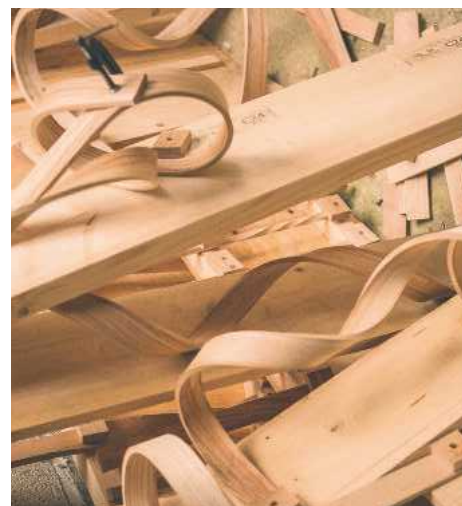
Steam-bending is an age-old process that allows wood to be manipulated into an array of remarkable and interesting shapes Photograph courtesy of www.tomraffield.com
