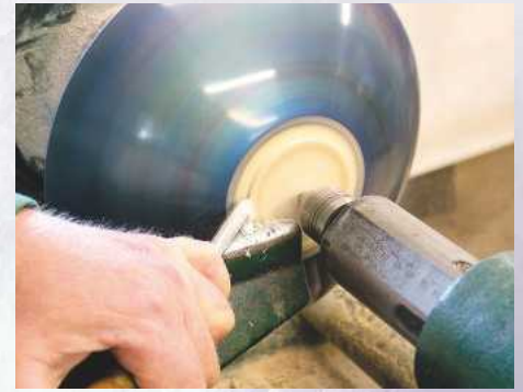
25 Reverse the bowl onto a mushroom-shaped dolly and remove the chucking spigot
