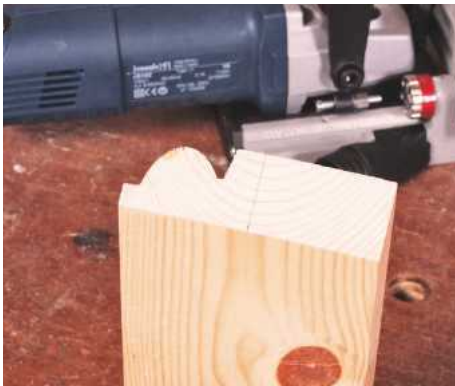
4 Set the joiner to position the biscuit centrally in the thickness of the timber
