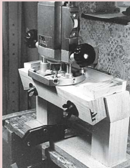
1 The original height of the 60° jig used to cut mortises in lower octagon frame members
