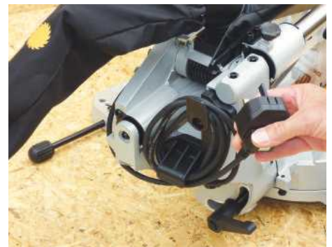
When not required, brackets at the rear allow the mains cable to be neatly wrapped for storage
