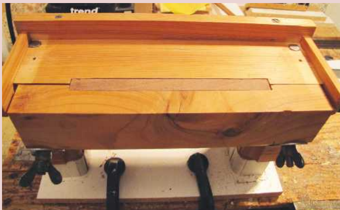
3 Side frame in 60° jig
