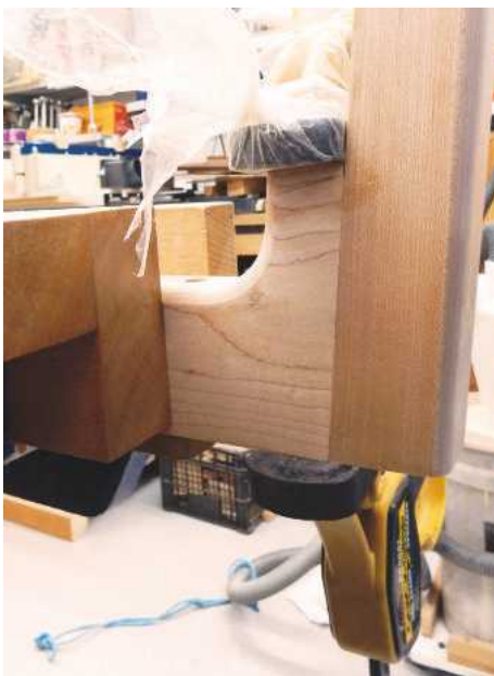
19 The next day, I cleaned out some of the cured epoxy so that the piece fitted back in place. More epoxy was then applied, albeit sparingly, and the component clamped in position
