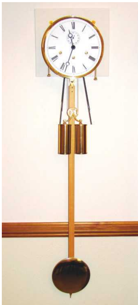
1 Movement and dial set up to check case dimensions
