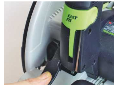
This lever controls the blade guard and will flip it back with ease
