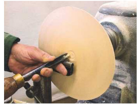
11 Once the cut is started, roll the tool anti-clockwise...
