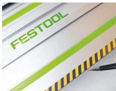
The guide rail, showing the plastic edge strip – a darker colour would have shown up better
