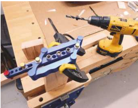
10 I used 10mm dowel joints: three in the top rail and one in the bottom rail. Mistake number 1: I managed to slip while drilling one of the holes in the top rail and therefore ended up with an oversize hole. To overcome this, I decided to use epoxy to glue the joints together, although I have to admit that I'd never done this before
