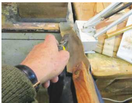
16 A few strokes against a stiffish piece of leather puts a final polish on the edge and removes any loose metal particles left over from the grinding
