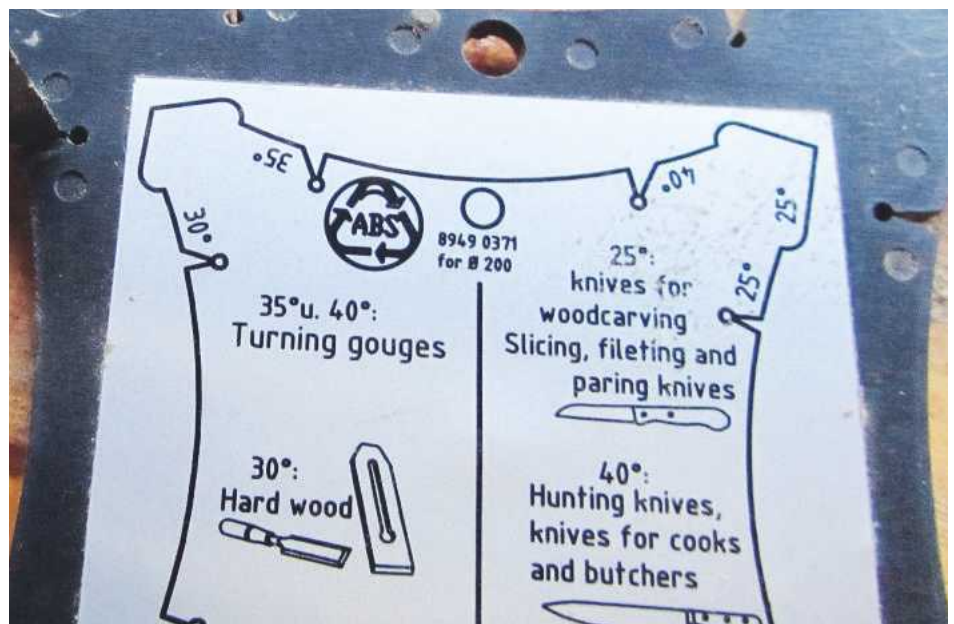
11 This angle gauge – like most of its kind – is too small to be reliably accurate; I spent 20 minutes cleaning to make sure it was readable enough for a photo!
