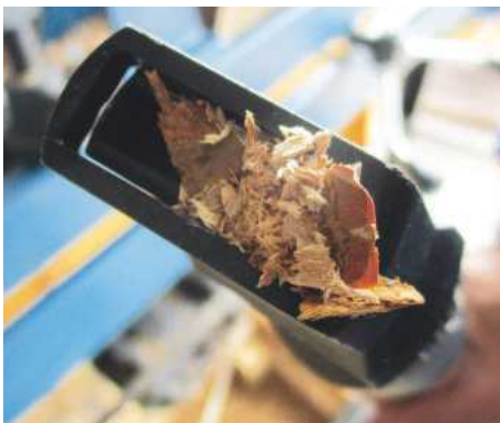
The crevice tool can get blocked with bigger chips
