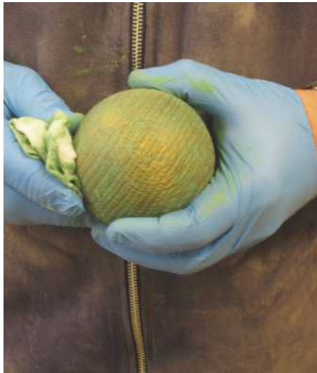
32 Work it in to all the low points in the texture before removing the excess with a rag. Naturally, the green areas on copper appear in the parts that can't be polished
