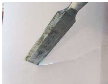
17 A smooth cut through paper is not a bad test of a blade. For my money, this edge is now ready to go back to work, not more than five minutes after starting
