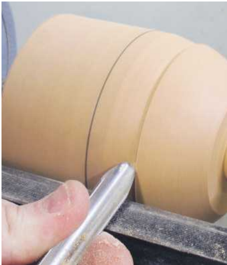
13 Using a spindle gouge, start with the bevel rubbing, lifting slightly to engage the cut and rolling over the end of the work. Ensure to keep the bevel in contact the whole time
