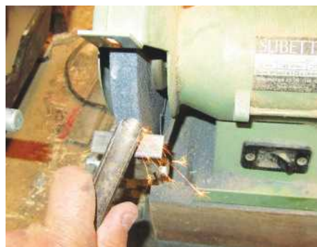
18 Turning tools aren't hard to sharpen freehand. Roll the bevel against the wheel until sparks just begin to fly over the nearside face. Lift the tool off frequently to let it cool and check the bevel is smooth. Finish off on a felt wheel, but don't bother removing any wire-edges; the lathe will do that in seconds
