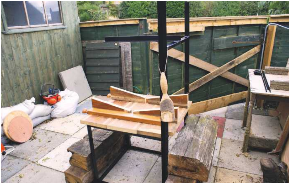
1 The structure of the chainsaw platform is made using 45mm angle iron, 900mm square. It has a table height of 900mm, on which I built a sturdy board with 'V' blocks to secure the timber. The chainsaw chair, as I call it, also uses a piece of 1,500mm angle iron and 3 x 600mm spikes secure the material from above while cutting
