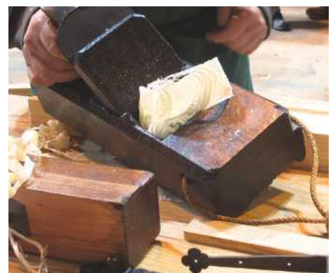
A monster of a cornice plane made by Philipson in around 1750. Although manufactured in England, it would almost certainly have been made for the US market as all the English cornices were made of plaster, not wood. The profile of the blade is around 100-125mm wide
