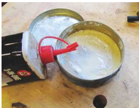
13 Jeweller's paste, used on leather wheels to polish an edge, often dries out in a workshop. It can be revived, however, by mixing in a little oil
