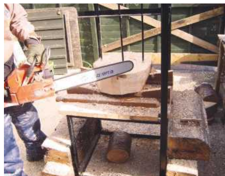
6 I then trim up the remainder of the blank as close to a circle as possible
