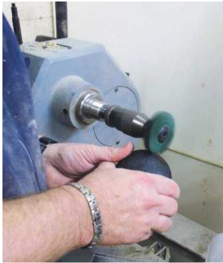
29 Get a good hold of the work when brushing away the carbon deposits from the ball; you must clean off all the loose material before painting the work
