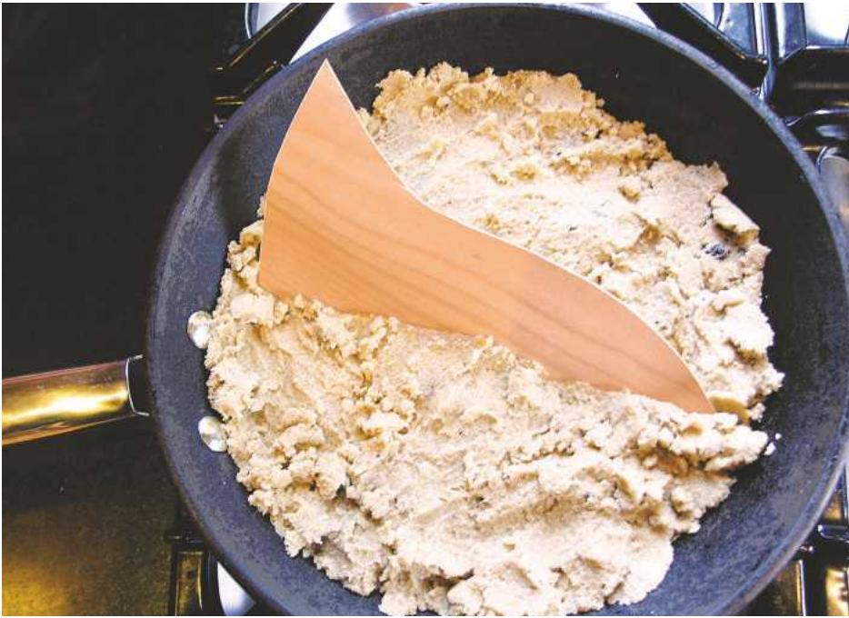
5 The veneers were shaded with hot sand to give definition between each. The sand was heated in a wok and the veneers dipped in with tweezers for a few seconds
