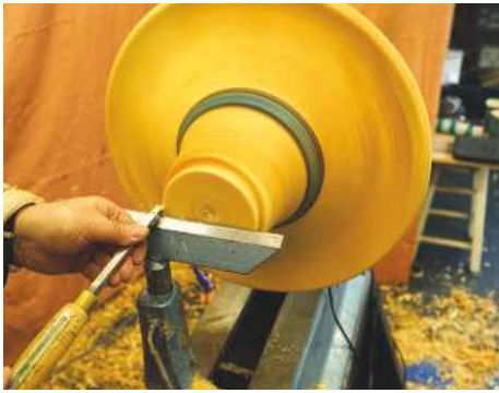
25 Using a 10mm parting tool, I crisp up the tenon using the 100mm Mega Jaws. Next, I reverse the hat until round making sure the brim is running absolutely true
