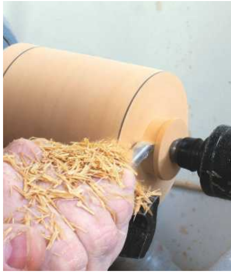
11 Use the 10mm round skew as a parting tool to remove the waste on either end down to about 20mm diameter. Ensure not to go thinner as this can weaken the wood
