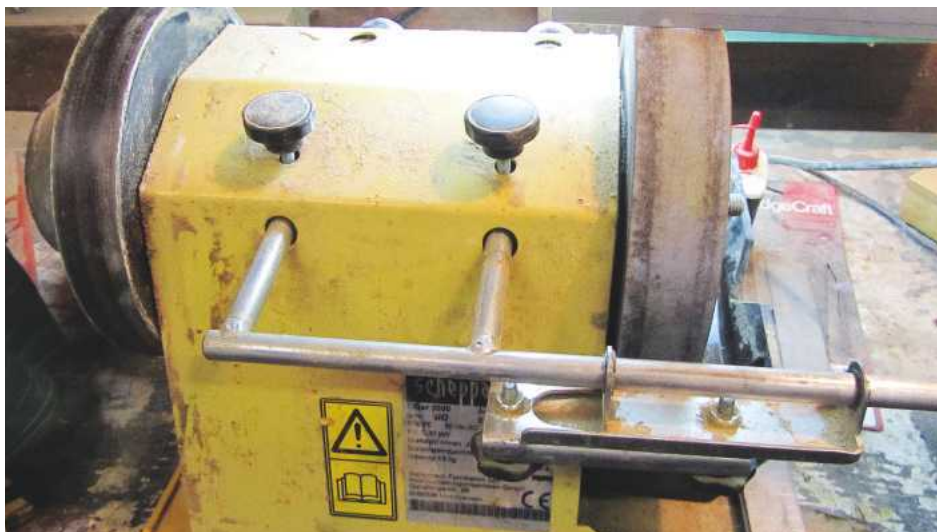
1 Most grindstones – like this ageing Schepach – have a water-cooled stone at one end, and one or more leather wheels at the other
