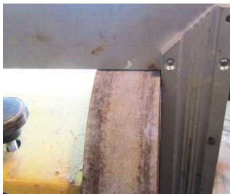
3 A set-square helps to ensure you don't inadvertently create a slope on the wheel
