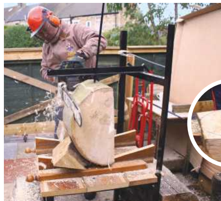
1 The structure of the chainsaw platform is made using 45mm angle iron, 900mm square. It has a table height of 900mm, on which I built a sturdy board with 'V' blocks to secure the timber. The chainsaw chair, as I call it, also uses a piece of 1,500mm angle iron and 3 x 600mm spikes secure the material from above while cutting
