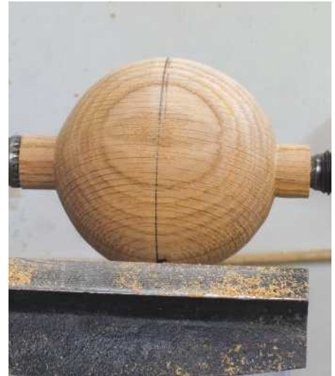
15 The shape at this stage is more of a rugby ball than a sphere. Keep removing the timber as you turn as well as the small waste sections off the end; this will leave a protrusion of about 5mm
