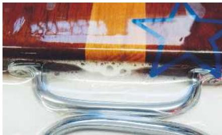
2 The air bubbling out of the end-grain once the vacuum had been formed
