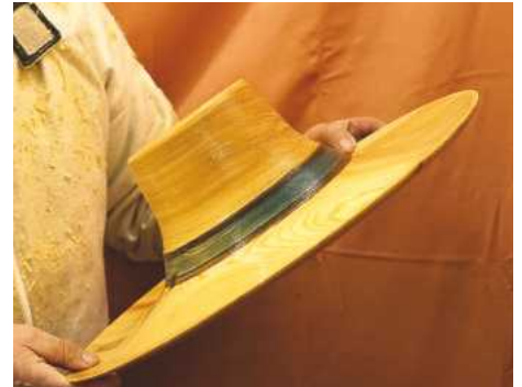
31 Now the turning process for the hat is completed, it's ready to go in the bending jig
