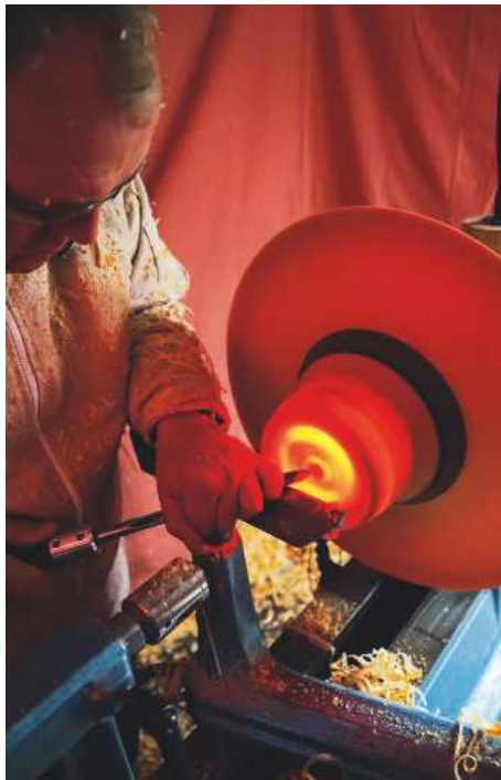
29 I reverse the hat and clean up the surface of the crown. I'm using a light box with a jam chuck mounted on it, into which I've recessed a group of torches. Alternately, use a jam chuck and check the thickness with callipers
