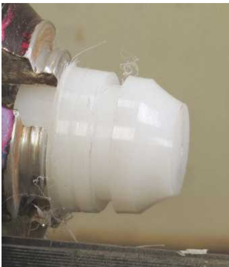
34 I decided to make a couple of small unobtrusive display stands for the balls from PTFE; this is a nylon product used in engineering
