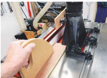
2 Here you can see the router setup being used on some plywood for another project. The board is run between the fence and the router bit from left to right. The featherboards are essential to prevent kickback and my push-stick helps keep it moving with fingers well away from the cutter. My dust extraction method for this is crude but very effective with the hood resting on top of featherboards with some duct tape to stop it moving – it also acts as a cutter guard. The top, bottom, sides and box body were cut slightly longer than needed, on a table saw crosscut jig, to allow for the final trimming of the box joint overhang
