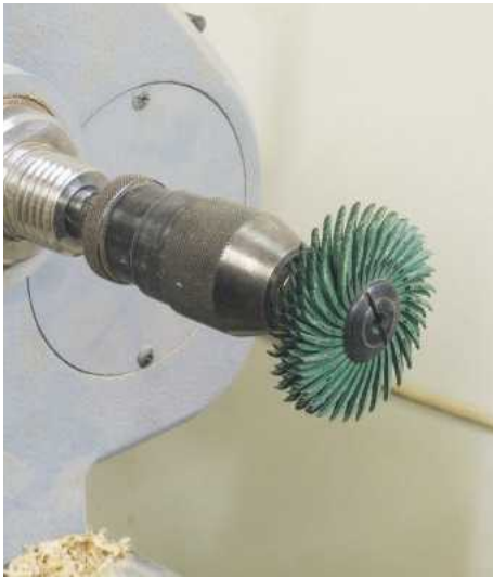
28 I've mounted my sanding brush on the lathe using a Morse taper drill chuck; just tap it into the headstock taper to stop it coming out
