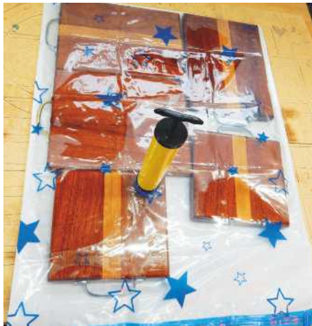
1 Geoff placed six boards – sapele and beech – into a vacuum bag, then added a generous amount of mineral oil before pumping the air out
