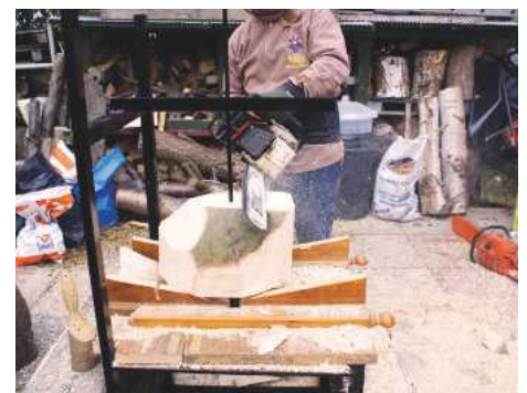
7 Next, I trim the corners at 45°, which takes more weight out of the blank. At this stage, the wet weight will be around 20-23kg
