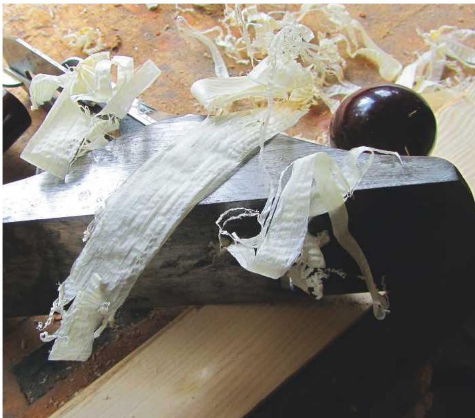
21 Clean, evenly translucent shavings are good evidence that the plane's blade is now square to the sole and scarily – if not terrifyingly – sharp
