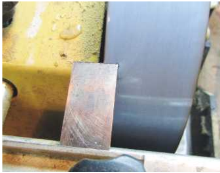
8 Two minutes of firm grinding remove the camber and raise a lumpy wire edge. The water in the stone stops the metal overheating
