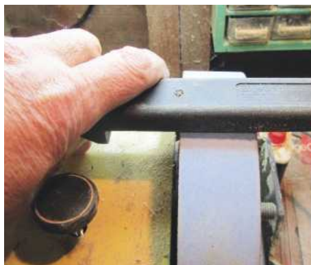
4 Any strong file or diamond-embedded abrasive plate can be used to flatten the wheel by hand
