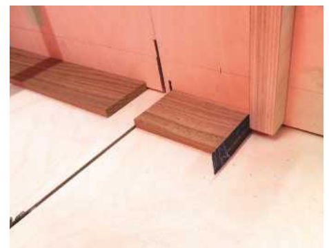
7 The drawer fronts were a fraction too long so were trimmed again using a piece of card against the fence stop, which acts as a spacer. The sides and back of the drawers were also cut slightly oversize and trimmed later for an exact fit
