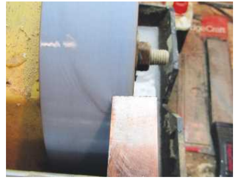
9 As you grind, move the blade back and forth across the wheel and out beyond both sides. This way, you minimise the risk of wearing the wheel unevenly and creating dips that will affect subsequent sharpening
