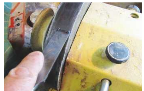
14 You can of course use a tool-holding jig when you hone a blade on a leather wheel, but I find it simpler to hold the bevel on the wheel by hand. The pattern of slurry build-up around the edge will tell you whether the wheel is getting right to the tip of the blade. So will the feel of the tool in your hand, and the sound of the wheel against the metal
