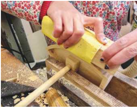
13 I then sanded the hull to make it smooth. I used 80 grit sandpaper and a block of wood
