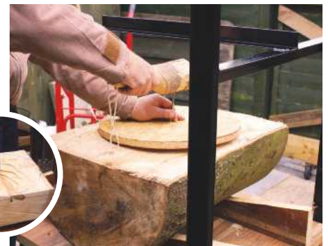
4 I mark the diameter with a compass or template and secure the blank with a central spike
