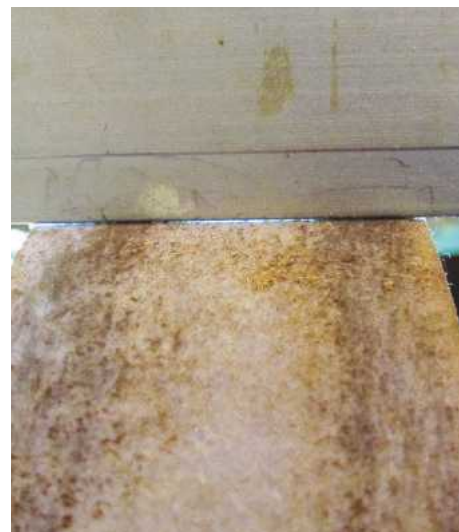
2 A straightedge reveals a hollow in the middle of the grindstone and a slope falling away on the left
