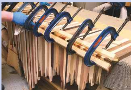
Gluing the top to the apron
