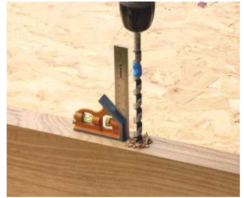
3 Mark the position of each floating shelf bracket on the rear of the oak. Bore 12mm holes with an auger bit, using a small square for accuracy
