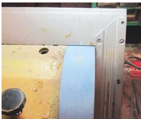
5 Cleaned, flattened, dressed and checked for square, the grindstone is ready to go back to work
