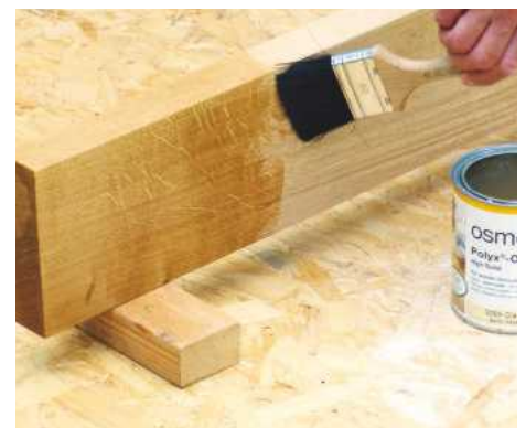
12 Vacuum to remove dust, then apply a suitable clear finish such as oil or polyurethane. I brushed on two coats of Osmo semi-matt Polyx Oil
