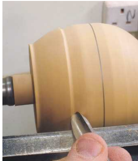
14 Do the same on the left-hand side, but be mindful not to remove too much timber at this stage. The line must stay on the work as this maintains the correct diameter
