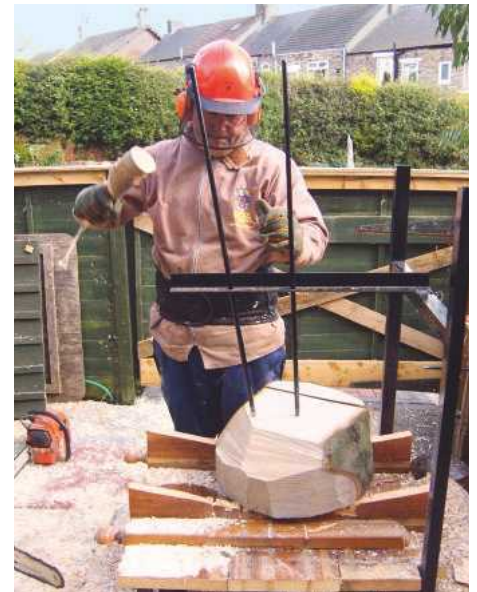
2 In preparation for turning a hat, I start with a piece of wood as a side-grain bowl blank, measuring a minimum of 400mm diameter x 200mm deep
