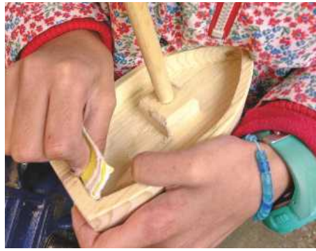
14 To finish, I did more sanding inside and out with finer sandpaper, which took a long time
