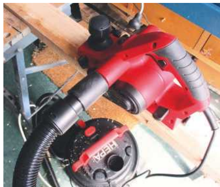
A flexible dust spout adaptor provides dust control on a planer...
