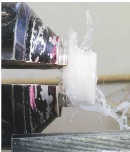
35 As you can see here, do be careful when turning this material as the shavings tend to get wrapped up all over the place and could potentially cause injury
