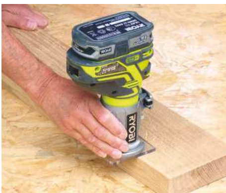
10 Routing a small, decorative chamfer along the front edges and ends adds the finishing touch. Check the depth setting first on scrap timber
