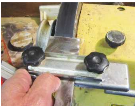
20 Once the plane was ready for polishing on the leather wheel, I was ready to finish it off by hand – you'll notice the jig is no longer riding on its bars
