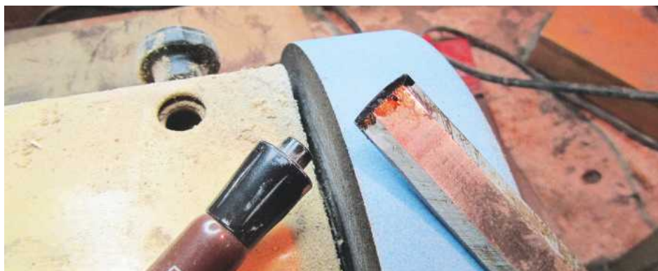
6 Woodturner Mick Hanbury recommends rubbing ink over a bevel before grinding. When you later inspect the blade, the ink marks give you an instant guide as to whether you're grinding evenly
