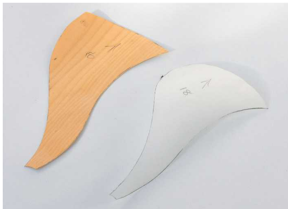
4 It's a simple task of carefully cutting around the template until you have an exact replica, though the varied grain of the veneer is obviously a challenge
