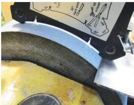
19 Plane blades demand a little more precision. Hence, here, a more determined attempt to repeat its 25° angle and set it firmly in a blade-holding jig
