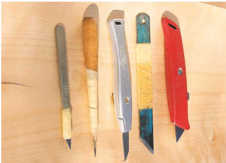
3 For cutting the veneers, I used several different knives. My favourite is one I make myself from old hacksaw blades (second from the right); these are less flexible than scalpel blades
