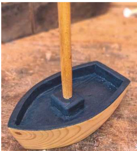
20 When the oil had dried, we finished by rubbing in wax polish to protect the surface
