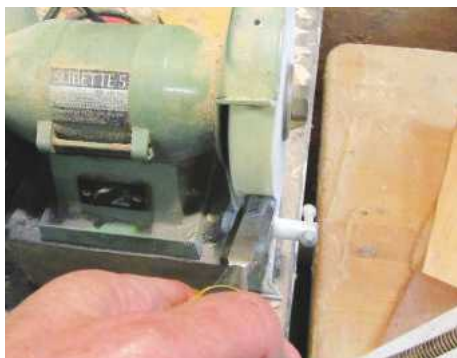
15 A felt wheel offers a quick method of polishing up the face or back of a blade, but remember to hold it tip-down against a wheel, which is spinning towards you, and remove it frequently so that the blade doesn't overheat and lose its 'temper' (hardness)
