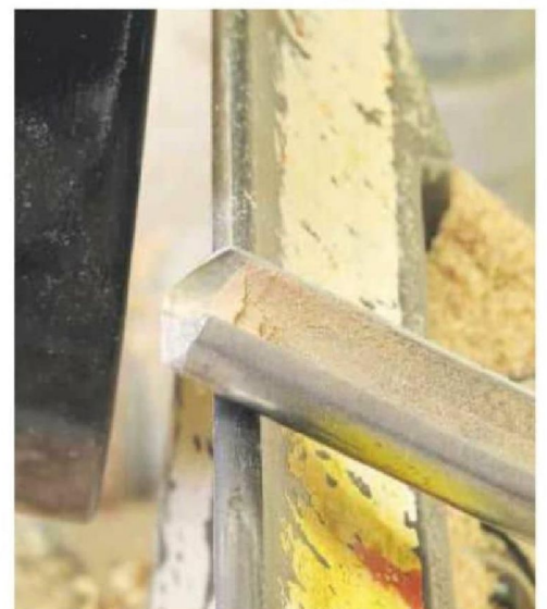
27 ... but here's the answer: this 10mm bowl gouge has an angle of about 60° and is very easy to use so long as you present the tool horizontally
