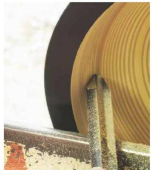
24 I opted for about 12mm for the rim; a light cut with the freshly sharpened tool gives me a good, clean surface ready for sanding
