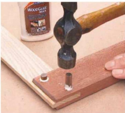
16 Next, cut two lengths of dowelling over size. Apply glue and insert both pieces through the stock
