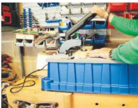
The Foreman is very easy to use: simply pull the trigger and plunge the handle
