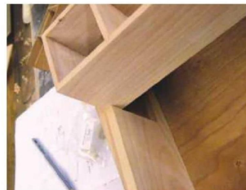
21 The slope supports extend under the rear compartment
