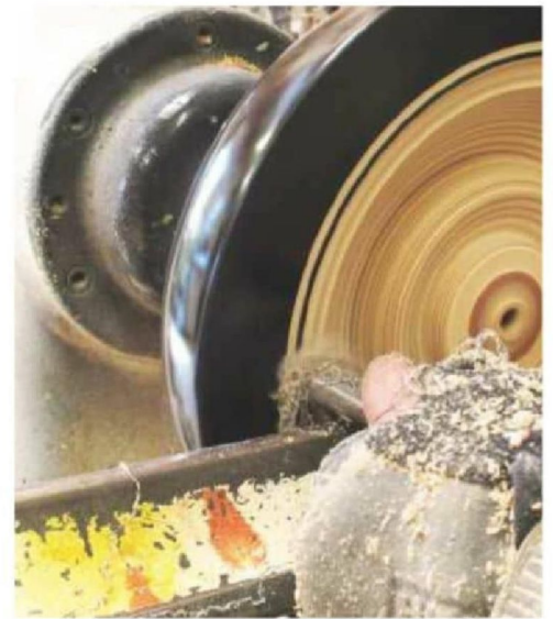
21 The black edge on the top will tend to make the bowl look thicker than it actually is, so I'm going to take the thickness down a little more than usual
