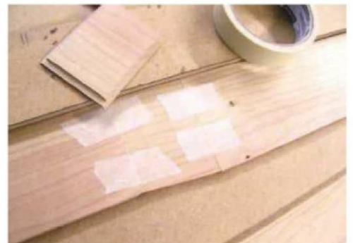
17 Stretch masking tape across the pieces
