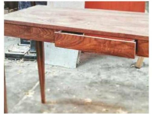
12 Testing the size of the drawers before gluing up...
