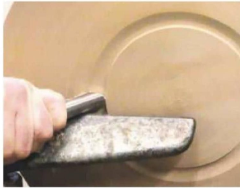
5 Cut a foot using the tip of the bowl gouge...
