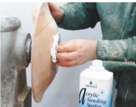
12 ... then apply acrylic sanding sealer
