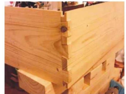
3 Here you can see the gap where the rebated grooves meet; this will need filling in the next step
