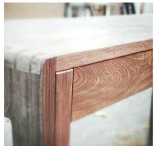
15 Aligning the drawer fronts with the frame prior to sanding
