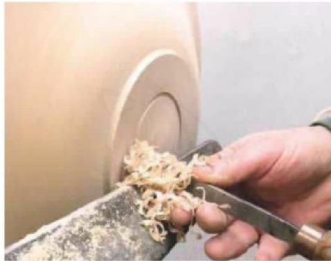
8 Cut the recess for the chuck using a parting tool
