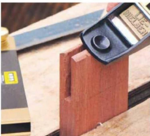
13 Mark both ends of the stock with a sliding bevel, then create decorative chamfers using a block plane
