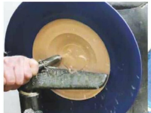
22 Hollow the platter in the usual way using a bowl gouge
