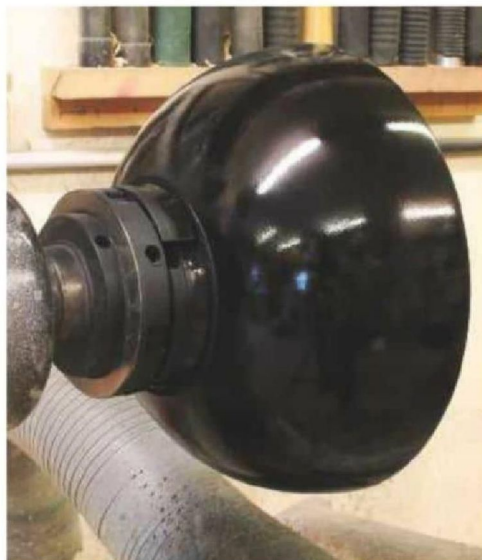
17 Super gloss! After a dodgy start and about 10 coats of black followed by a few coats of acrylic gloss lacquer, I've achieved a wet-look gloss finish
