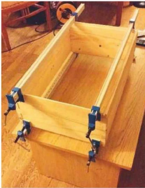
7 Everything glued up and clamped together
