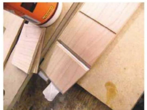
18 Apply a little bead of adhesive into the joints
