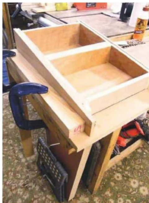
9 Everything must be clamped securely on a flat surface
