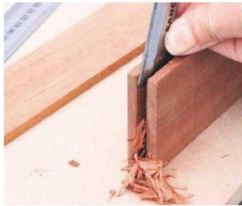
8 Chop back the bottom of the mortise with a 6mm chisel. Pare down the sides carefully with a wider blade
