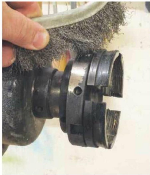
32 Because of the amount of black I sprayed on the bowl, I've ended up with a paint-covered chuck; this must be wire-brushed back until you can see the chrome again
