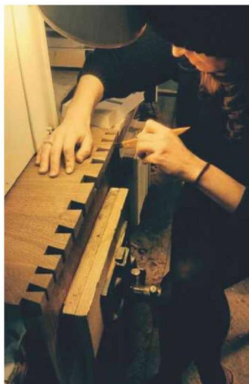
1 Marking out the pins
