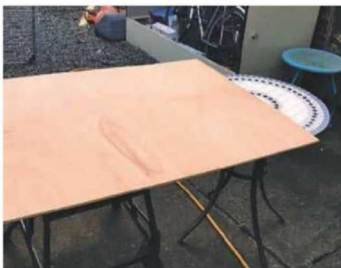
10 Half a sheet of plywood was used for skinning the frame
