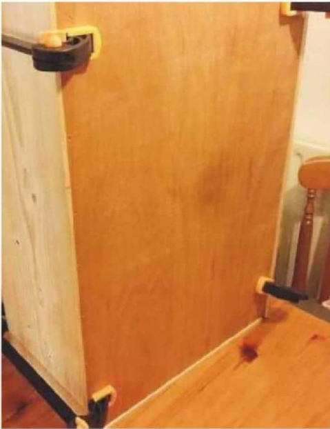
13 Here you can see the corner gap, which needed to be filled in, the plywood lip to be planed down, and the pin holes, which were still to be filled
