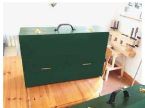
26 The completed fall front tool box, painted using Rustoleum All Surface racing green
