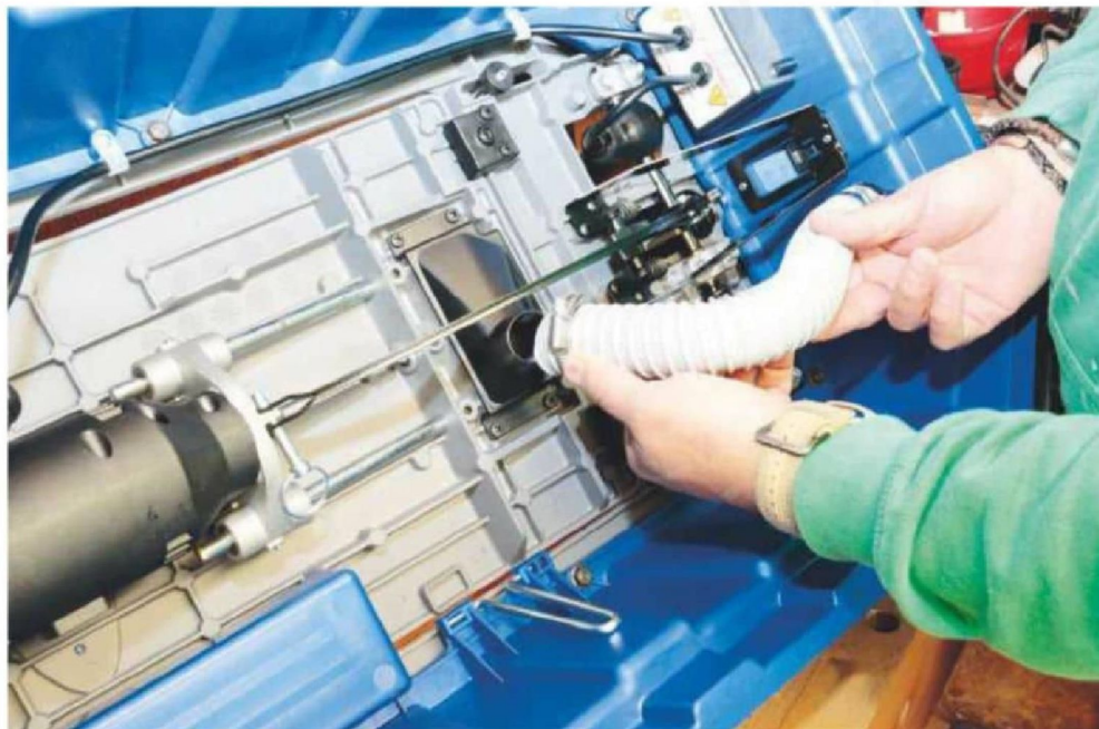
You have to connect the supplied link hose if you want to use an extractor
