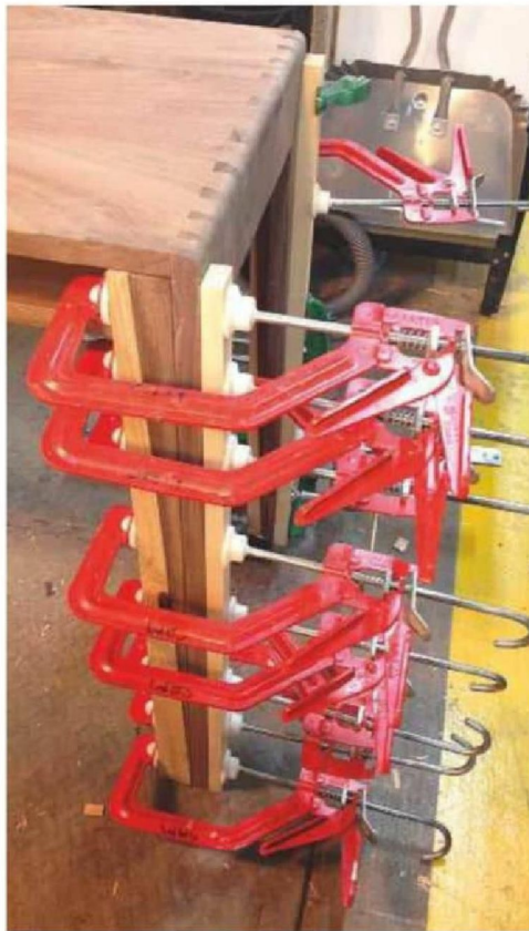
11 Gluing on the sloping panels to complete the legs (with a multitude of clamps!)
