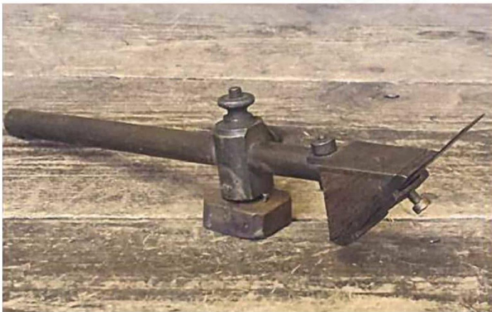
An extremely rare antique chamfer edge radial veneer cutting tool – an engineering marvel that would have been perfect for cutting circles in veneer with a chamfered 45° edge Photograph courtesy of www.tooltique.co.uk
