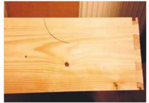
9 The curved lid edge is cut with a coping saw, matched on both sides, and the dovetails are spaced to allow the lid to be cut free
