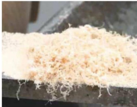
10 You should aim to get very fine shavings from the scraper
