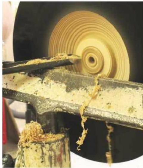
20 Removing stock from the centre will require repositioning of the tool so the bevel is in contact with the bowl; as the wood is revolving slower, smaller cuts are required
