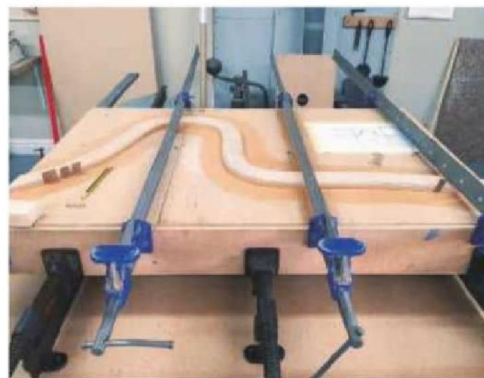
The combined leg and backrest setting in a press jig
