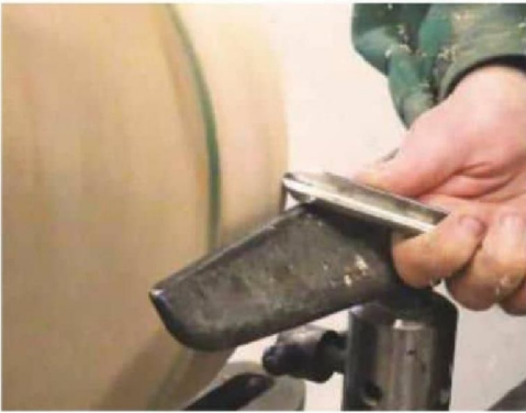
4 True up the edge with a push cut
