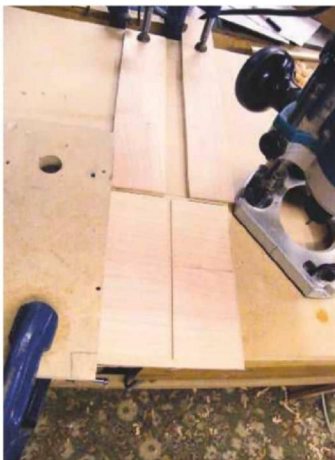
16 The lower edges are butted together
