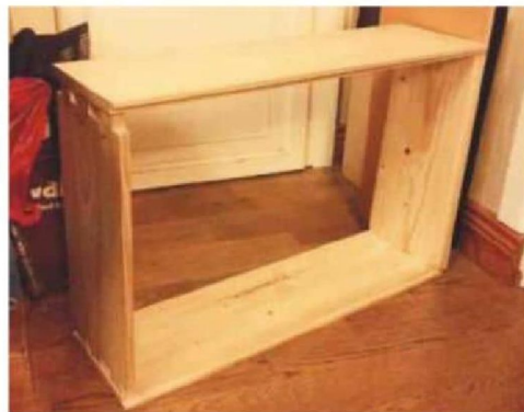
2 A quick test fit with dovetails – with one end cut and no pins
