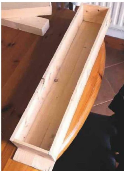
25 Well attached but the base is protruding
