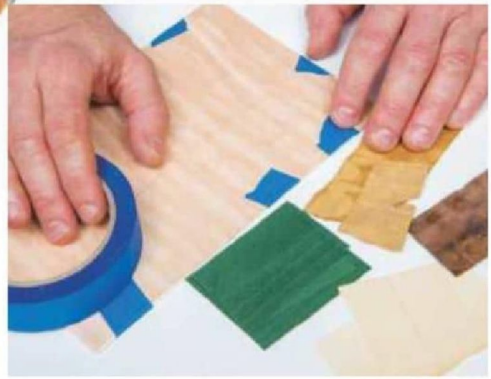
1 Once you've made a line drawing of your intended marquetry image and glued it down, tape the background veneer onto another piece of cardstock
