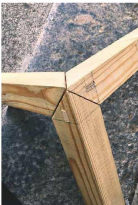
A three-way mitre joint
