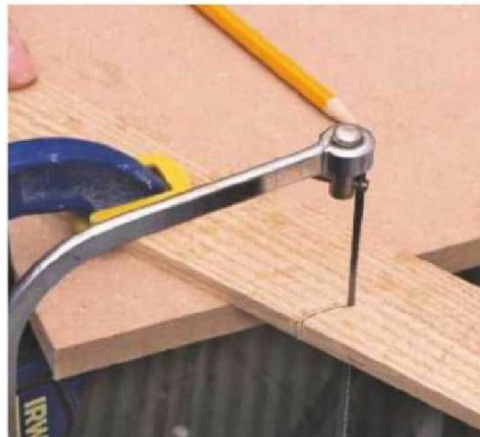
11 Cramp the blade firmly, then cut out the curve with a coping saw, keeping on the waste side of the line
