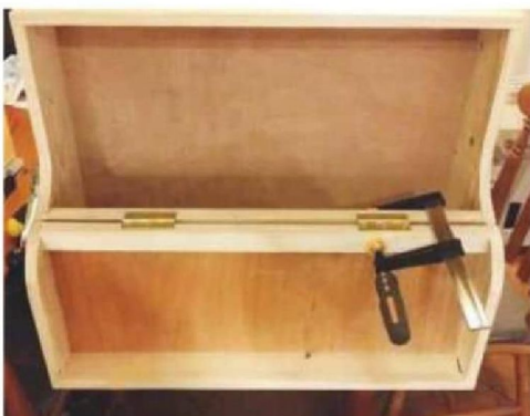
18 The hinges once installed
