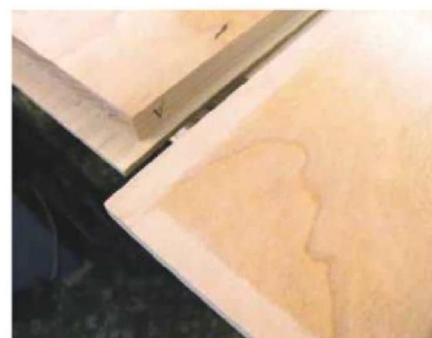
3 It's much easier to polish the inside of the box prior to assembly
