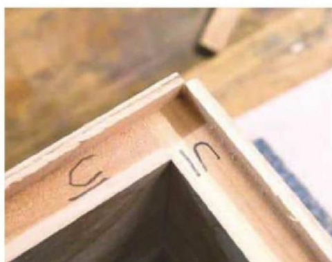
2 Note the lettering to keep each piece in its correct place
