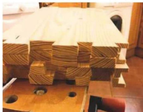
5 ... oops! Here you can see where the dovetails went wrong
