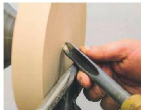
3 ... making light cuts with the bottom wing
