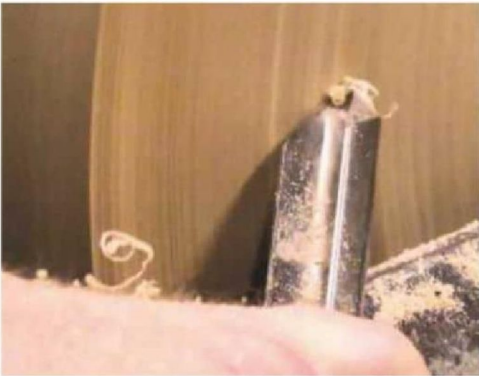
7 Rolling the tool up until the bevel rubs will give a cleaner cut
