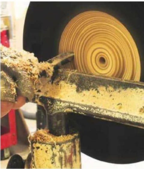
19 The removal of wood on the inside starts with me making simple sweeping cuts with the flute of the tool pointing towards 2 o'clock
