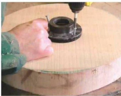
1 Fix a faceplate to the middle of the blank
