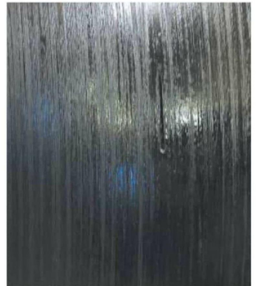
15 The first coat of spray has penetrated at a different rate
