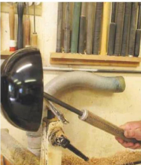
22 As you go deeper inside the bowl, the handle of the gouge will need to be dropped to position the gouge's bevel onto the surface that is to be cut
