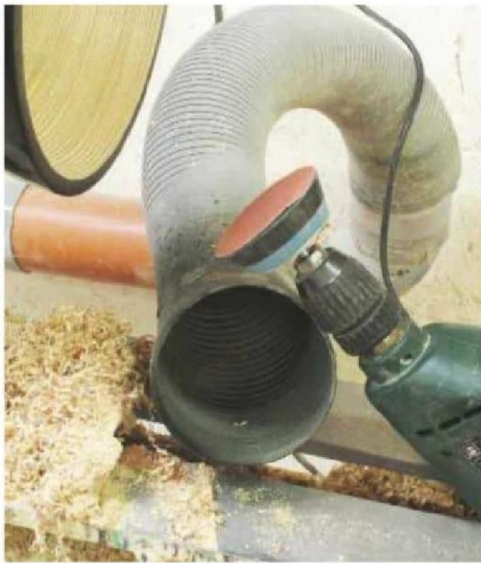
28 The big guns are out in the shape of the 75mm Simon Hope sanding pad with 80 grit; the corded drill works quicker than my cordless so that should remove even more wood
