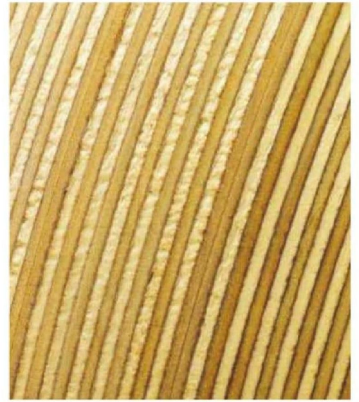
12 This photo shows the difference between a heavy stock removal cut and the lighter shear cut; the tool will blunt quickly when working on composite materials
