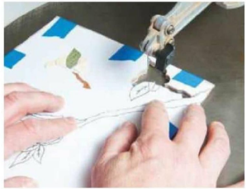
3 Using a scrollsaw fitted with a 2/0 blade on a low setting, start with the outside pieces and cut each part, one at a time
