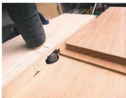
1 A scrap wood fence with a suitable dust extractor port works well
