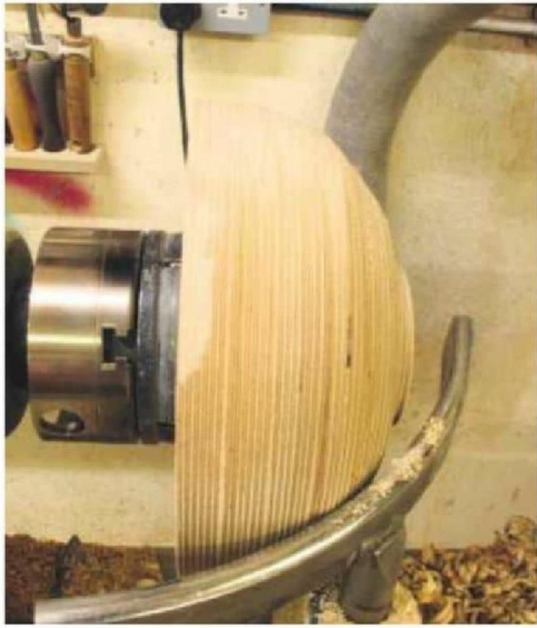
10 I want a simple curve on the outside; this stainless steel curved toolrest works as a guide for the bowl; just keep removing wood until it conforms to the shape
