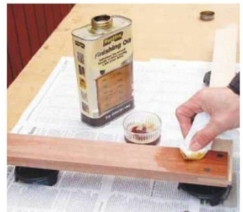
18 After sanding with 180 grit abrasive, wipe on a couple of coats of finishing oil, such as Rustins
