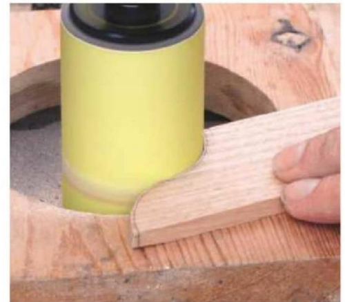
12 Clean up the curved end with a sanding drum mounted in a drill stand. Alternatively, use a rasp or file for shaping
