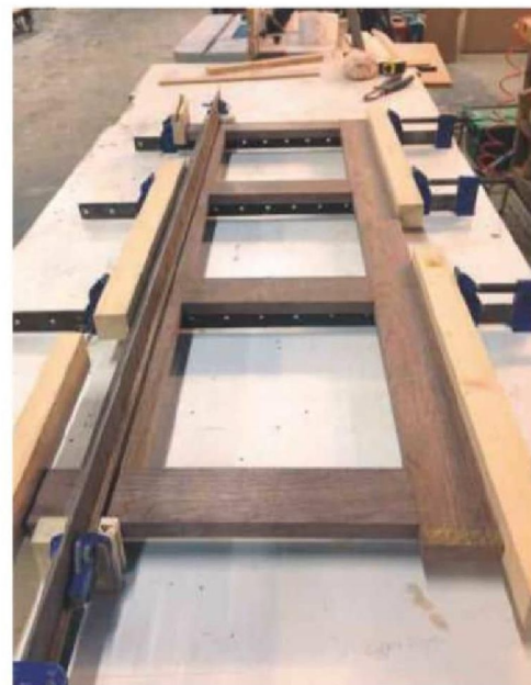
5 Gluing up the drawer frame
