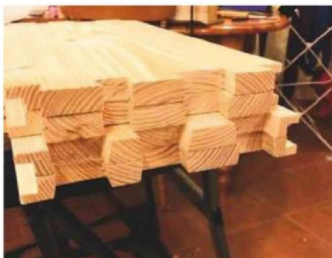
4 On the left-hand side you can see the rebate. All looks OK this end...
