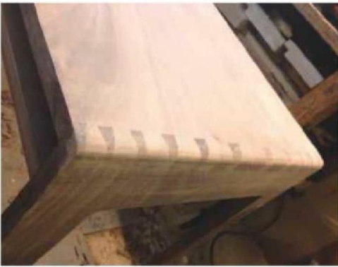
10 The desk top dovetails after planing to round off the edges
