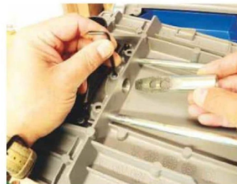
With the table removed the sleeve can be swapped for different drill sizes
