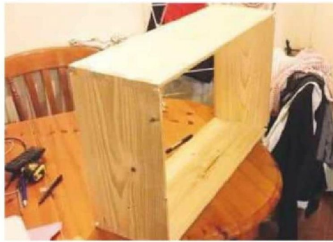
8 Here the dovetails have been trimmed flush
