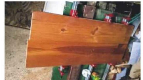
1 Clean up, plane and glue boards
