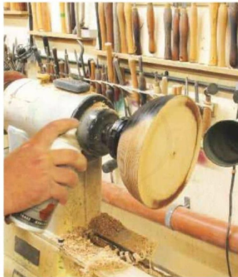
14 Sanding the outside will show me whether I need to do anything else to the surface prior to spraying
