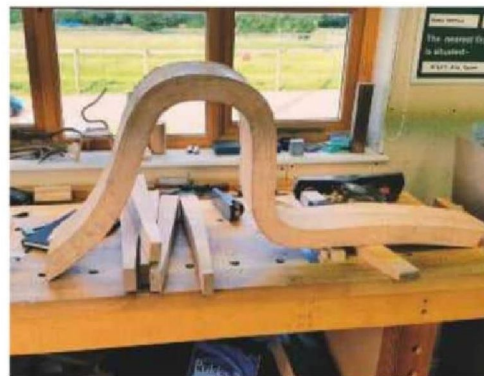
A completed leg section, prior to carving
