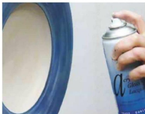
24 Apply several coats of acrylic lacquer to finish
