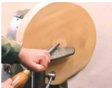
2 Use a swept-back bowl gouge to flatten the bottom...
