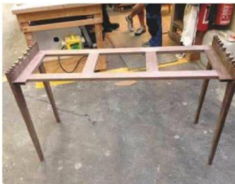
6 Slotting the frame for the drawers into place
