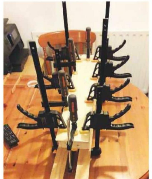
24 Gluing on and clamping the base
