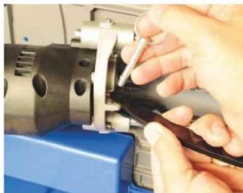
Removing this pin allows the motor to drop out, so you can remove the table
