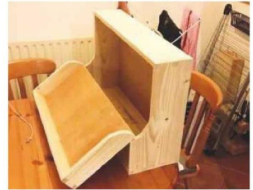
15 The box is cut to release the lid
