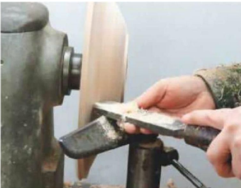
9 Refine the shape and clean up the surface using a round-nosed scraper
