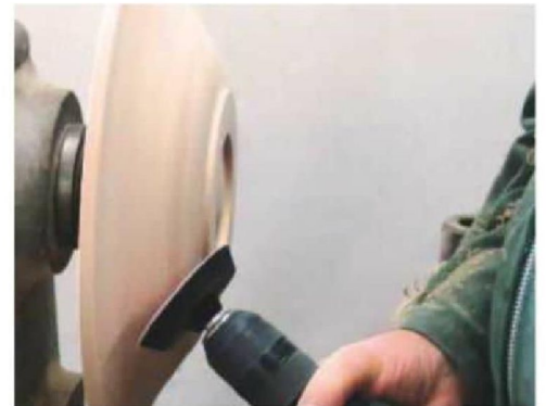
11 Power sand the outside down to 600 grit...
