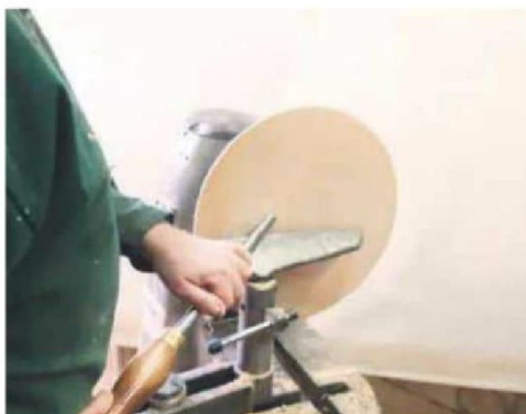
13 Turn the platter around and flatten the top side
