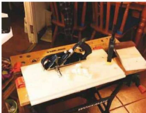
1 Showing the rebate required to accept the plywood skin
