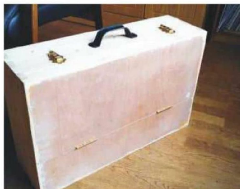
19 With all the hardware in place, the toolbox is now ready to paint
