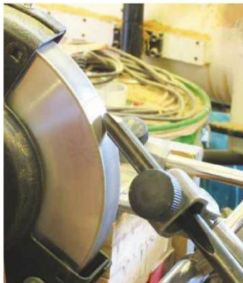
23 Even the Thompson gouge will need to be sharpened regularly; a jig gives consistent results and tends to remove less precious steel
