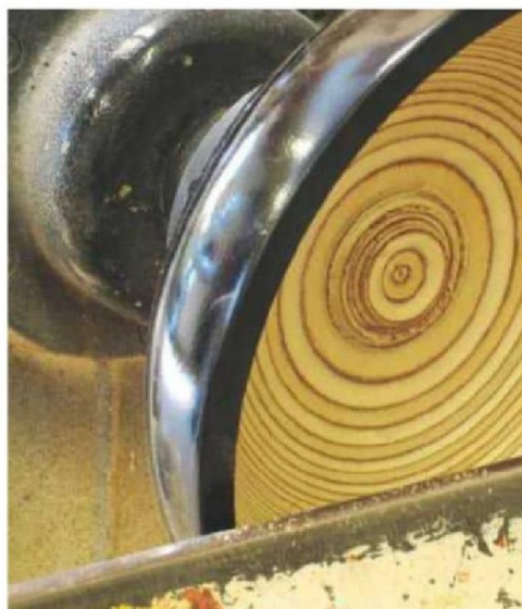
26 The only bit left to do now is the dreaded lump in the middle; this is always difficult to cut well with a standard bowl gouge sharpened to a 45° angle...
