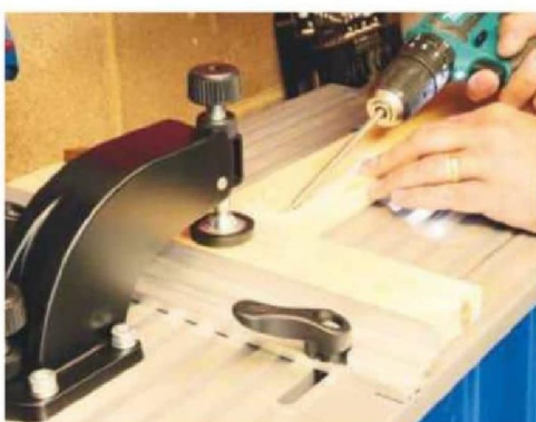
Once cut, the joints are screwed together in the normal manner
