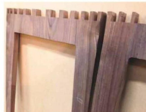
3 The completed leg pins ready for gluing up
