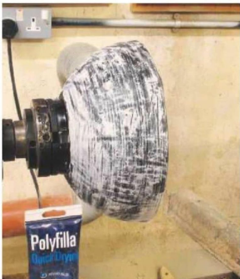
16 Thank goodness for Polyfilla! Apply it sparingly all over and then sand it back with the lathe off
