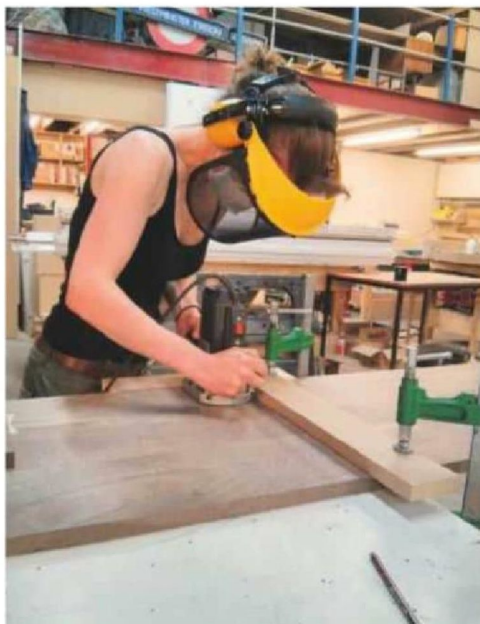
4 Routing the sliding dovetails for the drawer frame
