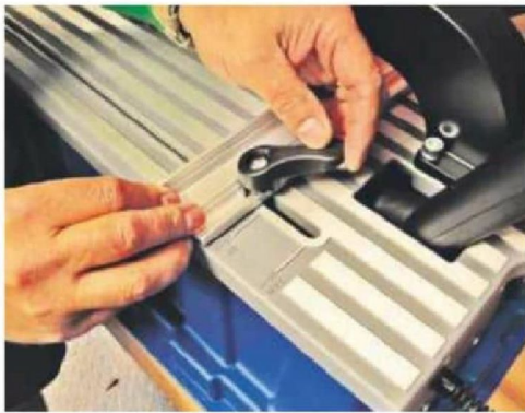
Common timber dimensions are marked to help set the fence
