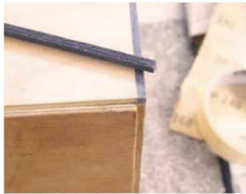
5 The beading should fit flush with the veneers
