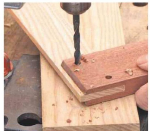
15 Mark out centres for 10mm diameter dowelling. Test for fit in scrap, then drill right through the stock
