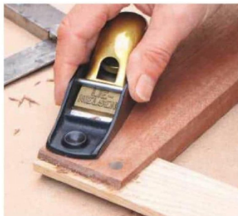
17 After the glue has dried, saw off excess from the dowels on both sides. Trim flush with a block plane
