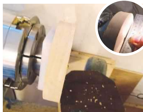
2 To turn the base, I needed to pack out my screw chuck, so therefore drilled an 8mm hole in a piece of plastic a little under 10mm thick, then threaded it onto the screw chuck. I put the same size hole in the centre of the base blank and mounted it on the lathe. Using the spindle roughing and spindle gouges, I turned the wood into the round and then covered out the face using the edge of a steel rule, which helped to ensure that there was a curve in the base. This allows the carousel stand to sit level on a flat surface
