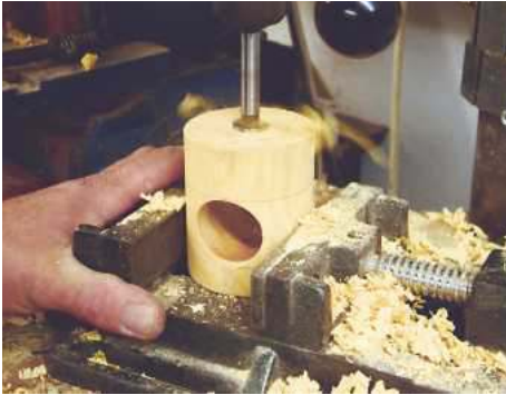
4 Find the centre of the body and drill a 7/16in hole for the thread...
