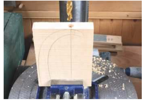
12 Support arm blank marked out and drilled for bushing
