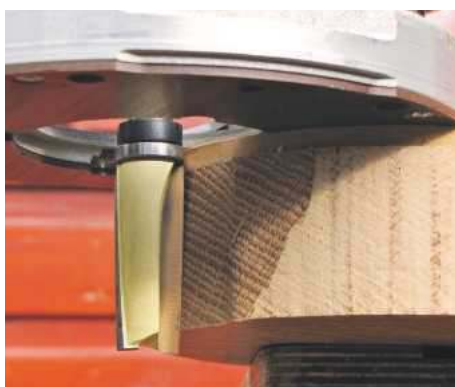
8 Secure the timber to a bench. Using a router, carefully follow the template using a bearing-guided flush-trim cutter
