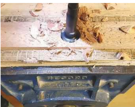
4a A piece of 2x1 in timber mounted in a bench vice, being drilled using a Forstner bit
