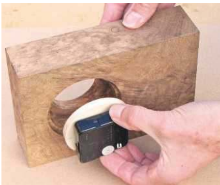
16 Cut an 8mm sycamore dial with a Dremel tool or flush-trim bit and template; check the movement fits in the recess
