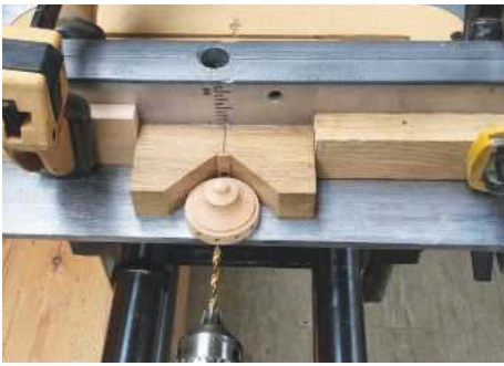
19 Set-up for drilling the connector peg holes
