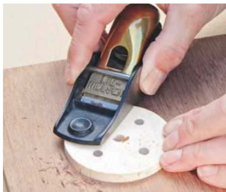
20 Allow glue to dry and trim away any excess with a block plane; sand dial to 320 grit and seal with lacquer or oil
