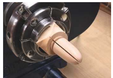
27 A split turning completed and ready for separating
