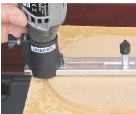
4 Cut out the template curve with a Dremel tool or router and trammel arm; alternatively, use a jigsaw and clean up
