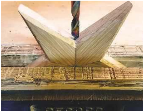
10a Drilling a hole into the bottom of the star, which will be held up by the 9mm metal rod
