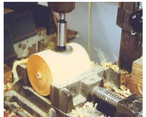
3 Drill a 38mm hole in the blank, holding it in a machine vice
