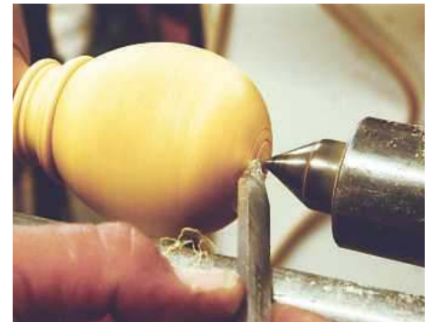
9 You can add a couple of decorative lines with the parting tool
