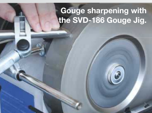
You can sharpen on the periphery...
