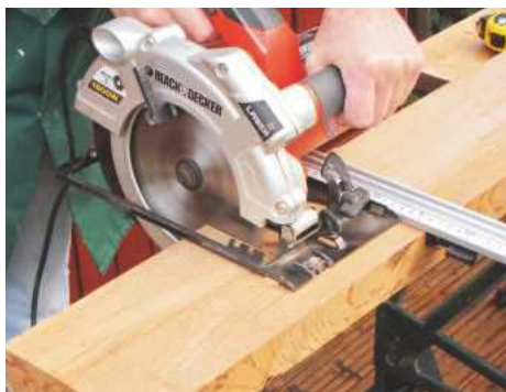
1 Thickness the timber to around 50mm, then saw to length; overall size of the clock blank is not too important here
