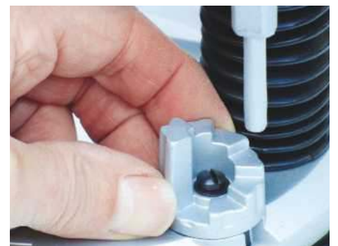
Built into the base is a rotating depth turret, which can be set at eight positions, though there's no fine adjuster screw built in
