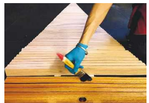
5 Staining each of the 2x1 in 'branches' using clear Danish oil, although you can use whichever finish you choose
