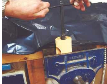
5 ... and cut the grooves for the thread by turning the tap while holding it in a vice
