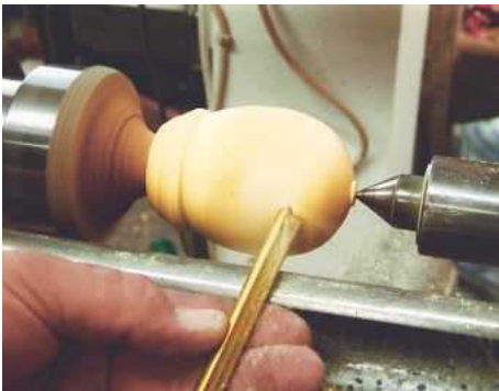
7 Gentle touch: with the lathe running at around 2,000rpm, carefully turn the body
