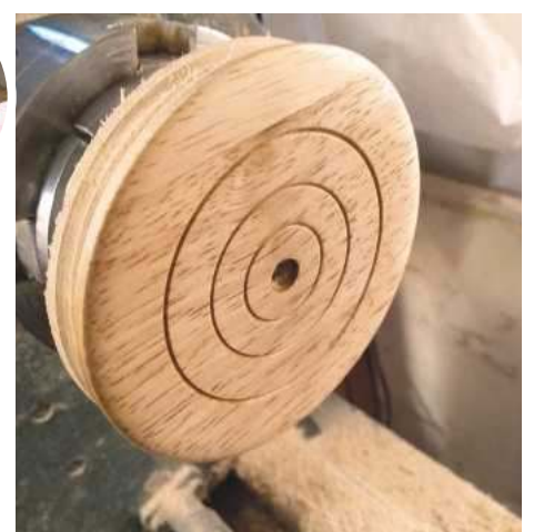
3 To finish the bottom of the base, I coated it with the beeswax and liquid paraffin mix, wiping off the excess, then sanded through the grits from 120 to 400. Next, I added a few rings with the tip of a skew chisel in case another woodturner picks the piece up to look underneath
