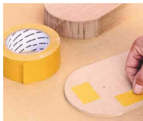
6 The template needs to be made accurately for routing; stick this to your clock blank with double-sided tape
