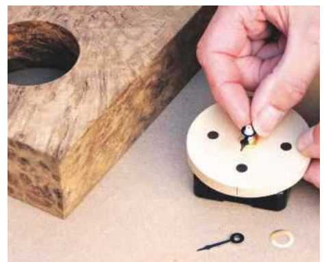
21 Mount the quartz movement on the back of the dial and carefully fit metal hour and minute hands (length is 24mm)
