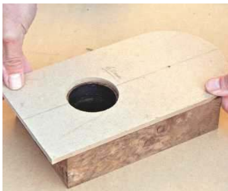
10 Rout a hole in the template with a Dremel tool to suit the clock dial; on both these clocks this is 60mm diameter
