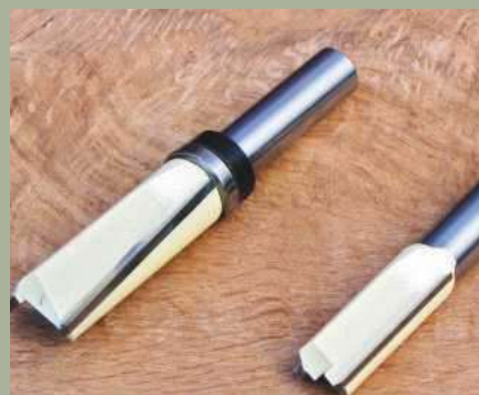
I removed waste with an Axcaliber 16mm twin-flute bit
