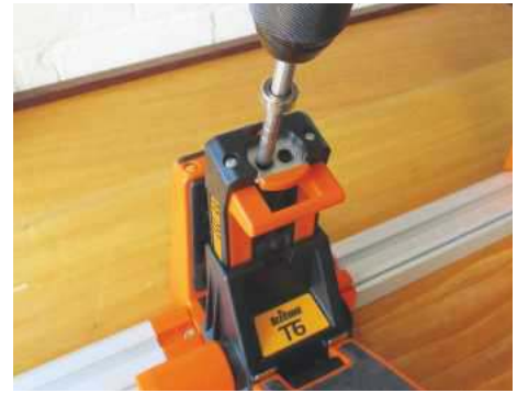
Even with a power drill attached it stays in place
