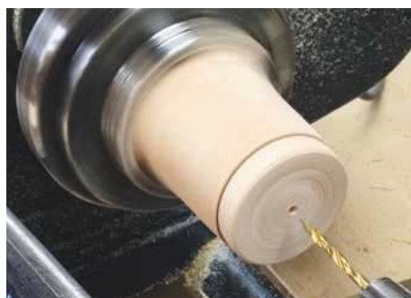
17 Cleaning up the bottom of the hub and drilling for the driveshaft connection
