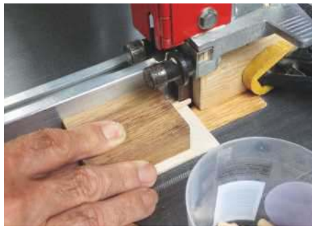
20 Jig used for slotting the connector pegs. The two pieces comprising the jig are glued together. A 6mm diameter x 5mm deep hole at the bottom of the top piece holds the dowel steady and a stop controls the length of cut
