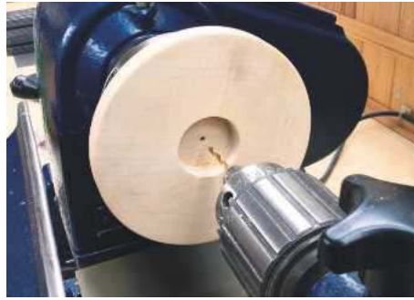
11 Recess created for glass bearing and drilling driveshaft access hole
