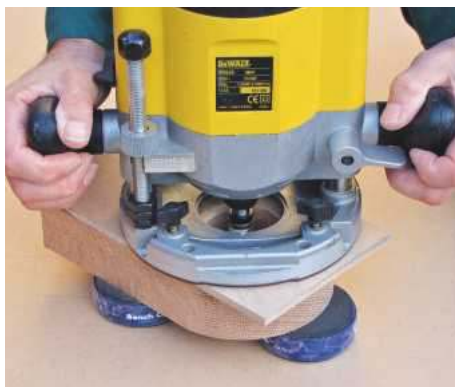
11 Position the template carefully on the front of the blank; rout around the inside at full depth using a flush-trim cutter
