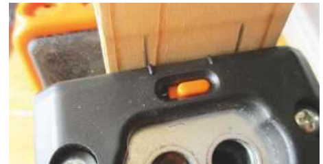
Drill guides on top of the jig
