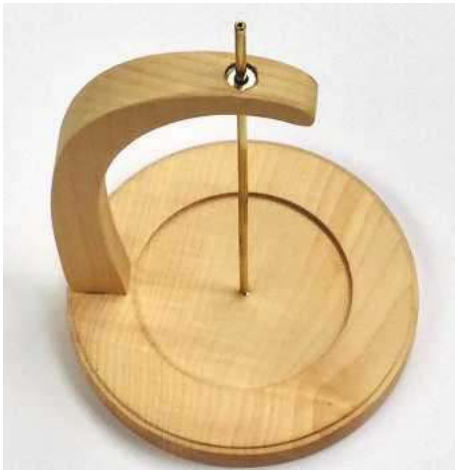
13 Support arm, bushing and driveshaft checked for alignment
