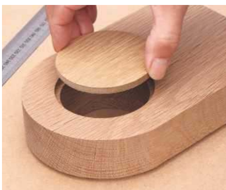
22 Cut rear cover plate from veneered MDF or hardwood; this is fitted with two countersunk brass screws
