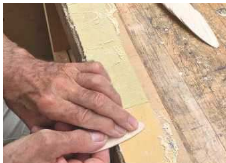
23 Sanding board used for trimming the sails
