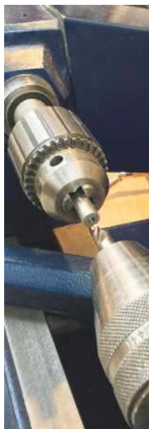
5 Using a centre drill countersink bit to make the steel bearing and bushing
