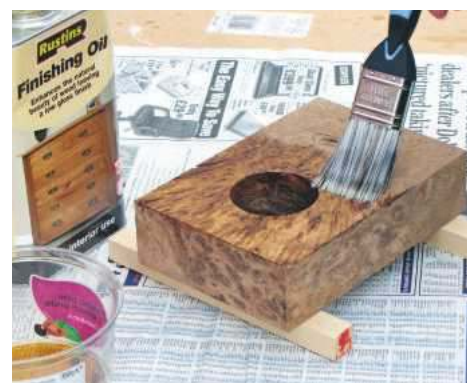
24 Brush on two coats of finishing oil, followed by a clear wax. Insert the dial, securing in place with a dab of glue
