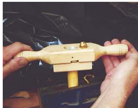
11 Groovy: hold the handle in the vice while cutting the thread
