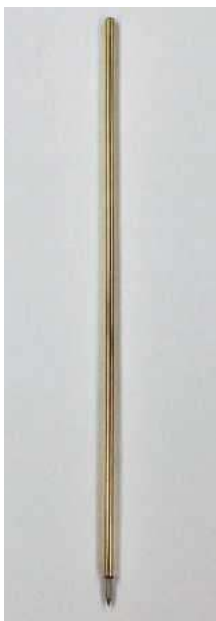
4 1.5mm inside diameter brass tubing fitted with 1.5mm steel wire ground to a needle point makes up the driveshaft
