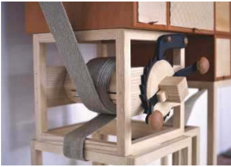
The cleverly designed tightening device literally pulls everything together
