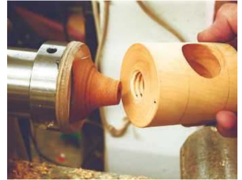
6 Mount the body on a jam chuck and bring the tailstock up for support
