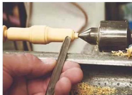
14 Mirror image: round over the cross-piece, ensuring both sides are identical
