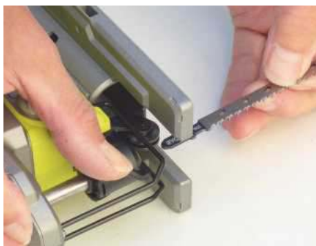
You push the spring-loaded holder forward, insert the blade end and release
