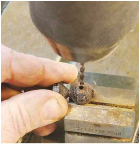
19 Just before gluing it all together, drill a cross hole in the ball cap – an engineer's 'V' block combined with the drill press is perfect for achieving an accurate hole. When using wenge, take the drilling slowly as it's prone to splintering
