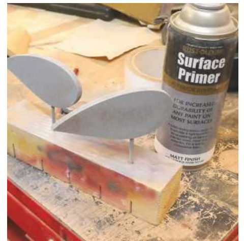
27 I worked out where the wings would attach to the body and drilled a hole to accept a small length of cane; this allowed me to hold them while I applied the gold spray paint
