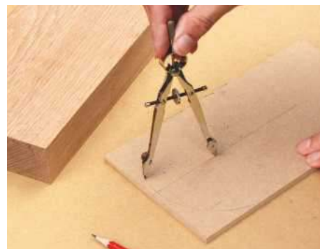
3 For a curved-top clock it's easiest to make a template from 6mm MDF; draw a 70mm radius with a compass
