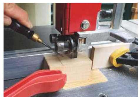
26 Cutting the slots for split turning the figures
