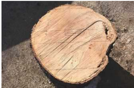
Cup (ring) shakes in a large bowl blank
