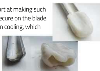
Blade guards for woodturning chisels, made using Polymorph
