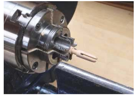
21 A connector peg finished and ready for parting off
