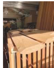
Oak door linings planed down to angles on both sides using the cradle
