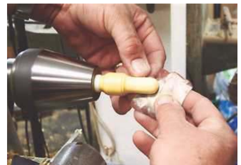
15 Wrap the handle in masking tape and put it in the chuck to sand
