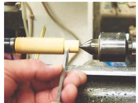
12 Mount the handle back onto the lathe and turn a spigot for the cross-piece, which...
