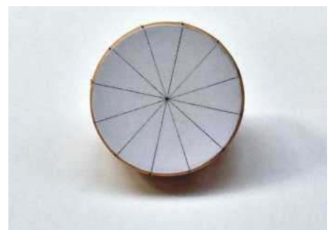
18 A cardboard template is used to locate the connector holes
