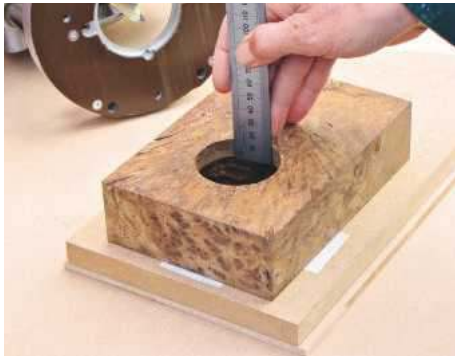
13 Check that the depth of the front hole is enough for the clock spindle and hands; quartz movements are available in three sizes
