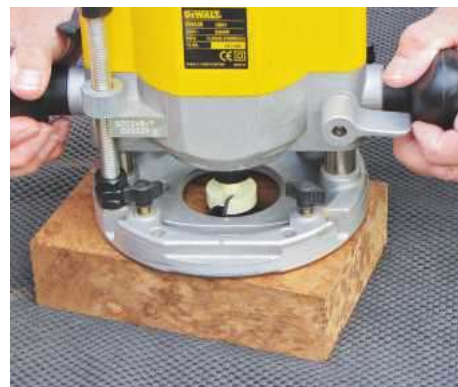
12 Now use the template with a 75mm-diameter hole to rout from the back; finish with a rebate cutter for the rear plate
