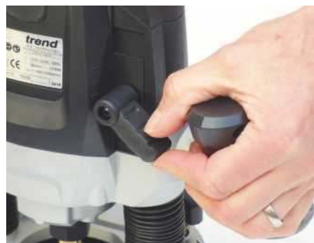
The sturdy locking lever at the front is not spring-loaded, but it's easy to reach and operate with your left hand
