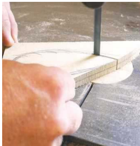
26 The wings can then be cut from some scrap 6mm MDF. I stuck them together with double-sided tape, which allowed me to sand them smooth on a disc sander. Once done, you should be left with two identical shapes
