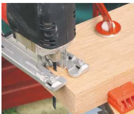
5 Draw around the template onto the blank; cut with a jigsaw or bandsaw, keeping to within 3mm of the pencil line
