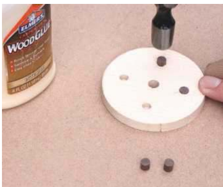
19 Carefully mark 3, 6, 9 and 12 positions on the dial; drill to half depth with a 6.5mm bit and glue dots in place
