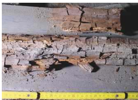
Wood decay caused by Serpula lacrymans (called true dry rot, which is a type of brown rot)
