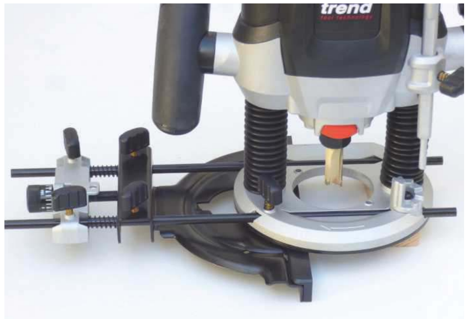
Unlike those on the T10/11 routers, the T7's fence is made mostly from steel
