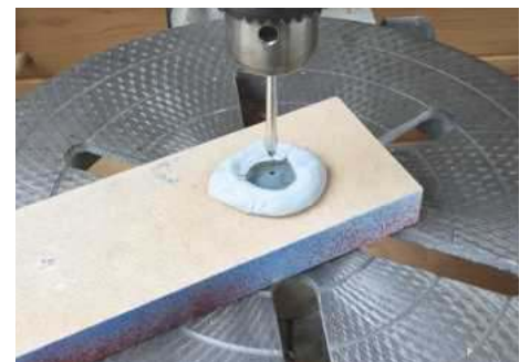
7 Drilling the glass half bead
