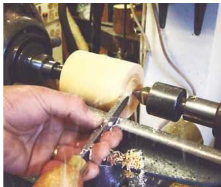
2 Mount the block between centres on the lathe and true up both ends
