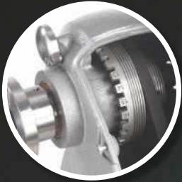
Heavy-duty spindle lock and 24 point indexing
