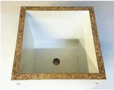
1 The chipboard box with a hole drilled into the centre
