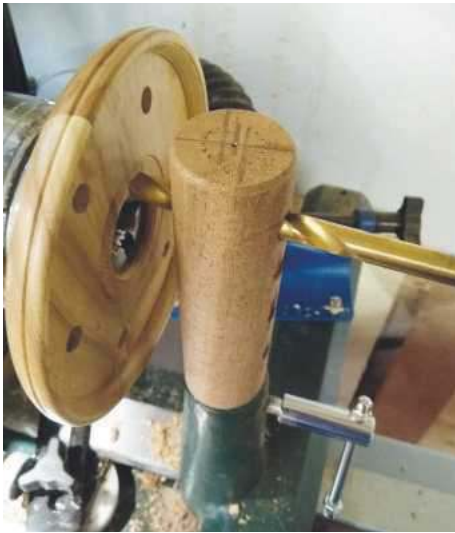
25 Before finishing with the jig, I lowered it so that the drill tip was closer to the centre of the platter. I then used a little hand pressure to mark the platter at four points, which would take the screw eyes for hanging the platter later
