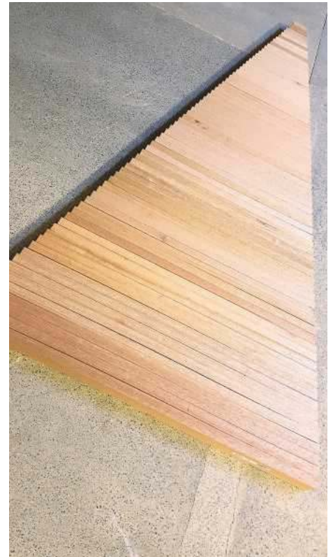
3b All the lengths cut and laid out to show the Christmas tree shape
