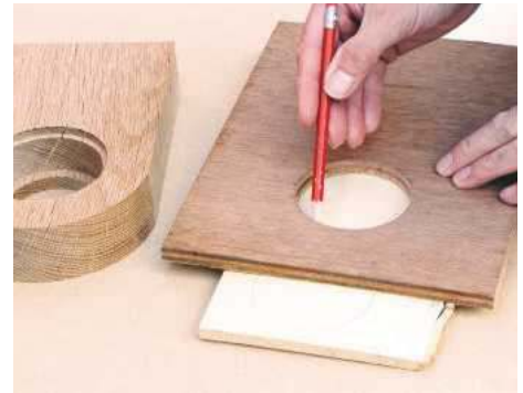
15 Make another template with a cutout to match the dial diameter (here 75mm). You can then draw on to the contrasting wood
