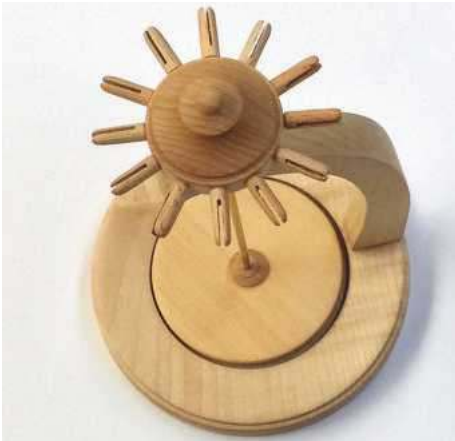
22 Test fitting the 12 connector pegs
