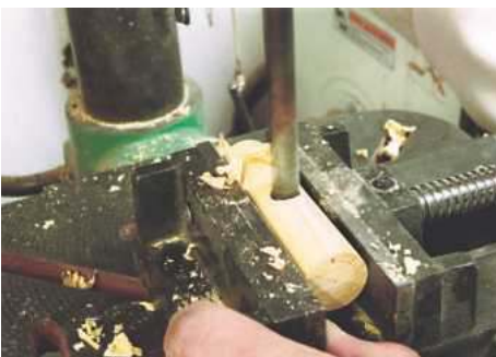
13 ... is held in a machine vice and drilled to receive the spigot
