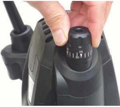
Fortunately, the T7 incorporates a fine adjuster for tweaking cutter depth precisely
