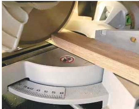
3a Using a mitre saw set at 90° to cut the 75 individual lengths of 2x1 in timber
