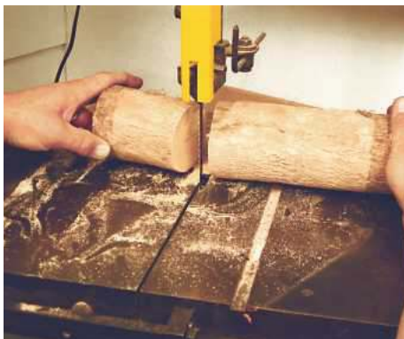
1 Select a clean piece of boxwood and cut a piece for the nutcracker's body
