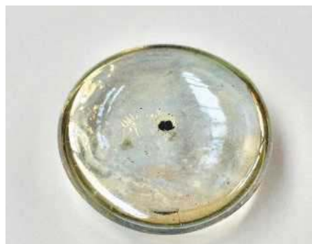
8 Glass half bead bearing with 'V' hole drilled
