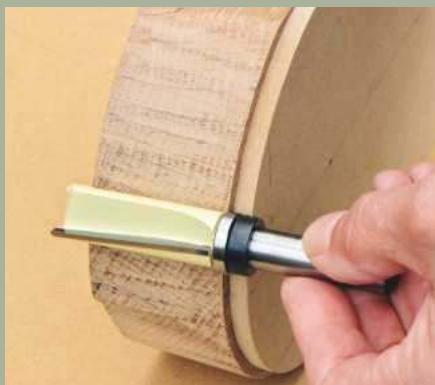
This project calls for a flush-trim bit with top roller bearing
