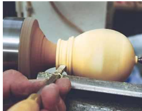
8 Raise the toolrest slightly and use a 6mm scraper to turn the concave
