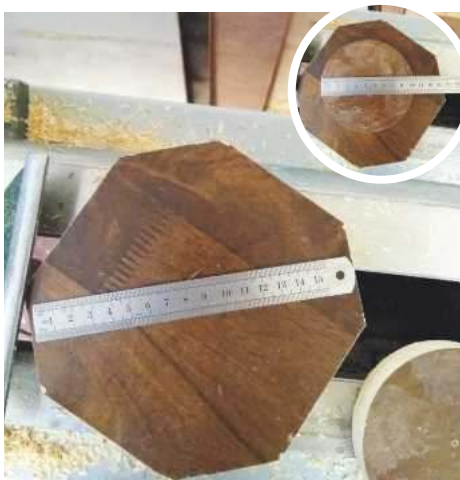
1 The turning started with a base and platter. The base requires a blank approximately 110mm across and the platter needs to be a little more than 150mm
