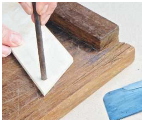
17 Hour marker dots on the dial are made from 6mm walnut dowelling; drill a 6.5mm hole to check the dowel fits snugly
