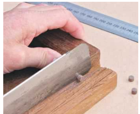
18 Saw dots to length (about 6mm is adequate) with a fine-tooth saw; sand the ends lightly to remove any whiskers
