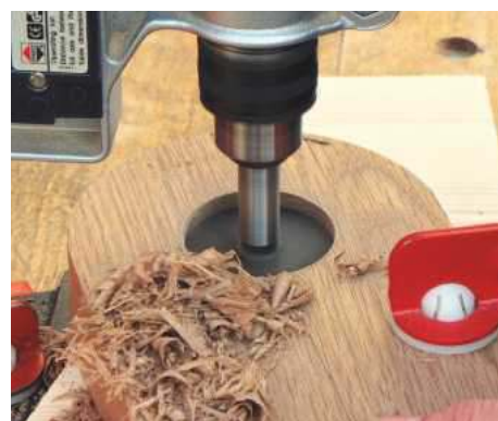
9 Mark the centre of the clock movement, then bore all the way through the blank with a large-diameter (54mm) Forstner bit
