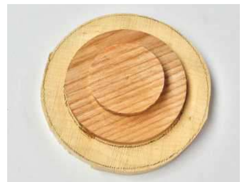
9 Maple blank for the turntable base attached to a chuck interface using hot-melt glue
