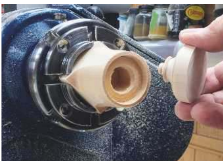
16 Reverse mounting the hub in a jam chuck
