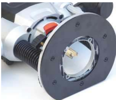
The substantial cast alloy base is D-shaped, so you can run its flat edge against a guide fence for arguably more consistent cutting
