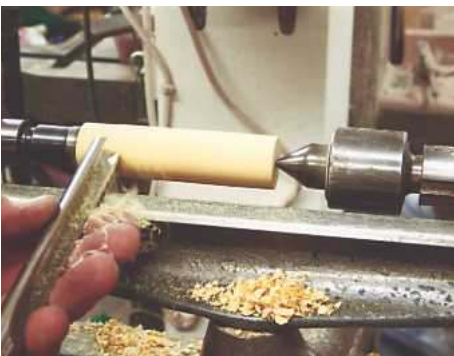
10 Picking up the thread: turn the boxwood to 1in and no larger!
