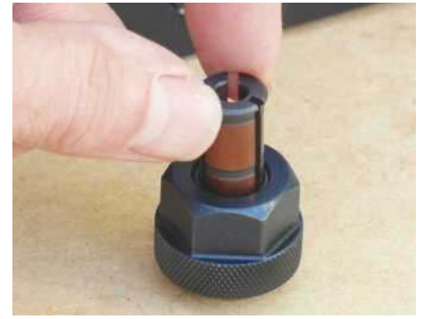
The 1/4in sleeve is simply inserted into the larger one, with a flange at the end to prevent it dropping down too far
