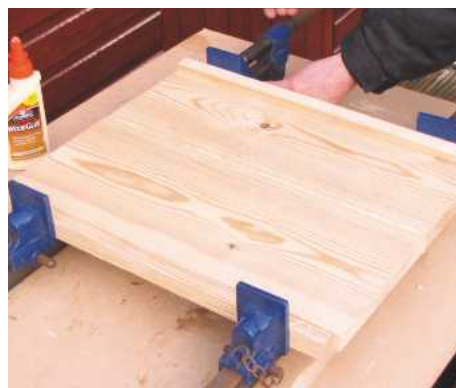
1 You'll need to glue boards together to get sufficient height for the box. Check edges are straight first
