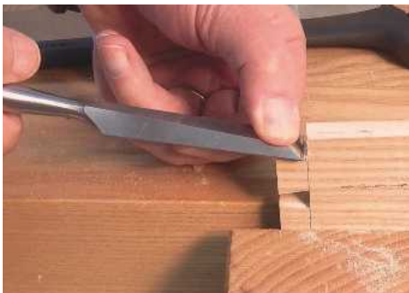
25 Remove any tiny step in the corner with a sharp chisel – note the pressure holding the back flat on the cheek of the tail
