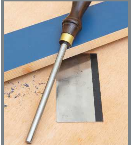
It isn't just straight lines: shaped and gooseneck scraper cards can be used on all manner of profiles
