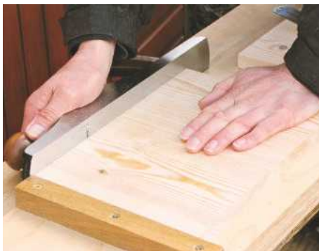
4 Trim sawn ends with a plane to get them dead square. A shooting board is handy for this task
