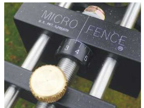
The rotary depth collar is laser-etched with very clear graduations, enabling you to tweak a setting easily
