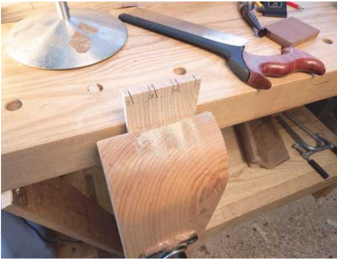
16 Repeat this until all the tail cheeks are cut down to the shoulder line
