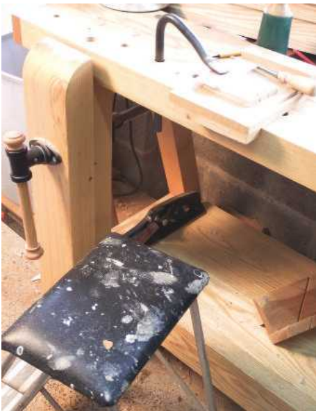
18 With a stool in position and the workpiece clamped down, I'm ready to chisel out the sockets
