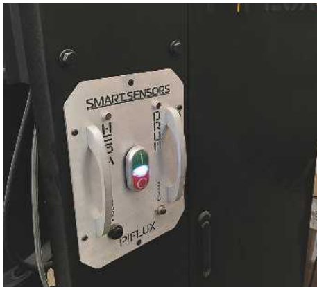
The control panel with ‘Smart Sensors’ – ‘Bag Full’ and ‘Filter Clean’ LEDs
