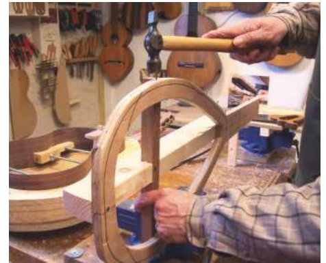
37 Nails act as anchor points for the elastic bands
