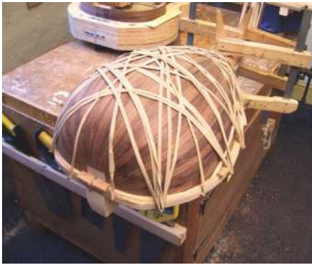
41 Long bands hold the bowl down onto the soundboard
