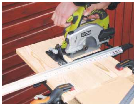
3 Cross-cut panels as required, running the saw against an edge guide or batten for accuracy
