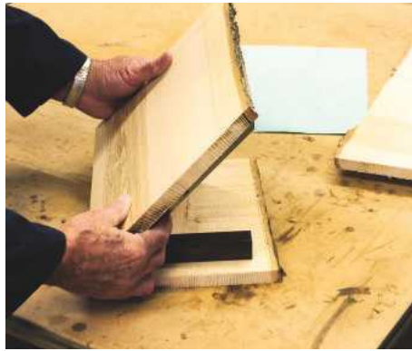
3 An adjustable sliding bevel helps set the angle of the slope
