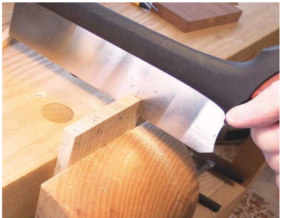
15 Then track down the line to the shoulder
