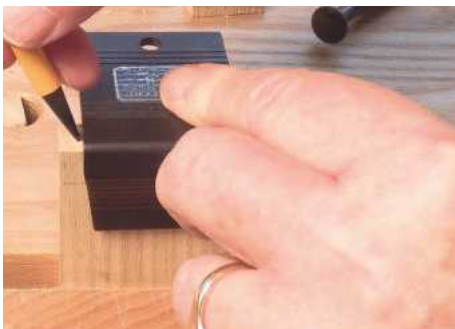
10 ... and slide the template up until it touches it
