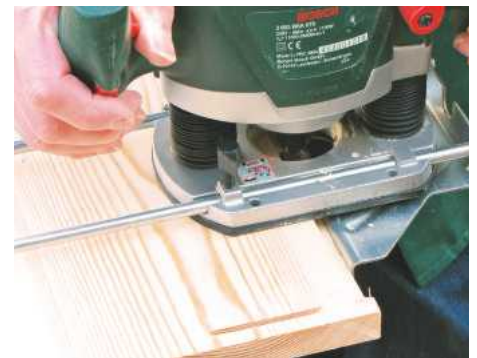
6 Rout a rebate along the inside edges of front, back and sides for the base. Use an offcut to check depth
