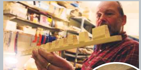
Tim prefers to use a composite of wood for the bridge, while other makers have used one solid block
