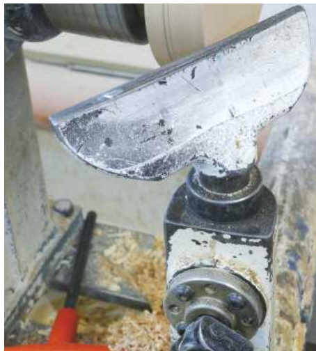
14 Another useful thing you can add to your lathe is a moveable collar on the stem of the toolrest. As I have to move the toolrest through 90° when turning the base, it will stay at the same height as I move it, thus saving time
