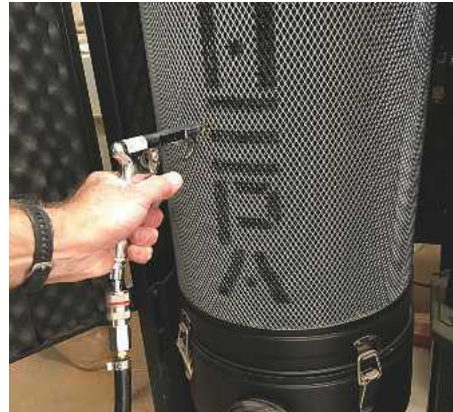
Filter cleaning is easy and dust-free with an air-line and a length of hose
