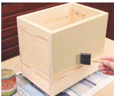
17 Fill any defects and sand the box. Finish with paint or varnish, using oil on the inside surfaces
