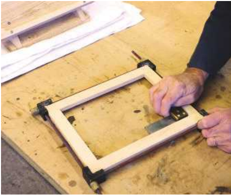
8 The retaining frame is checked for square
