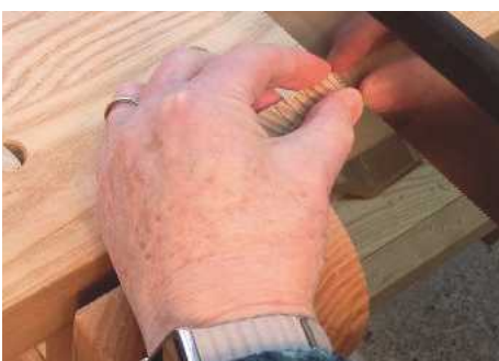
14 I use a 'pinch' grip to control the saw as I start the cut, with the saw flat on the timber – it's easy to check and tweak the alignment
