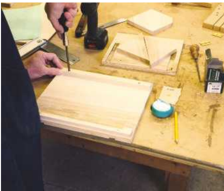
5 A recessed strip at the bottom stops the iPad moving too far left and right and another finishes it off at the top
