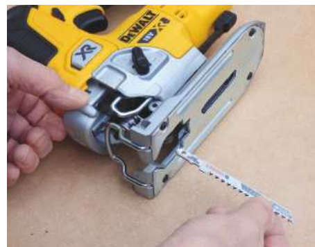
To change the blade, you open out the hinged, spring-loaded alloy lever at the front of the tool to insert or release it from the mechanism
