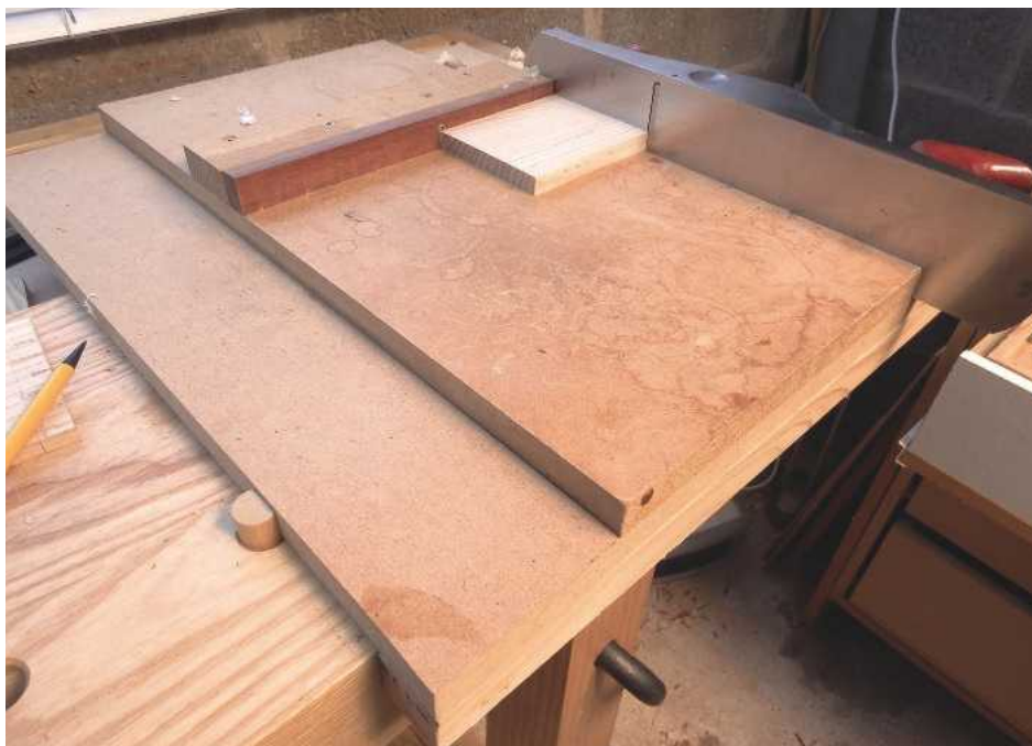
1 Begin by squaring up the ends – a task made light and easy by this simple shooting board
