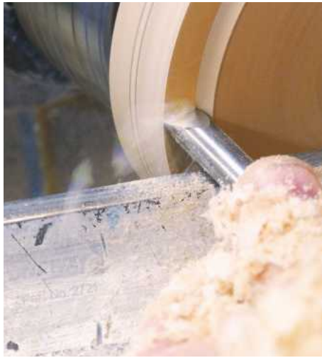
11 Shaping is best done with the tools you feel most comfortable with. The 10mm round skew chisel is perfect for taking a full width cut down to the fillet on the edge of the base
