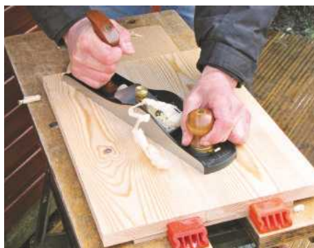
2 Once the glue has cured, remove any dried beads and true up the surface with a bench plane
