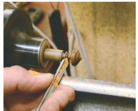
6 Use the parting tool and a detail gouge to turn the finial. Keep the detail crisp
