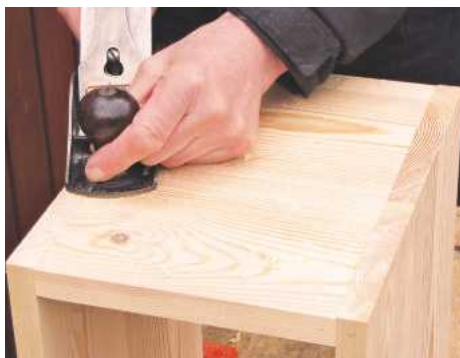
8 Cramp the box to the bench top and trim slightly proud end-grain flush with a finely-set plane
