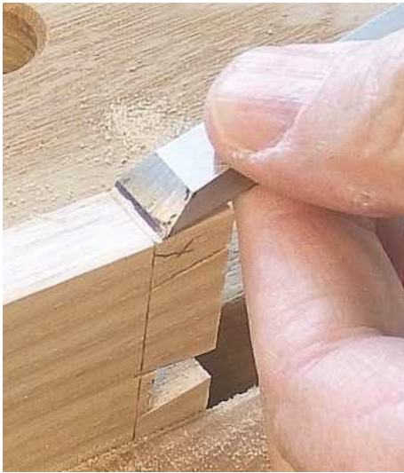
22 Position a chisel about 2mm on the waste side of the shoulder line and gently but firmly push towards it
