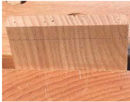
8 When you're happy with it, step across again, stabbing in at each point, then repeat the other way. That's three nicely-spaced tails pinpointed
