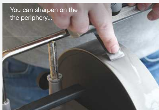
Gouge sharpening with the SVD-186 Gouge Jig.
