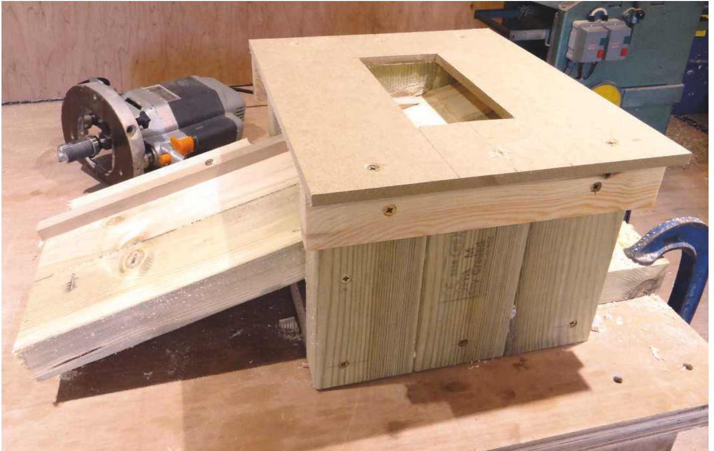
9 Here's one I made earlier: a jig for routing a slant. I adjusted the angle of the ramp and the cuts were made in a matter of minutes
