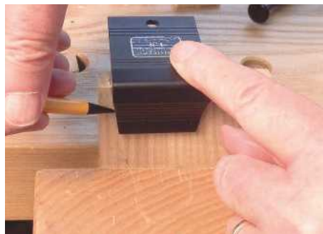
11 This dovetail 'saddle' marker lets me mark the end and face in one operation, reducing the risk of error
