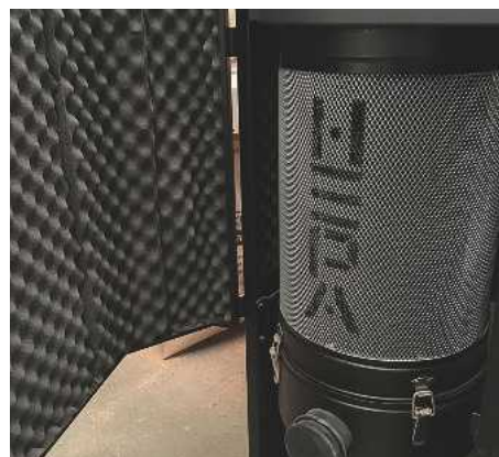
The HEPA filter takes care of dust down to 1 micron and the acoustic lining keeps everything remarkably quiet
