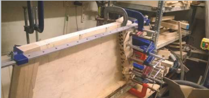
Drilling holes into the dulcimer destined for the Bolshoi Ballet, to make it lighter
