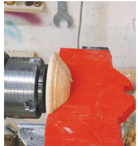
15 Both bases have to be the same so I used a plastic gauge, which was originally for marking out shapes of tiles to check both ogee shapes on the top
