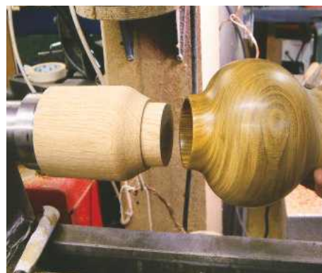
1 To turn the bottom, put the container onto a jam chuck. Support it with the tailstock
