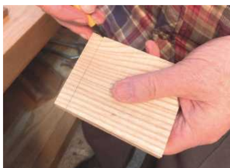
4 Running a pencil along the line makes it more visible and aids accuracy
