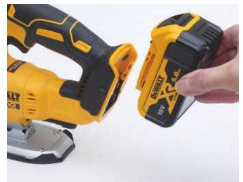
Like most cordless saws, the battery slots on to the back of the tool
