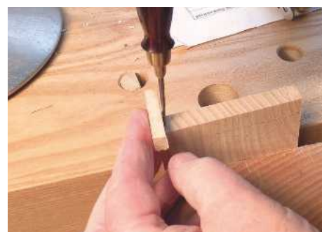
5 Using an awl – or one leg of the dividers – set the half-pin marks about 5 or 6mm from each edge – a scrap of wood makes a handy gauge
