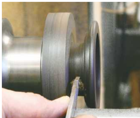
5 Turn the top of the lid and part it off with a fine parting tool
