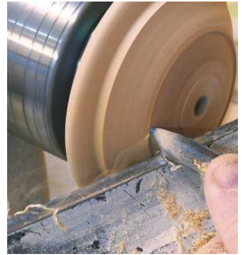
12 The rest of the shaping, including the bead on the edge and the ogee design, is completed using a short bevel signature gouge. Wherever possible, cut with the grain, so that the bevel of the tool is in contact with the surface
