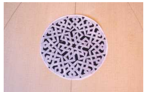
32 A photocopied rosette pattern glued into place
