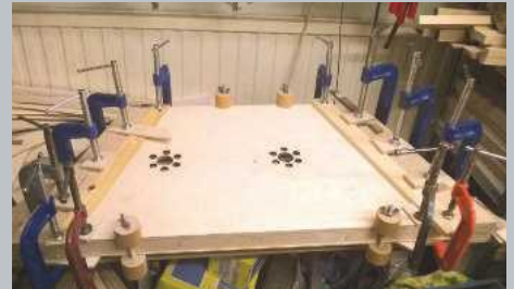
An even spread of pressure is maintained with lots of clamps
