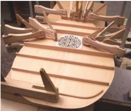
35 The soundboard bracing pattern
