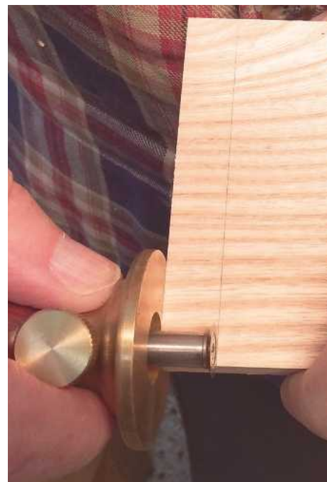
2 Use the cutting gauge to slice a nice, fine shoulder line around the ends of the timber
