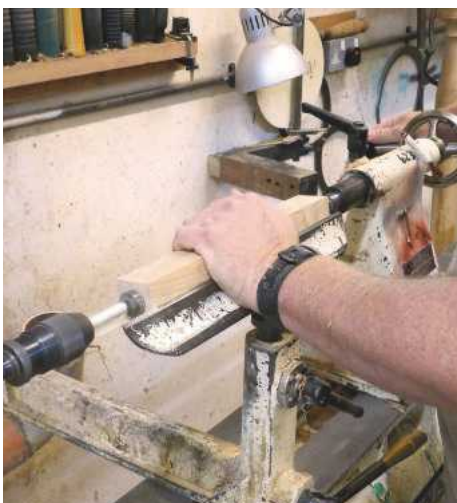
16 It's easier to drill the hole for the candle cup first. I have a drill in the headstock and a drive centre in the tailstock. Hold the square wood against the toolrest and advance the wood by turning the hand-wheel
