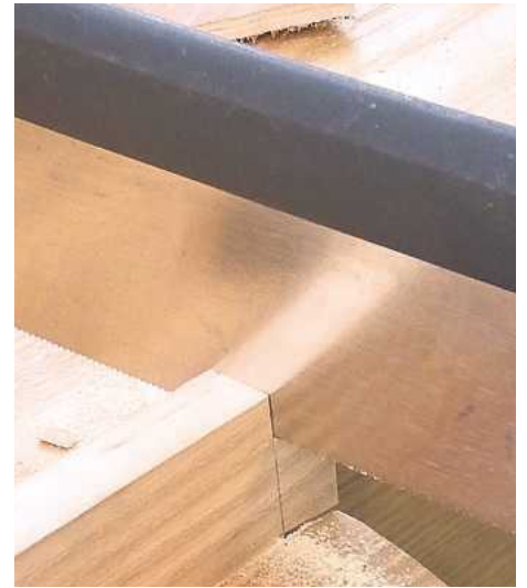
24 Rest the saw against the shoulder, line it up vertically and cut down to the tail, stopping carefully on the edge of the tail
