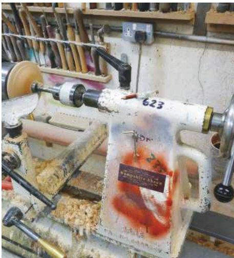
13 I've got a new addition to my big Oneway lathe – a speed handle for the tailstock, which will make drilling much easier. I used a 30mm sawtooth machine bit to drill a hole around 20mm deep
