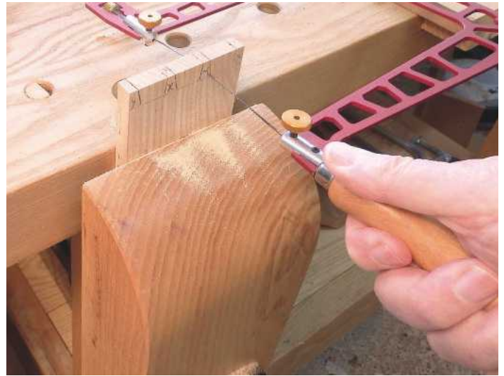
17 Remove the bulk of the waste between the tails with a fret saw a few millimetres above the shoulder line
