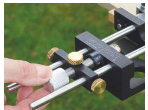
A full rotation equals 1mm of travel, with increments of \frac{1}{20} th of a millimetre
