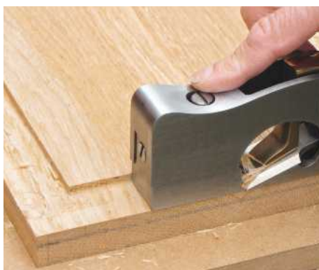
15 Rout a rebate all around the lid to a depth of about 5mm. Clean up with a shoulder plane or abrasives
