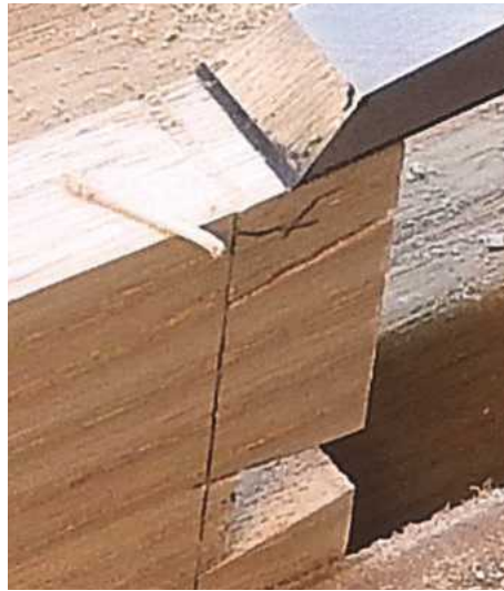
23 This will turn the line into a trough with one vertical side to position the saw perfectly for the shoulder cut
