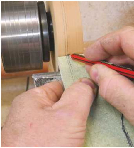
10 Here I've drawn out the base onto the end of my rod; this means I can transfer the positions of the shapes easily onto the spinning blank. This keeps the base and stem designs together
