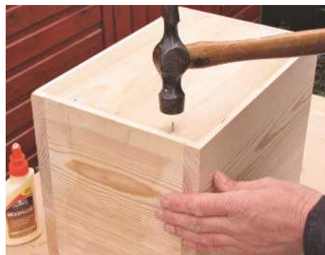
10 Apply glue and pin the base to the box. Pre-drill holes at the ends to prevent the timber from splitting
