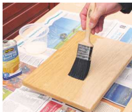
16 Round the edges of the lid and sand with fine abrasive paper. Brush on three coats of food-safe oil finish
