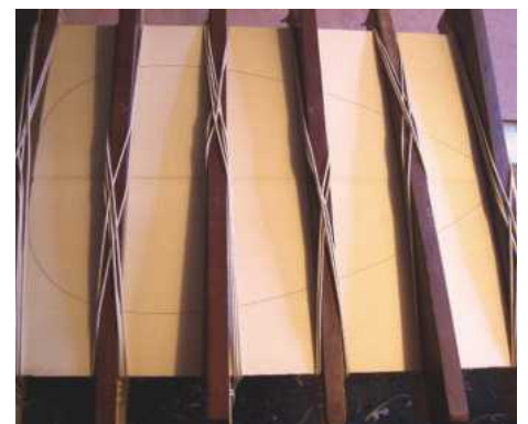
30 The soundboard in the wedge and lace jig
