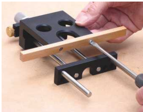
Two pre-drilled, 177mm cherry facings are included, which are screwed to the edge of the guide for straight routing
