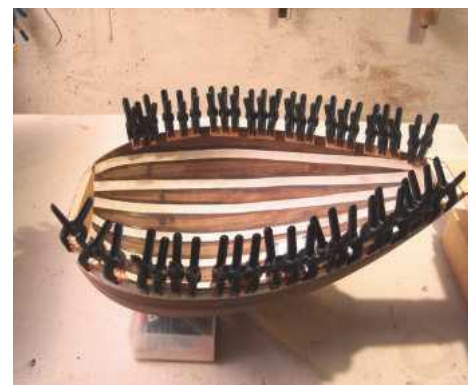
40 Small spring clips hold the linings in place as the glue cures
