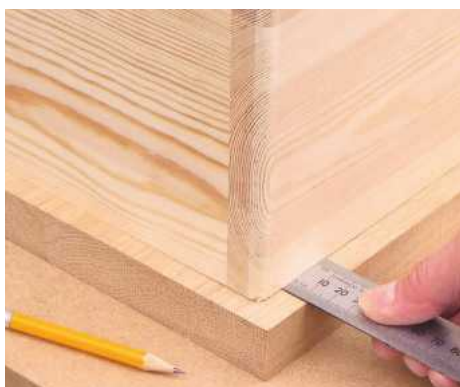
14 True up the top and bottom and cut the lid to size. With box above, mark the positions of rebates
