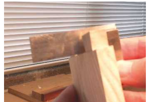
27 Check the internal shoulders with a square
