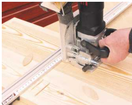
5 Mark out positions for No.20 biscuits in the panels and cut matching slots with your biscuit jointer
