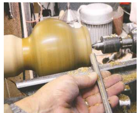
2 Use the gouge to turn the bottom flat and to round over the base
