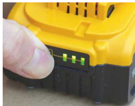
Charge time is about 70 minutes, with status LEDs indicating remaining juice via a small button
