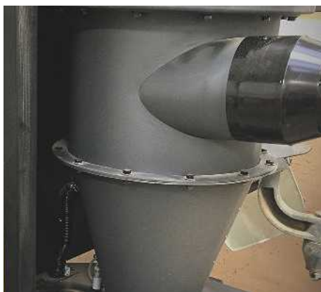
The big difference is the cyclone, which helps to keep the filter clean and maintains airflow
