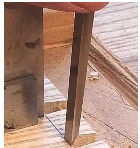
21 For the final cut, position a square behind the chisel and feel the chisel into the gauge line. You might like to tilt the handle a shade forward to undercut slightly, ensuring that the shoulders will seat down nicely
