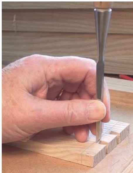
19 Position the chisel to take fine slices, working back towards the line
