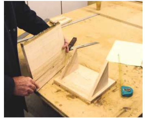
4 The two angled pieces are cut and tested
