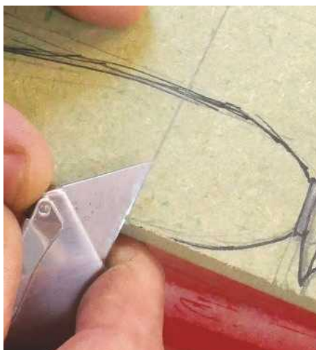
17 Bring all the positions of the details to the edge of the rod, then use a knife to notch out a small 'V'; this will help to keep the correct position of the pencil when it comes to marking out
