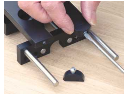
A pair of half-round Delrin spacers enable it to be used against curved edges, creating two points of contact as you move the router...
