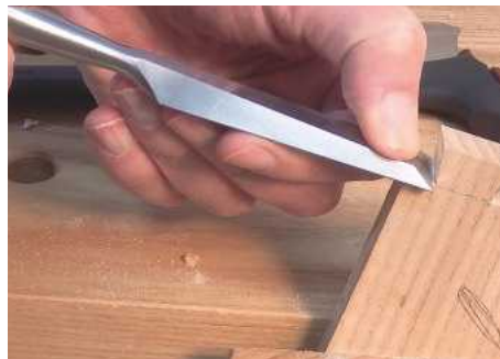
26 Then repeat if necessary with the chisel against the shoulder
