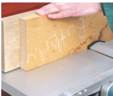
12 Plane up suitable hardwood for the breadboard lid. Ideally this should be at least 25mm-thick
