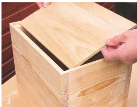
9 Mark out and saw the base slightly oversize. Plane edges until this is a snug fit in the rebates
