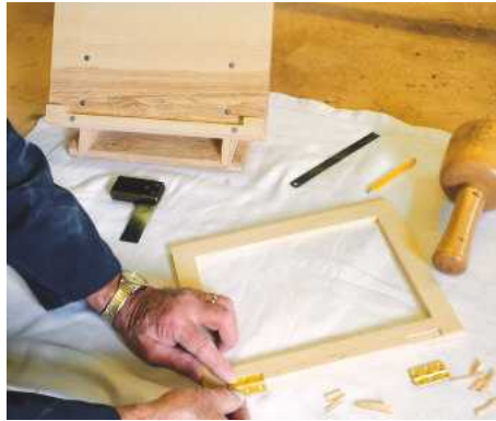
9 Hinges onto the frame first, then...
