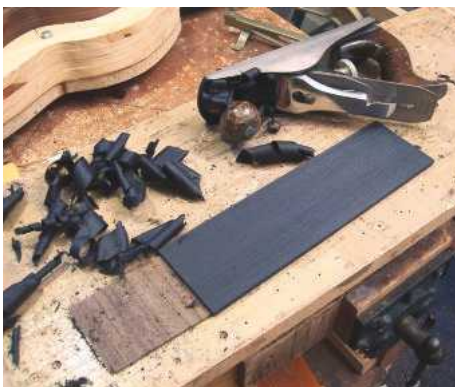
44 The fingerboard under preparation
