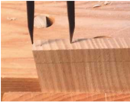
7 Lightly step them across and adjust by trial and error until the point lands a few millimetres past the other half-pin mark. The gap indicates the width your pins will be
