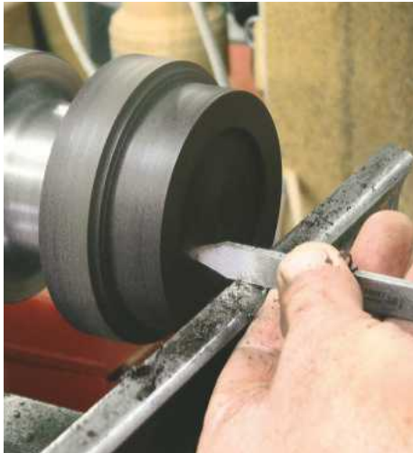
3 Cut the recess in the lid with a parting tool. Make it a loose fit
