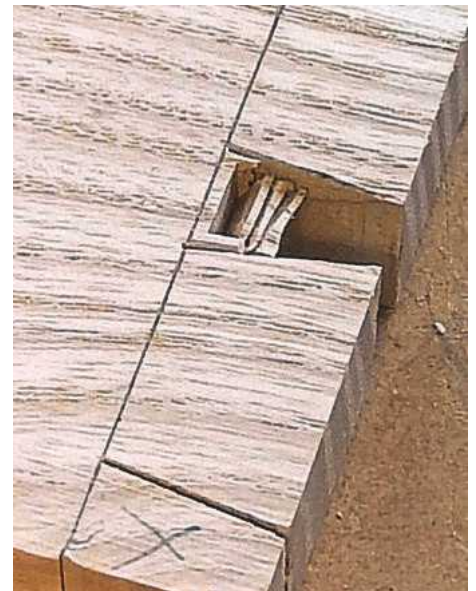
20 Use a mallet to tap gently through to about the mid-way point, then move the chisel back and repeat to take fine slices
