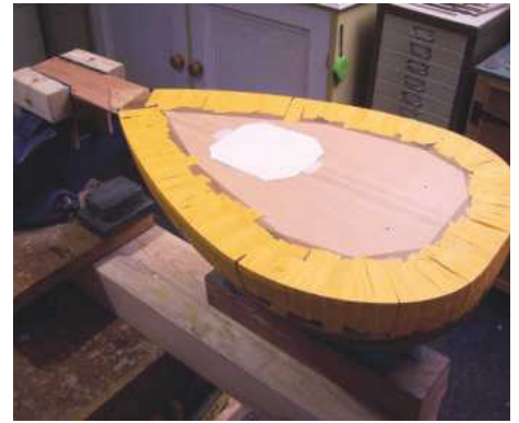
43 Masking tape holds the bindings in place
