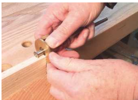
3 Cutting the edge shoulder line deeply into the tail piece will help later on
