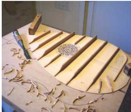
36 The brace ends are scalloped
