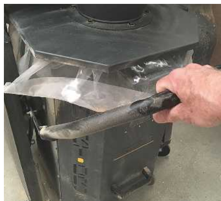
After ‘docking’, just push down the big lever and you’re done
